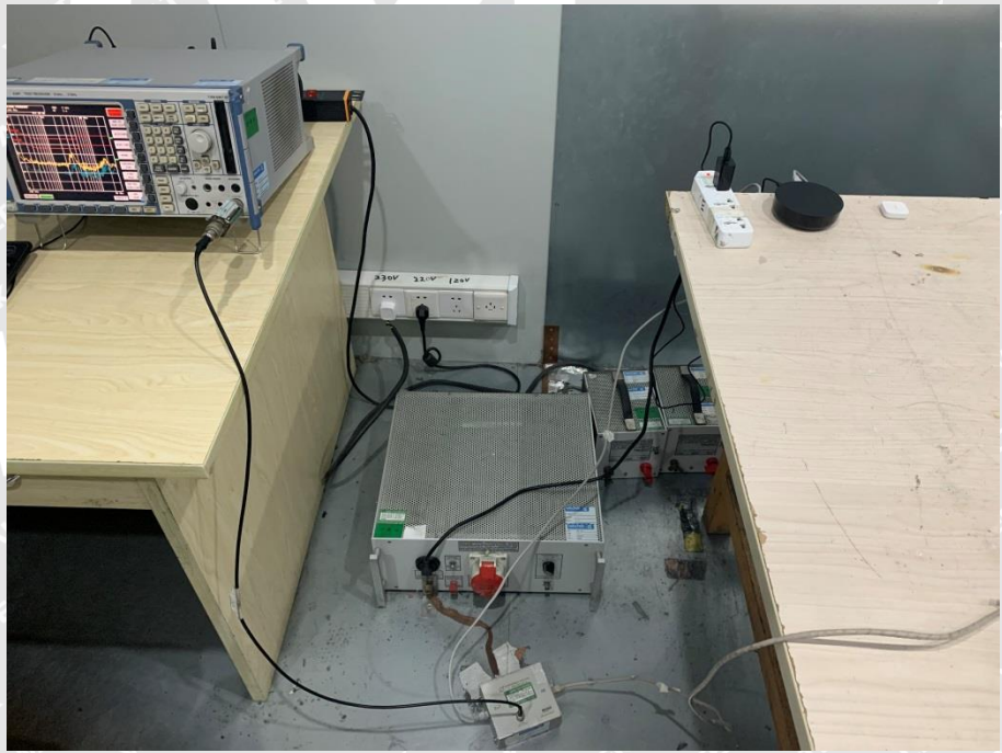
Conducted Emission Test Setup(RJ45 Port)
