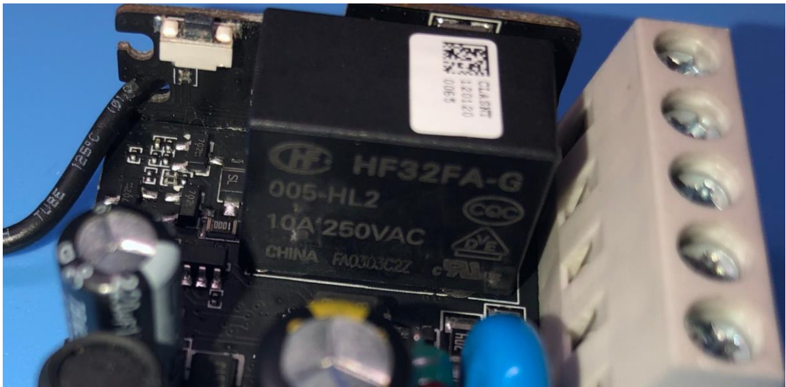
Close-up view of relay
