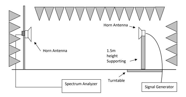
Note: for frequency lower than the 1GHz, the horn antennas among the two block diagrams above should be replaced with dipole antennas (or other antennas provided they can be referenced to a dipole).
