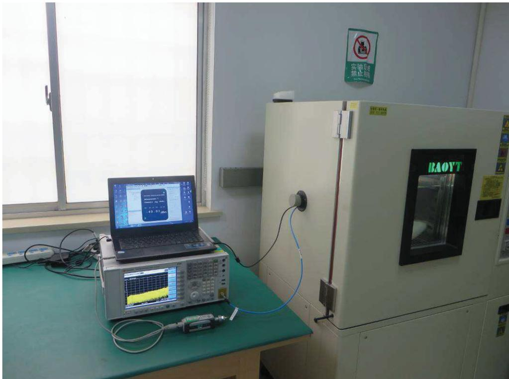
**Photograph 3: Set-up for Receiver Blocking tests**
