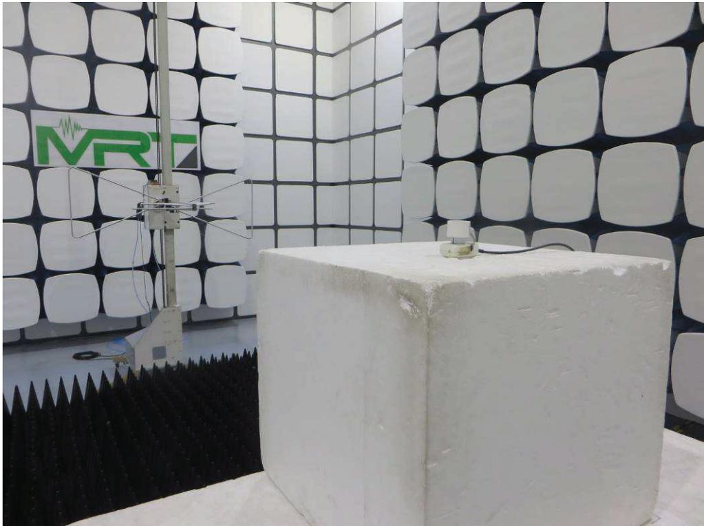
**Photograph 5: Set-up for radiated spurious emission, 1GHz – 18GHz**
