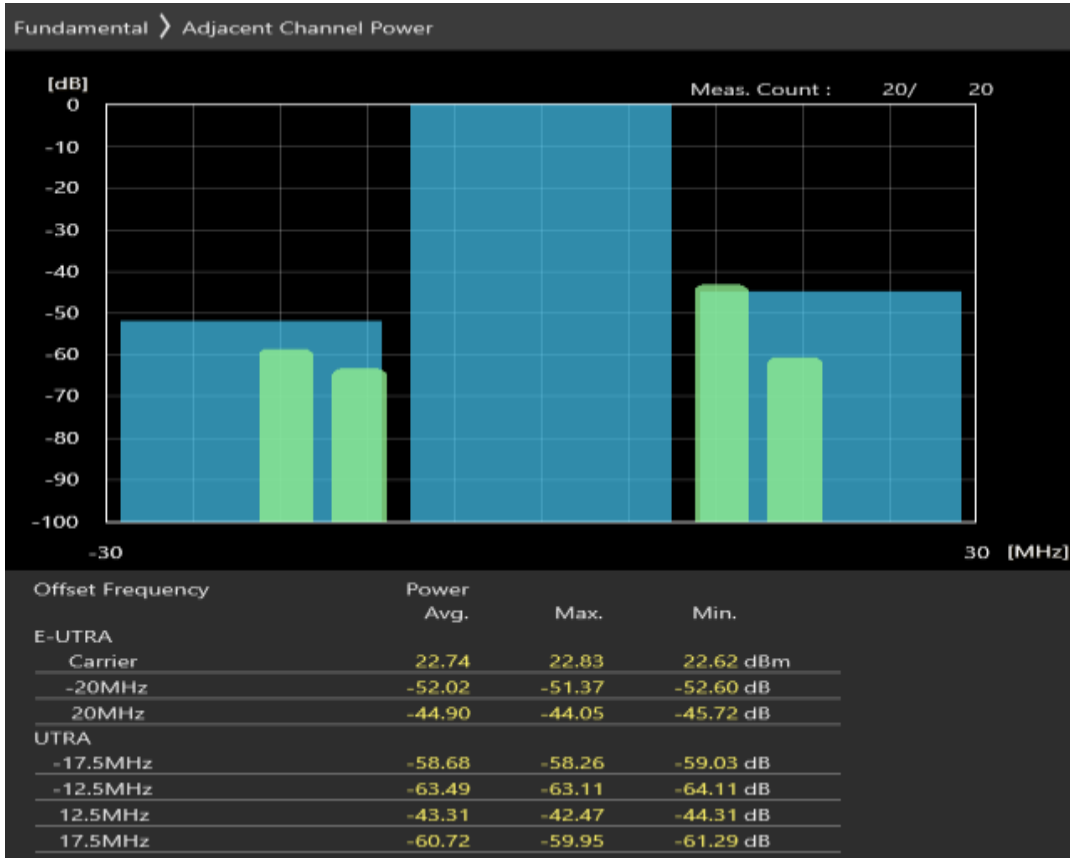
Band7 QAM16 BW=20MHz Channel=21100 RB Size=100 Position=#0
