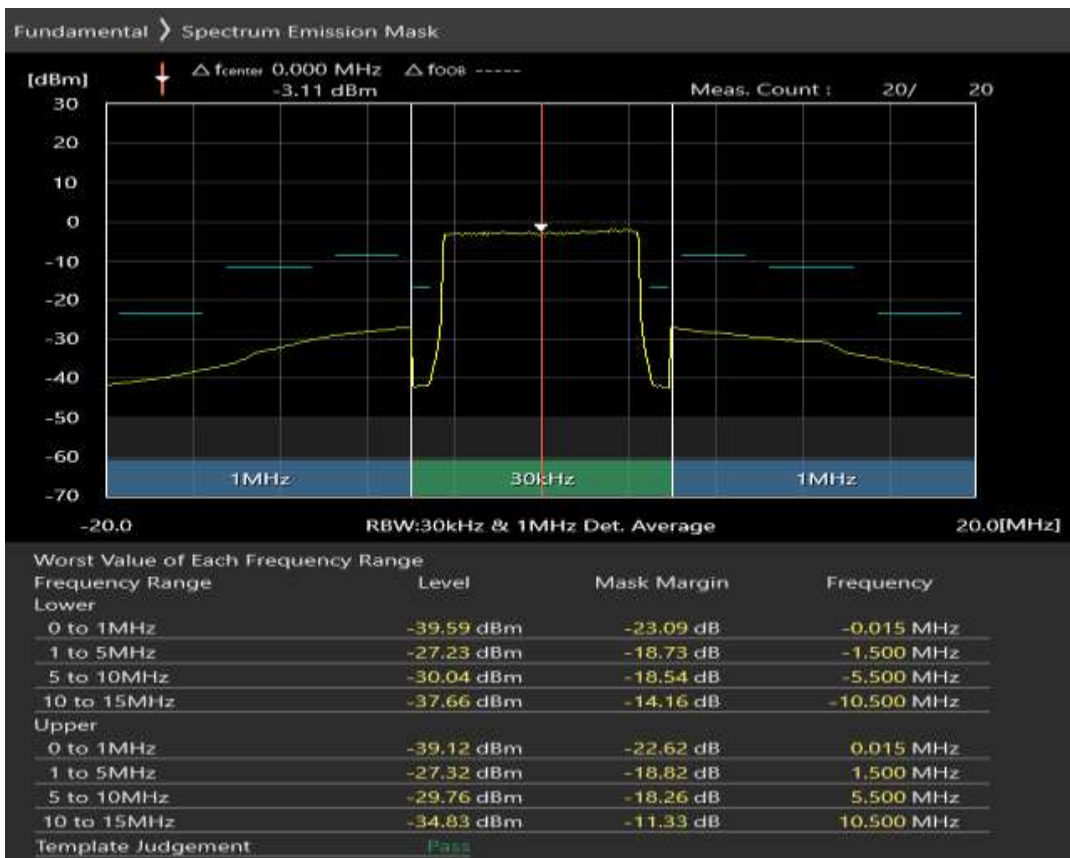
Band7 QPSK BW=10MHz Channel=21100 RB Size=12 Position=#0
