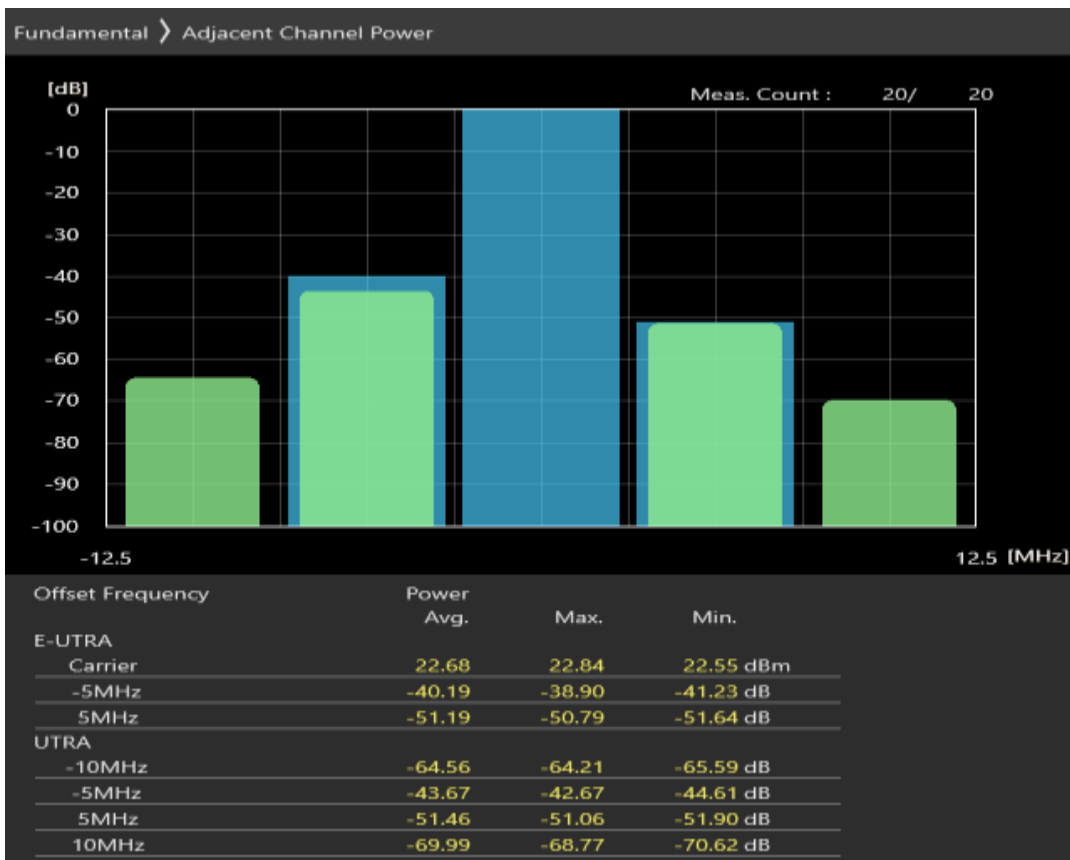
Band1 QAM16 BW=5MHz Channel=18025 RB Size=8 Position=#Max
