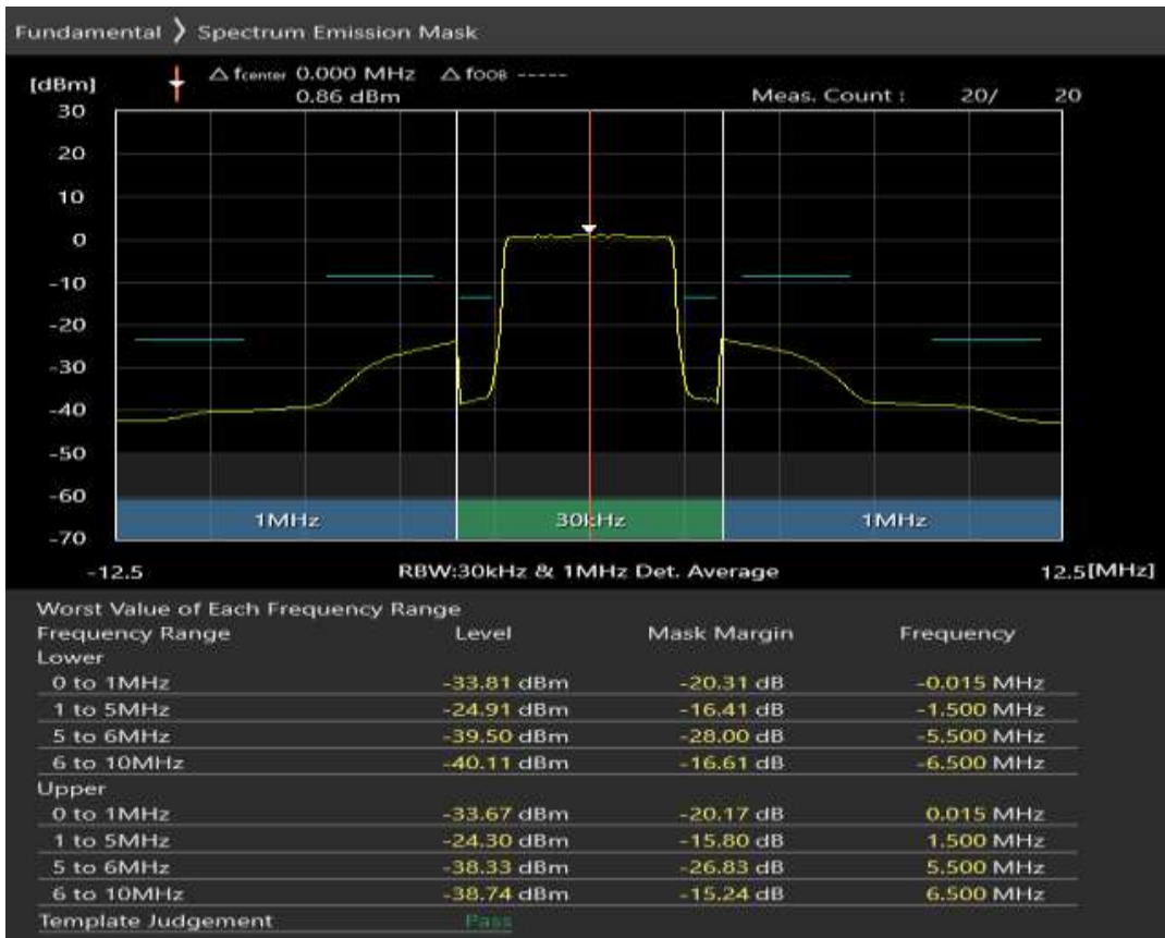
Band1 QAM16 BW=5MHz Channel=18575 RB Size=8 Position=#0
