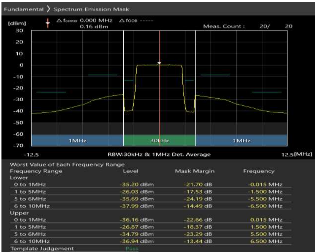
Band7 QPSK BW=5MHz Channel=21100 RB Size=8 Position=#0
