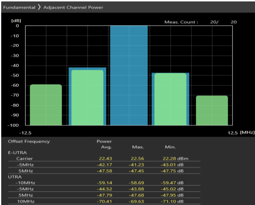
Band3 QAM16 BW=5MHz Channel=19925 RB Size=8 Position=#Max
