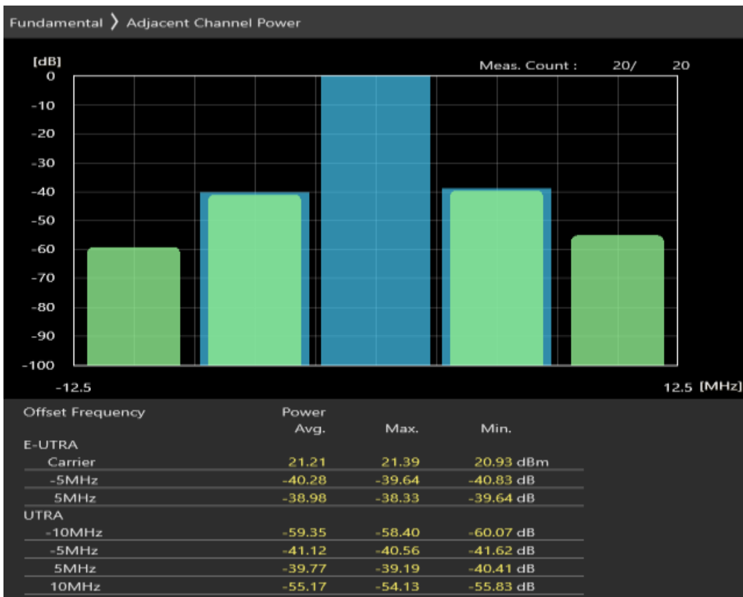
Band3 QPSK BW=5MHz Channel=19575 RB Size=8 Position=#0
