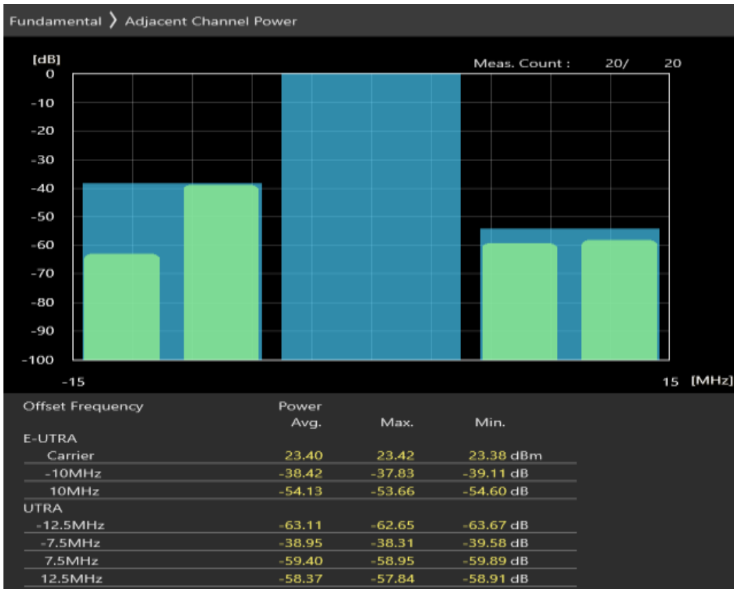
Band8 QPSK BW=10MHz Channel=21625 RB Size=12 Position=#Max
