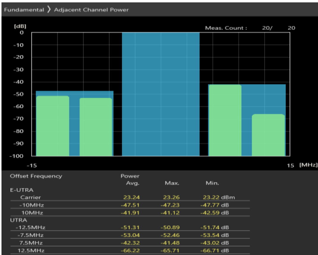
Band3 QPSK BW=10MHz Channel=1990 RB Size=50 Position=#0
