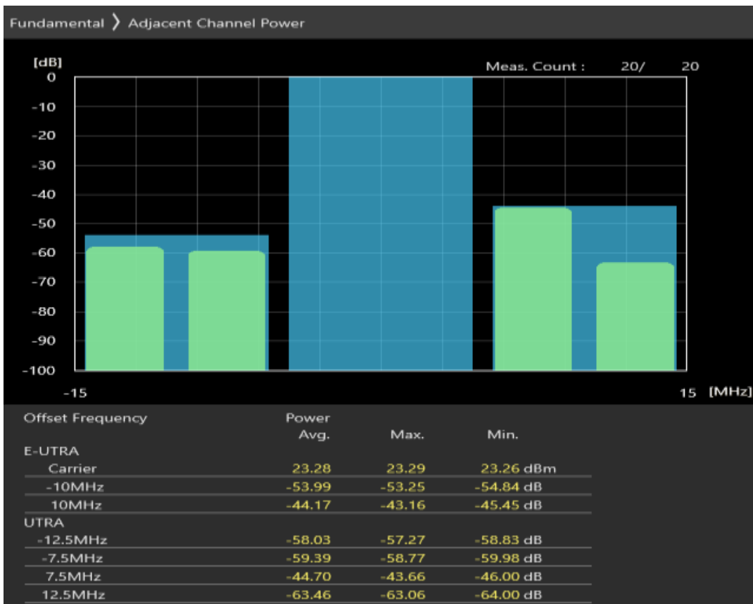
Band8 QPSK BW=10MHz Channel=21625 RB Size=50 Position=#0
