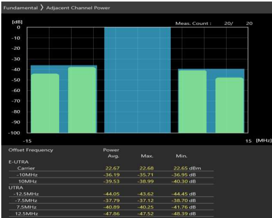
Band7 QAM16 BW=10MHz Channel=21400 RB Size=12 Position=#0
