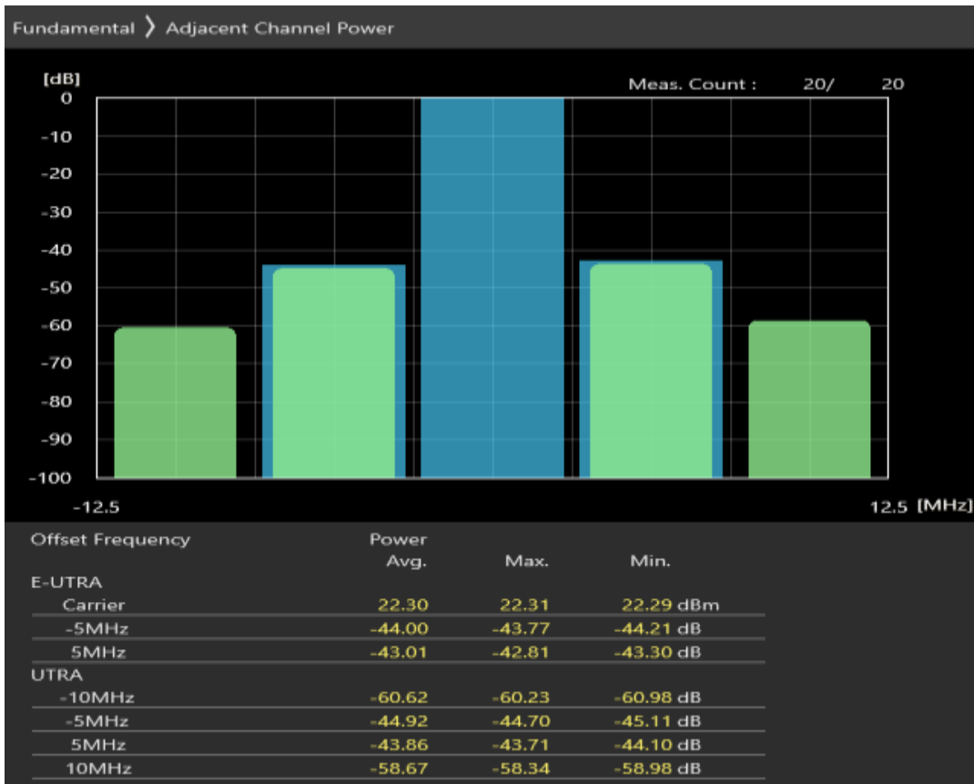
Band1 QAM16 BW=5MHz Channel=18300 RB Size=8 Position=#0
