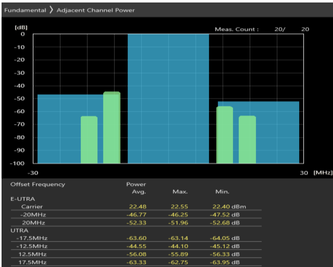
Band1 QAM16 BW=20MHz Channel=18500 RB Size=18 Position=#Max
