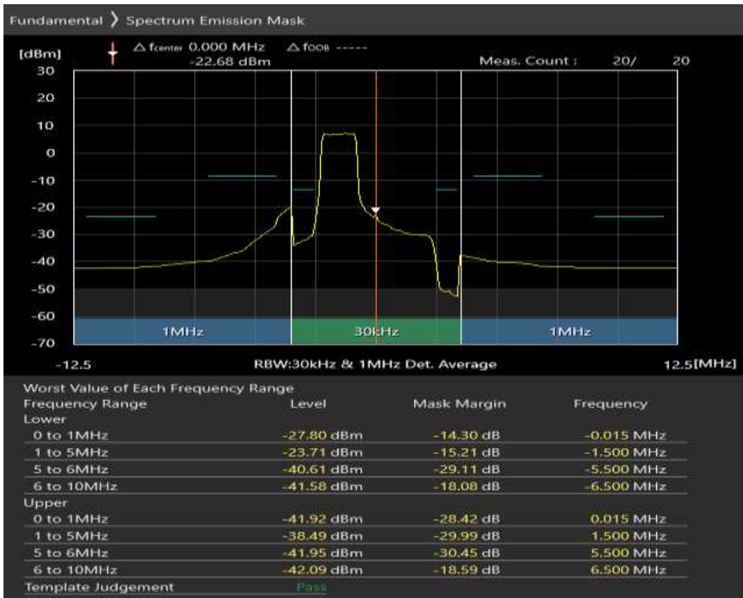
Band7 QPSK BW=5MHz Channel=20775 RB Size=8 Position=#Max
