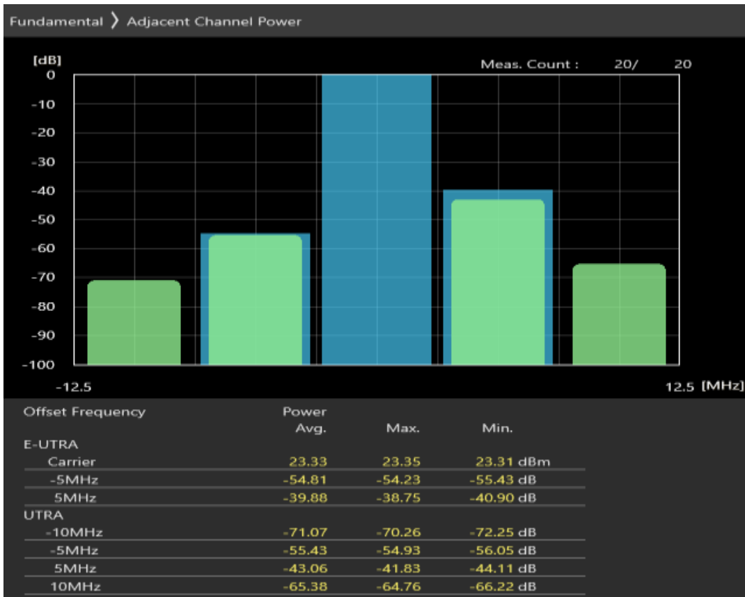
Band8 QPSK BW=5MHz Channel=21625 RB Size=25 Position=#0
