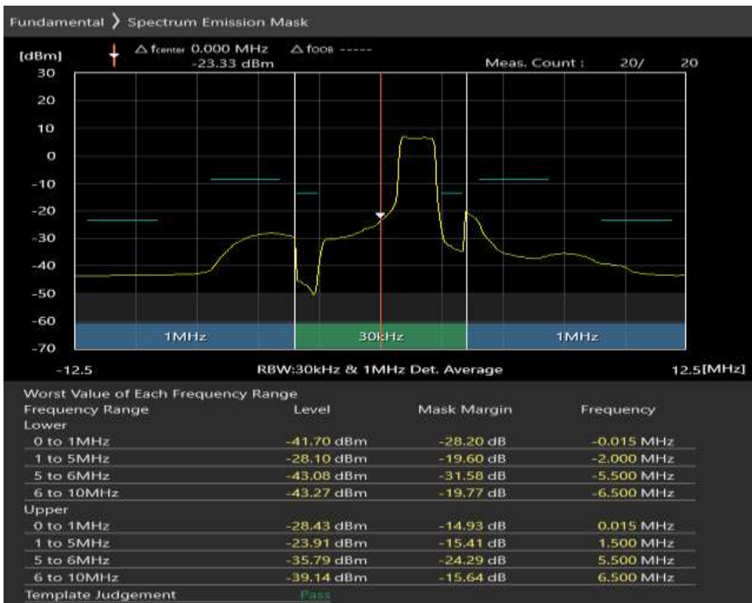
Band3 QPSK BW=5MHz Channel=19575 RB Size=25 Position=#0
