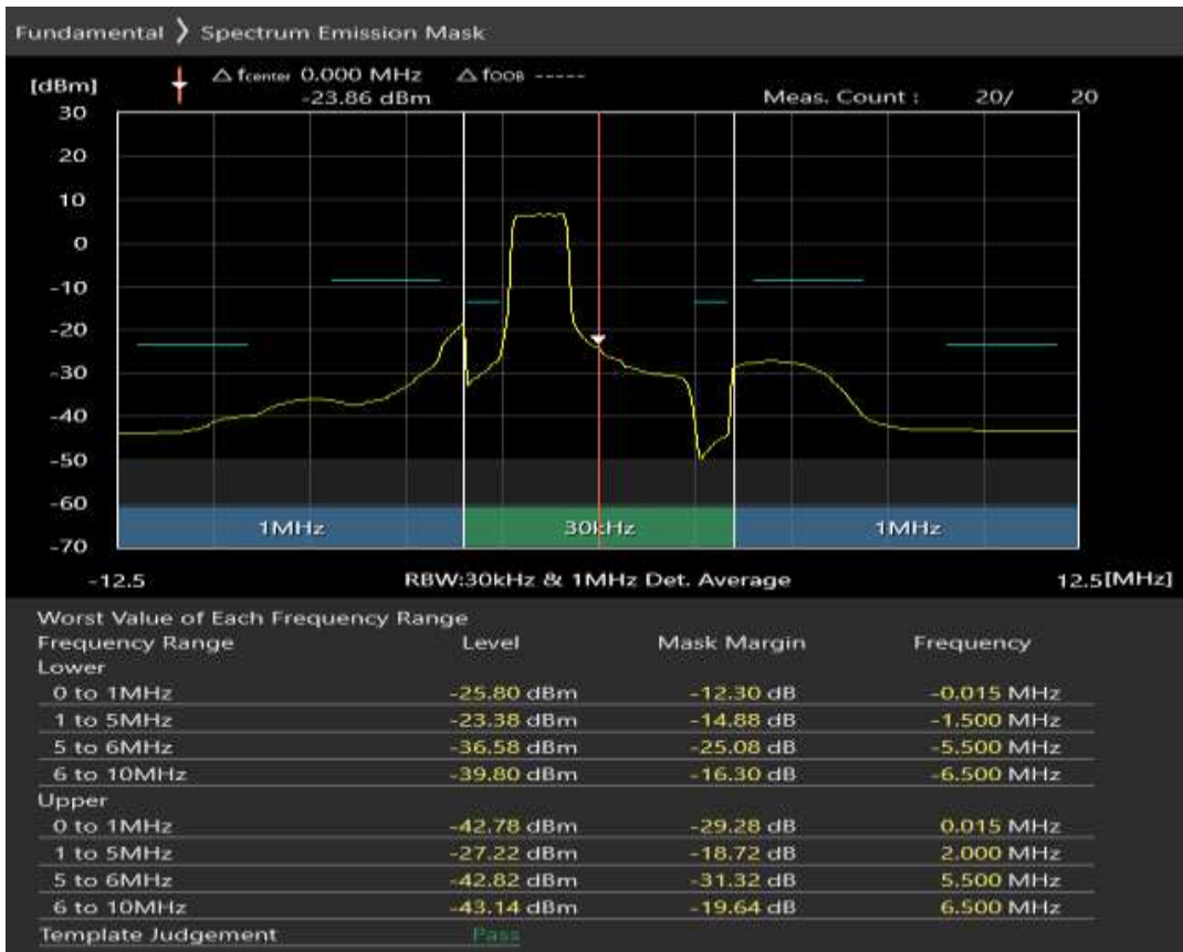
Band3 QPSK BW=5MHz Channel=19225 RB Size=8 Position=#Max
