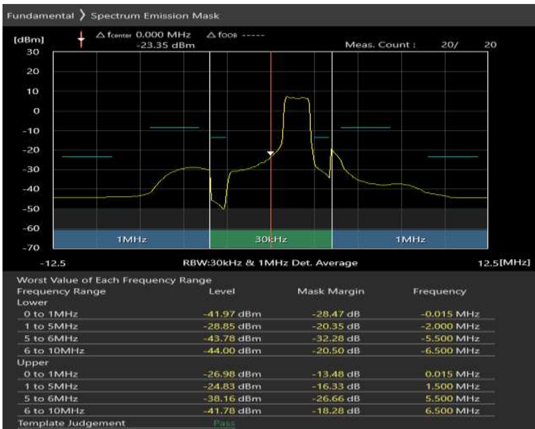
Band3 QPSK BW=5MHz Channel=19925 RB Size=25 Position=#0
