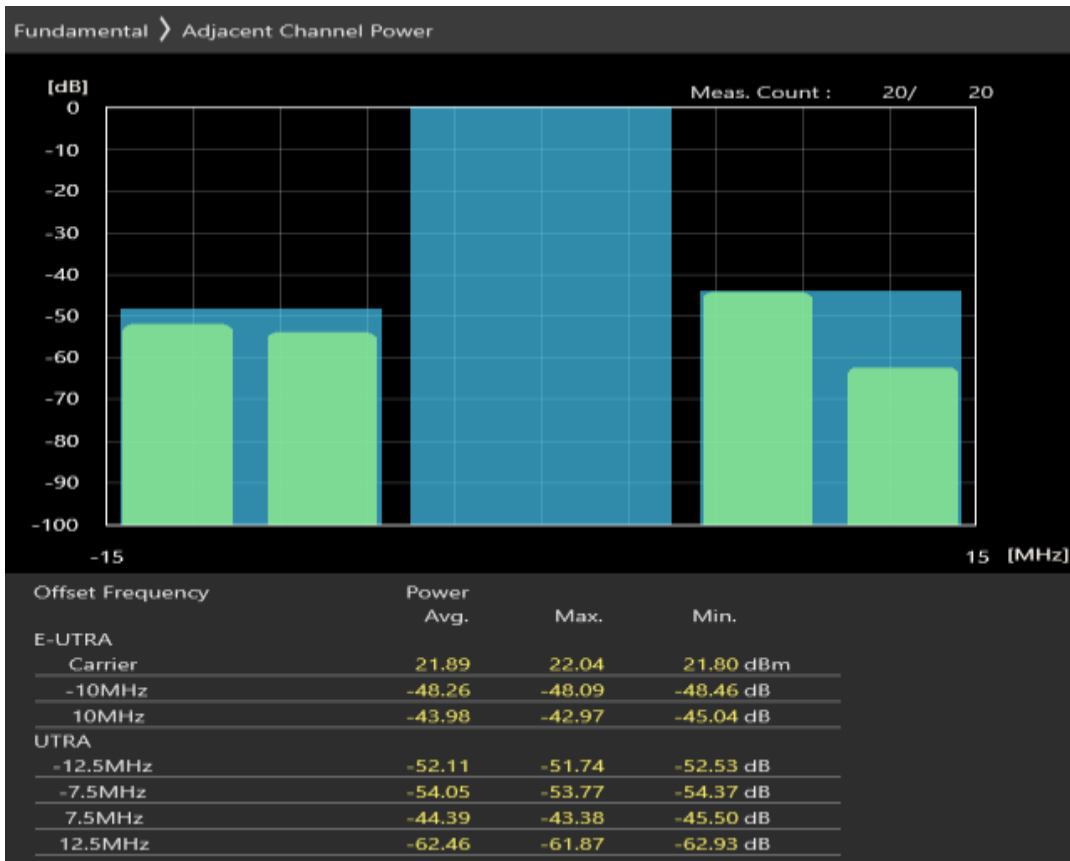
Band3 QAM16 BW=10MHz Channel=19575 RB Size=50 Position=#0
