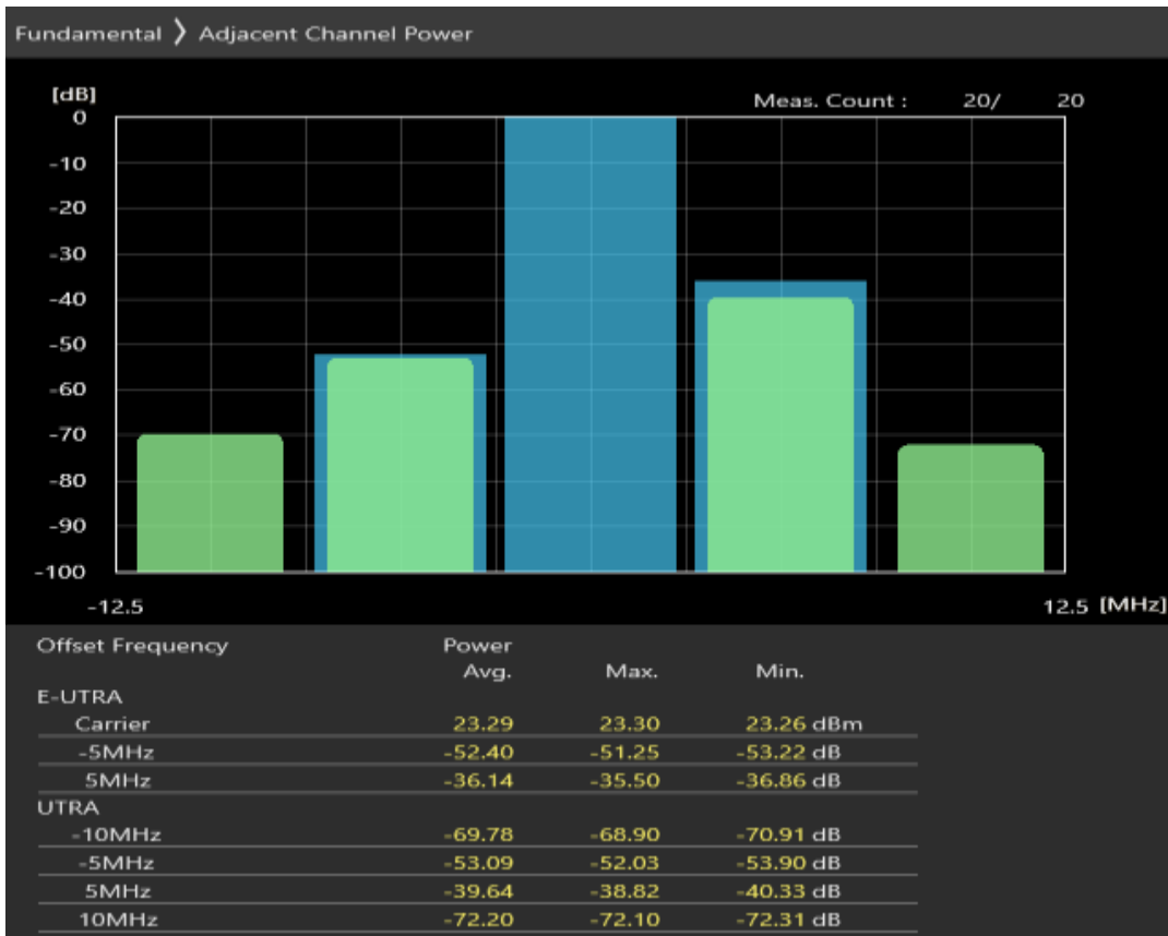
Band8 QPSK BW=5MHz Channel=21775 RB Size=25 Position=#0
