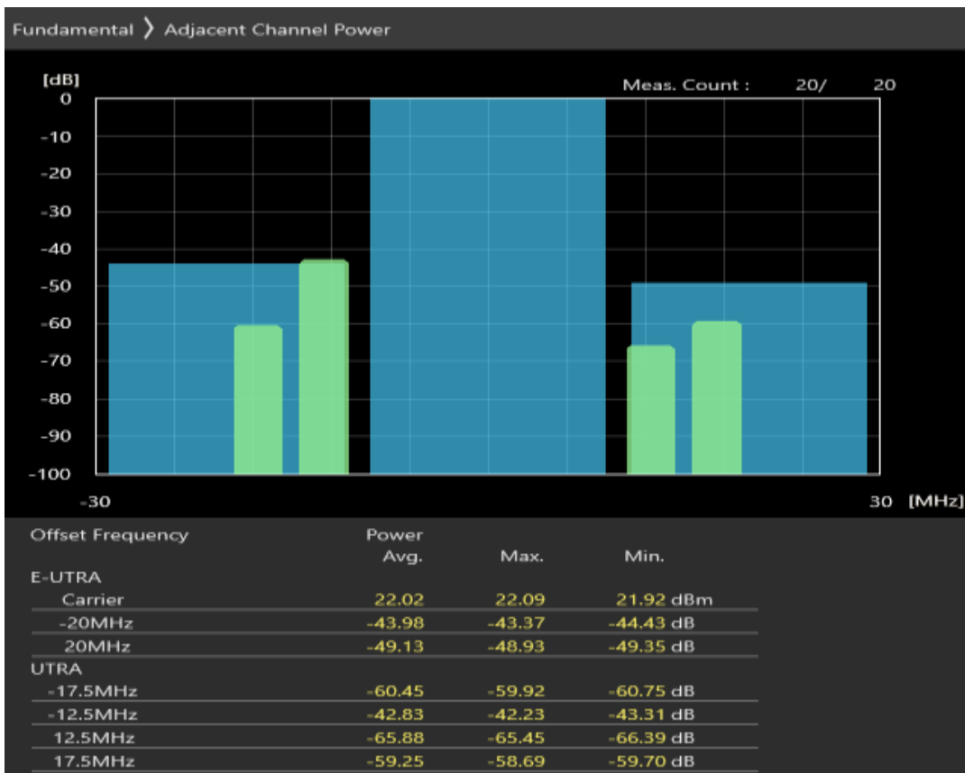
Band3 QAM16 BW=20MHz Channel=19575 RB Size=18 Position=#Max
