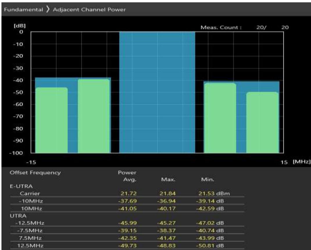
Band7 QPSK BW=20MHz Channel=20850 RB Size=18 Position=#0
