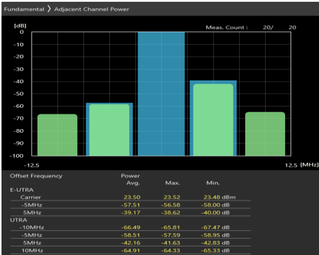
Band7 QPSK BW=5MHz Channel=21100 RB Size=25 Position=#0
