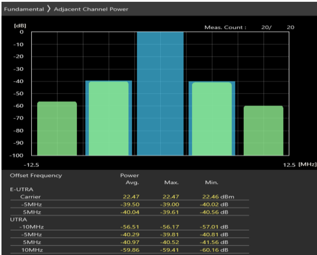
Band8 QAM16 BW=5MHz Channel=21625 RB Size=8 Position=#0
