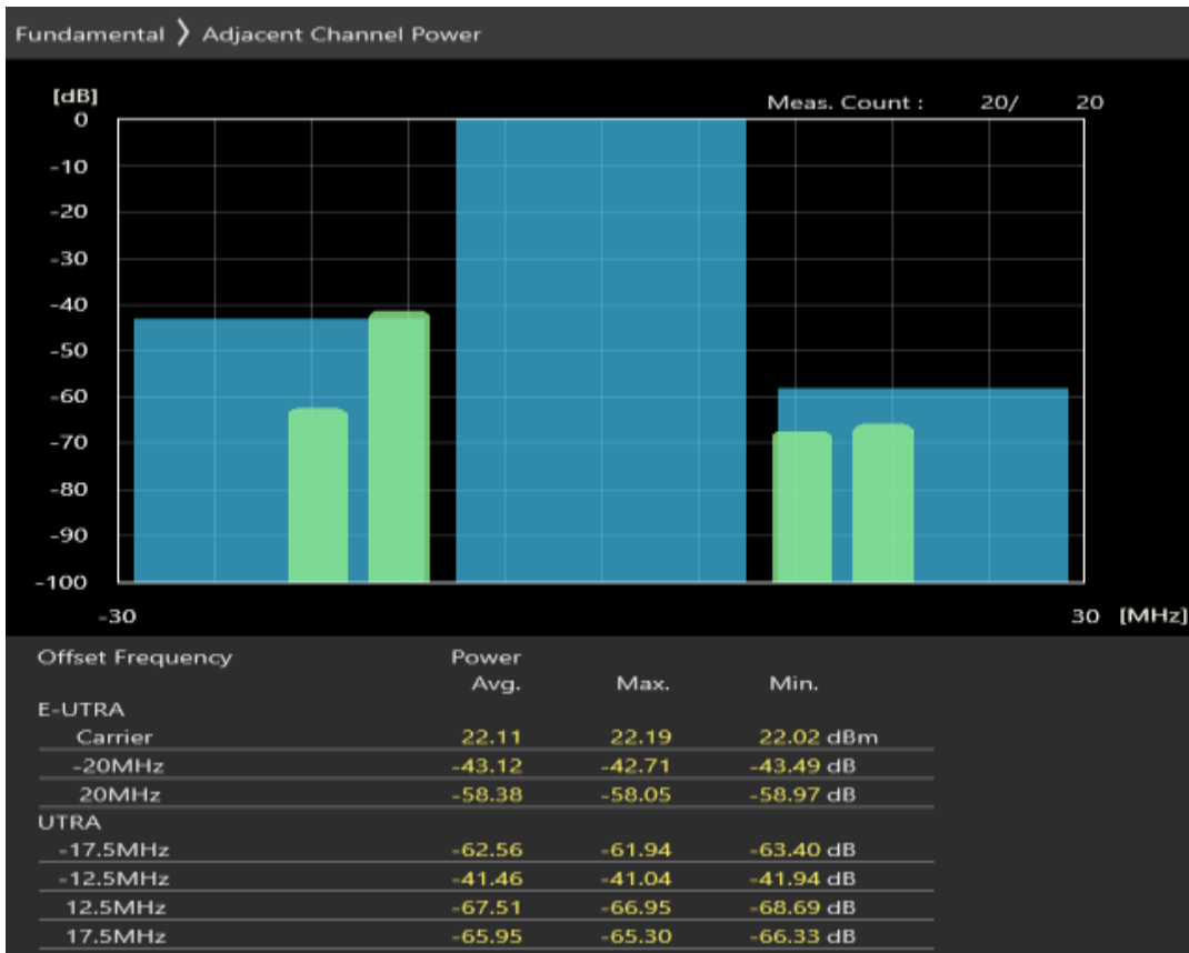
Band3 QAM16 BW=20MHz Channel=19850 RB Size=18 Position=#Max
