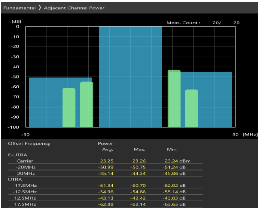
Band1 QPSK BW=20MHz Channel=18500 RB Size=100 Position=#0
