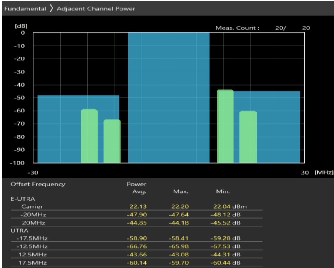
Band3 QAM16 BW=20MHz Channel=19575 RB Size=100 Position=#0
