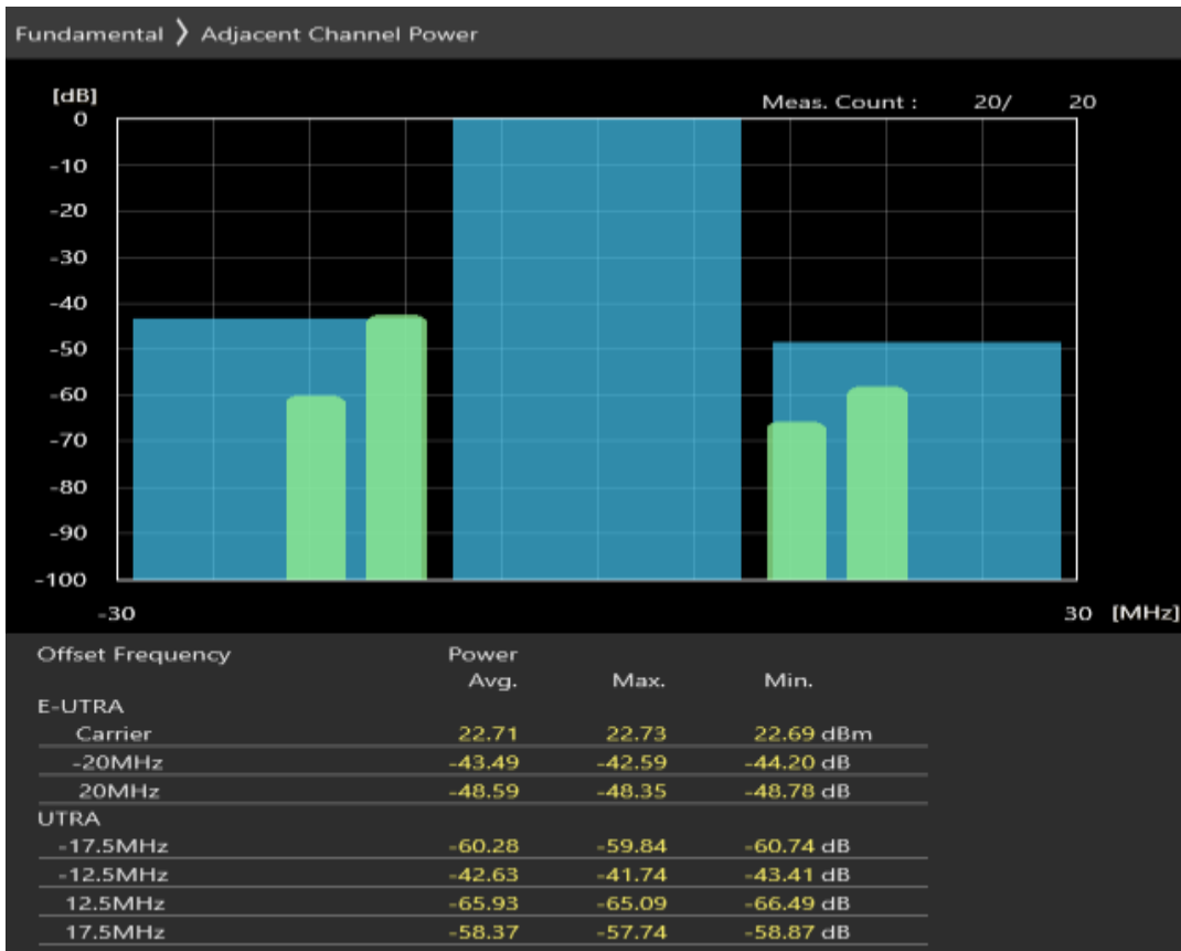
Band3 QPSK BW=20MHz Channel=19575 RB Size=18 Position=#Max
