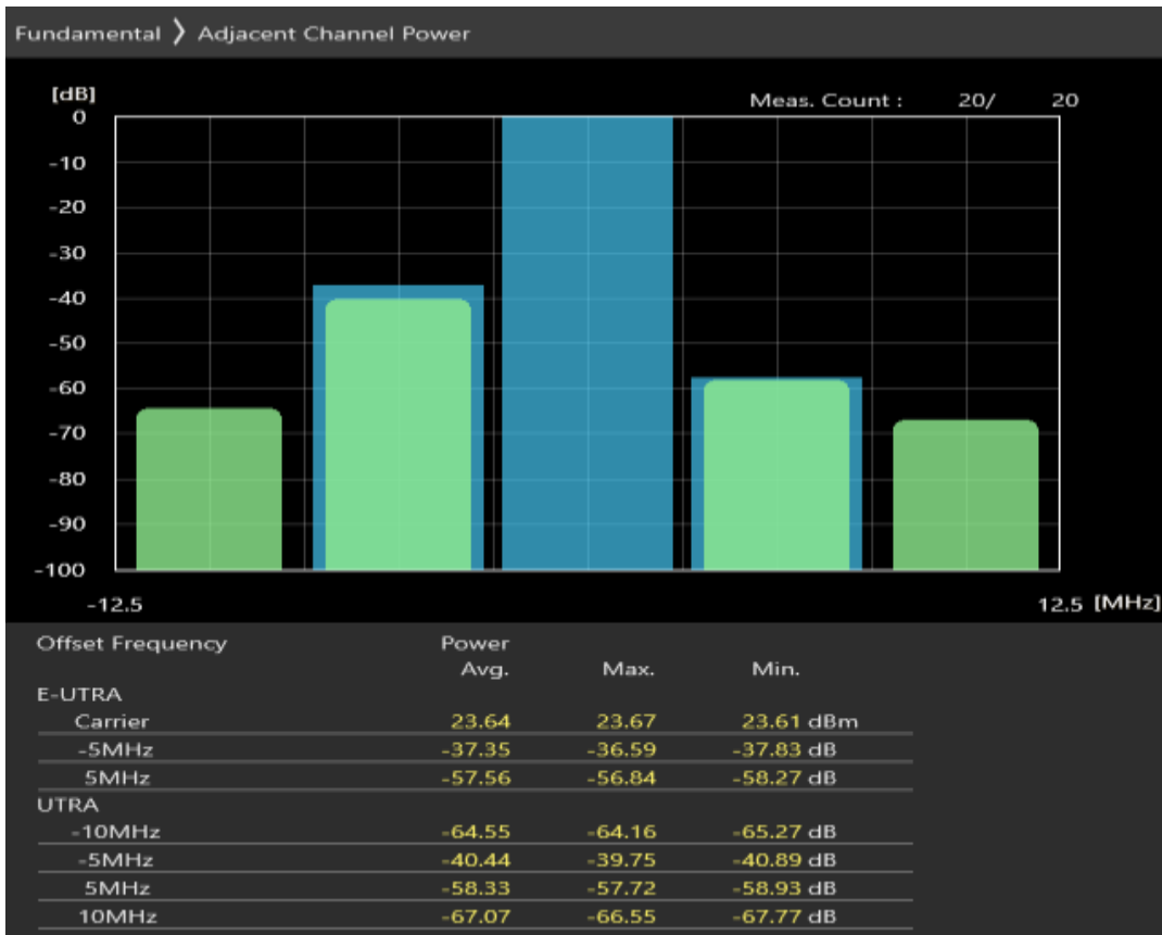
Band7 QPSK BW=5MHz Channel=21425 RB Size=8 Position=#Max
