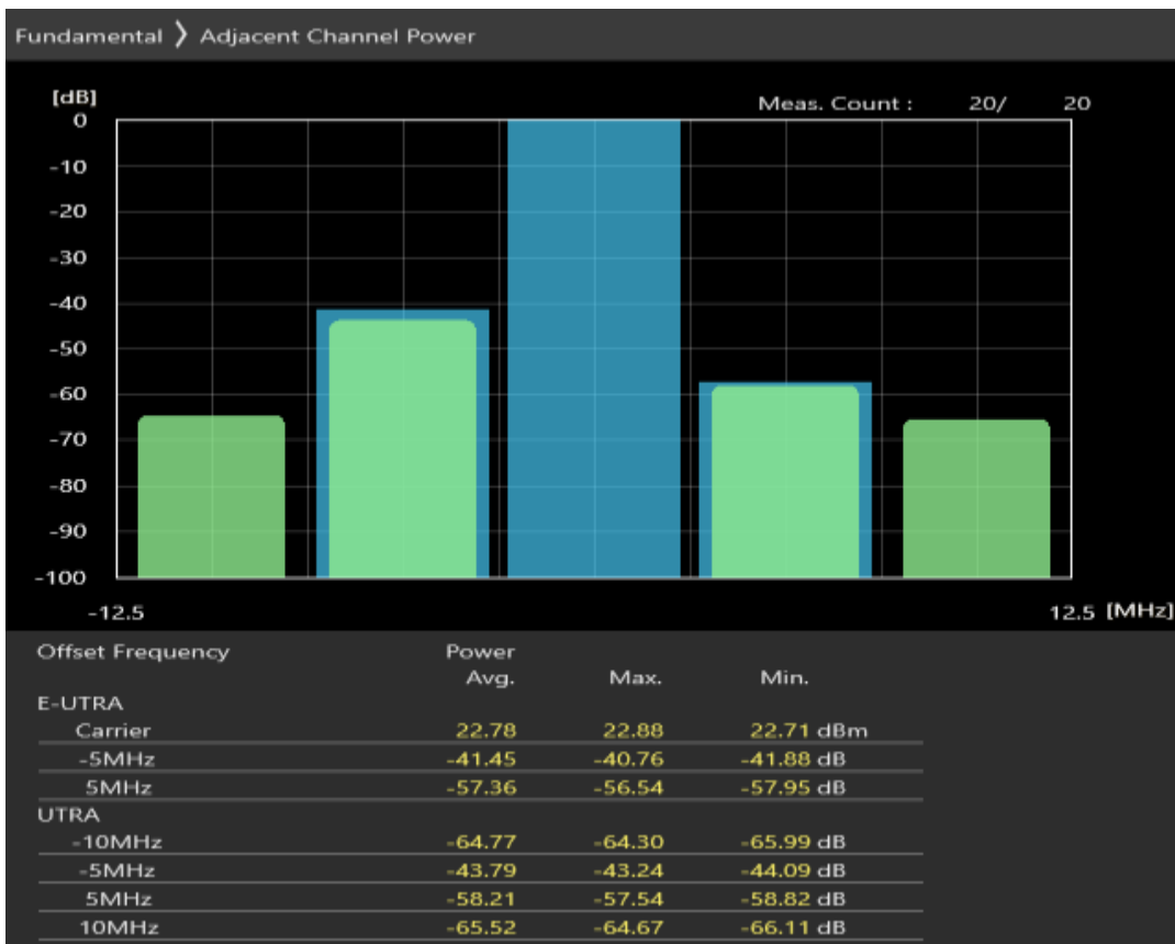
Band7 QAM16 BW=5MHz Channel=20775 RB Size=8 Position=#Max
