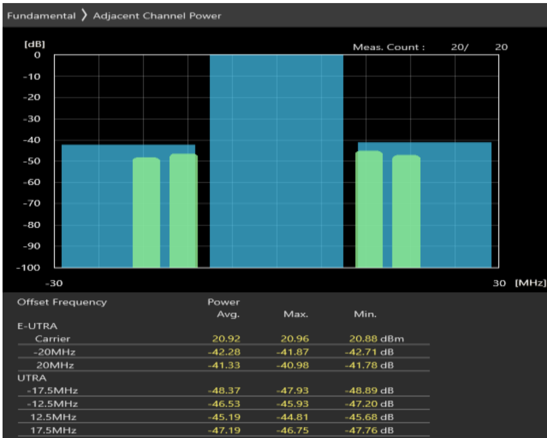
Band3 QPSK BW=20MHz Channel=19850 RB Size=18 Position=#0
