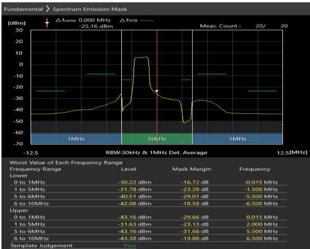
Band1 QAM16 BW=5MHz Channel=18300 RB Size=8 Position=#Max
