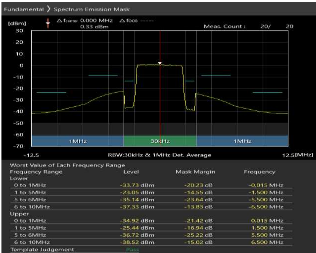
Band7 QPSK BW=10MHz Channel=20800 RB Size=12 Position=#0
