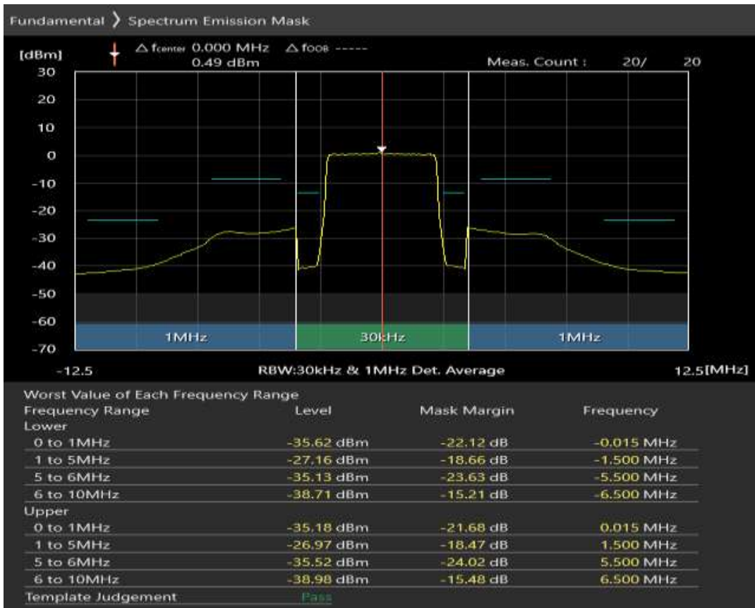
Band3 QAM16 BW=5MHz Channel=19575 RB Size=8 Position=#0
