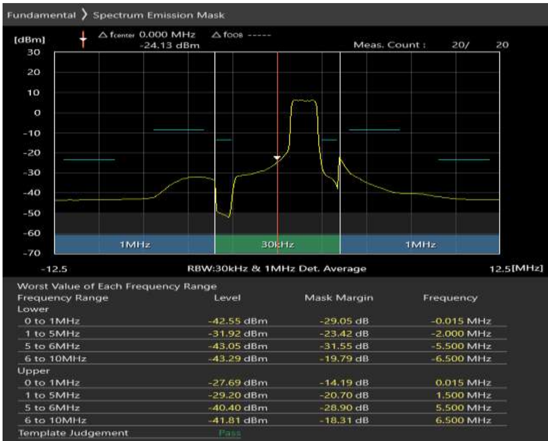
Band1 QAM16 BW=5MHz Channel=18575 RB Size=25 Position=#0
