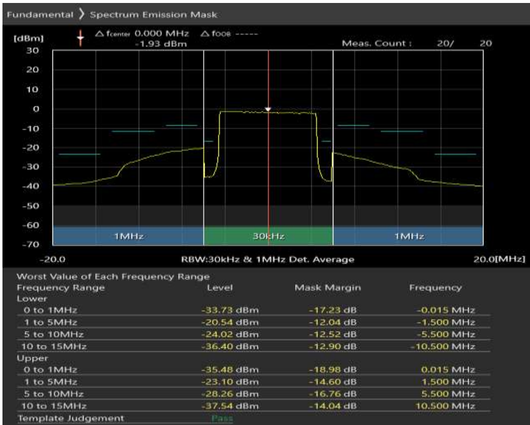
Band7 QAM16 BW=10MHz Channel=21400 RB Size=12 Position=#0
