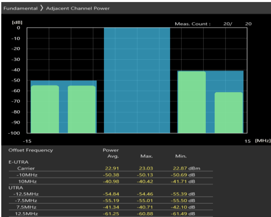
Band3 QPSK BW=10MHz Channel=19250 RB Size=50 Position=#0
