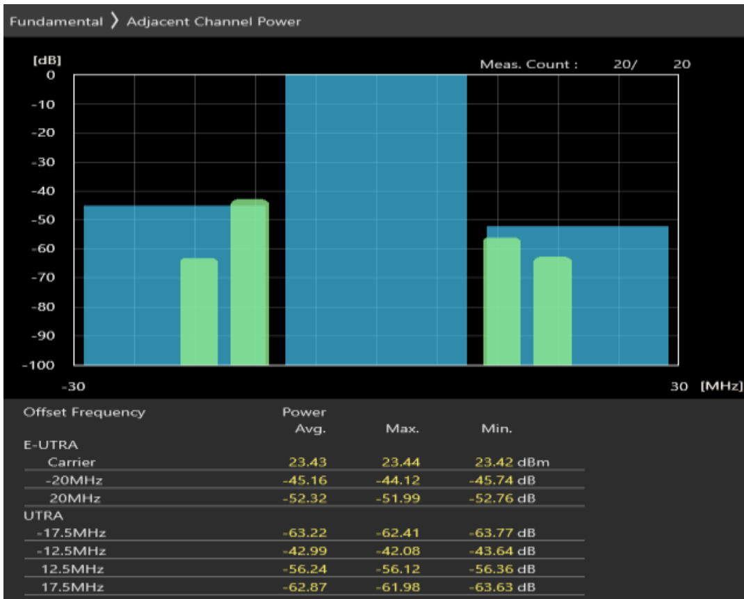
Band1 QPSK BW=20MHz Channel=18500 RB Size=18 Position=#Max
