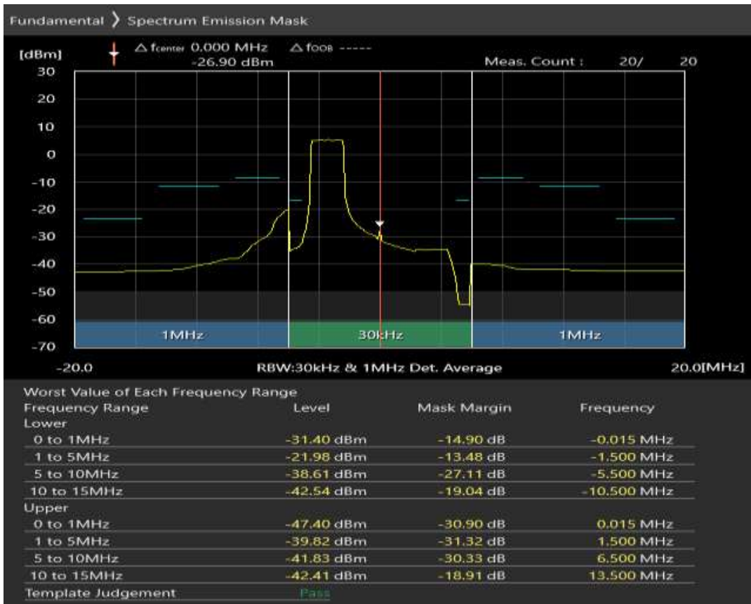
Band7 QPSK BW=10MHz Channel=20800 RB Size=12 Position=#Max
