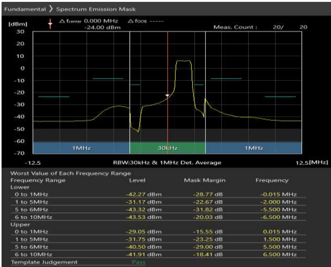
Band1 QAM16 BW=5MHz Channel=18300 RB Size=25 Position=#0
