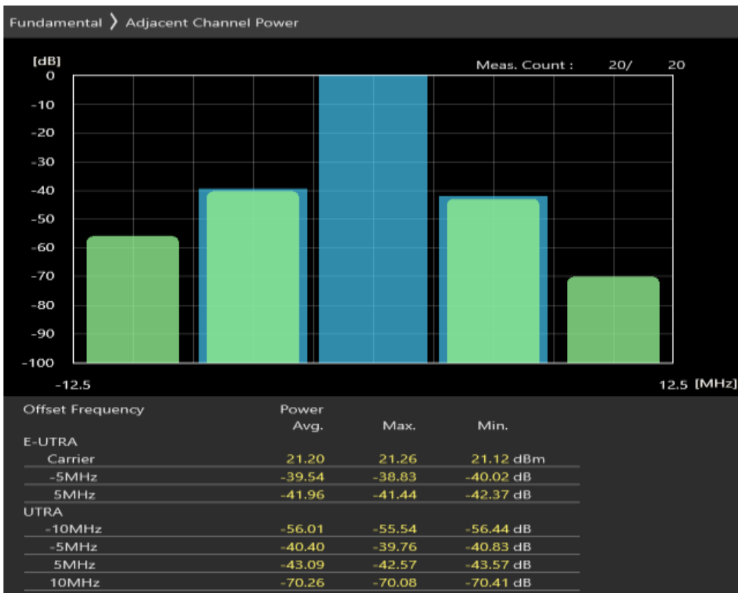
Band8 QPSK BW=10MHz Channel=21500 RB Size=12 Position=#0
