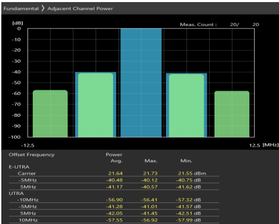
Band7 QPSK BW=5MHz Channel=21425 RB Size=8 Position=#0
