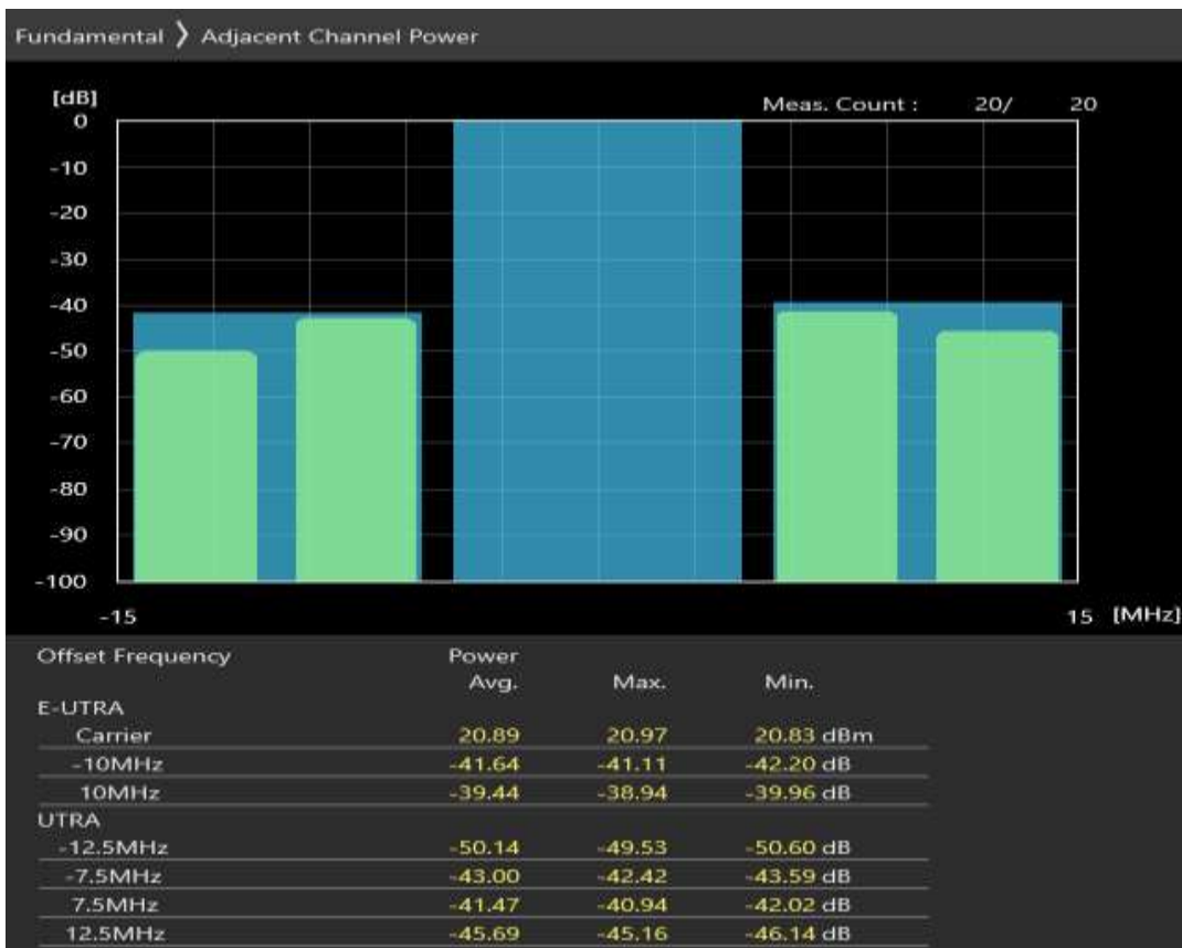
Band3 QPSK BW=10MHz Channel=19575 RB Size=12 Position=#0
