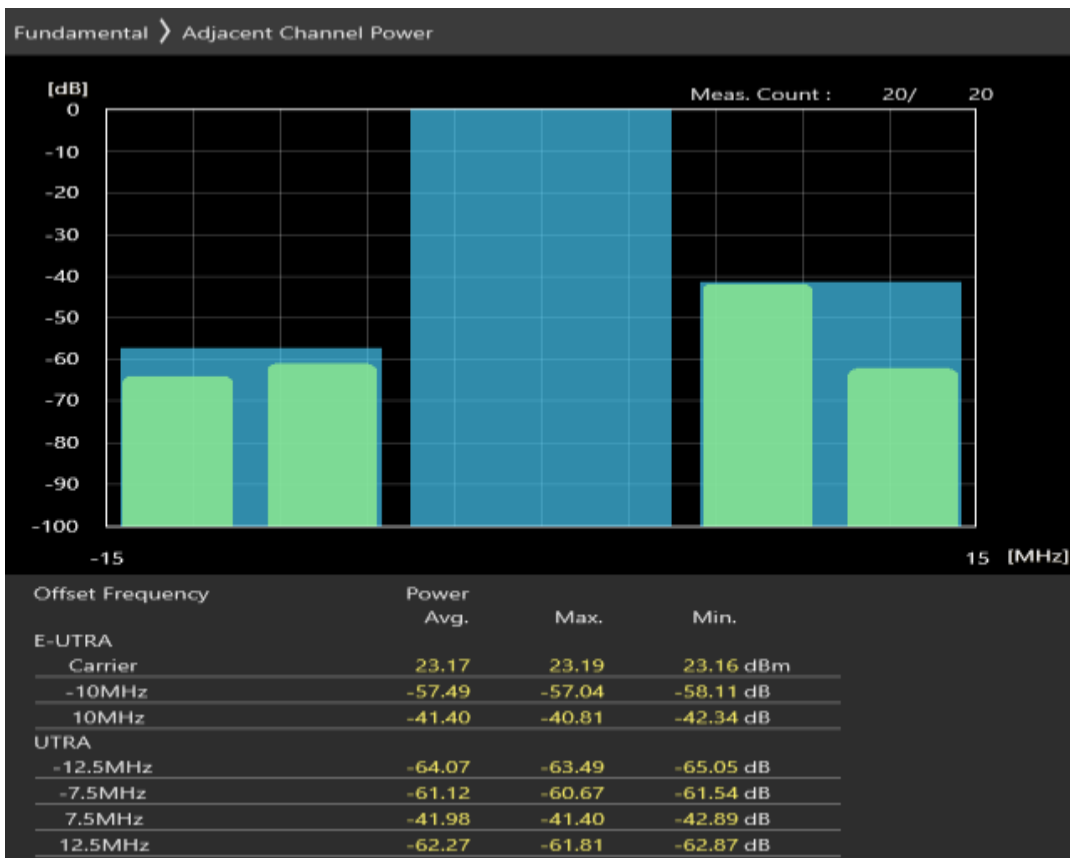
Band8 QPSK BW=10MHz Channel=21500 RB Size=50 Position=#0
