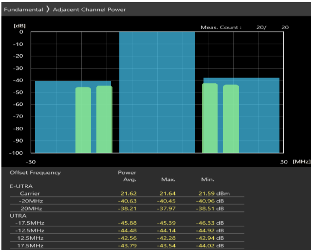
Band7 QPSK BW=20MHz Channel=21100 RB Size=18 Position=#0
