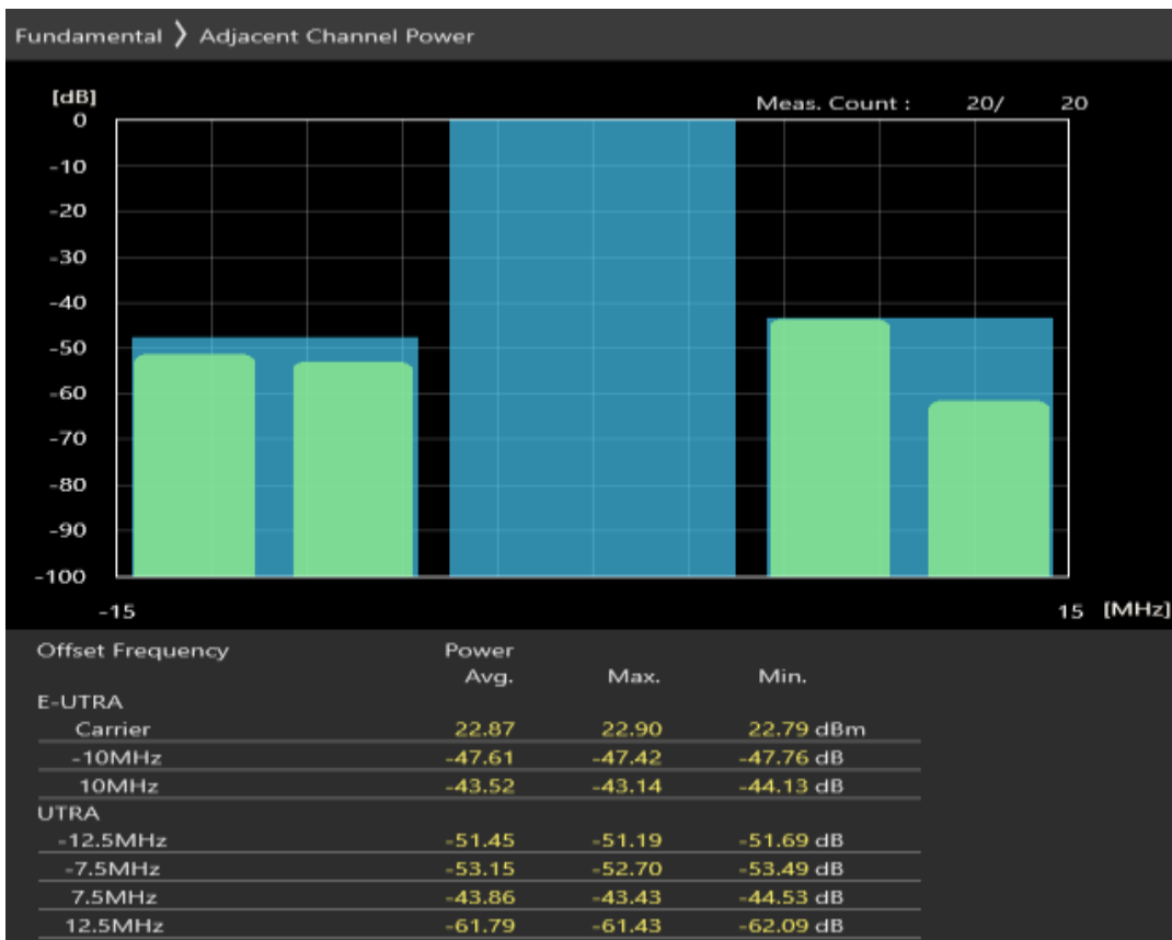
Band3 QPSK BW=10MHz Channel=19575 RB Size=50 Position=#0
