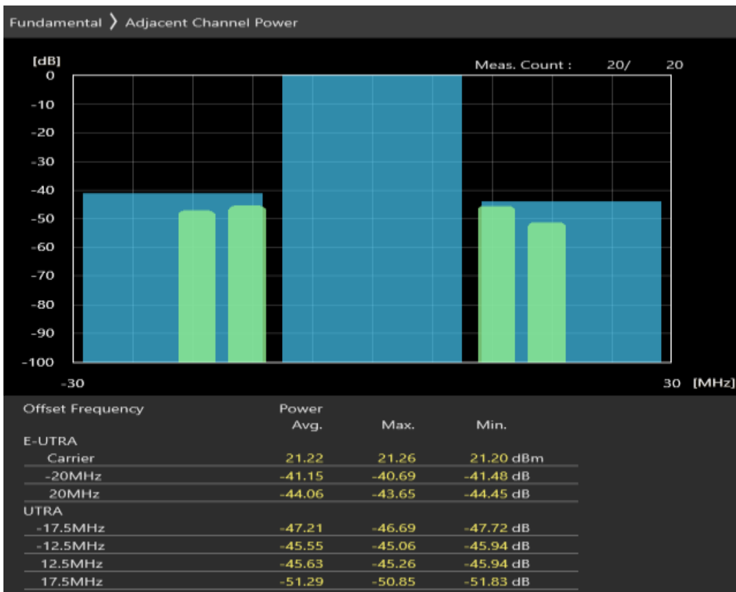
Band7 QPSK BW=5MHz Channel=20775 RB Size=8 Position=#0
