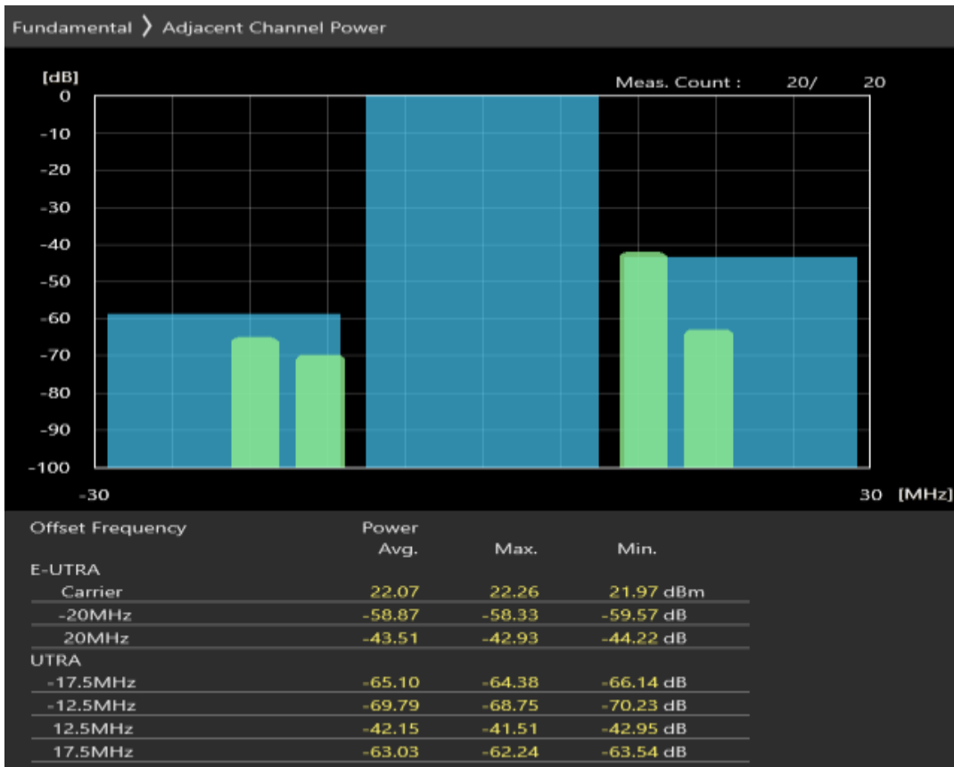
Band3 QAM16 BW=20MHz Channel=19300 RB Size=100 Position=#0
