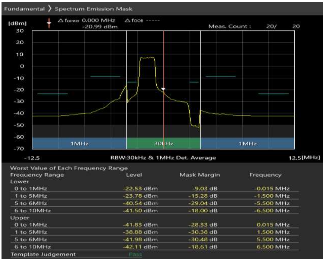
Band7 QPSK BW=5MHz Channel=21100 RB Size=8 Position=#Max
