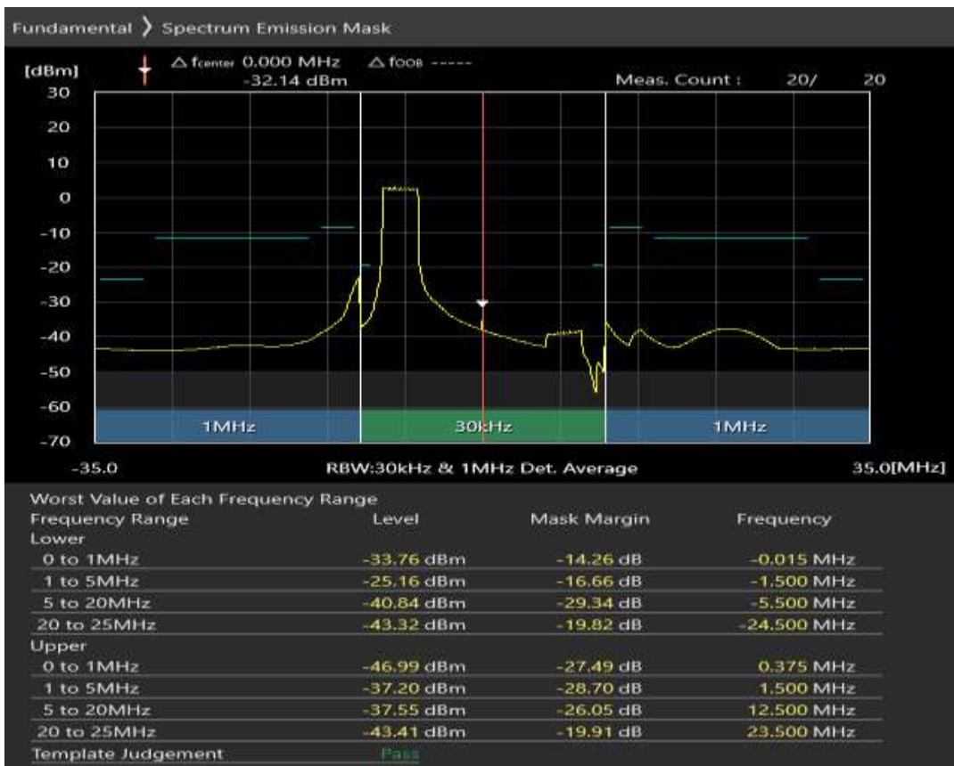
Band1 QAM16 BW=20MHz Channel=18500 RB Size=18 Position=#Max
