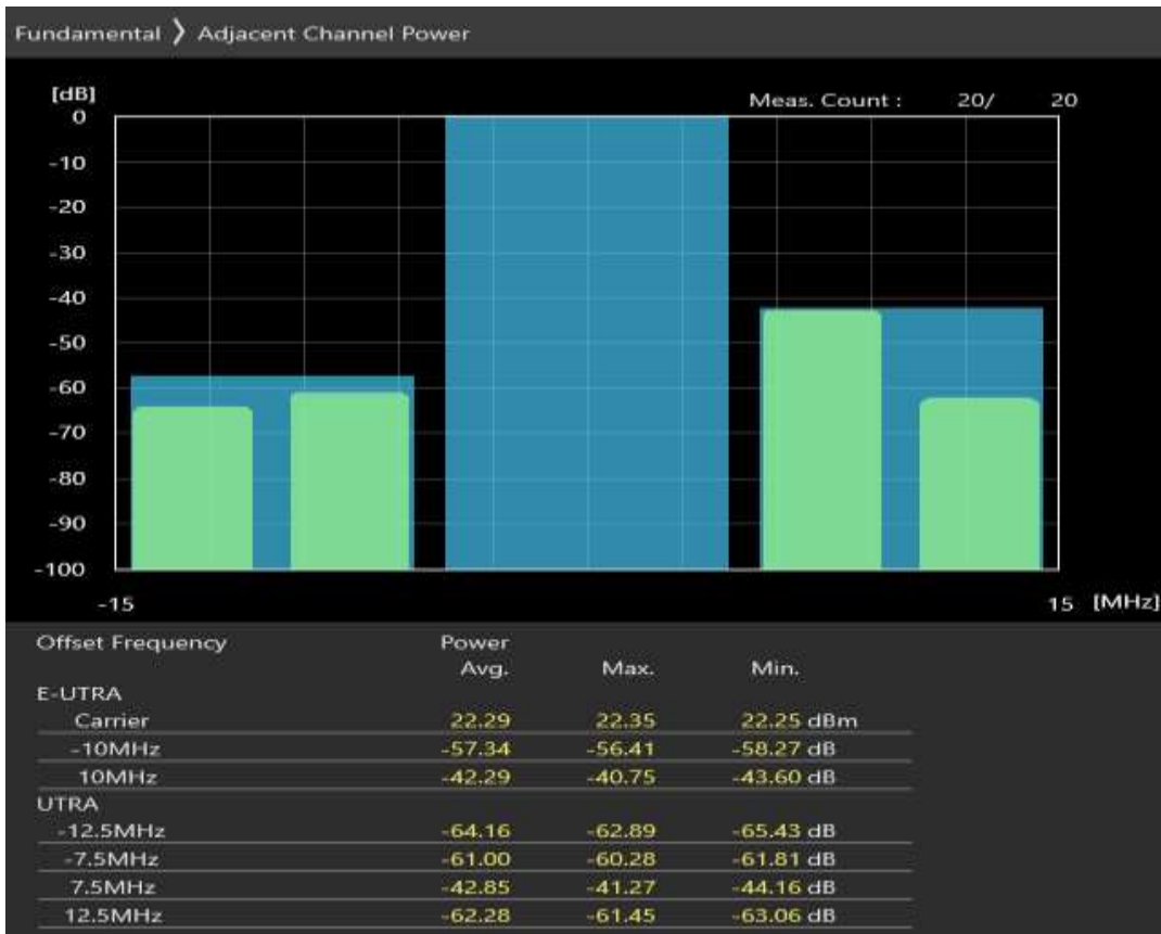
Band8 QAM16 BW=10MHz Channel=21500 RB Size=50 Position=#0
