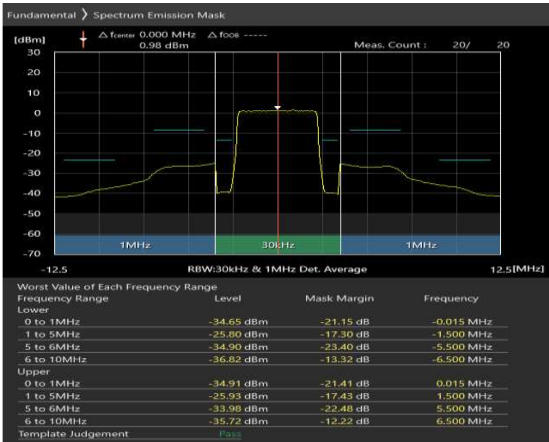
Band7 QAM16 BW=5MHz Channel=20775 RB Size=8 Position=#0
