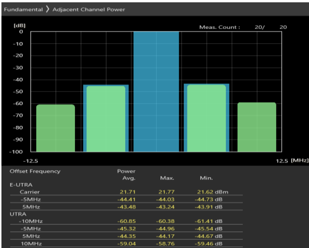
Band1 QPSK BW=5MHz Channel=18575 RB Size=8 Position=#0
