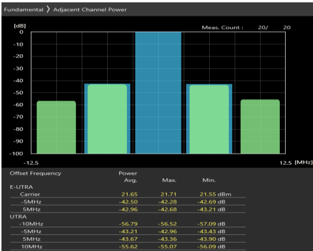
Band7 QPSK BW=5MHz Channel=21100 RB Size=8 Position=#0
