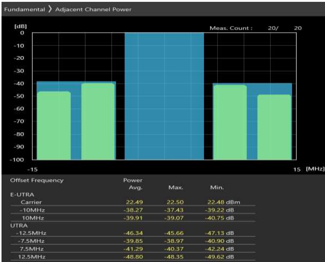
Band8 QAM16 BW=10MHz Channel=21625 RB Size=12 Position=#0
