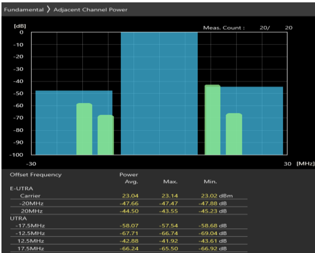
Band3 QPSK BW=20MHz Channel=19850 RB Size=100 Position=#0
