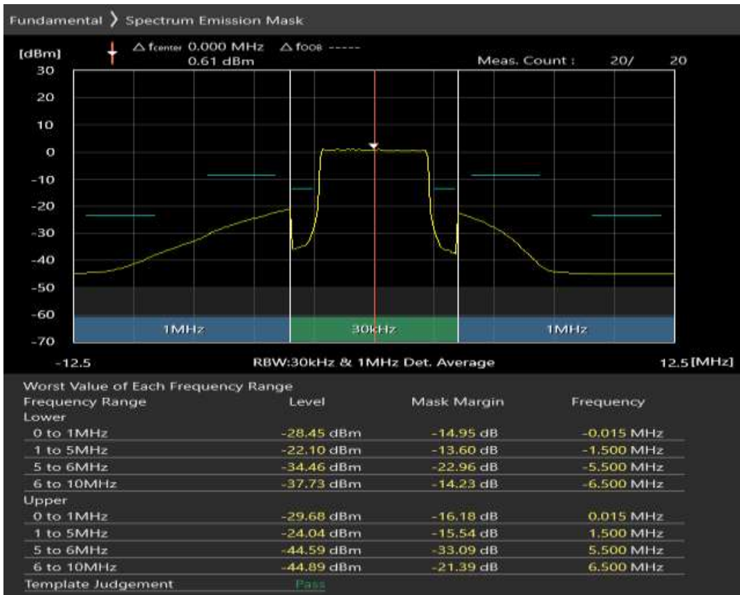
Band8 QPSK BW=10MHz Channel=21500 RB Size=12 Position=#0
