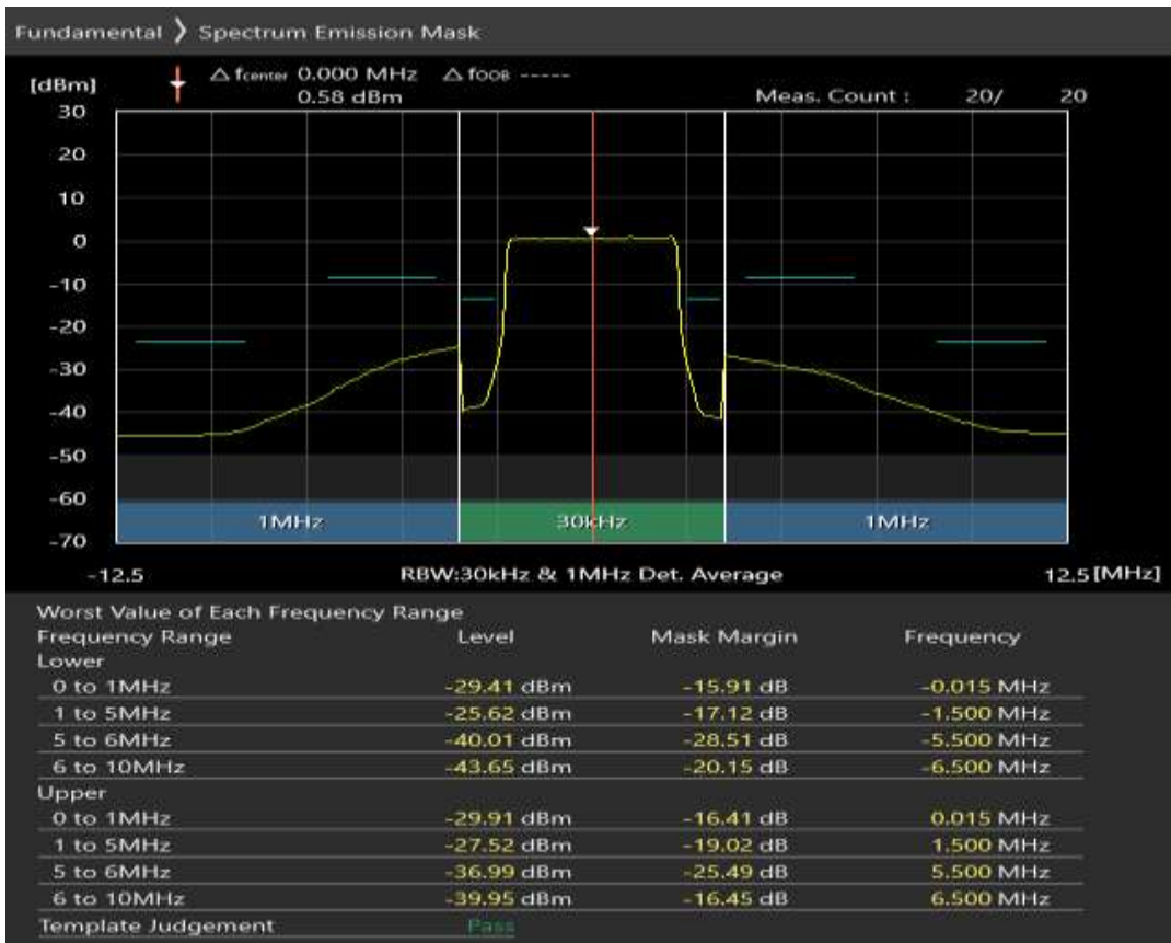
Band8 QPSK BW=5MHz Channel=21625 RB Size=8 Position=#0
