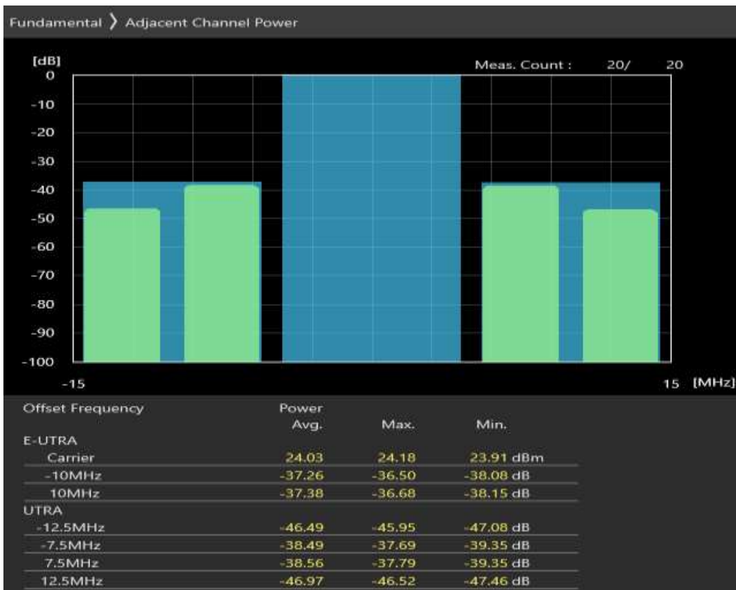
Band7 QAM16 BW=10MHz Channel=21400 RB Size=12 Position=#0
