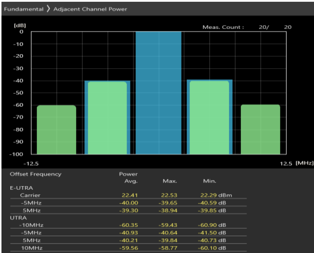
Band3 QPSK BW=5MHz Channel=19575 RB Size=8 Position=#0
