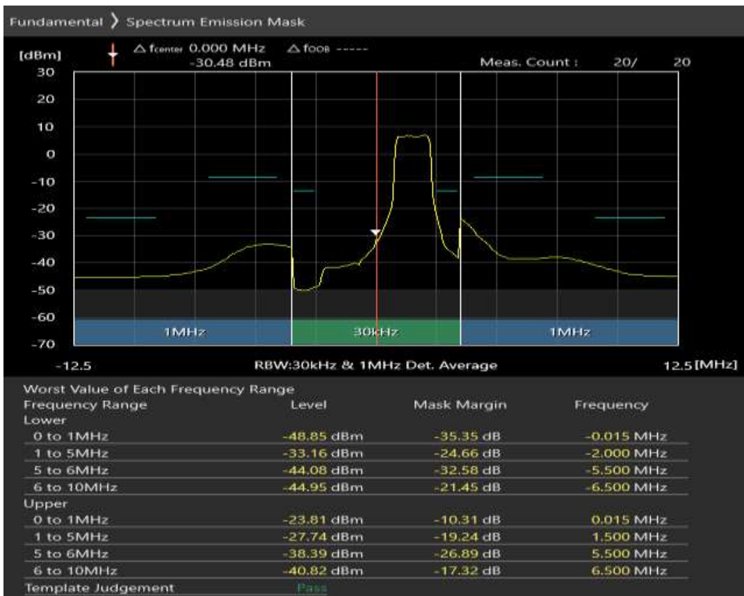
Band8 QAM16 BW=5MHz Channel=21475 RB Size=25 Position=#0
