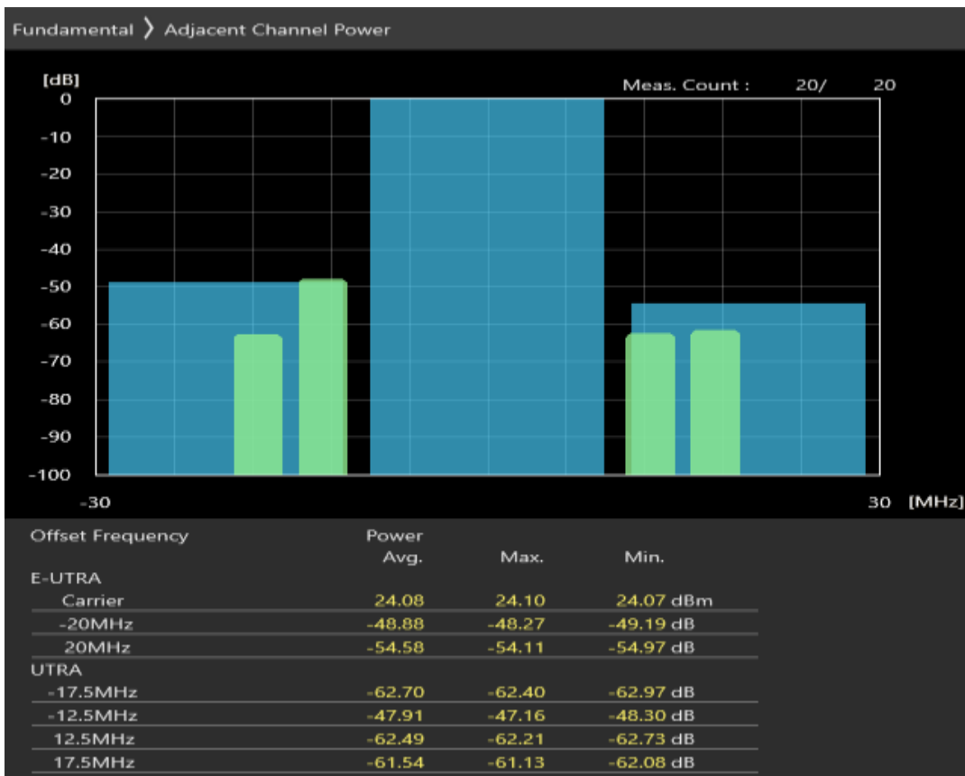
Band20 QPSK BW=20MHz Channel=24350 RB Size=18 Position=#Max
