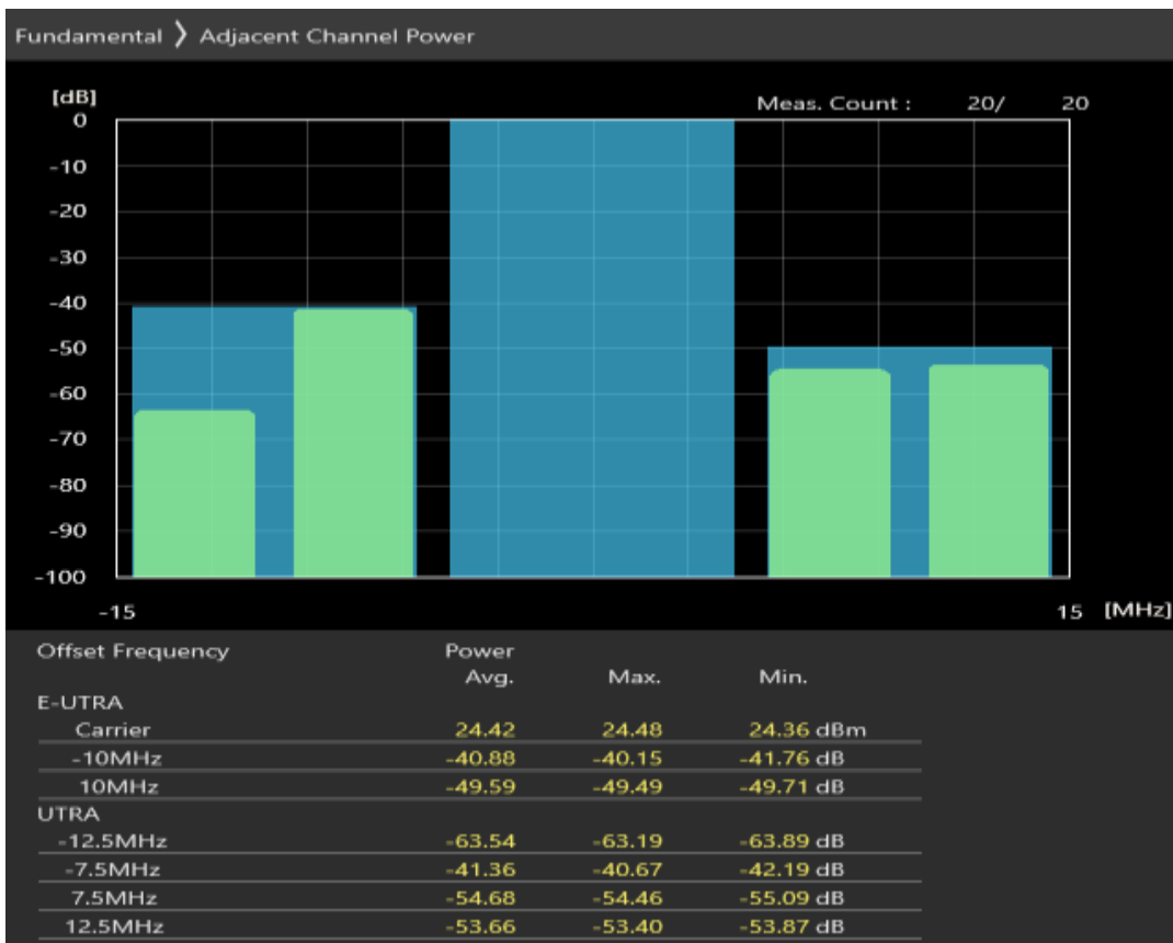
Band3 QPSK BW=10MHz Channel=19250 RB Size=12 Position=#Max
