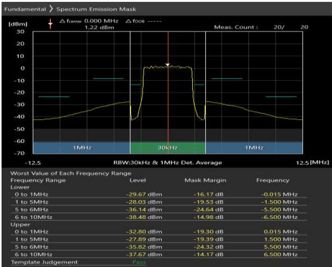
Band40 QPSK BW=5MHz Channel=39150 RB Size=8 Position=#0
