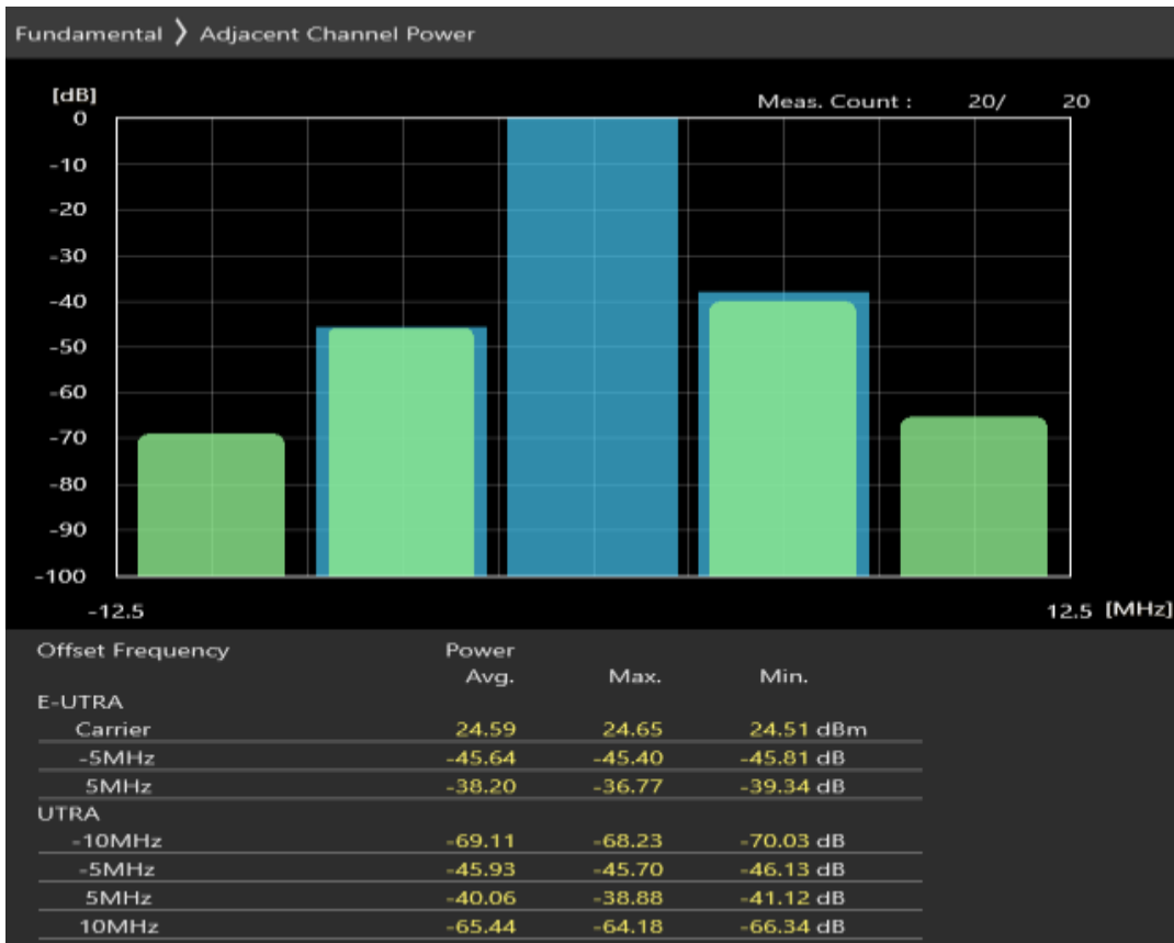
Band3 QPSK BW=5MHz Channel=19925 RB Size=25 Position=#0
