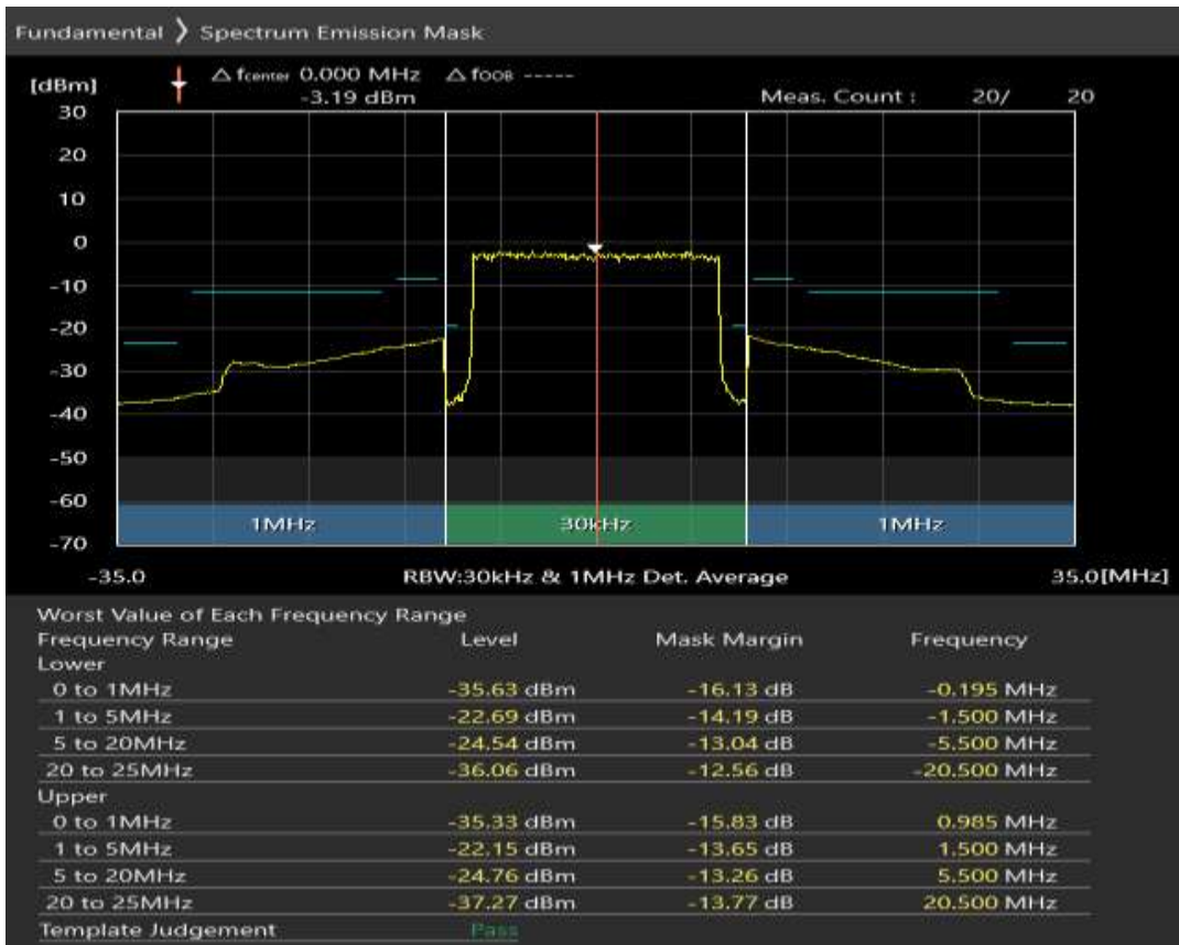
Band40 QAM16 BW=20MHz Channel=39150 RB Size=18 Position=#0
