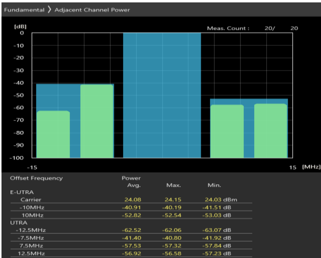
Band20 QPSK BW=10MHz Channel=24400 RB Size=12 Position=#Max
