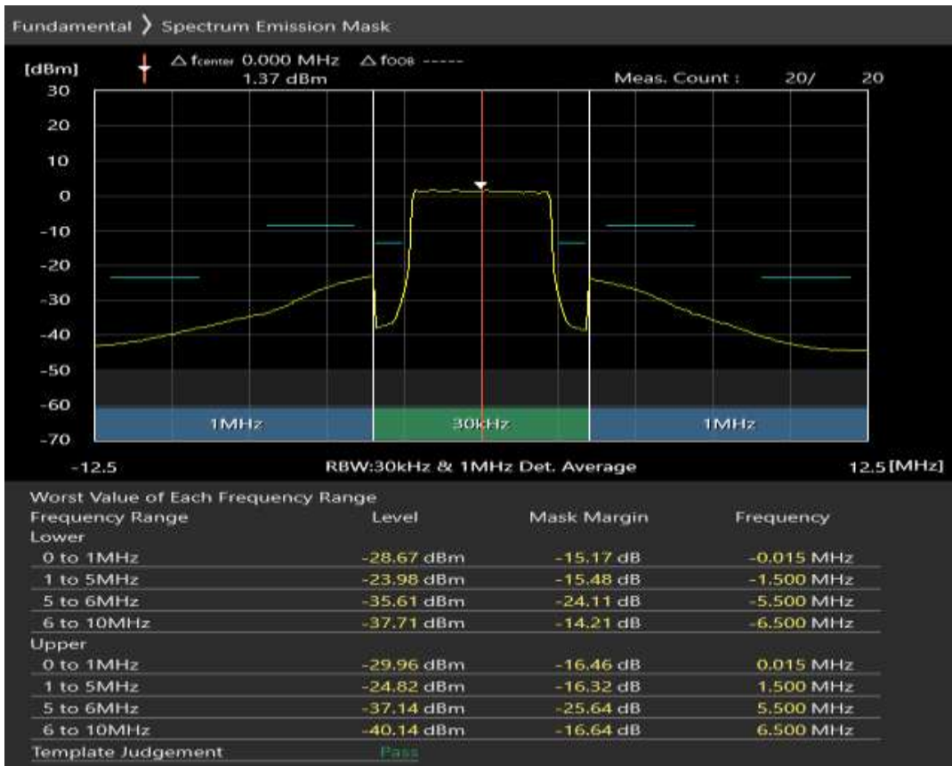
Band3 QPSK BW=10MHz Channel=19250 RB Size=12 Position=#0
