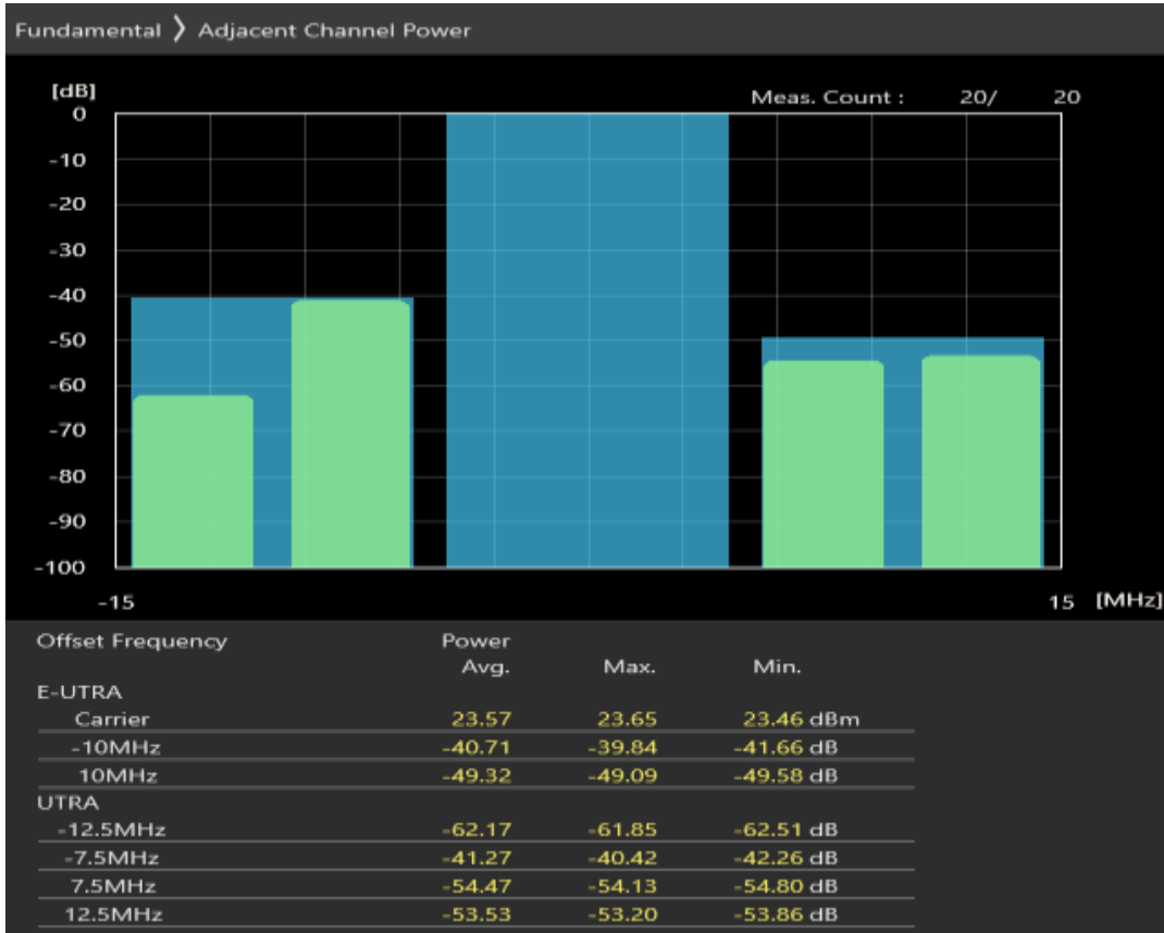
Band3 QAM16 BW=10MHz Channel=19575 RB Size=12 Position=#Max
