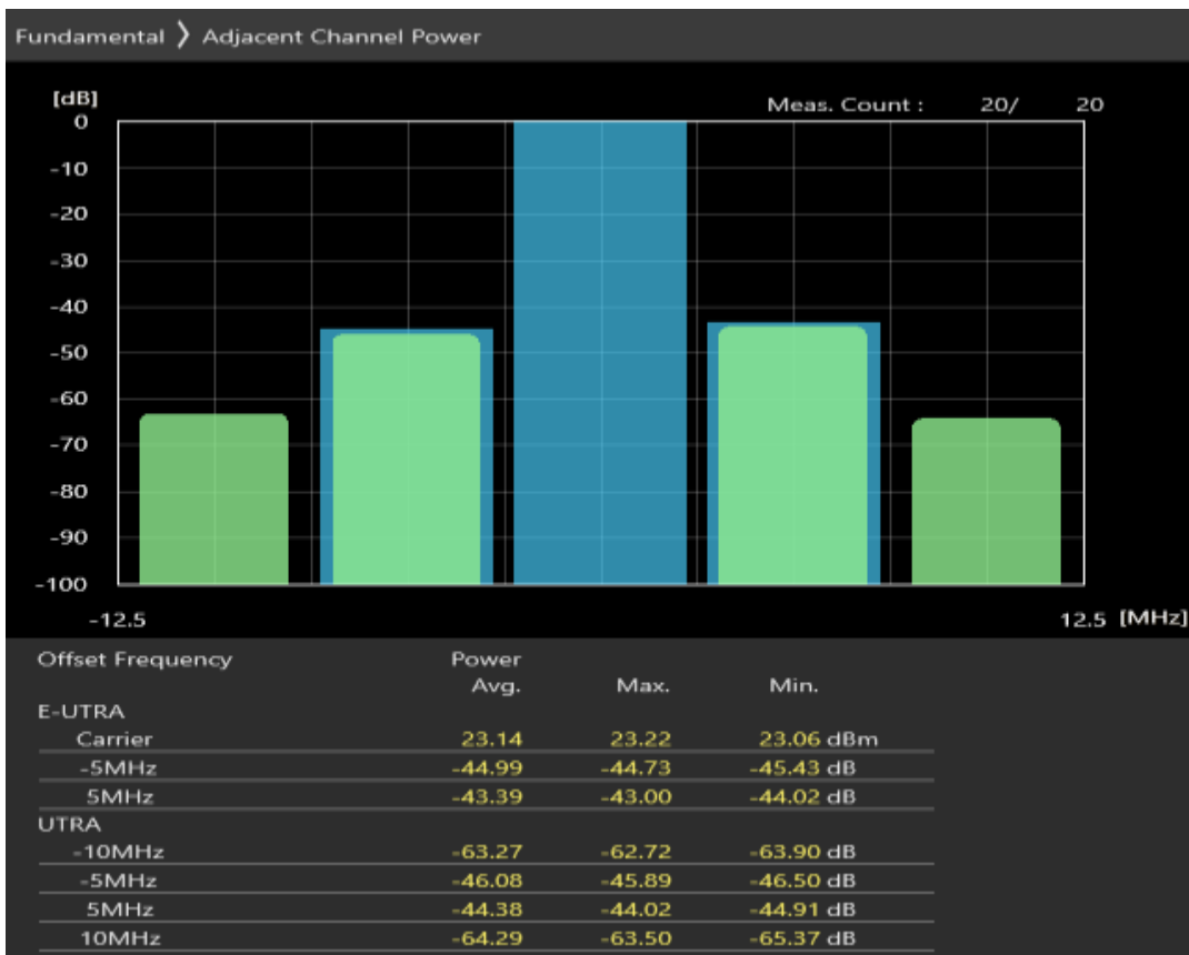
Band20 QAM16 BW=5MHz Channel=24300 RB Size=8 Position=#0
