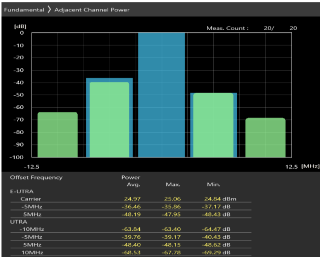
Band7 QPSK BW=5MHz Channel=21425 RB Size=8 Position=#Max
