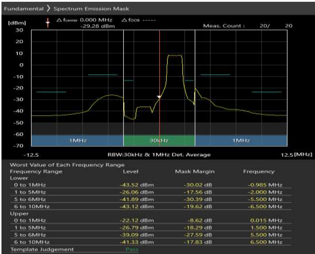
Band1 QPSK BW=5MHz Channel=18025 RB Size=25 Position=#0
