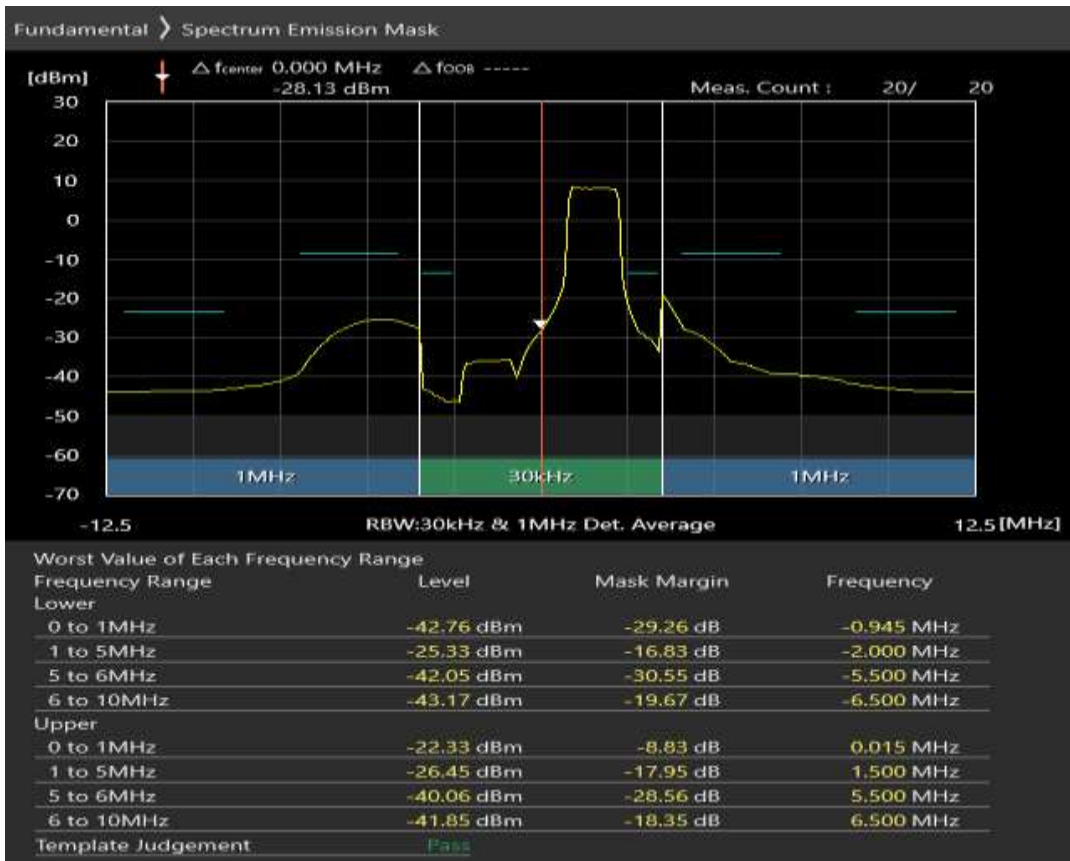
Band1 QPSK BW=5MHz Channel=18300 RB Size=25 Position=#0
