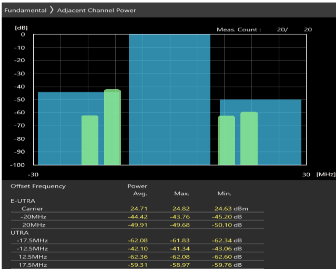
Band7 QPSK BW=20MHz Channel=21350 RB Size=18 Position=#Max
