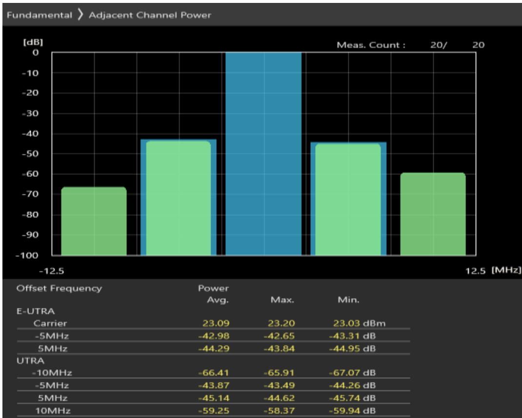
Band8 QAM16 BW=5MHz Channel=21475 RB Size=8 Position=#0
