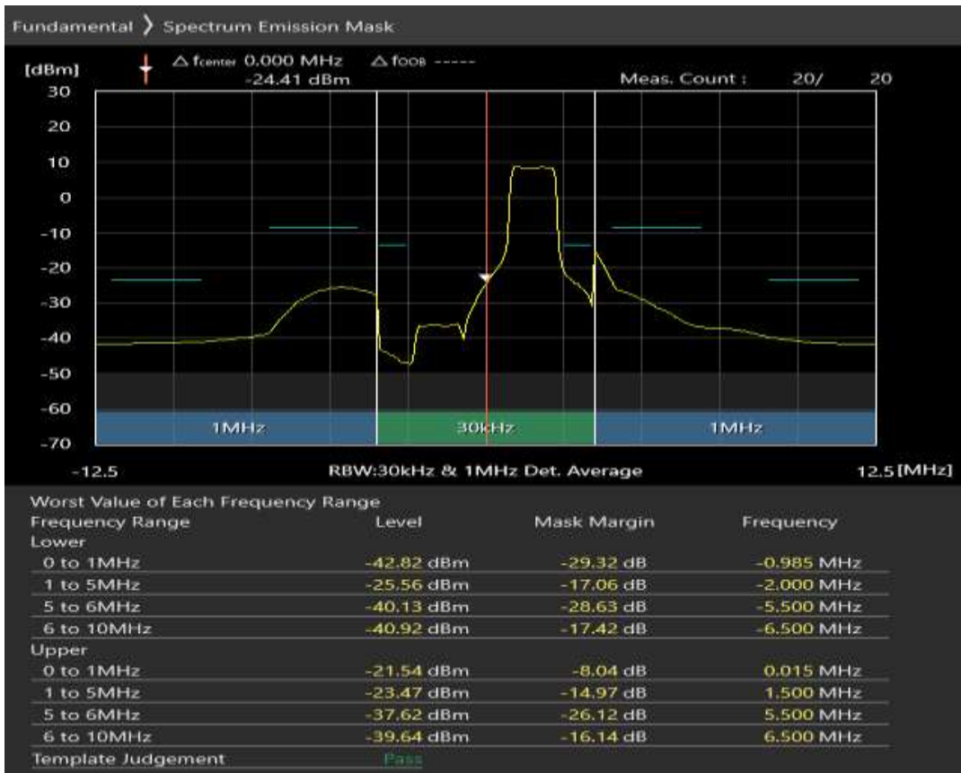
Band7 QPSK BW=5MHz Channel=21425 RB Size=25 Position=#0
