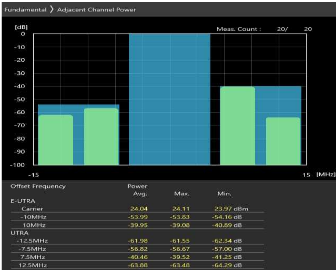
Band8 QPSK BW=10MHz Channel=21500 RB Size=50 Position=#0
