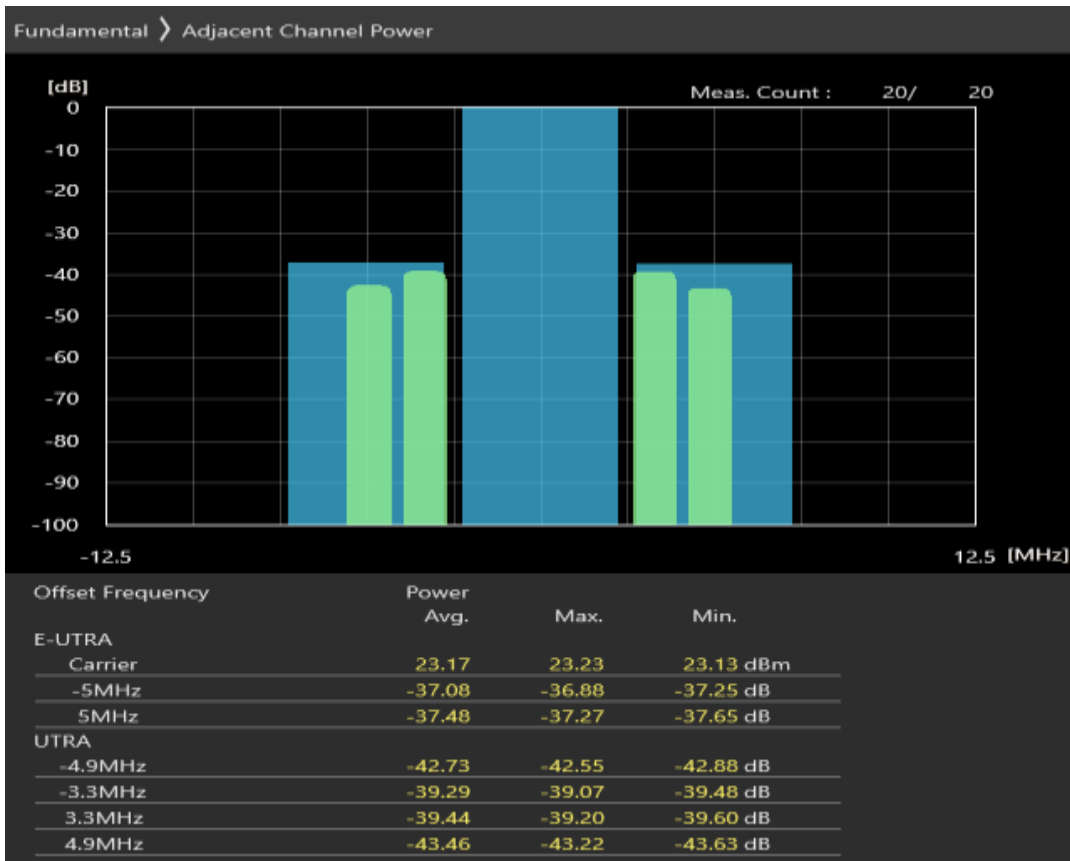
Band40 QPSK BW=10MHz Channel=38700 RB Size=12 Position=#0
