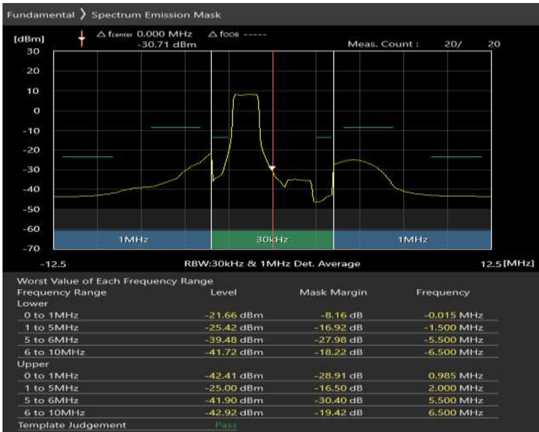
Band1 QPSK BW=5MHz Channel=18575 RB Size=8 Position=#Max
