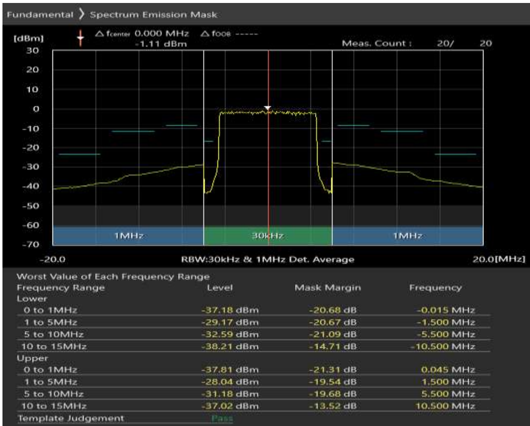
Band40 QPSK BW=10MHz Channel=39150 RB Size=12 Position=#0
