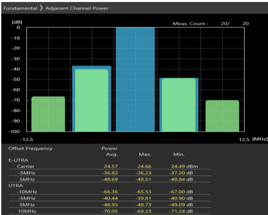
Band3 QPSK BW=5MHz Channel=19575 RB Size=8 Position=#Max
