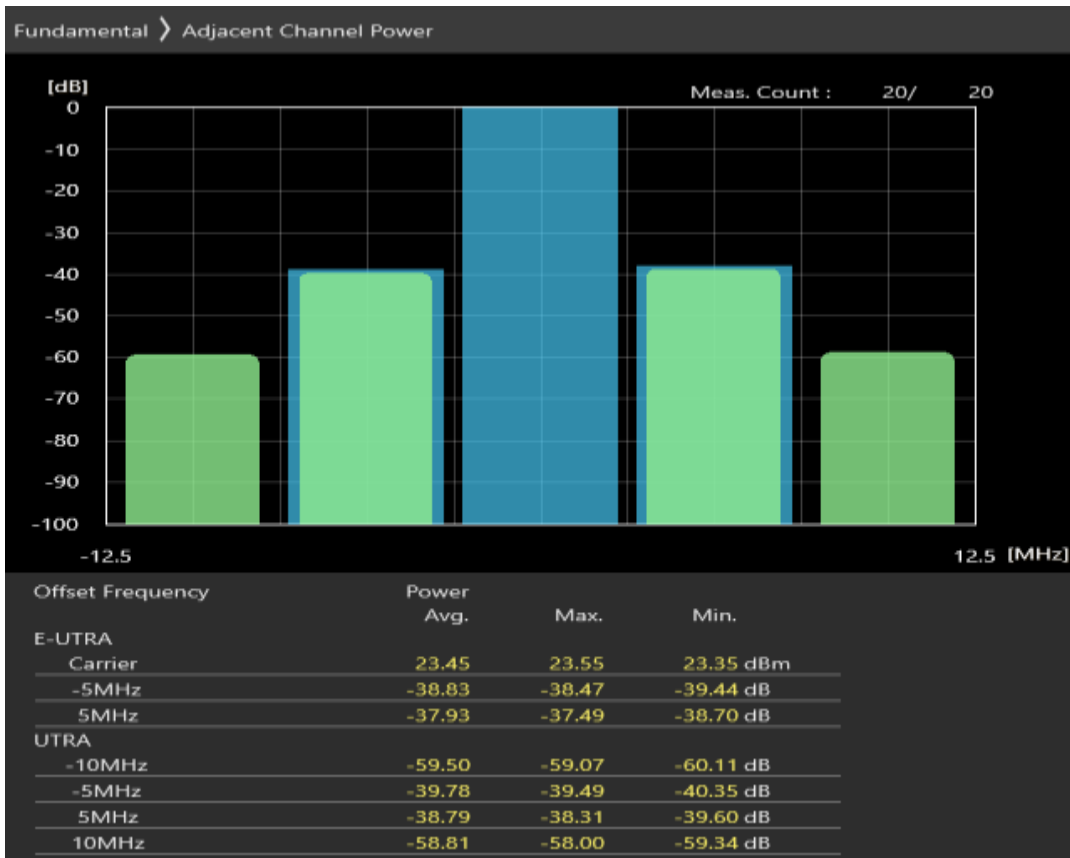
Band3 QAM16 BW=5MHz Channel=19225 RB Size=8 Position=#0
