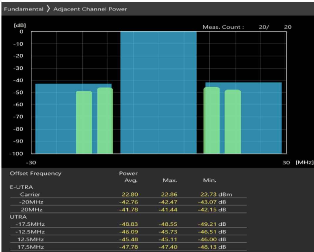
Band7 QPSK BW=20MHz Channel=21350 RB Size=18 Position=#0
