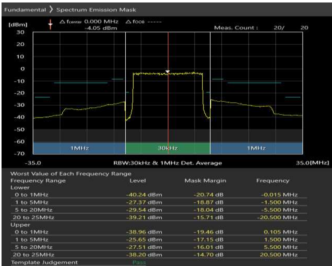
Band40 QAM16 BW=20MHz Channel=38750 RB Size=18 Position=#0
