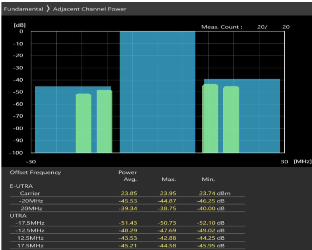
Band7 QAM16 BW=20MHz Channel=20850 RB Size=18 Position=#0
