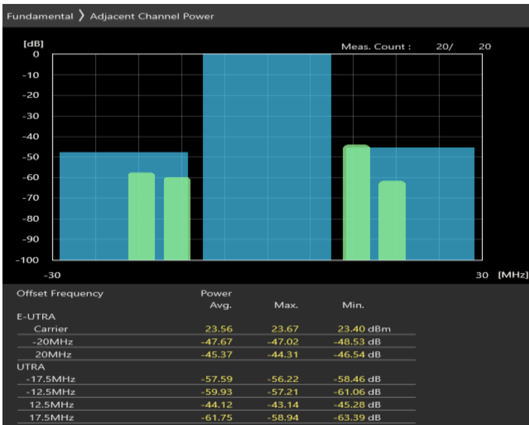
Band3 QAM16 BW=20MHz Channel=19850 RB Size=100 Position=#0
