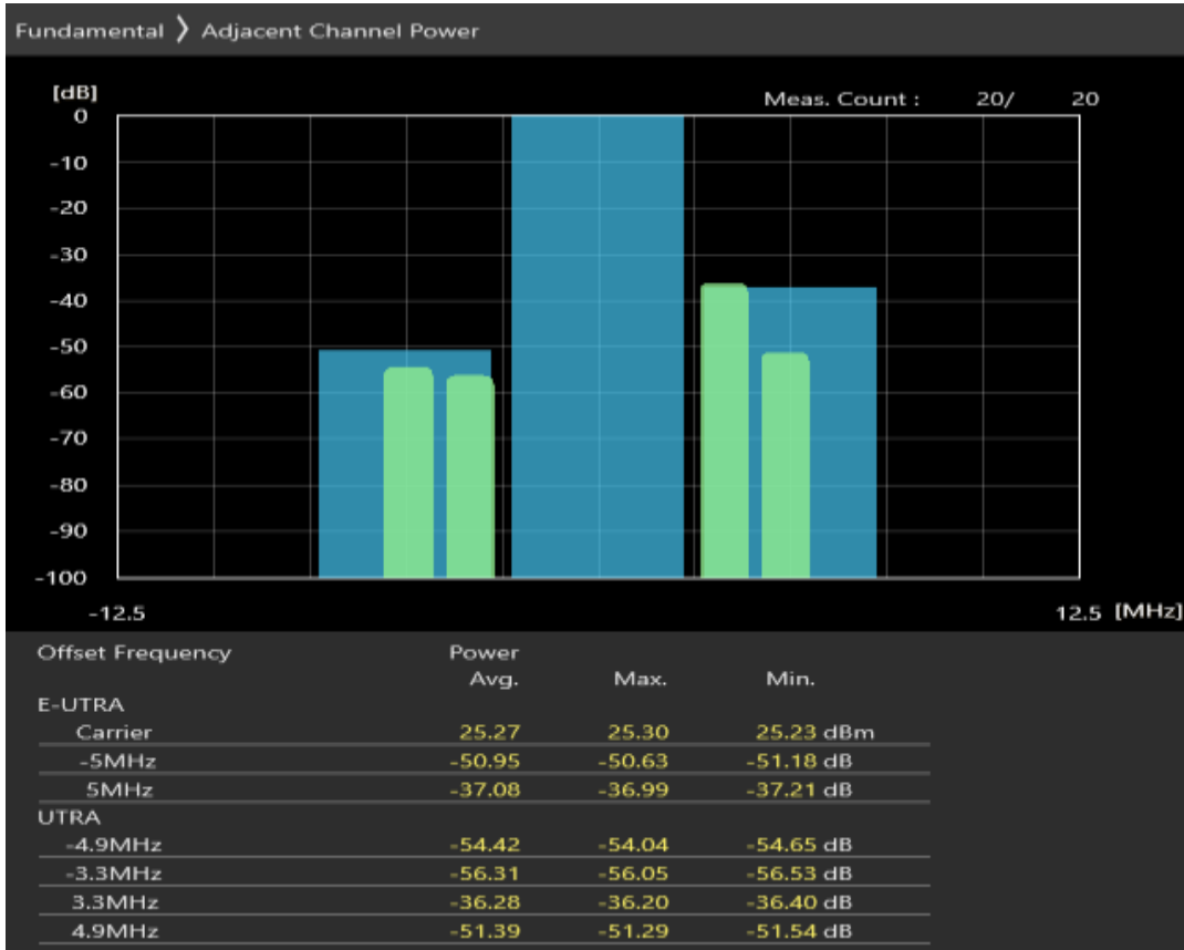
Band40 QPSK BW=5MHz Channel=39150 RB Size=25 Position=#0
