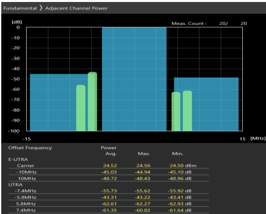
Band40 QPSK BW=10MHz Channel=38700 RB Size=12 Position=#Max
