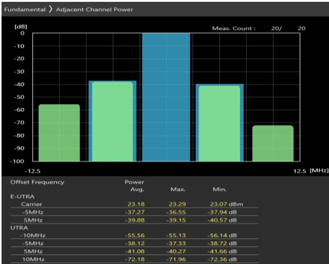
Band8 QAM16 BW=5MHz Channel=21775 RB Size=8 Position=#0
