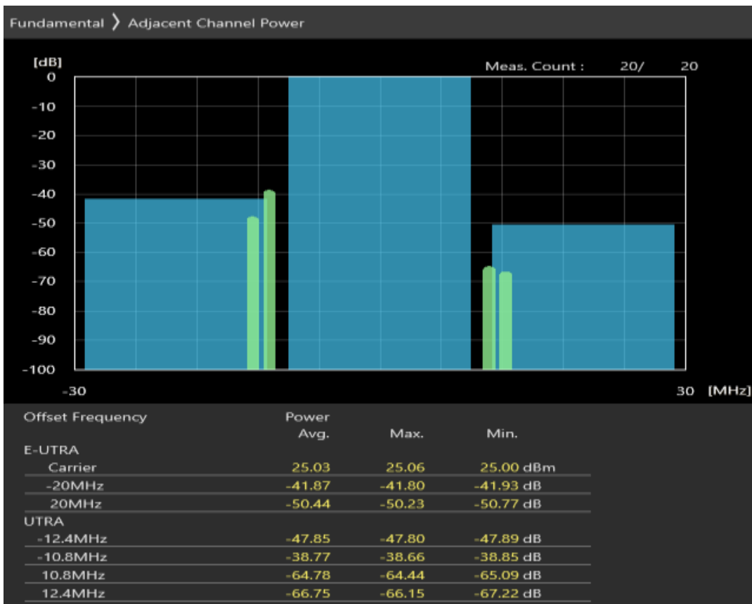
Band40 QPSK BW=20MHz Channel=39150 RB Size=18 Position=#Max
