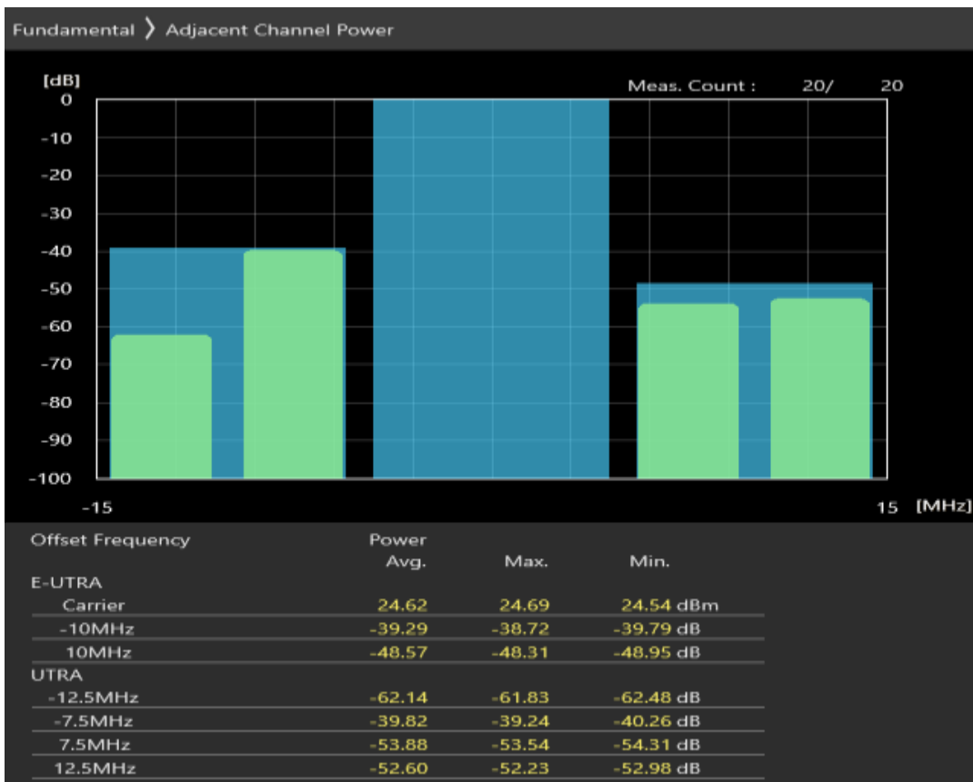
Band3 QPSK BW=10MHz Channel=19575 RB Size=12 Position=#Max
