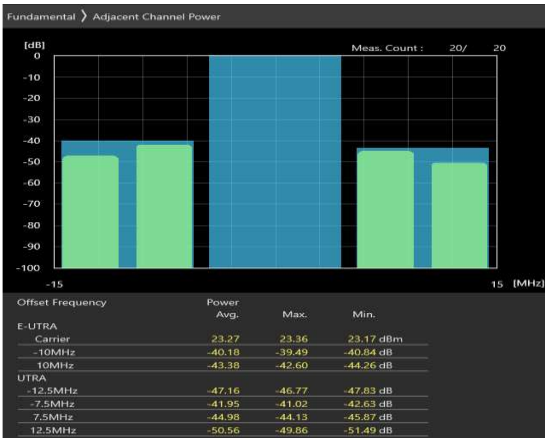
Band8 QAM16 BW=10MHz Channel=21625 RB Size=12 Position=#0
