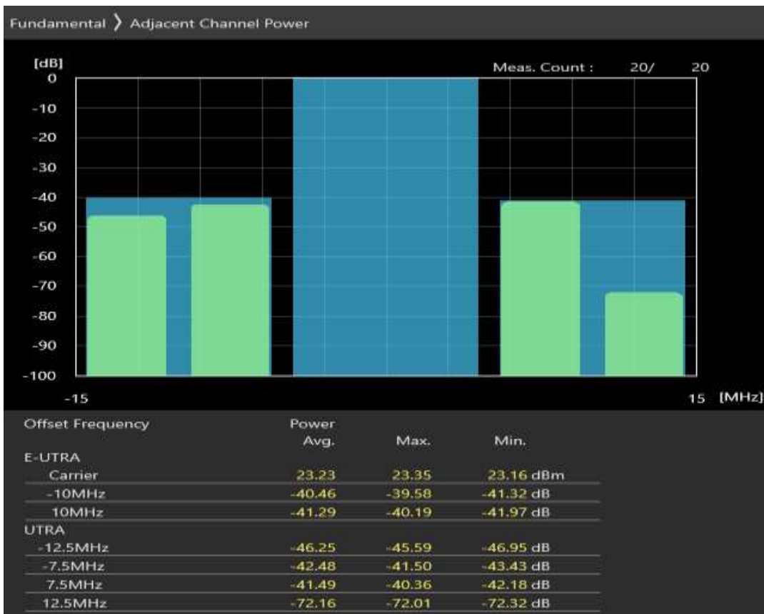
Band8 QAM16 BW=10MHz Channel=21750 RB Size=12 Position=#0
