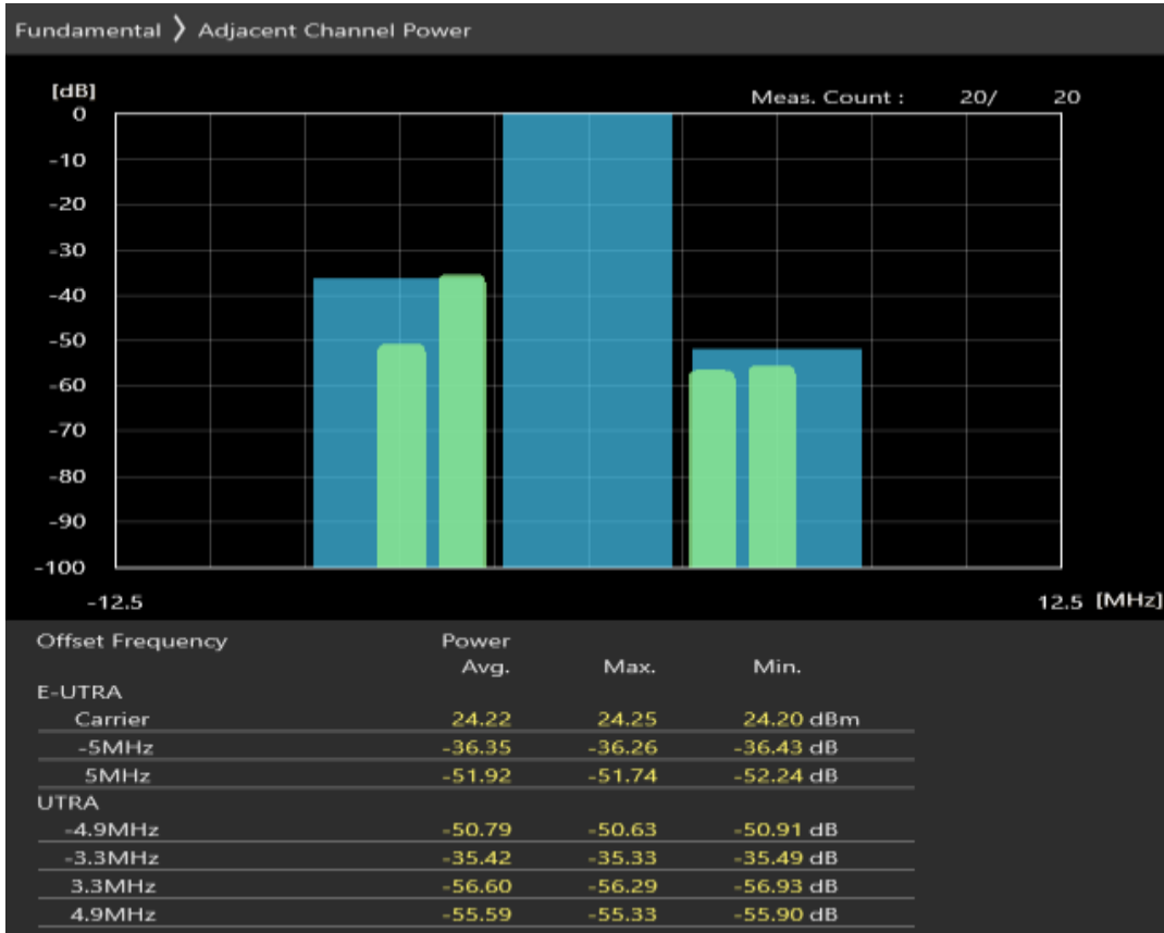
Band40 QAM16 BW=5MHz Channel=39625 RB Size=8 Position=#Max
