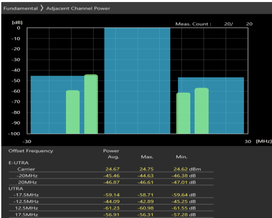
Band1 QPSK BW=20MHz Channel=18500 RB Size=18 Position=#Max
