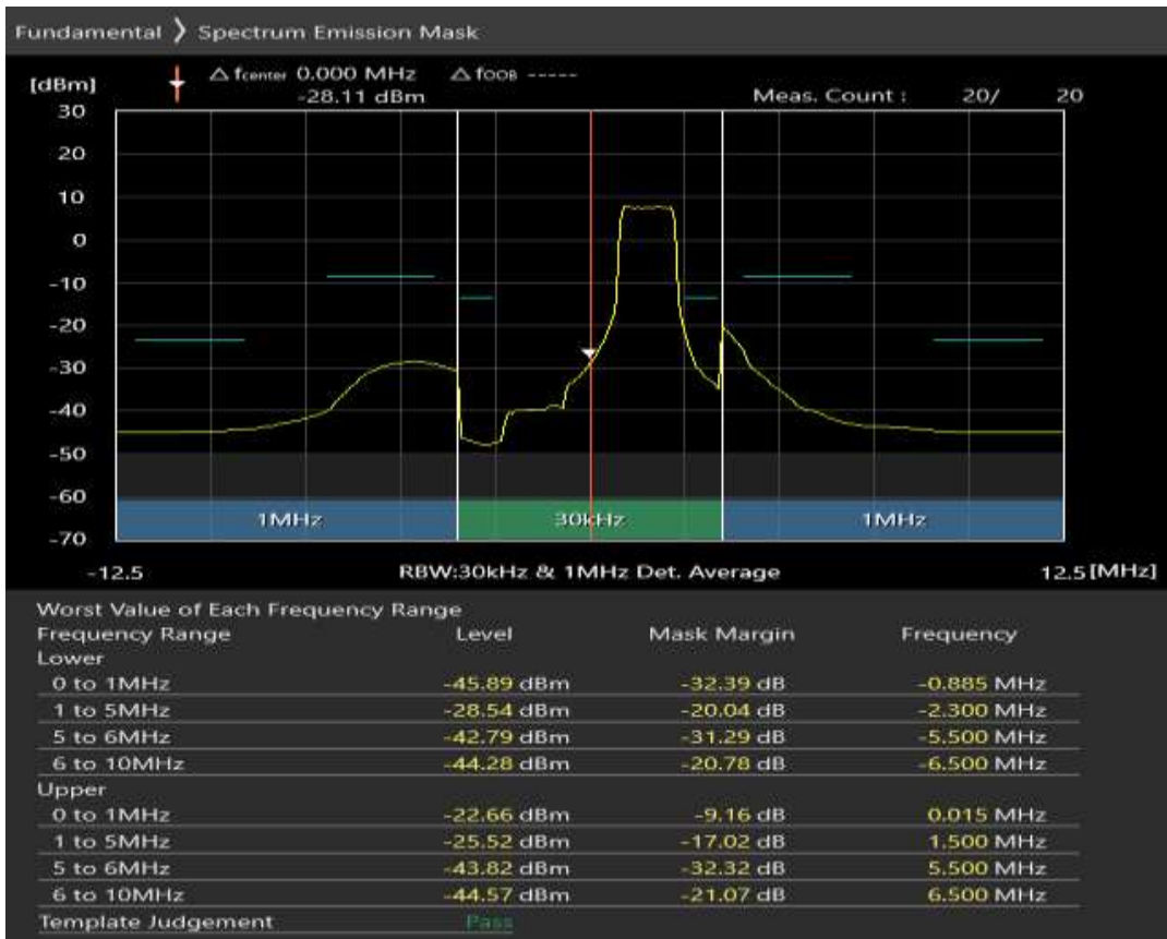
Band8 QPSK BW=5MHz Channel=21775 RB Size=25 Position=#0
