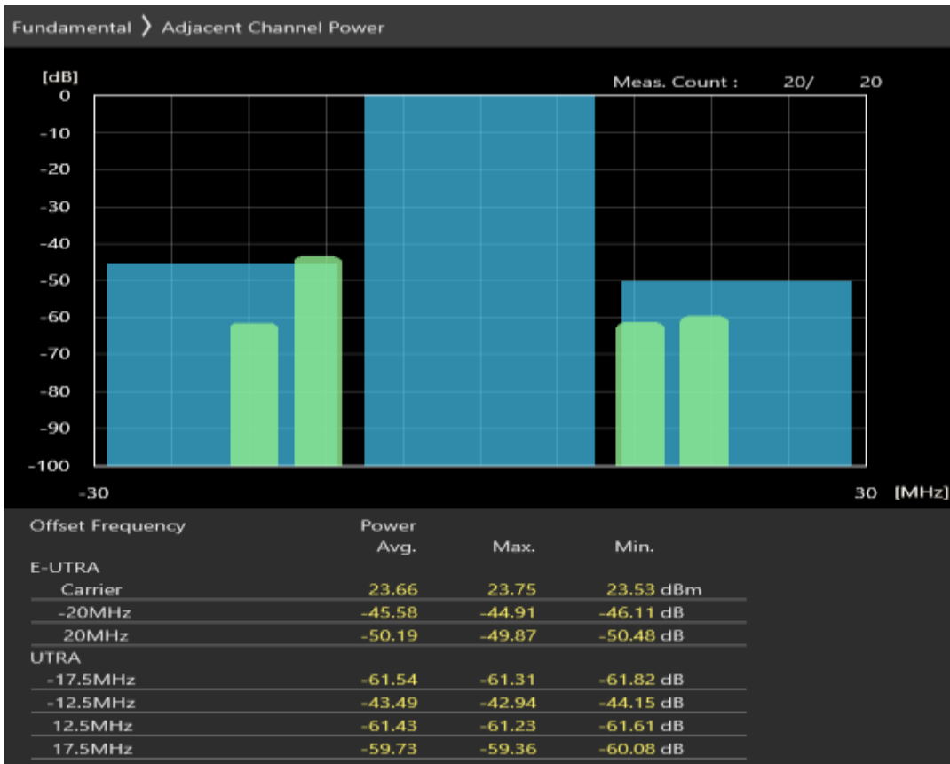
Band7 QAM16 BW=20MHz Channel=21350 RB Size=18 Position=#Max
