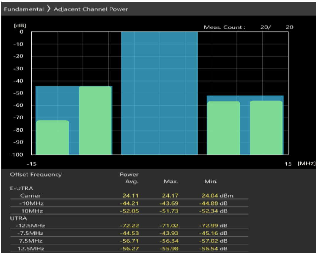
Band8 QPSK BW=10MHz Channel=21500 RB Size=12 Position=#Max
