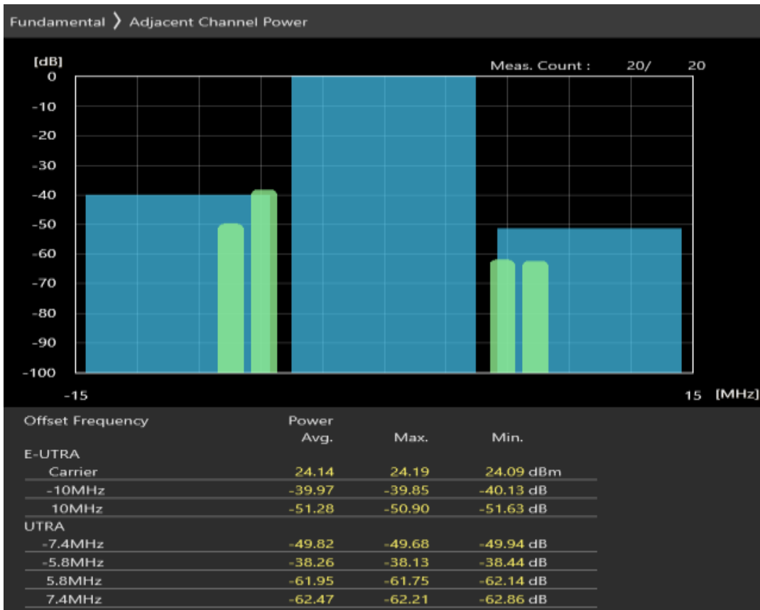
Band40 QAM16 BW=10MHz Channel=39150 RB Size=12 Position=#Max
