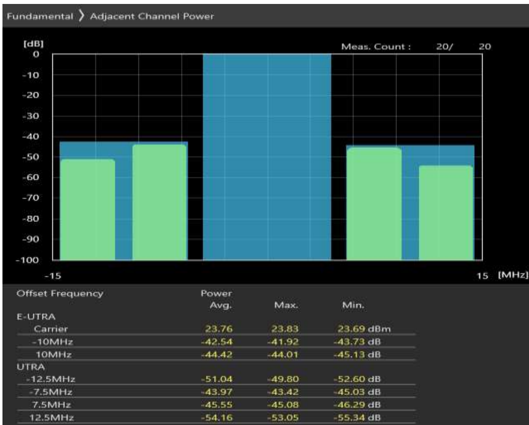
Band3 QAM16 BW=10MHz Channel=1990 RB Size=12 Position=#0
