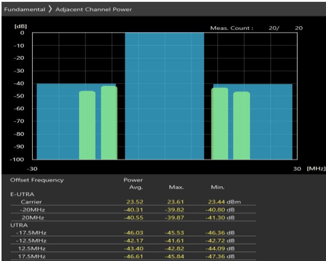
Band3 QAM16 BW=20MHz Channel=19300 RB Size=18 Position=#0
