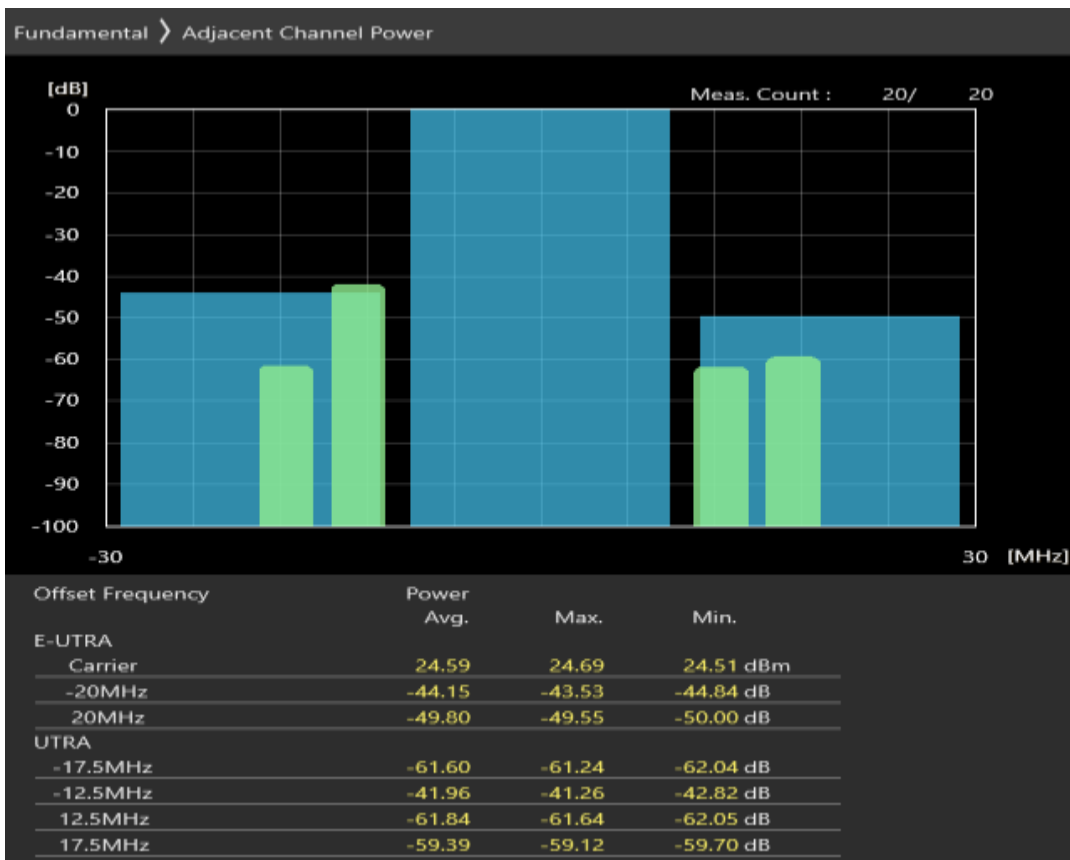
Band7 QPSK BW=20MHz Channel=21100 RB Size=18 Position=#Max
