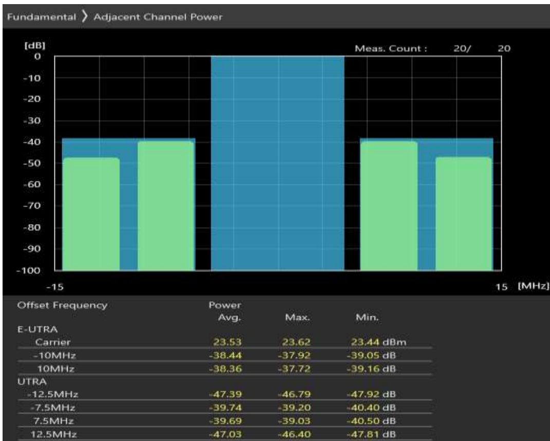
Band3 QAM16 BW=10MHz Channel=19250 RB Size=12 Position=#0
