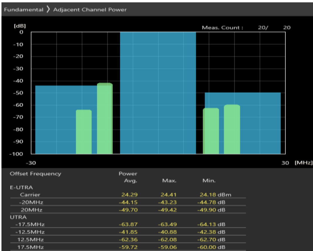
Band3 QPSK BW=20MHz Channel=19300 RB Size=18 Position=#Max
