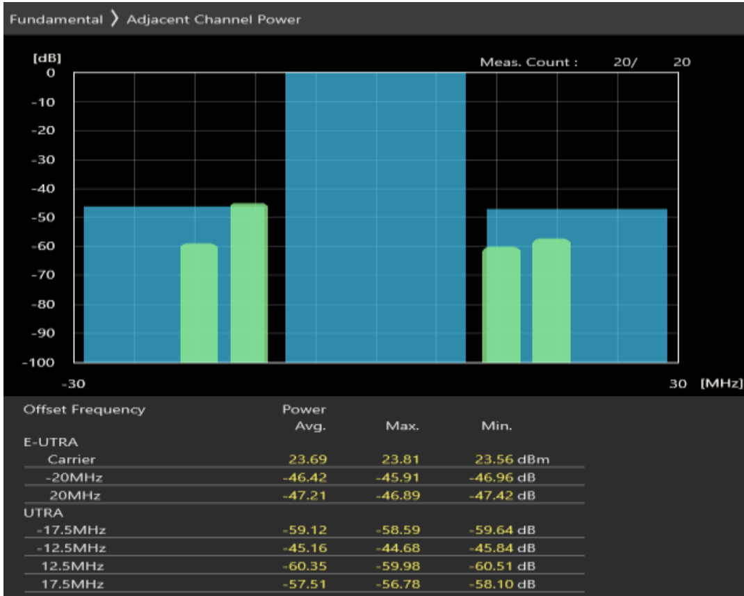
Band1 QAM16 BW=20MHz Channel=18500 RB Size=18 Position=#Max
