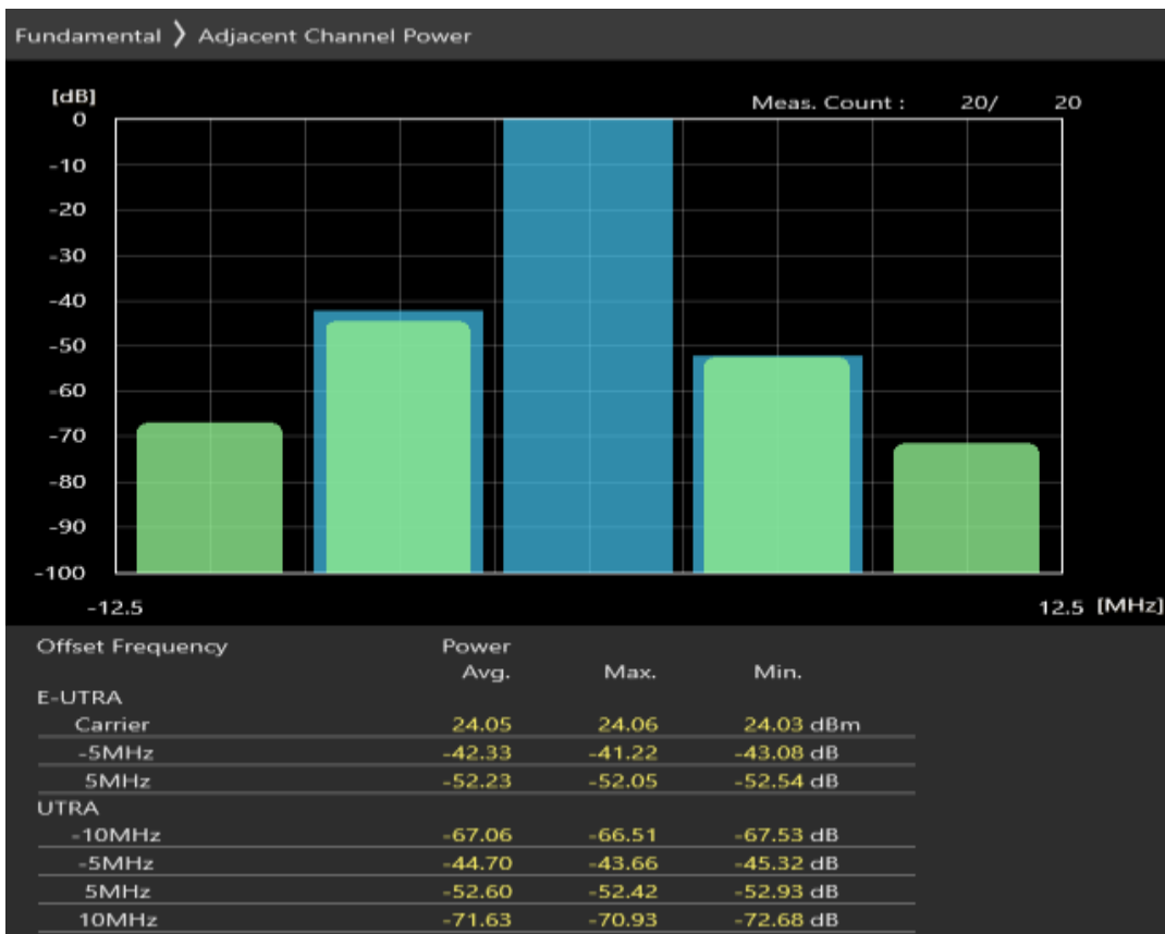
Band8 QPSK BW=5MHz Channel=21475 RB Size=8 Position=#Max
