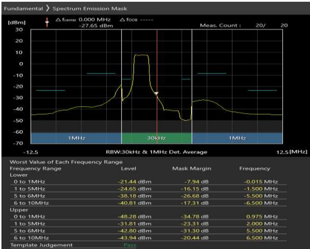
Band8 QPSK BW=5MHz Channel=21625 RB Size=8 Position=#Max
