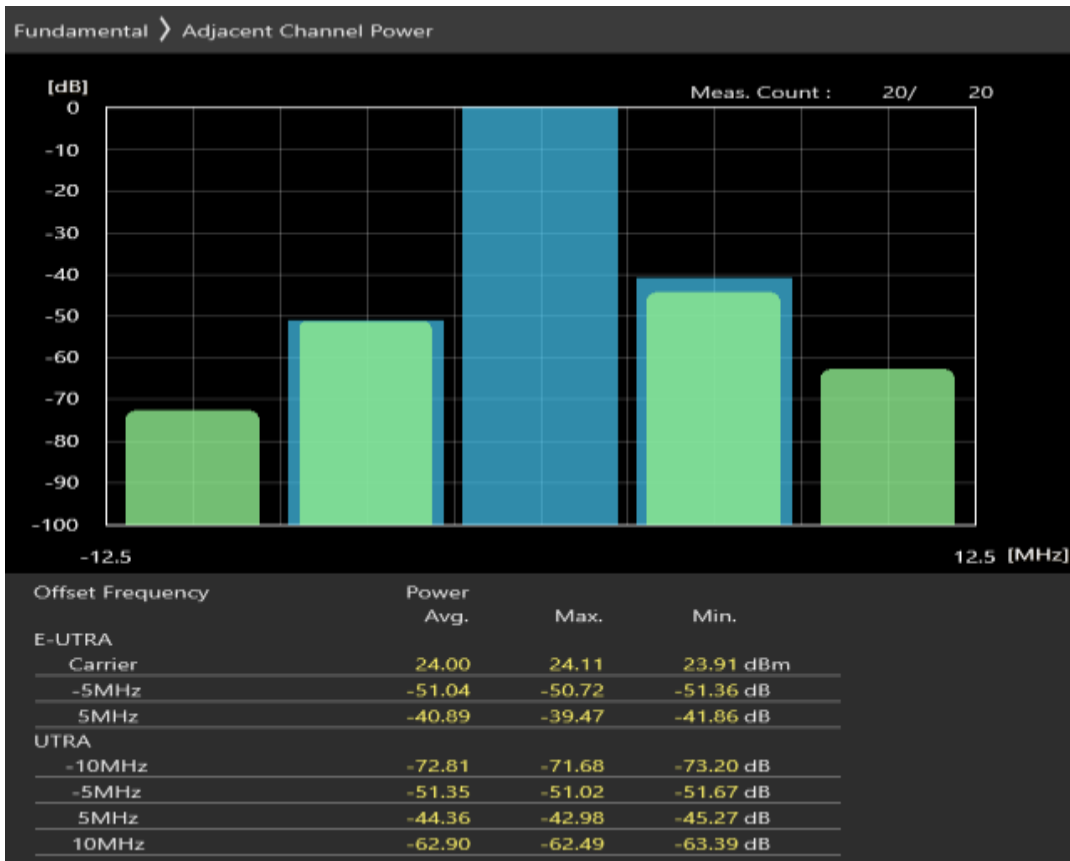
Band20 QPSK BW=5MHz Channel=24300 RB Size=25 Position=#0
