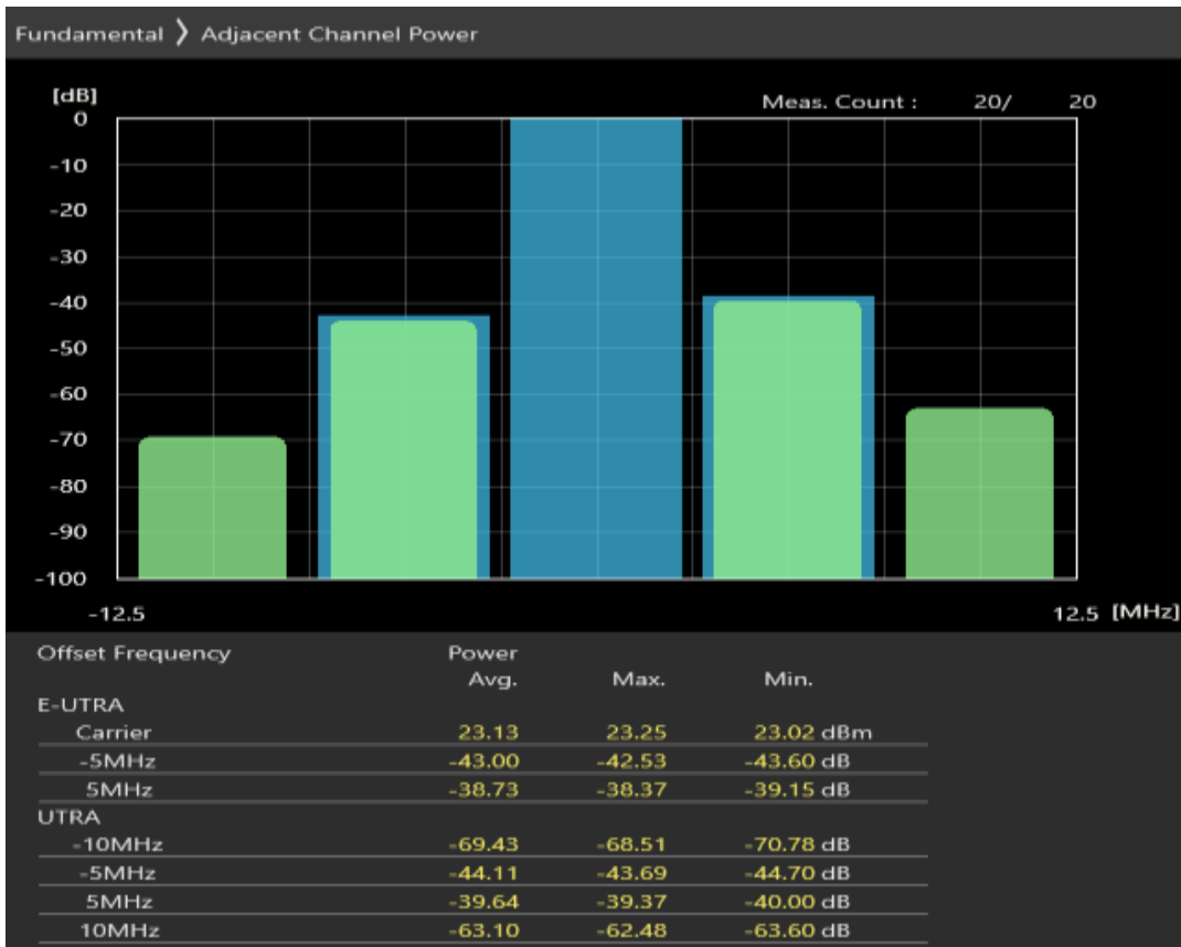
Band20 QAM16 BW=5MHz Channel=24175 RB Size=8 Position=#0
