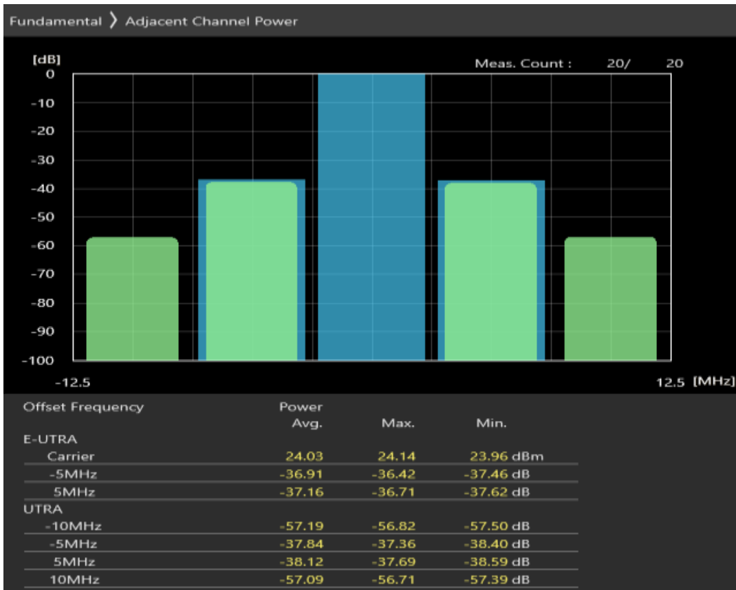
Band7 QAM16 BW=5MHz Channel=21425 RB Size=8 Position=#0
