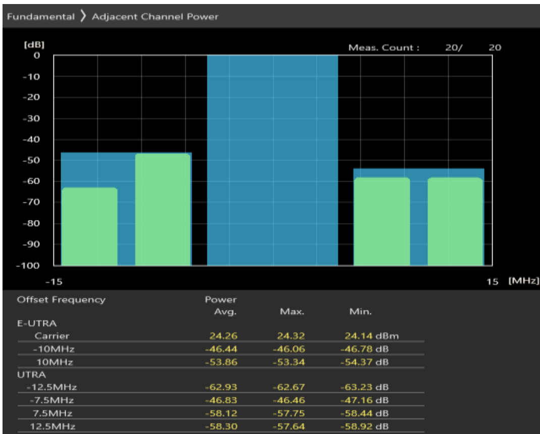
Band20 QPSK BW=10MHz Channel=24300 RB Size=12 Position=#Max
