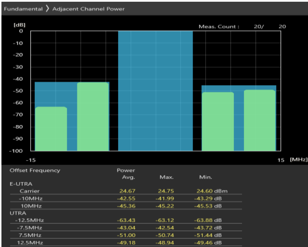
Band1 QPSK BW=10MHz Channel=18050 RB Size=12 Position=#Max
