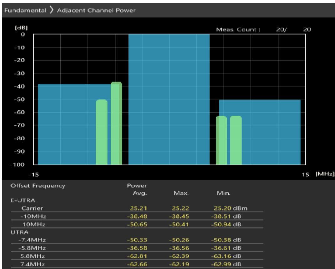
Band40 QPSK BW=10MHz Channel=39150 RB Size=12 Position=#Max
