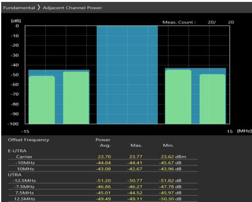
Band1 QAM16 BW=10MHz Channel=18550 RB Size=12 Position=#0
