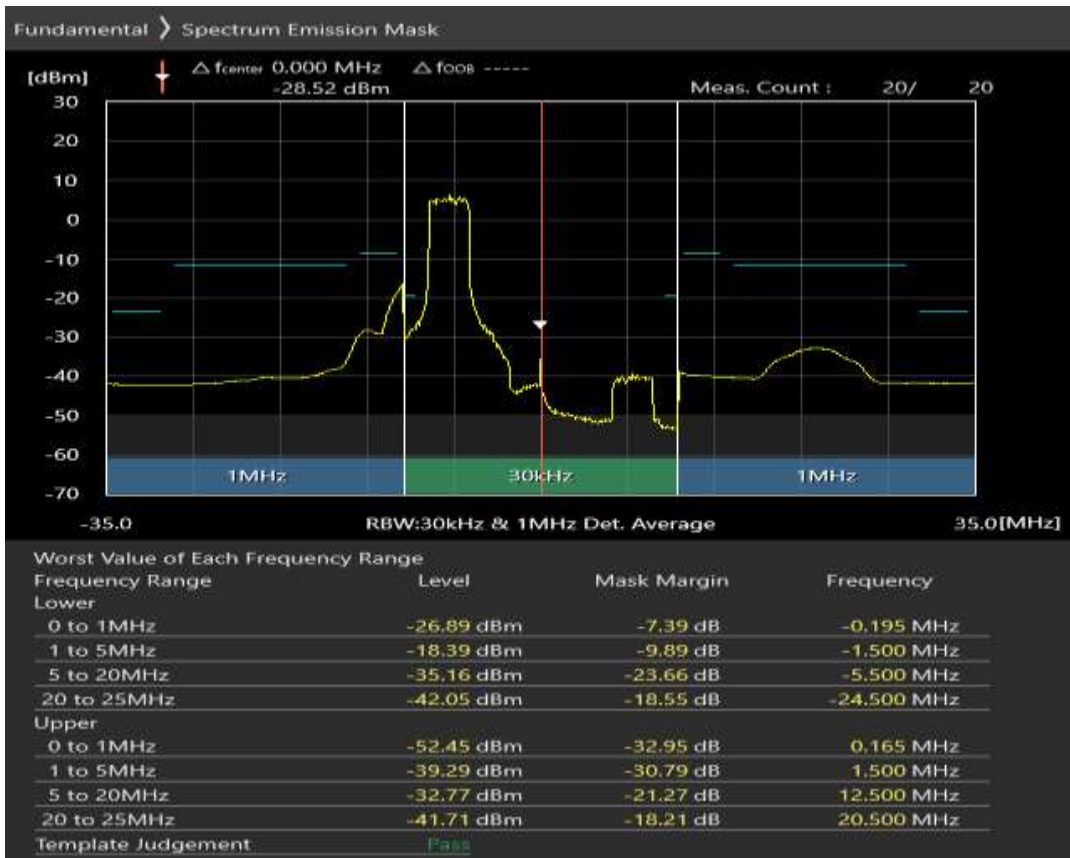
Band40 QPSK BW=20MHz Channel=39150 RB Size=18 Position=#Max
