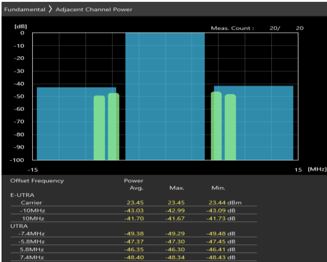
Band40 QAM16 BW=10MHz Channel=38700 RB Size=12 Position=#0
