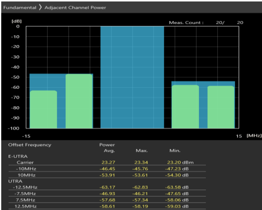
Band20 QAM16 BW=10MHz Channel=24300 RB Size=12 Position=#Max
