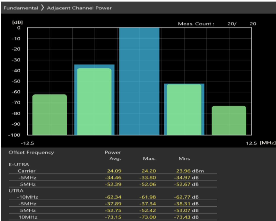
Band8 QPSK BW=5MHz Channel=21775 RB Size=8 Position=#Max
