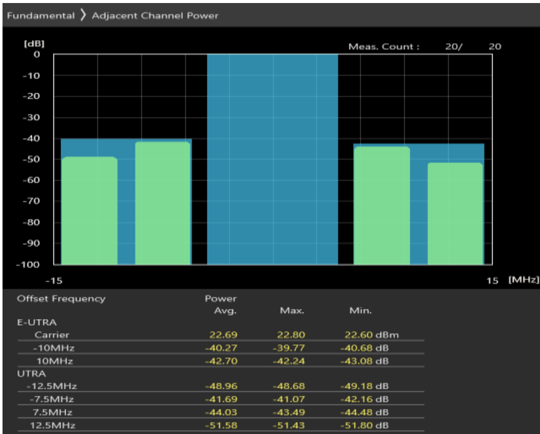
Band1 QPSK BW=10MHz Channel=18550 RB Size=12 Position=#0
