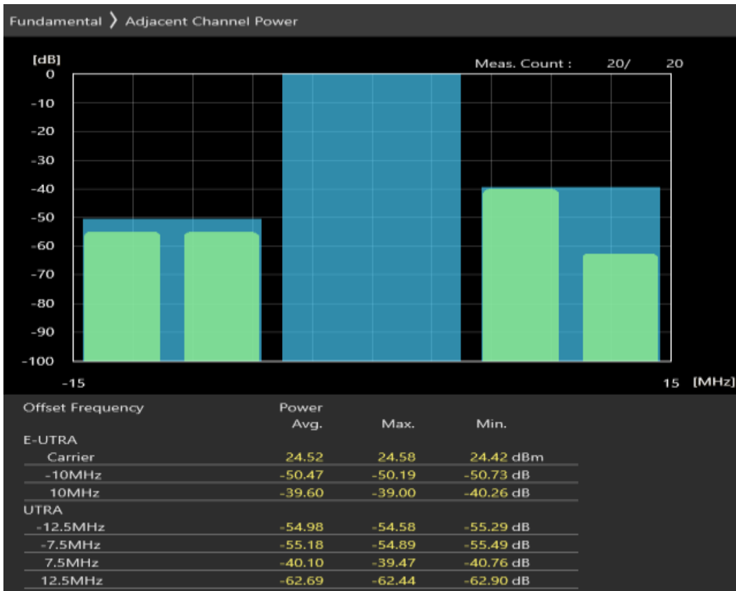
Band3 QPSK BW=10MHz Channel=19250 RB Size=50 Position=#0
