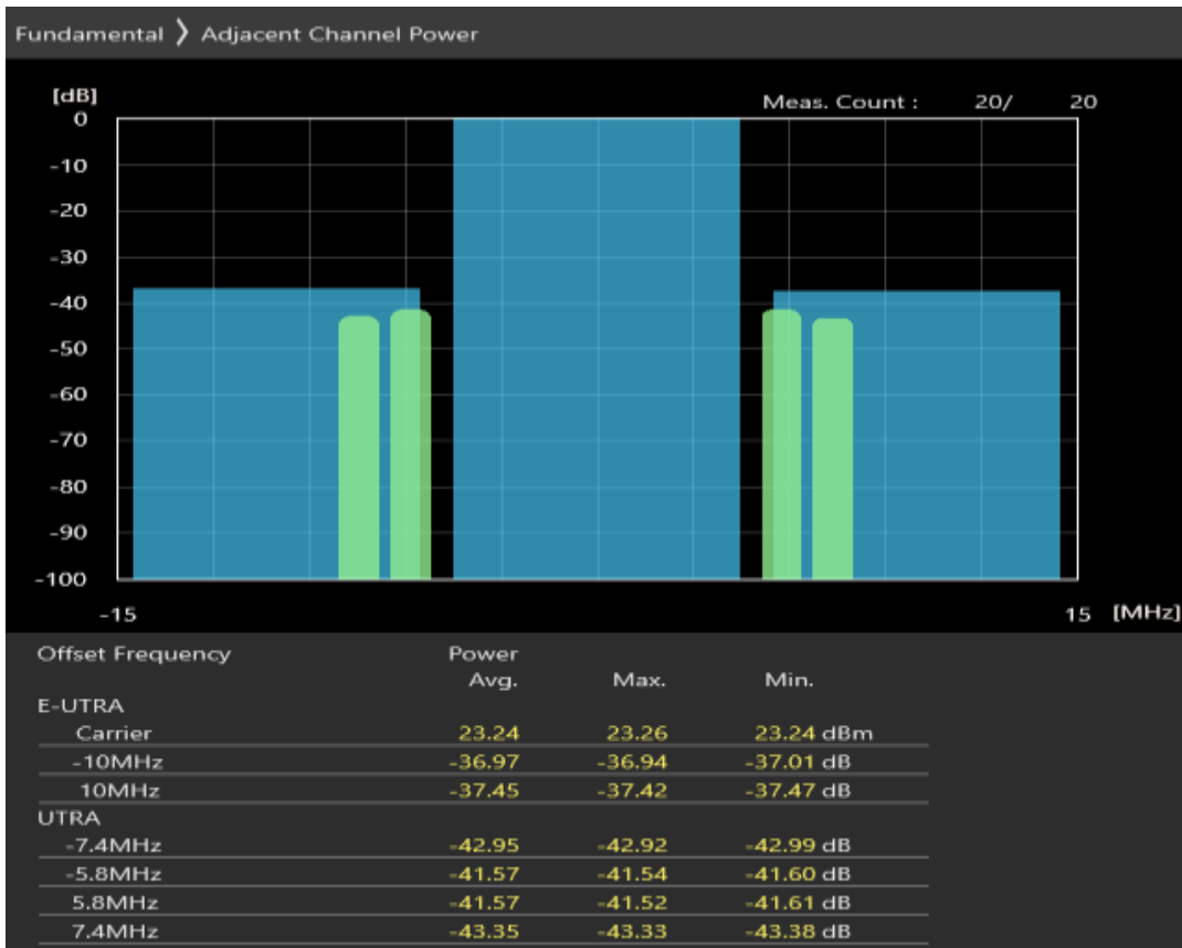
Band40 QPSK BW=20MHz Channel=38750 RB Size=18 Position=#0
