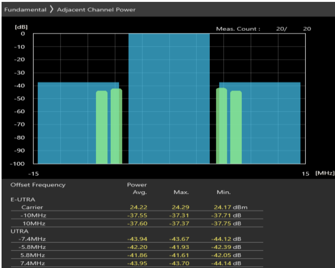
Band40 QAM16 BW=10MHz Channel=39150 RB Size=12 Position=#0
