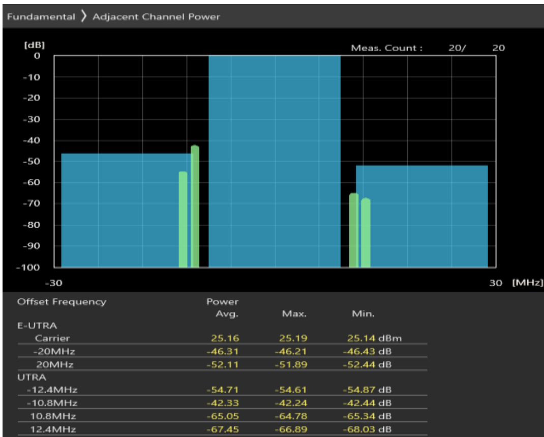
Band40 QPSK BW=20MHz Channel=39550 RB Size=18 Position=#Max
