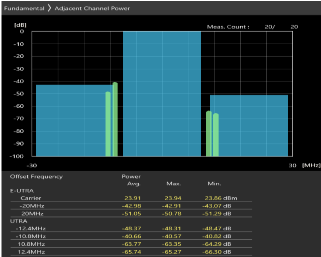
Band40 QAM16 BW=20MHz Channel=39150 RB Size=18 Position=#Max
