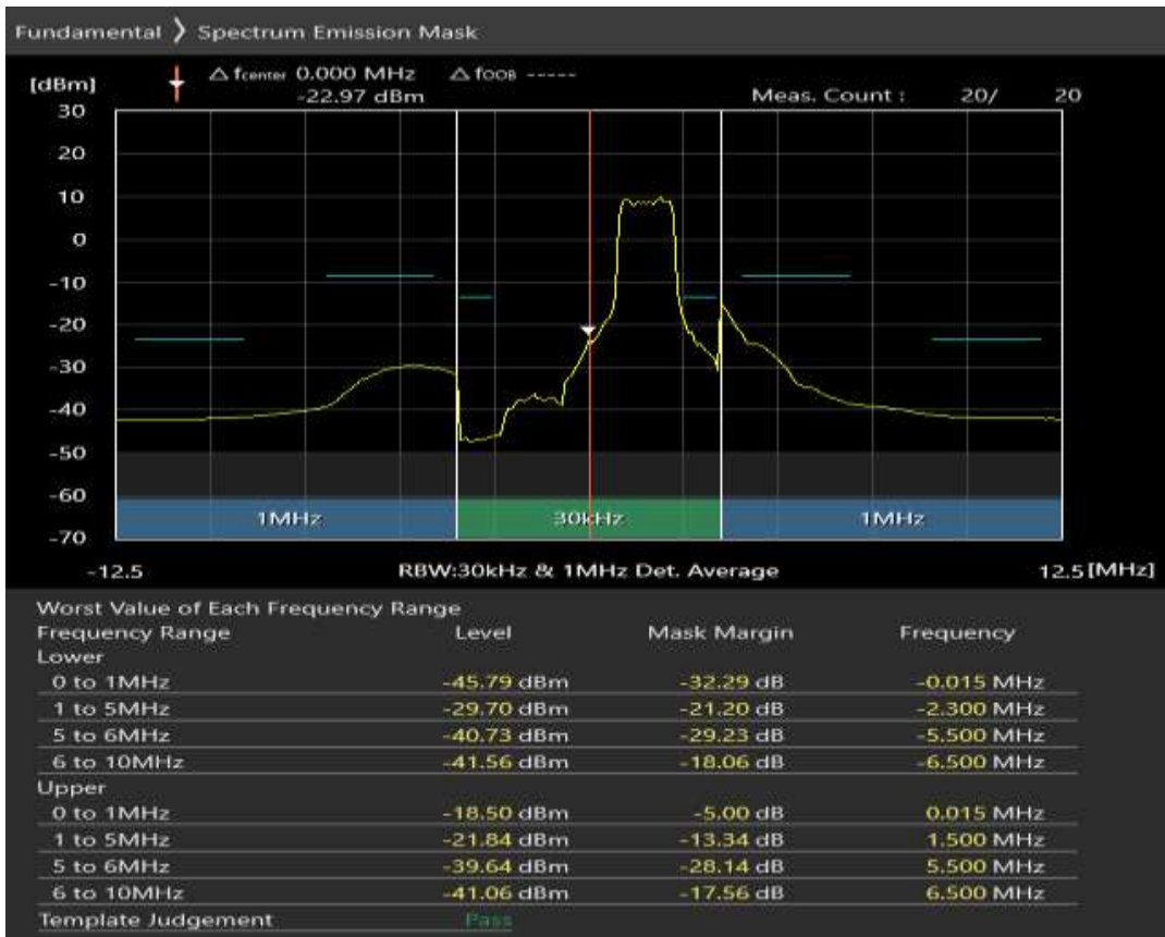
Band40 QPSK BW=5MHz Channel=39150 RB Size=25 Position=#0
