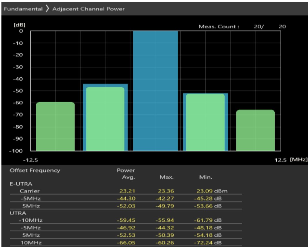
Band20 QAM16 BW=5MHz Channel=24300 RB Size=8 Position=#Max
