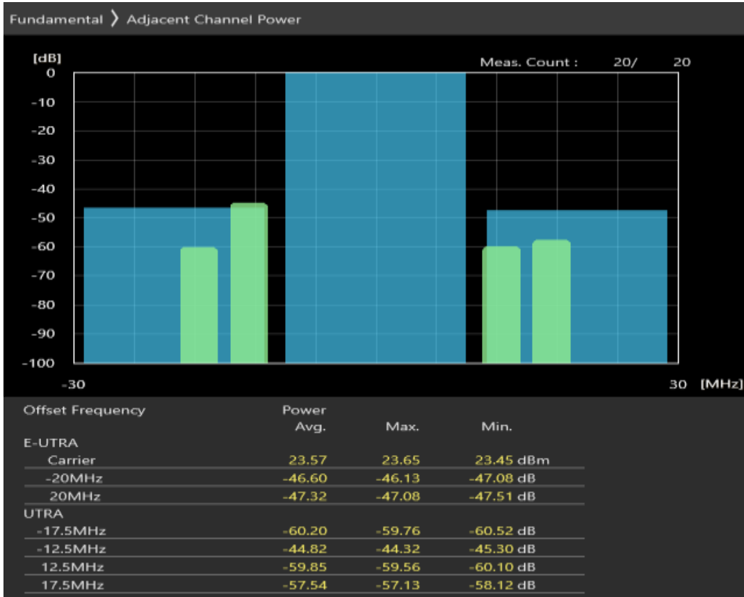
Band1 QAM16 BW=20MHz Channel=18100 RB Size=18 Position=#Max
