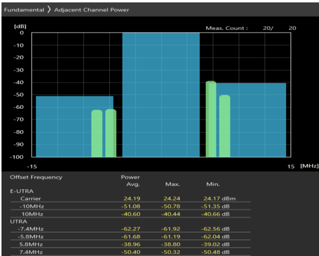
Band40 QAM16 BW=10MHz Channel=39150 RB Size=50 Position=#0
