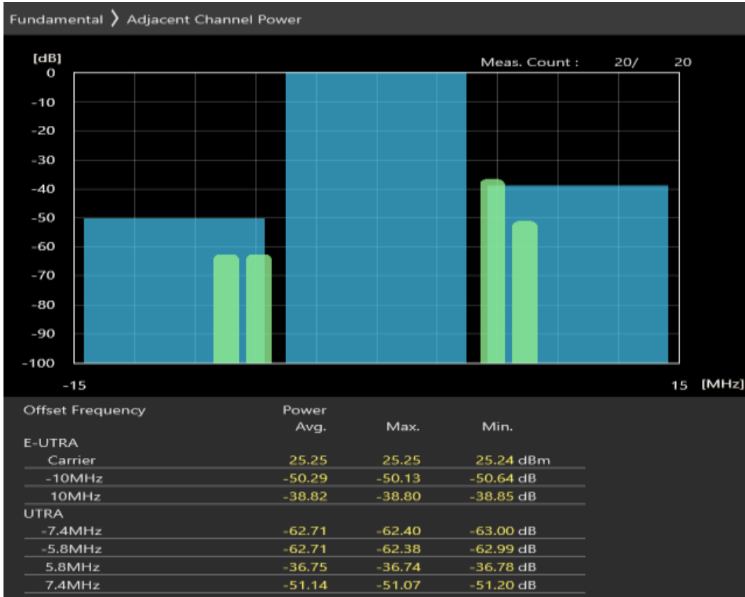
Band40 QPSK BW=10MHz Channel=39150 RB Size=50 Position=#0
