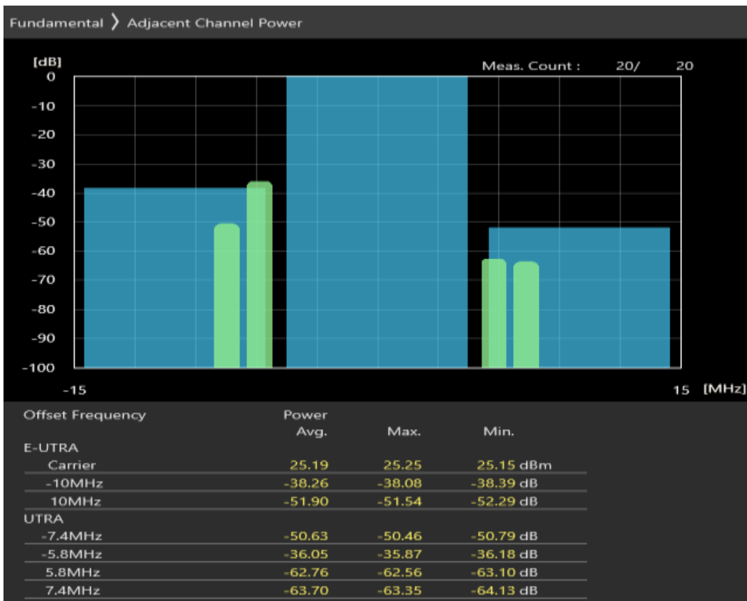
Band40 QPSK BW=10MHz Channel=39600 RB Size=12 Position=#Max
