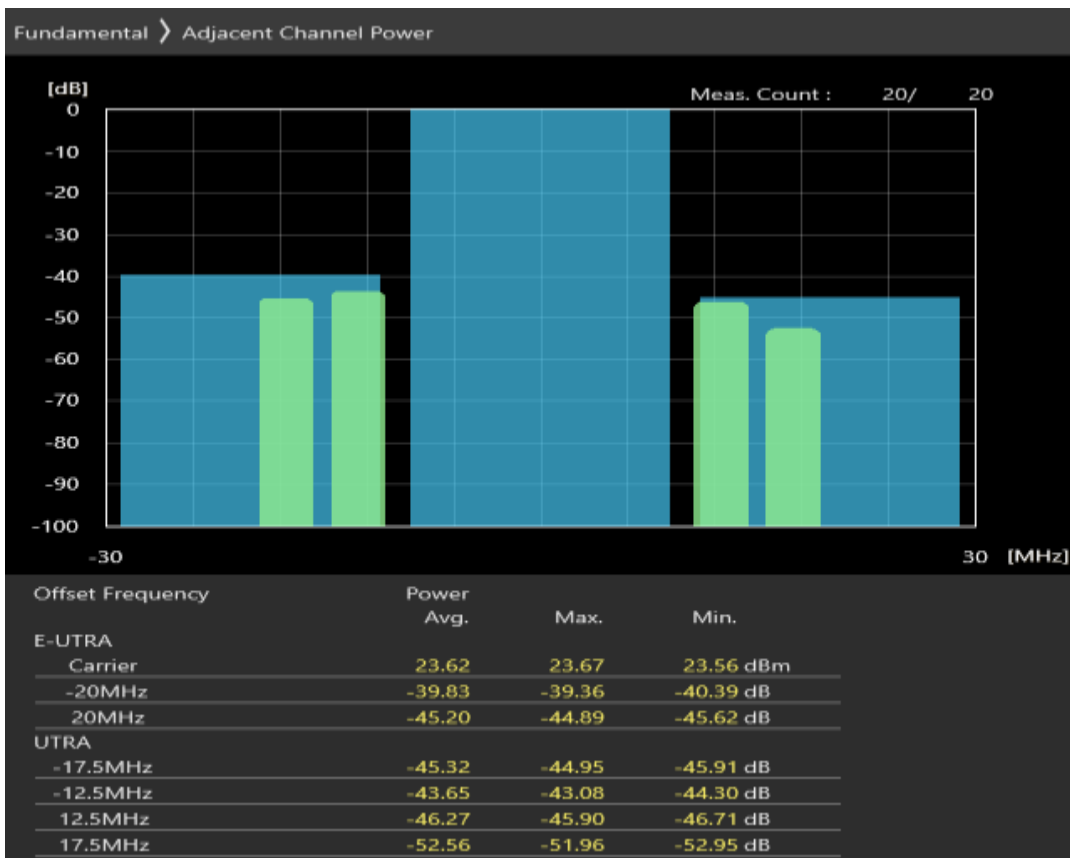
Band3 QAM16 BW=20MHz Channel=19850 RB Size=18 Position=#0
