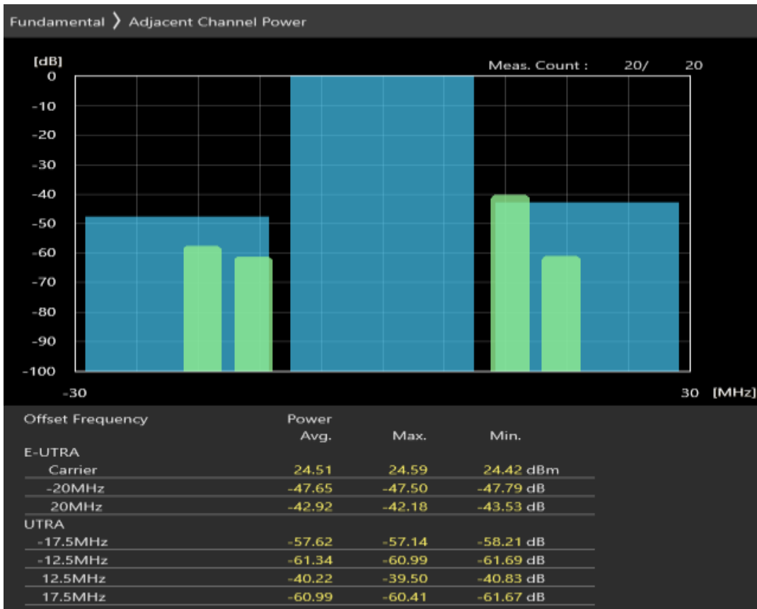
Band3 QPSK BW=20MHz Channel=19575 RB Size=100 Position=#0
