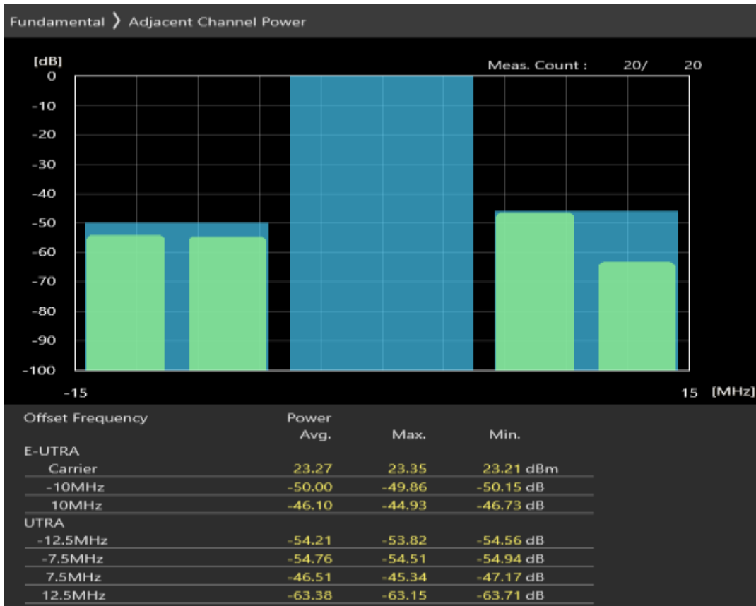
Band8 QAM16 BW=10MHz Channel=21625 RB Size=50 Position=#0
