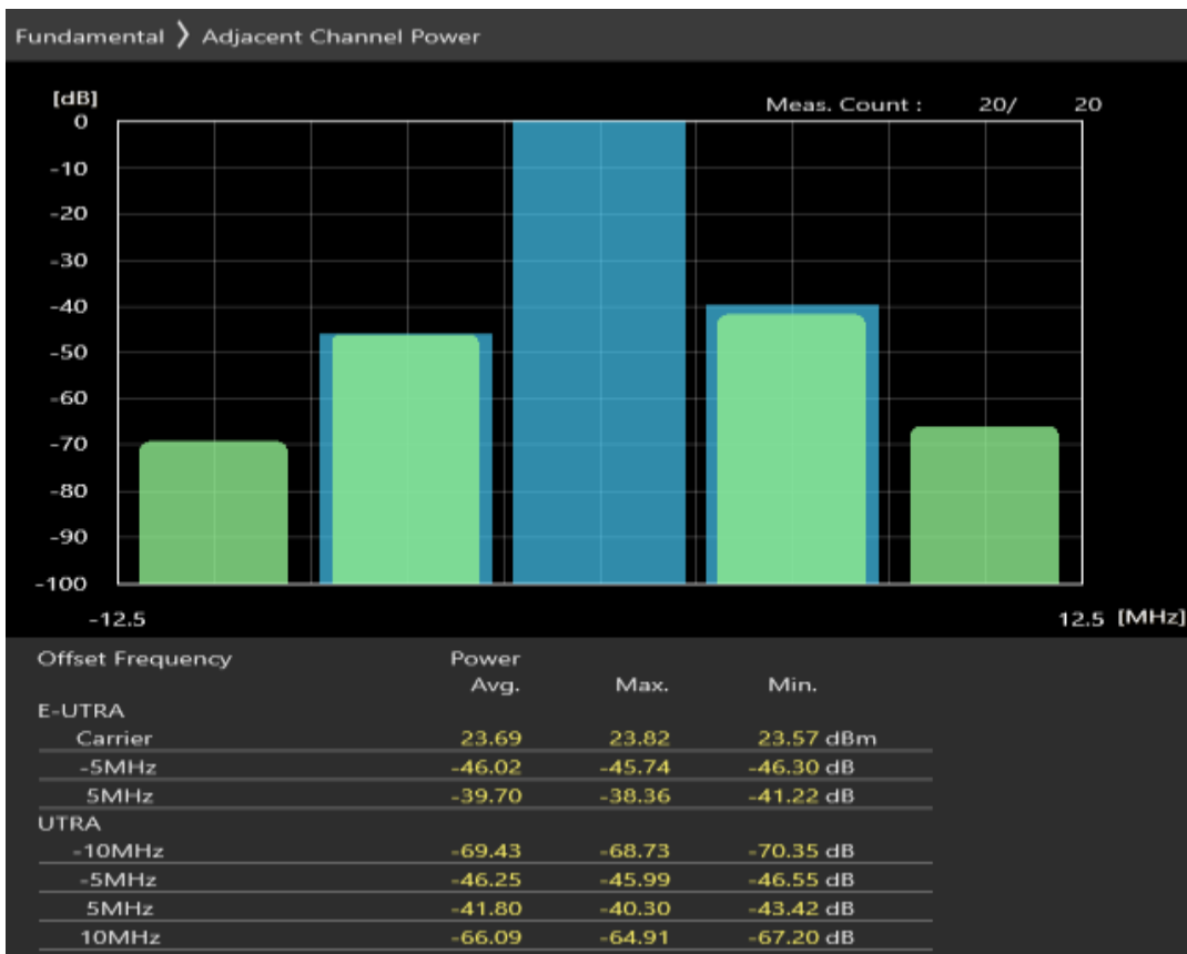
Band3 QAM16 BW=5MHz Channel=19925 RB Size=25 Position=#0
