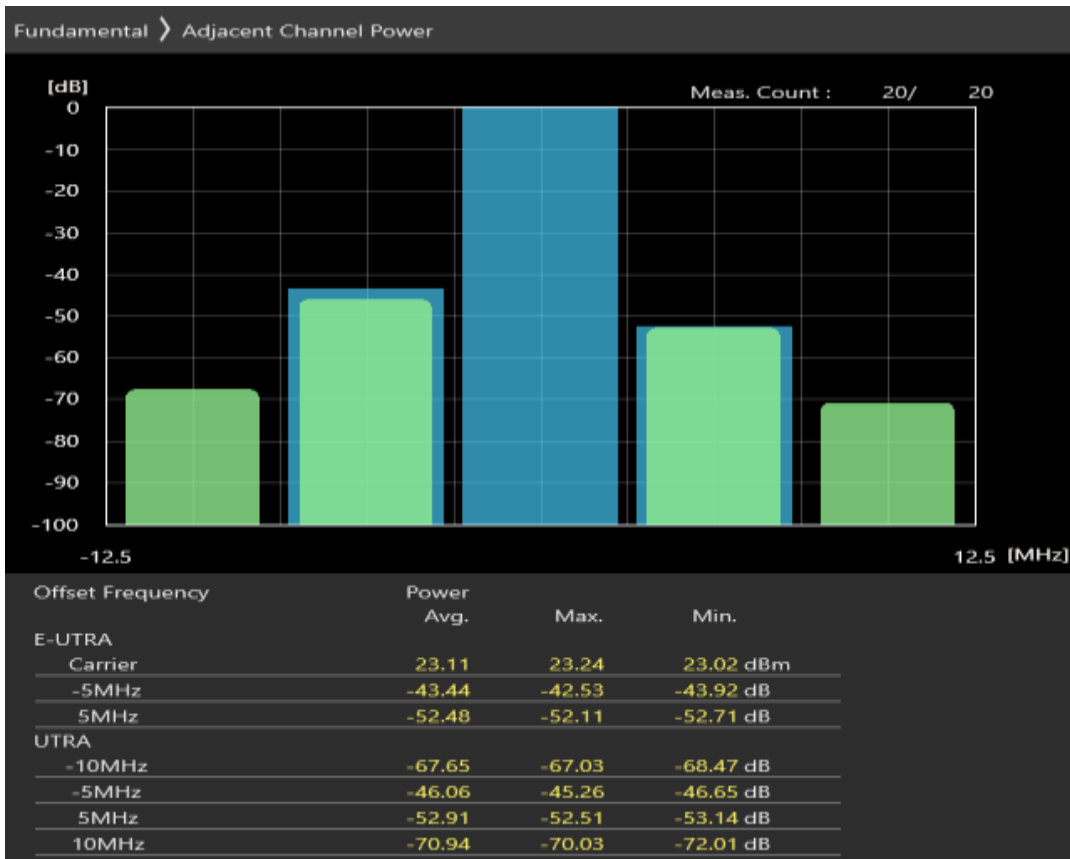
Band8 QAM16 BW=5MHz Channel=21475 RB Size=8 Position=#Max
