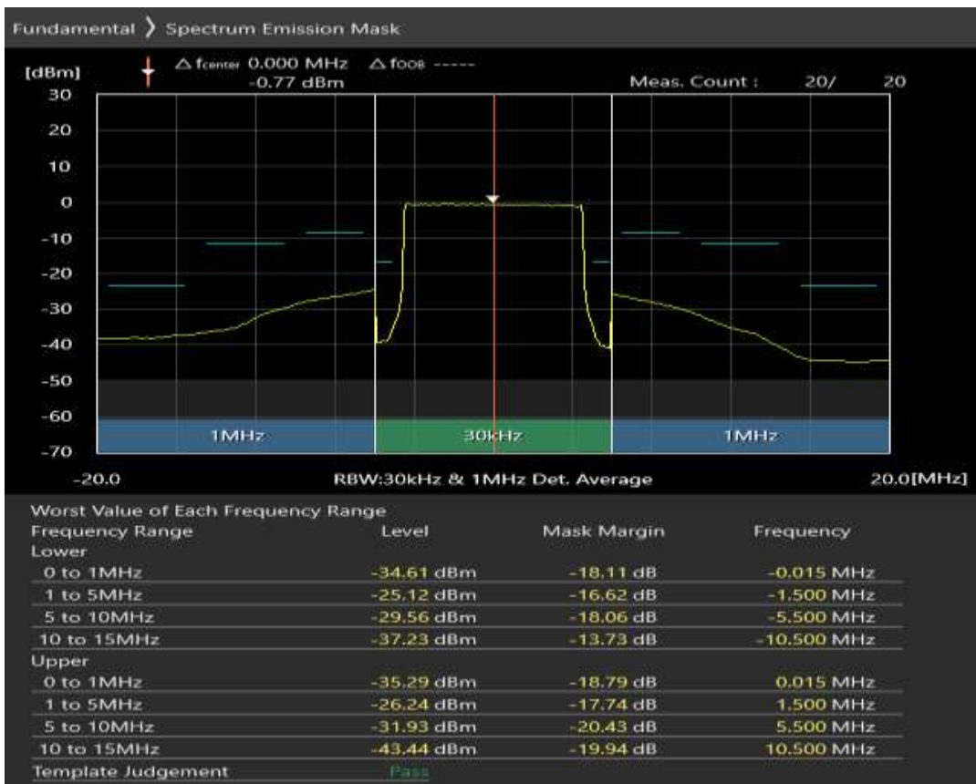
Band3 QAM16 BW=10MHz Channel=1990 RB Size=12 Position=#0
