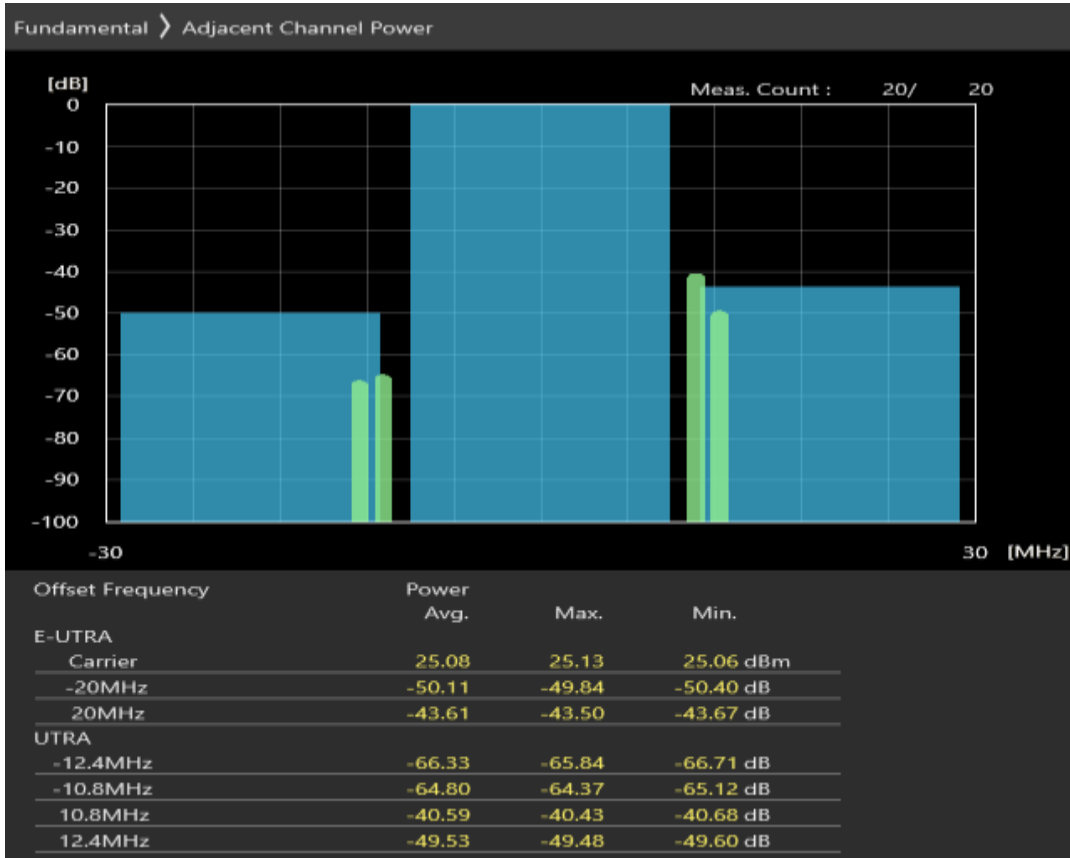
Band40 QPSK BW=20MHz Channel=39150 RB Size=100 Position=#0
