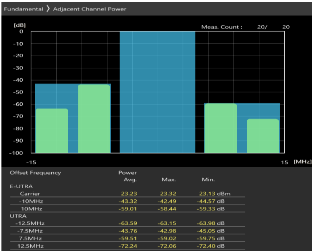
Band8 QAM16 BW=10MHz Channel=21750 RB Size=12 Position=#Max
