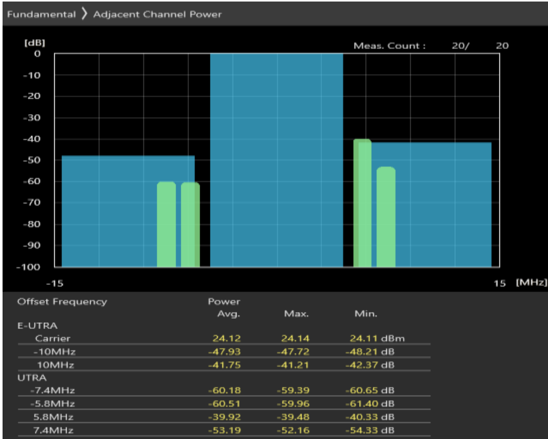
Band40 QPSK BW=10MHz Channel=38700 RB Size=50 Position=#0
