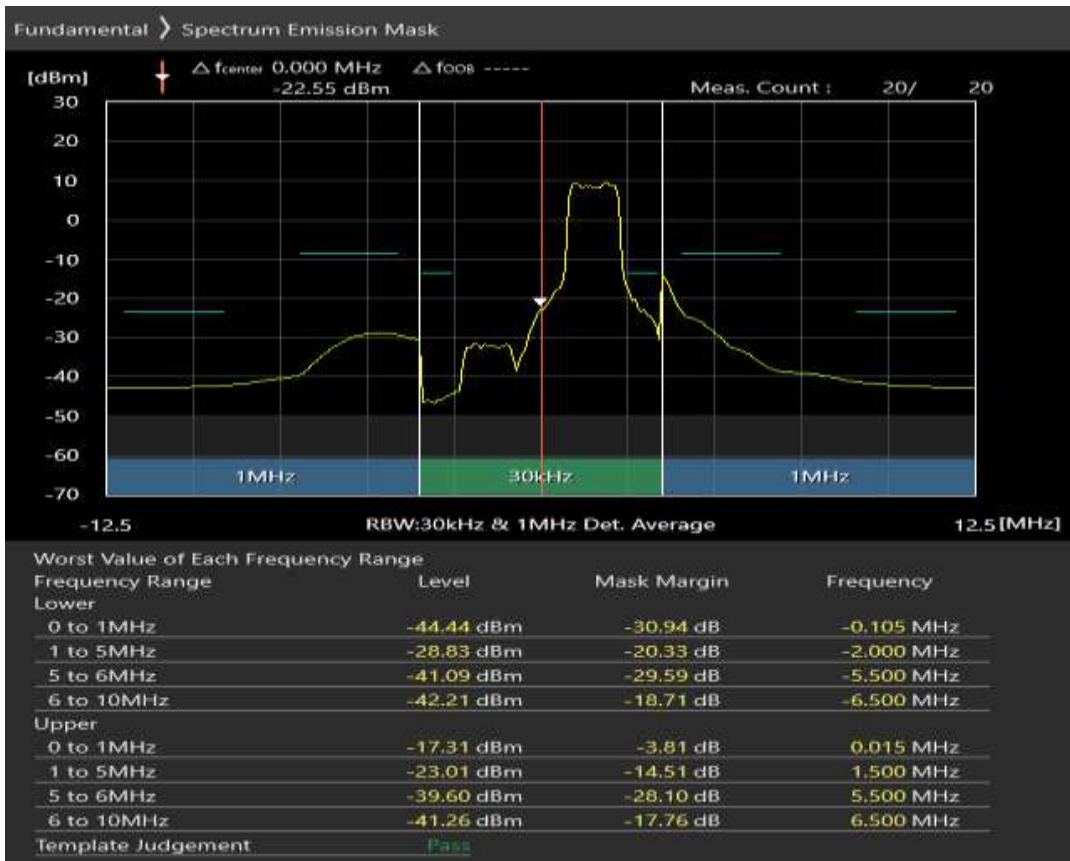
Band40 QPSK BW=5MHz Channel=39625 RB Size=25 Position=#0
