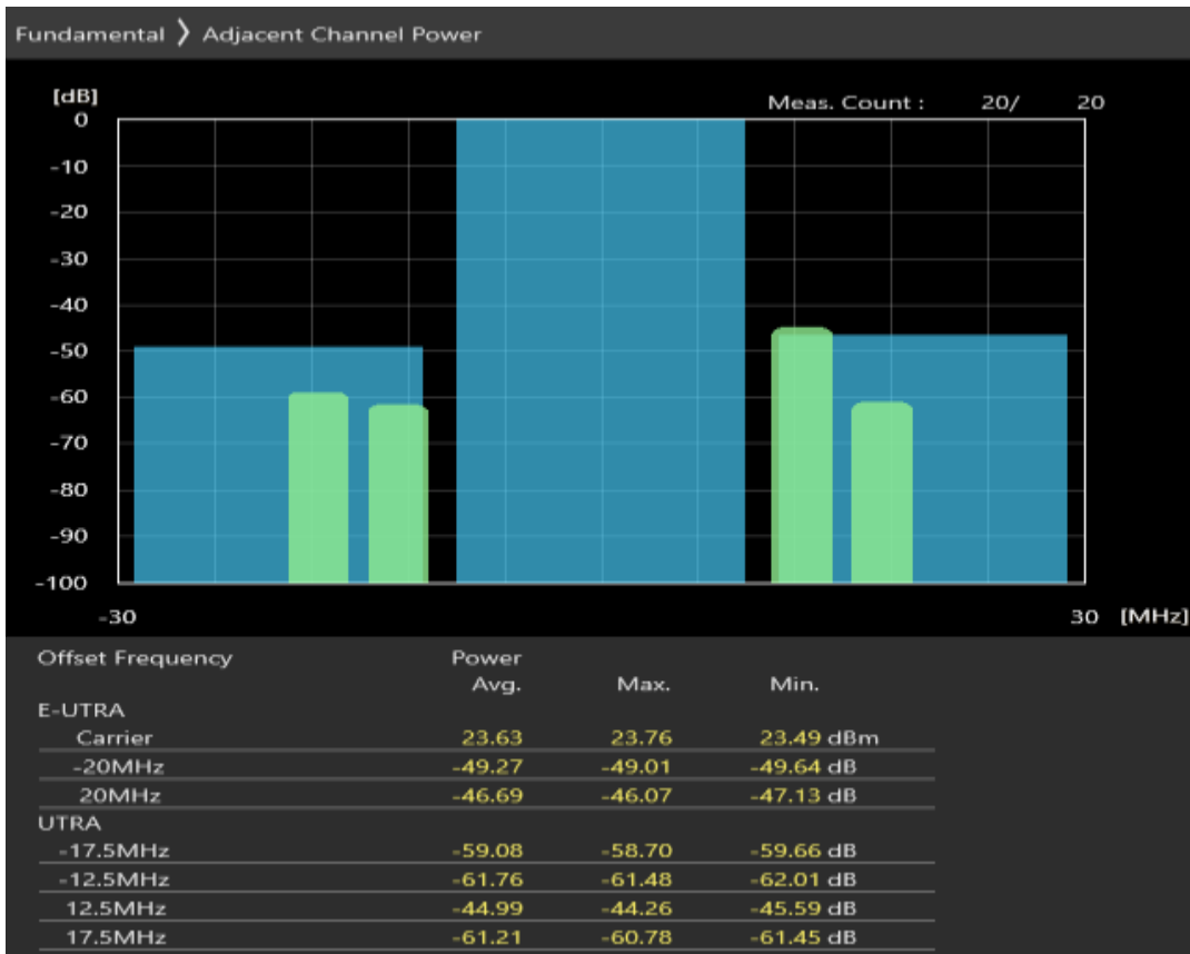
Band1 QAM16 BW=20MHz Channel=18100 RB Size=100 Position=#0
