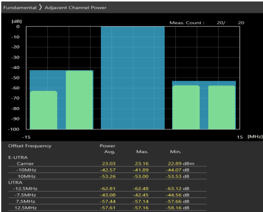
Band20 QAM16 BW=10MHz Channel=24400 RB Size=12 Position=#Max
