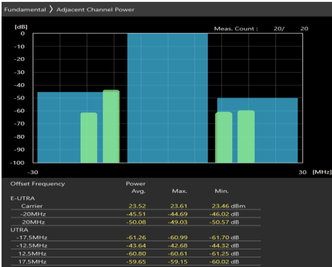
Band7 QAM16 BW=20MHz Channel=21100 RB Size=18 Position=#Max
