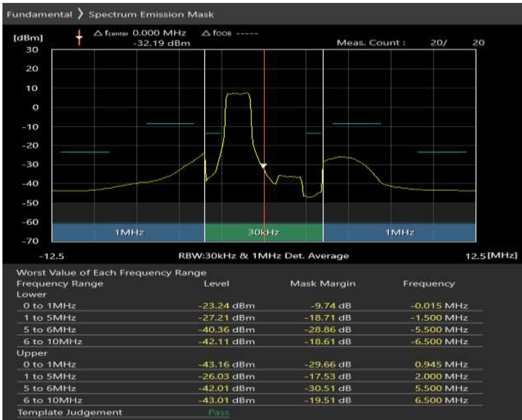
Band1 QAM16 BW=5MHz Channel=18575 RB Size=8 Position=#Max
