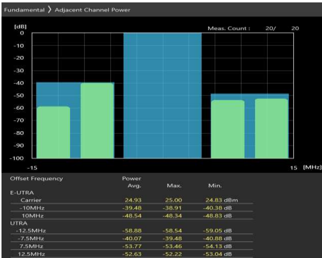
Band7 QPSK BW=10MHz Channel=21400 RB Size=12 Position=#Max
