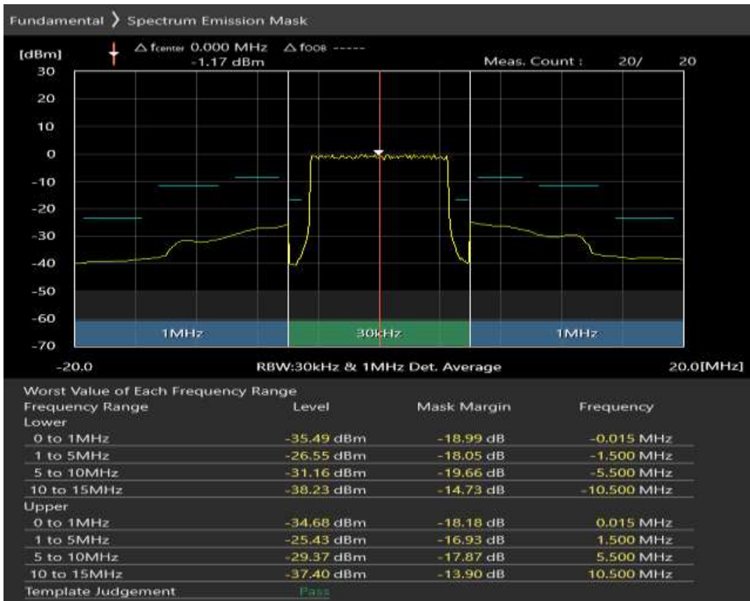
Band40 QAM16 BW=10MHz Channel=38700 RB Size=12 Position=#0
