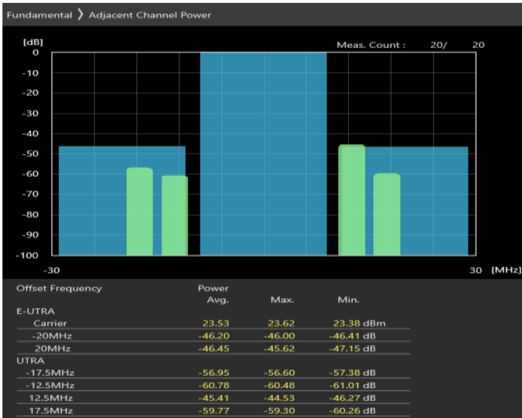
Band1 QAM16 BW=20MHz Channel=18500 RB Size=100 Position=#0
