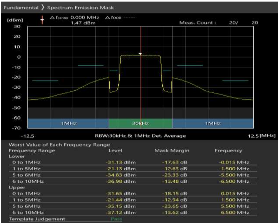
Band7 QPSK BW=10MHz Channel=20800 RB Size=12 Position=#0
