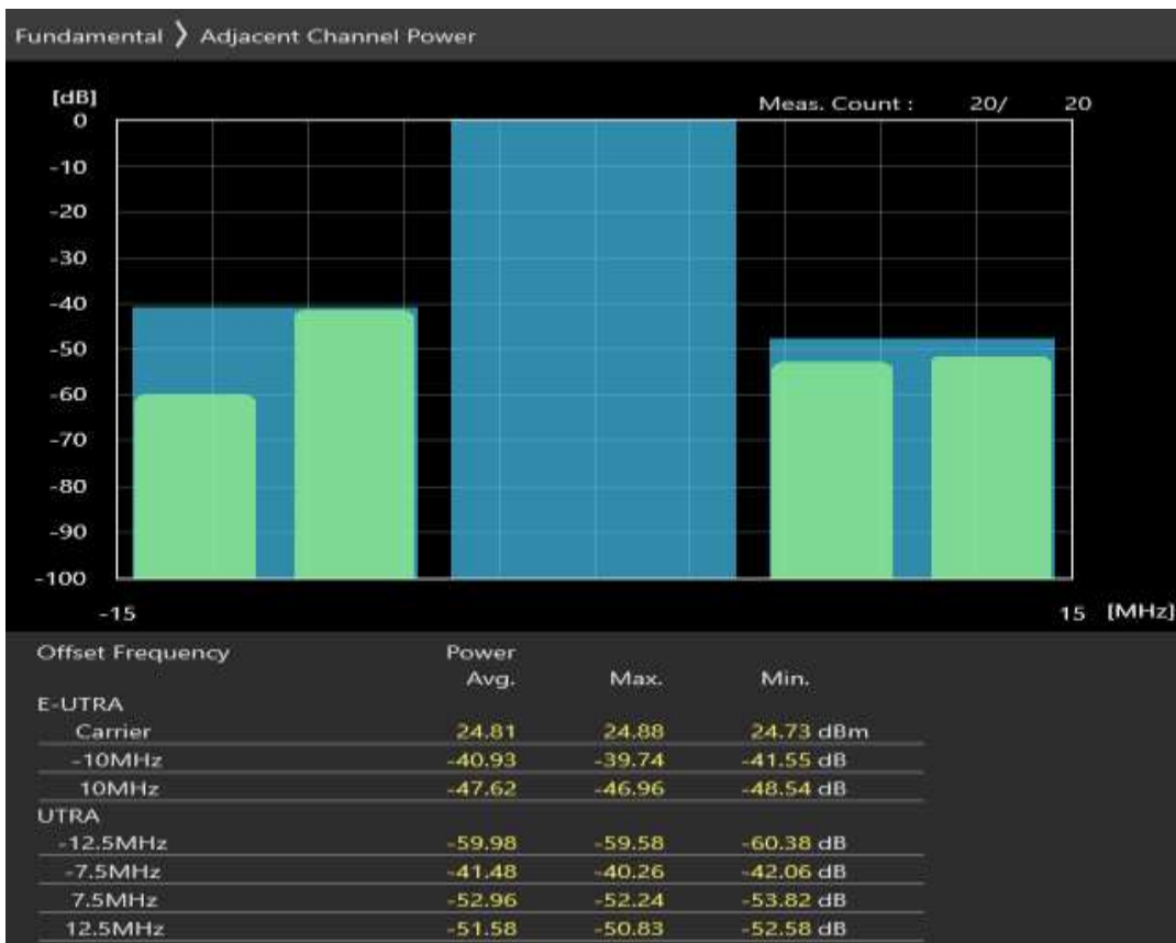
Band7 QPSK BW=10MHz Channel=20800 RB Size=12 Position=#Max
