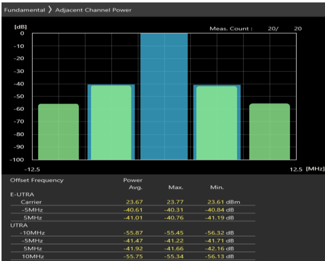
Band1 QAM16 BW=5MHz Channel=18025 RB Size=8 Position=#0
