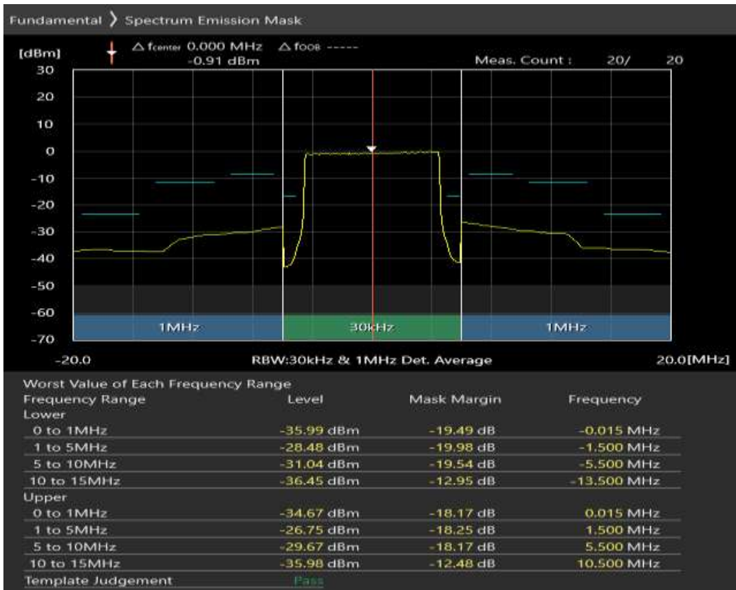
Band1 QAM16 BW=10MHz Channel=18550 RB Size=12 Position=#0
