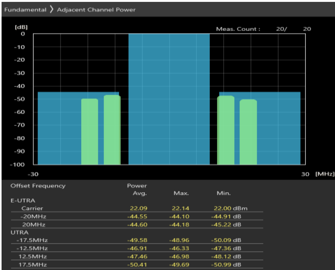
Band20 QPSK BW=20MHz Channel=24350 RB Size=18 Position=#0
