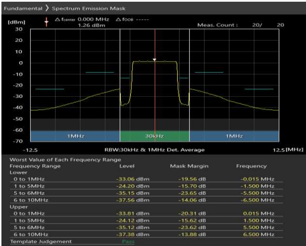
Band7 QPSK BW=5MHz Channel=21425 RB Size=8 Position=#0
