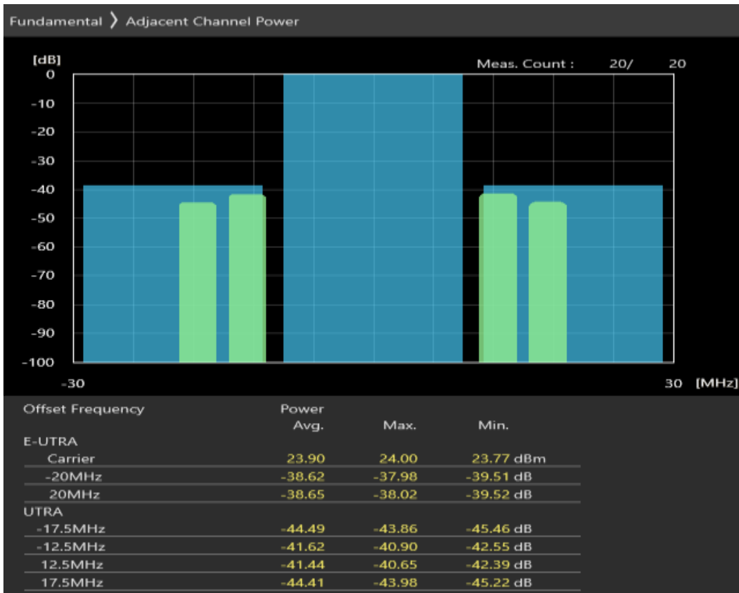
Band7 QAM16 BW=20MHz Channel=21350 RB Size=18 Position=#0
