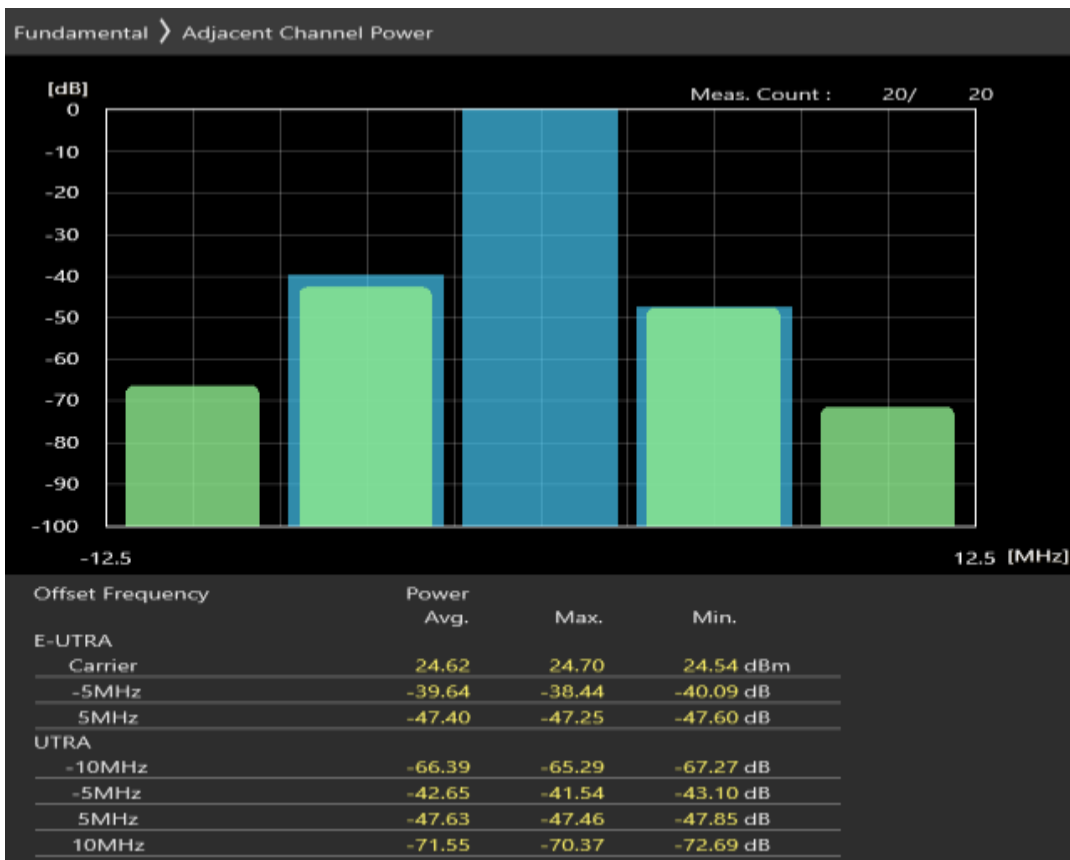
Band1 QPSK BW=5MHz Channel=18300 RB Size=8 Position=#Max
