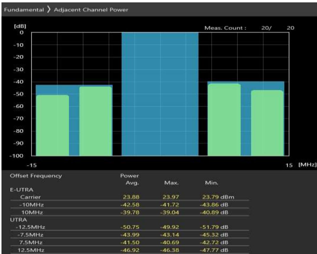
Band7 QAM16 BW=10MHz Channel=20800 RB Size=12 Position=#0
