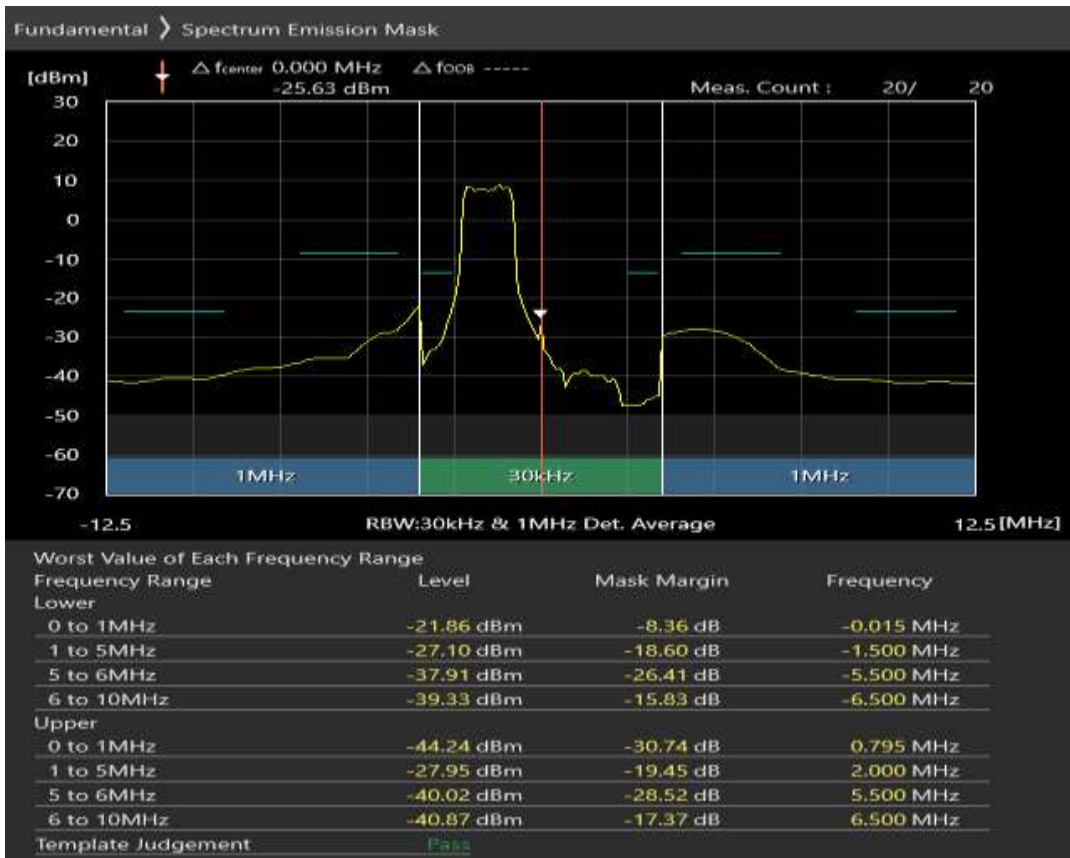
Band40 QPSK BW=5MHz Channel=38675 RB Size=8 Position=#Max
