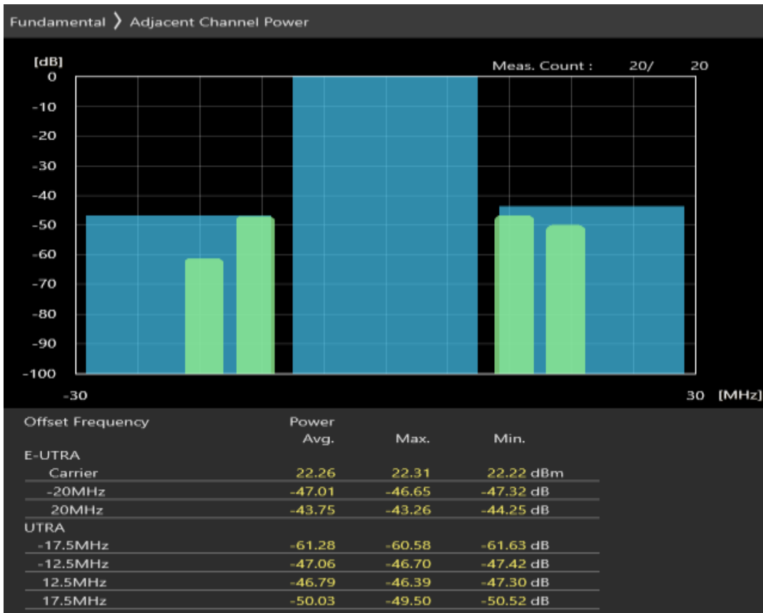
Band20 QPSK BW=20MHz Channel=24300 RB Size=18 Position=#0
