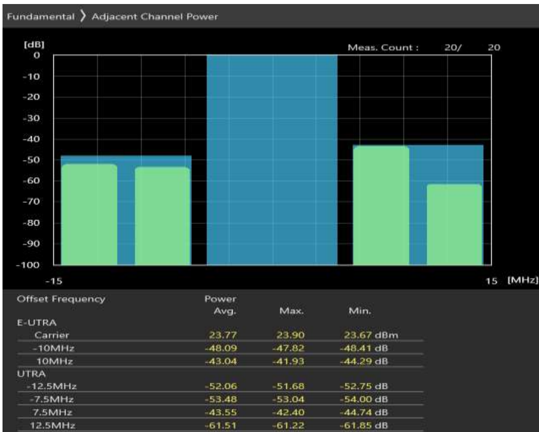
Band7 QAM16 BW=10MHz Channel=21100 RB Size=50 Position=#0
