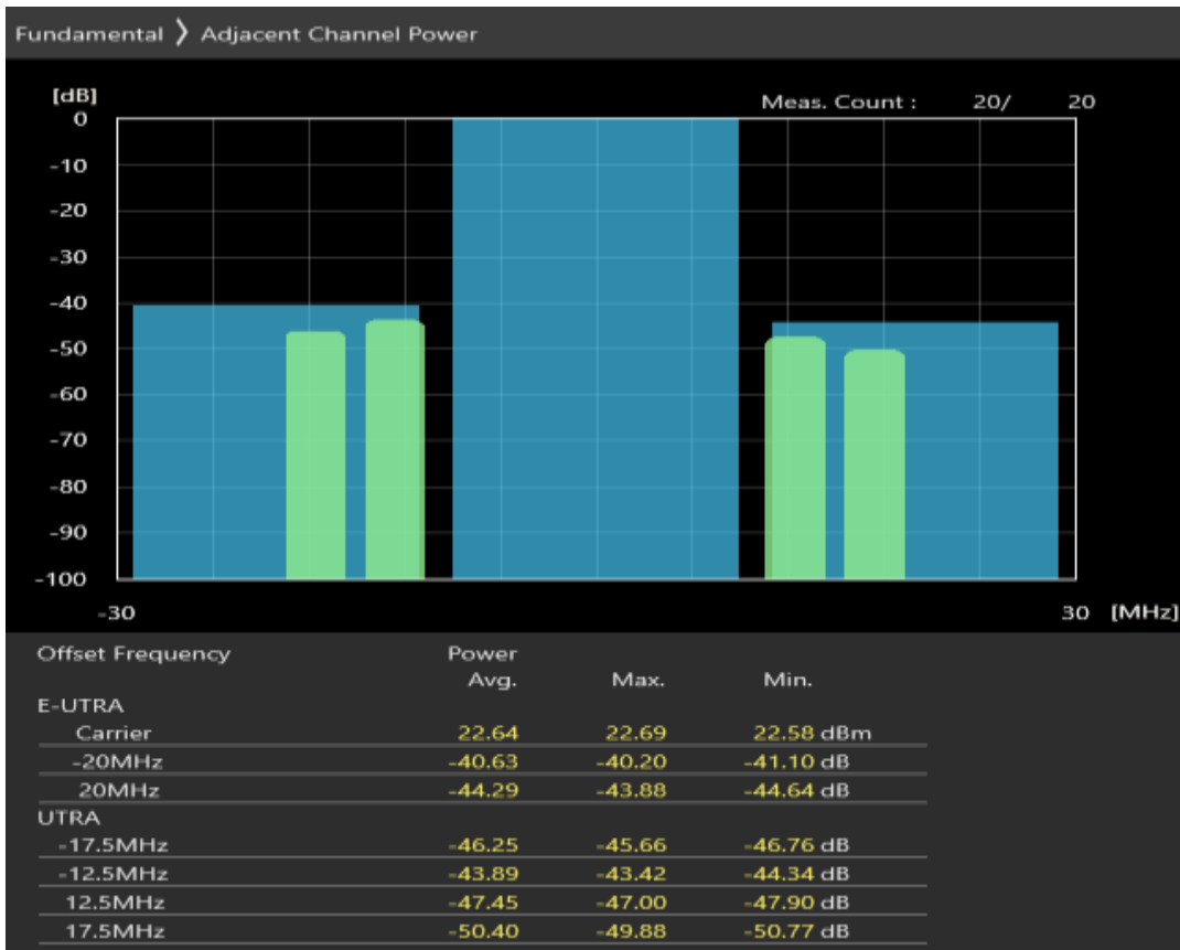
Band1 QPSK BW=20MHz Channel=18500 RB Size=18 Position=#0
