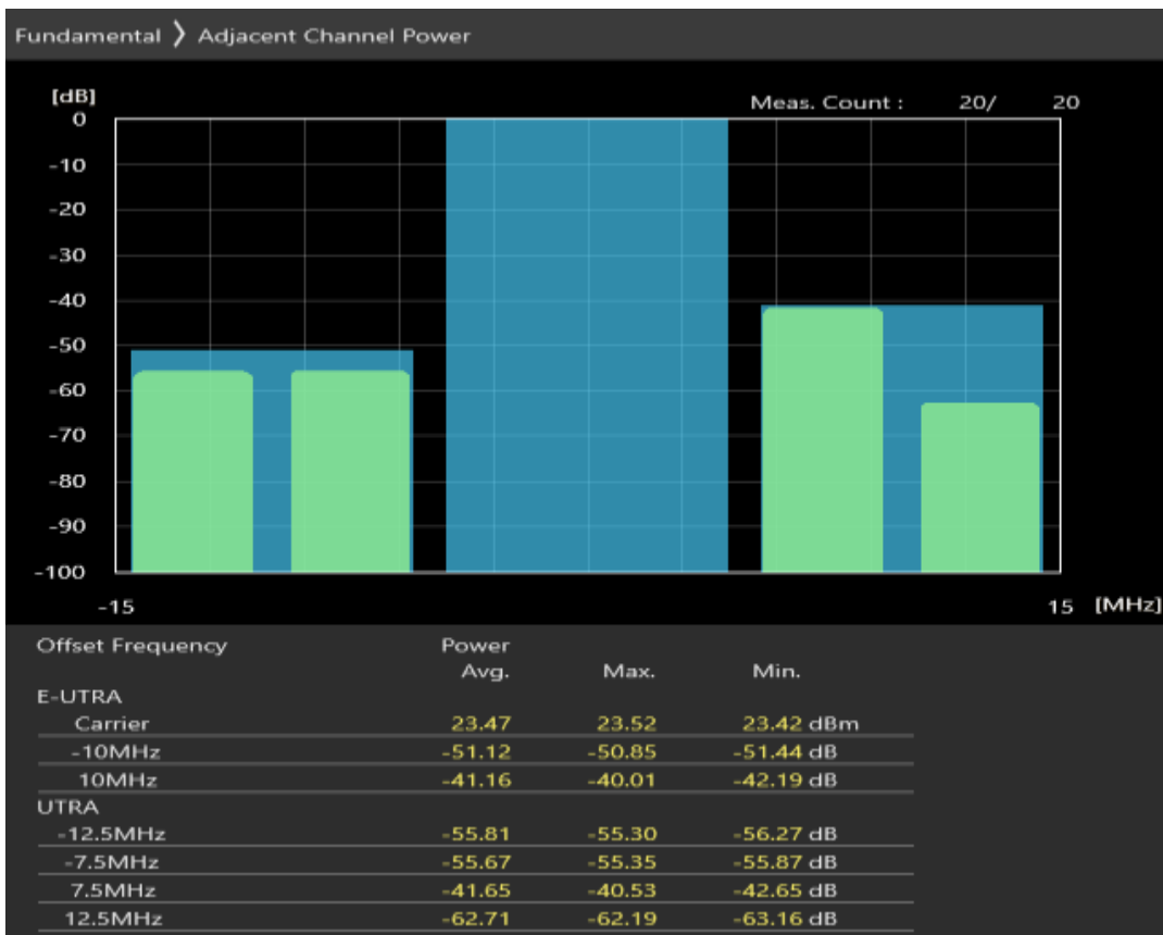
Band3 QAM16 BW=10MHz Channel=19250 RB Size=50 Position=#0
