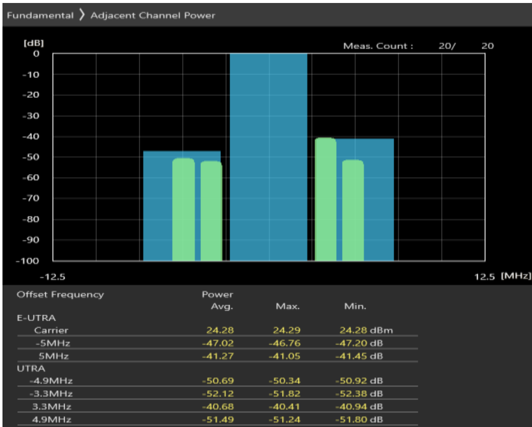
Band40 QPSK BW=5MHz Channel=38675 RB Size=25 Position=#0
