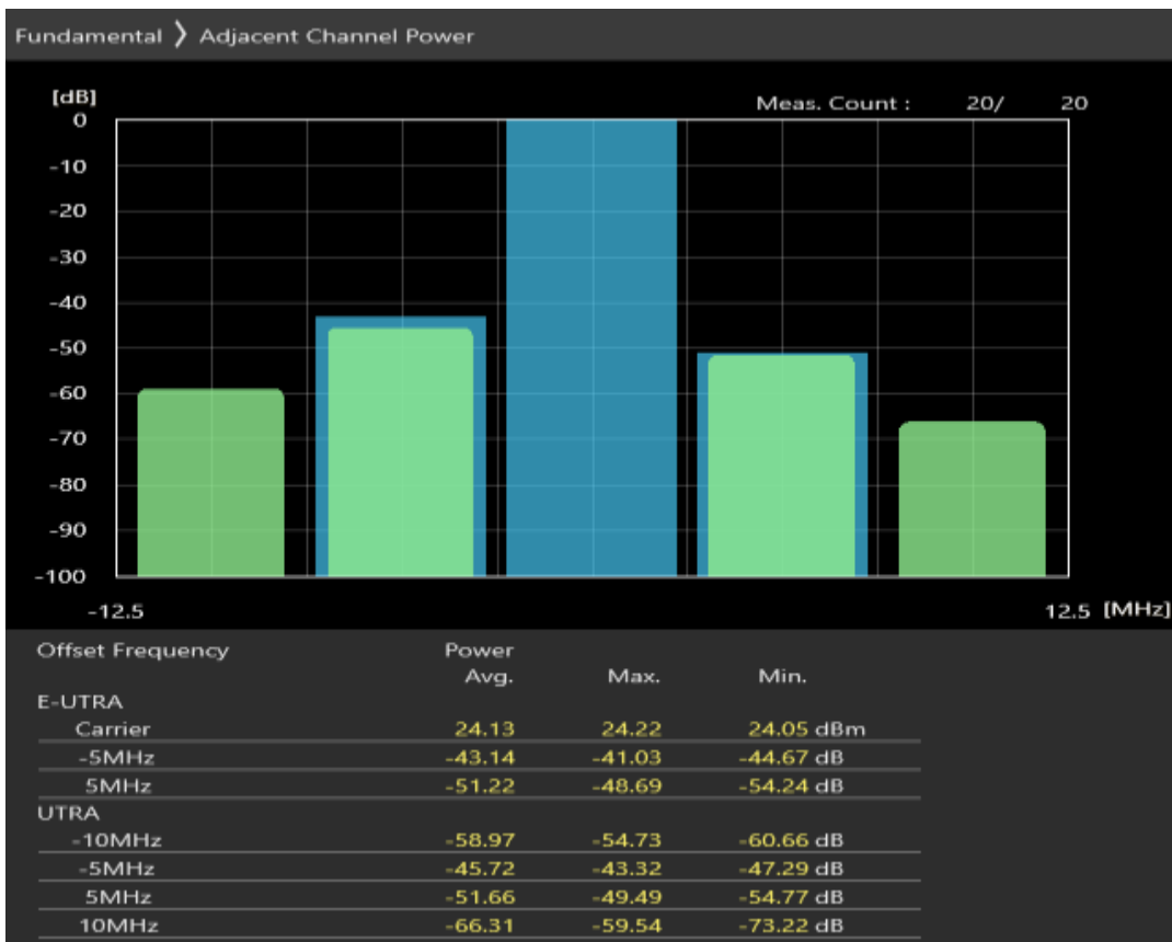
Band20 QPSK BW=5MHz Channel=24300 RB Size=8 Position=#Max
