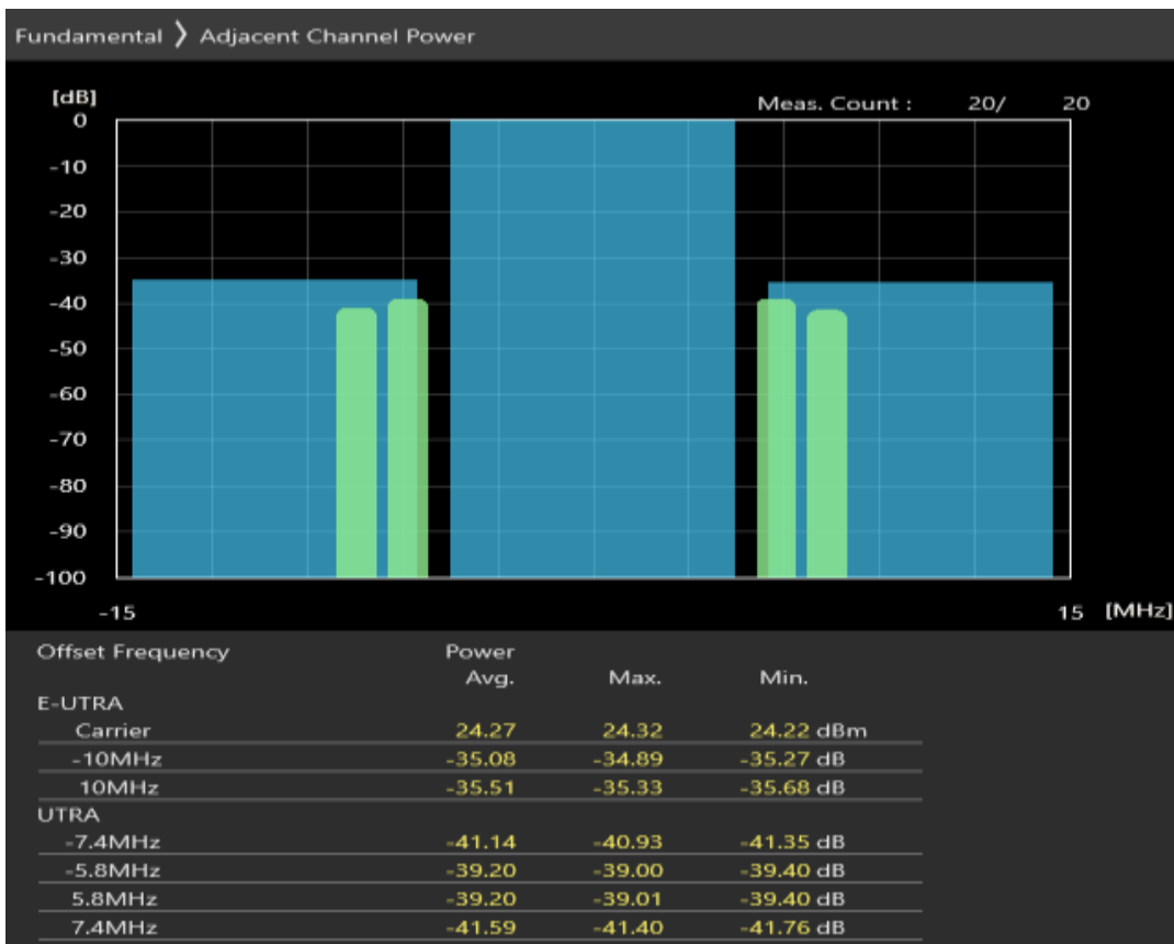
Band40 QAM16 BW=10MHz Channel=39600 RB Size=12 Position=#0
