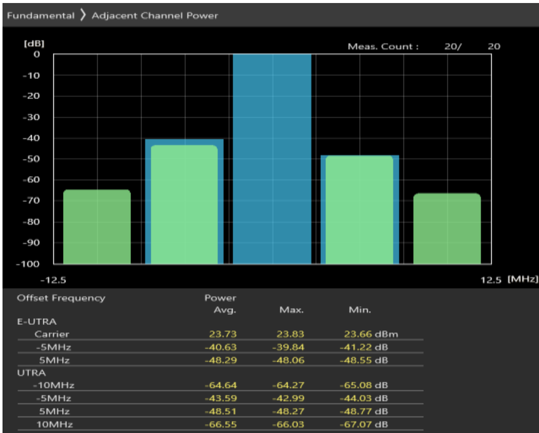
Band7 QAM16 BW=5MHz Channel=20775 RB Size=8 Position=#Max
