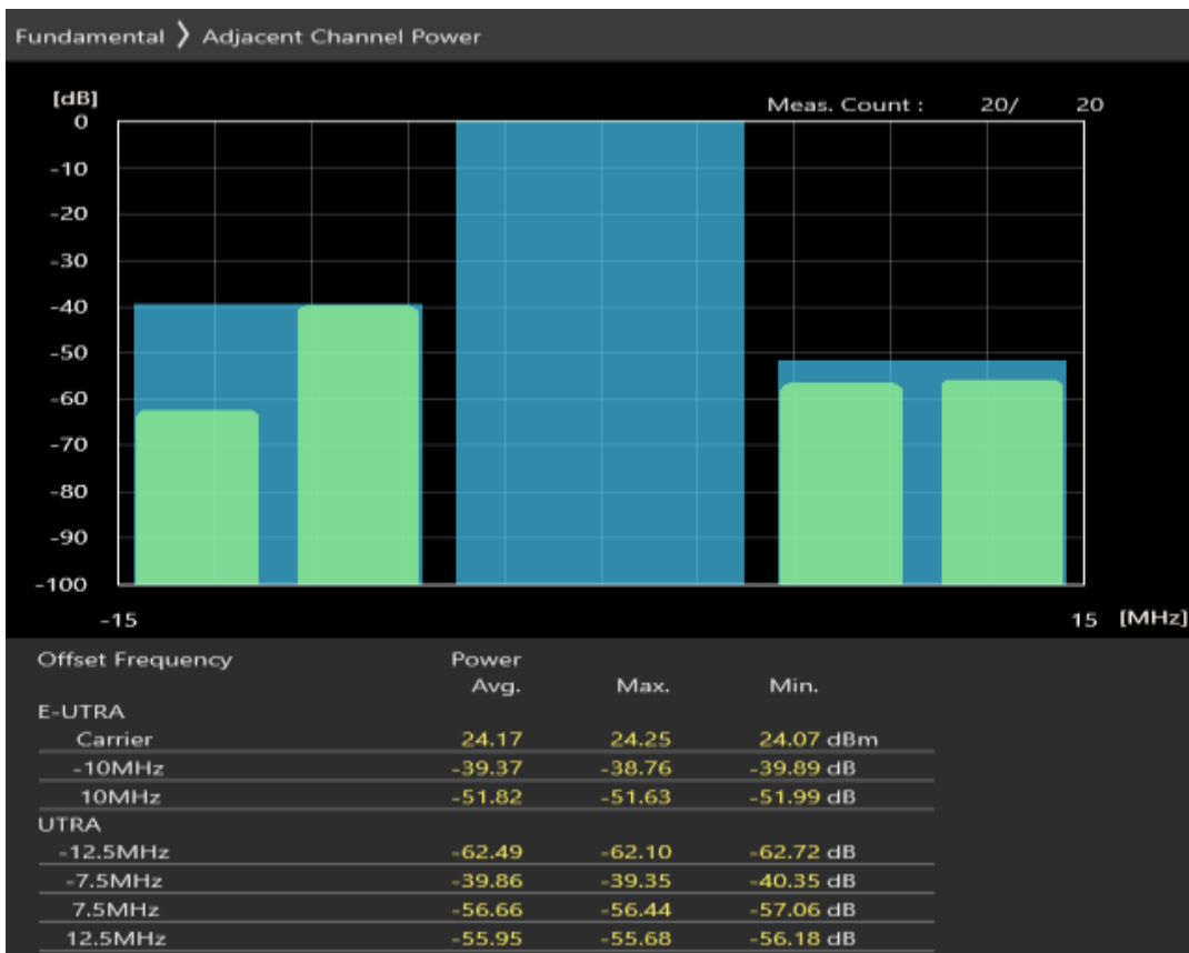
Band8 QPSK BW=10MHz Channel=21625 RB Size=12 Position=#Max
