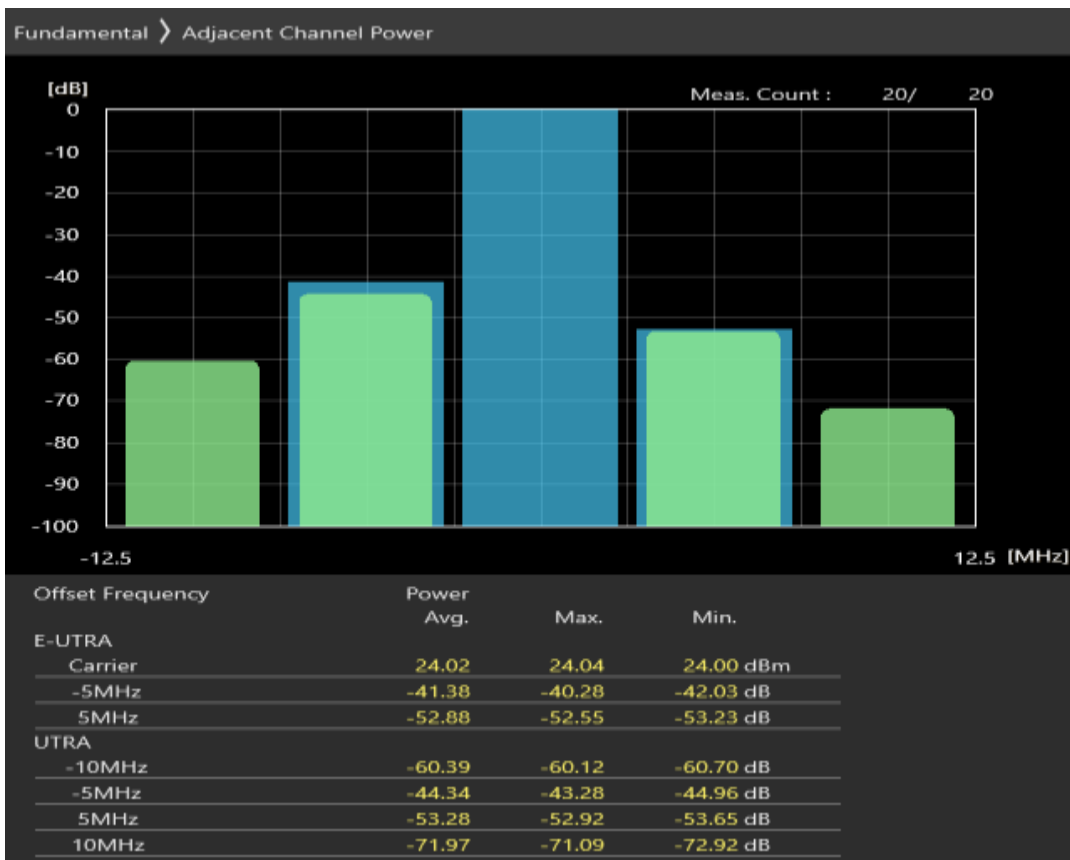
Band20 QPSK BW=5MHz Channel=24425 RB Size=8 Position=#Max
