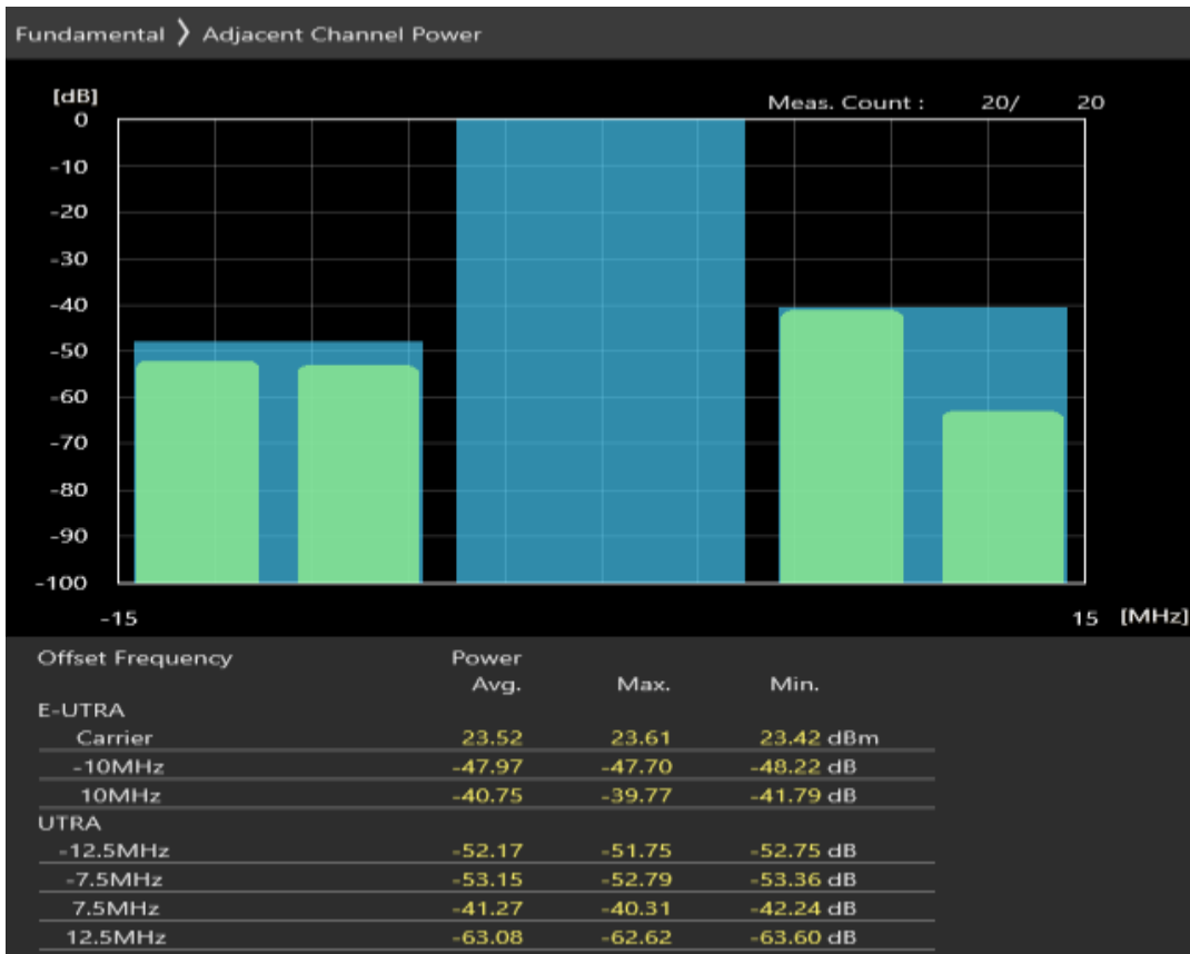
Band3 QAM16 BW=10MHz Channel=19575 RB Size=50 Position=#0
