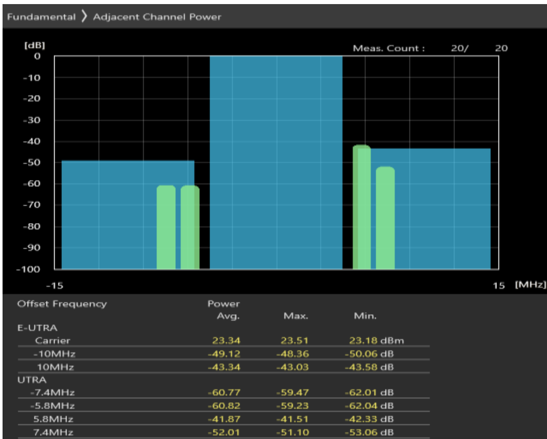
Band40 QAM16 BW=10MHz Channel=38700 RB Size=50 Position=#0
