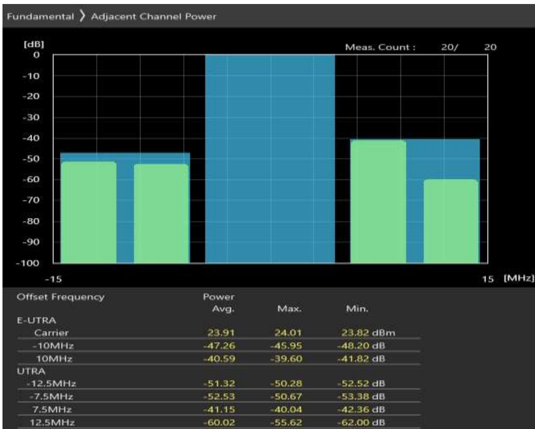
Band7 QAM16 BW=10MHz Channel=21400 RB Size=50 Position=#0
