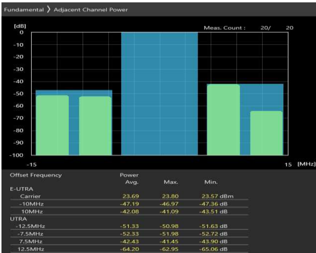
Band3 QAM16 BW=10MHz Channel=1990 RB Size=50 Position=#0
