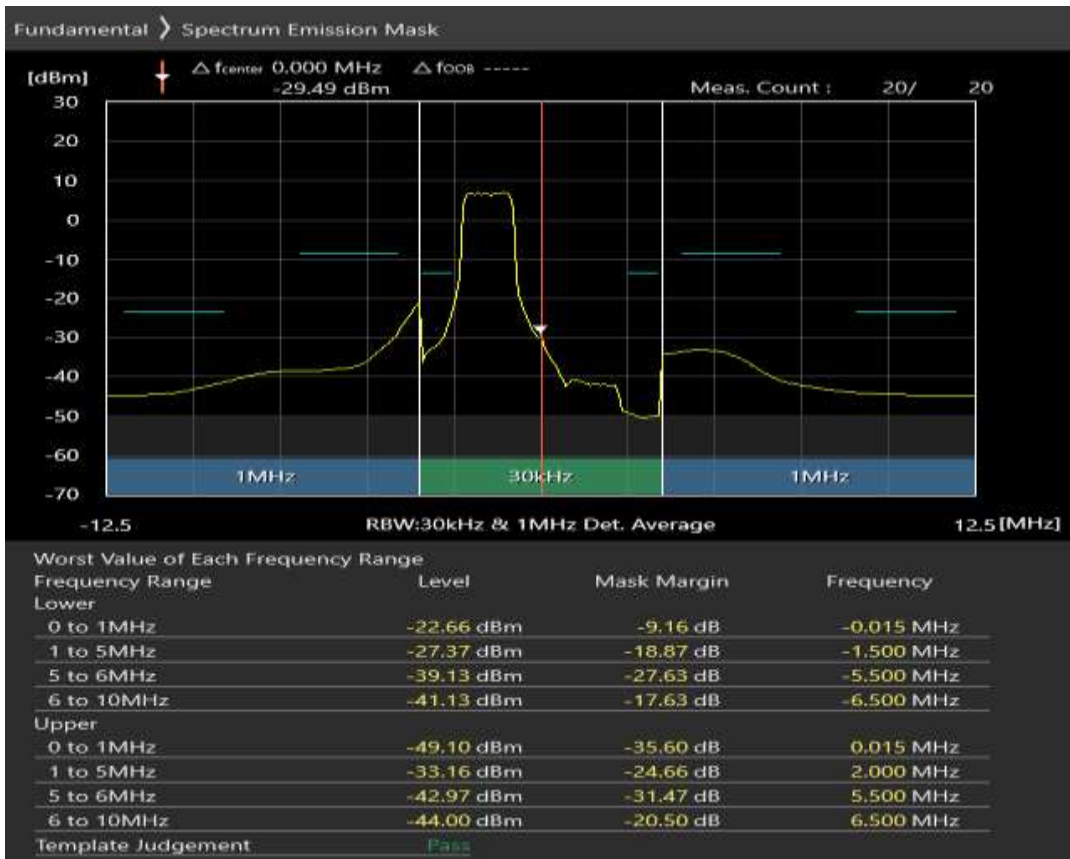
Band8 QAM16 BW=5MHz Channel=21625 RB Size=8 Position=#Max
