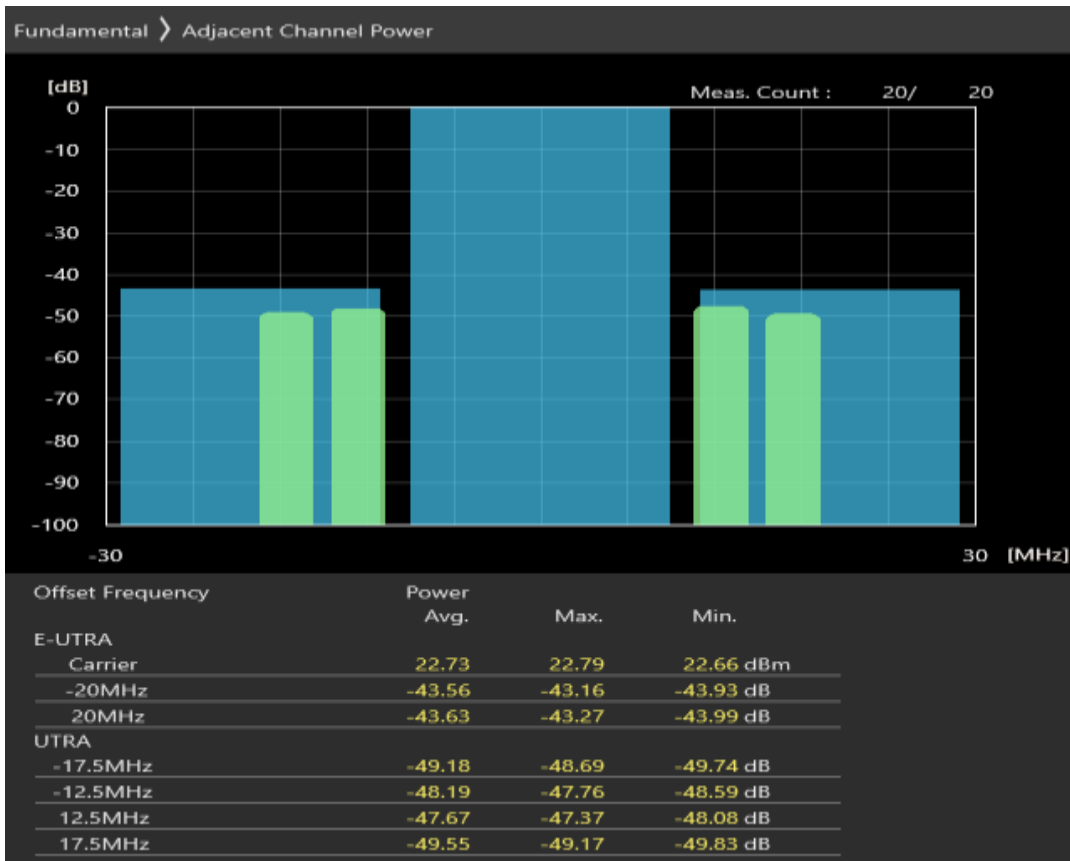
Band20 QPSK BW=5MHz Channel=24175 RB Size=8 Position=#0
