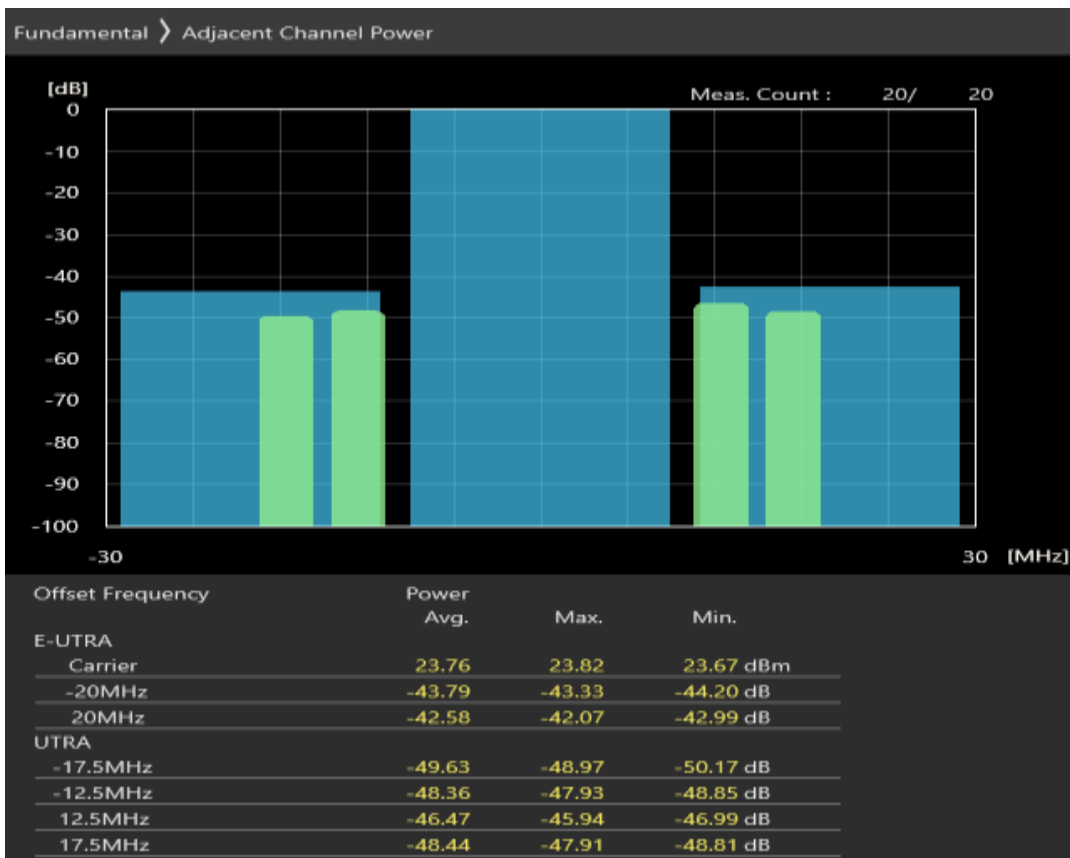
Band1 QAM16 BW=20MHz Channel=18500 RB Size=18 Position=#0
