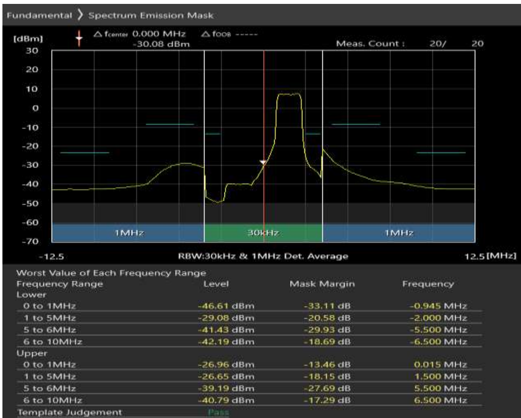
Band7 QAM16 BW=5MHz Channel=20775 RB Size=25 Position=#0
