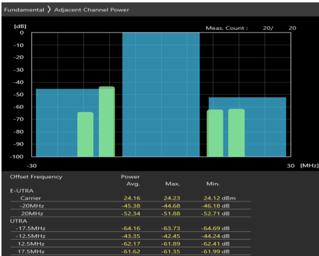
Band20 QPSK BW=20MHz Channel=24300 RB Size=18 Position=#Max
