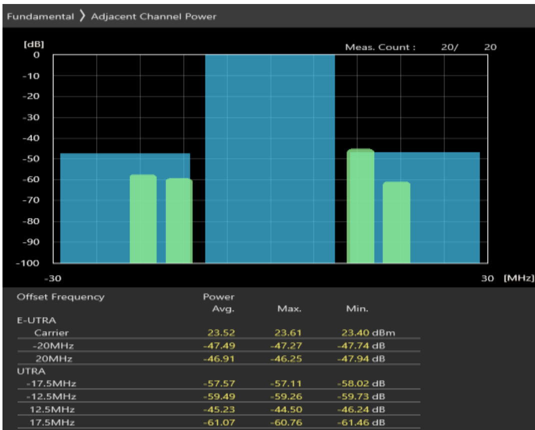
Band1 QAM16 BW=20MHz Channel=18300 RB Size=100 Position=#0
