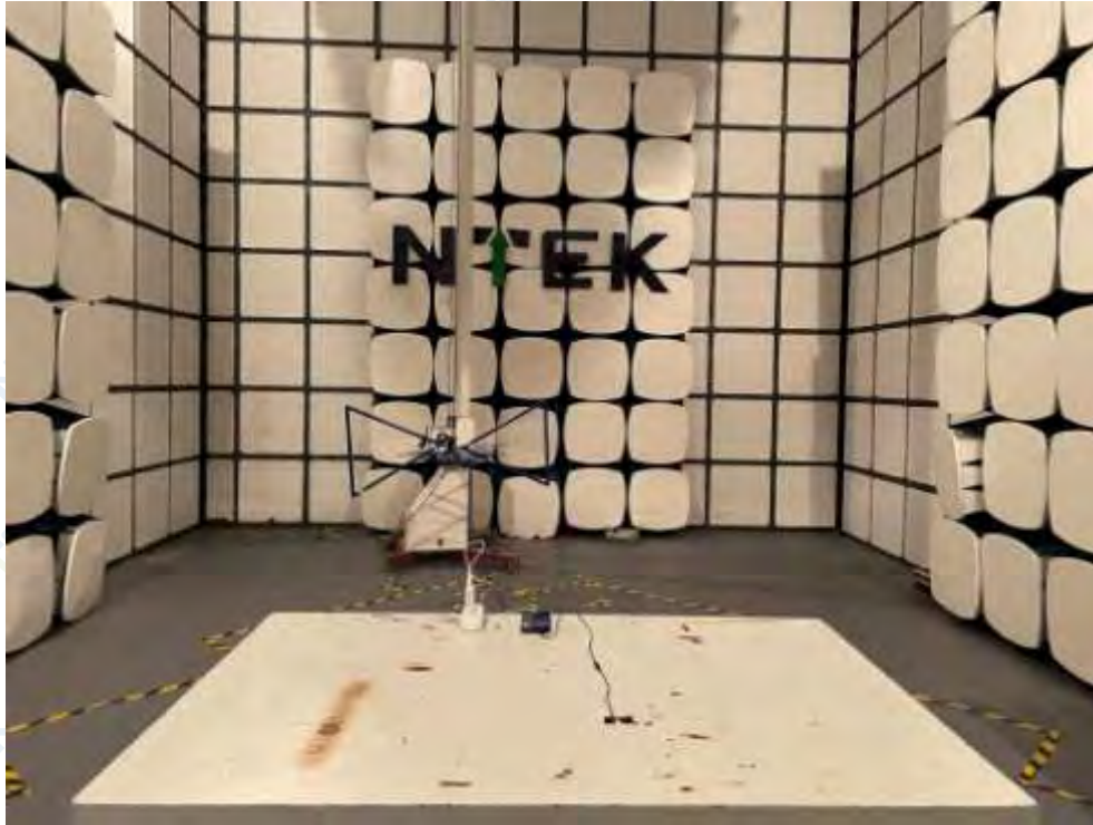
Radiated Measurement Photo
