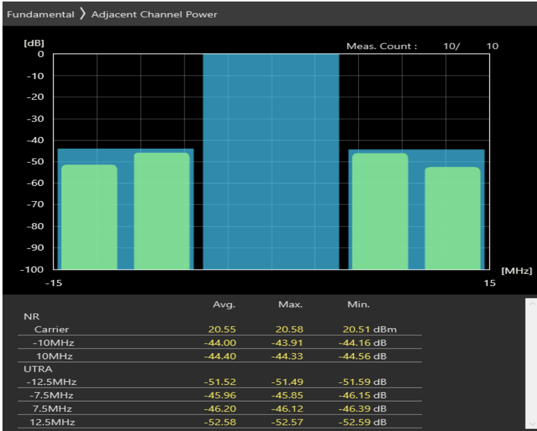
n1 SCS=30kHz DFT_QAM256 BW=20MHz Channel=386000 RB=1@0
