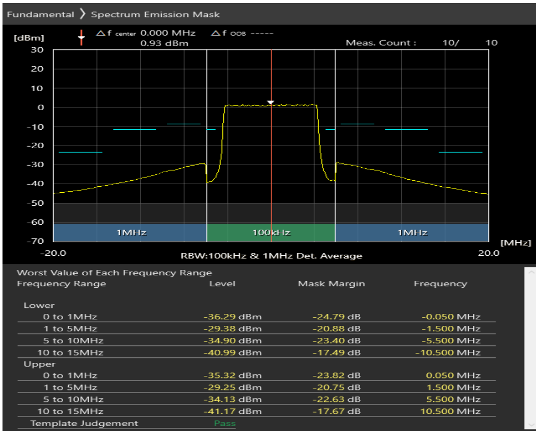
n38 SCS=30kHz DFT_BPSK BW=20MHz Channel=516000 RB=1@0
