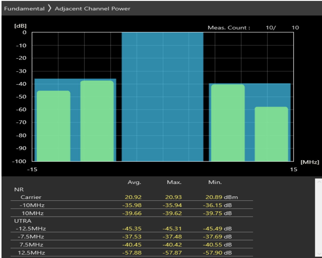
n28 SCS=30kHz CP_QAM64 BW=10MHz Channel=148600 RB=1@23
