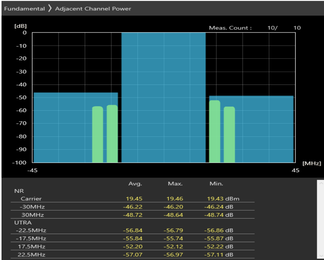
n3 SCS=30kHz DFT_QPSK BW=30MHz Channel=354000 RB=75@0
