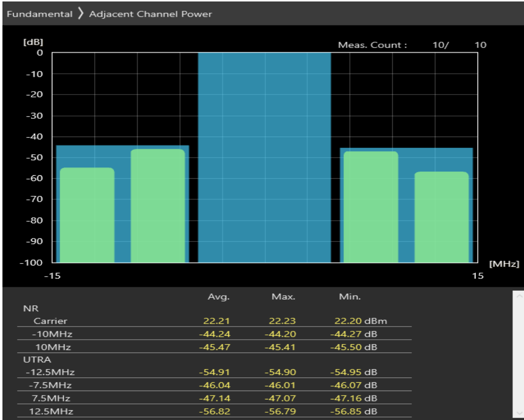
n3 SCS=30kHz DFT_QAM16 BW=10MHz Channel=356000 RB=1@23
