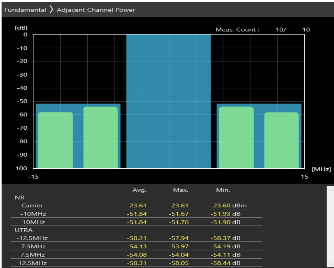
n77 SCS=30kHz DFT_BPSK BW=10MHz Channel=620334 RB=1@0
