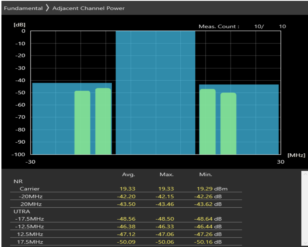
n1 SCS=30kHz DFT_QPSK BW=10MHz Channel=385000 RB=12@6
