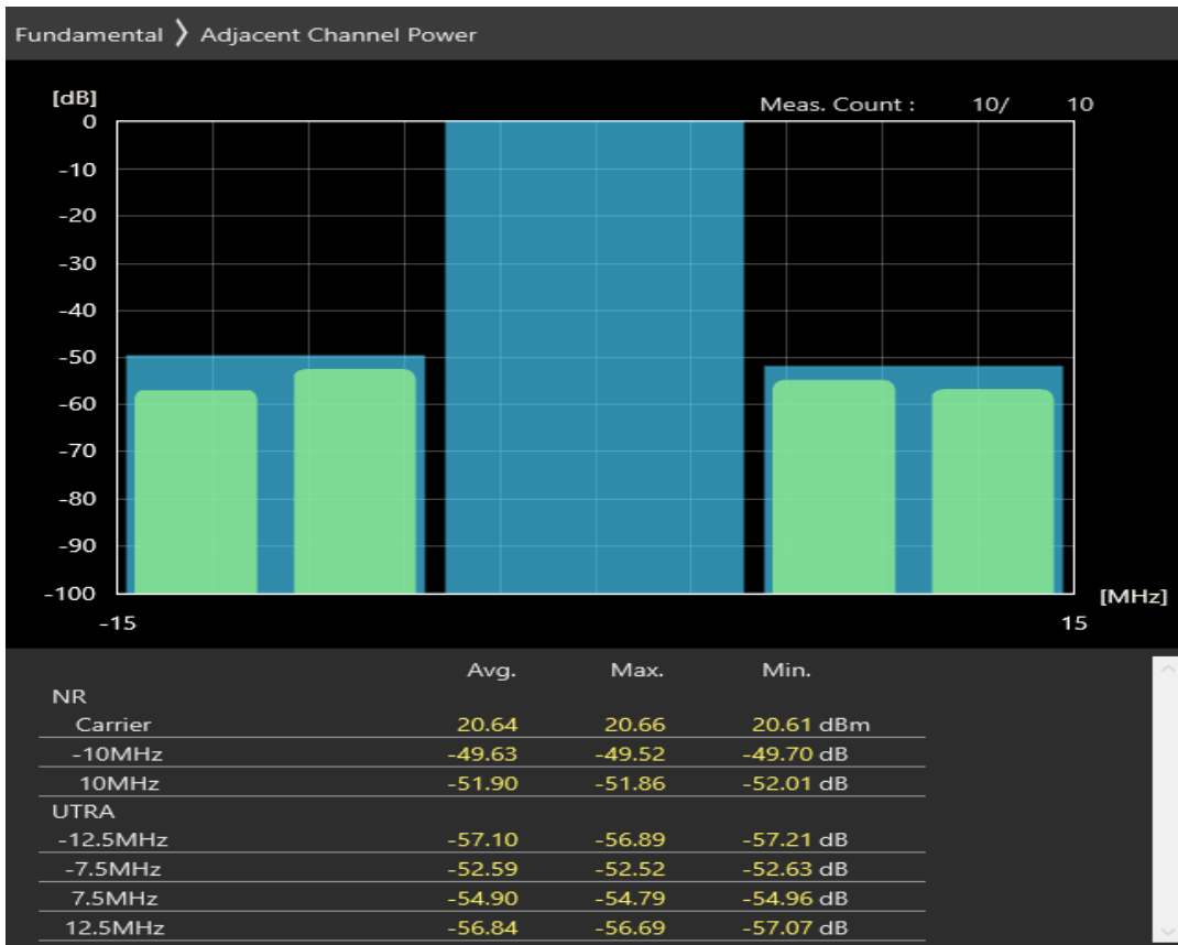
n77 SCS=30kHz CP_QPSK BW=10MHz Channel=620334 RB=24@0
