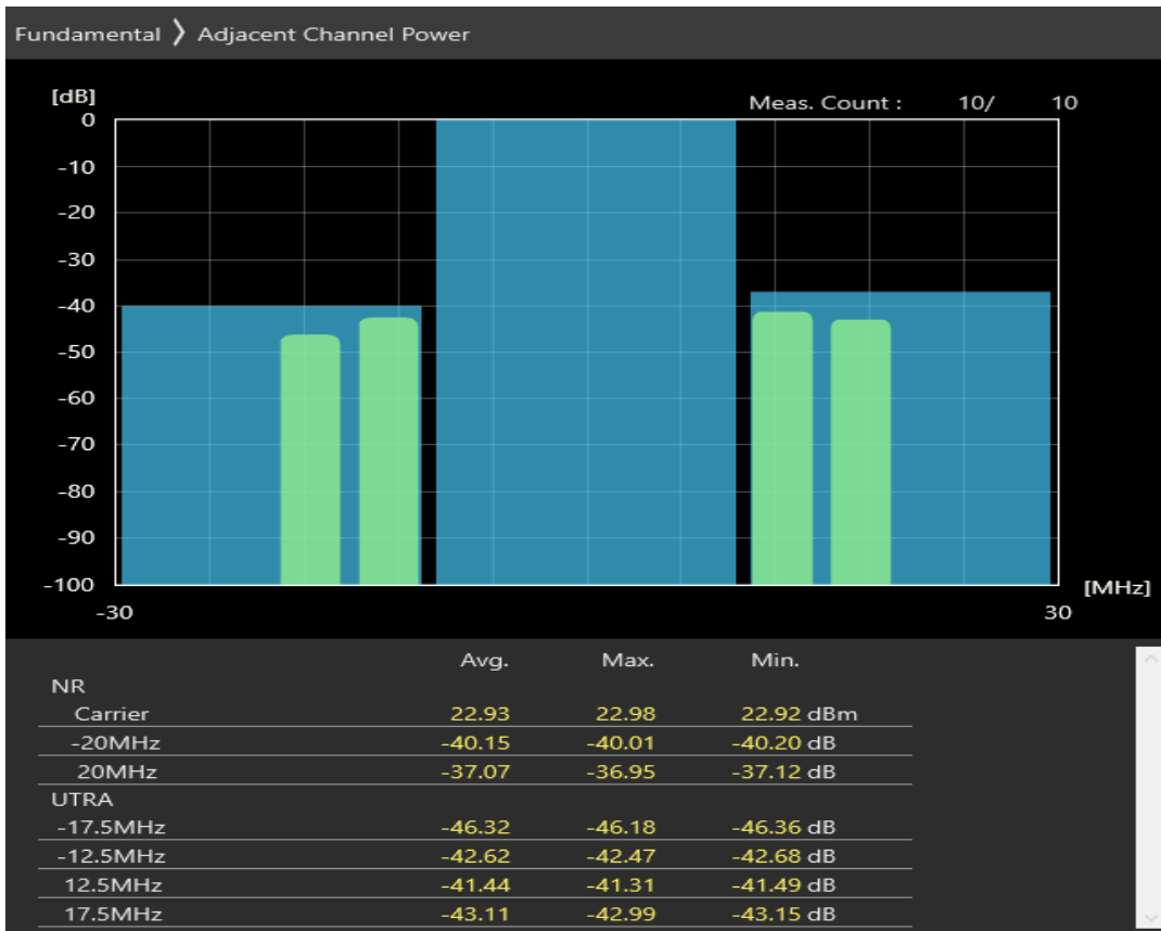
n8 SCS=30kHz DFT_QAM16 BW=20MHz Channel=178000 RB=25@12
