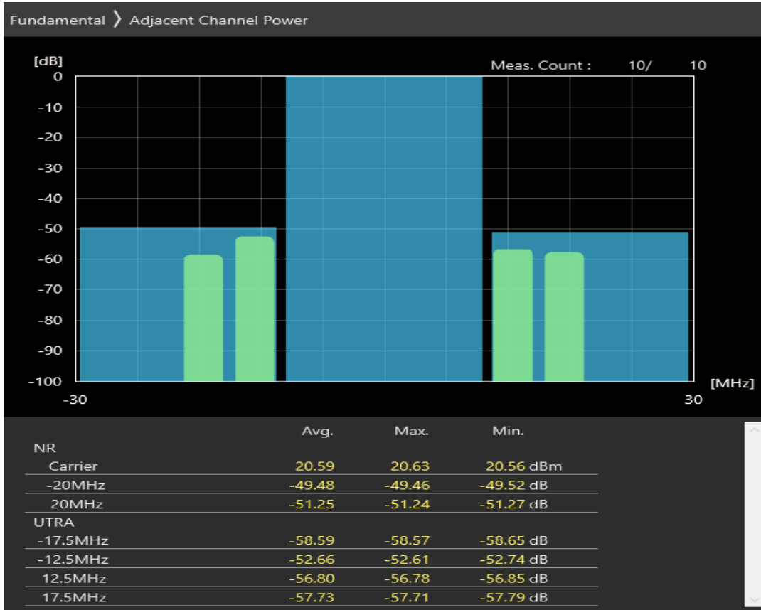
n28 SCS=30kHz CP_QAM16 BW=20MHz Channel=142600 RB=25@12
