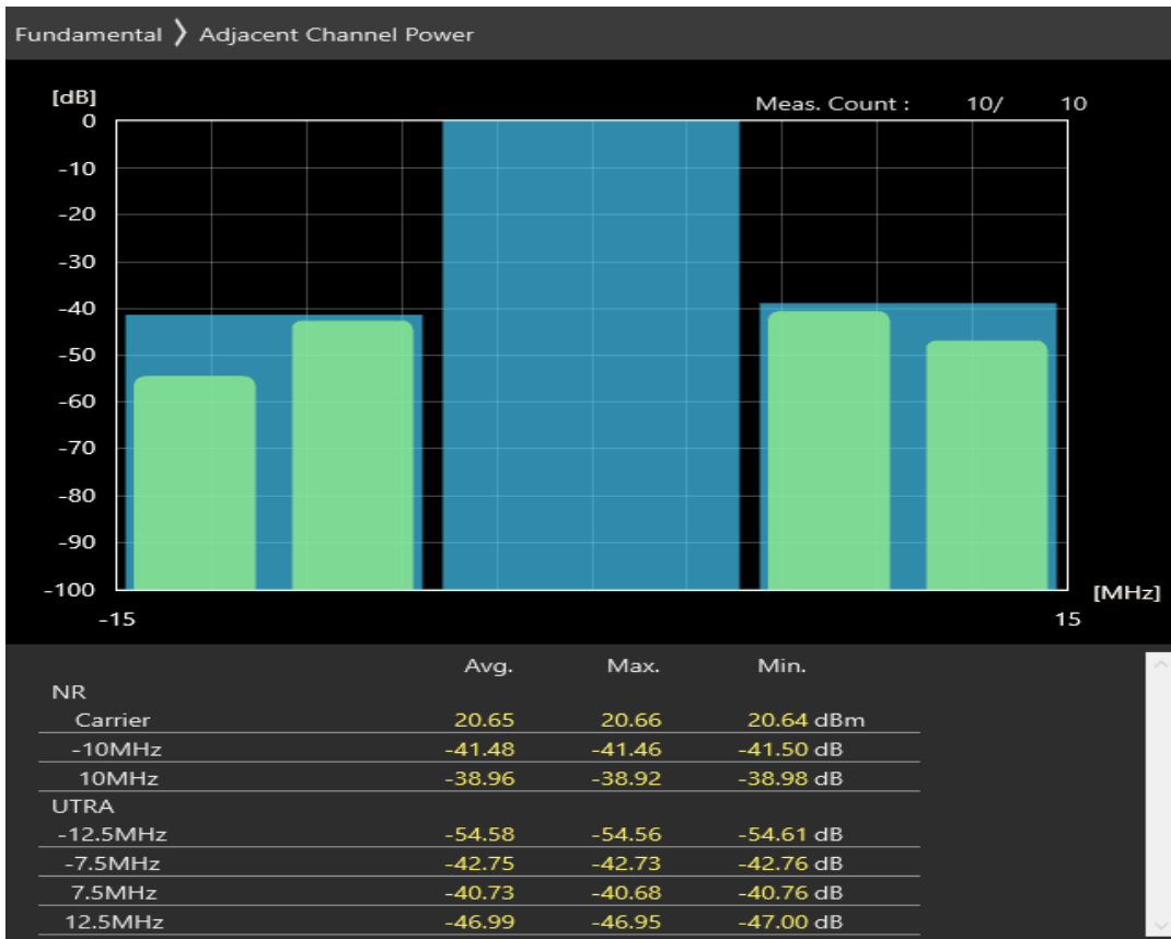
n28 SCS=30kHz CP_QAM64 BW=10MHz Channel=141600 RB=1@0
