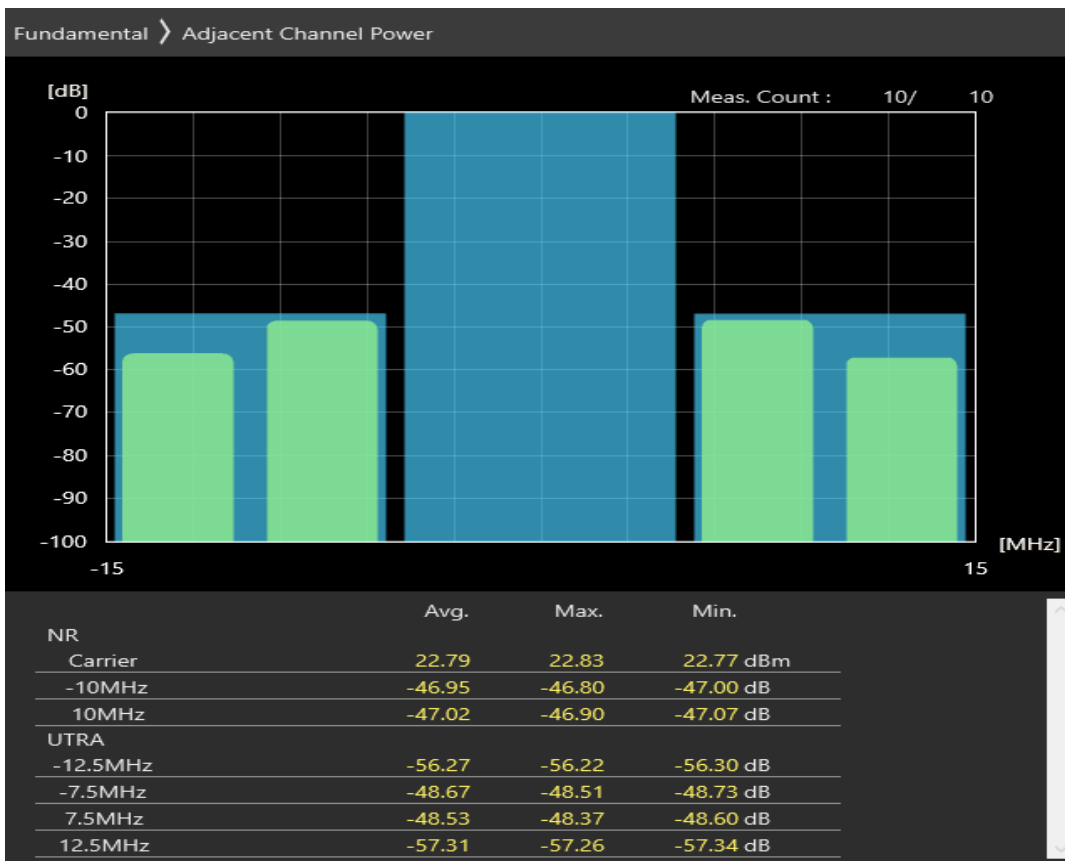
n20 SCS=30kHz DFT_QAM16 BW=10MHz Channel=171400 RB=1@23
