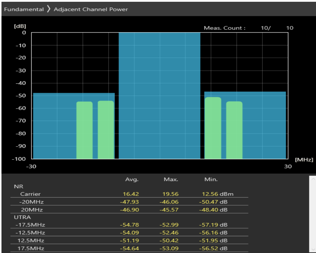
n1 SCS=30kHz CP_QAM256 BW=20MHz Channel=394000 RB=51@0
