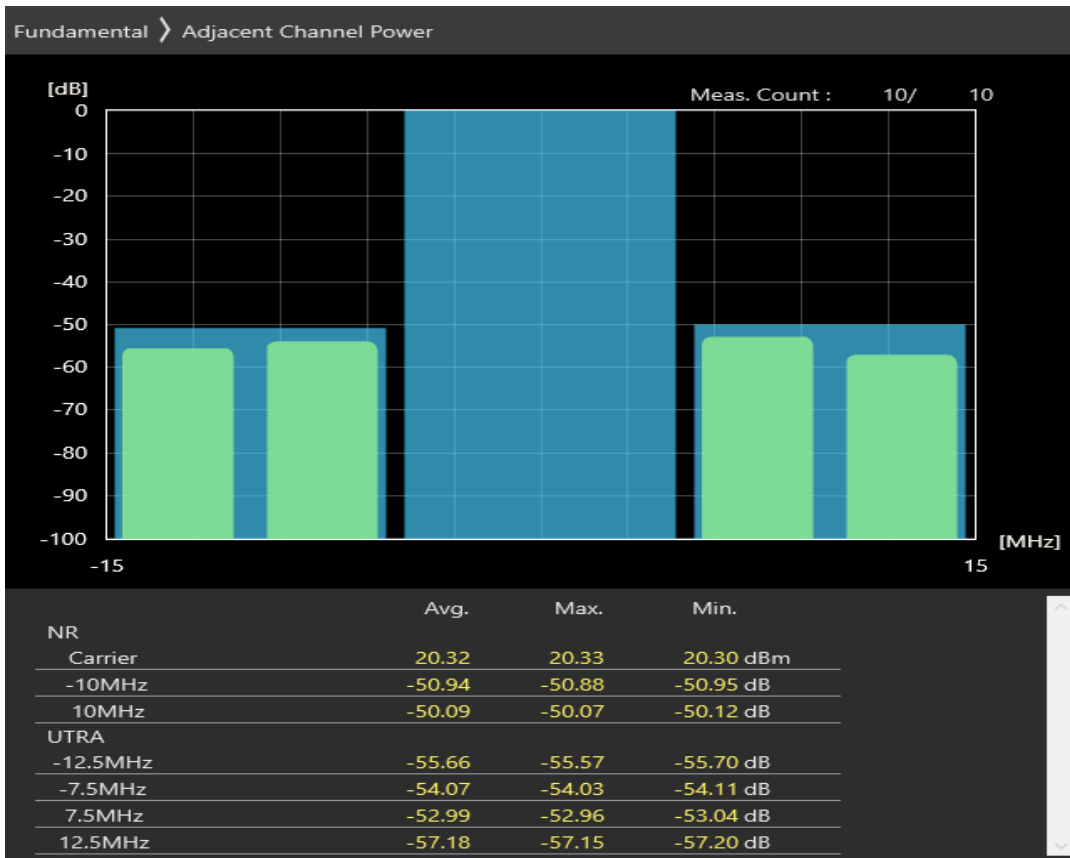
n20 SCS=30kHz CP_QAM16 BW=10MHz Channel=171400 RB=24@0
