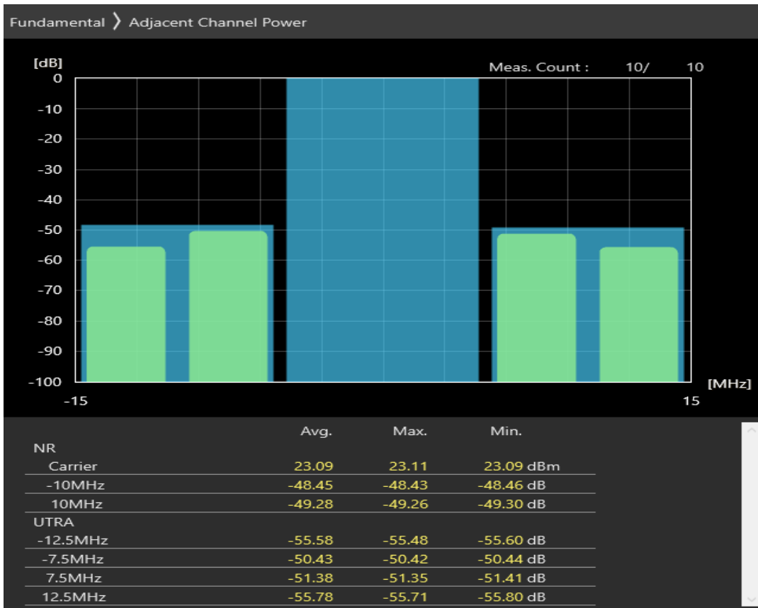
n77 SCS=30kHz DFT_QPSK BW=10MHz Channel=620334 RB=12@6
