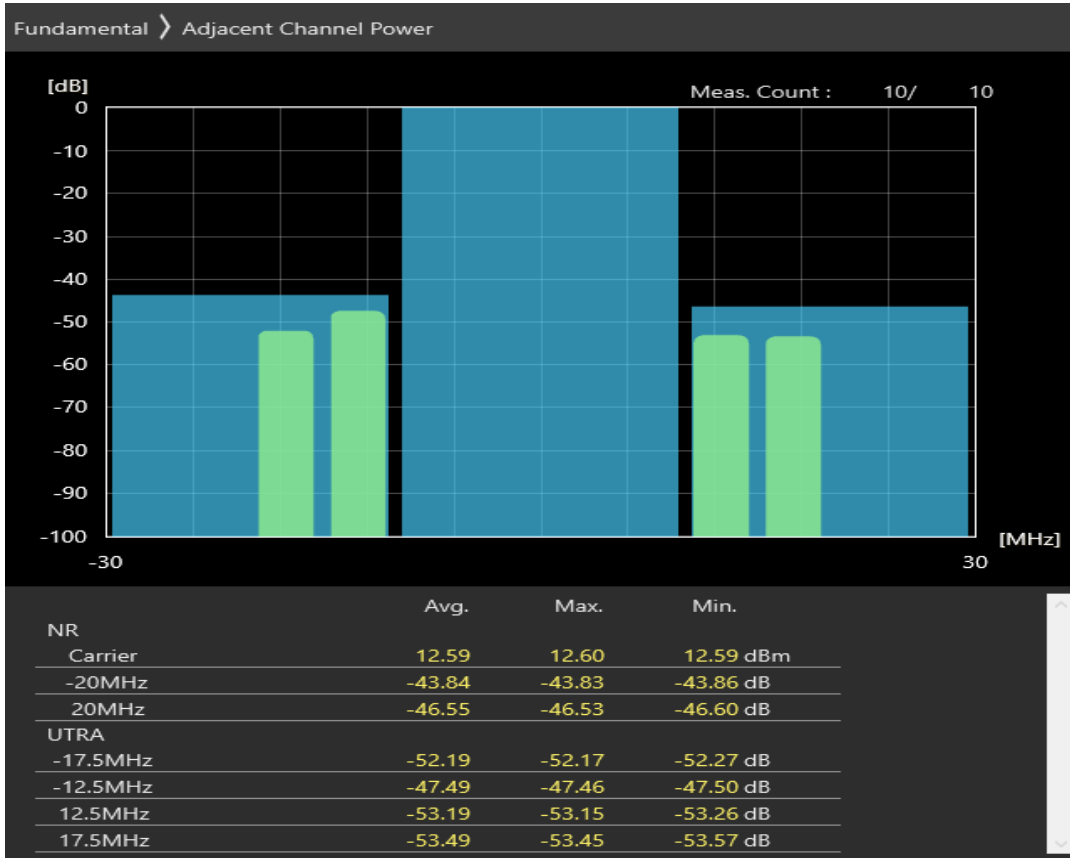
n8 SCS=30kHz CP_QAM64 BW=20MHz Channel=178000 RB=1 @0
