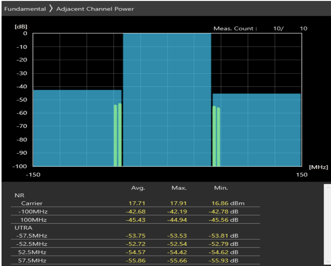
n77 SCS=30kHz DFT_QAM16 BW=100MHz Channel=676666 RB=1@272
