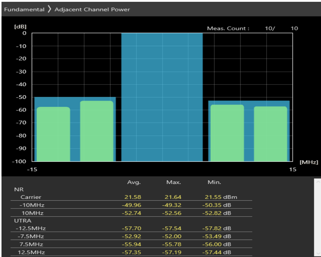
n8 SCS=30kHz DFT_QAM64 BW=10MHz Channel=177000 RB=24@0
