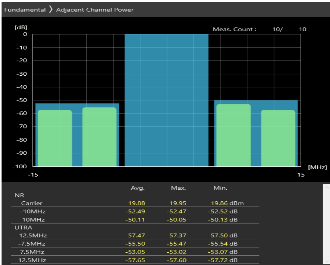
n77 SCS=30kHz CP_QAM64 BW=10MHz Channel=679666 RB=24@0
