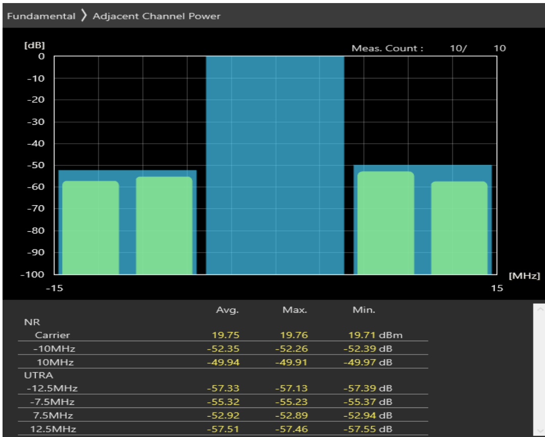
n77 SCS=30kHz CP_QAM16 BW=10MHz Channel=679666 RB=24@0
