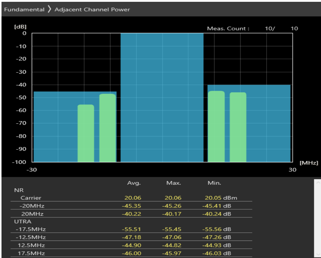
n28 SCS=30kHz DFT_QAM256 BW=20MHz Channel=142600 RB=1@0
