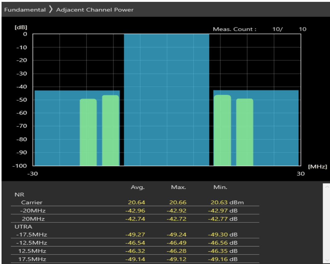
n38 SCS=30kHz DFT_QAM16 BW=20MHz Channel=522000 RB=25@12
