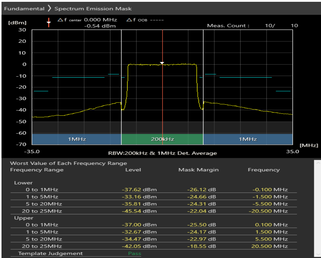
n1 SCS=30kHz CP_QAM256 BW=20MHz Channel=386000 RB=1@0
