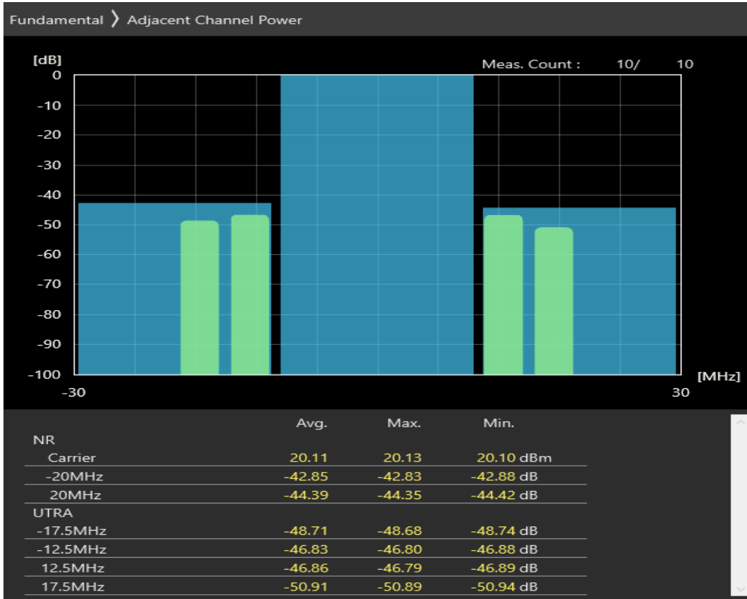
n20 SCS=30kHz DFT_QAM64 BW=20MHz Channel=170400 RB=1@50
