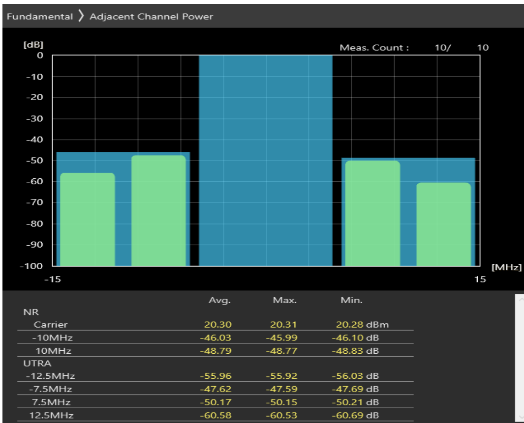
n28 SCS=30kHz DFT_BPSK BW=10MHz Channel=148600 RB=1@23
