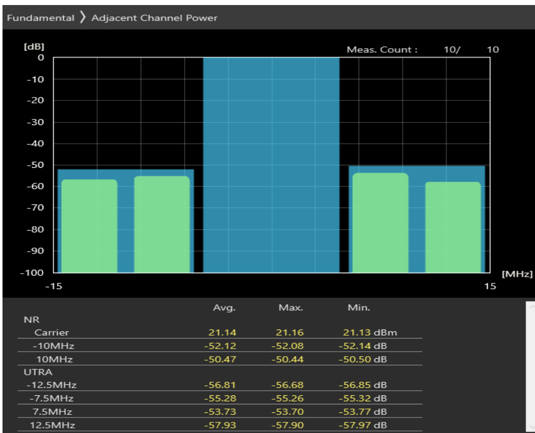
n20 SCS=30kHz DFT_QAM64 BW=10MHz Channel=171400 RB=24@0
