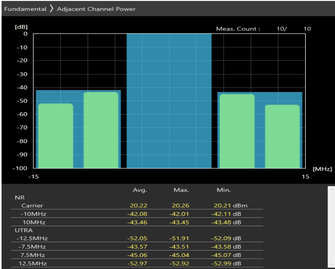
n77 SCS=30kHz CP_QPSK BW=10MHz Channel=679666 RB=12@6
