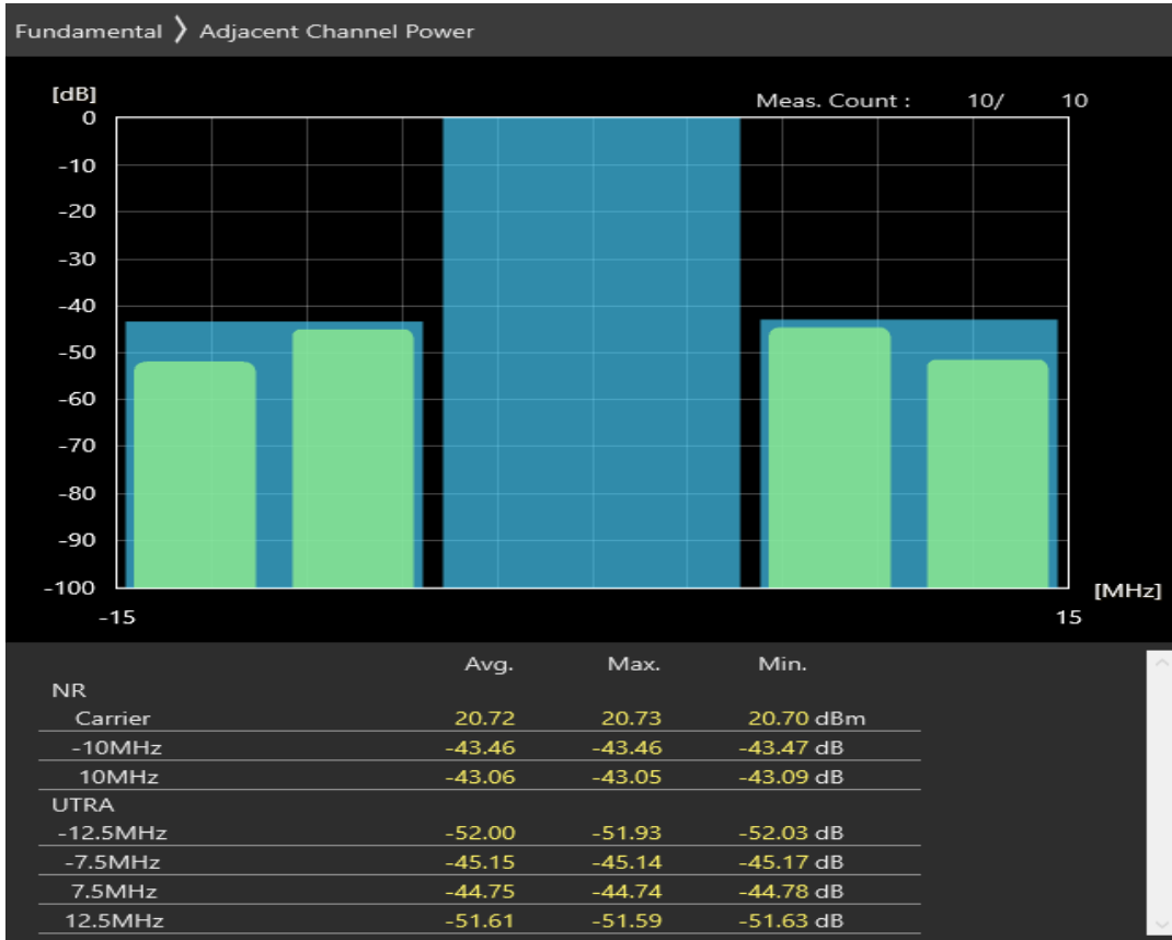
n38 SCS=30kHz DFT_BPSK BW=20MHz Channel=516000 RB=25@12
