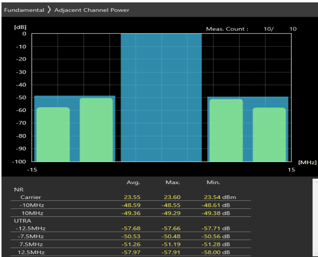
n77 SCS=30kHz DFT_QAM16 BW=10MHz Channel=679666 RB=1@23
