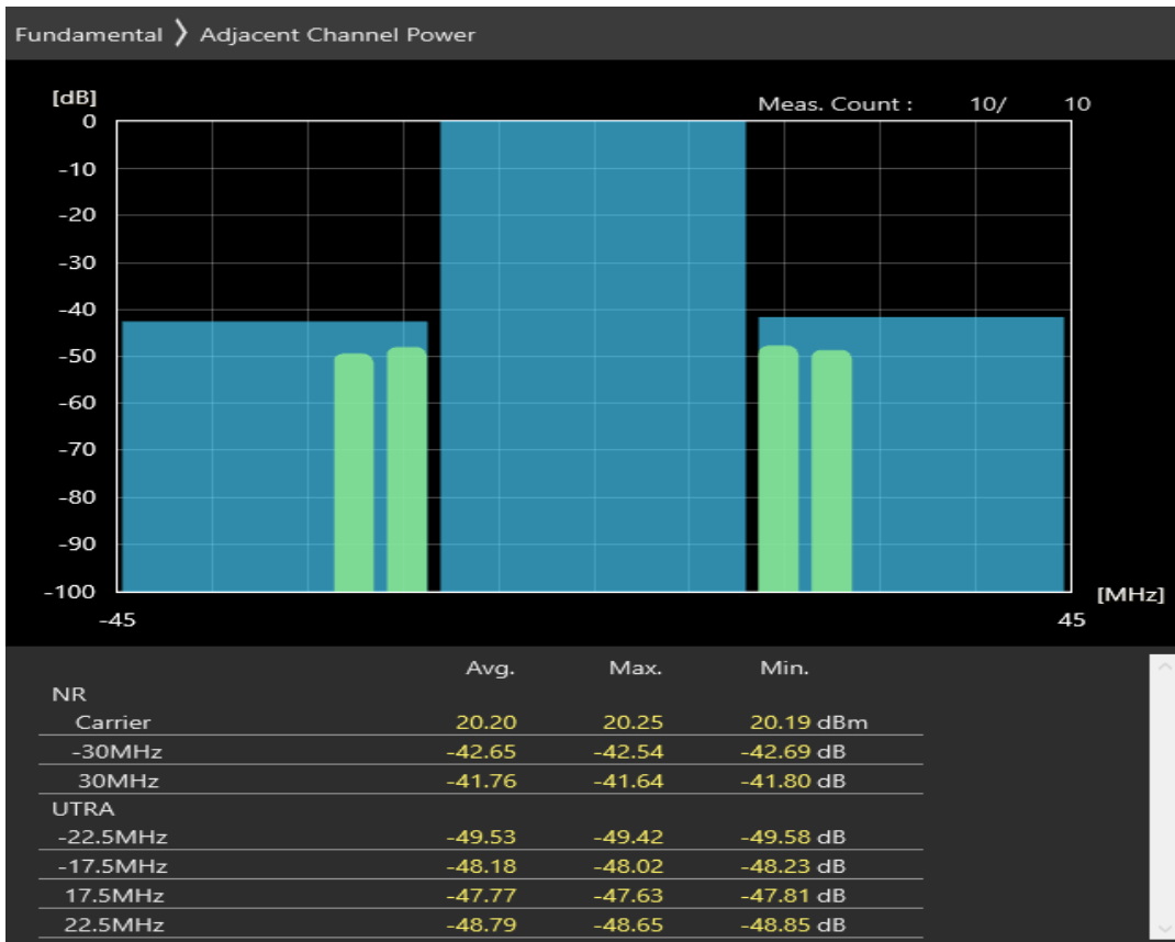
n3 SCS=30kHz CP_QPSK BW=30MHz Channel=345000 RB=39@19
