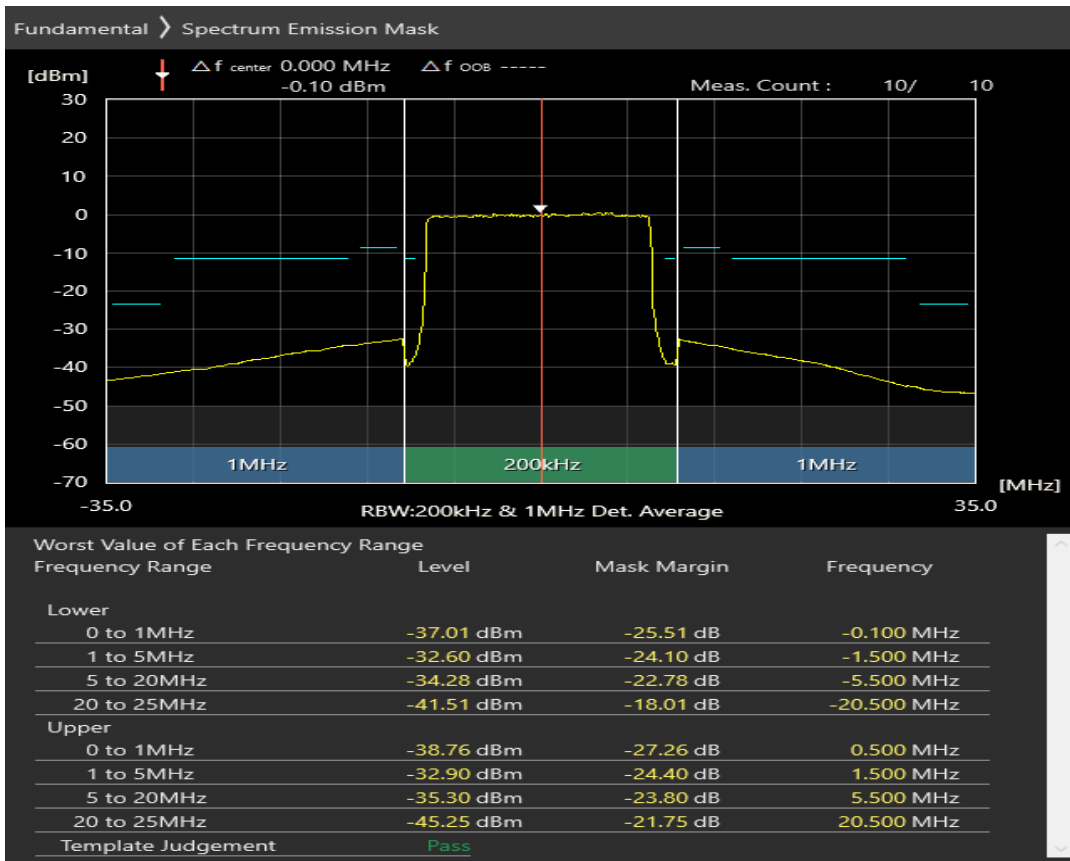
n1 SCS=30kHz DFT_QPSK BW=20MHz Channel=394000 RB=1@50
