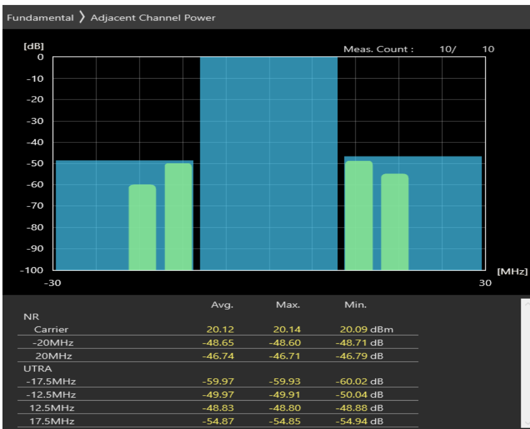
n28 SCS=30kHz DFT_BPSK BW=20MHz Channel=142600 RB=1@0
