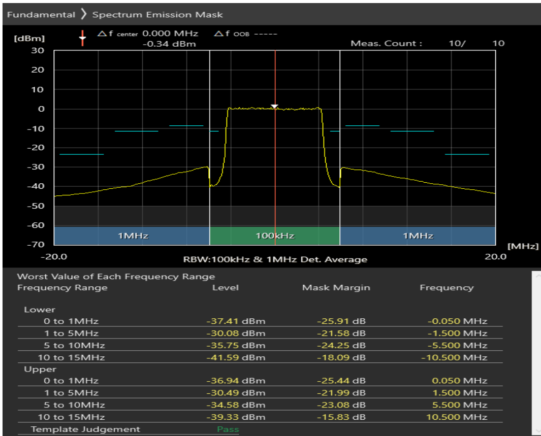
n1 SCS=30kHz DFT_BPSK BW=10MHz Channel=395000 RB=1@23
