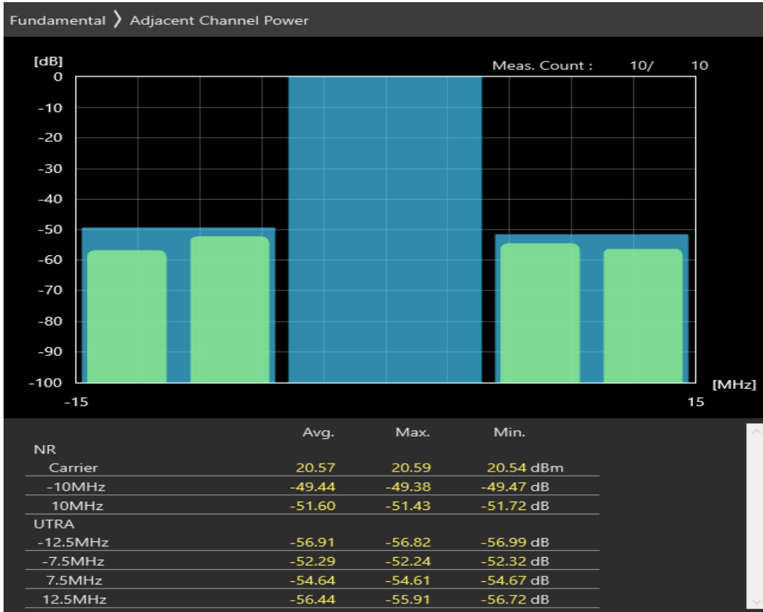
n78 SCS=30kHz CP_QAM256 BW=10MHz Channel=647000 RB=24@0
