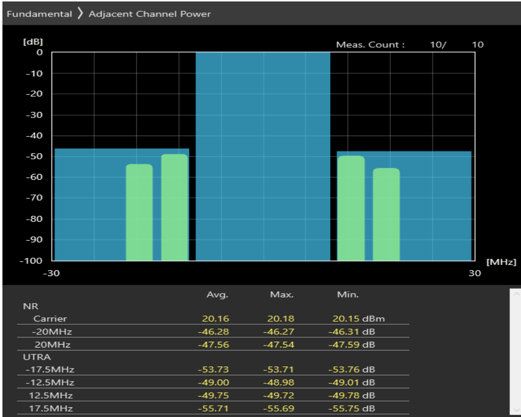
n20 SCS=30kHz DFT_BPSK BW=20MHz Channel=170400 RB=1@50
