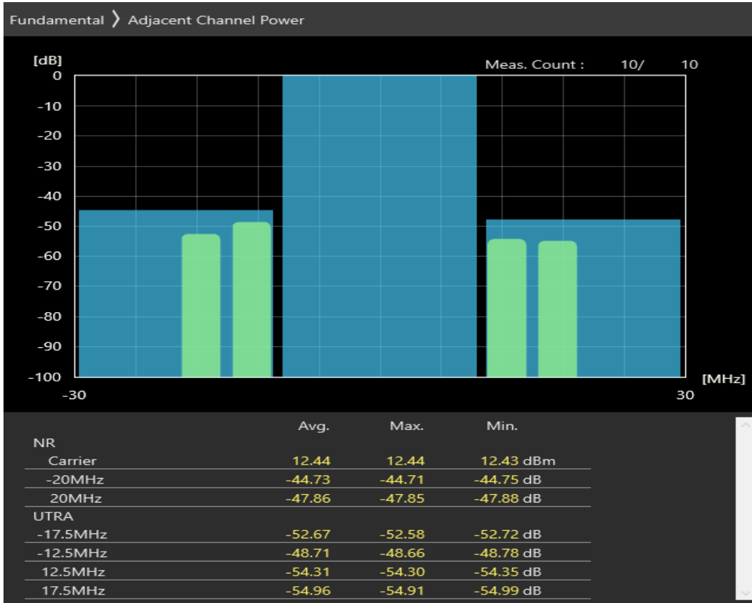
n28 SCS=30kHz CP_QAM64 BW=20MHz Channel=147600 RB=1@50
