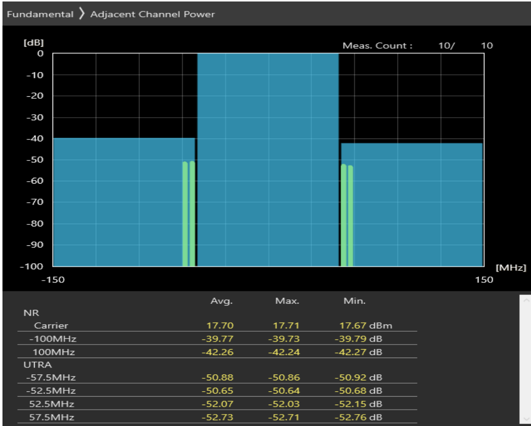
n77 SCS=30kHz CP_QPSK BW=100MHz Channel=676666 RB=137@68
