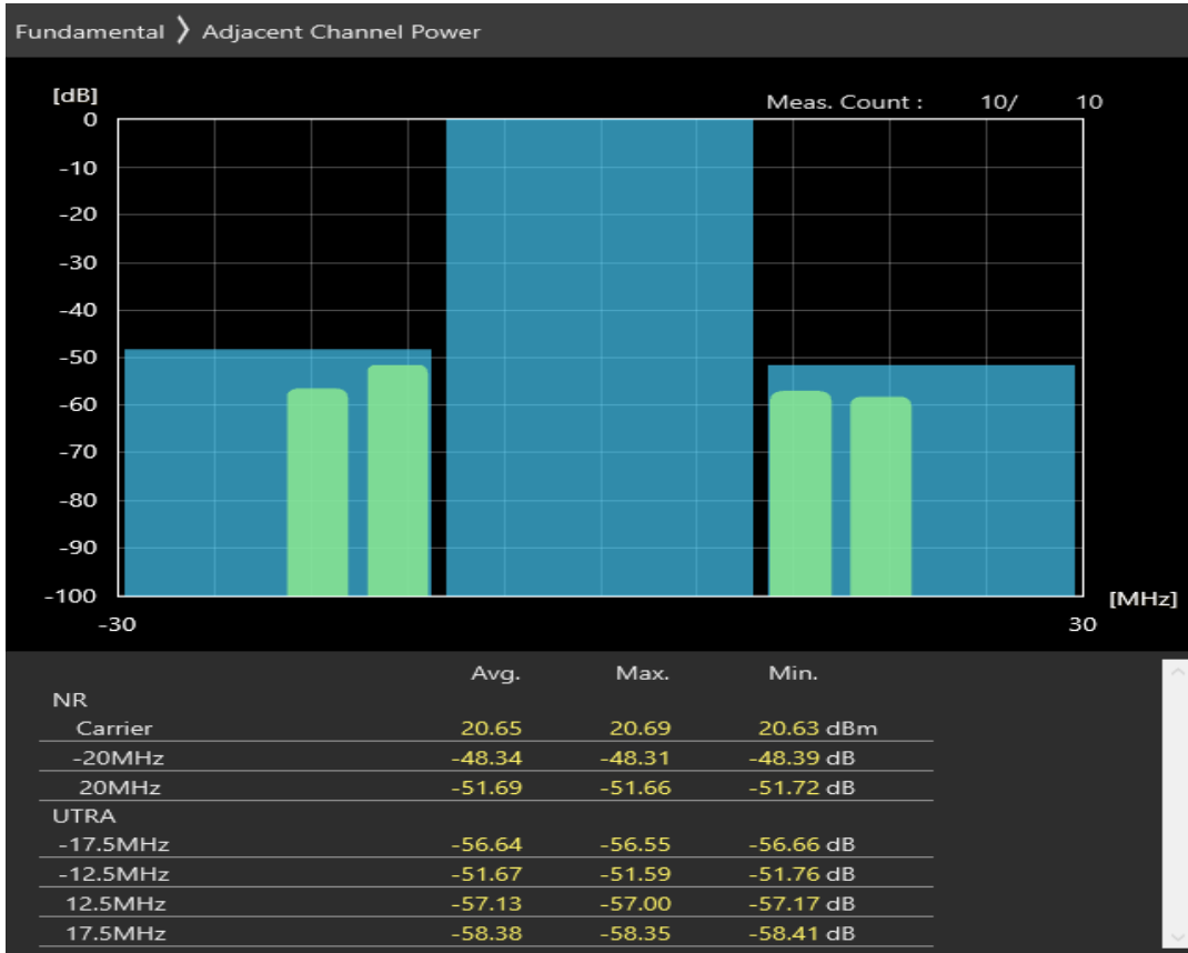
n77 SCS=30kHz DFT_BPSK BW=10MHz Channel=620334 RB=12@6
