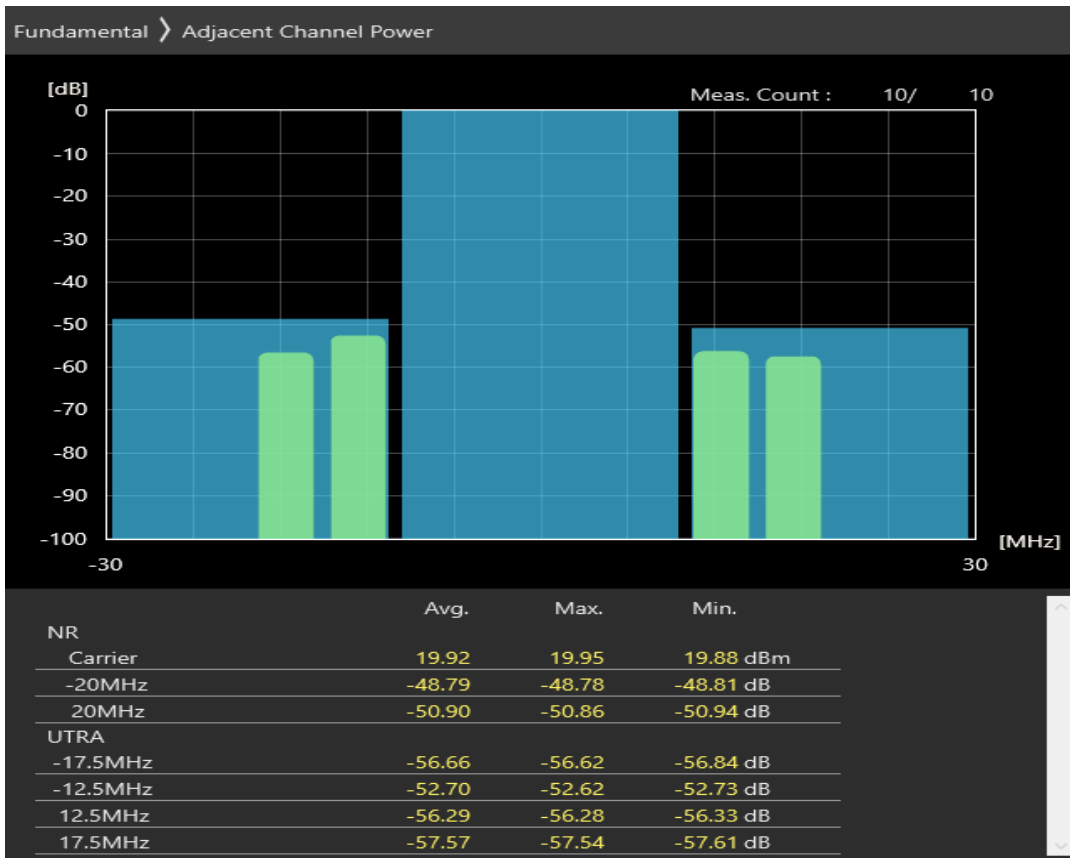
n1 SCS=30kHz CP_QPSK BW=20MHz Channel=394000 RB=1@50
