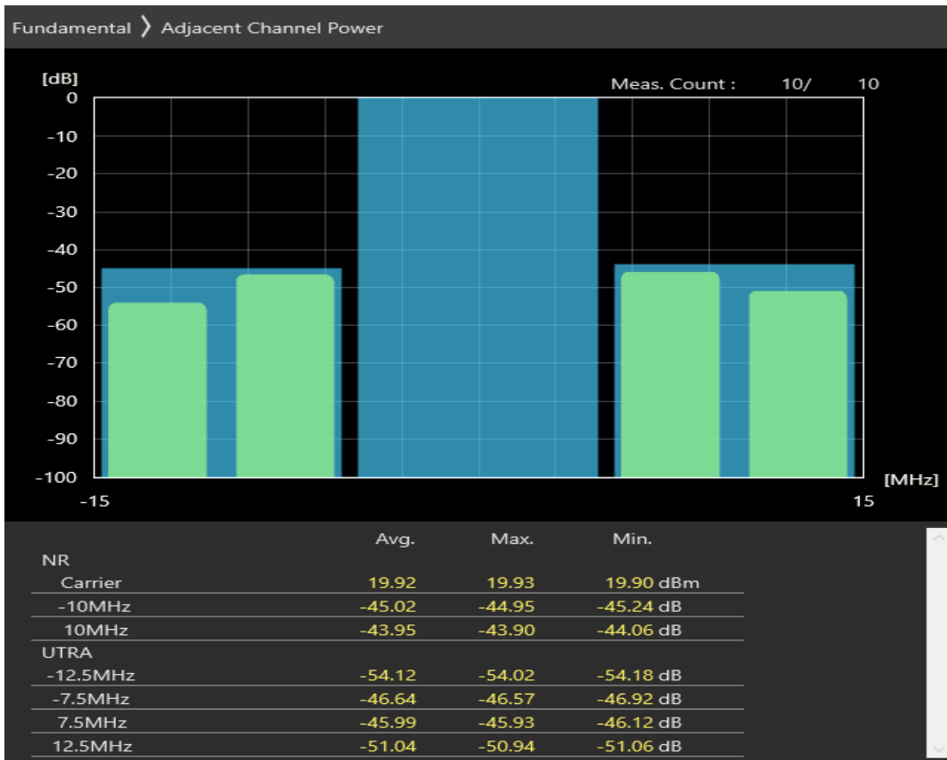
n20 SCS=30kHz DFT_BPSK BW=10MHz Channel=171400 RB=12@6
