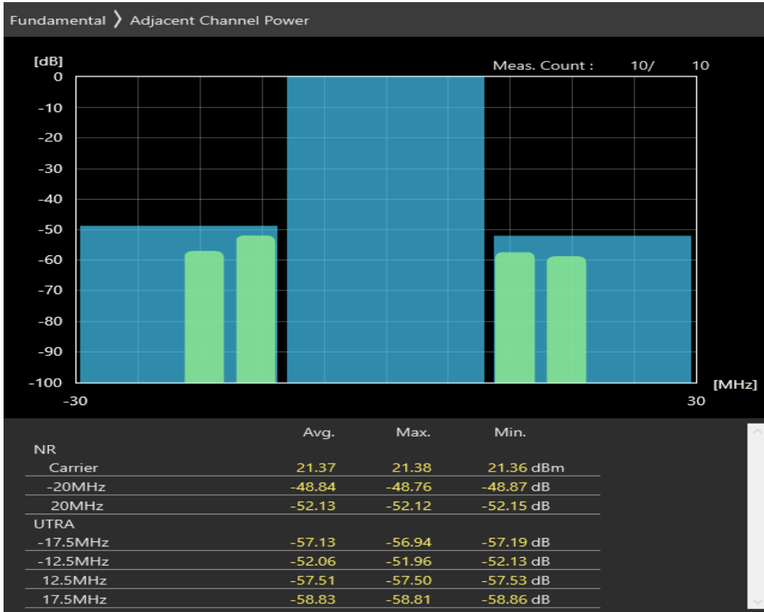
n38 SCS=30kHz CP_QAM16 BW=20MHz Channel=516000 RB=51@0
