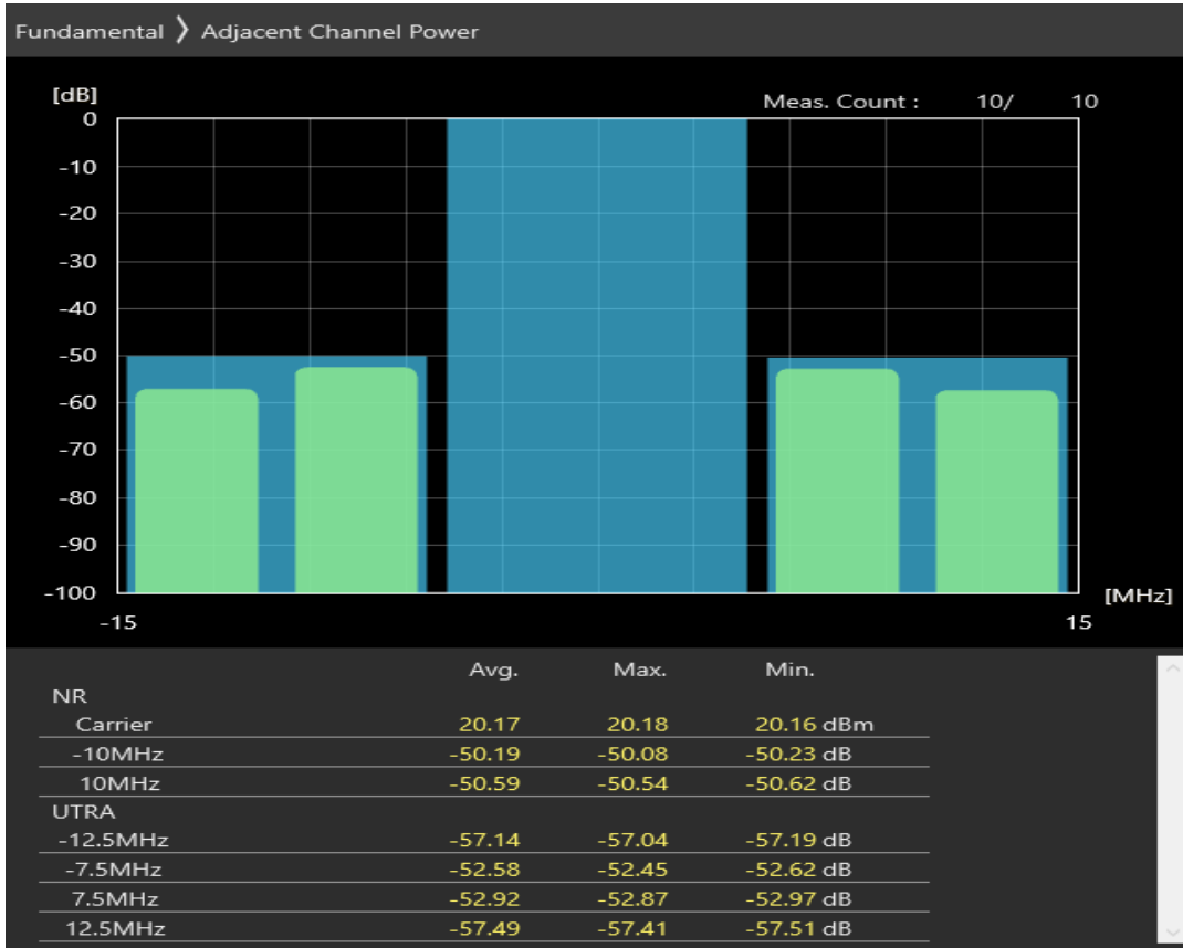
n77 SCS=30kHz CP_QAM16 BW=10MHz Channel=679666 RB=1@23
