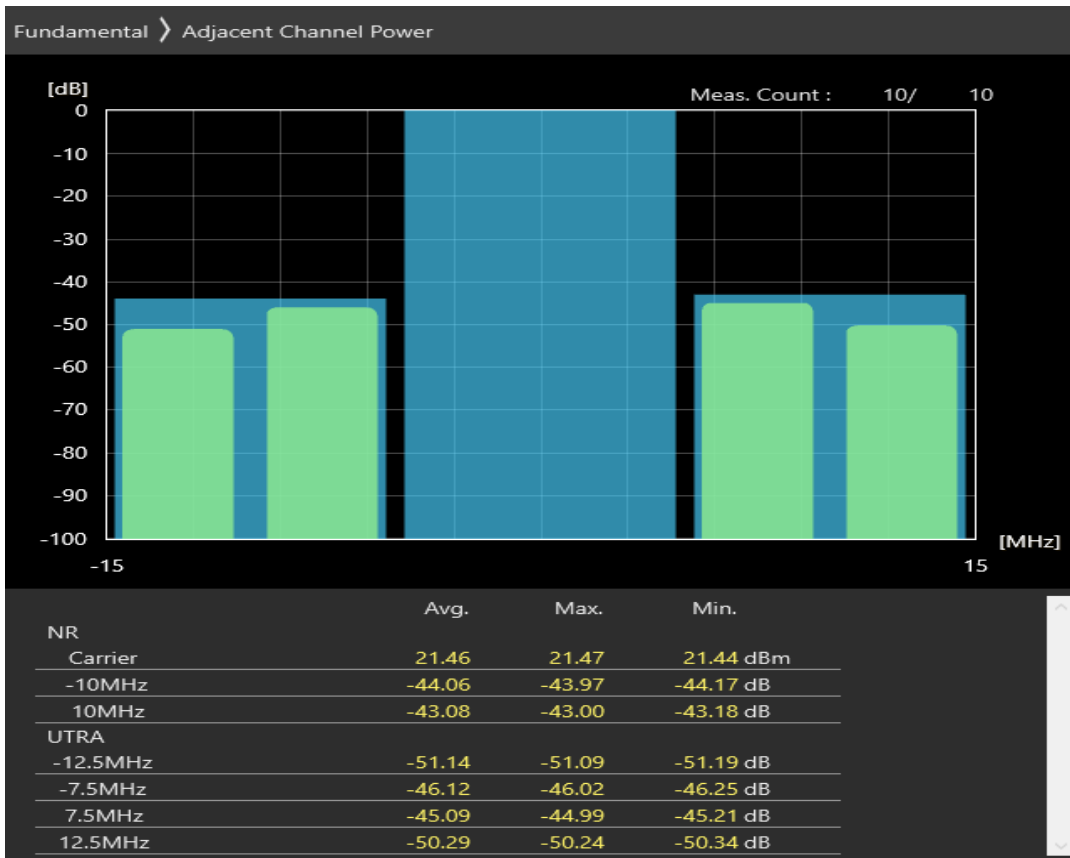
n3 SCS=30kHz CP_QPSK BW=10MHz Channel=343000 RB=12@6
