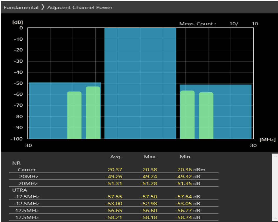
n20 SCS=30kHz CP_QAM16 BW=20MHz Channel=168400 RB=25@12
