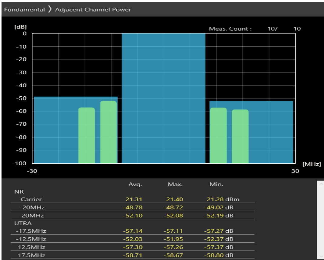
n38 SCS=30kHz CP_QAM64 BW=20MHz Channel=516000 RB=1@0
