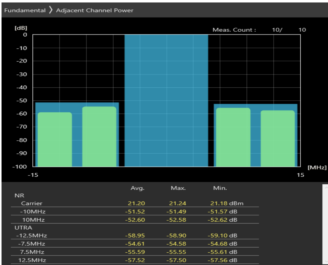
n28 SCS=30kHz DFT_QAM64 BW=10MHz Channel=141600 RB=24@0
