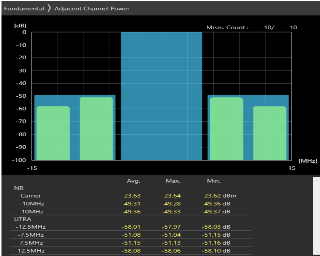
n77 SCS=30kHz DFT_QPSK BW=10MHz Channel=620334 RB=1@0
