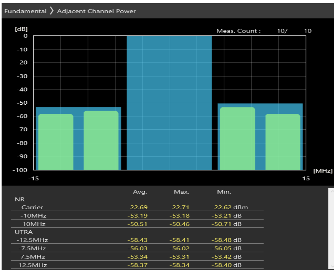
n77 SCS=30kHz DFT_QAM16 BW=10MHz Channel=679666 RB=24@0
