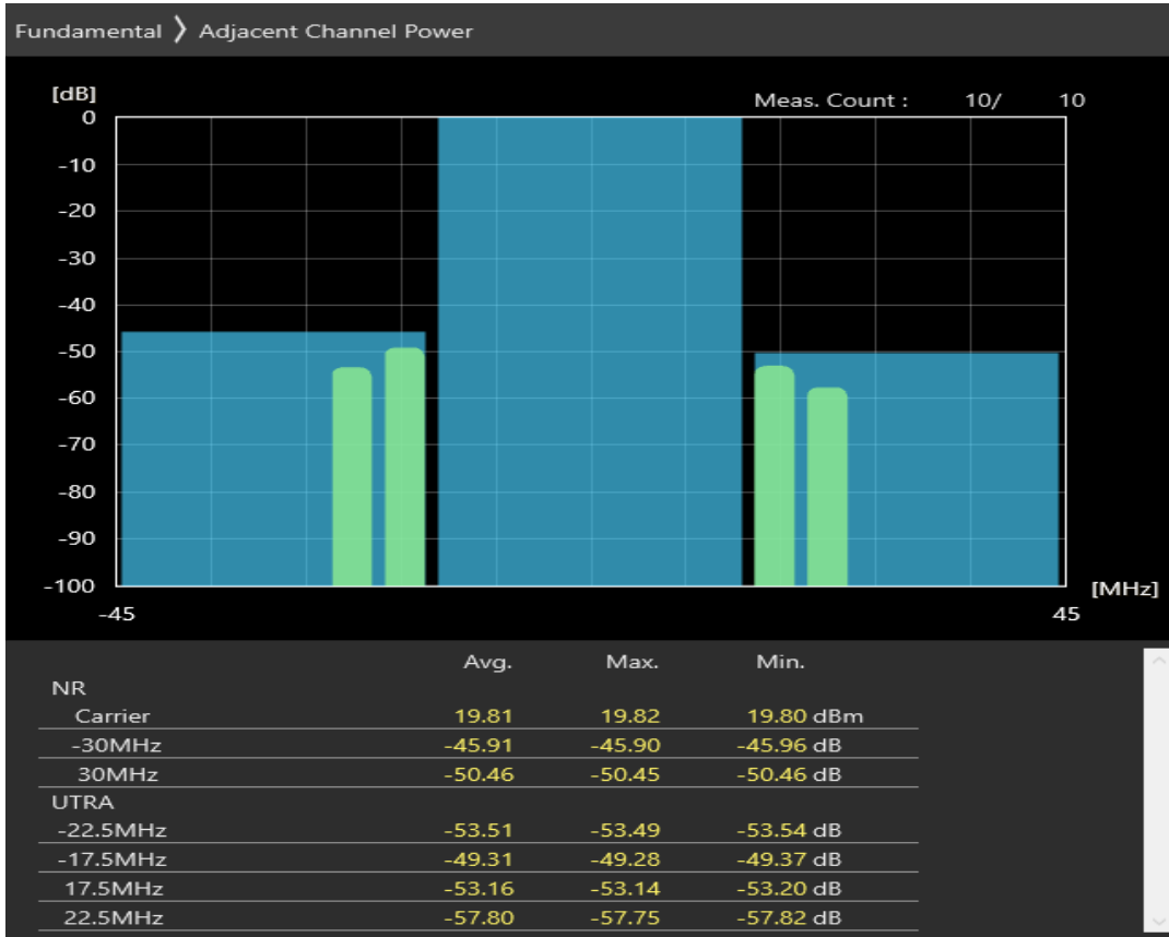
n3 SCS=30kHz DFT_BPSK BW=30MHz Channel=354000 RB=1@77
