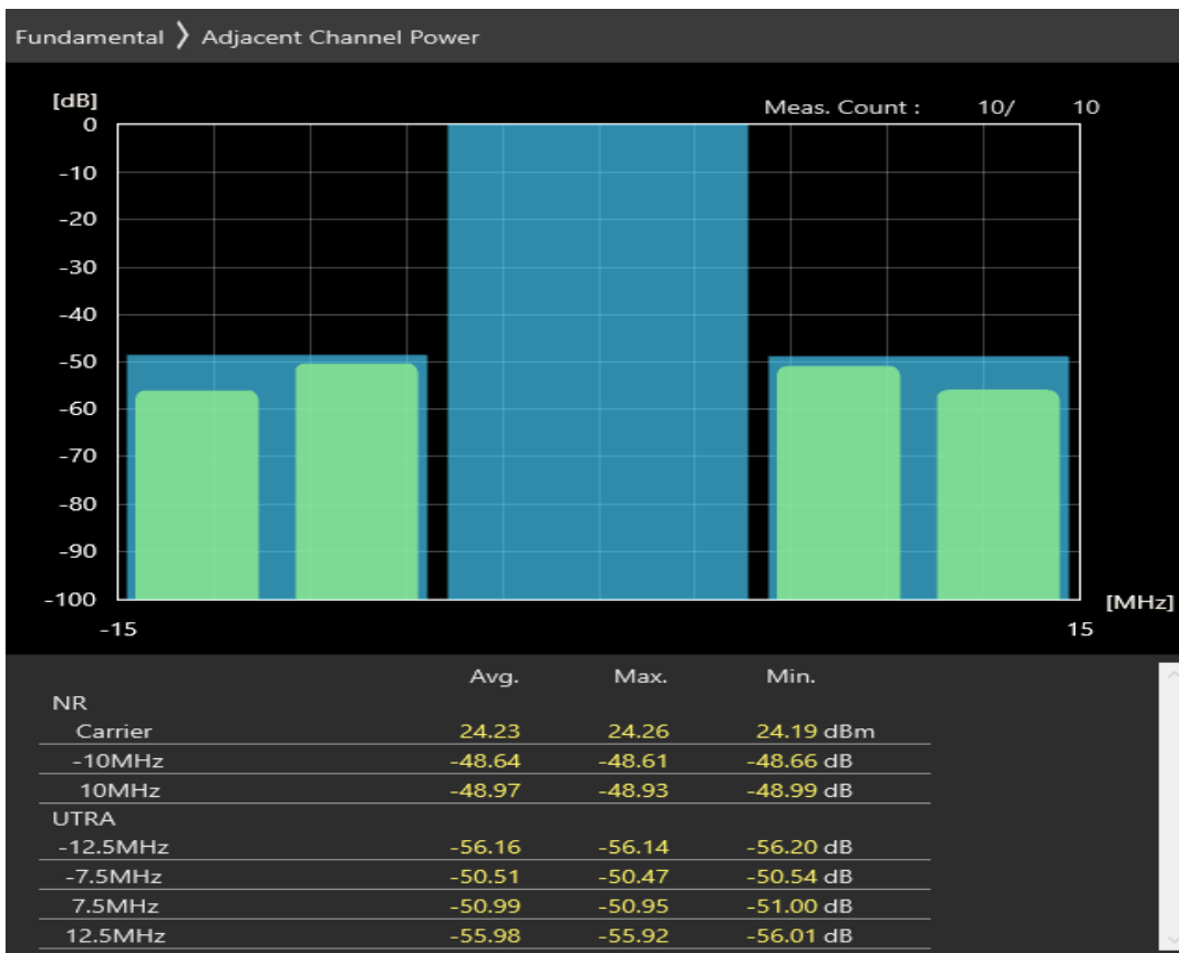
n78 SCS=30kHz DFT_BPSK BW=10MHz Channel=653000 RB=1@23
