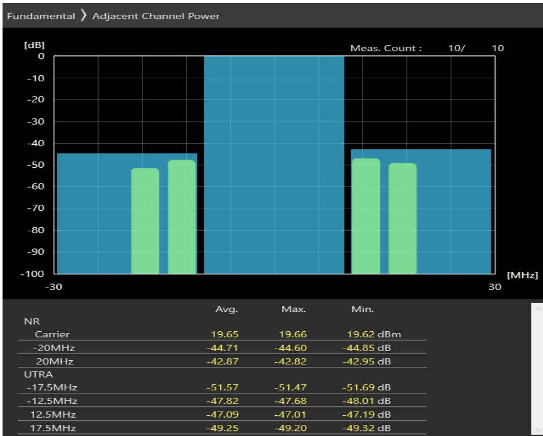
n1 SCS=30kHz DFT_BPSK BW=20MHz Channel=394000 RB=1@50
