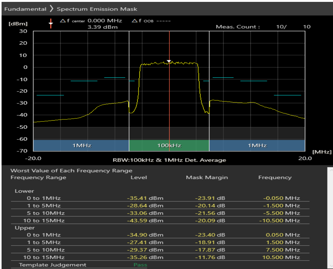
n28 SCS=30kHz DFT_QAM16 BW=10MHz Channel=141600 RB=1@0
