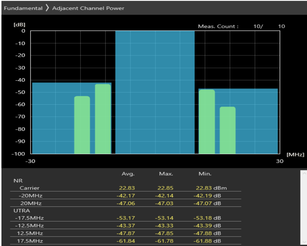
n28 SCS=30kHz DFT_QAM16 BW=20MHz Channel=147600 RB=1@50
