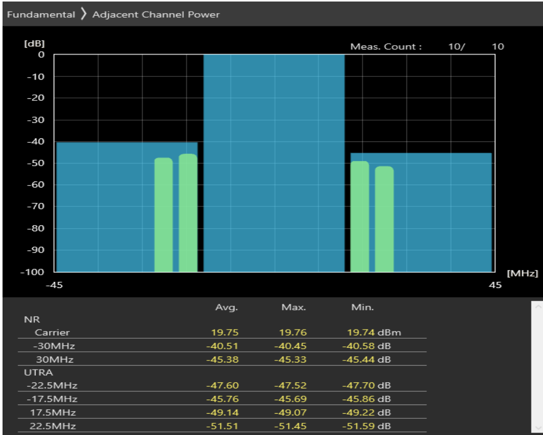
n3 SCS=30kHz DFT_QAM64 BW=30MHz Channel=354000 RB=1@77
