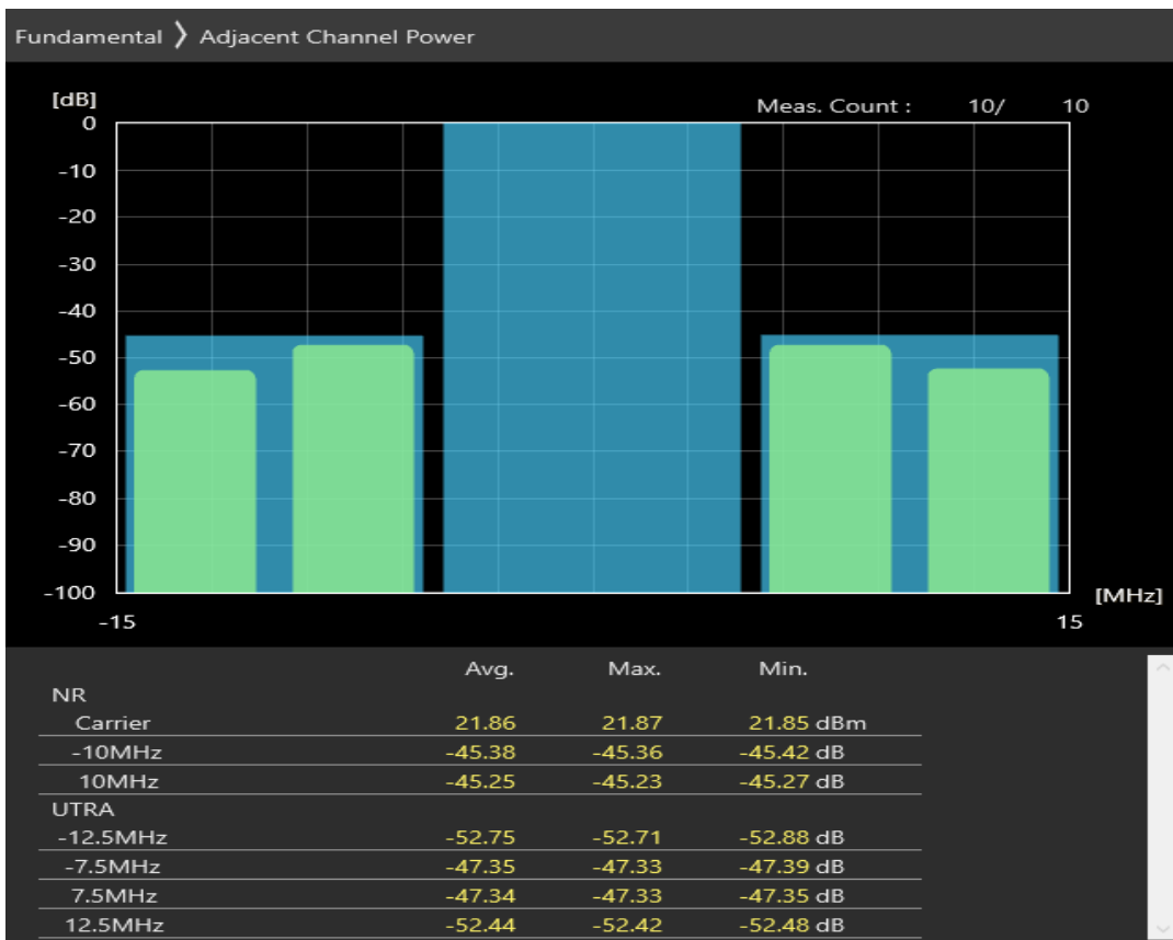
n78 SCS=30kHz CP_QAM16 BW=10MHz Channel=653000 RB=12@6
