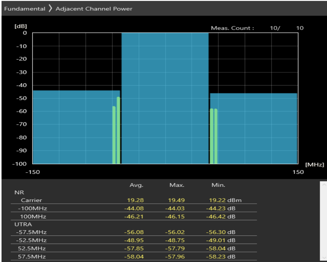
n77 SCS=30kHz CP_QAM64 BW=100MHz Channel=623334 RB=273@0
