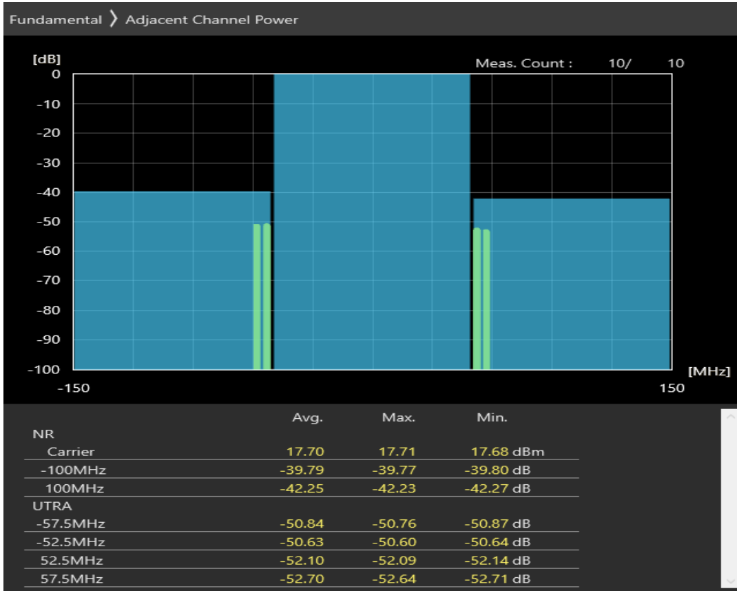
n77 SCS=30kHz DFT_QPSK BW=100MHz Channel=676666 RB=135@67
