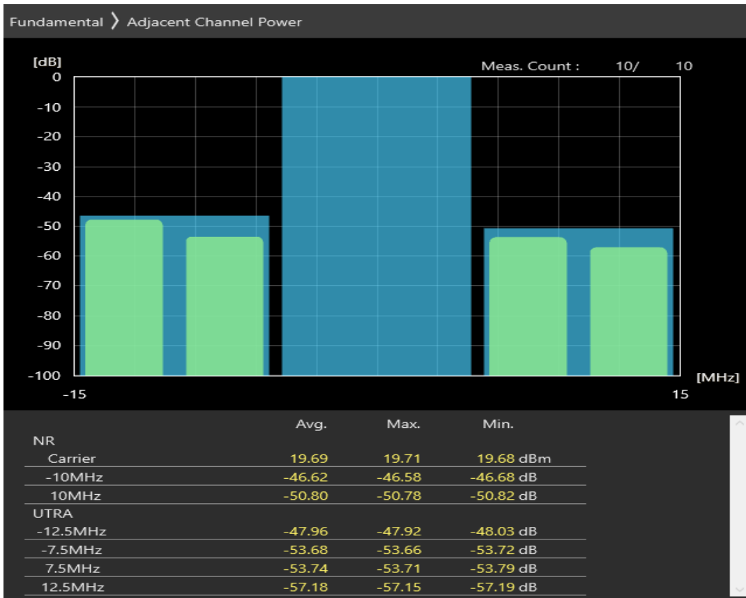
n3 SCS=30kHz CP_QAM64 BW=10MHz Channel=356000 RB=24@0
