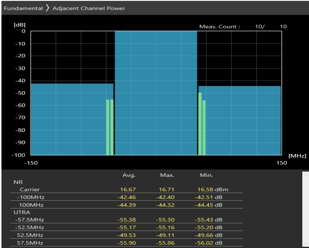
n77 SCS=30kHz DFT_QPSK BW=100MHz Channel=676666 RB=270@0
