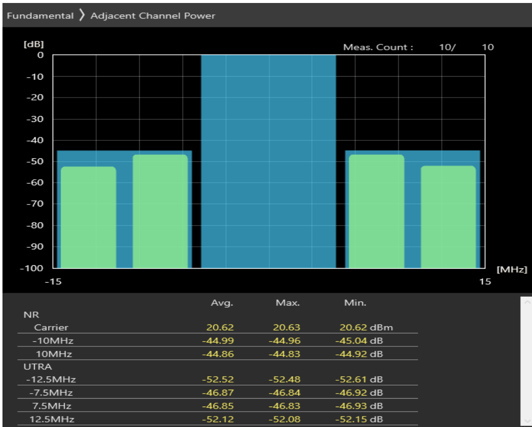
n78 SCS=30kHz CP_QAM256 BW=10MHz Channel=647000 RB=1@0
