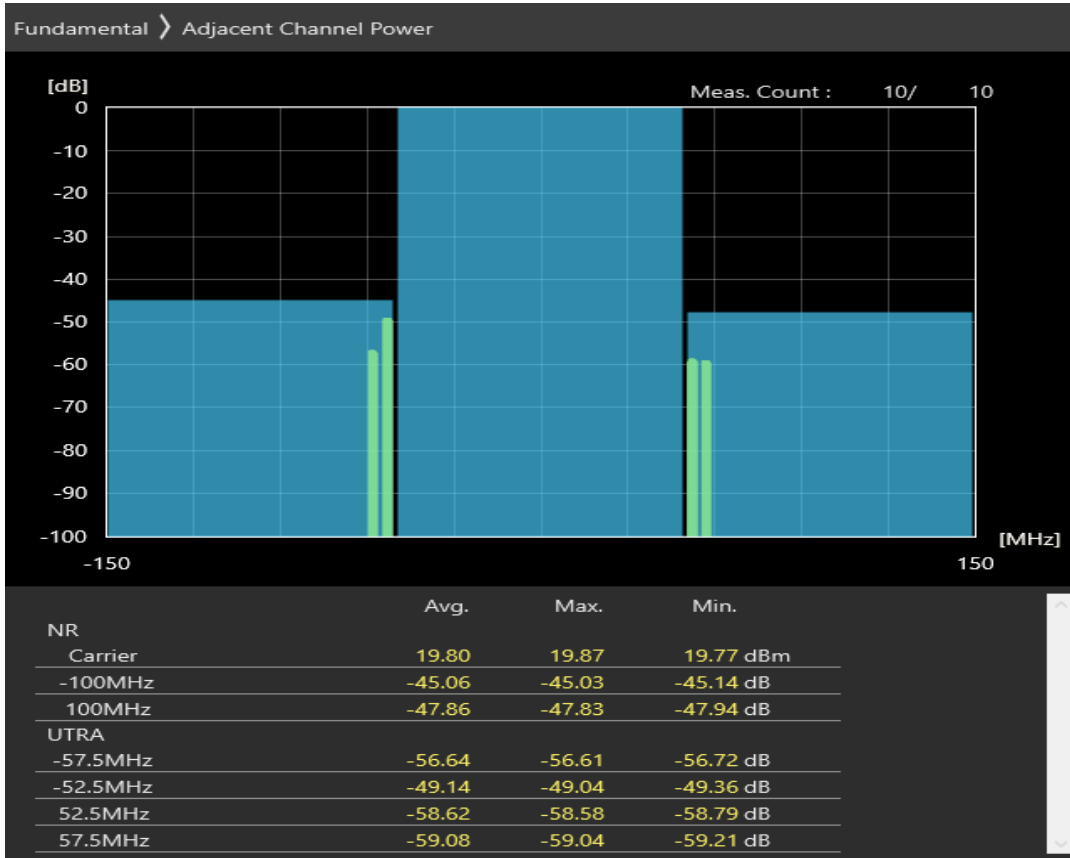
n78 SCS=30kHz CP_QAM64 BW=100MHz Channel=650000 RB=273@0
