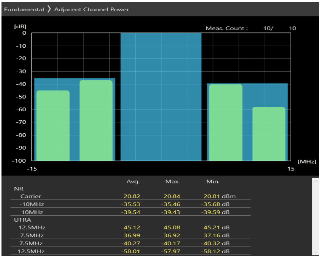
n28 SCS=30kHz CP_QAM16 BW=10MHz Channel=148600 RB=12@6
