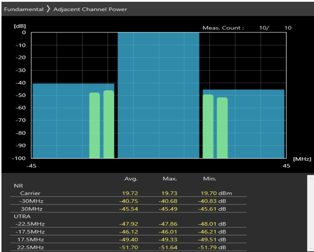
n3 SCS=30kHz DFT_QAM16 BW=30MHz Channel=354000 RB=36@18
