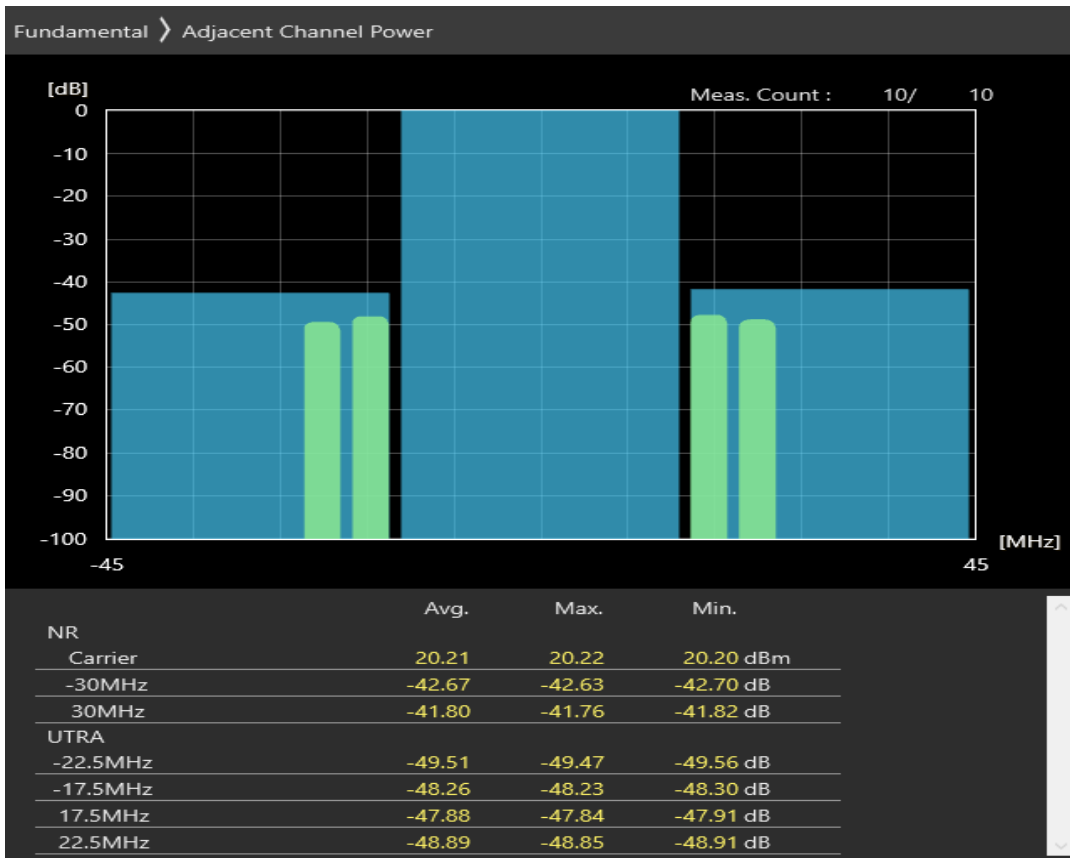
n3 SCS=30kHz DFT_QPSK BW=30MHz Channel=345000 RB=36@18
