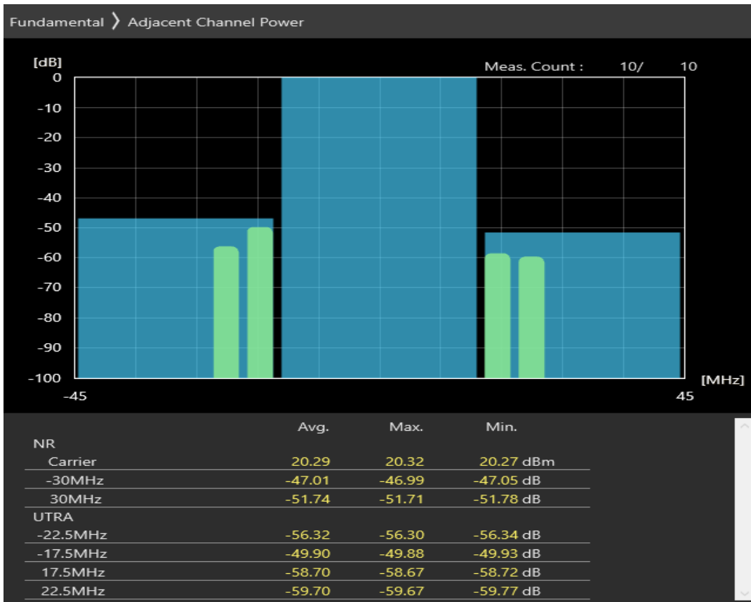
n3 SCS=30kHz CP_QAM16 BW=30MHz Channel=354000 RB=39@19
