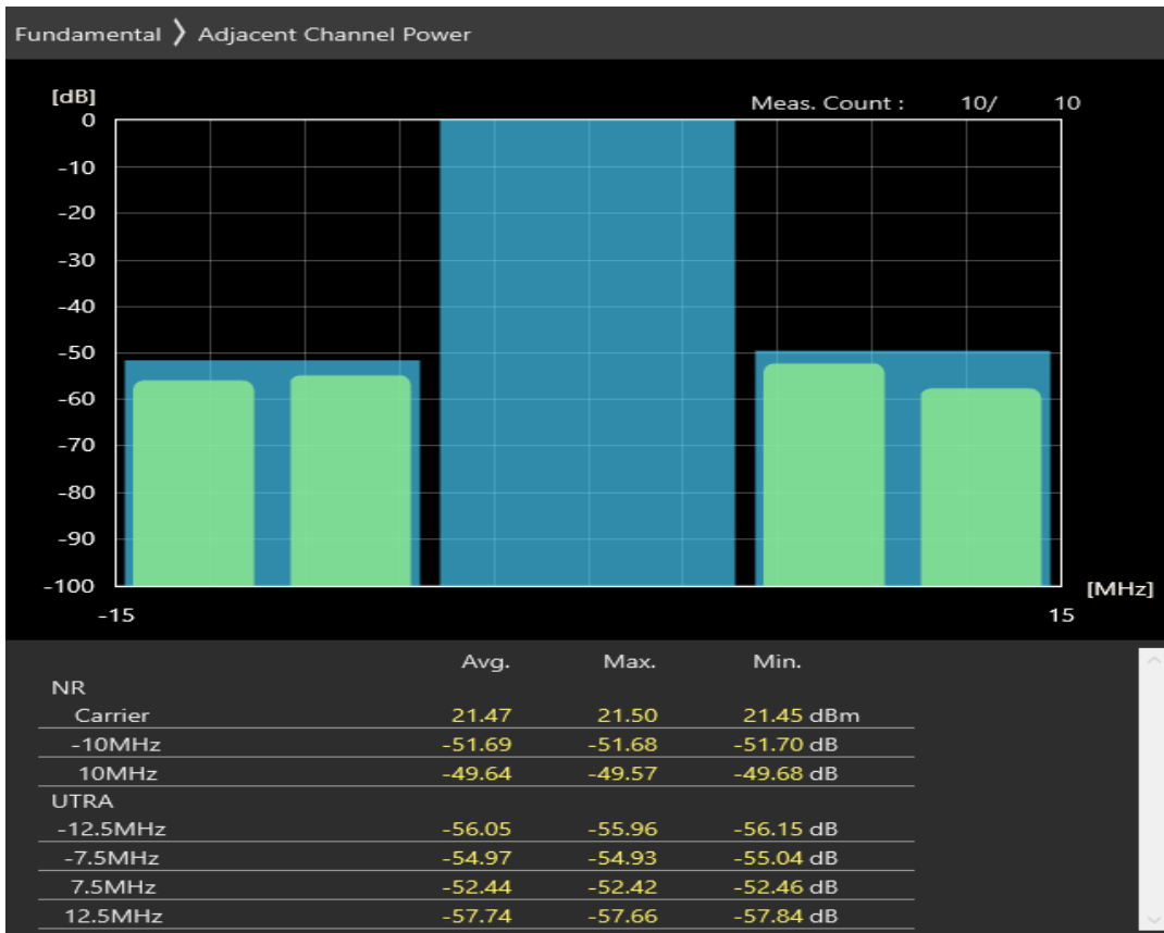
n78 SCS=30kHz CP_QAM256 BW=10MHz Channel=653000 RB=24@0
