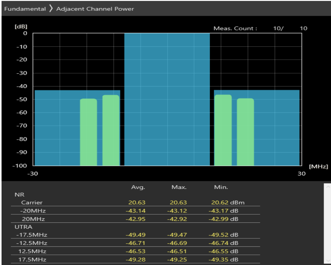
n38 SCS=30kHz DFT_QAM256 BW=20MHz Channel=522000 RB=1@50
