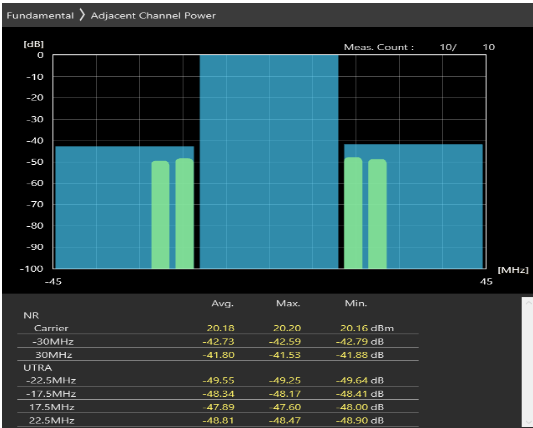
n3 SCS=30kHz DFT_QAM256 BW=30MHz Channel=345000 RB=1@0
