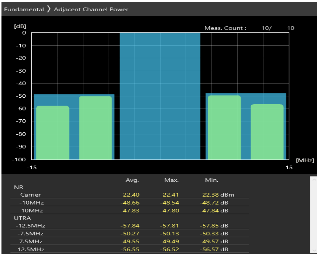
n20 SCS=30kHz DFT_QAM16 BW=10MHz Channel=167400 RB=1@0
