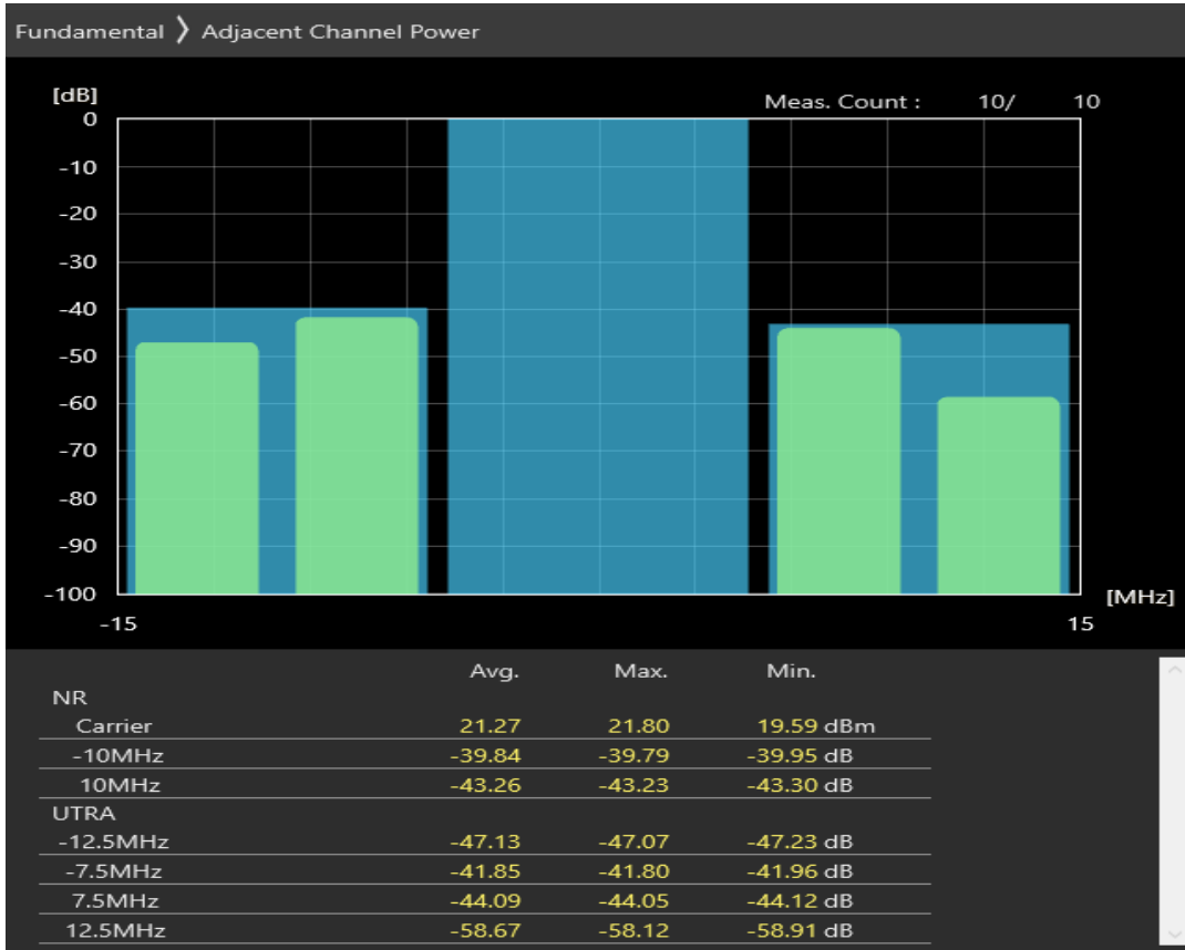
n28 SCS=30kHz DFT_QAM64 BW=10MHz Channel=148600 RB=1@23
