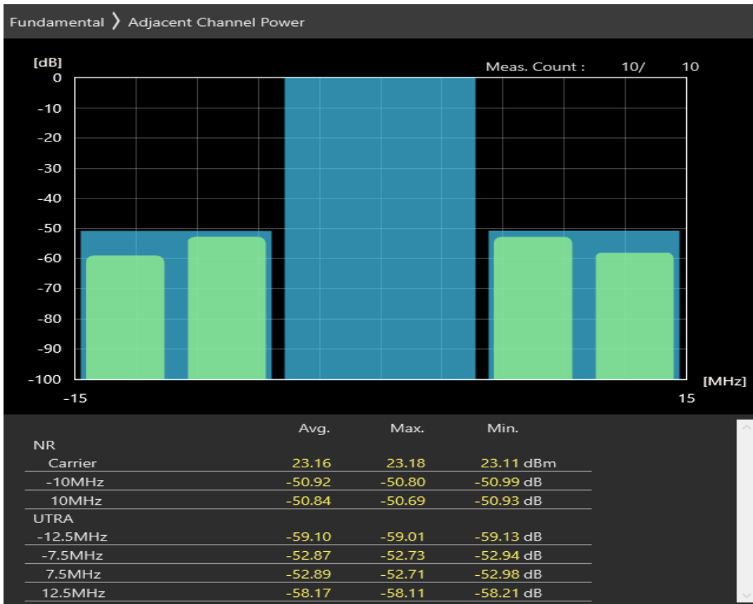
n1 SCS=30kHz DFT_BPSK BW=10MHz Channel=385000 RB=1@0
