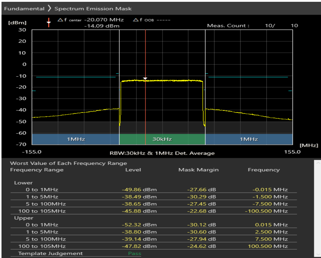
n78 SCS=30kHz DFT_QPSK BW=100MHz Channel=650000 RB=1@0
