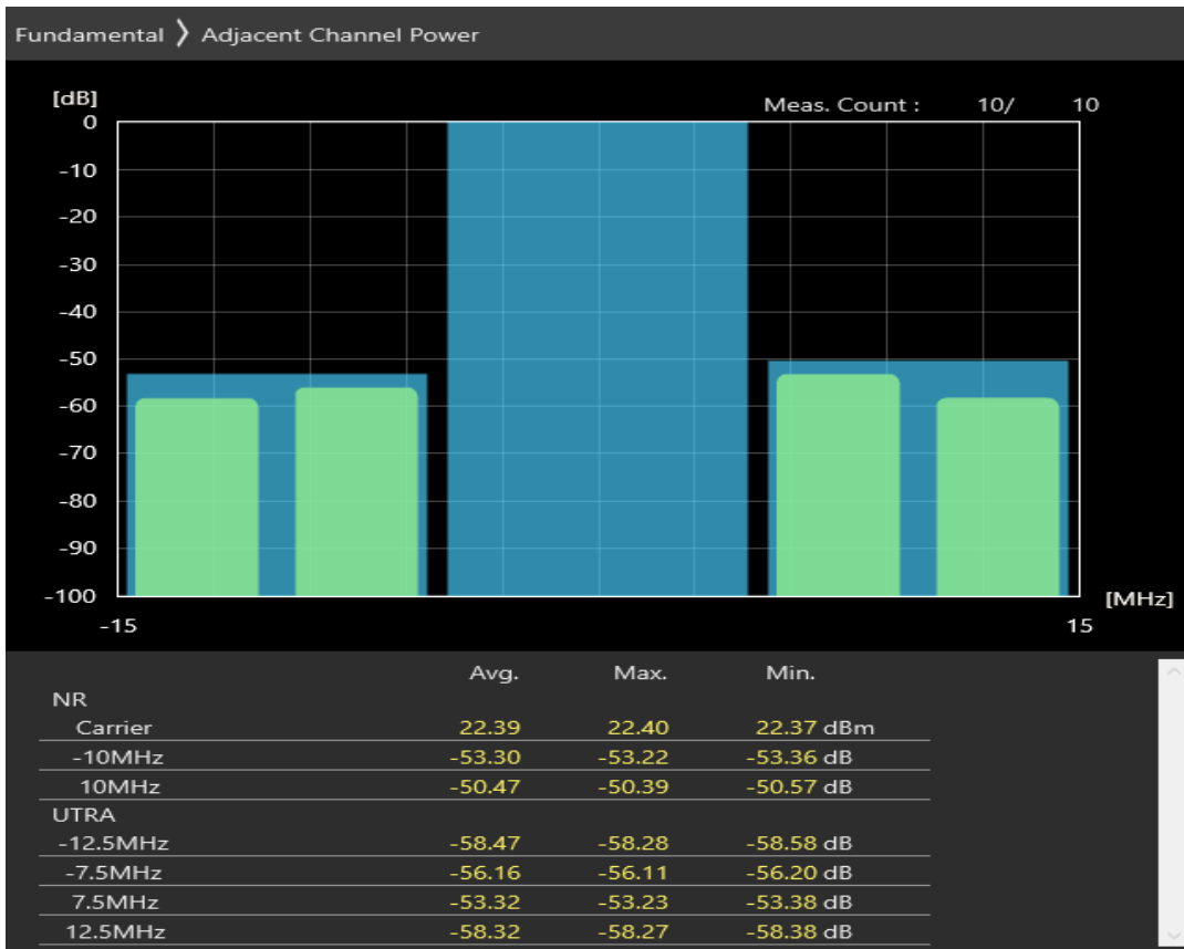
n78 SCS=30kHz DFT_QAM256 BW=10MHz Channel=653000 RB=24@0
