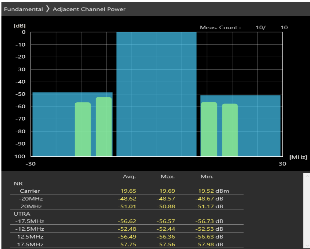
n1 SCS=30kHz DFT_BPSK BW=20MHz Channel=386000 RB=25@12
