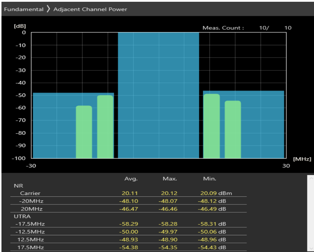
n28 SCS=30kHz DFT_QAM16 BW=20MHz Channel=142600 RB=1@0
