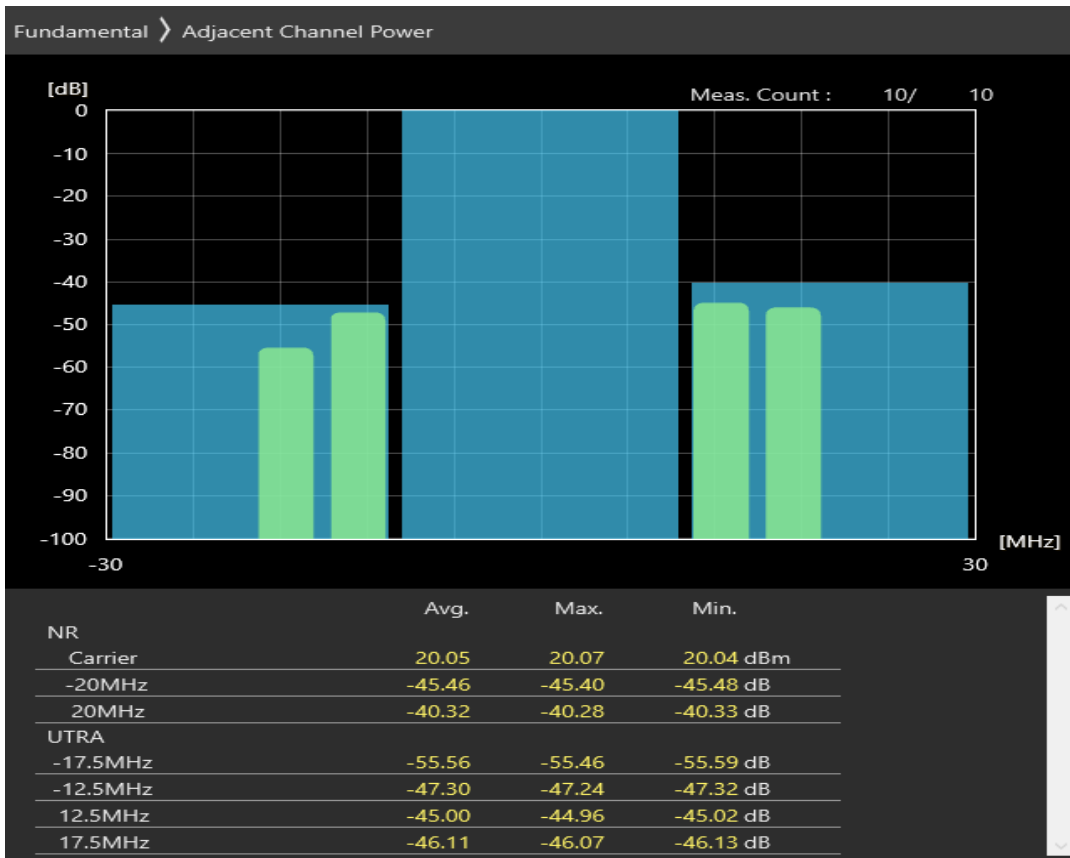
n28 SCS=30kHz DFT_QAM64 BW=20MHz Channel=142600 RB=1@0
