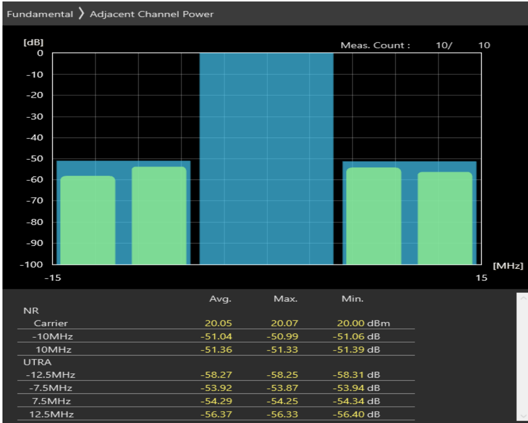
n28 SCS=30kHz CP_QAM64 BW=10MHz Channel=141600 RB=24@0
