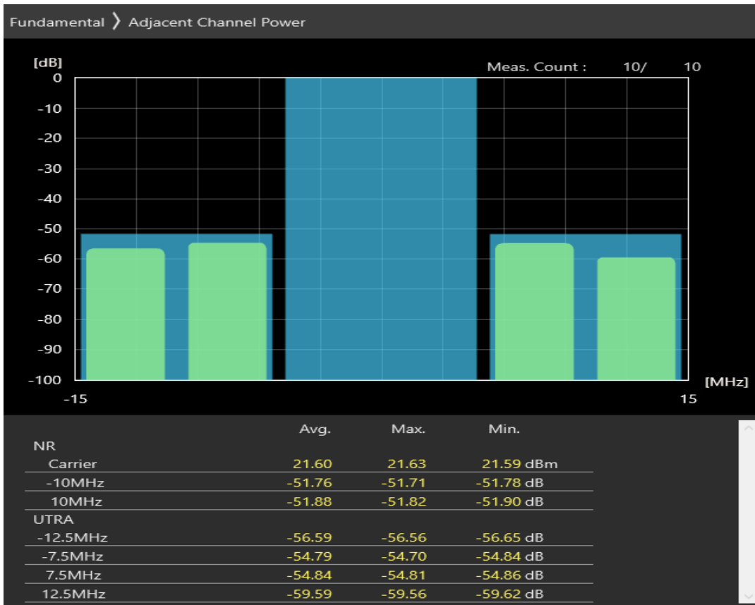
n28 SCS=30kHz DFT_QAM16 BW=10MHz Channel=148600 RB=24@0
