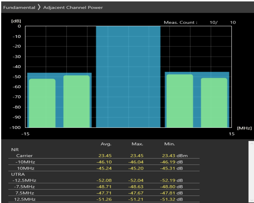
n3 SCS=30kHz DFT_QPSK BW=10MHz Channel=343000 RB=12@6
