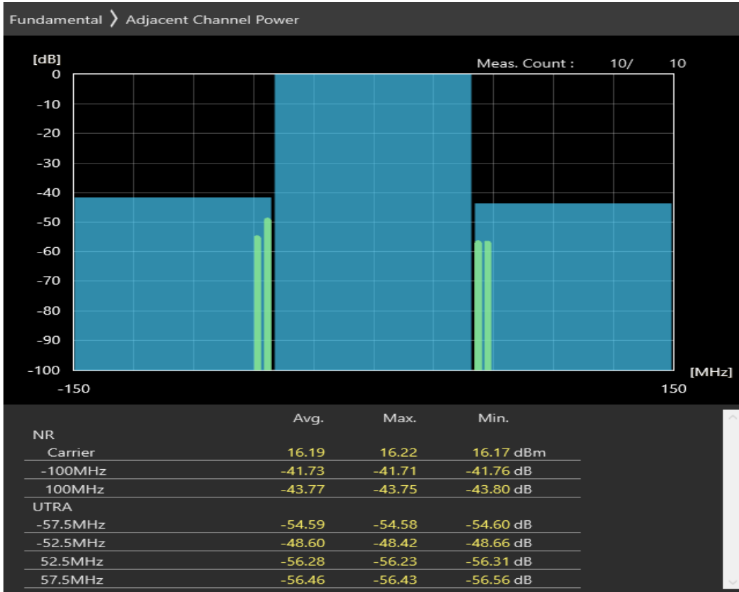
n77 SCS=30kHz DFT_QAM256 BW=100MHz Channel=623334 RB=270@0
