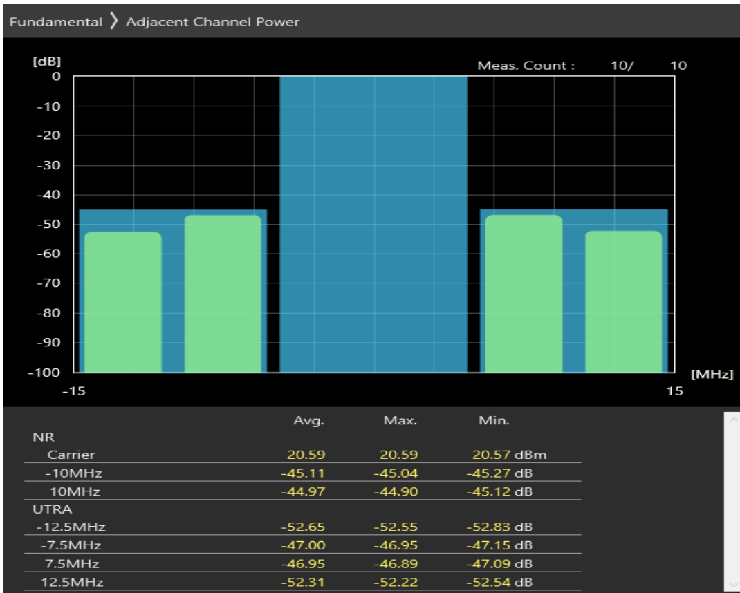
n78 SCS=30kHz DFT_BPSK BW=10MHz Channel=653000 RB=12@6
