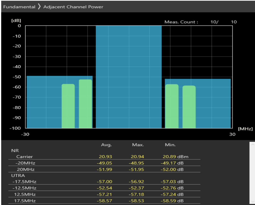
n38 SCS=30kHz CP_QAM64 BW=20MHz Channel=516000 RB=51@0
