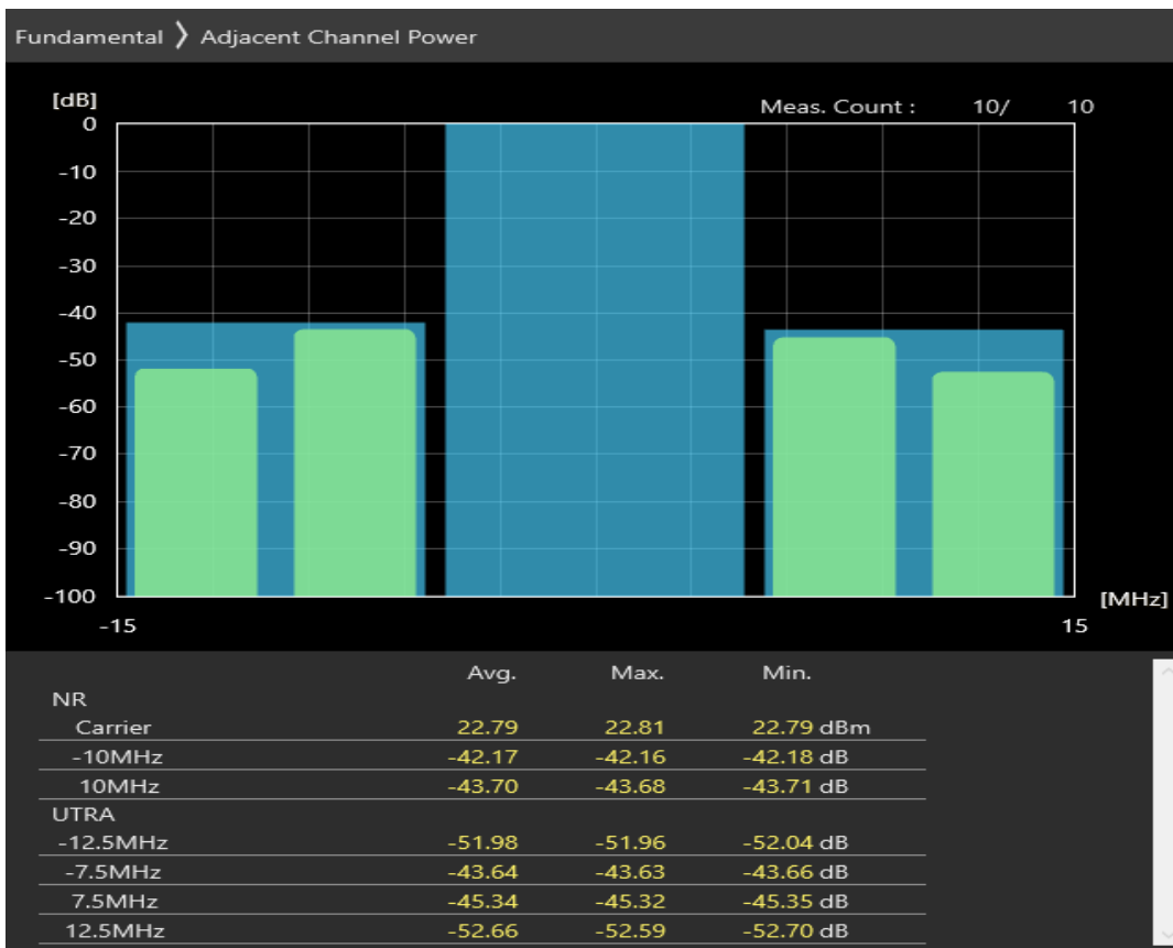
n77 SCS=30kHz DFT_QAM64 BW=10MHz Channel=679666 RB=1@23
