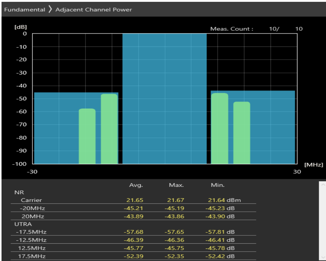
n28 SCS=30kHz CP_QAM16 BW=20MHz Channel=142600 RB=1@0
