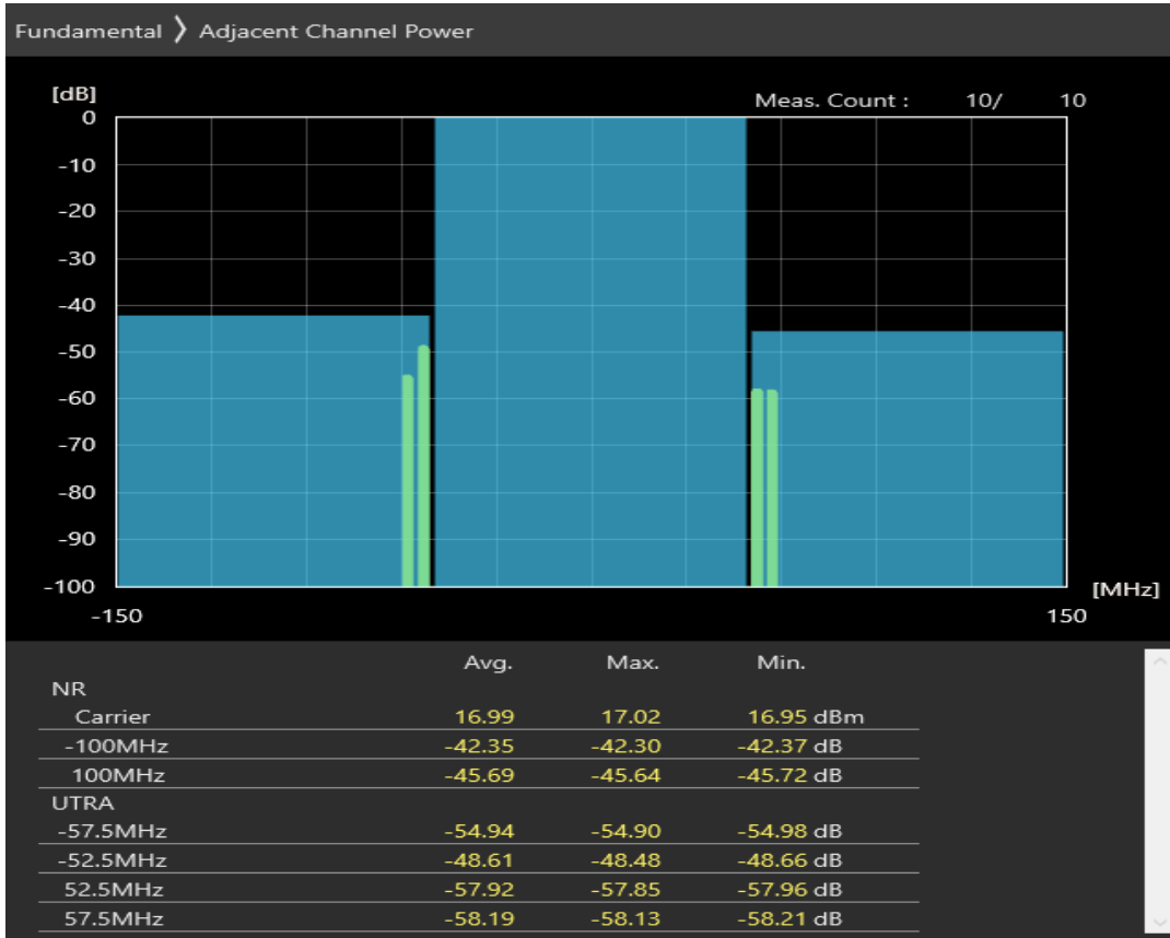
n78 SCS=30kHz DFT_BPSK BW=10MHz Channel=647000 RB=12@6
