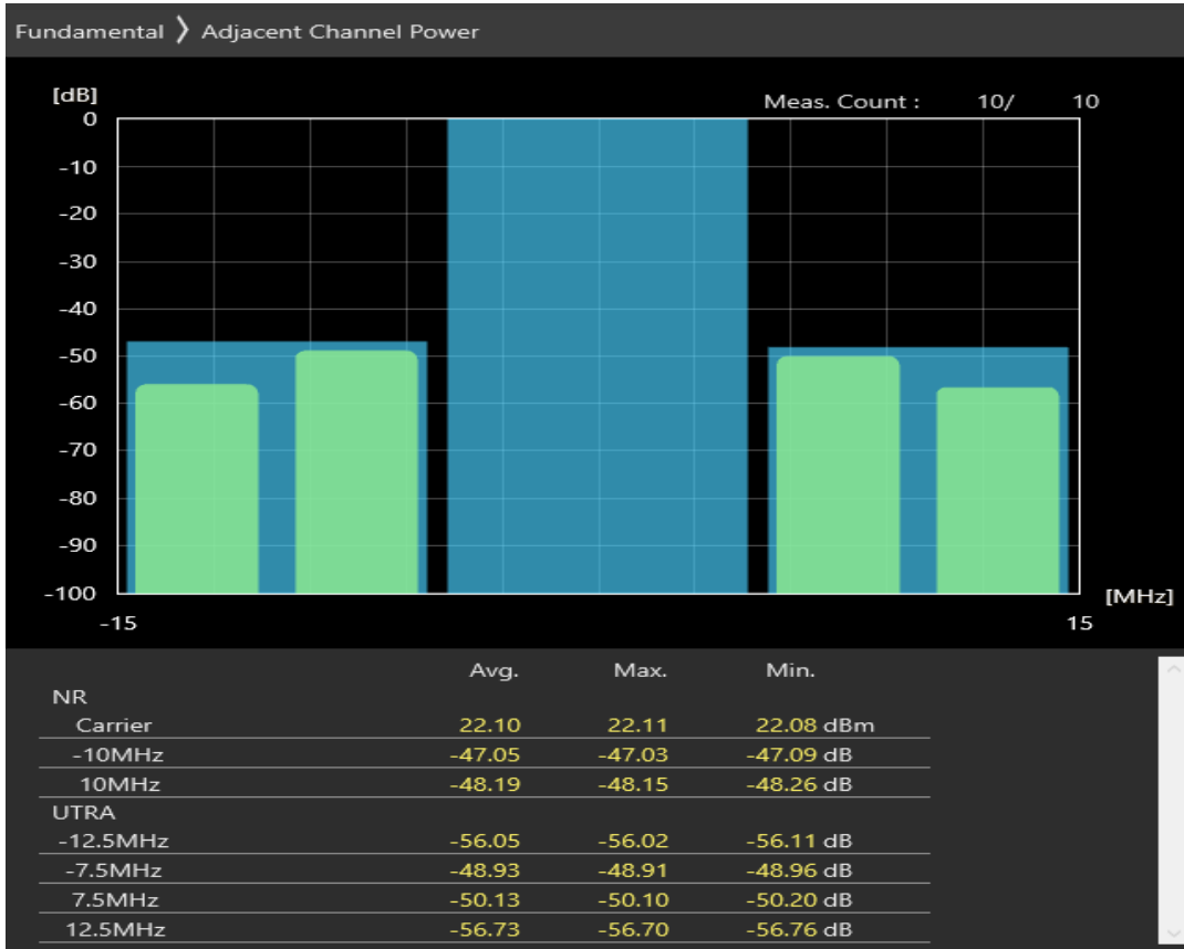
n1 SCS=30kHz DFT_QAM16 BW=10MHz Channel=395000 RB=1@23
