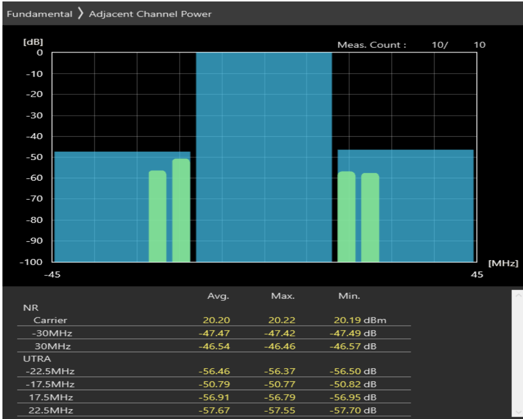
n3 SCS=30kHz DFT_QAM64 BW=30MHz Channel=345000 RB=75@0
