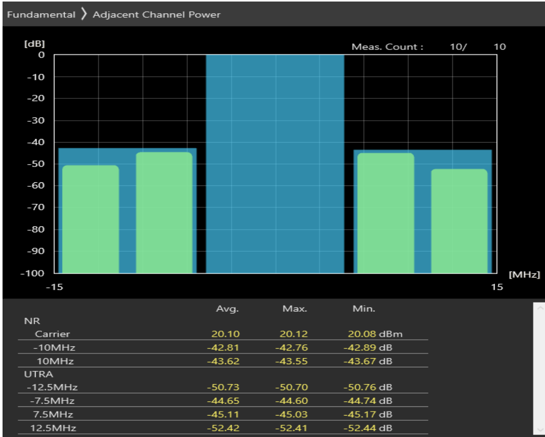
n20 SCS=30kHz CP_QAM256 BW=10MHz Channel=171400 RB=1@23
