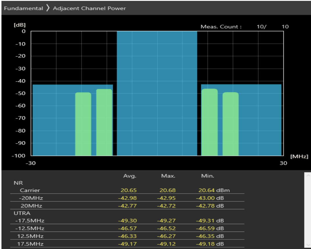
n38 SCS=30kHz DFT_QAM64 BW=20MHz Channel=522000 RB=1@50
