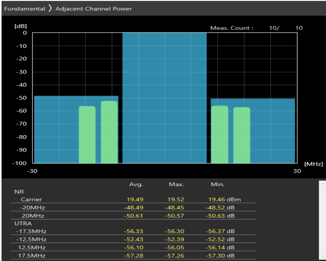
n1 SCS=30kHz CP_QAM256 BW=20MHz Channel=394000 RB=1@50
