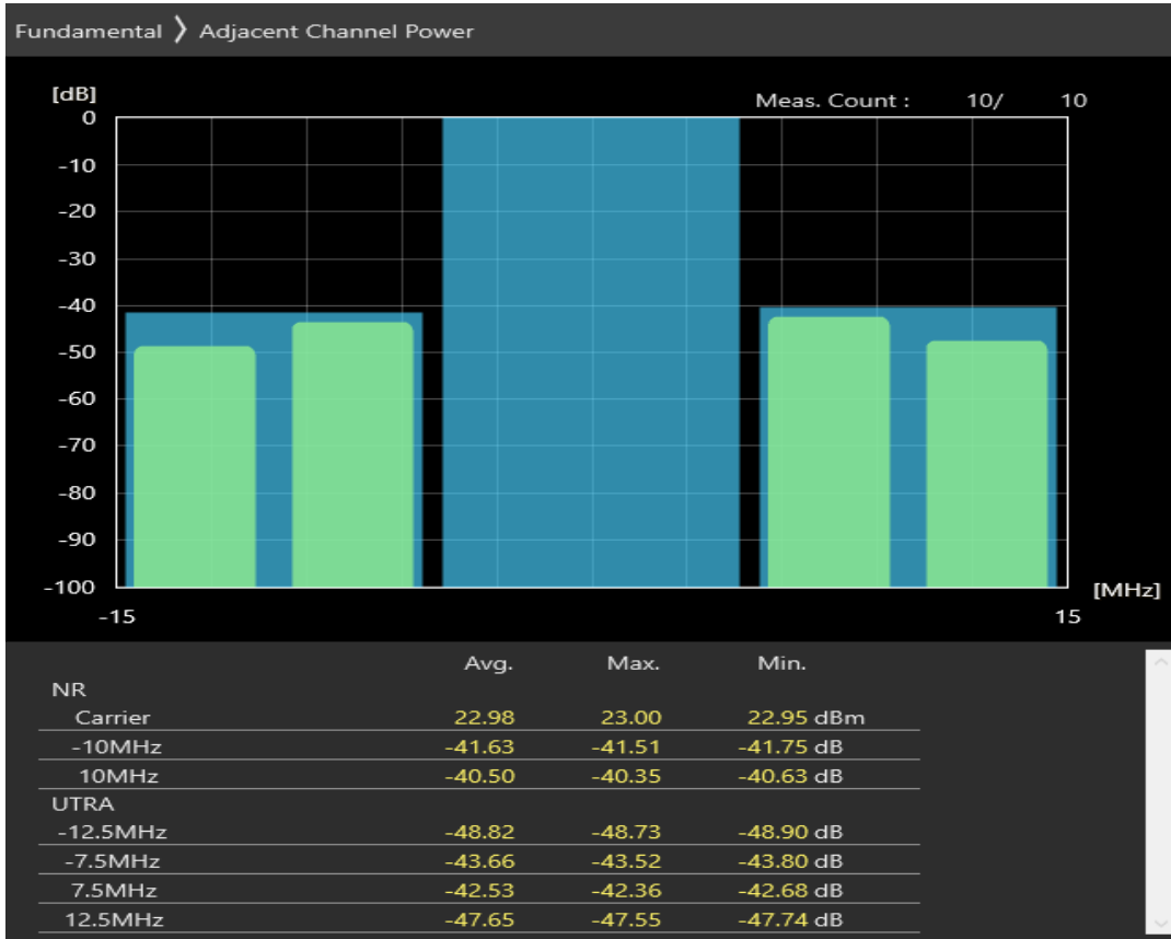
n3 SCS=30kHz DFT_QAM16 BW=10MHz Channel=343000 RB=12@6
