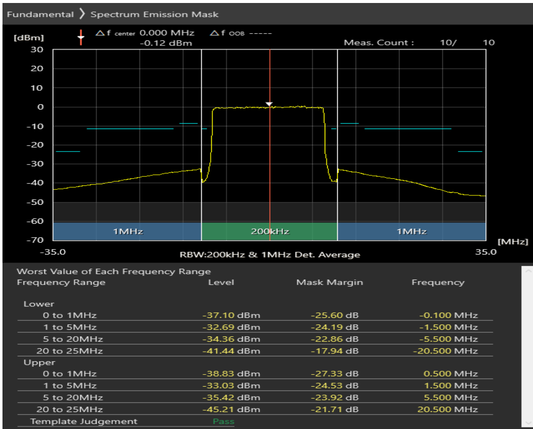
n1 SCS=30kHz DFT_QAM16 BW=20MHz Channel=394000 RB=1@50
