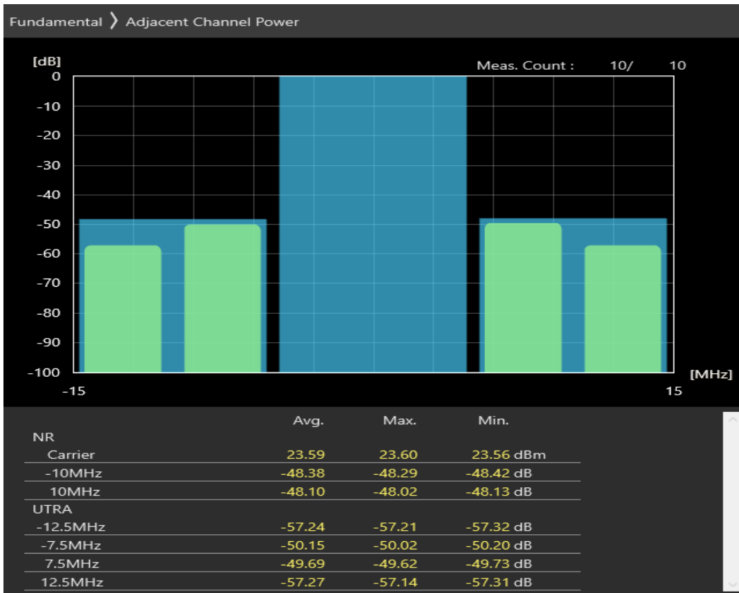
n38 SCS=30kHz DFT_QAM16 BW=10MHz Channel=515000 RB=1@0
