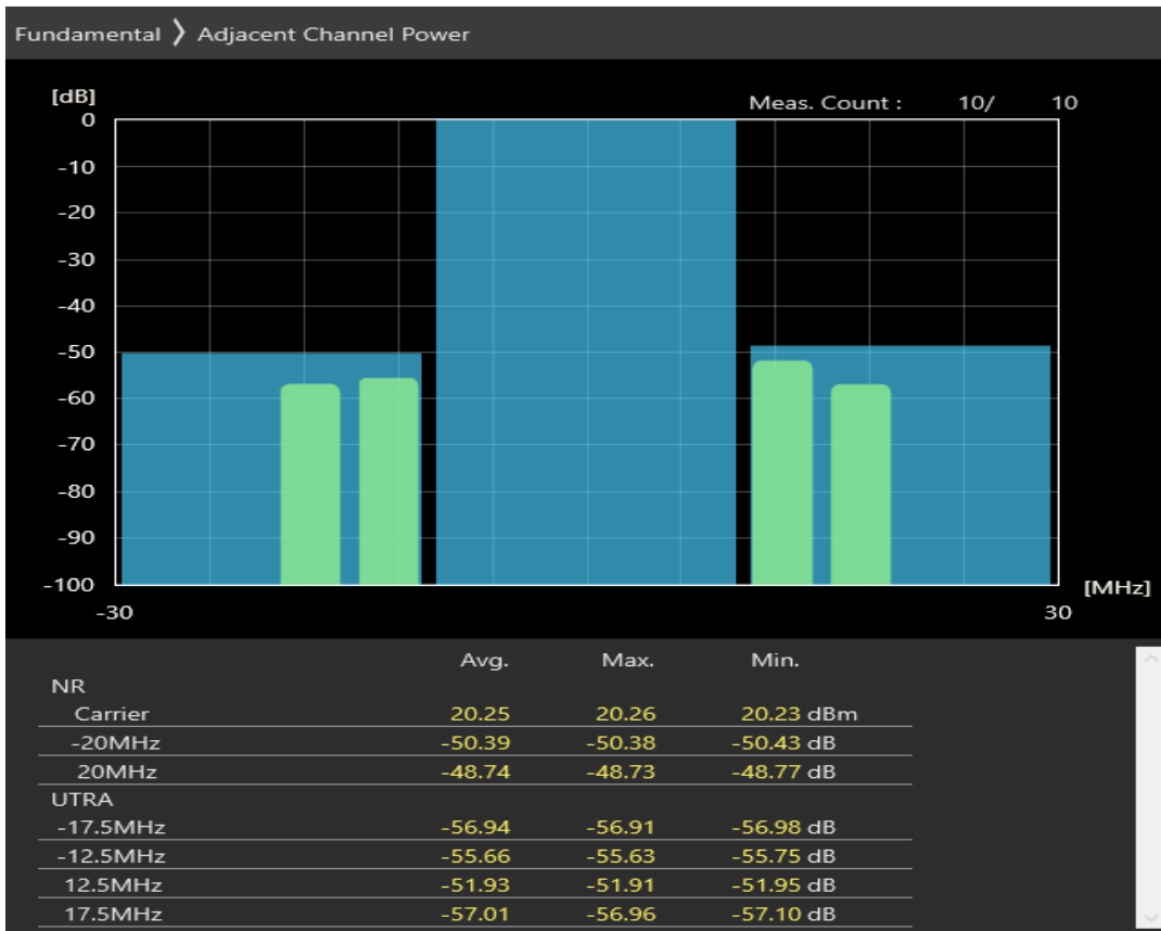
n20 SCS=30kHz CP_QAM16 BW=20MHz Channel=170400 RB=51@0
