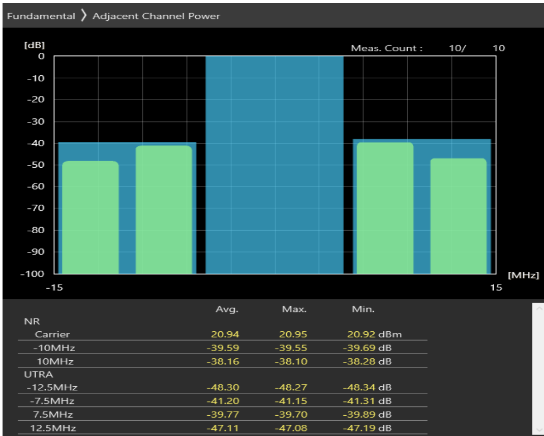
n3 SCS=30kHz CP_QAM64 BW=10MHz Channel=343000 RB=1@0
