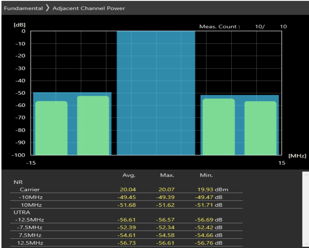
n77 SCS=30kHz CP_QAM64 BW=10MHz Channel=620334 RB=24@0
