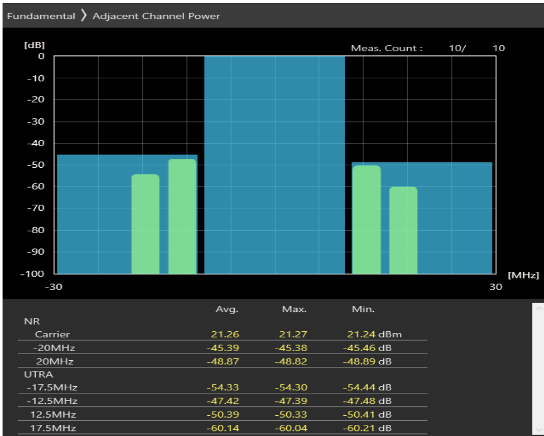
n8 SCS=30kHz CP_QAM16 BW=20MHz Channel=181000 RB=1@50
