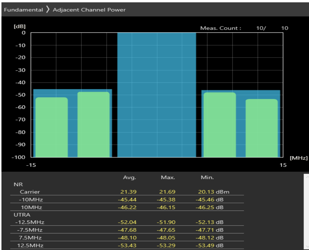
n20 SCS=30kHz DFT_QAM64 BW=10MHz Channel=171400 RB=1@23
