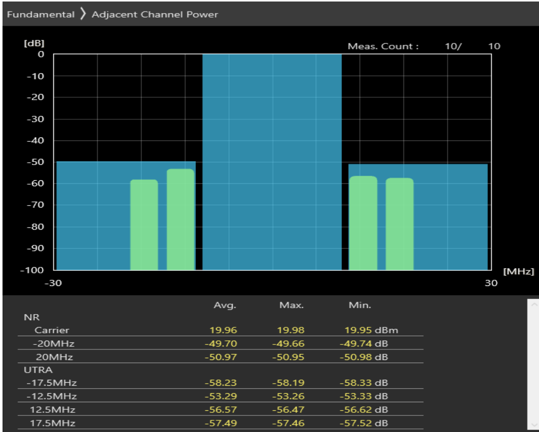
n28 SCS=30kHz CP_QAM256 BW=20MHz Channel=142600 RB=51@0
