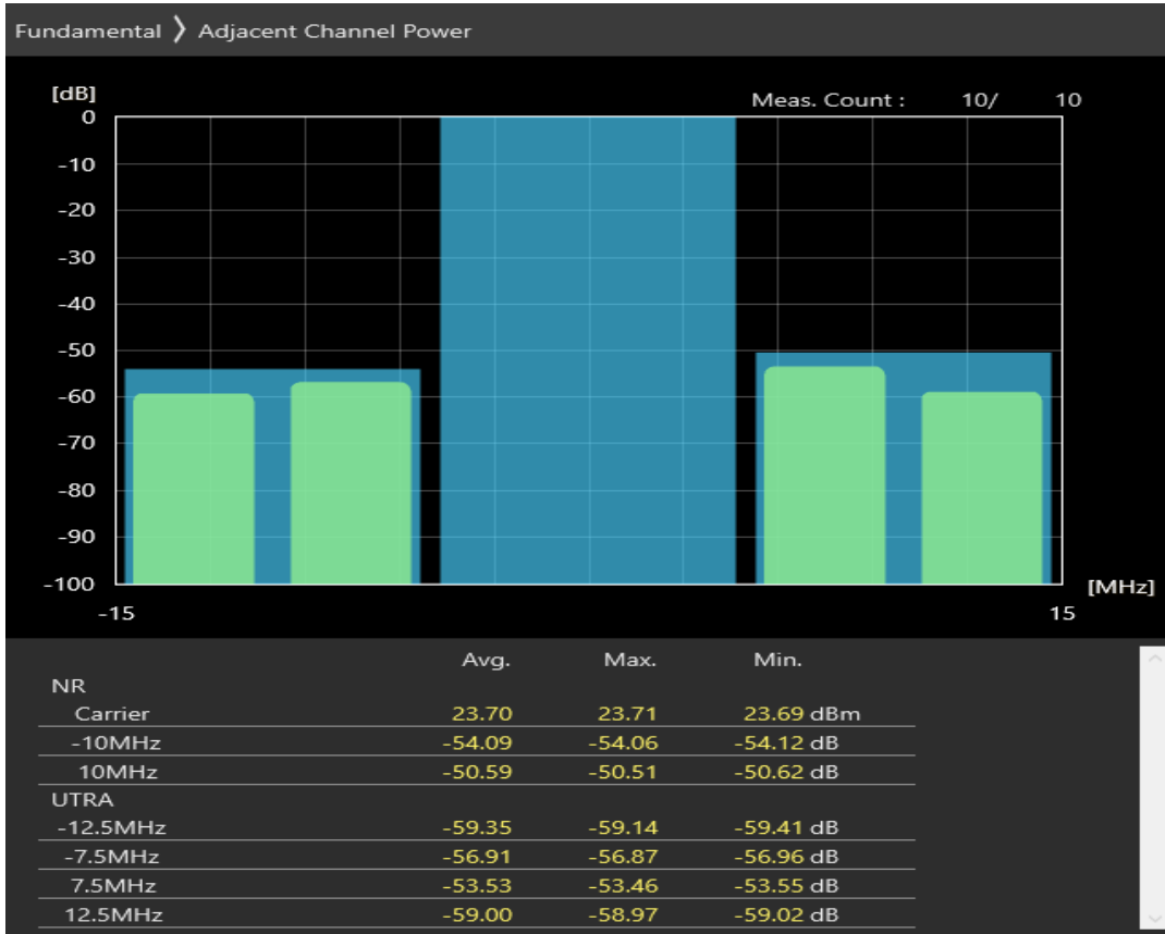
n78 SCS=30kHz DFT_QPSK BW=10MHz Channel=653000 RB=24@0
