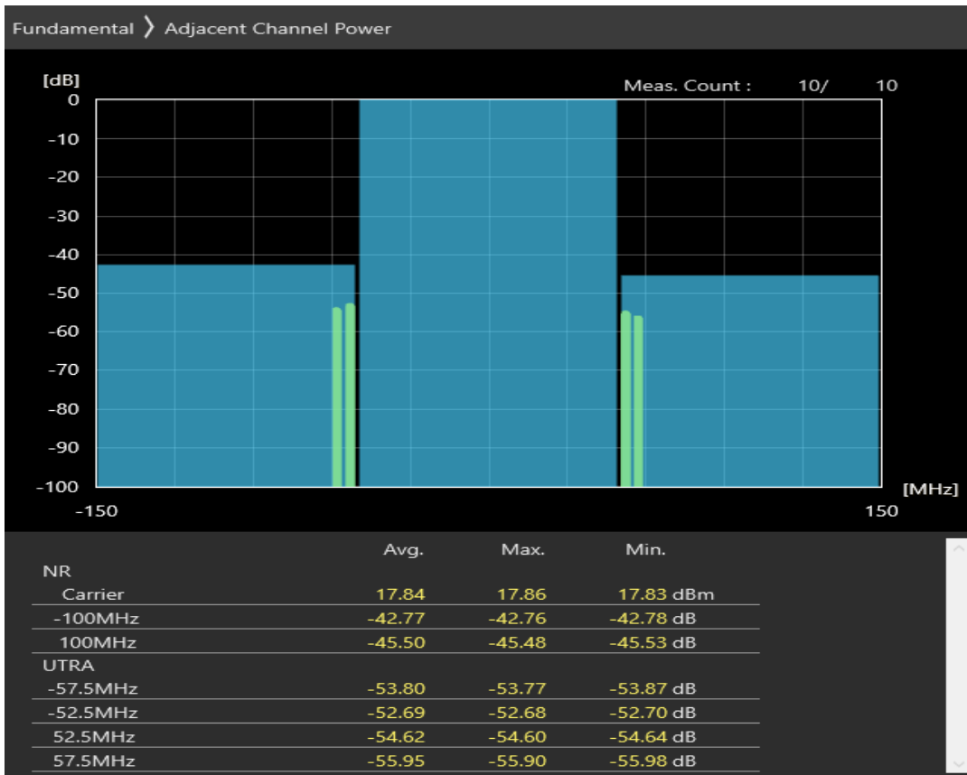
n77 SCS=30kHz DFT_QPSK BW=100MHz Channel=676666 RB=1@272
