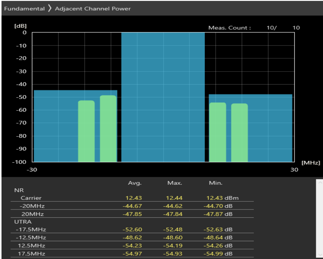
n28 SCS=30kHz CP_QAM256 BW=20MHz Channel=147600 RB=1@50
