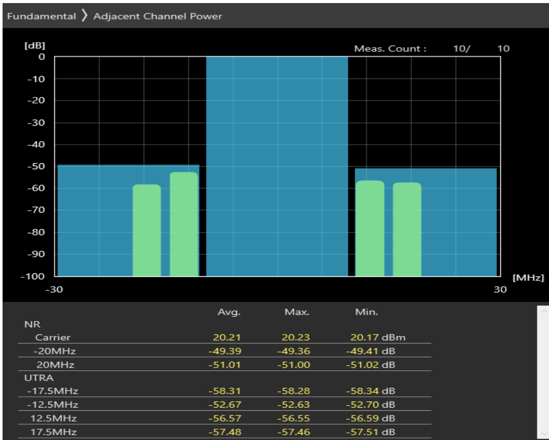
n28 SCS=30kHz CP_QAM64 BW=20MHz Channel=142600 RB=1@0
