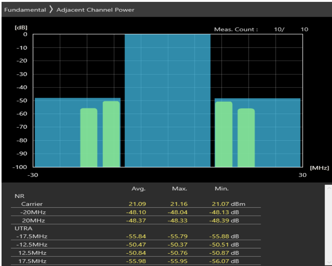
n38 SCS=30kHz DFT_QAM16 BW=20MHz Channel=516000 RB=1@0
