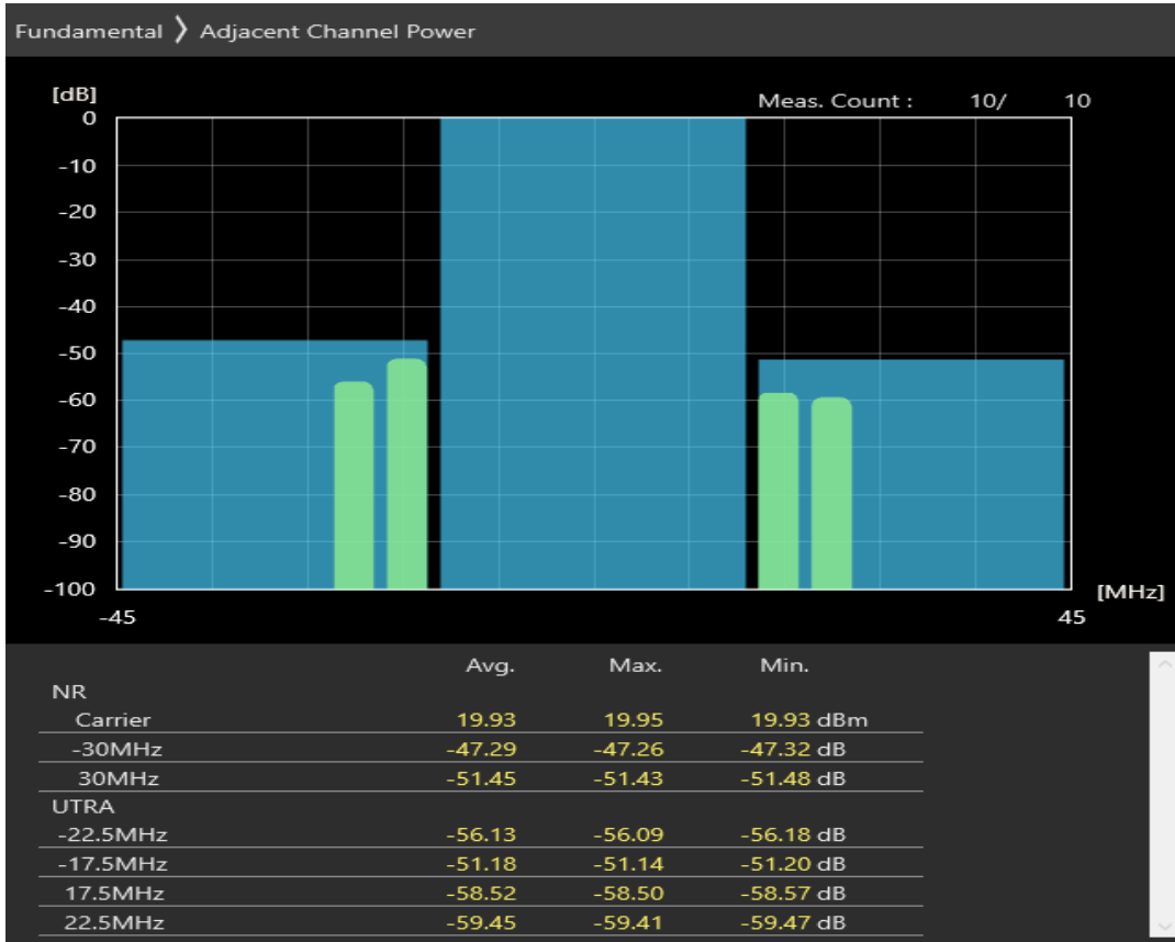
n3 SCS=30kHz CP_QAM256 BW=30MHz Channel=354000 RB=1@77
