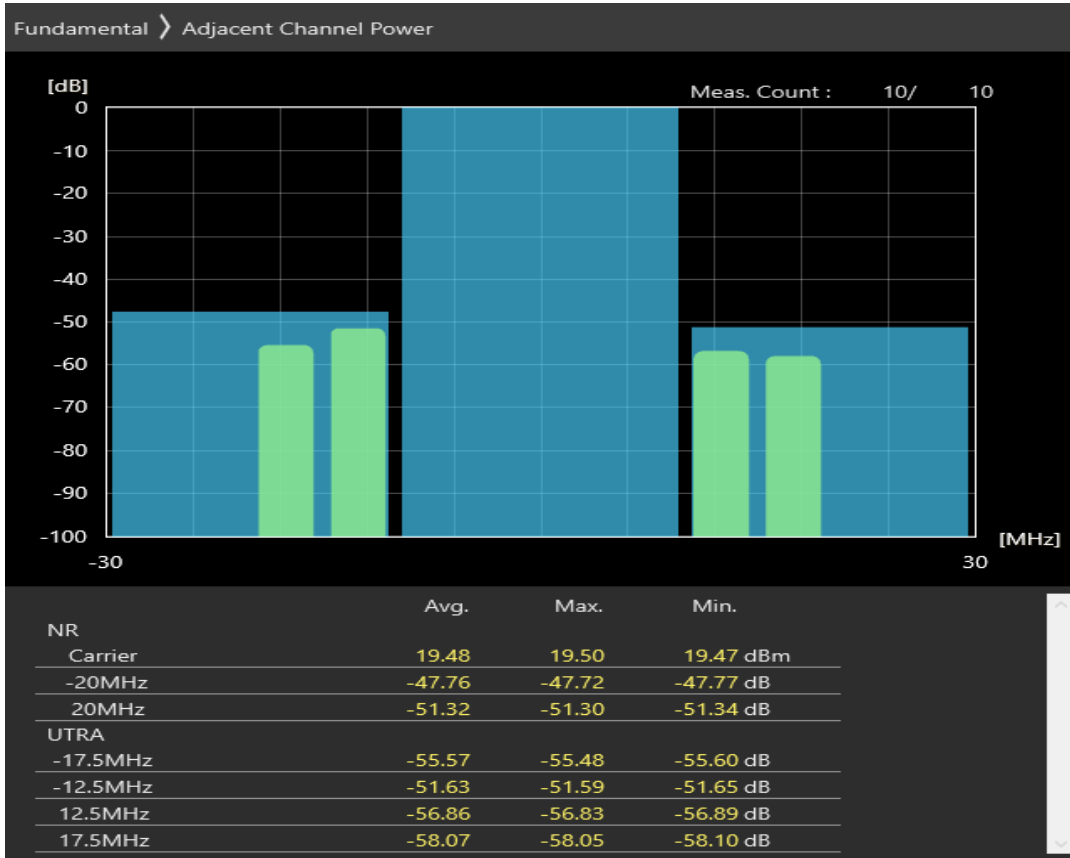
n1 SCS=30kHz CP_QAM64 BW=10MHz Channel=385000 RB=1@0
