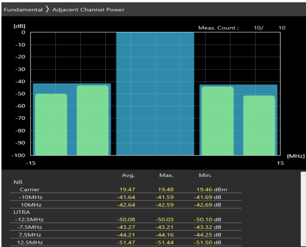
n1 SCS=30kHz CP_QAM64 BW=20MHz Channel=386000 RB=1 @0
