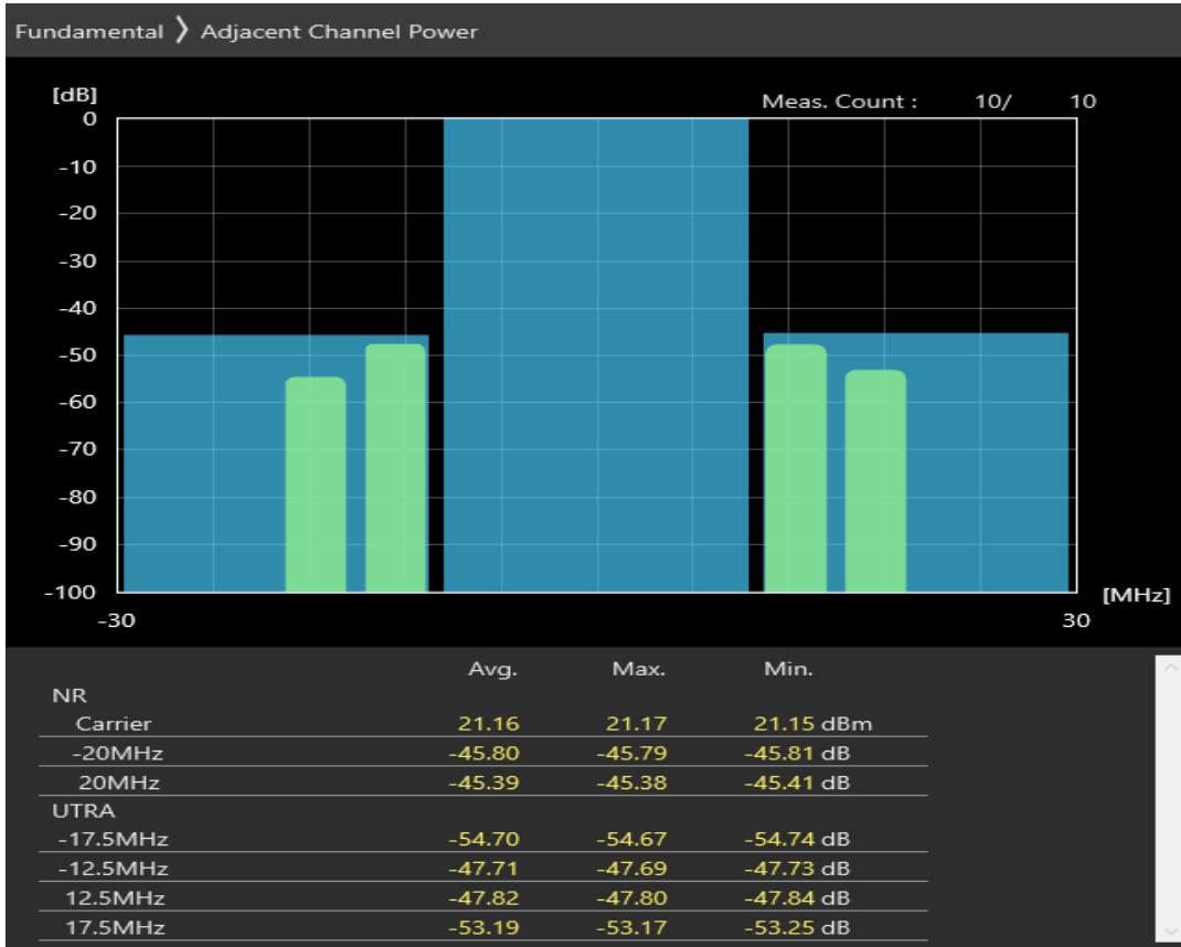
n1 SCS=30kHz CP_QAM16 BW=20MHz Channel=386000 RB=51 @0
