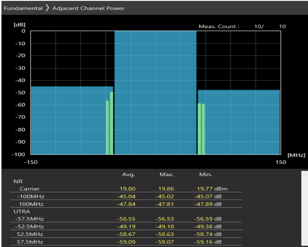
n78 SCS=30kHz DFT_BPSK BW=100MHz Channel=650000 RB=270@0
