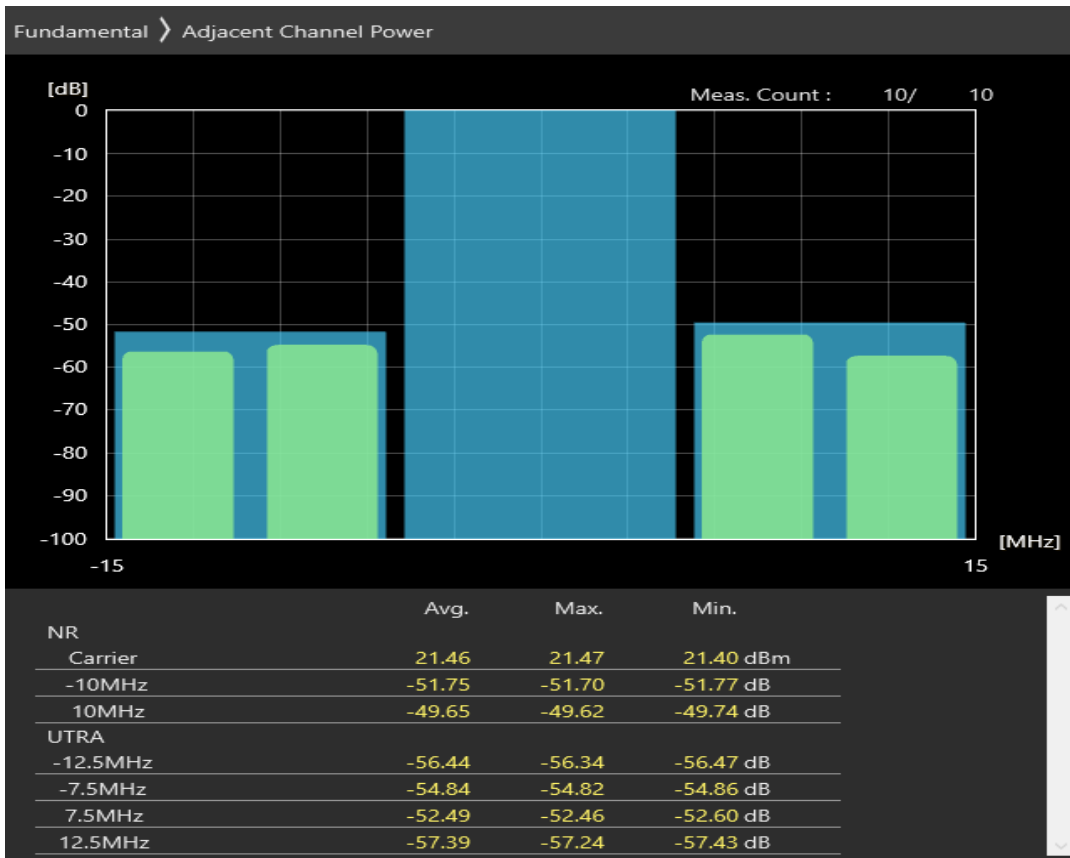
n78 SCS=30kHz CP_QAM64 BW=10MHz Channel=653000 RB=24@0
