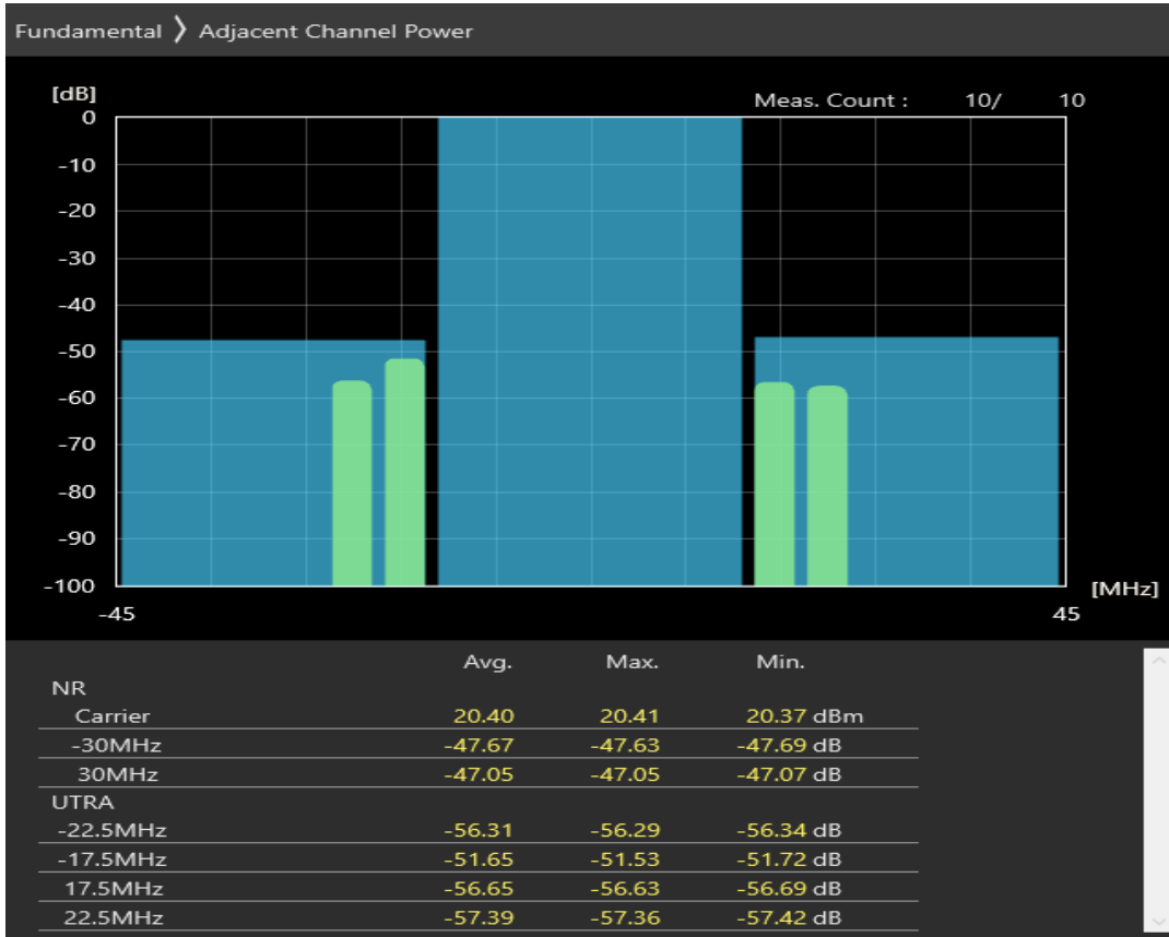
n3 SCS=30kHz CP_QAM16 BW=30MHz Channel=345000 RB=78@0
