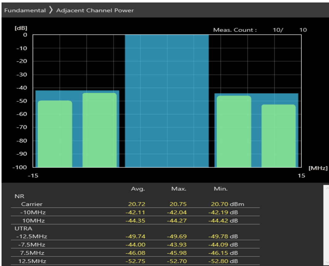
n3 SCS=30kHz DFT_QAM256 BW=10MHz Channel=356000 RB=1@23
