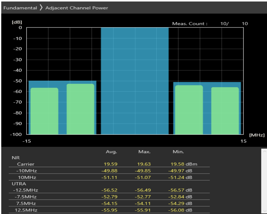
n1 SCS=30kHz CP_QAM256 BW=10MHz Channel=385000 RB=24@0
