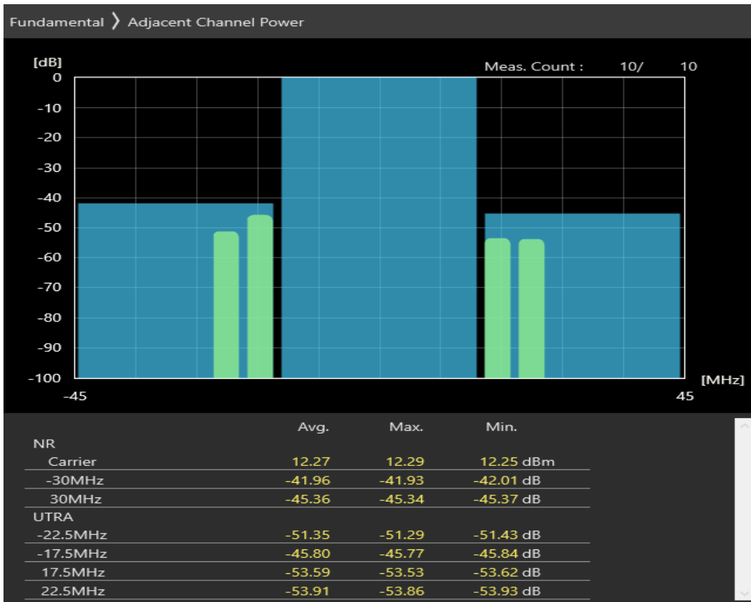
n3 SCS=30kHz CP_QAM256 BW=30MHz Channel=354000 RB=78@0
