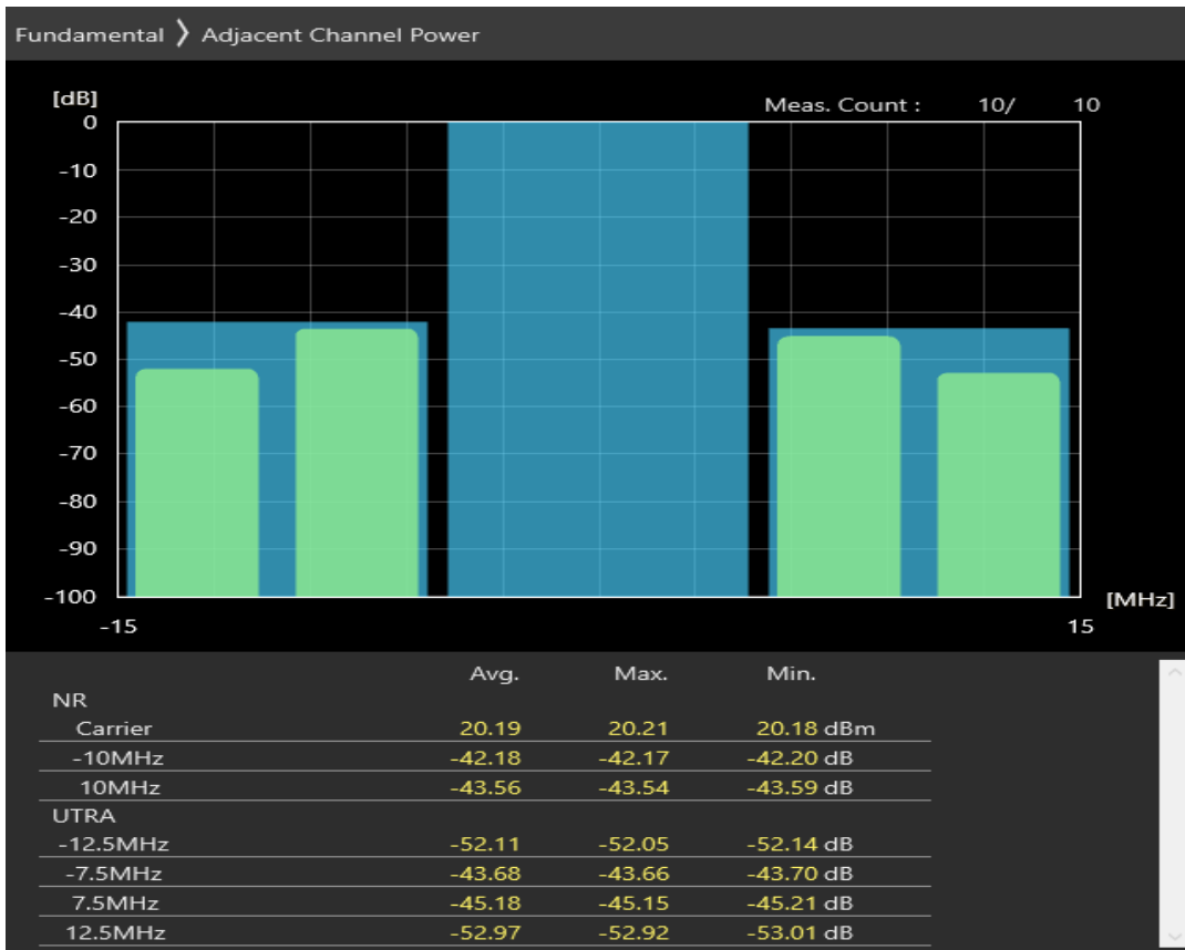
n77 SCS=30kHz CP_QAM16 BW=10MHz Channel=679666 RB=12@6
