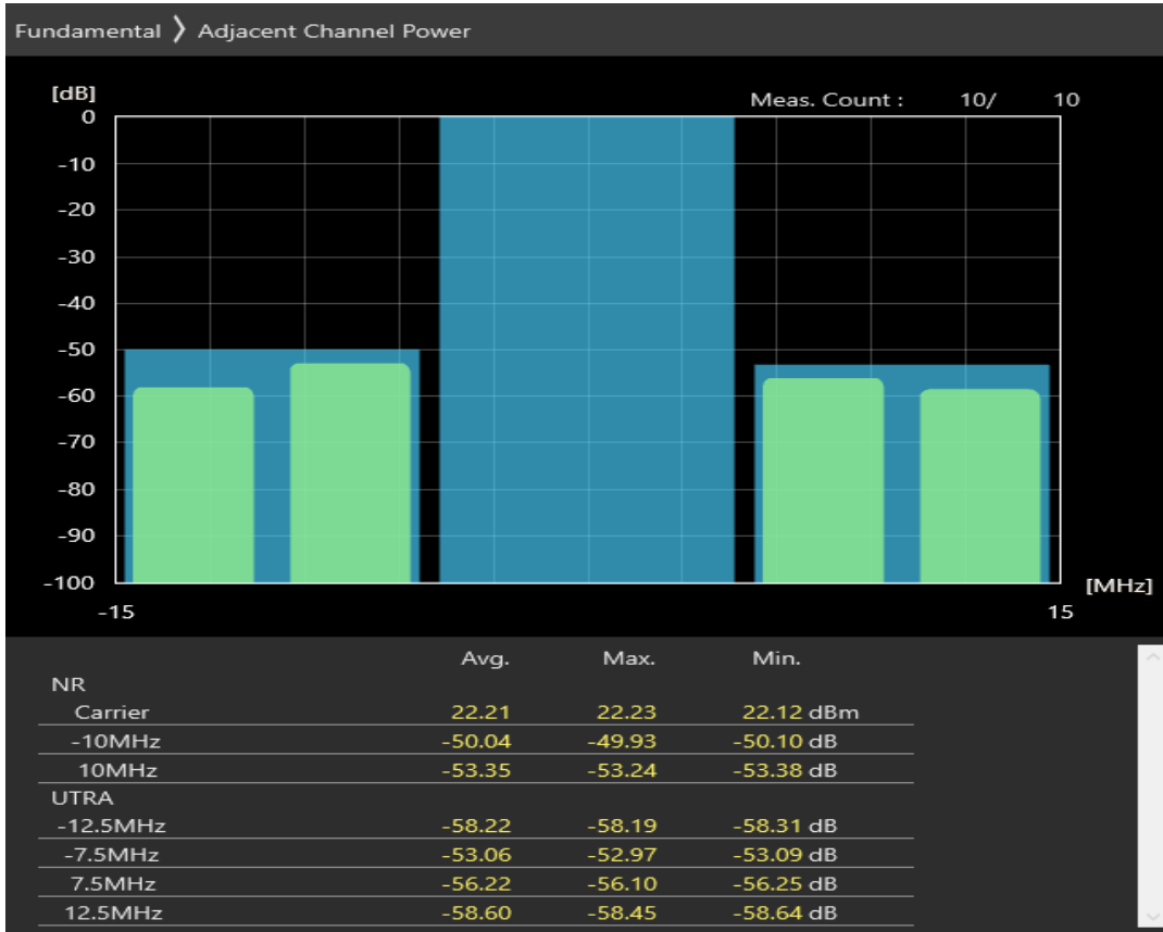
n78 SCS=30kHz DFT_QAM16 BW=10MHz Channel=647000 RB=24@0
