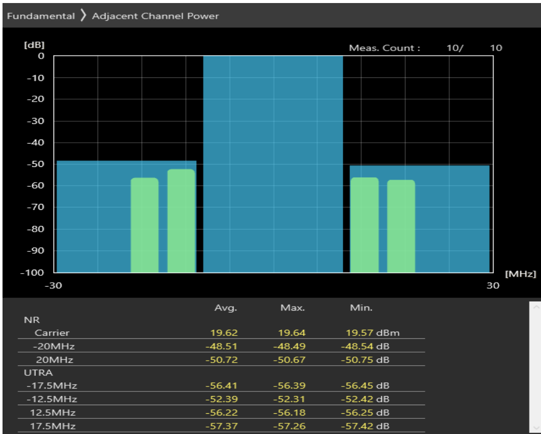
n1 SCS=30kHz DFT_QPSK BW=20MHz Channel=386000 RB=25@12
