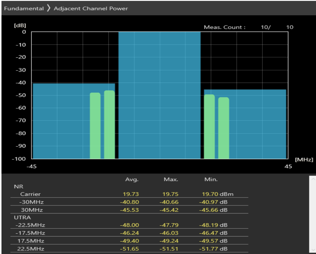
n3 SCS=30kHz DFT_QAM256 BW=30MHz Channel=354000 RB=1@77
