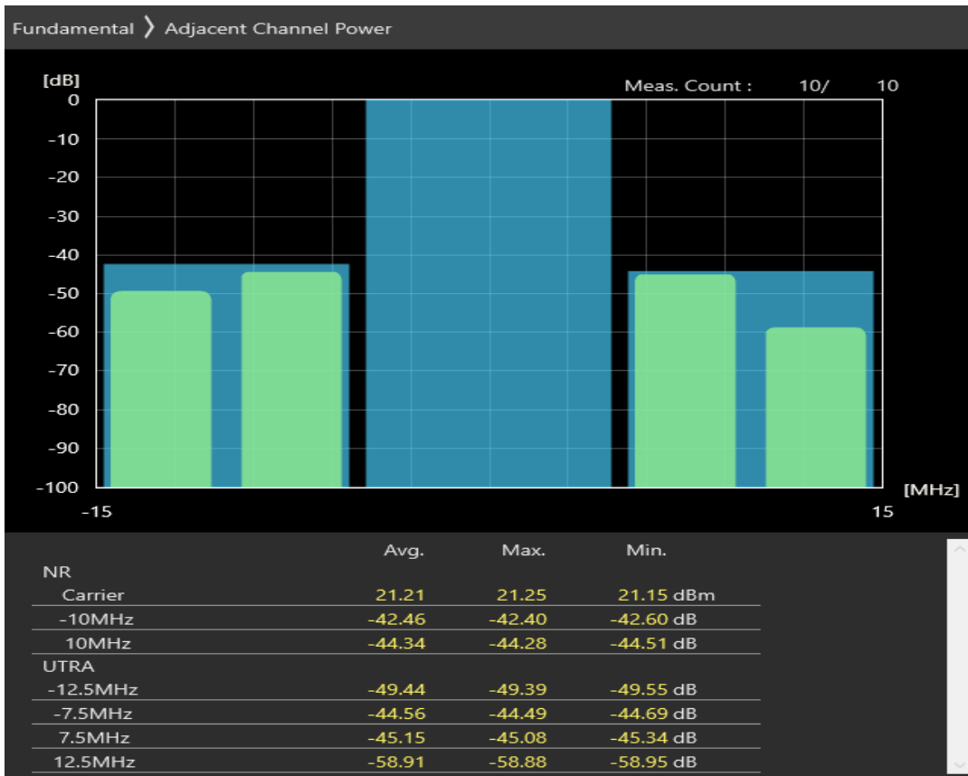
n8 SCS=30kHz DFT_QAM256 BW=10MHz Channel=182000 RB=1@23
