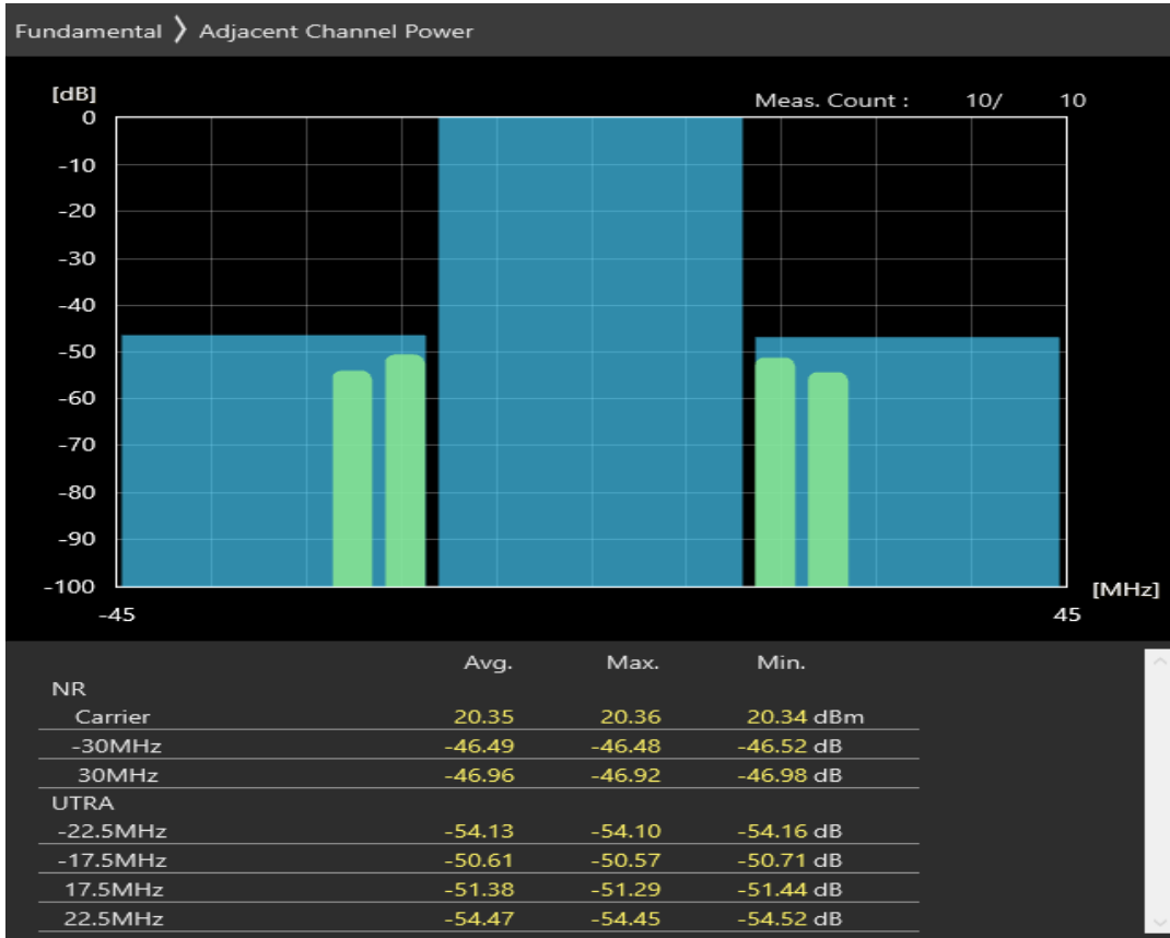
n3 SCS=30kHz DFT_QPSK BW=30MHz Channel=345000 RB=1@0
