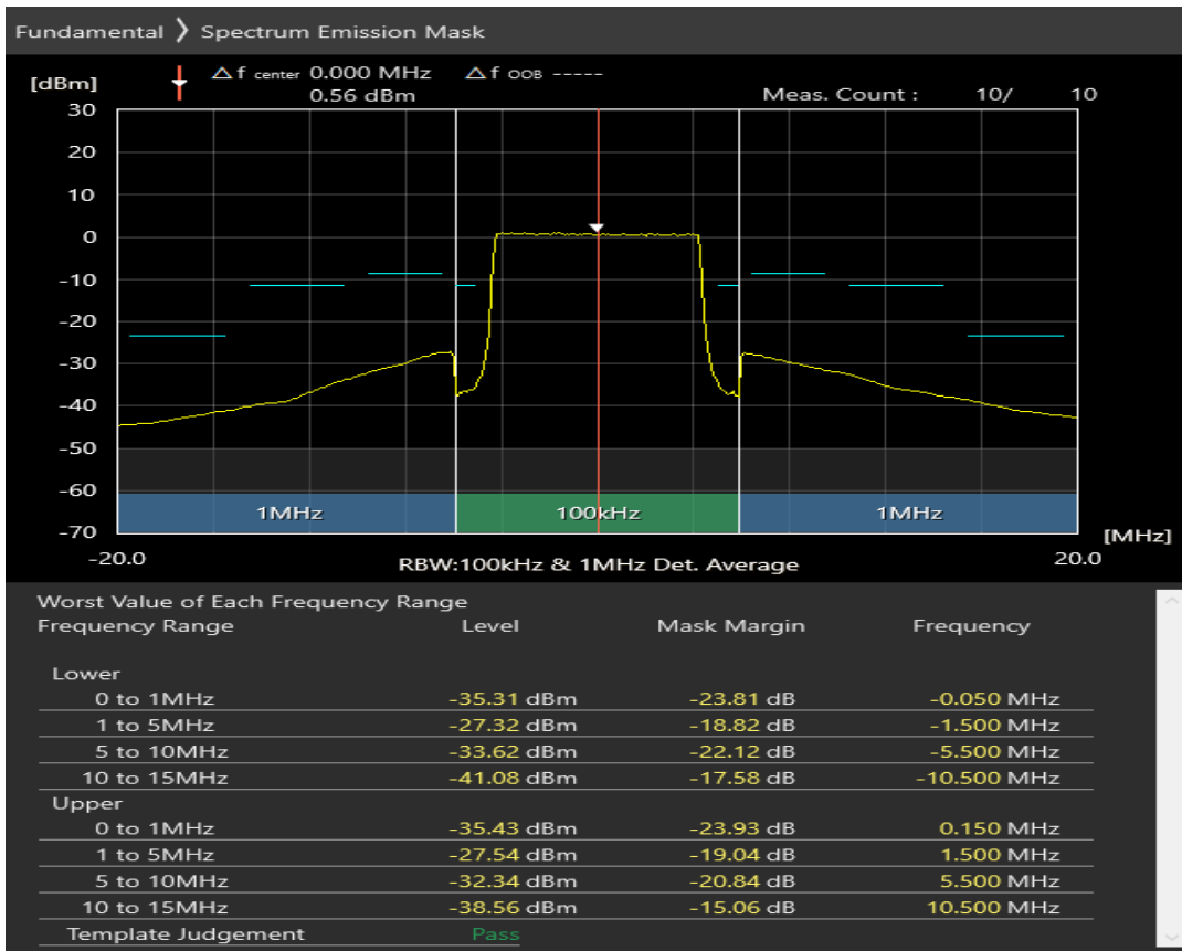
n1 SCS=30kHz CP_QAM16 BW=10MHz Channel=385000 RB=1@0
