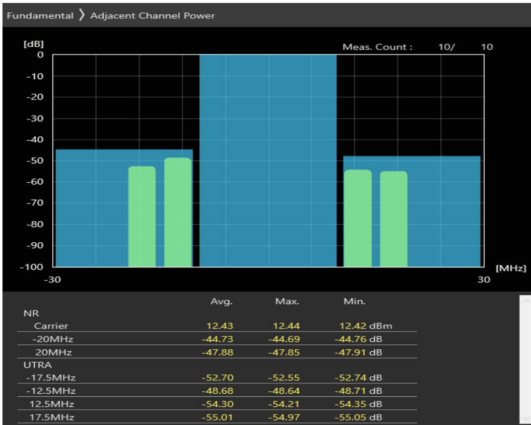
n28 SCS=30kHz CP_QAM16 BW=20MHz Channel=147600 RB=25@12
