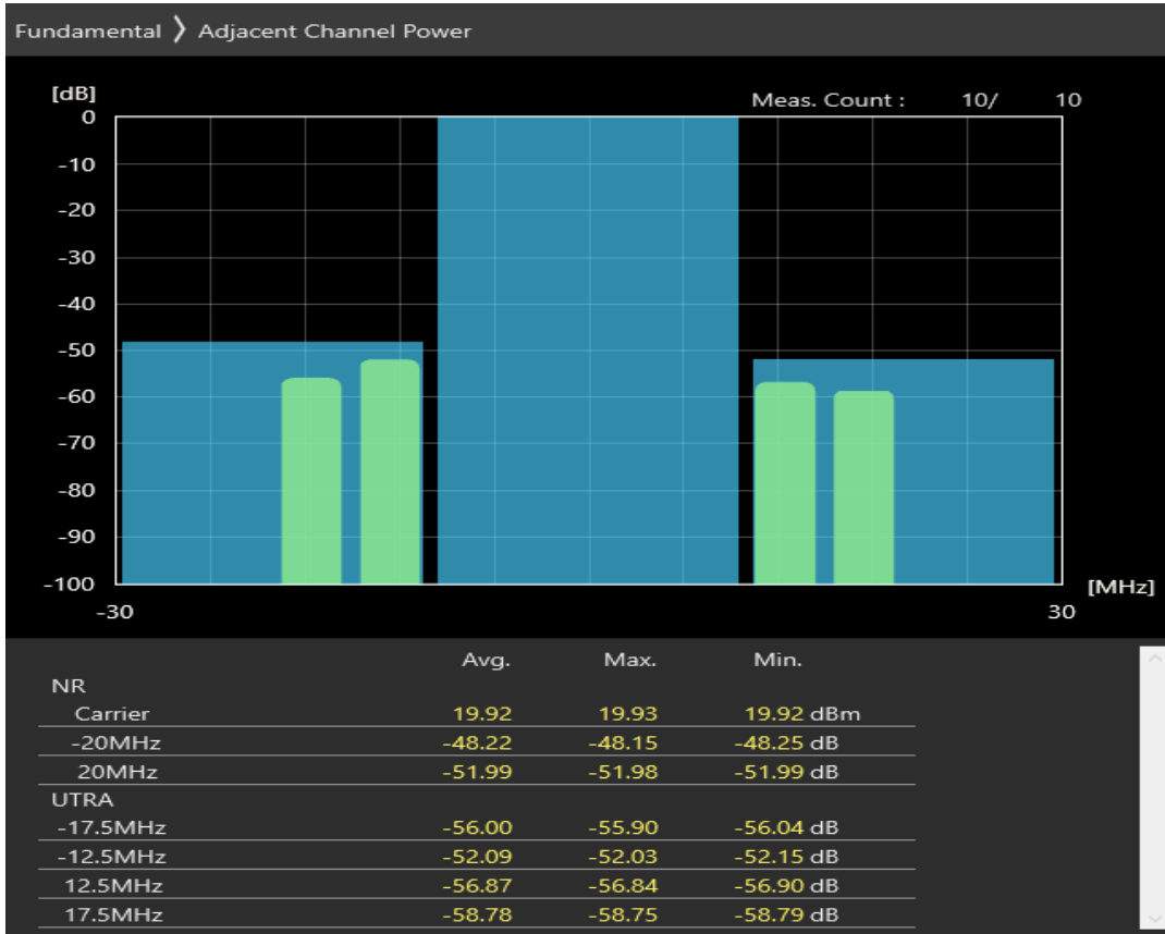
n28 SCS=30kHz DFT_BPSK BW=10MHz Channel=141600 RB=12@6
