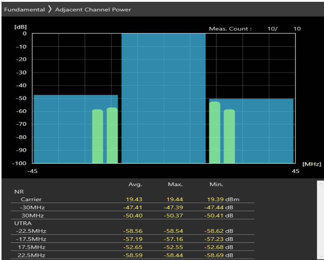
n3 SCS=30kHz DFT_BPSK BW=30MHz Channel=354000 RB=75@0
