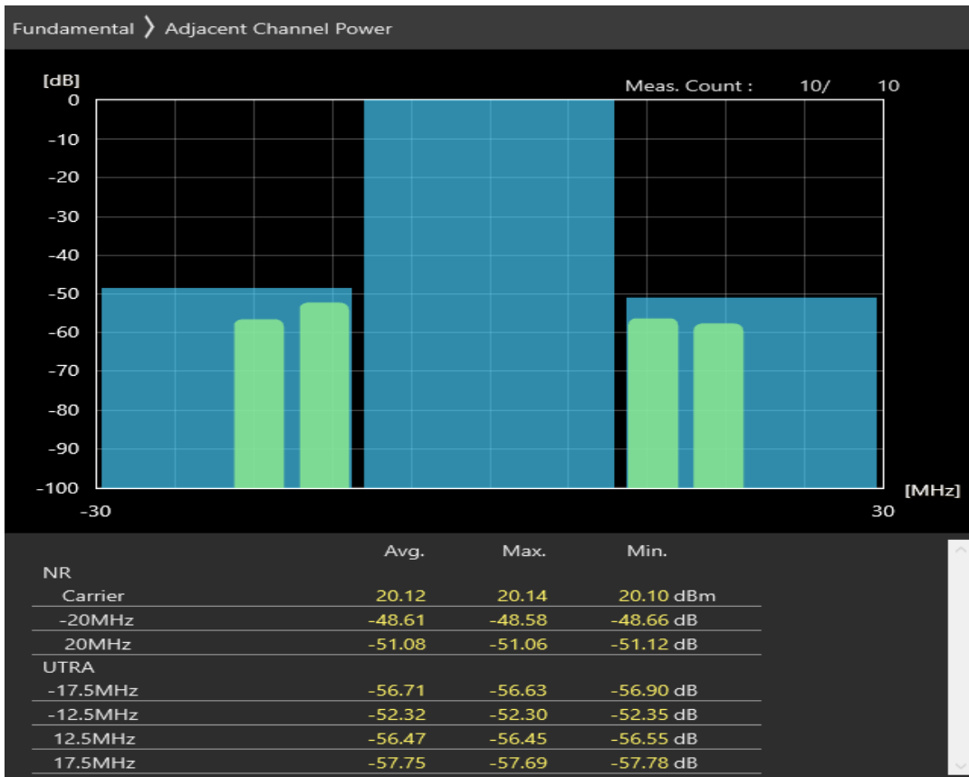
n1 SCS=30kHz CP_QAM16 BW=20MHz Channel=394000 RB=1 @50
