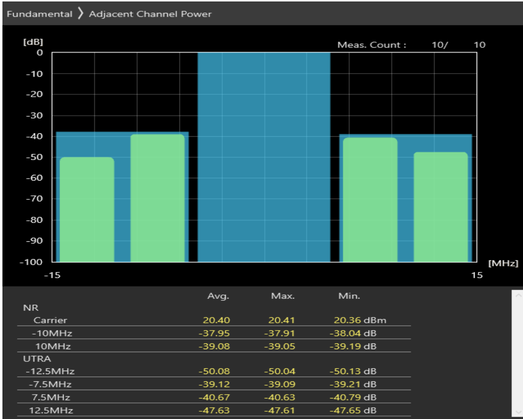
n8 SCS=30kHz DFT_BPSK BW=10MHz Channel=182000 RB=12@6
