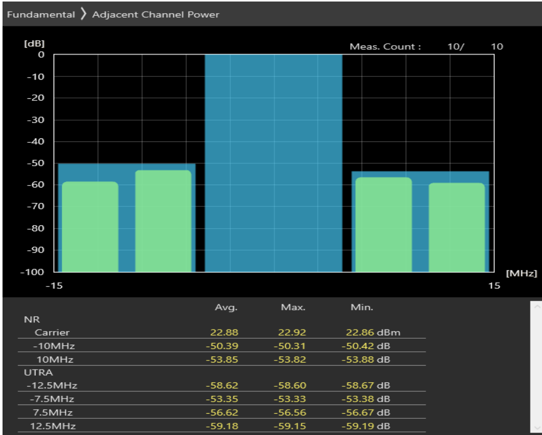
n78 SCS=30kHz DFT_BPSK BW=10MHz Channel=647000 RB=24@0
