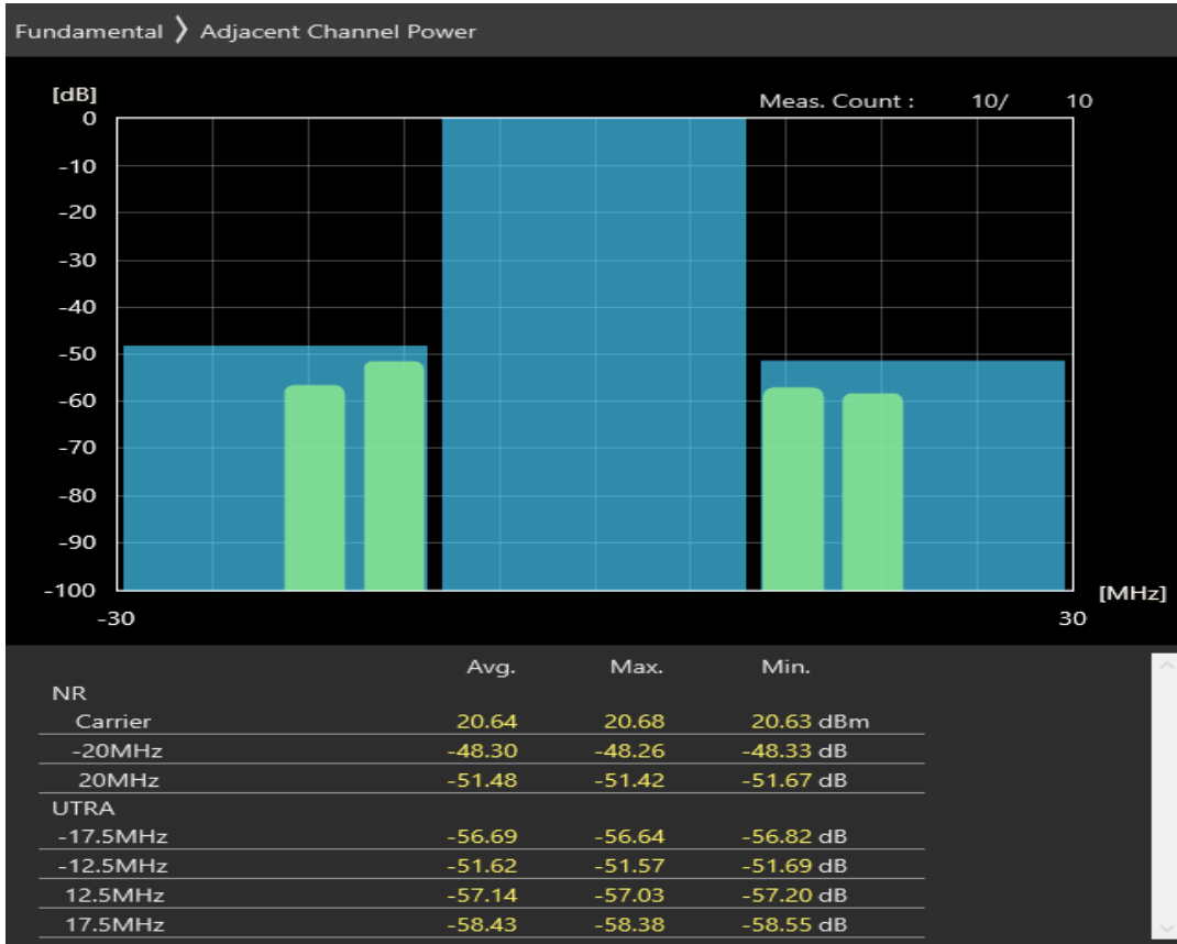
n38 SCS=30kHz CP_QAM256 BW=20MHz Channel=522000 RB=1@50
