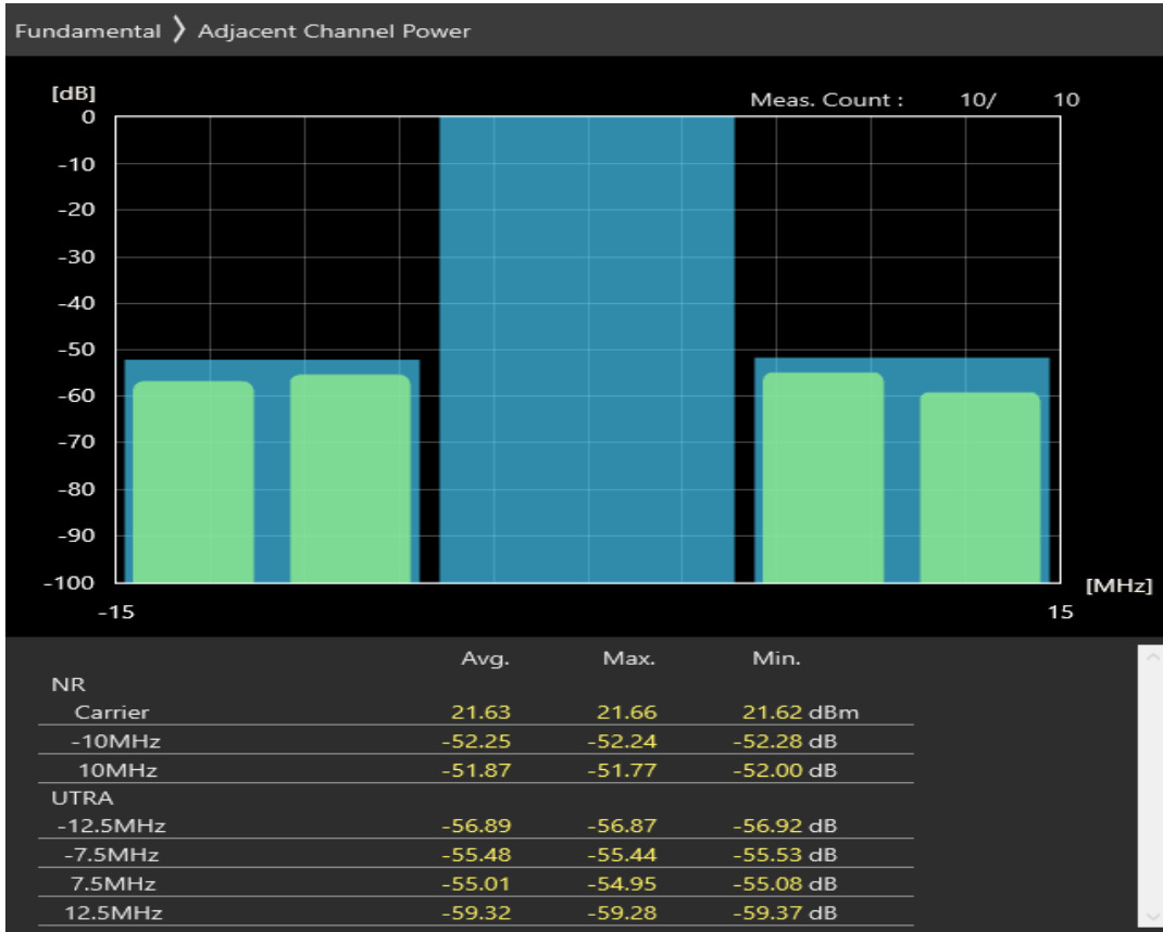
n8 SCS=30kHz DFT_QAM16 BW=10MHz Channel=182000 RB=24@0
