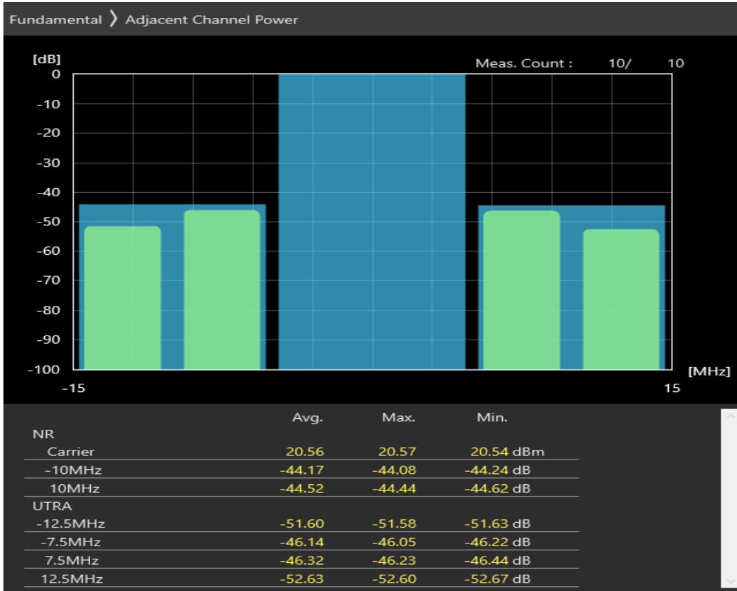
n1 SCS=30kHz DFT_QAM64 BW=20MHz Channel=386000 RB=1@0
