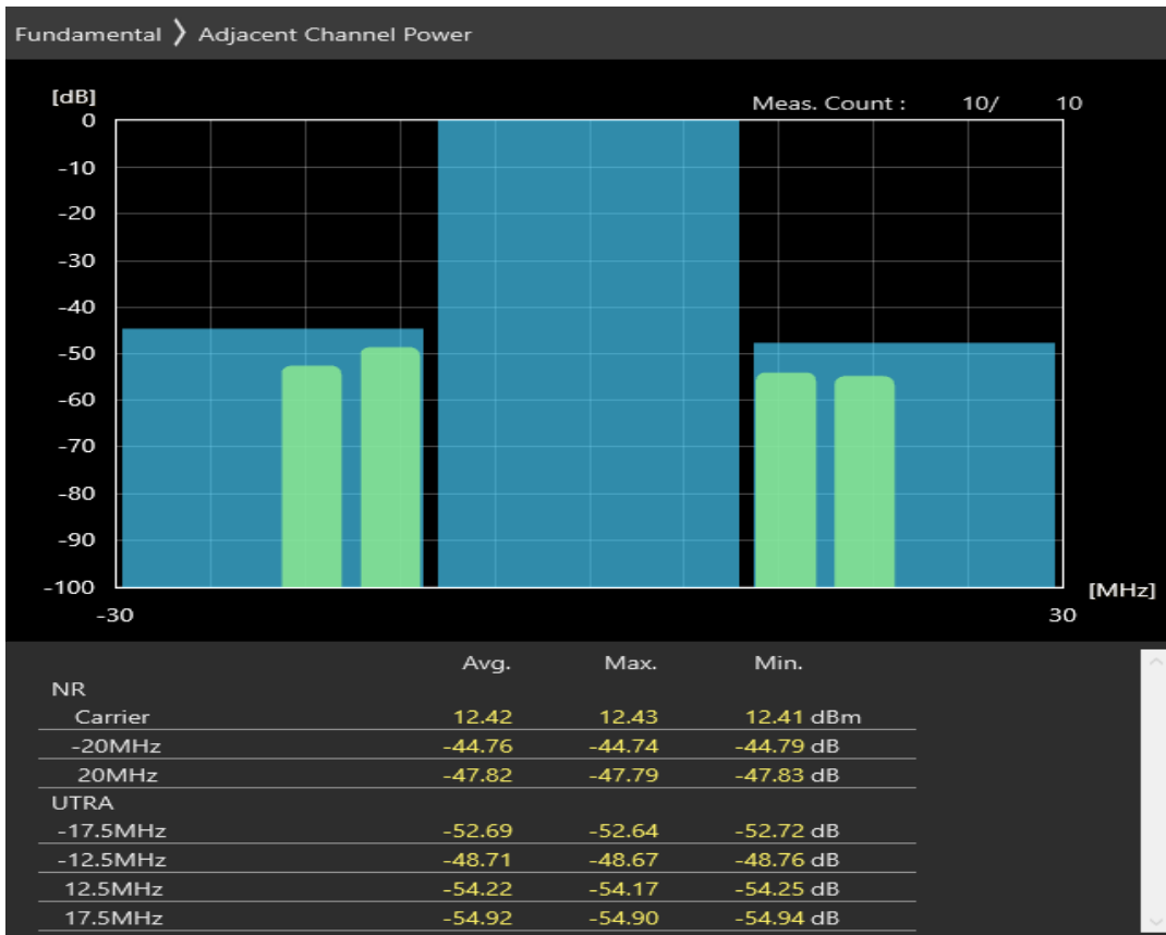
n28 SCS=30kHz CP_QAM16 BW=20MHz Channel=147600 RB=51 @0
