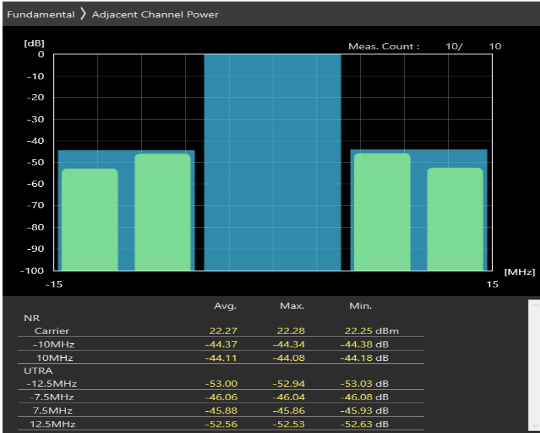
n38 SCS=30kHz DFT_QAM64 BW=10MHz Channel=523000 RB=1@23
