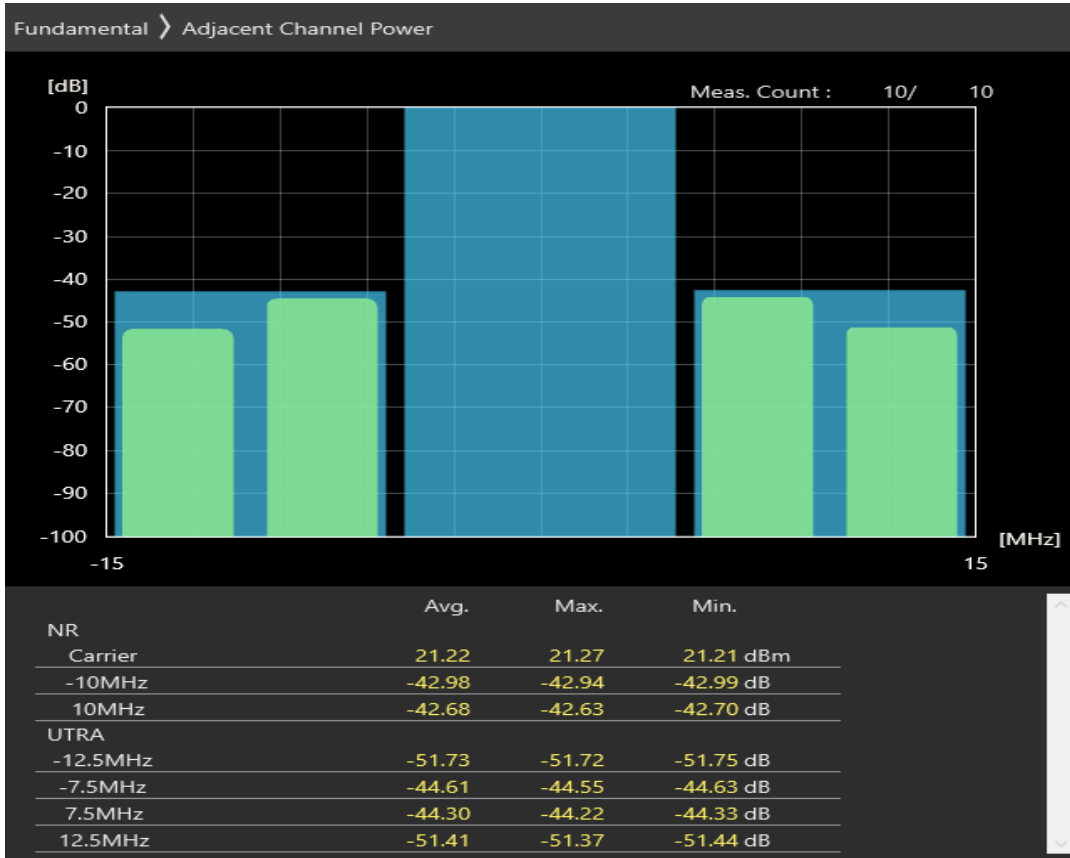
n38 SCS=30kHz CP_QAM64 BW=10MHz Channel=523000 RB=1 @23
