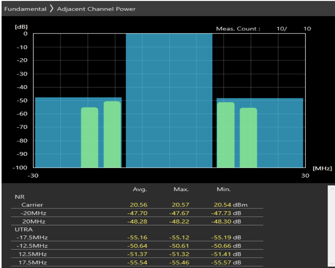
n38 SCS=30kHz DFT_QAM16 BW=20MHz Channel=522000 RB=1@50
