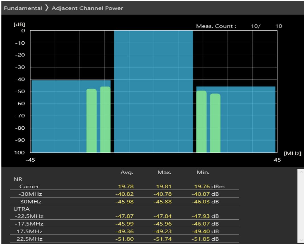
n3 SCS=30kHz DFT_QPSK BW=30MHz Channel=354000 RB=36@18
