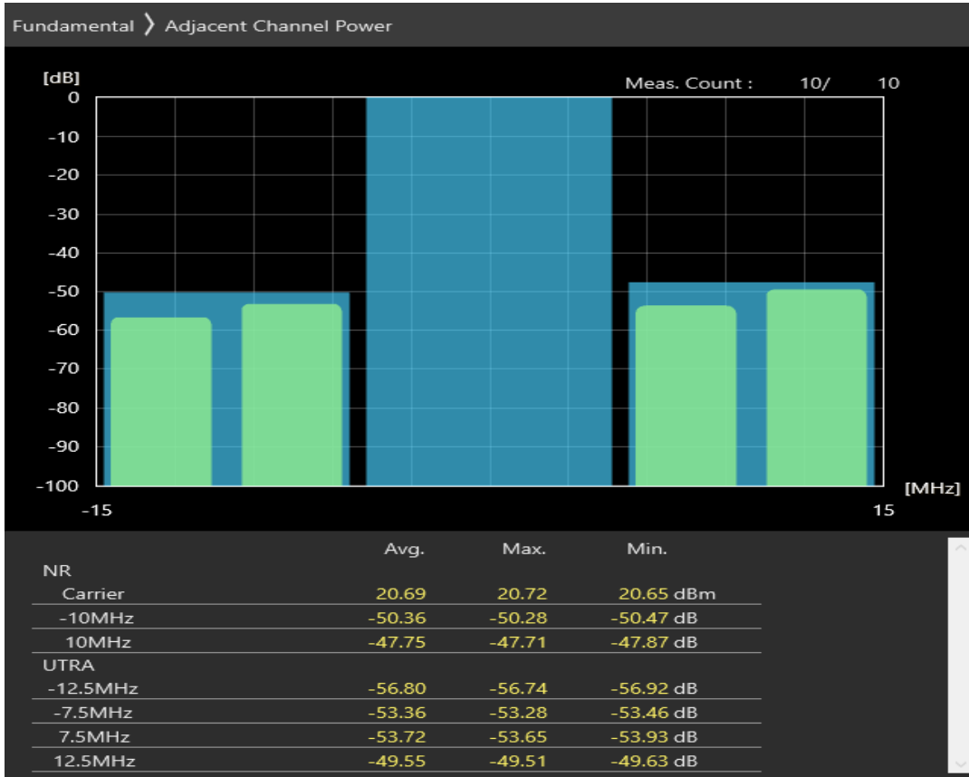
n3 SCS=30kHz CP_QAM16 BW=10MHz Channel=343000 RB=24@0
