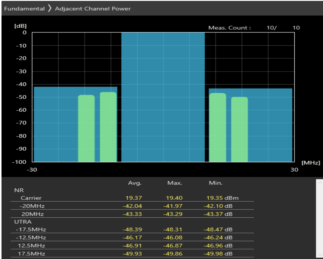
n1 SCS=30kHz DFT_QAM256 BW=10MHz Channel=385000 RB=1@0
