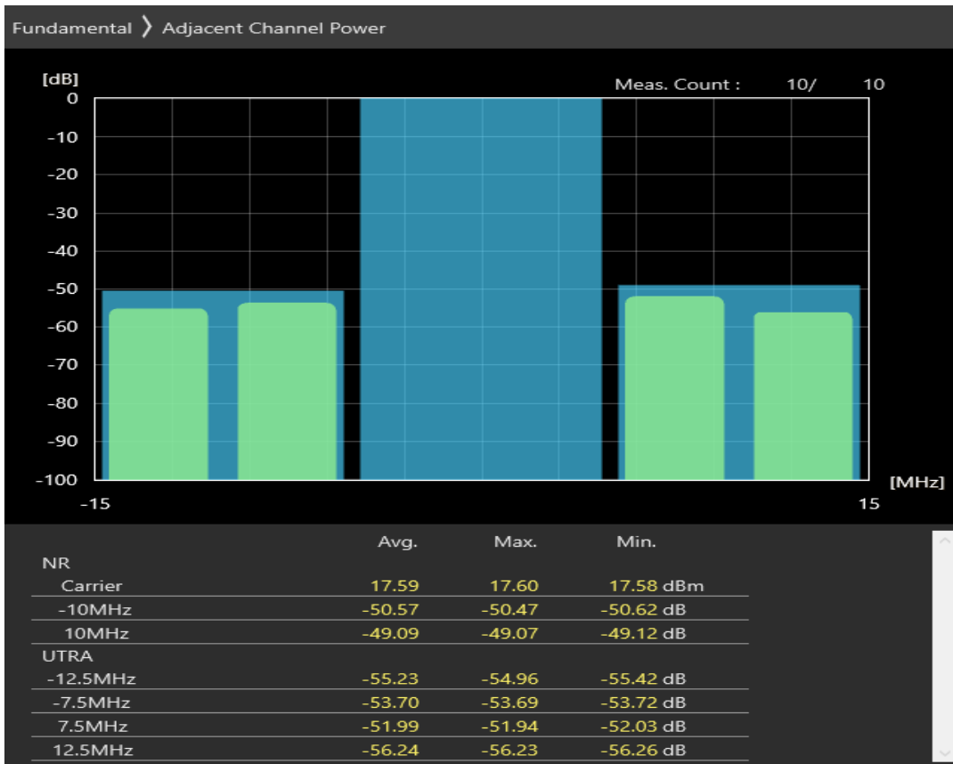
n77 SCS=30kHz DFT_BPSK BW=10MHz Channel=679666 RB=24@0
