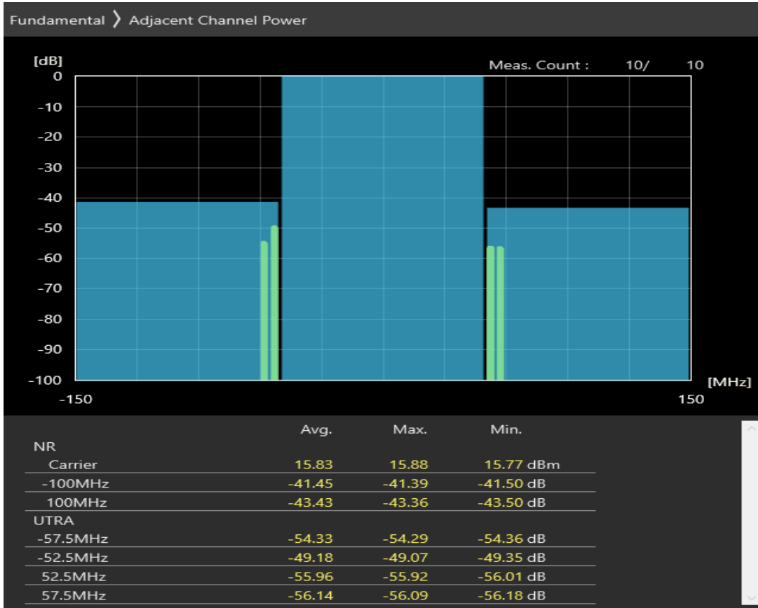
n77 SCS=30kHz DFT_BPSK BW=100MHz Channel=623334 RB=270@0
