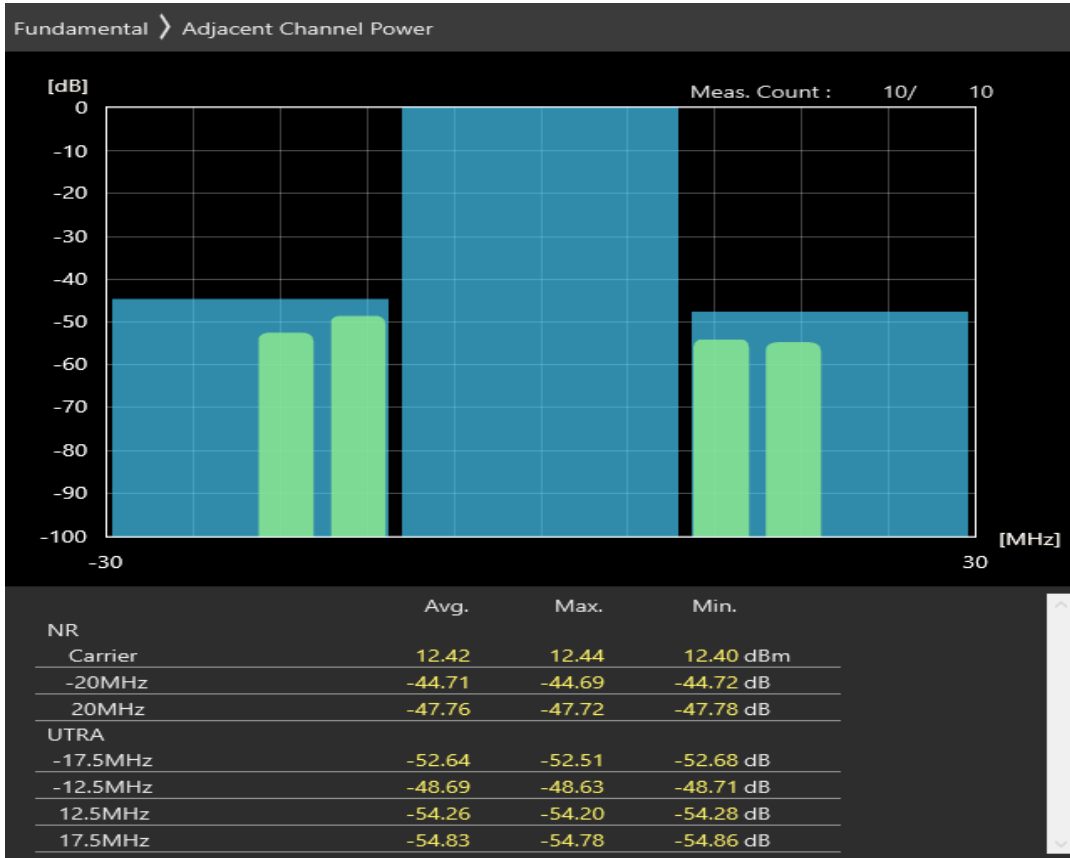
n3 SCS=30kHz DFT_BPSK BW=10MHz Channel=343000 RB=12@6
