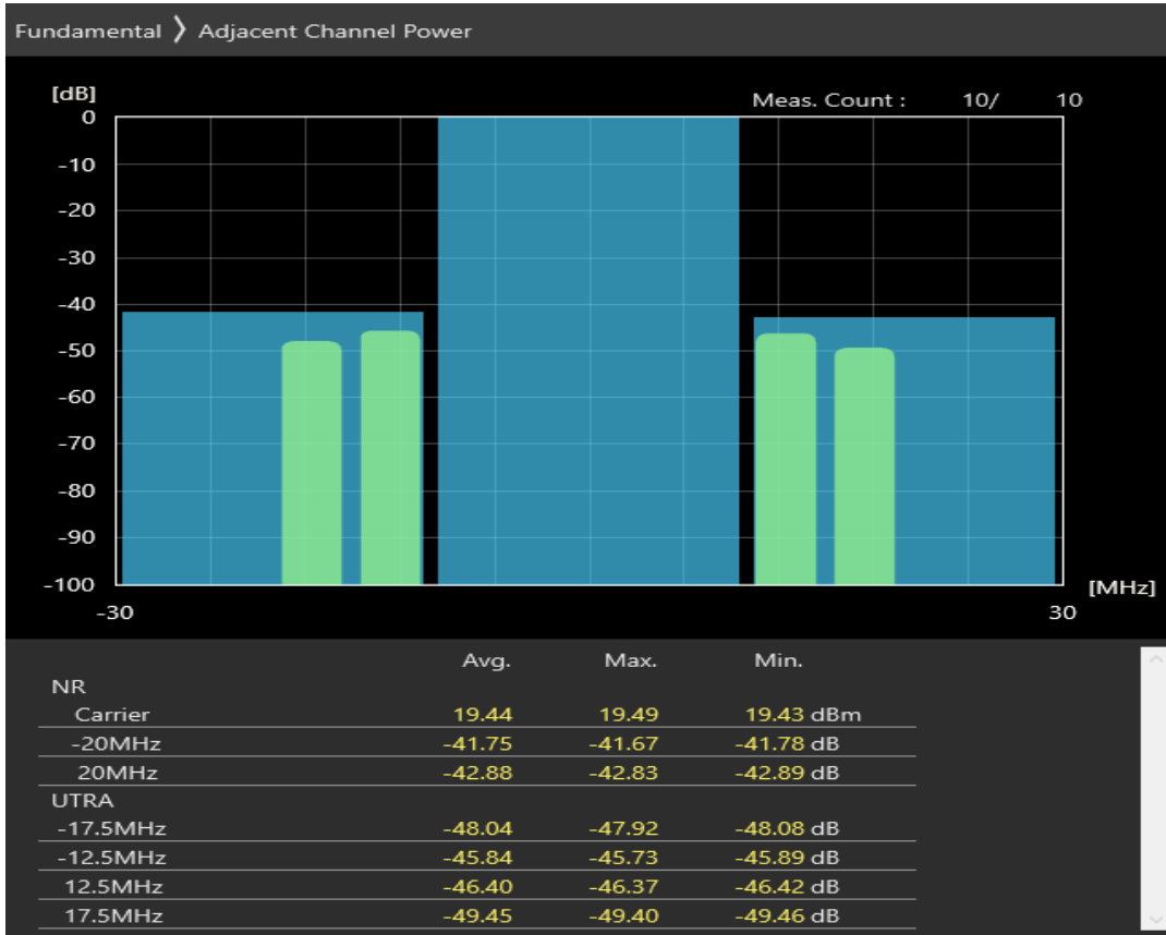
n20 SCS=30kHz DFT_BPSK BW=10MHz Channel=167400 RB=12@6
