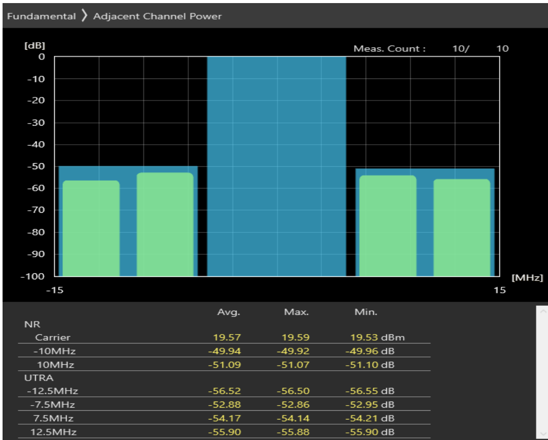
n1 SCS=30kHz CP_QAM64 BW=10MHz Channel=385000 RB=24@0
