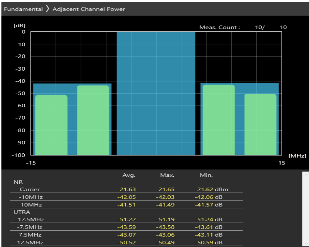
n38 SCS=30kHz CP_QAM64 BW=10MHz Channel=515000 RB=1@0
