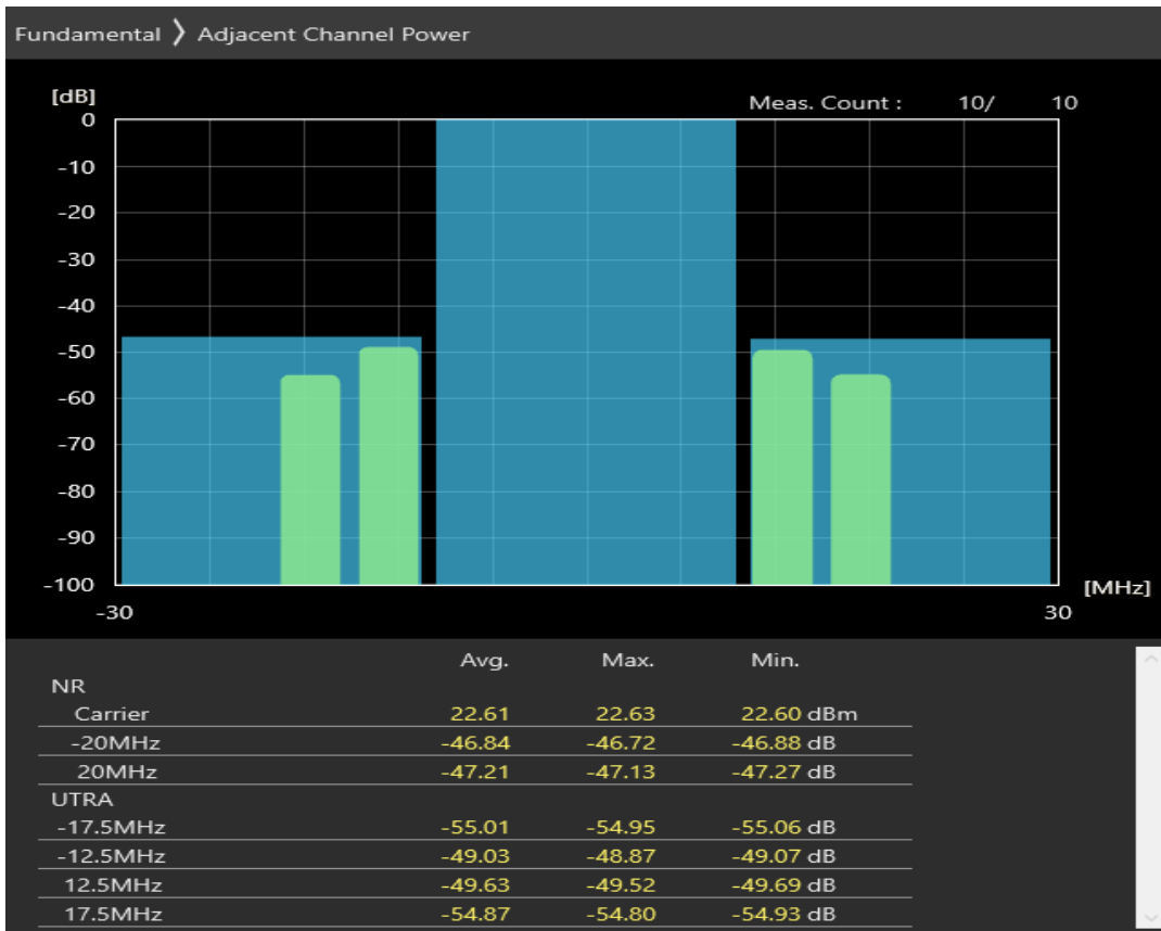
n38 SCS=30kHz CP_QAM16 BW=20MHz Channel=516000 RB=1@0
