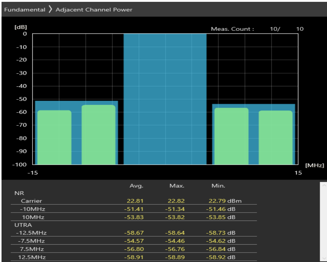
n1 SCS=30kHz DFT_BPSK BW=10MHz Channel=385000 RB=24@0
