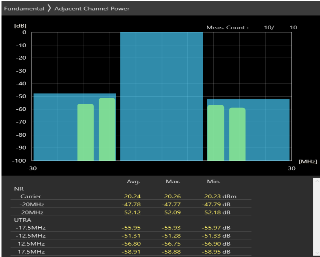
n20 SCS=30kHz CP_QAM64 BW=20MHz Channel=170400 RB=1@50
