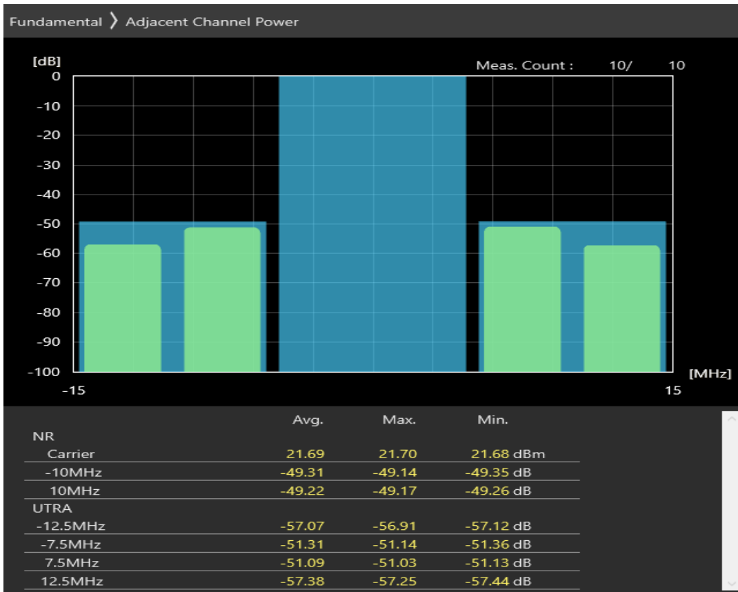
n38 SCS=30kHz CP_QPSK BW=10MHz Channel=523000 RB=1@23
