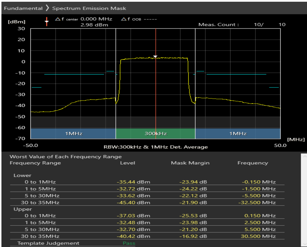
n3 SCS=30kHz DFT_QAM16 BW=30MHz Channel=345000 RB=1@0
