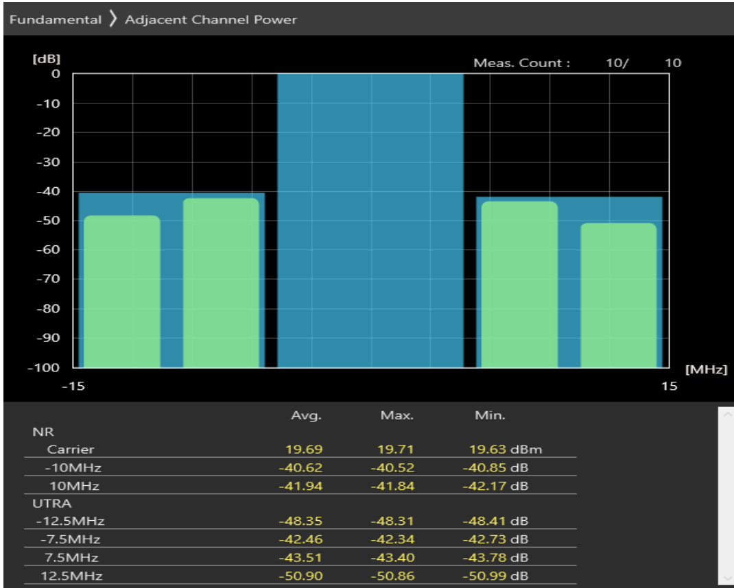
n3 SCS=30kHz DFT_BPSK BW=30MHz Channel=345000 RB=36@18
