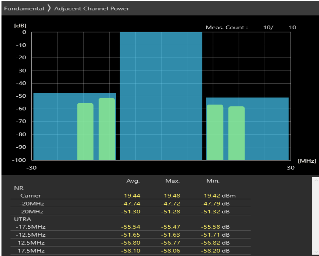
n1 SCS=30kHz CP_QPSK BW=10MHz Channel=385000 RB=12@6
