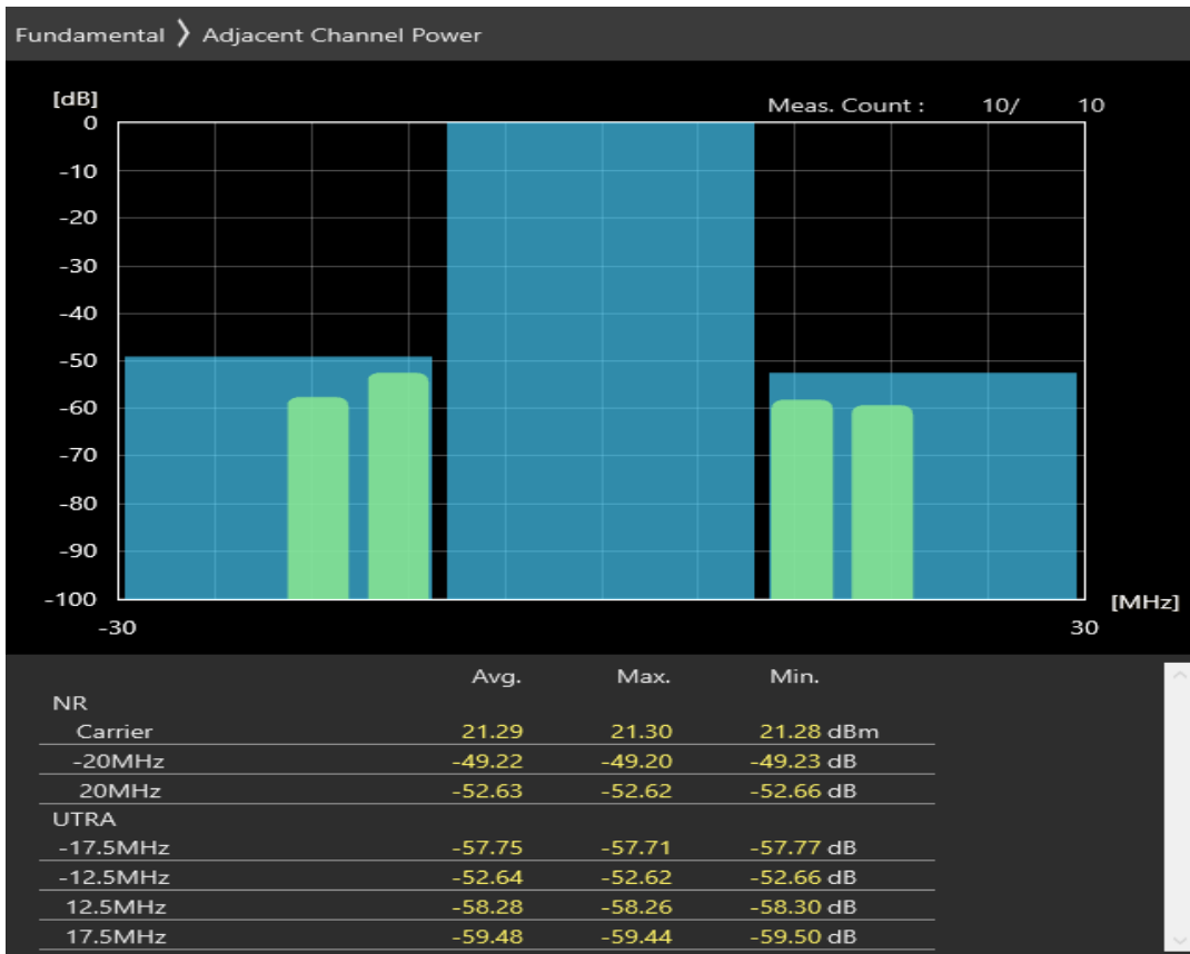
n8 SCS=30kHz CP_QAM16 BW=20MHz Channel=178000 RB=25 @12
