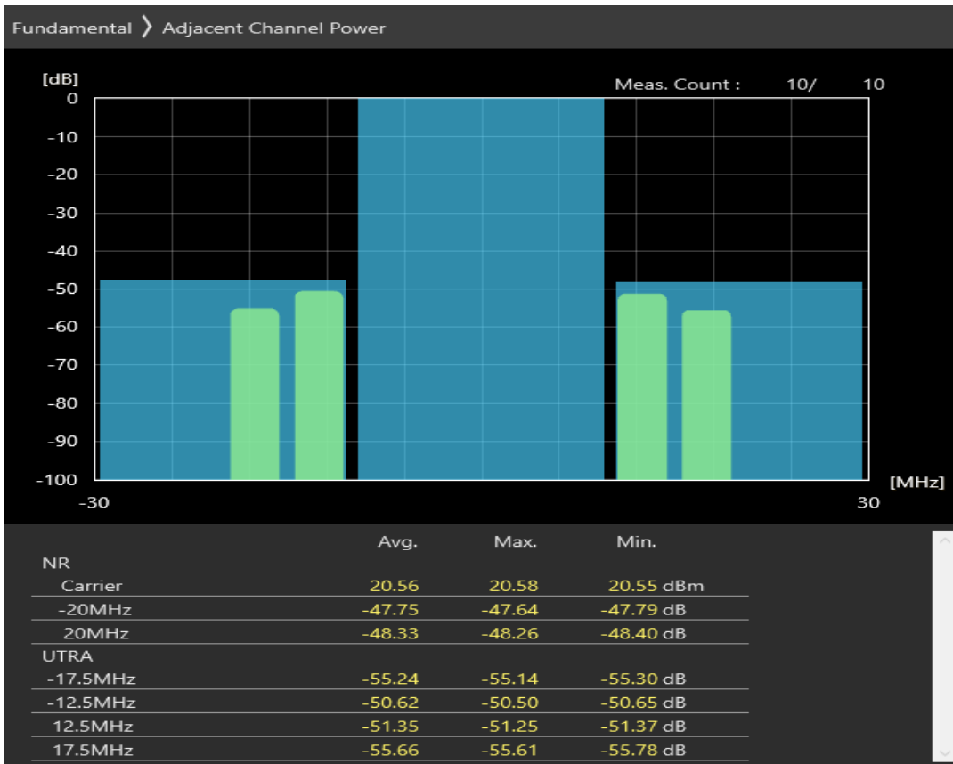
n38 SCS=30kHz DFT_QPSK BW=20MHz Channel=522000 RB=1@50
