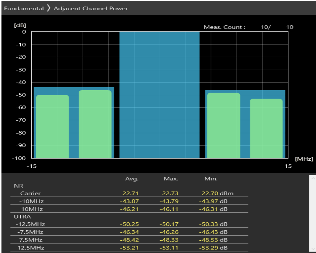
n3 SCS=30kHz DFT_QPSK BW=10MHz Channel=356000 RB=12@6
