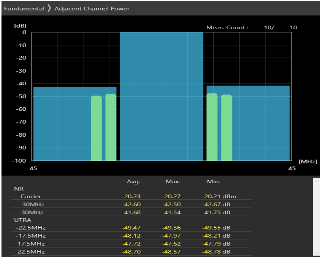
n3 SCS=30kHz DFT_QAM16 BW=30MHz Channel=345000 RB=36@18
