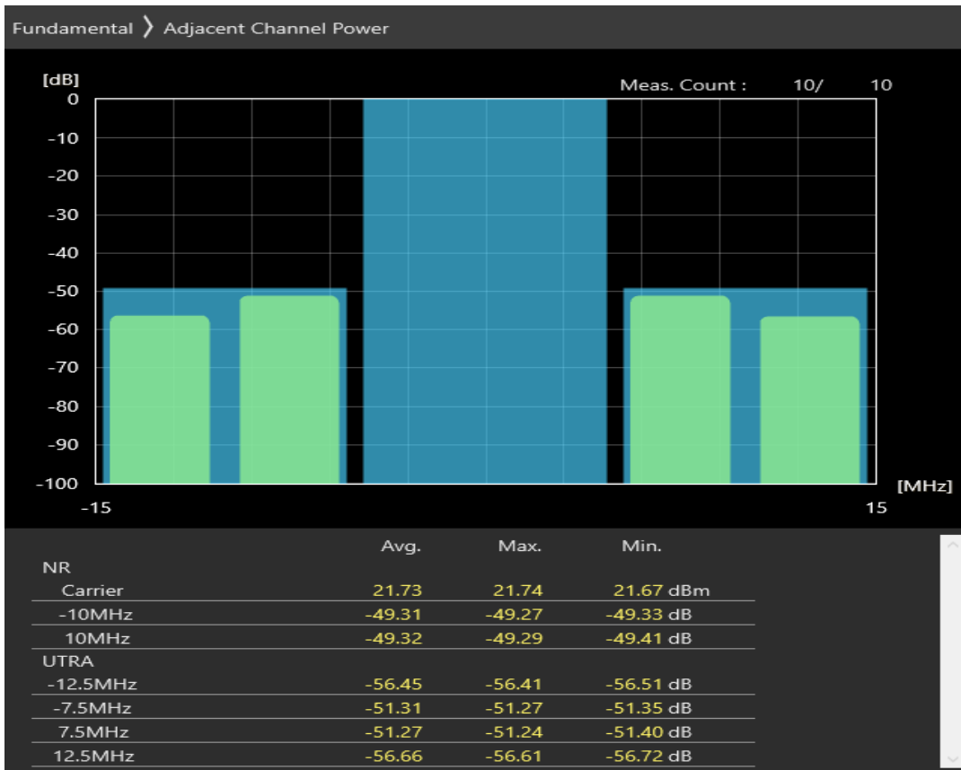
n77 SCS=30kHz CP_QAM16 BW=10MHz Channel=620334 RB=1@0
