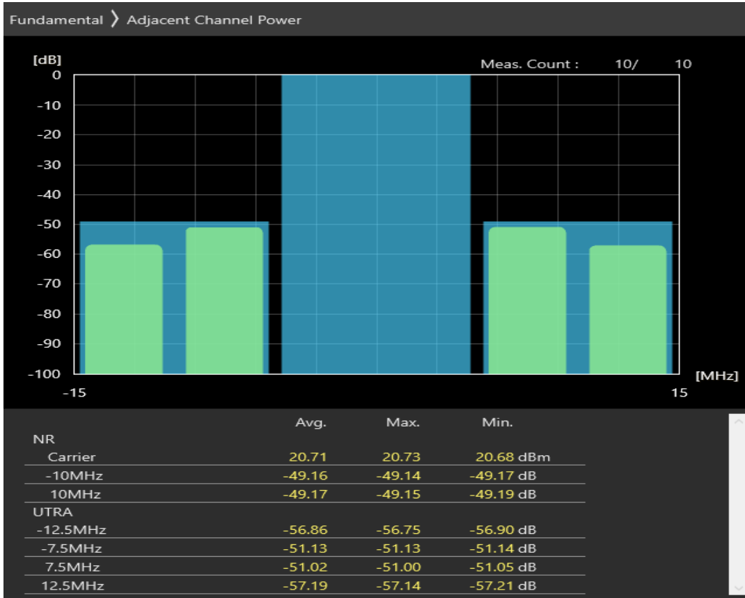
n38 SCS=30kHz DFT_BPSK BW=10MHz Channel=523000 RB=1@23
