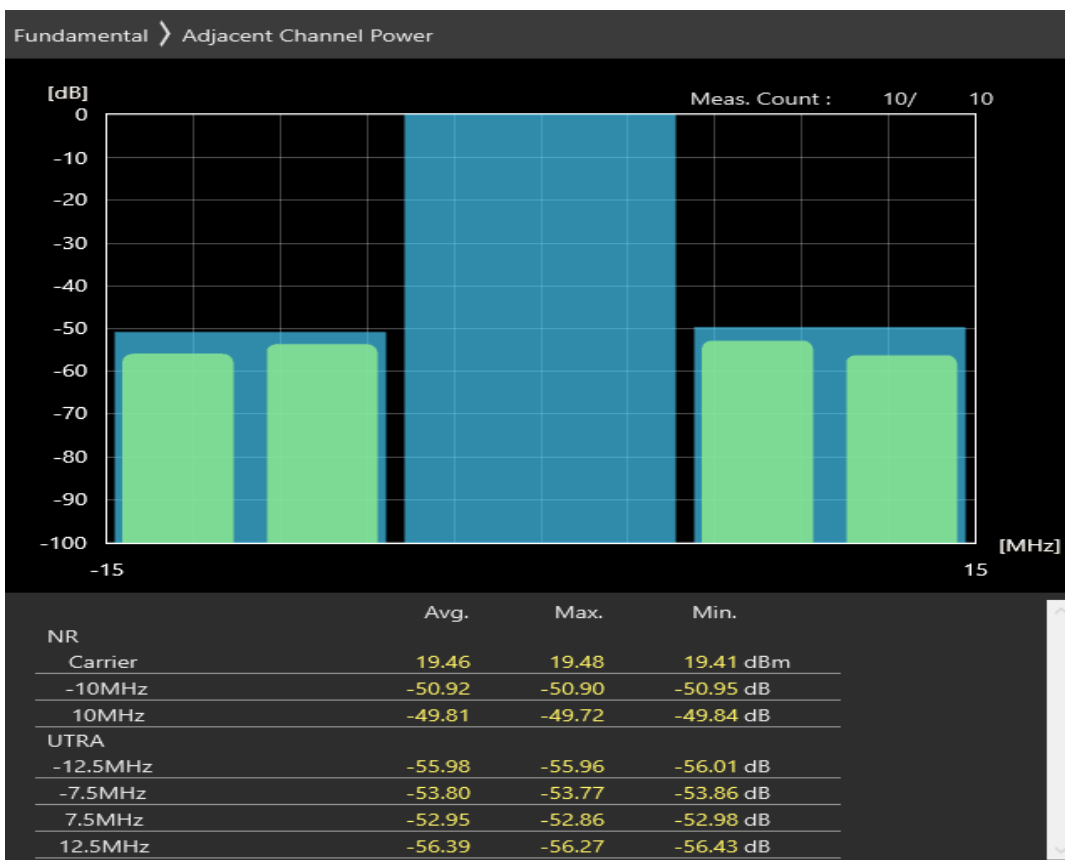
n1 SCS=30kHz CP_QAM64 BW=10MHz Channel=395000 RB=24@0
