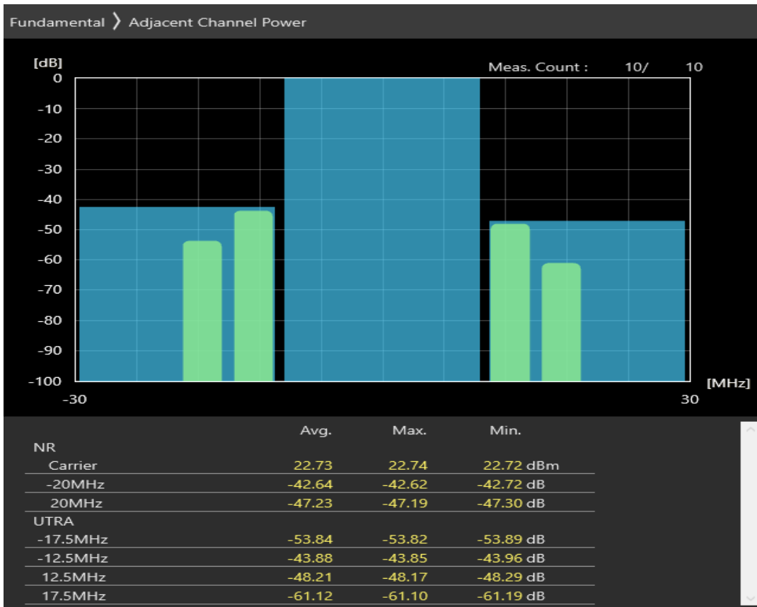
n8 SCS=30kHz DFT_QAM16 BW=20MHz Channel=181000 RB=1@50
