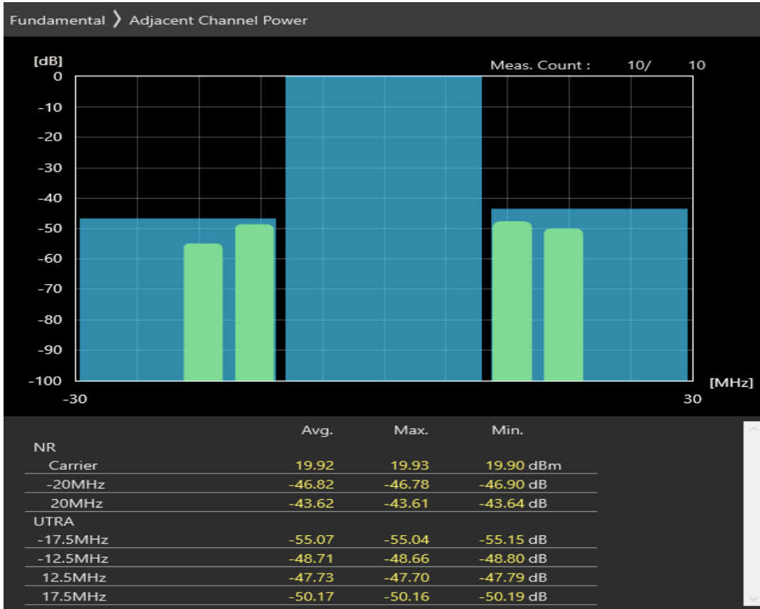
n20 SCS=30kHz DFT_QAM16 BW=20MHz Channel=168400 RB=25@12
