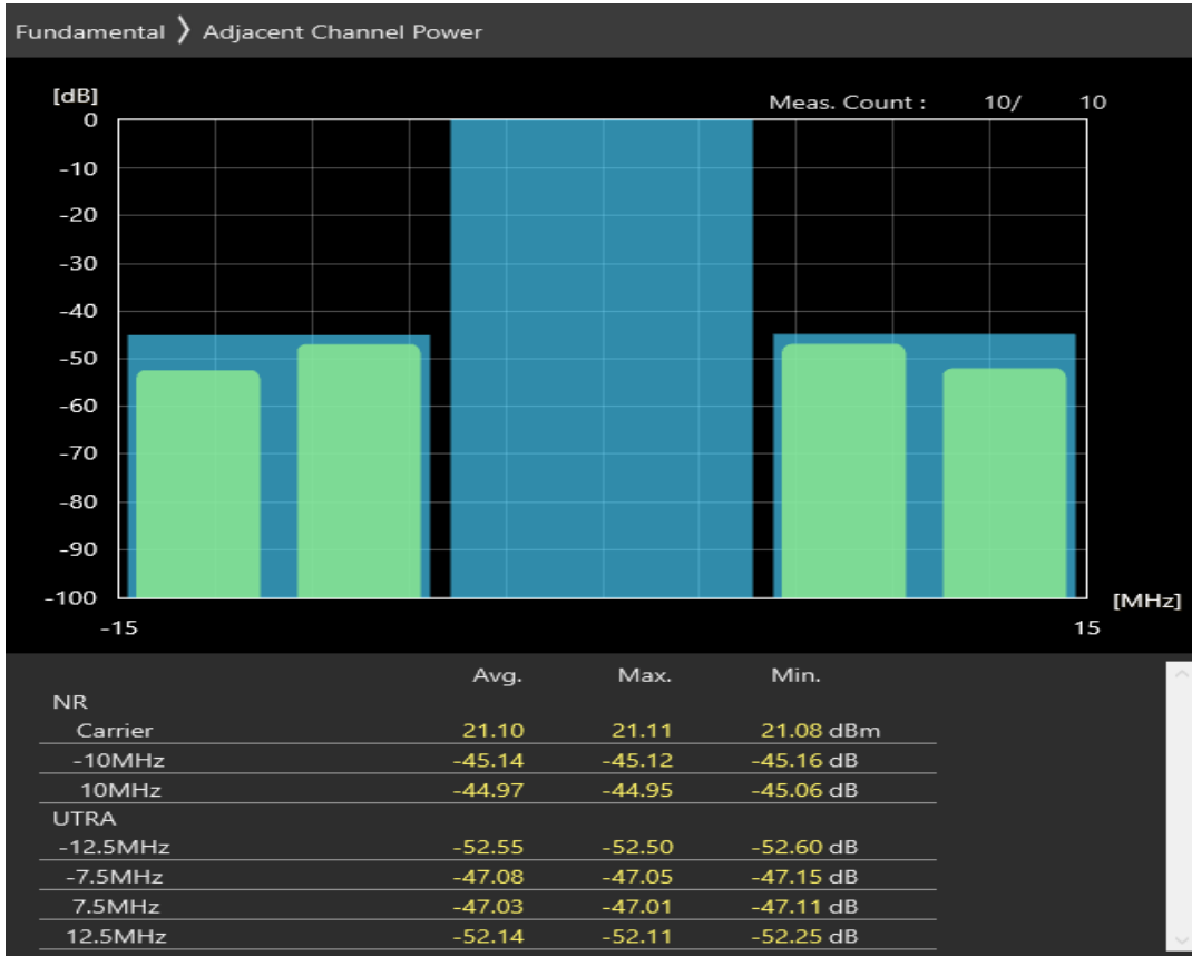
n78 SCS=30kHz CP_QPSK BW=10MHz Channel=647000 RB=1@0
