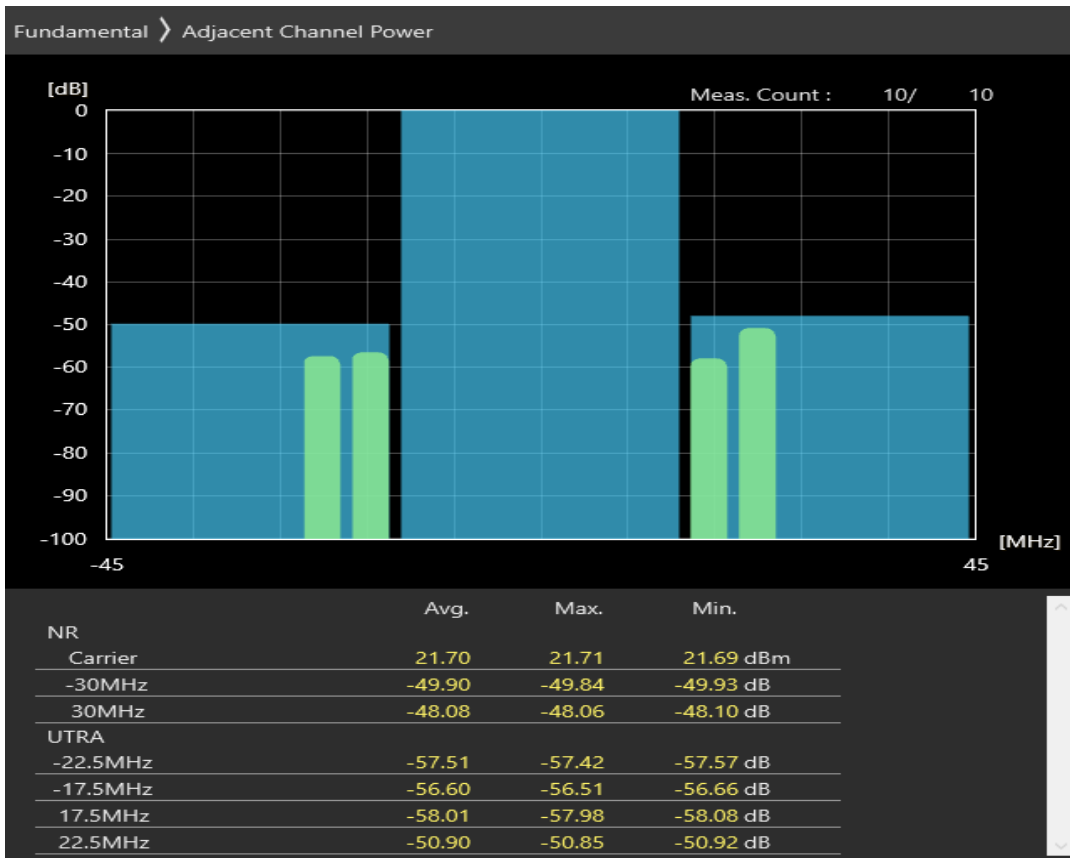
n3 SCS=30kHz CP_QAM16 BW=30MHz Channel=345000 RB=1@0
