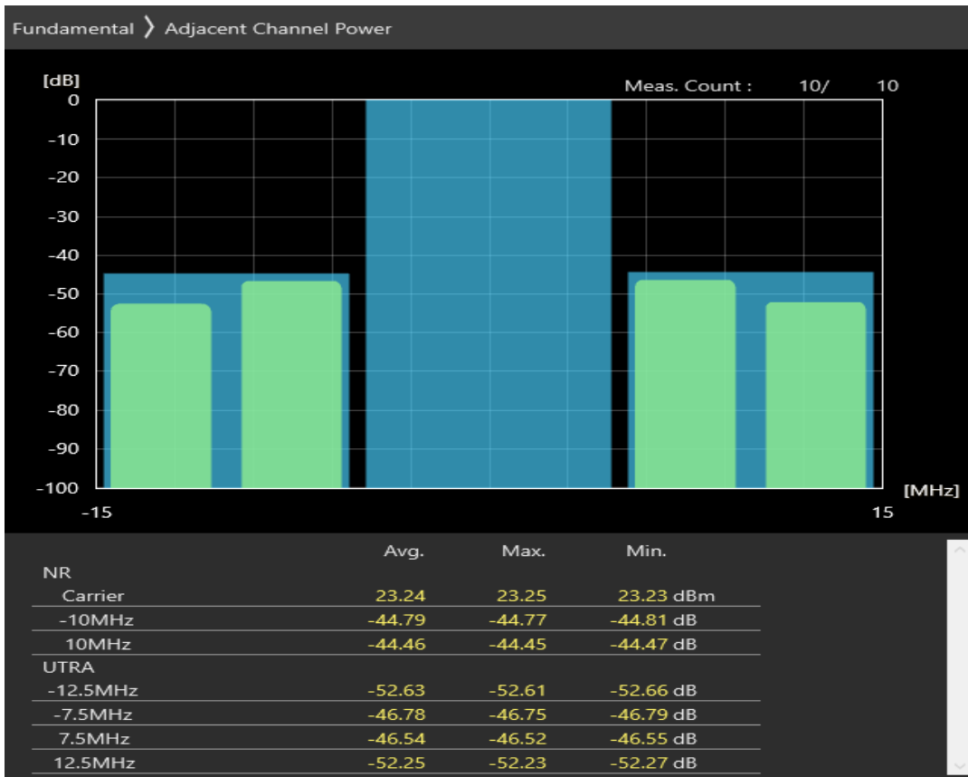
n38 SCS=30kHz DFT_QPSK BW=10MHz Channel=523000 RB=1@23
