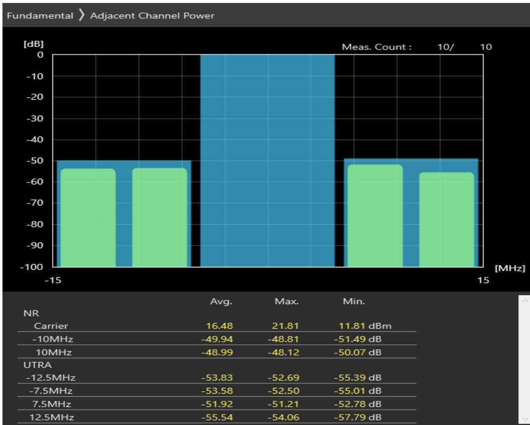
n78 SCS=30kHz CP_QAM16 BW=10MHz Channel=653000 RB=24@0
