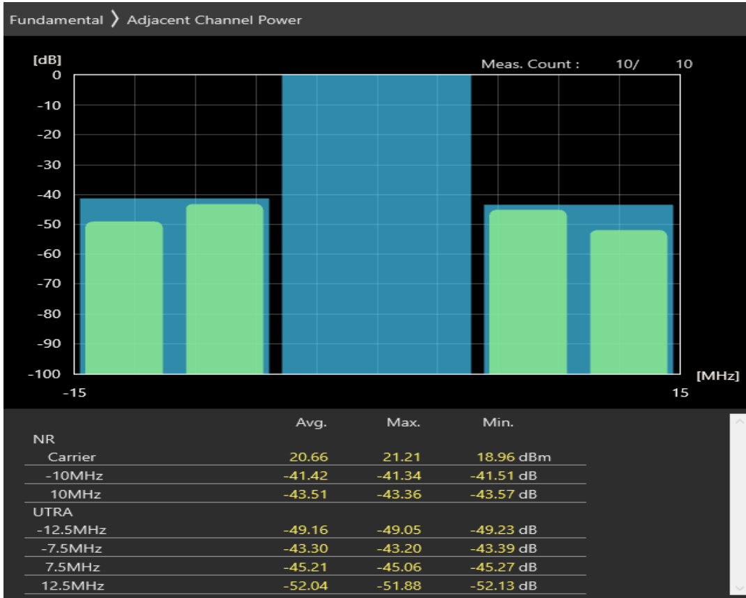
n3 SCS=30kHz DFT_QAM64 BW=10MHz Channel=356000 RB=1@23
