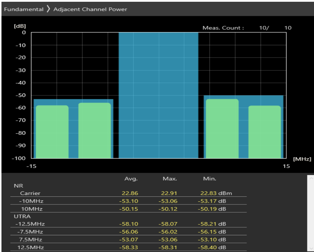
n78 SCS=30kHz DFT_QAM16 BW=10MHz Channel=653000 RB=24@0
