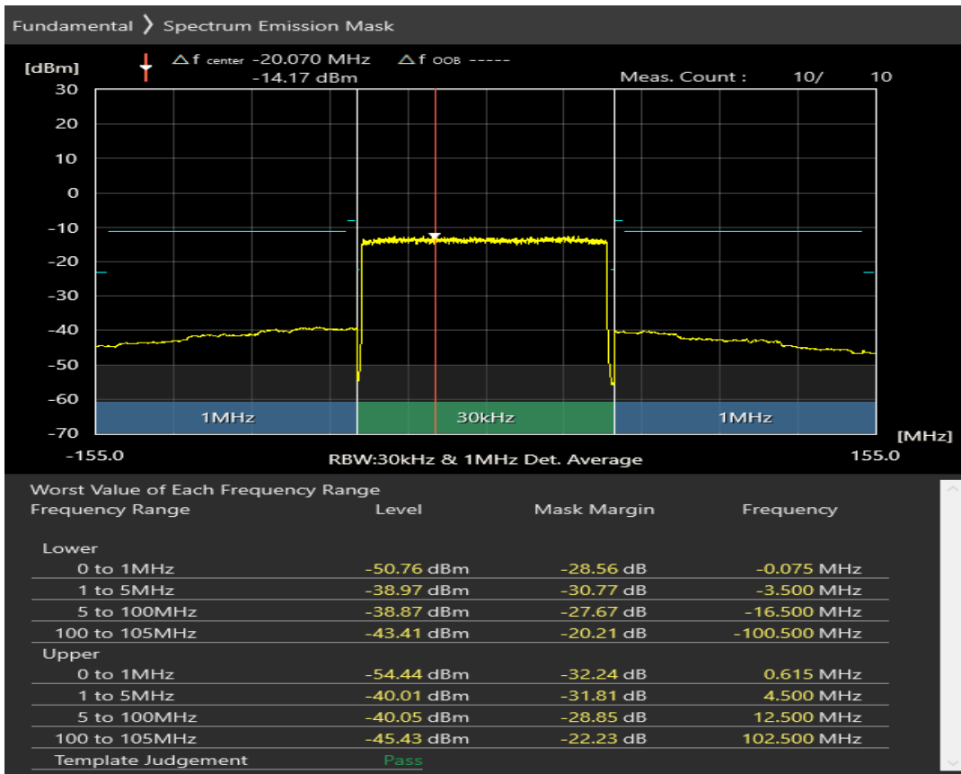
n77 SCS=30kHz DFT_QAM256 BW=100MHz Channel=623334 RB=1@0
