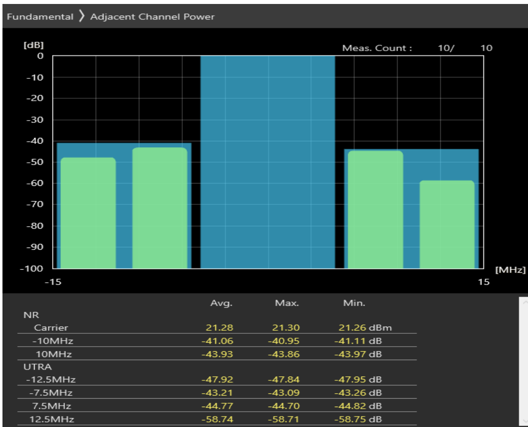
n28 SCS=30kHz DFT_QAM256 BW=10MHz Channel=148600 RB=1@23
