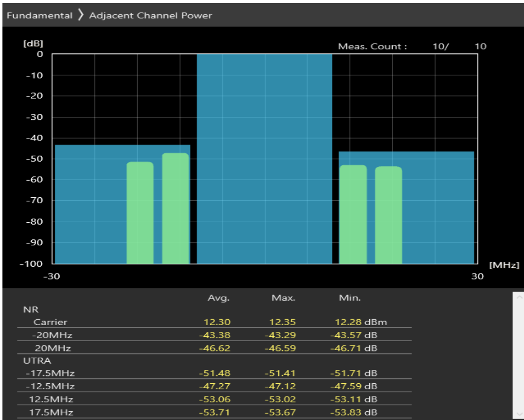
n8 SCS=30kHz CP_QAM64 BW=20MHz Channel=181000 RB=1 @50
