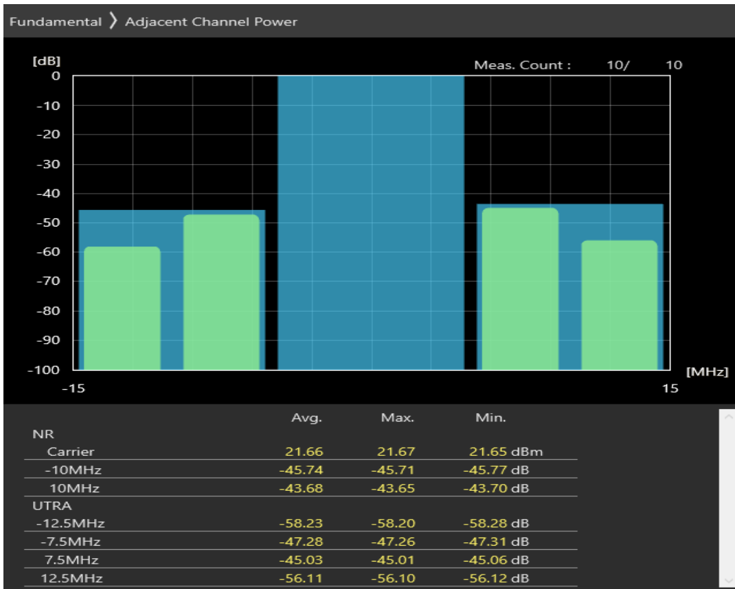
n28 SCS=30kHz CP_QAM16 BW=10MHz Channel=141600 RB=1@0
