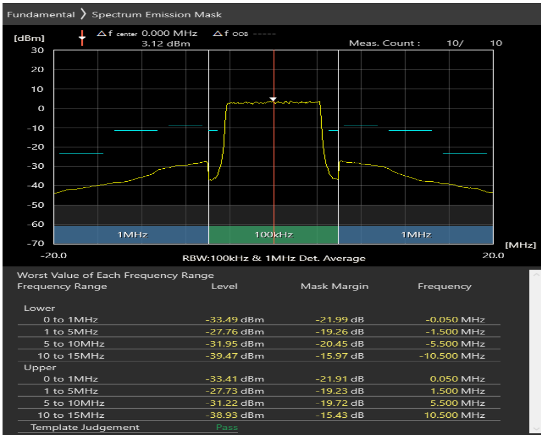
n38 SCS=30kHz DFT_QAM64 BW=10MHz Channel=515000 RB=1@0
