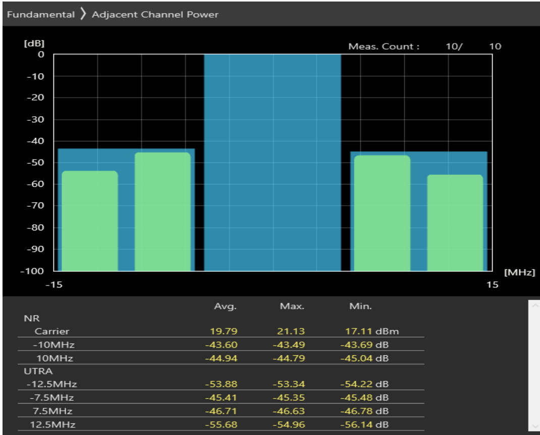
n3 SCS=30kHz CP_QAM16 BW=10MHz Channel=356000 RB=1@23
