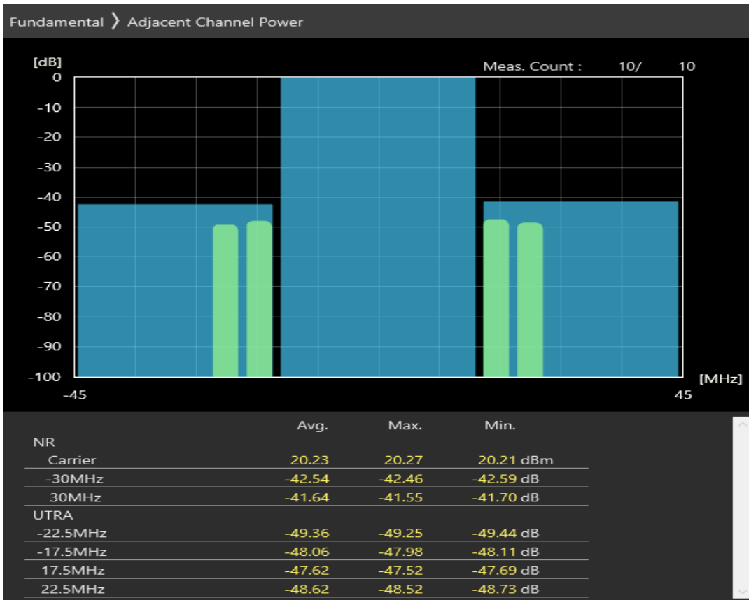
n3 SCS=30kHz DFT_QAM64 BW=30MHz Channel=345000 RB=1@0
