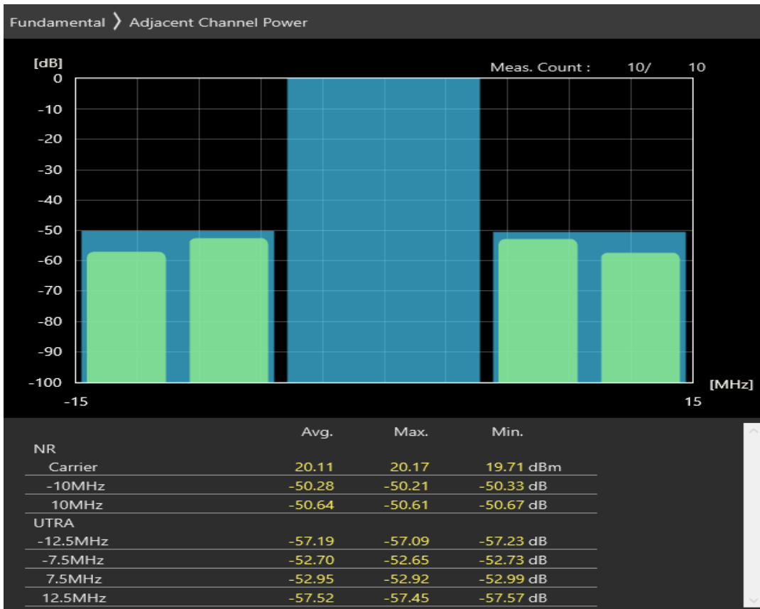
n77 SCS=30kHz CP_QPSK BW=10MHz Channel=679666 RB=1@23
