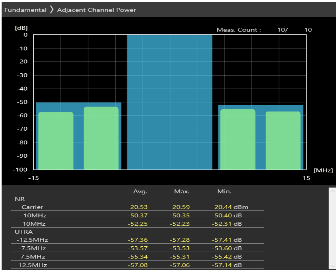
n1 SCS=30kHz DFT_QAM64 BW=10MHz Channel=385000 RB=24@0
