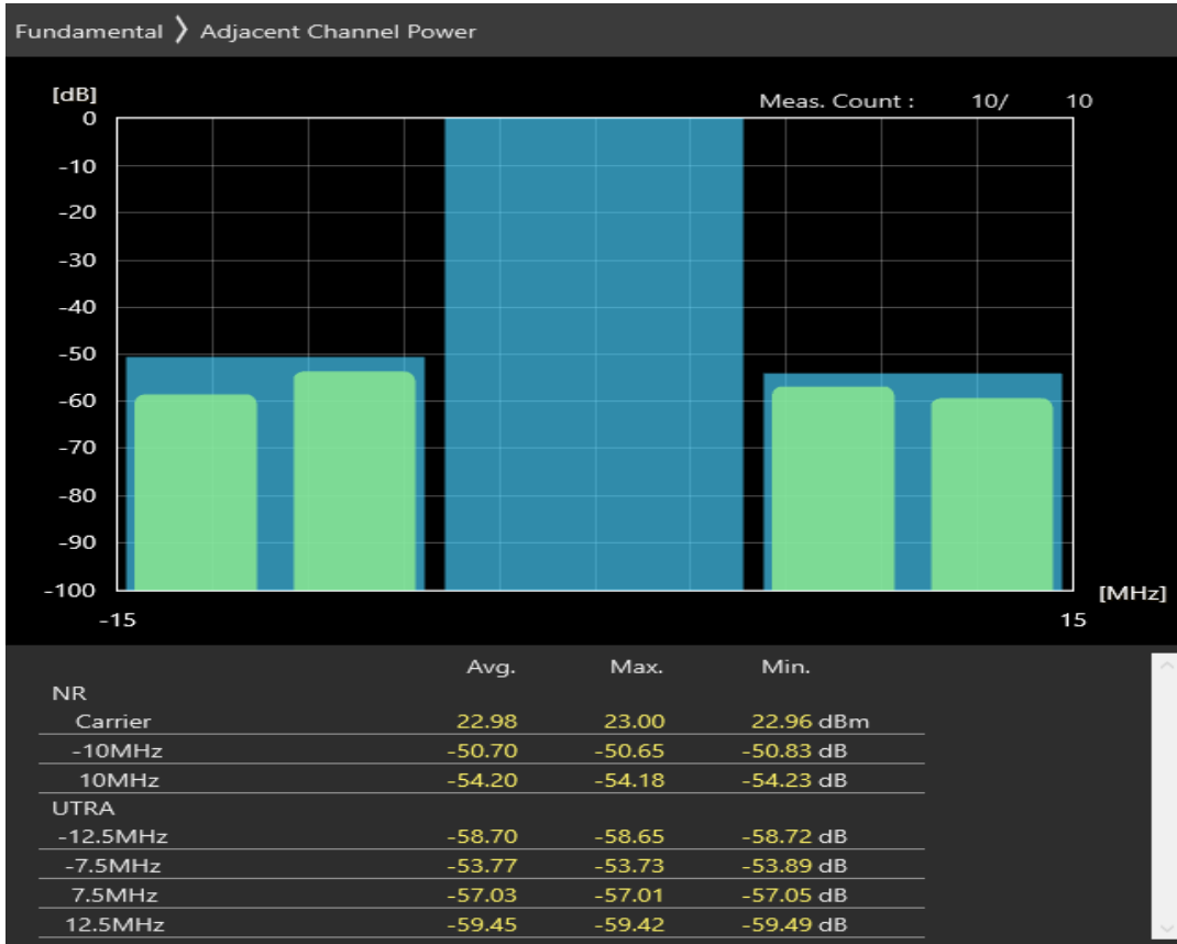
n77 SCS=30kHz DFT_BPSK BW=10MHz Channel=620334 RB=24@0
