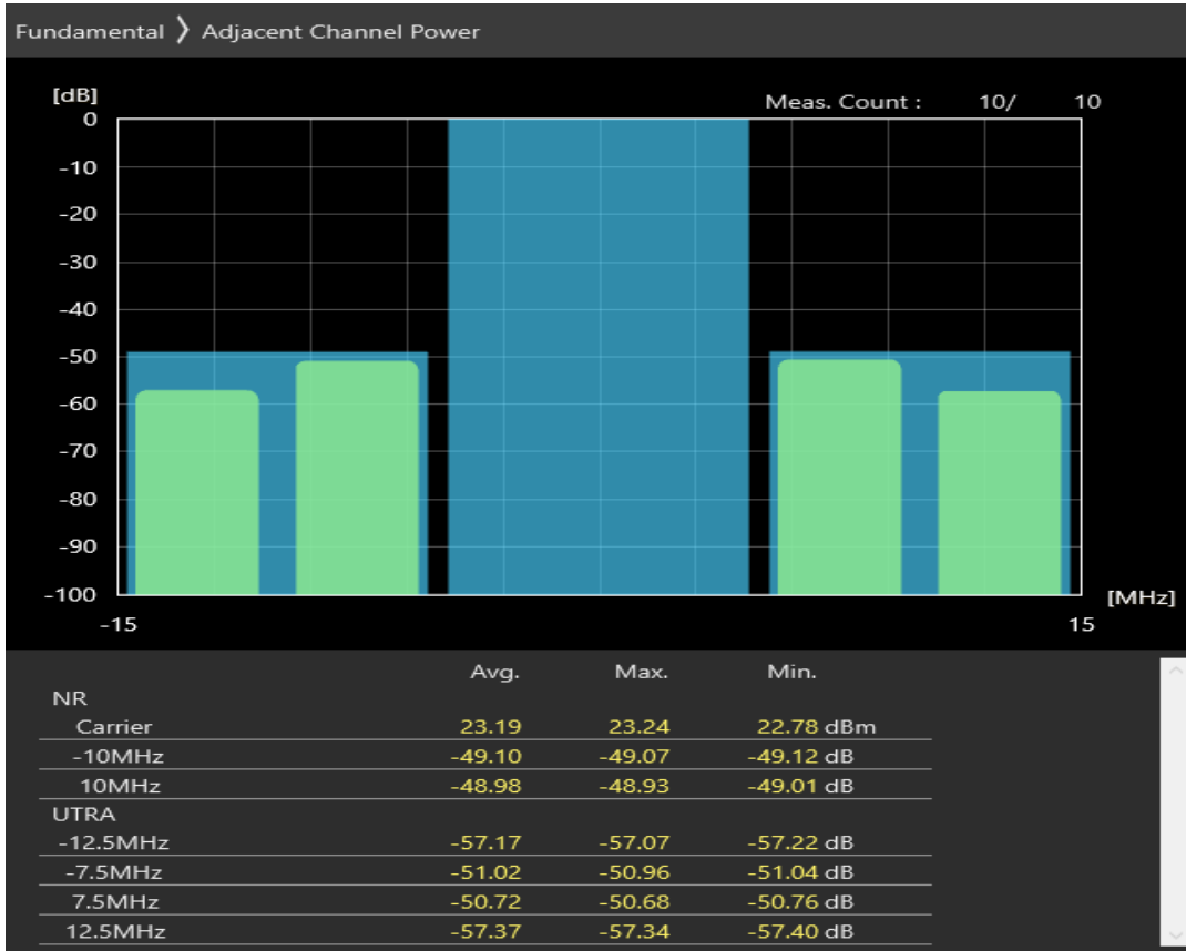
n38 SCS=30kHz DFT_QAM16 BW=10MHz Channel=523000 RB=1@23
