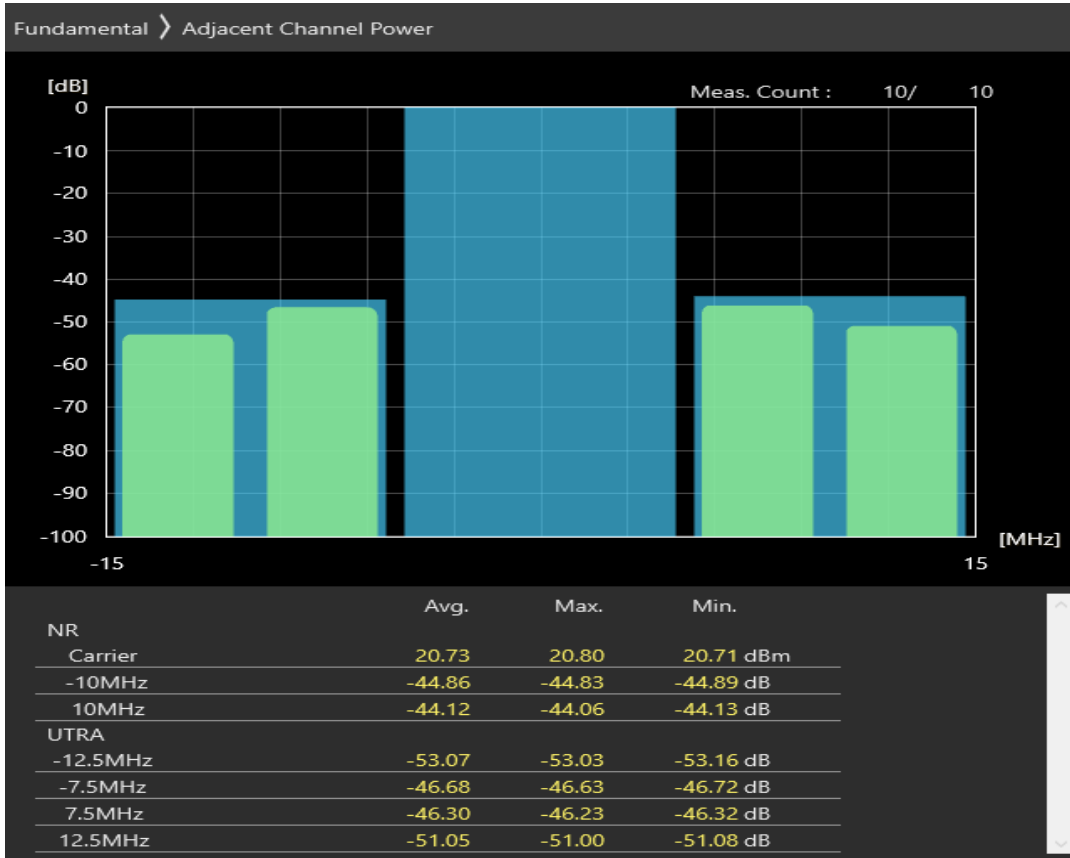
n1 SCS=30kHz DFT_QAM64 BW=10MHz Channel=395000 RB=1@23
