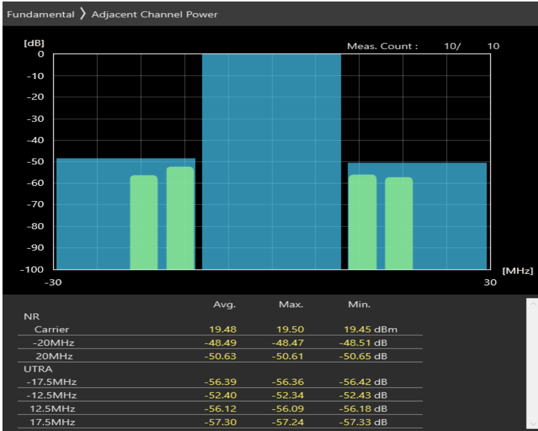
n1 SCS=30kHz CP_QAM64 BW=20MHz Channel=394000 RB=1@50
