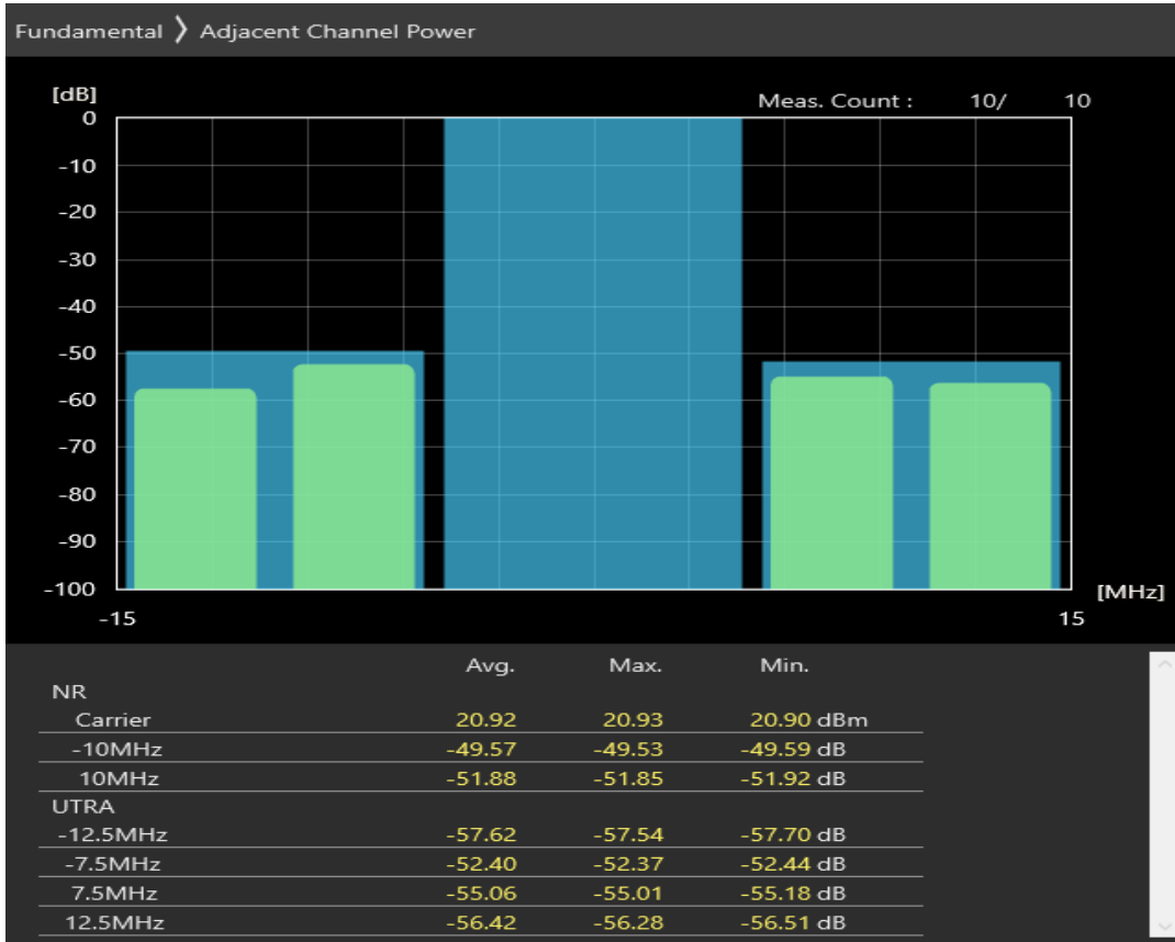
n78 SCS=30kHz CP_QAM16 BW=10MHz Channel=647000 RB=24@0
