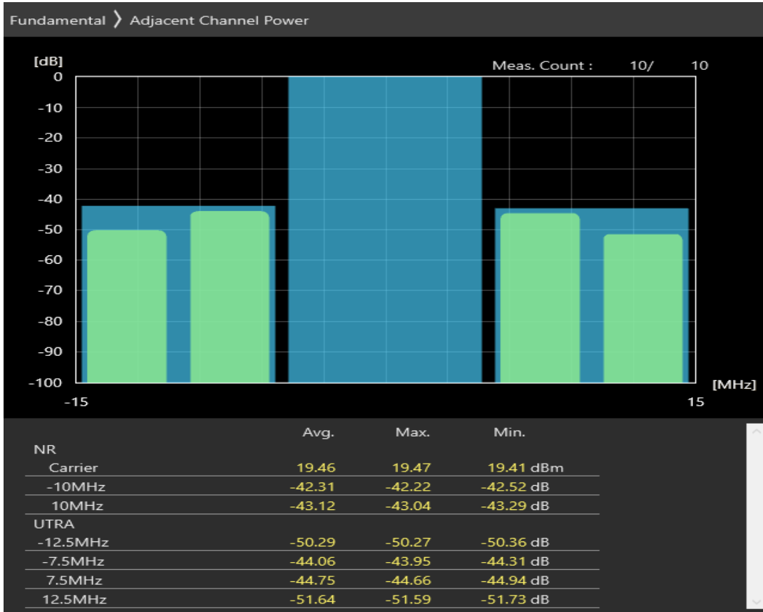
n1 SCS=30kHz DFT_BPSK BW=20MHz Channel=386000 RB=1@0
