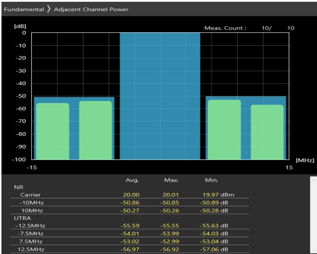
n20 SCS=30kHz CP_QAM64 BW=10MHz Channel=171400 RB=24@0
