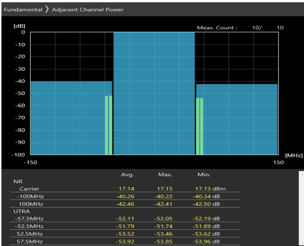
n77 SCS=30kHz DFT_QAM16 BW=100MHz Channel=623334 RB=135@67
