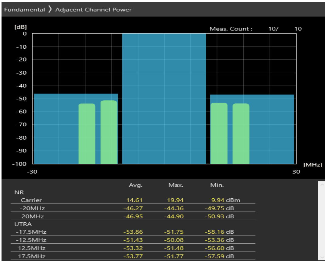
n28 SCS=30kHz CP_QAM256 BW=20MHz Channel=142600 RB=1@0
