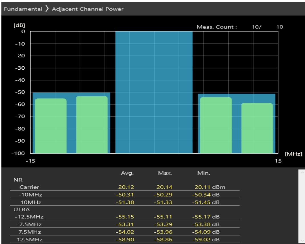
n28 SCS=30kHz CP_QAM64 BW=10MHz Channel=148600 RB=24@0
