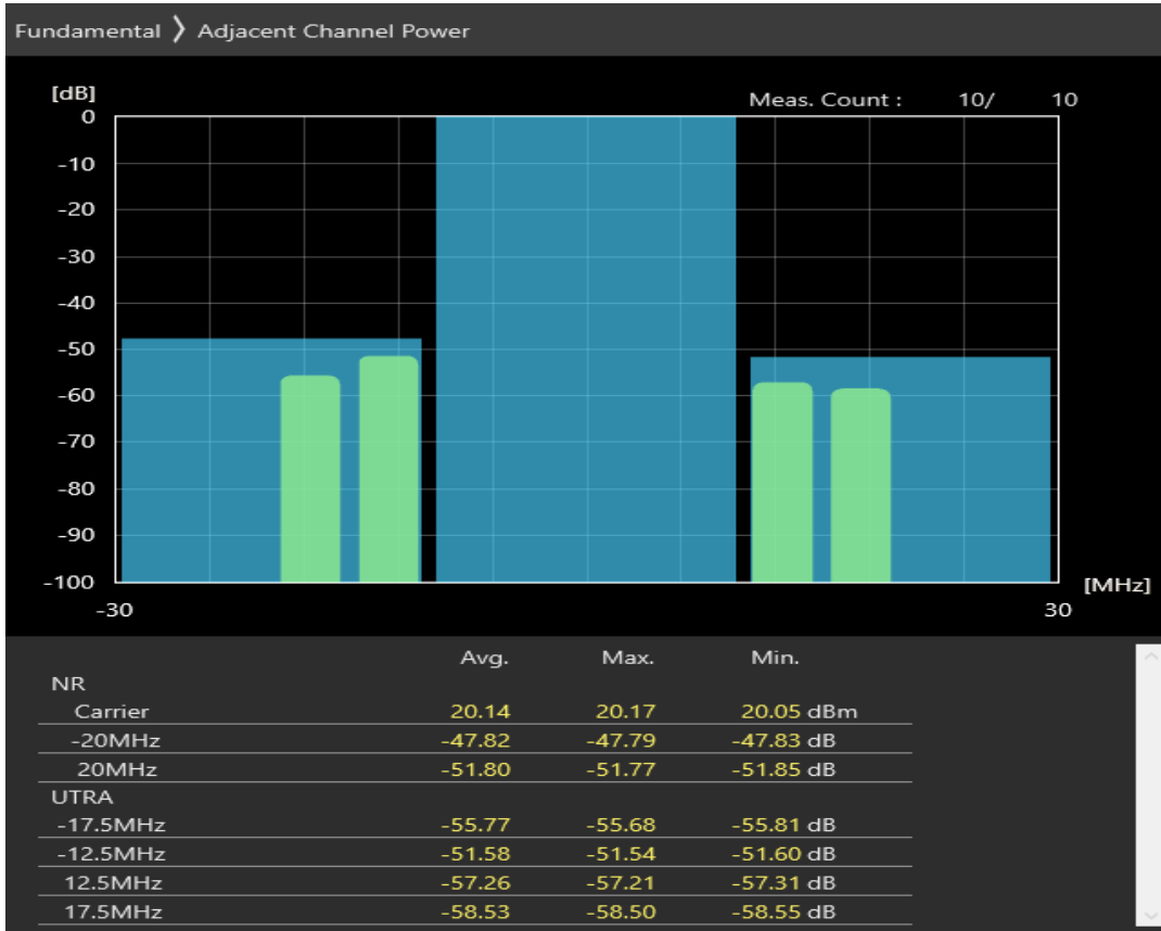
n1 SCS=30kHz CP_QAM256 BW=10MHz Channel=385000 RB=1@0
