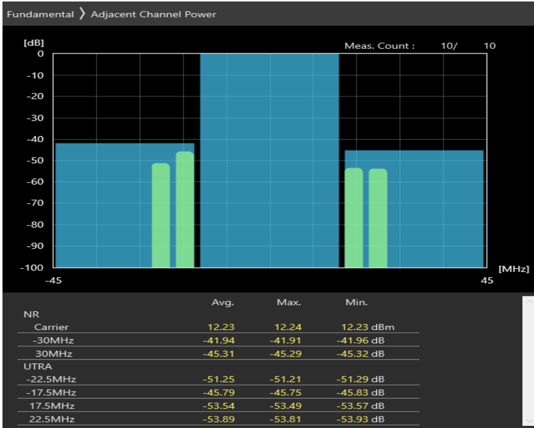
n38 SCS=30kHz DFT_BPSK BW=10MHz Channel=515000 RB=12@6
