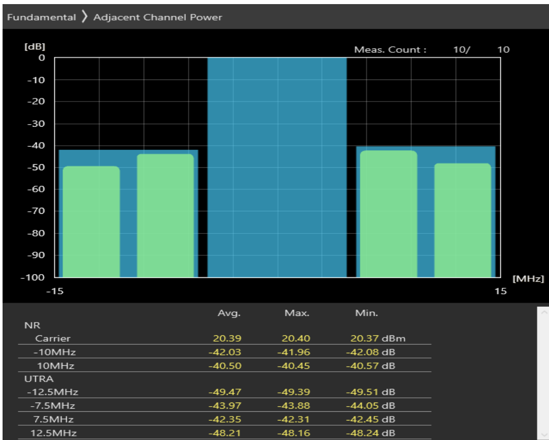
n3 SCS=30kHz DFT_BPSK BW=10MHz Channel=356000 RB=12@6
