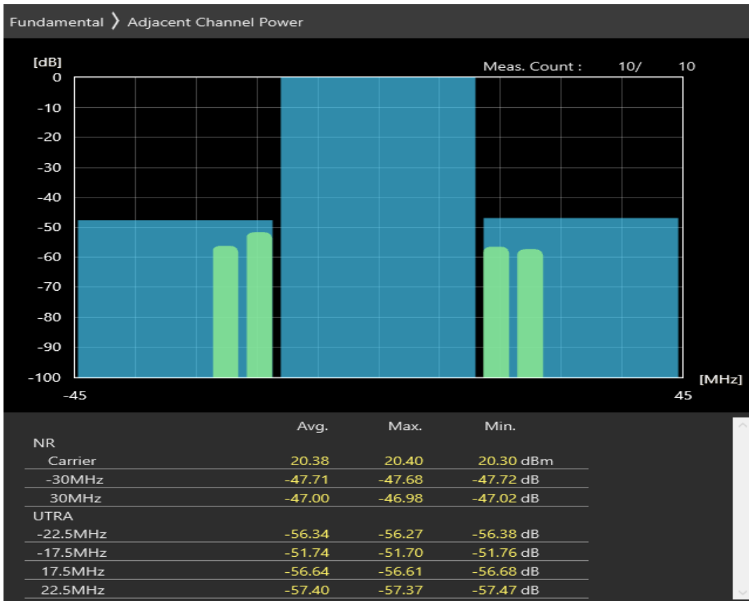
n3 SCS=30kHz CP_QAM64 BW=30MHz Channel=345000 RB=1@0
