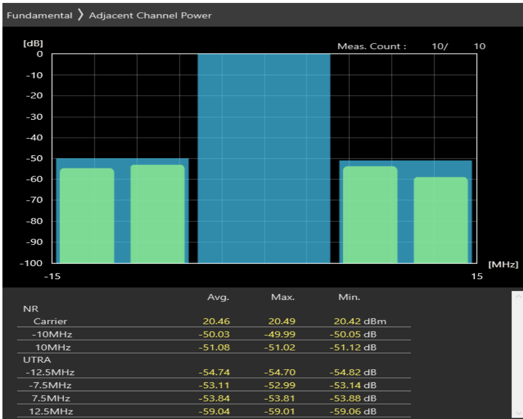
n28 SCS=30kHz CP_QAM16 BW=10MHz Channel=148600 RB=24@0
