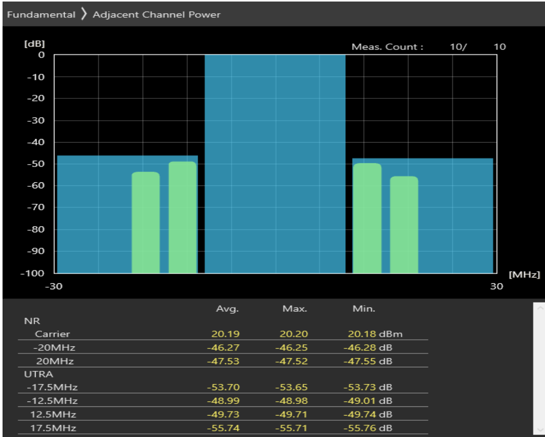
n20 SCS=30kHz DFT_QAM16 BW=20MHz Channel=170400 RB=1@50
