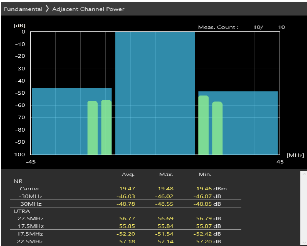
n3 SCS=30kHz CP_QAM64 BW=30MHz Channel=354000 RB=78@0
