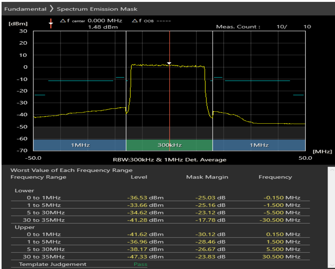
n3 SCS=30kHz CP_QPSK BW=30MHz Channel=354000 RB=1@77
