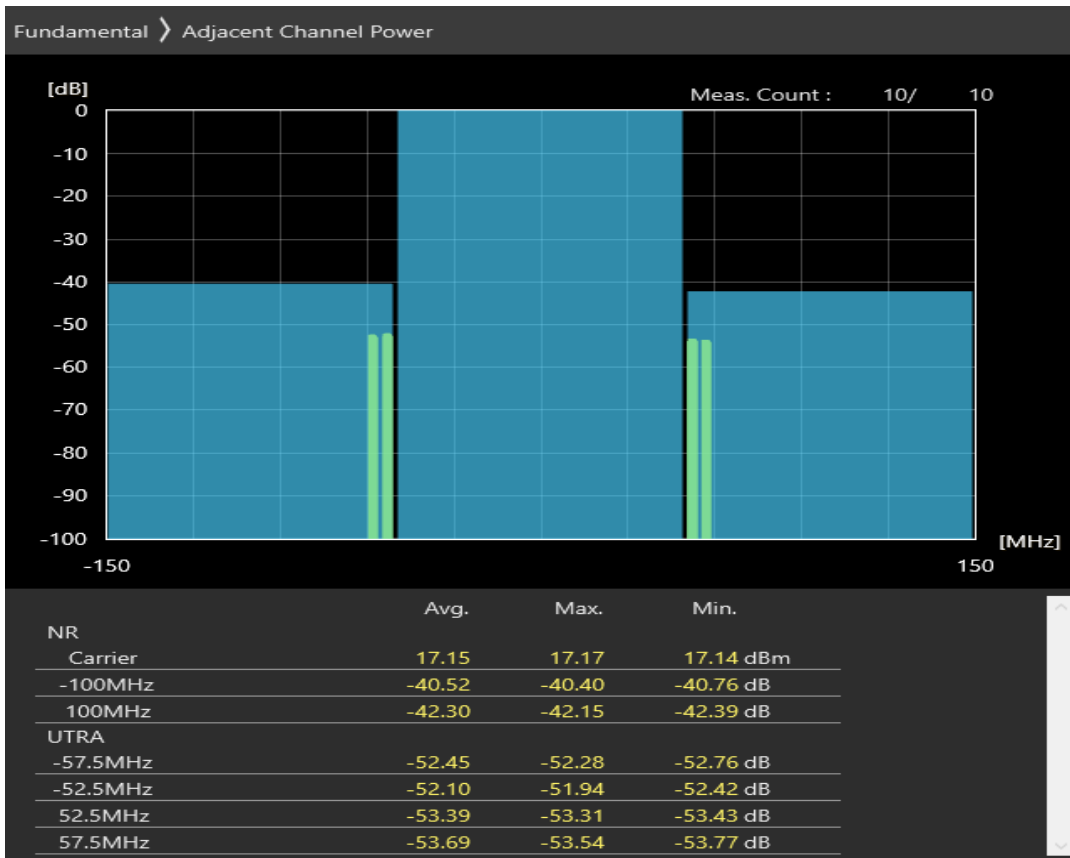
n77 SCS=30kHz DFT_QPSK BW=100MHz Channel=623334 RB=135@67
