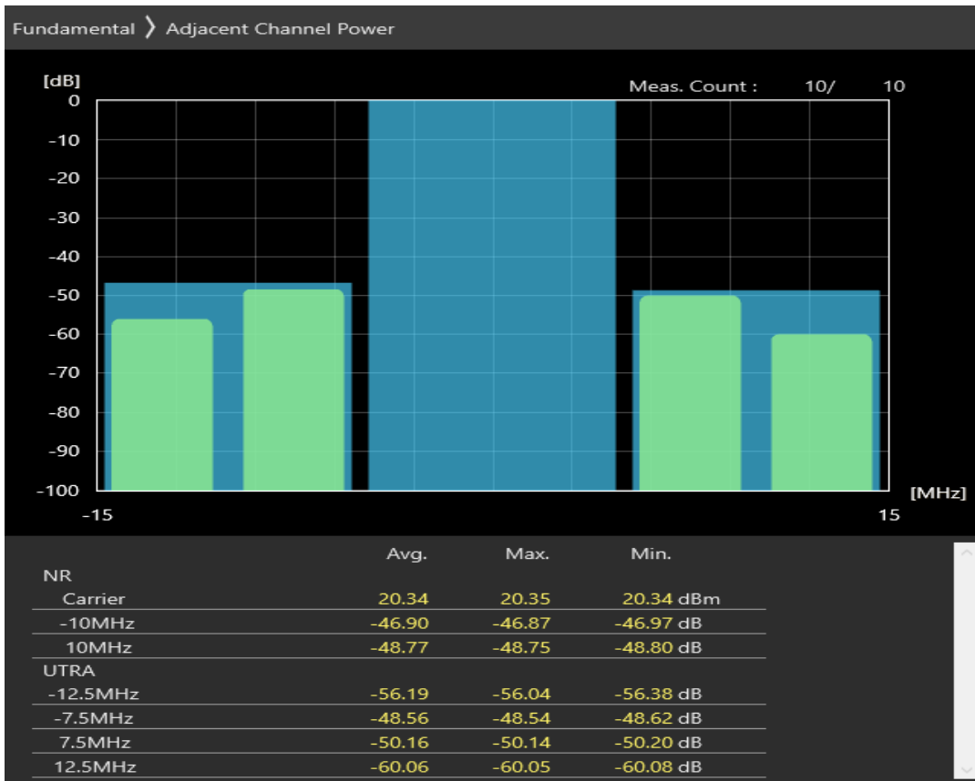
n8 SCS=30kHz DFT_BPSK BW=10MHz Channel=182000 RB=1@23
