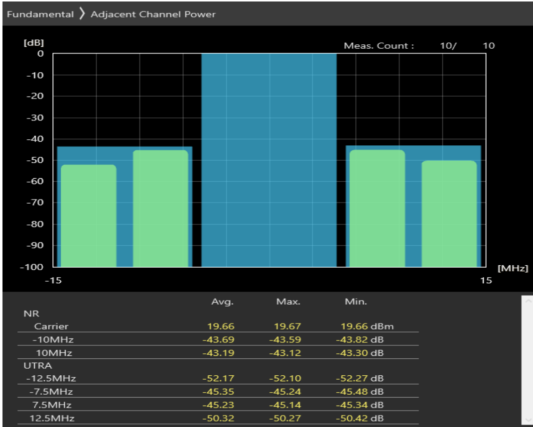
n1 SCS=30kHz CP_QAM256 BW=10MHz Channel=395000 RB=1@23
