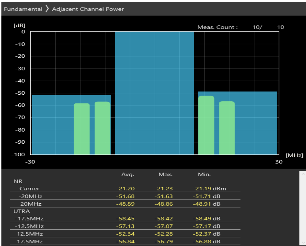
n38 SCS=30kHz CP_QAM16 BW=20MHz Channel=522000 RB=51 @0
