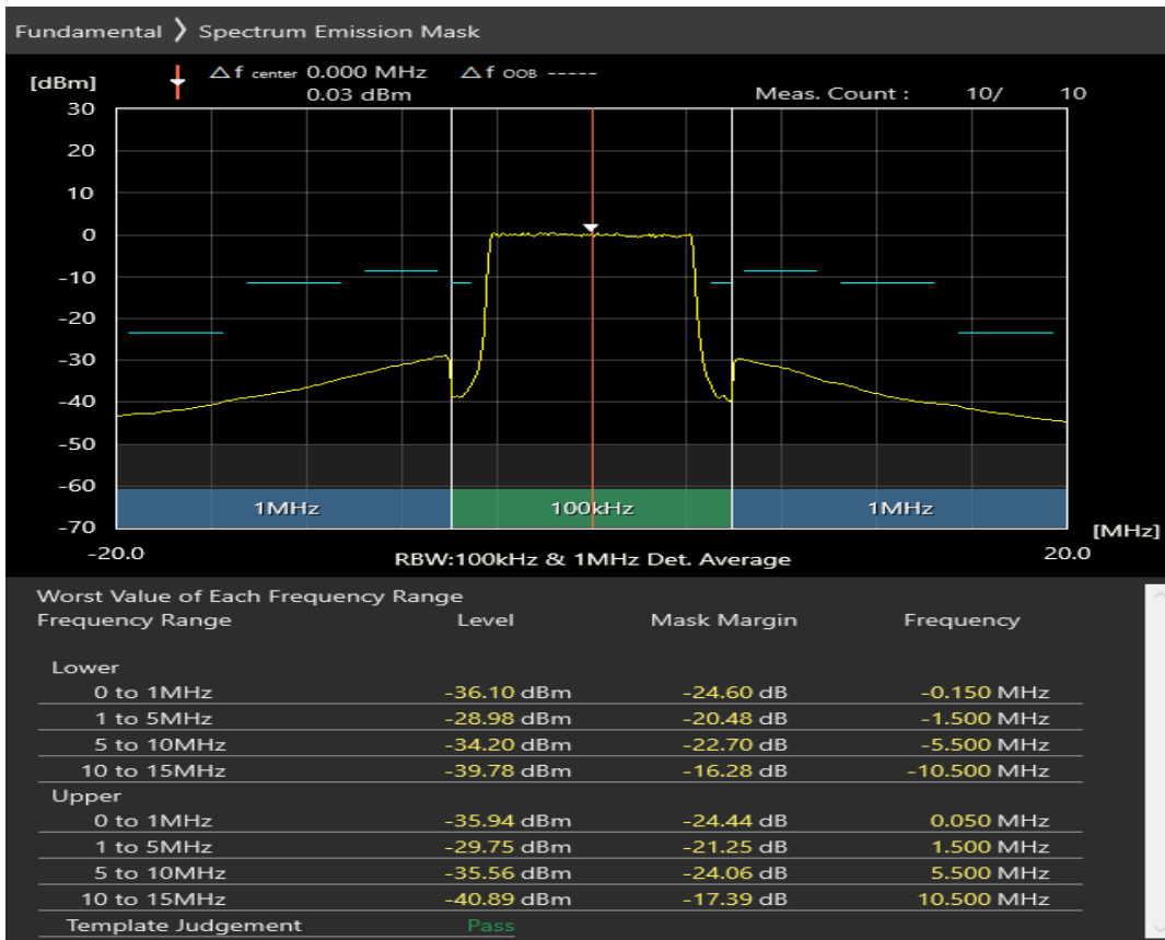
n1 SCS=30kHz DFT_QAM64 BW=10MHz Channel=395000 RB=1@23
