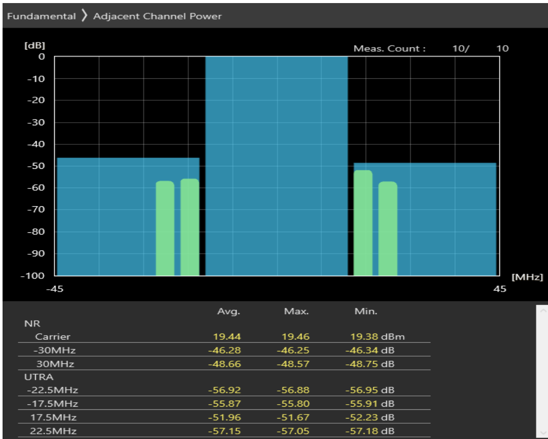
n3 SCS=30kHz DFT_QAM64 BW=30MHz Channel=354000 RB=75@0
