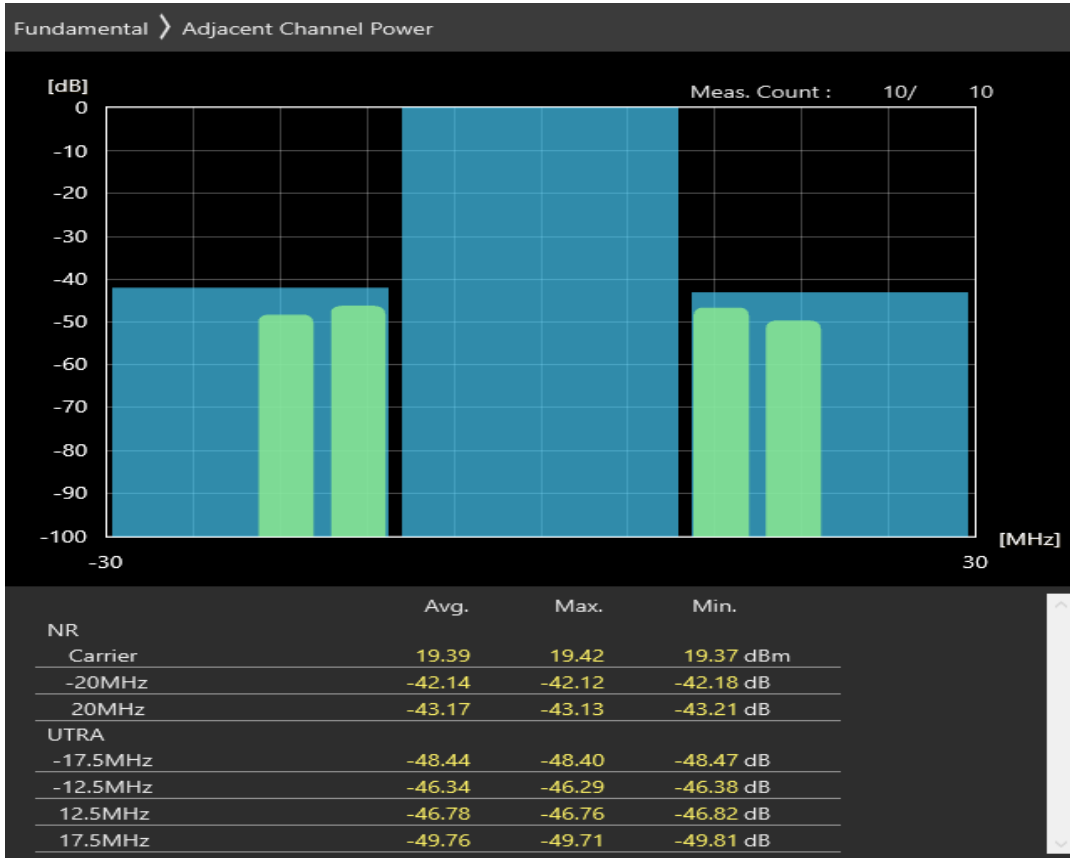
n1 SCS=30kHz DFT_QAM16 BW=10MHz Channel=385000 RB=12@6
