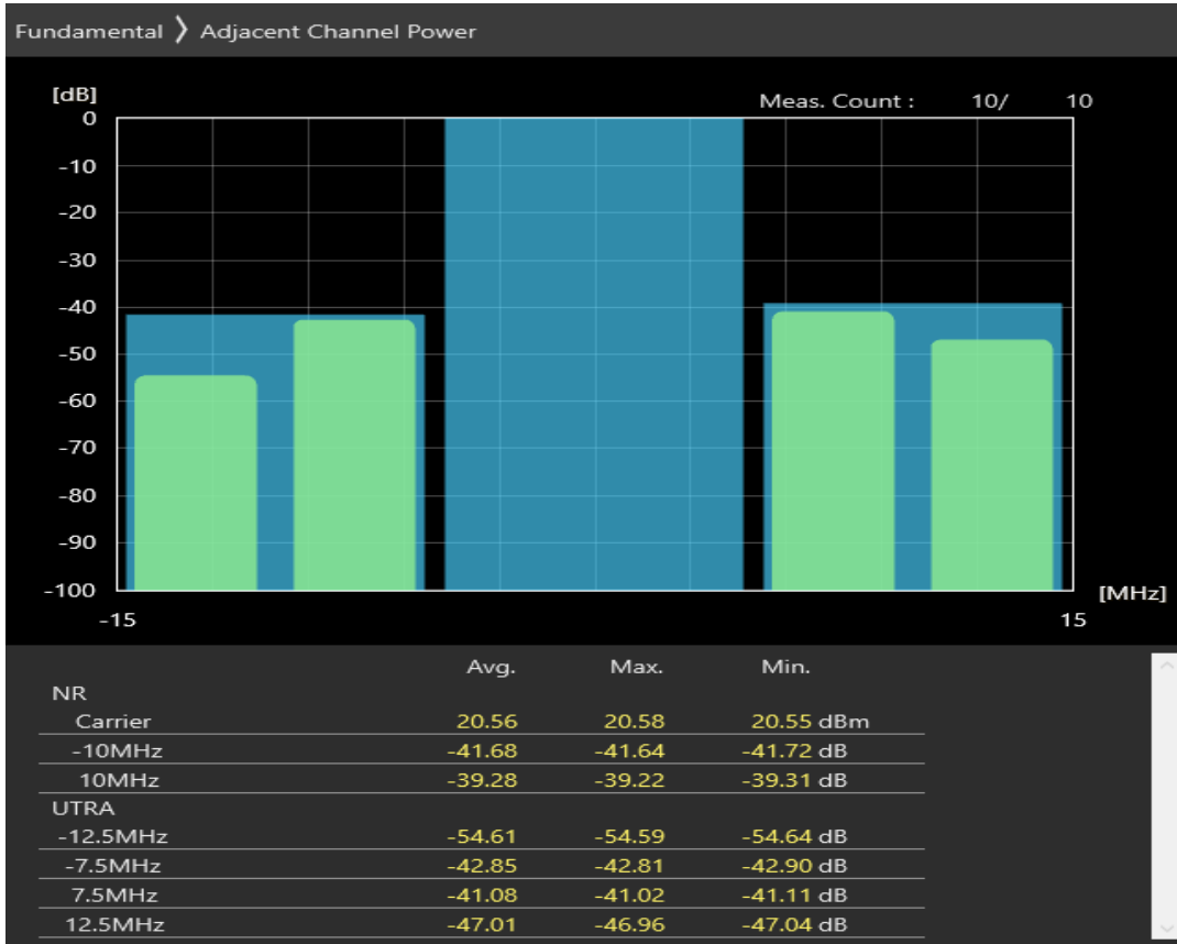
n28 SCS=30kHz CP_QAM16 BW=10MHz Channel=141600 RB=12@6
