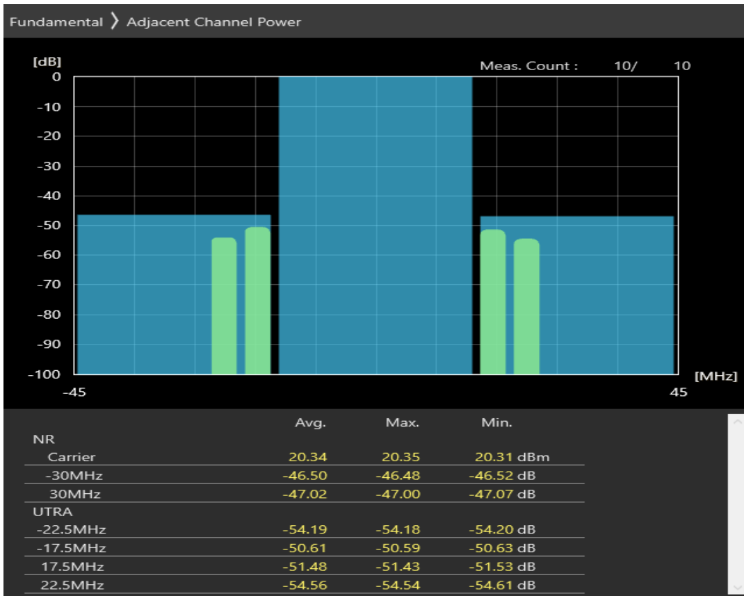
n3 SCS=30kHz DFT_BPSK BW=30MHz Channel=345000 RB=1@0
