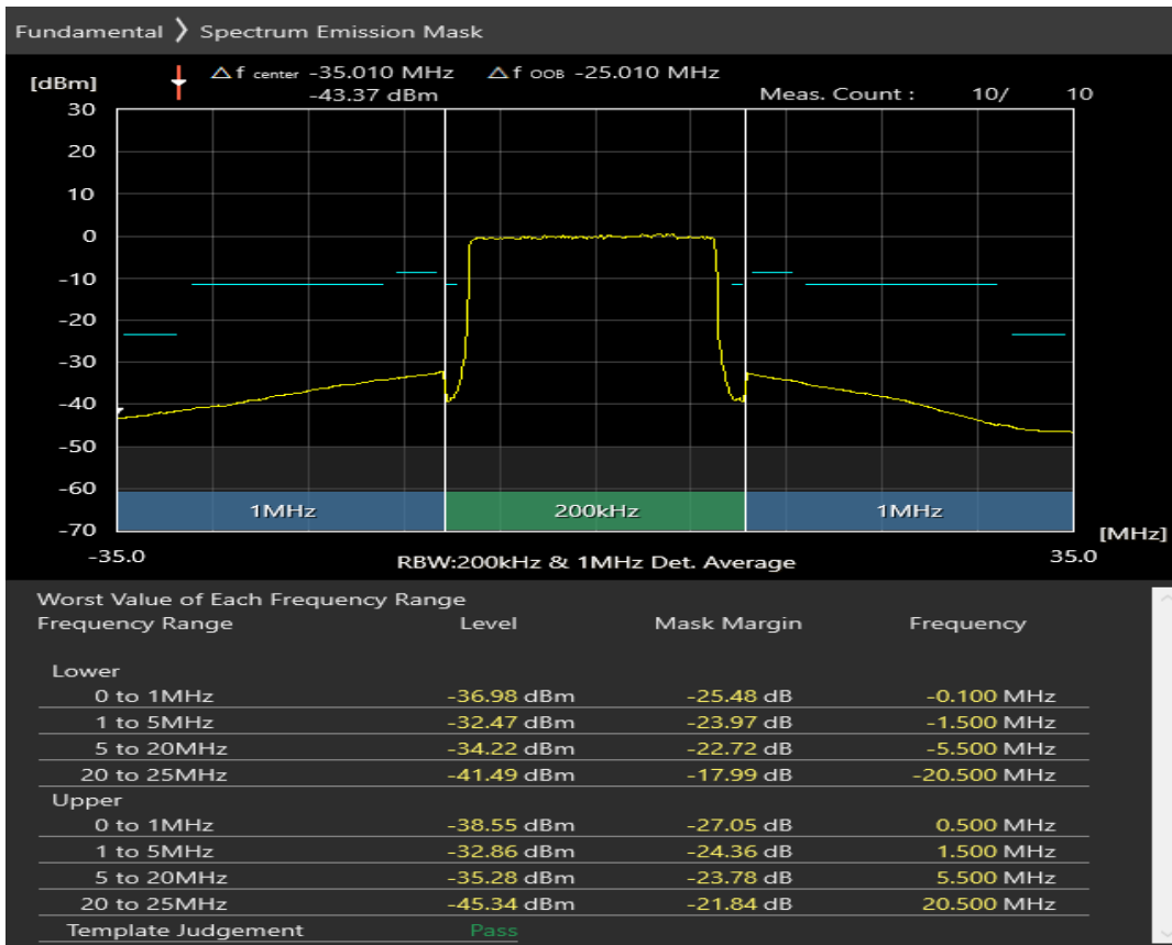
n1 SCS=30kHz DFT_QAM64 BW=20MHz Channel=394000 RB=1@50
