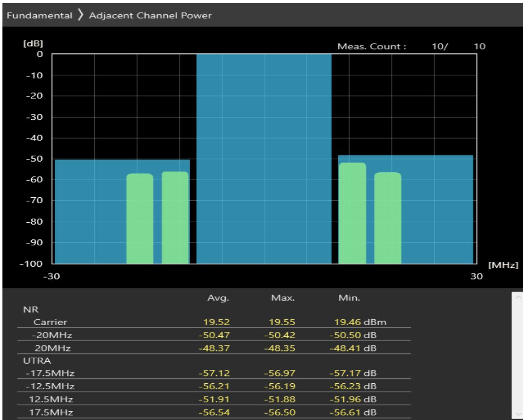
n1 SCS=30kHz CP_QAM64 BW=20MHz Channel=394000 RB=51@0
