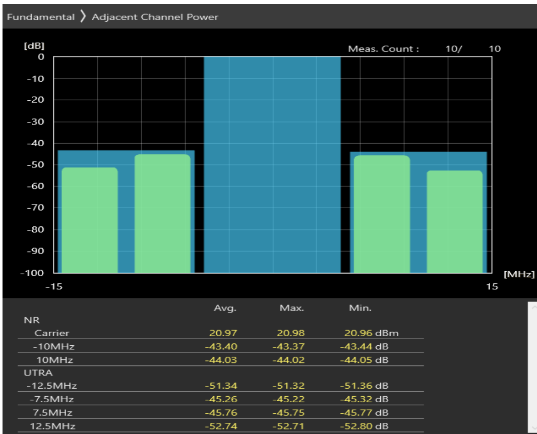
n1 SCS=30kHz DFT_QAM16 BW=20MHz Channel=386000 RB=1@0
