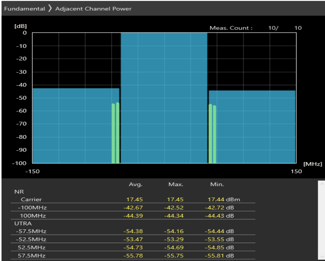
n77 SCS=30kHz DFT_QPSK BW=100MHz Channel=623334 RB=1@0
