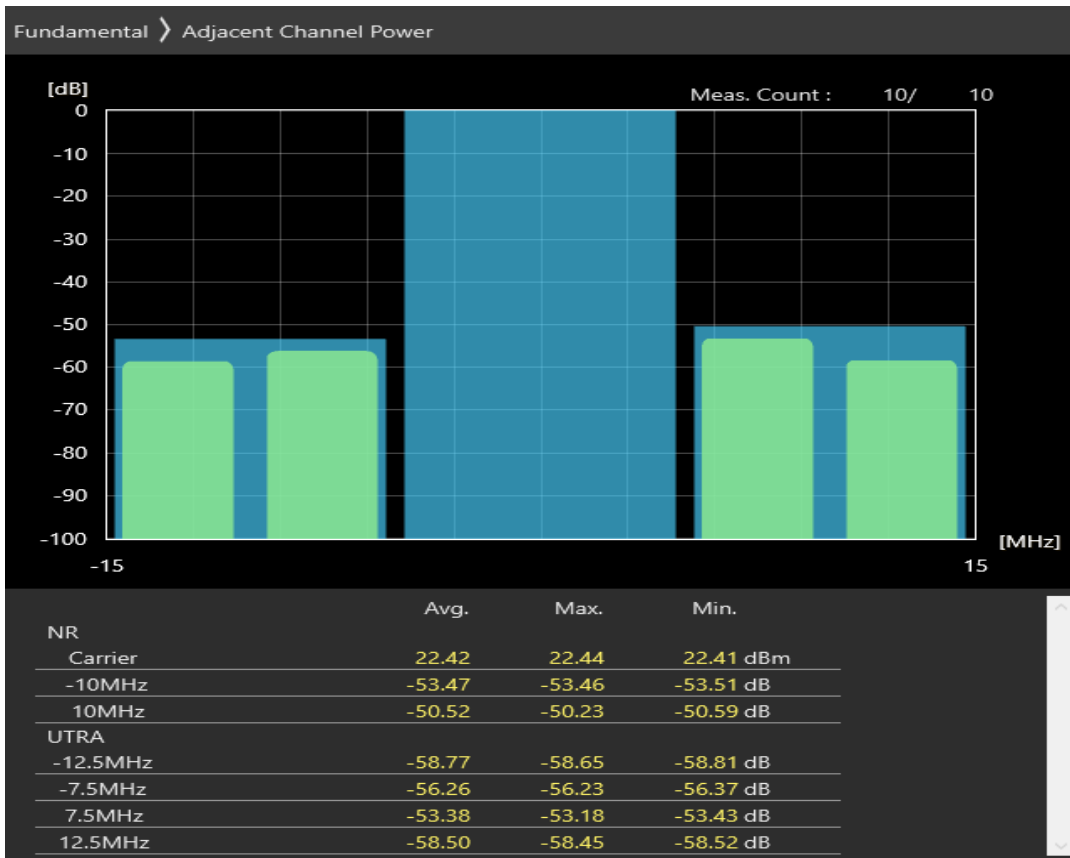
n78 SCS=30kHz DFT_QAM64 BW=10MHz Channel=653000 RB=24@0
