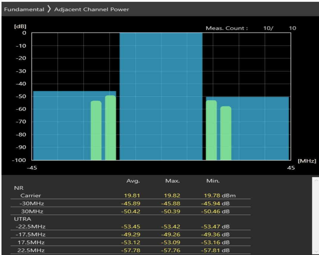
n3 SCS=30kHz DFT_QPSK BW=30MHz Channel=354000 RB=1@77
