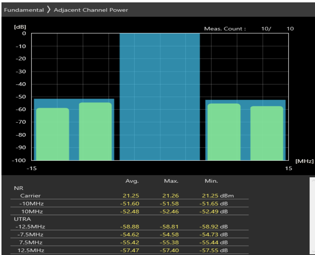
n28 SCS=30kHz DFT_QAM16 BW=10MHz Channel=141600 RB=24@0
