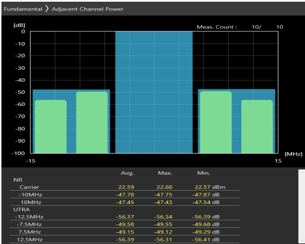
n38 SCS=30kHz CP_QAM16 BW=10MHz Channel=515000 RB=1@0
