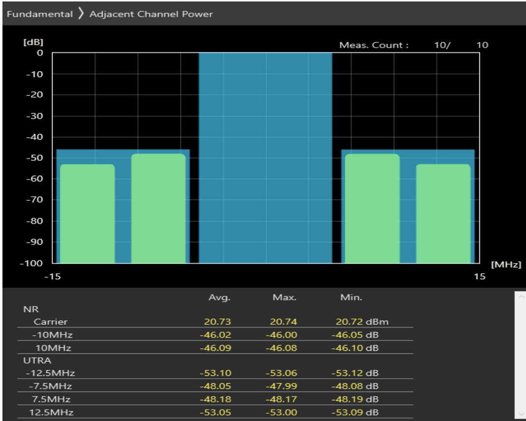
n77 SCS=30kHz CP_QAM16 BW=10MHz Channel=620334 RB=12@6
