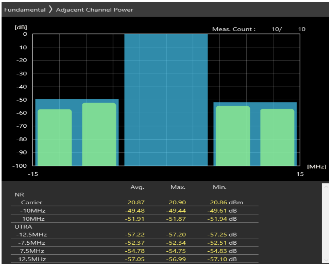
n78 SCS=30kHz CP_QPSK BW=10MHz Channel=647000 RB=24@0
