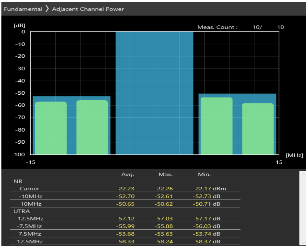
n38 SCS=30kHz DFT_QAM16 BW=10MHz Channel=523000 RB=24@0
