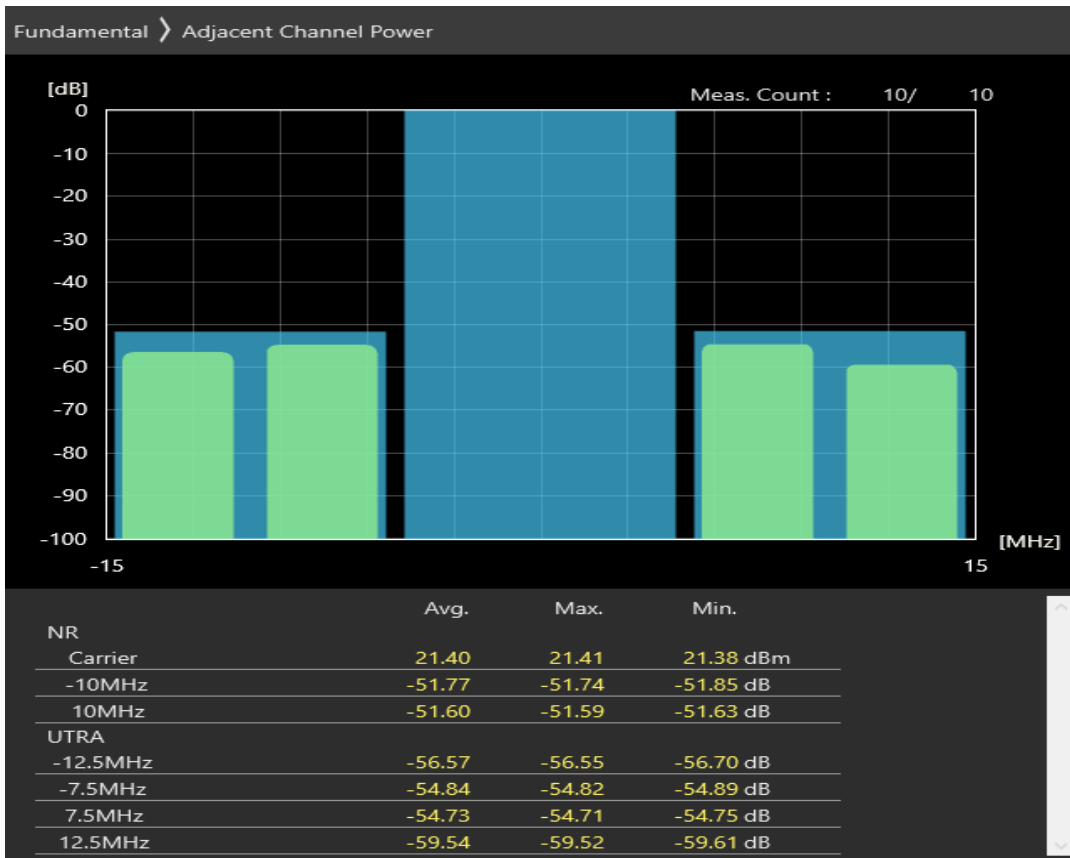
n28 SCS=30kHz DFT_QAM64 BW=10MHz Channel=148600 RB=24@0
