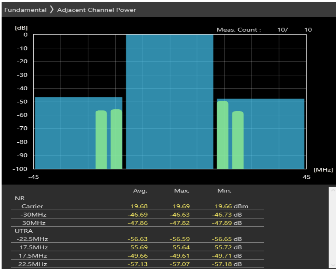
n3 SCS=30kHz CP_QAM16 BW=30MHz Channel=354000 RB=78@0
