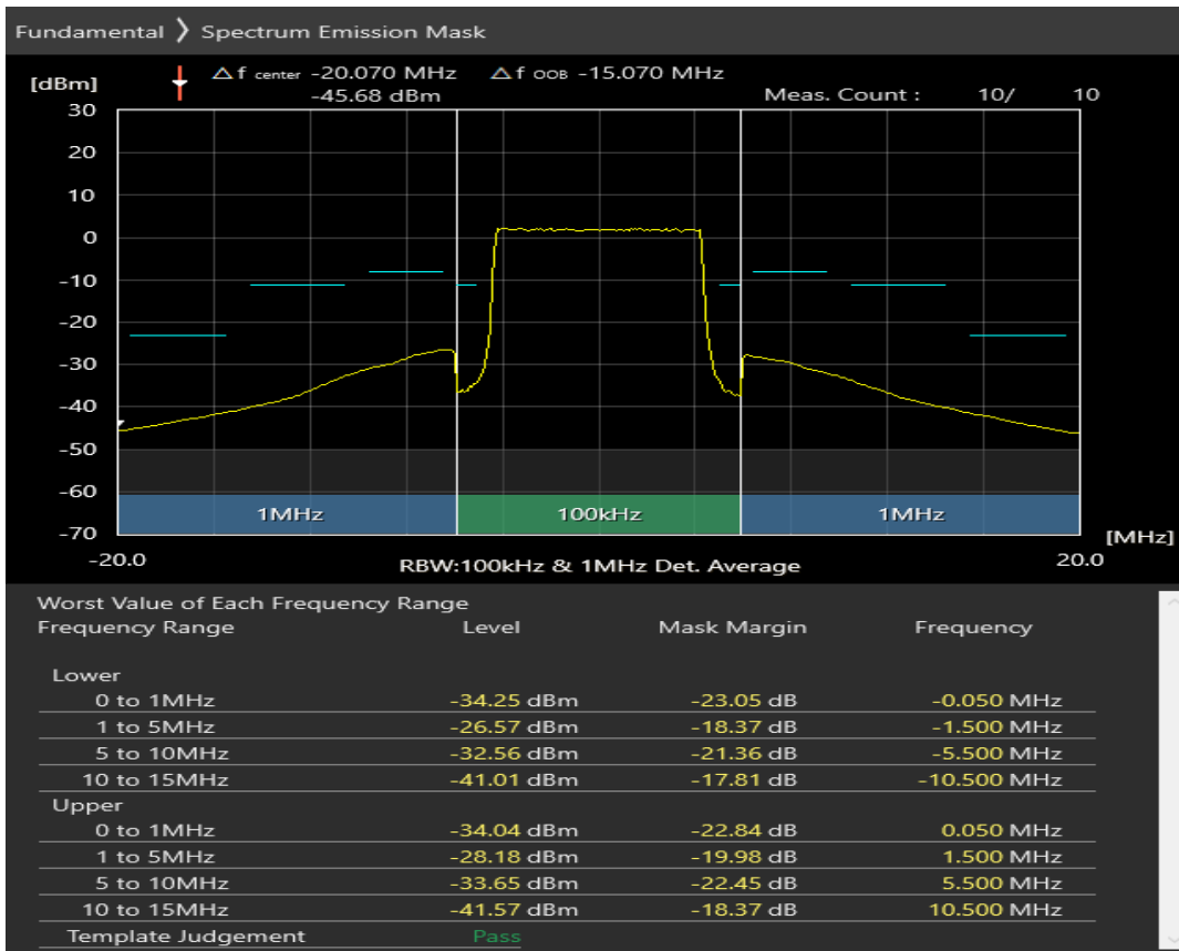
n77 SCS=30kHz DFT_BPSK BW=100MHz Channel=623334 RB=1@0
