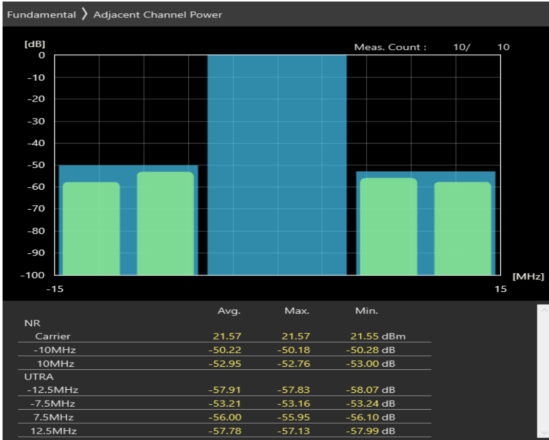
n77 SCS=30kHz DFT_QAM16 BW=10MHz Channel=620334 RB=24@0
