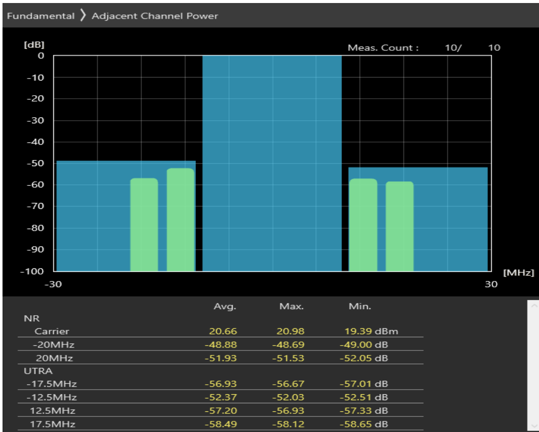
n38 SCS=30kHz CP_QAM256 BW=20MHz Channel=516000 RB=1@0
