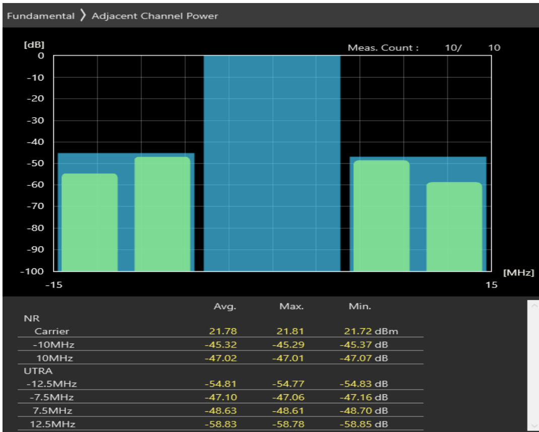
n8 SCS=30kHz CP_QAM16 BW=10MHz Channel=182000 RB=1@23
