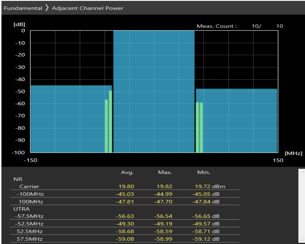
n78 SCS=30kHz CP_QAM256 BW=100MHz Channel=650000 RB=273@0
