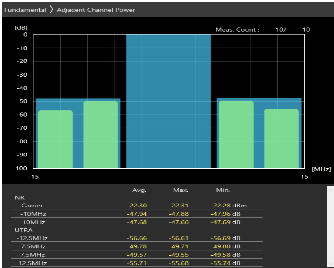
n1 SCS=30kHz DFT_QAM16 BW=10MHz Channel=385000 RB=1@0
