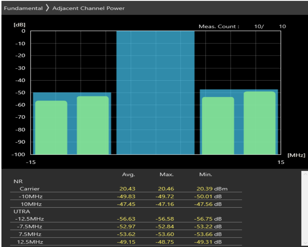
n3 SCS=30kHz CP_QAM64 BW=10MHz Channel=343000 RB=24@0
