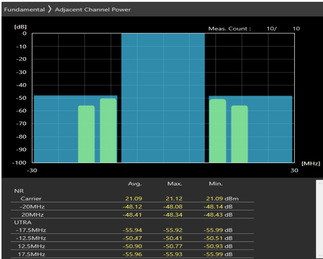
n38 SCS=30kHz DFT_BPSK BW=20MHz Channel=516000 RB=1@0
