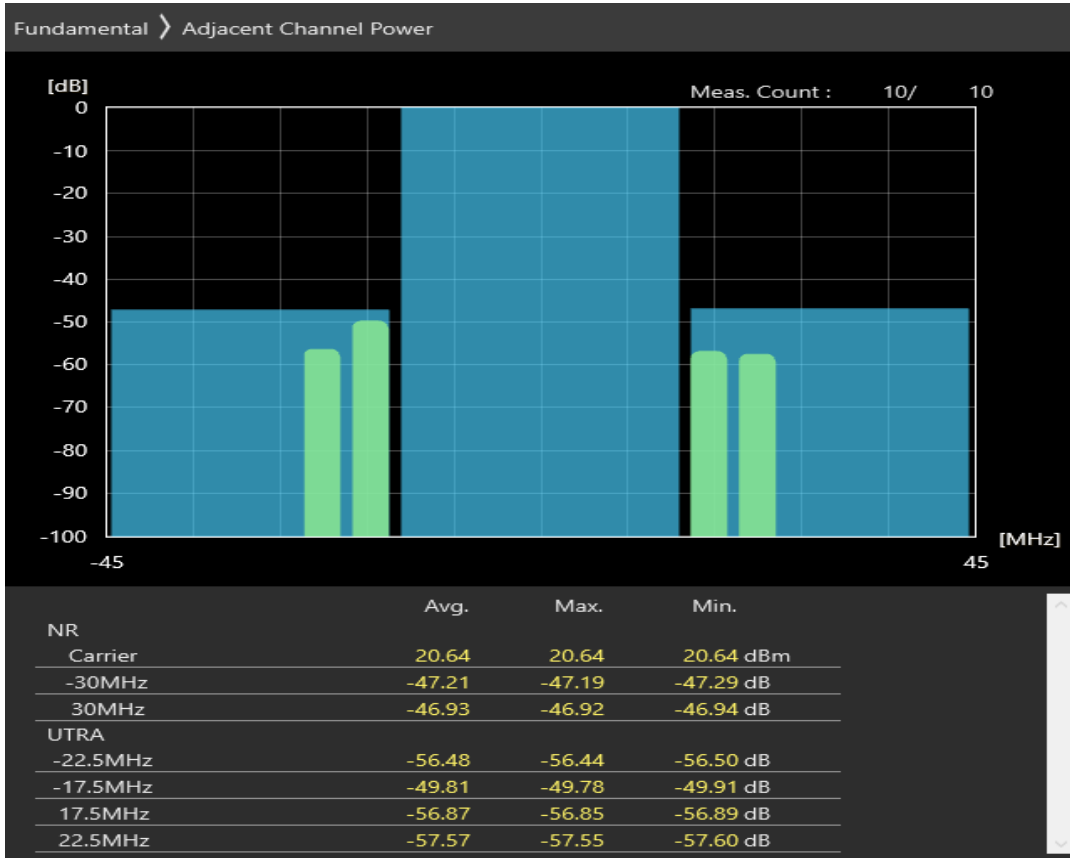
n3 SCS=30kHz CP_QAM16 BW=30MHz Channel=345000 RB=39@19
