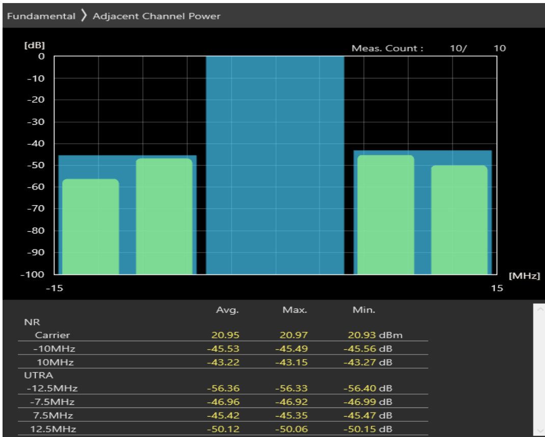
n28 SCS=30kHz CP_QPSK BW=10MHz Channel=141600 RB=12@6
