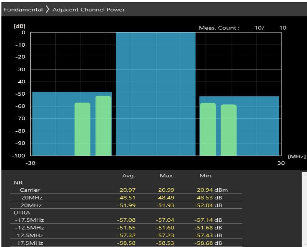
n38 SCS=30kHz DFT_BPSK BW=20MHz Channel=522000 RB=25@12
