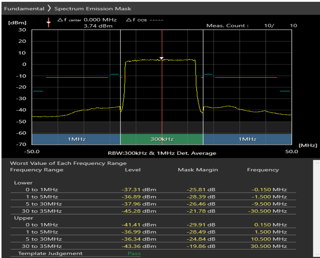
n3 SCS=30kHz DFT_QPSK BW=30MHz Channel=345000 RB=1@0
