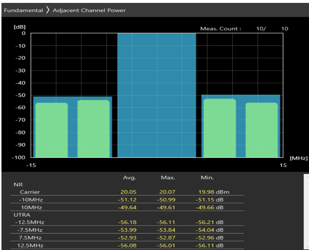
n1 SCS=30kHz CP_QAM16 BW=10MHz Channel=395000 RB=24@0
