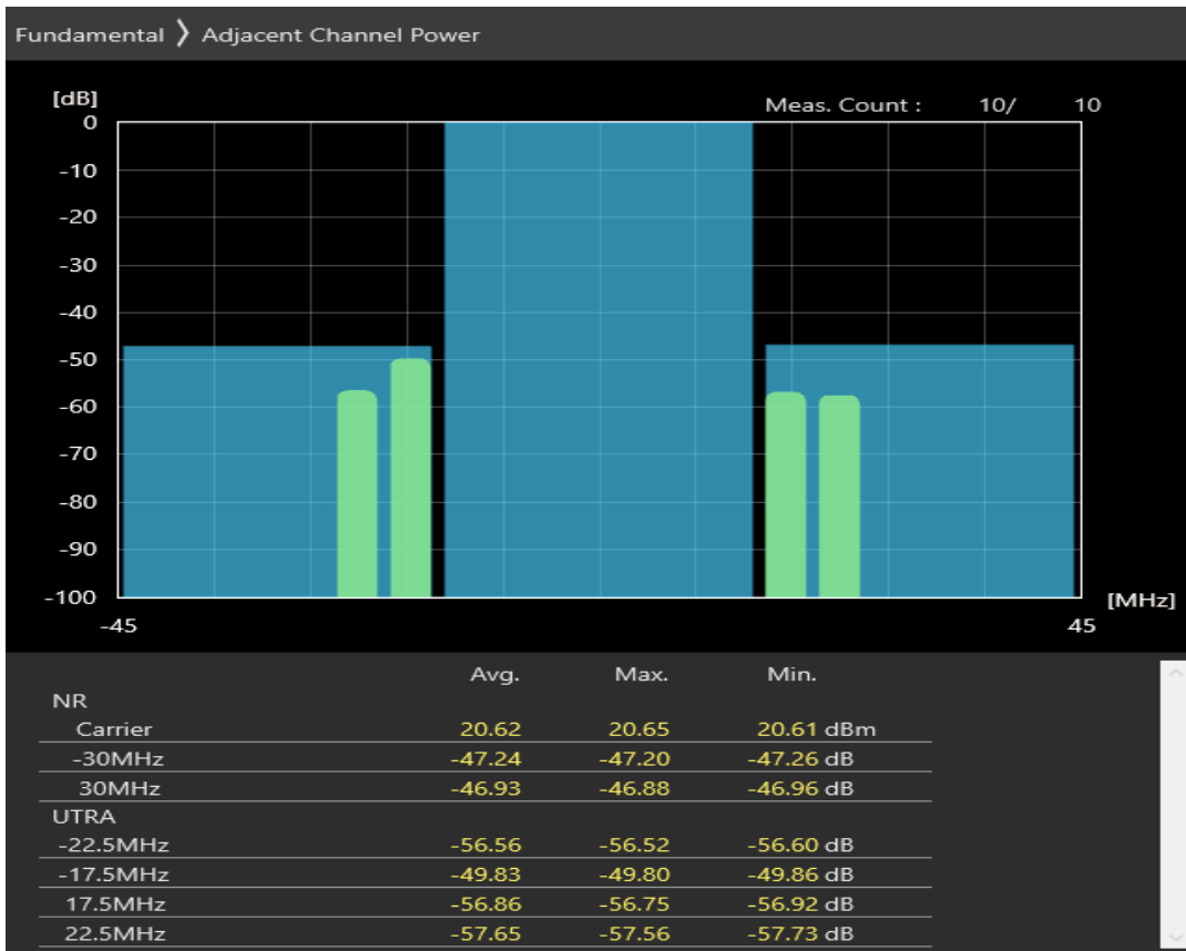
n3 SCS=30kHz CP_QPSK BW=30MHz Channel=345000 RB=78@0
