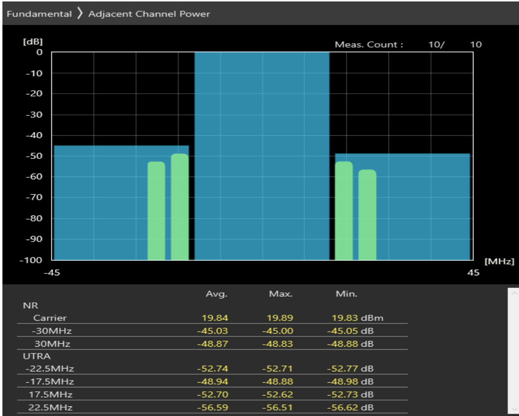
n3 SCS=30kHz DFT_QAM16 BW=30MHz Channel=354000 RB=1@77
