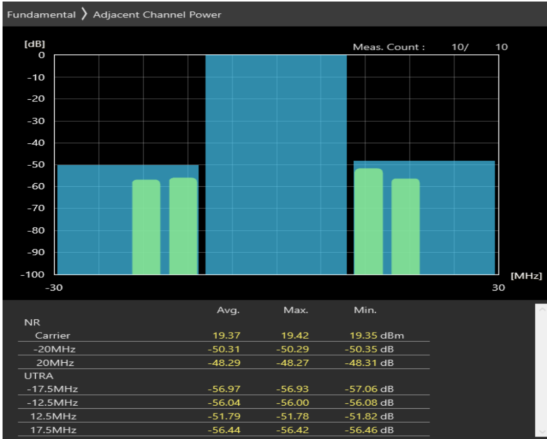
n1 SCS=30kHz DFT_QAM16 BW=20MHz Channel=394000 RB=25@12
