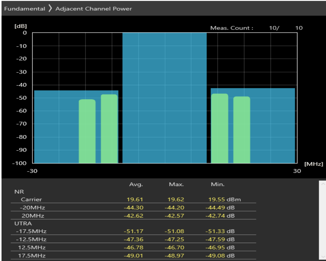
n1 SCS=30kHz DFT_QAM256 BW=20MHz Channel=394000 RB=1@50
