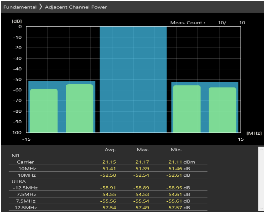
n28 SCS=30kHz DFT_QAM256 BW=10MHz Channel=141600 RB=24@0
