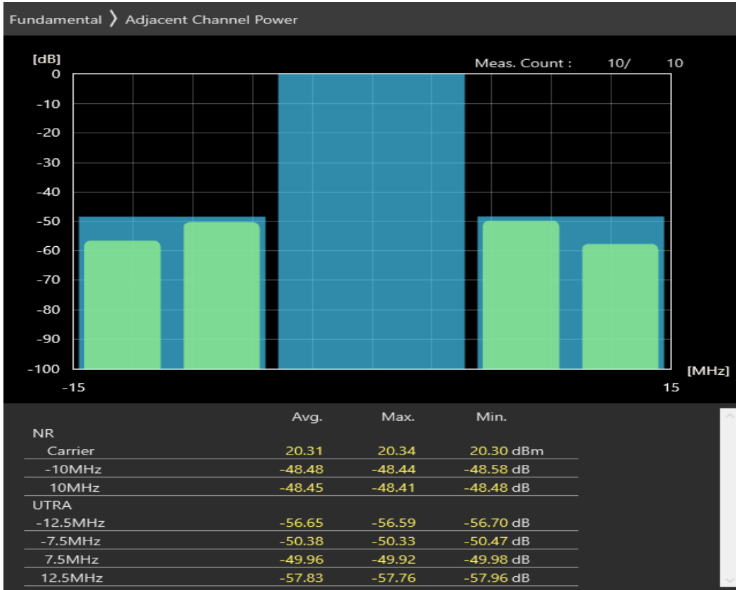
n20 SCS=30kHz DFT_BPSK BW=10MHz Channel=171400 RB=1@23
