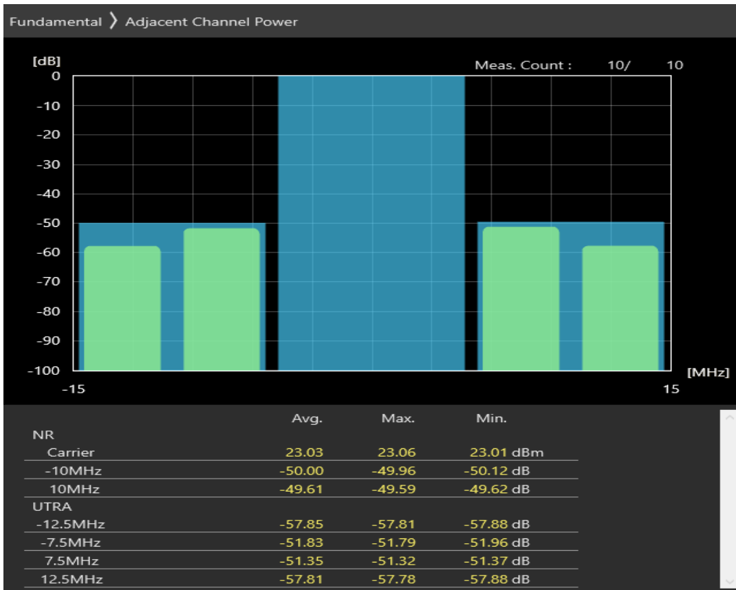
n78 SCS=30kHz DFT_QAM16 BW=10MHz Channel=647000 RB=1@0
