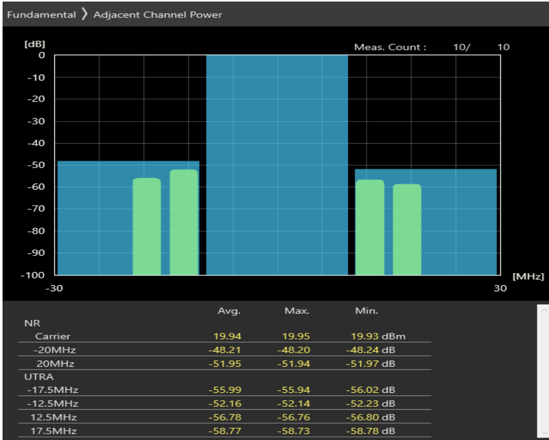
n20 SCS=30kHz CP_QAM256 BW=20MHz Channel=170400 RB=1@50
