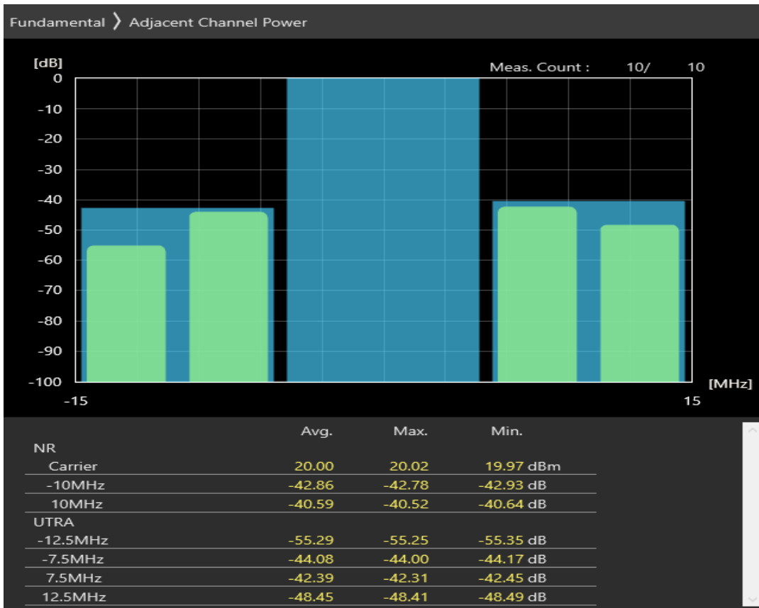
n28 SCS=30kHz DFT_BPSK BW=10MHz Channel=148600 RB=12@6
