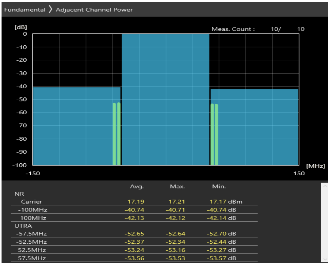
n77 SCS=30kHz DFT_QAM256 BW=100MHz Channel=623334 RB=1@0
