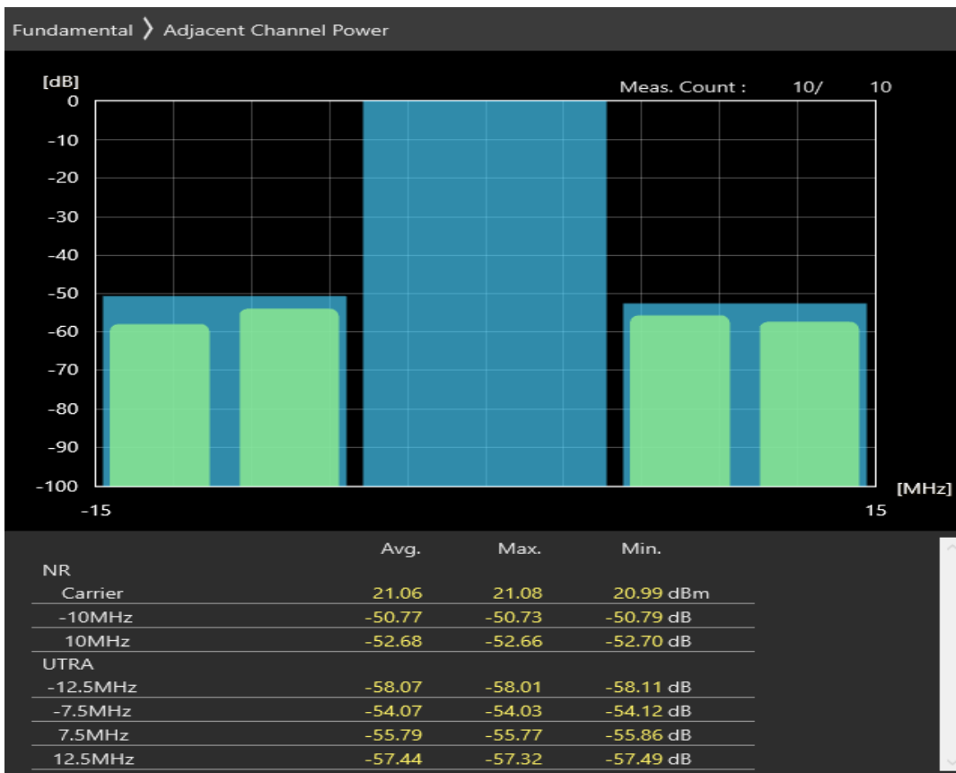
n20 SCS=30kHz DFT_QAM64 BW=10MHz Channel=167400 RB=24@0
