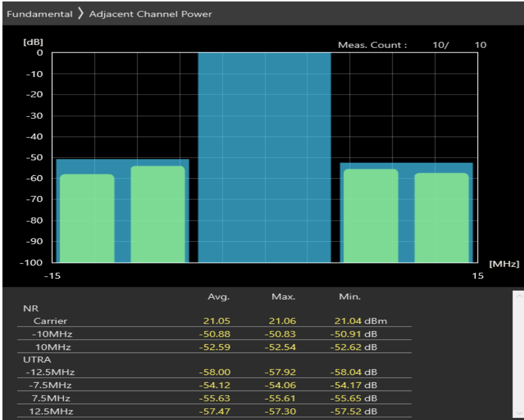
n20 SCS=30kHz DFT_QAM16 BW=10MHz Channel=167400 RB=24@0
