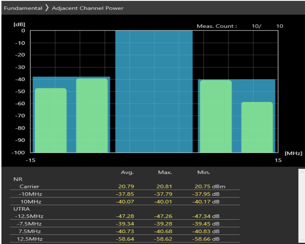
n8 SCS=30kHz CP_QAM16 BW=10MHz Channel=182000 RB=12@6
