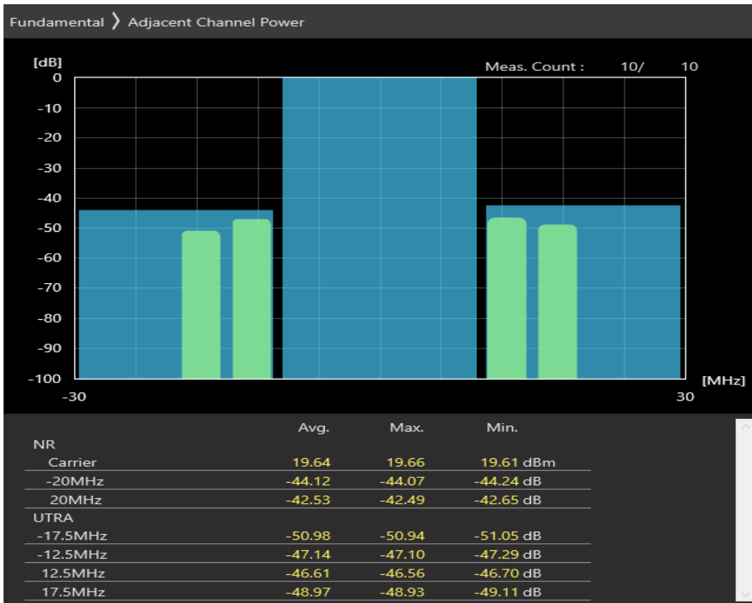
n1 SCS=30kHz DFT_QAM16 BW=20MHz Channel=394000 RB=1@50
