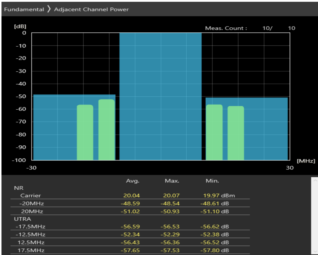
n1 SCS=30kHz CP_QAM16 BW=20MHz Channel=386000 RB=25@12
