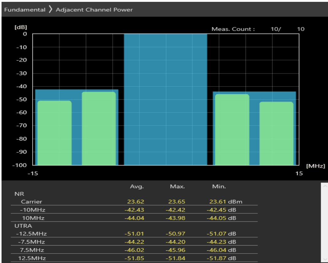
n77 SCS=30kHz DFT_QAM16 BW=10MHz Channel=679666 RB=12@6
