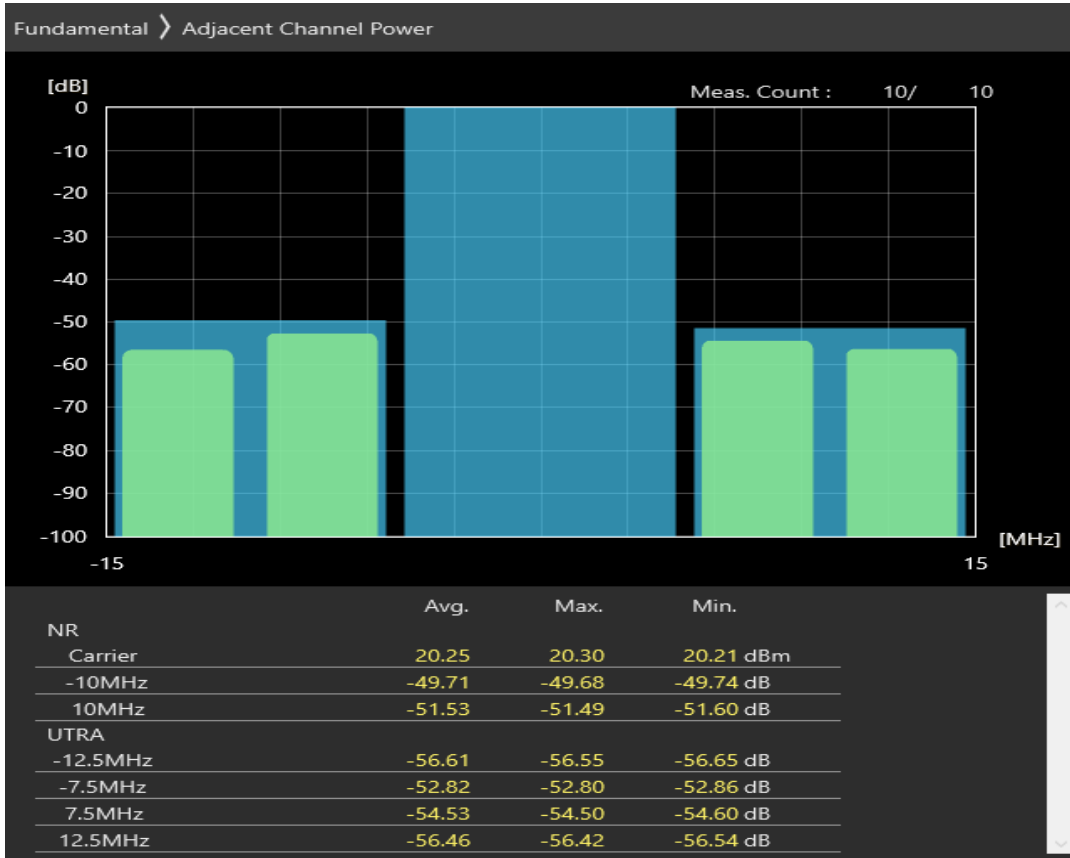
n1 SCS=30kHz CP_QAM16 BW=10MHz Channel=385000 RB=24@0
