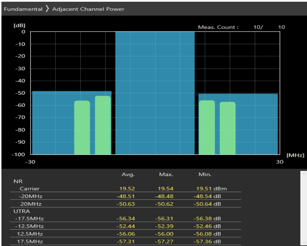
n1 SCS=30kHz CP_QAM256 BW=20MHz Channel=386000 RB=51@0
