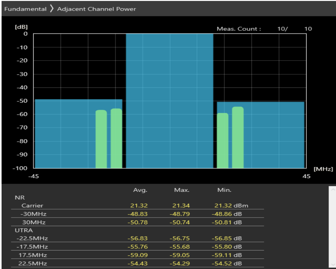
n3 SCS=30kHz CP_QAM16 BW=30MHz Channel=354000 RB=1@77
