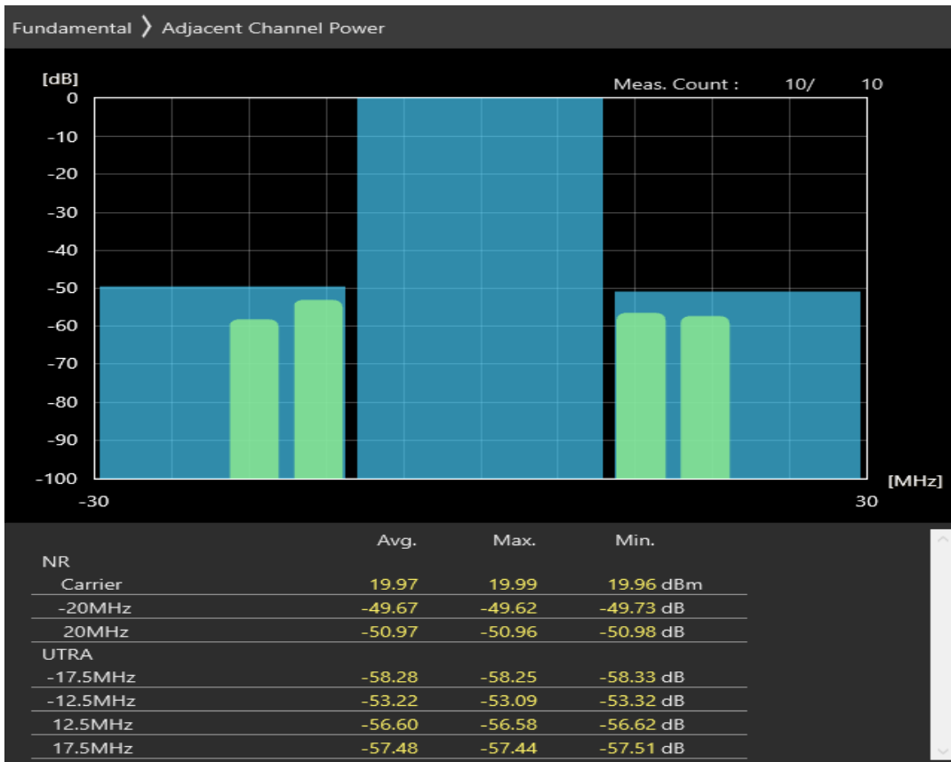
n28 SCS=30kHz DFT_BPSK BW=20MHz Channel=147600 RB=25@12
