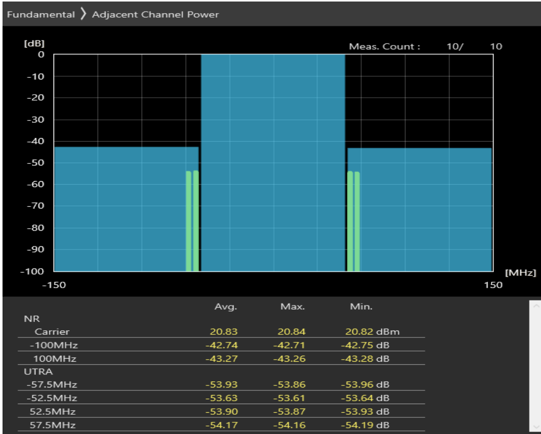
n78 SCS=30kHz DFT_QAM16 BW=100MHz Channel=650000 RB=135@67
