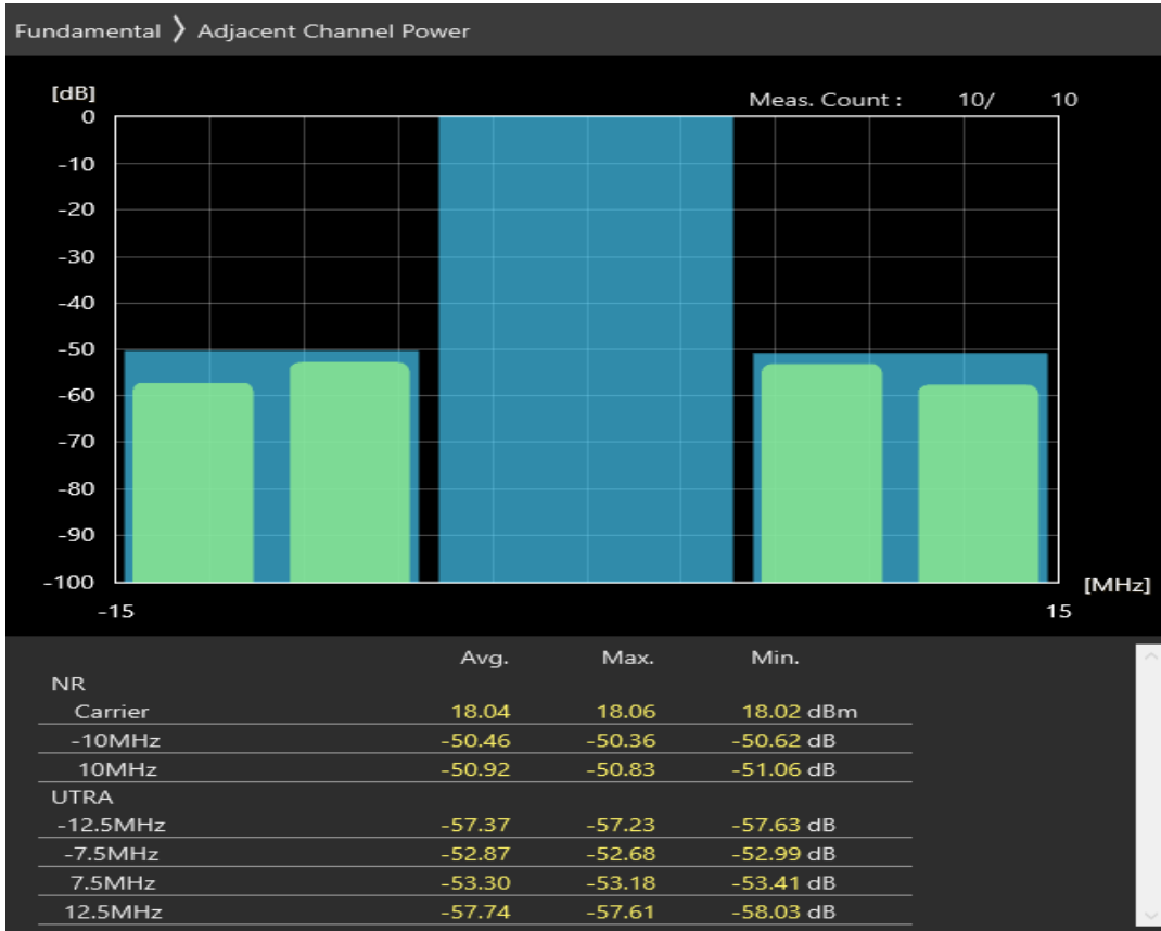
n77 SCS=30kHz DFT_BPSK BW=10MHz Channel=679666 RB=1@23
