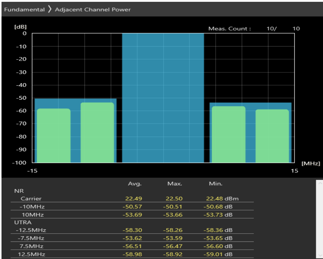
n77 SCS=30kHz DFT_QPSK BW=10MHz Channel=620334 RB=24@0
