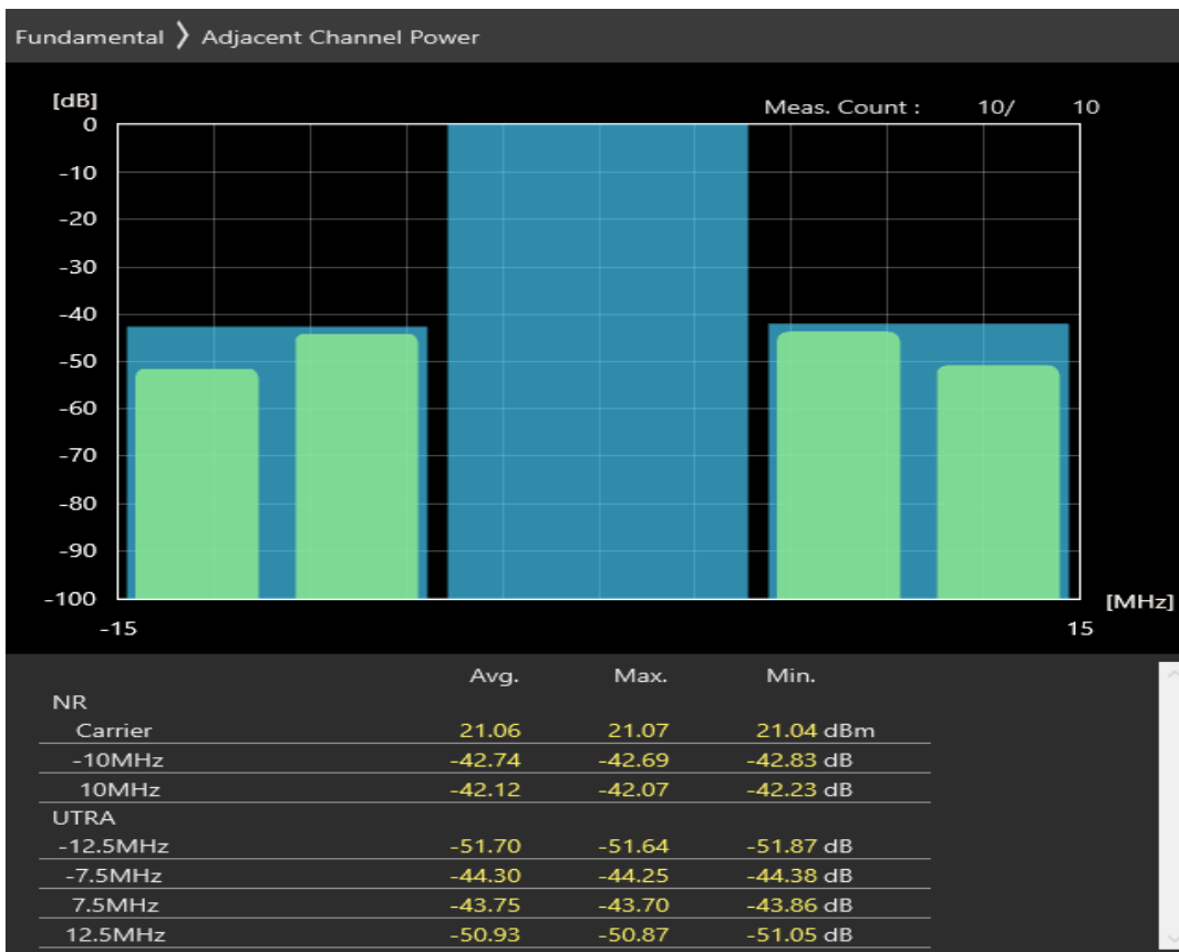
n38 SCS=30kHz DFT_BPSK BW=10MHz Channel=523000 RB=12@6
