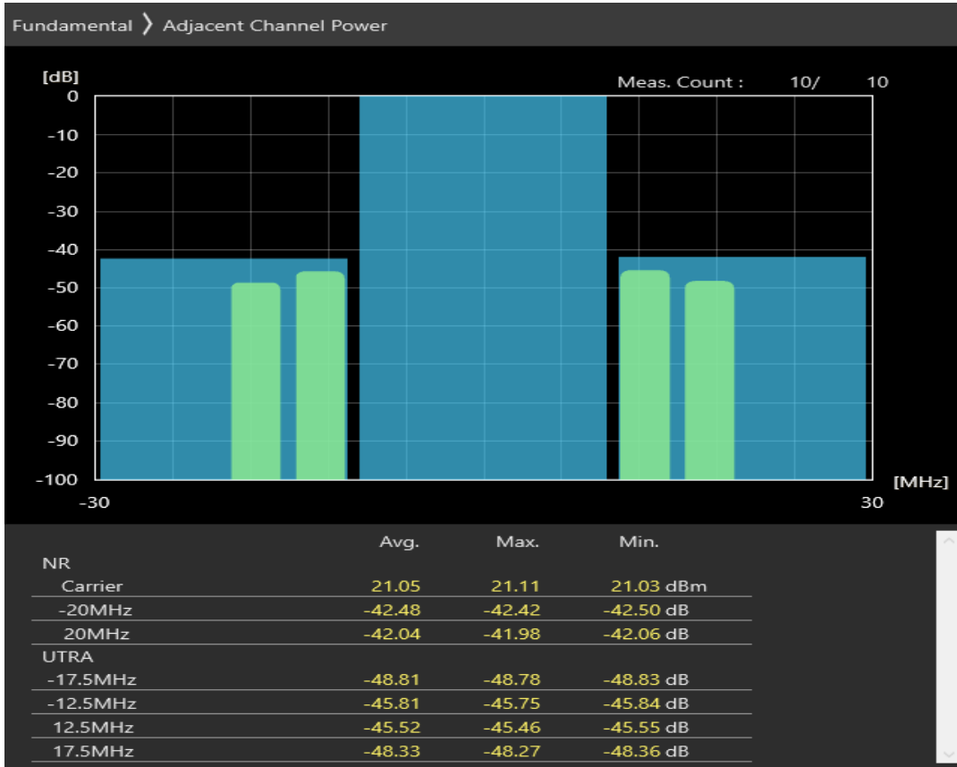
n38 SCS=30kHz DFT_QAM16 BW=20MHz Channel=516000 RB=25@12
