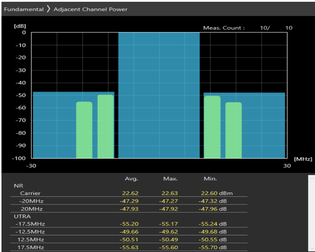
n38 SCS=30kHz CP_QPSK BW=20MHz Channel=522000 RB=1@50
