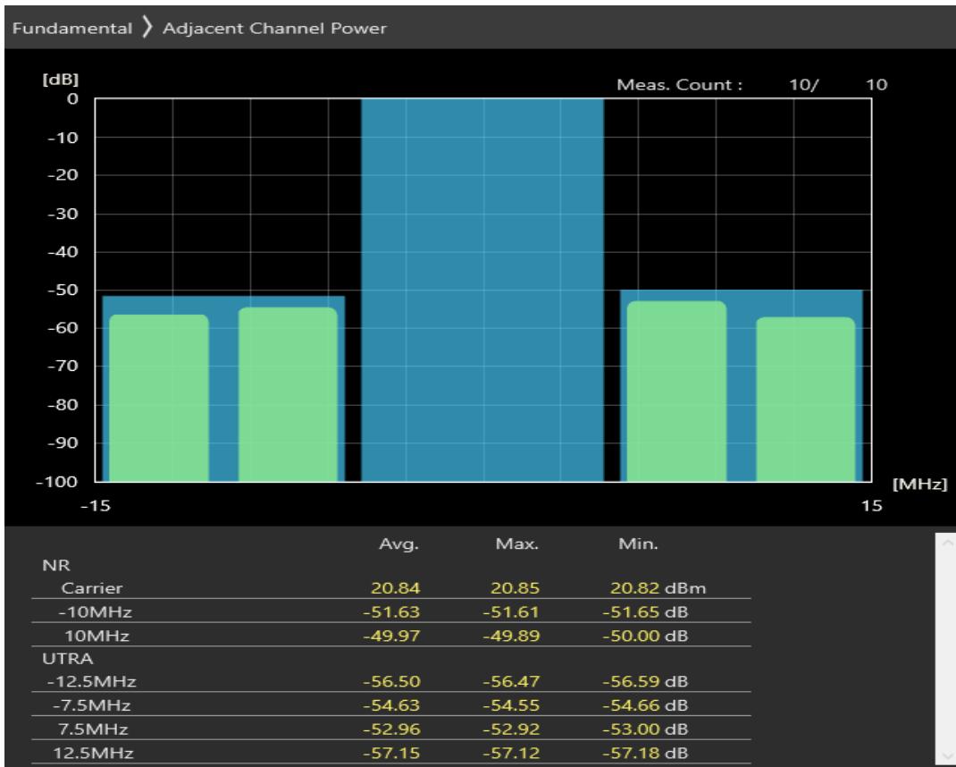
n38 SCS=30kHz CP_QAM64 BW=10MHz Channel=523000 RB=24 @0
