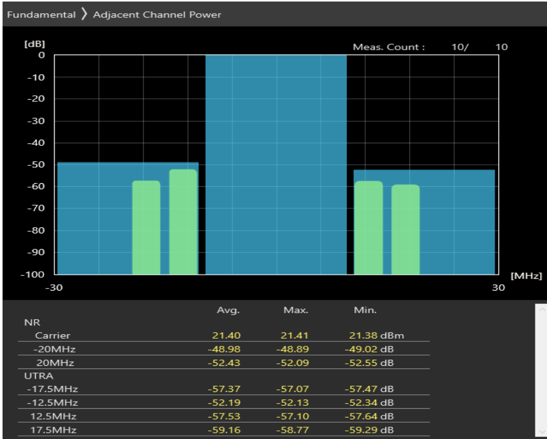
n38 SCS=30kHz CP_QAM16 BW=20MHz Channel=516000 RB=25@12
