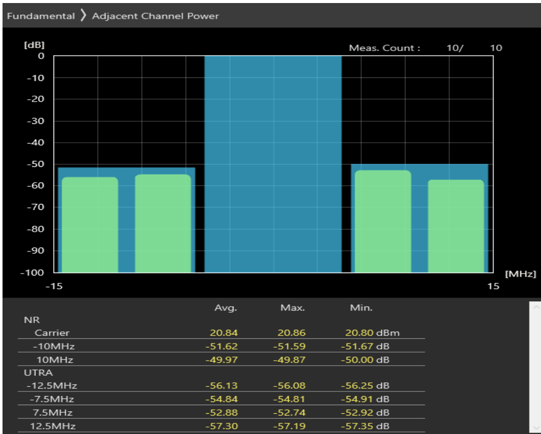
n38 SCS=30kHz DFT_BPSK BW=10MHz Channel=523000 RB=24@0
