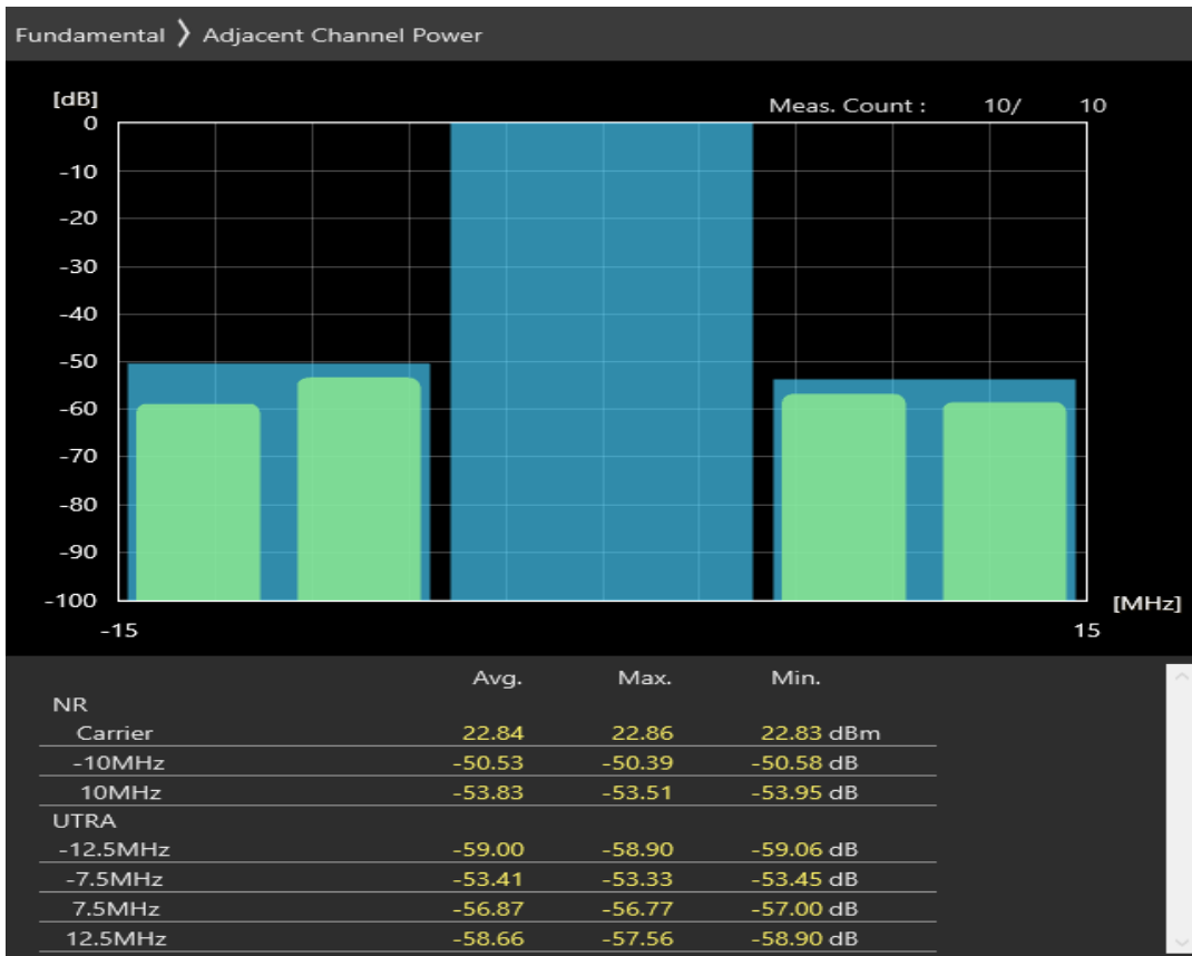
n78 SCS=30kHz DFT_QPSK BW=10MHz Channel=647000 RB=24@0
