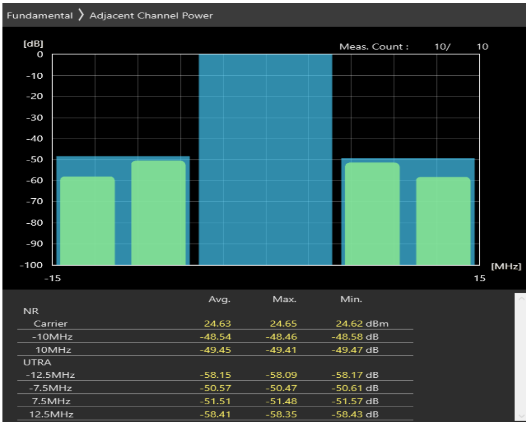
n77 SCS=30kHz DFT_QPSK BW=10MHz Channel=679666 RB=1@23
