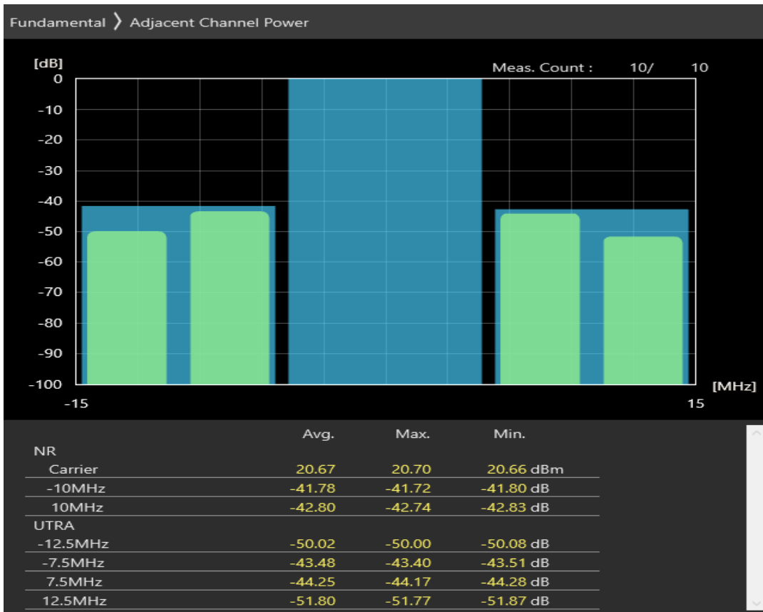
n20 SCS=30kHz CP_QAM16 BW=10MHz Channel=171400 RB=12@6
