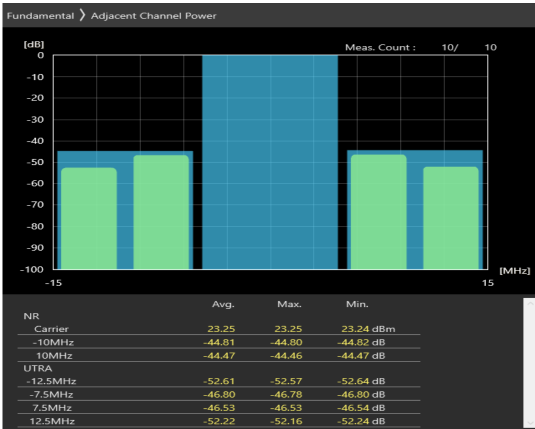
n38 SCS=30kHz DFT_QAM16 BW=10MHz Channel=523000 RB=12@6
