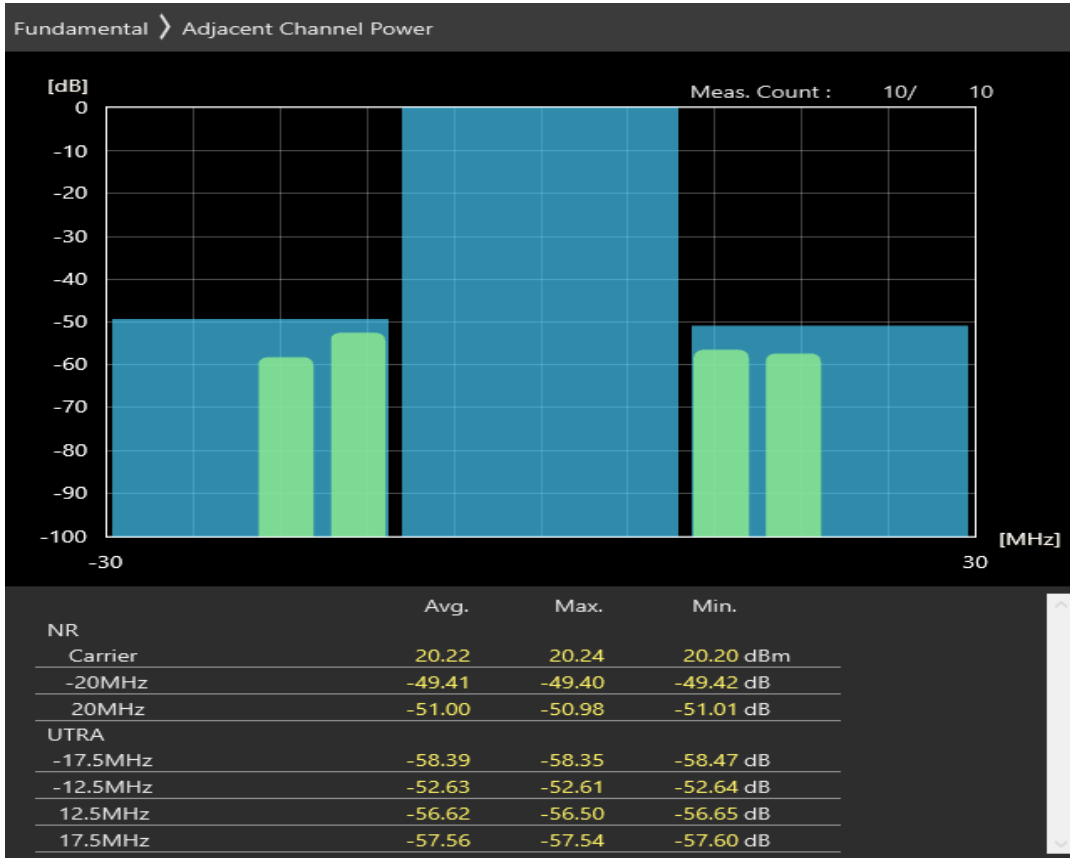
n28 SCS=30kHz CP_QAM16 BW=20MHz Channel=142600 RB=51@0
