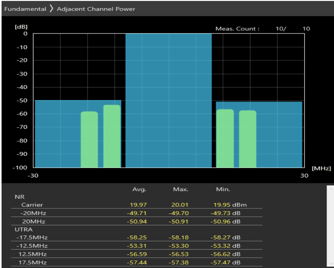
n28 SCS=30kHz CP_QAM64 BW=20MHz Channel=142600 RB=51@0
