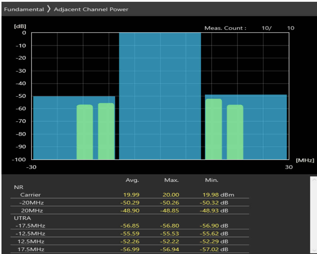
n20 SCS=30kHz CP_QAM64 BW=20MHz Channel=170400 RB=51@0
