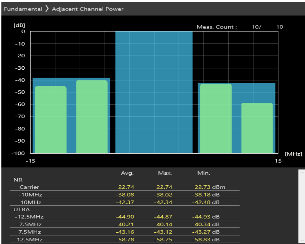
n28 SCS=30kHz DFT_QAM16 BW=10MHz Channel=148600 RB=12@6
