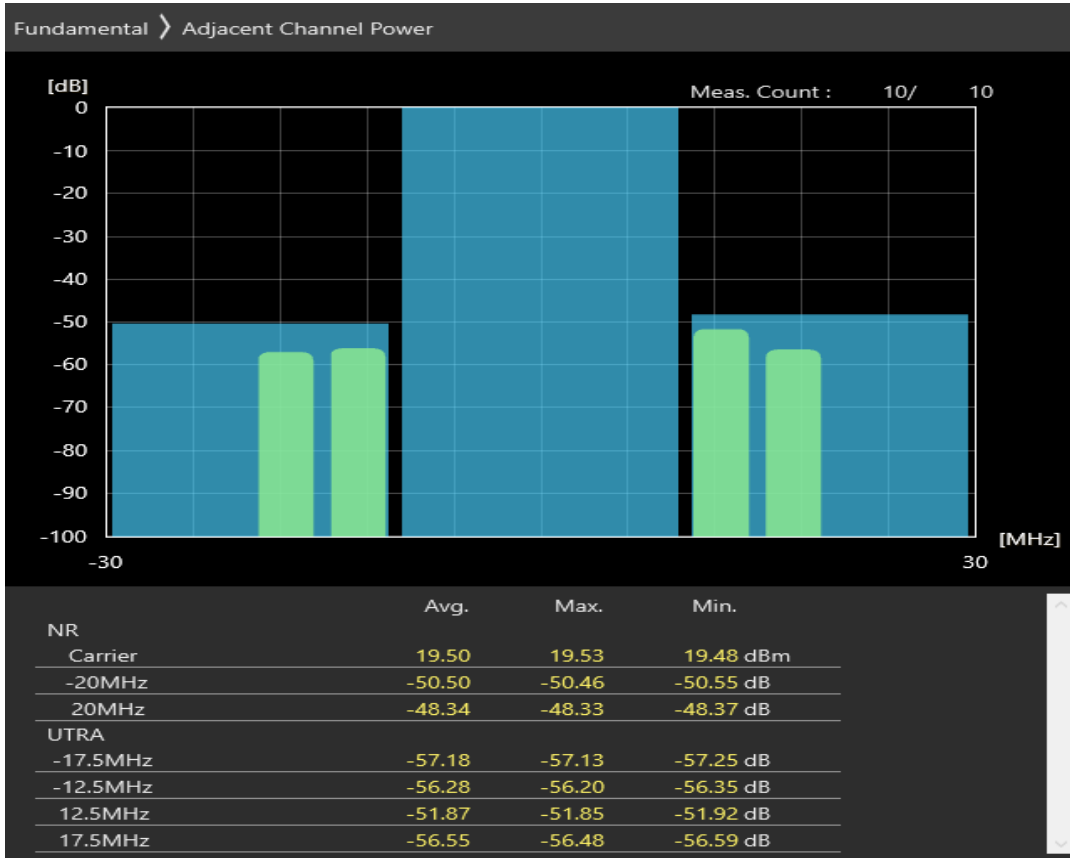
n1 SCS=30kHz DFT_BPSK BW=20MHz Channel=394000 RB=25@12
