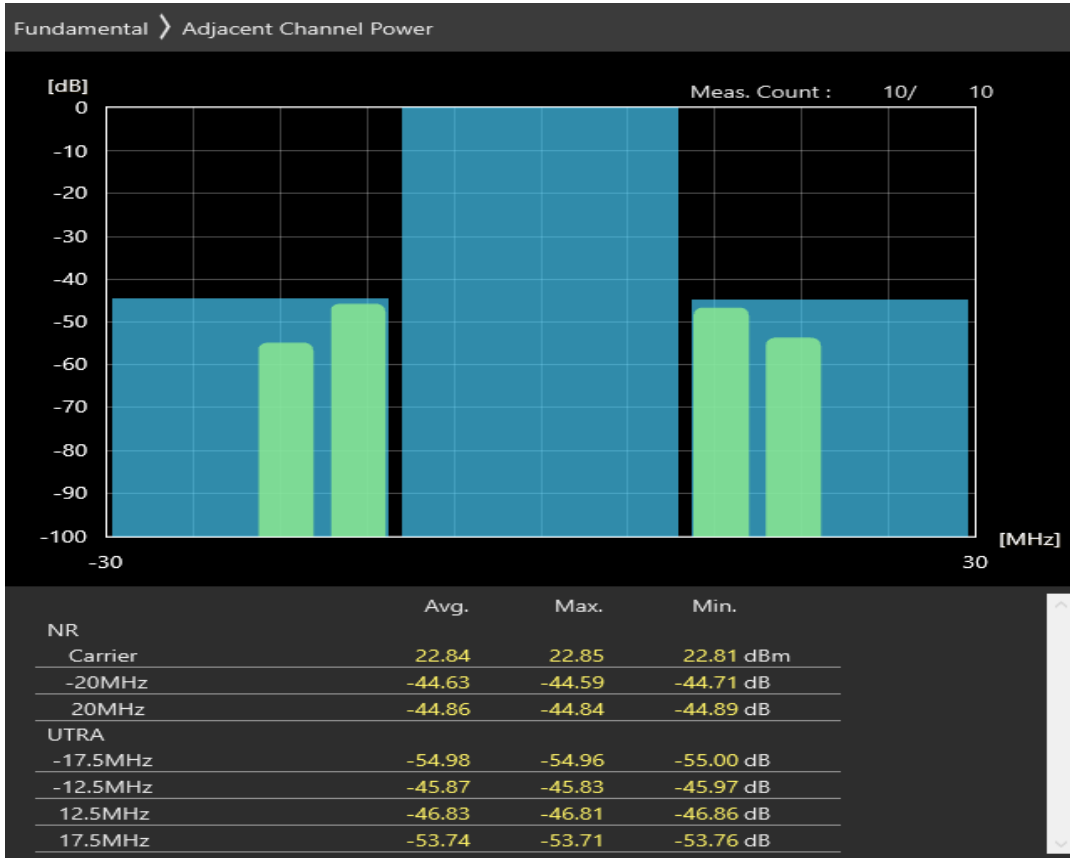
n8 SCS=30kHz DFT_QAM16 BW=20MHz Channel=178000 RB=1@0
