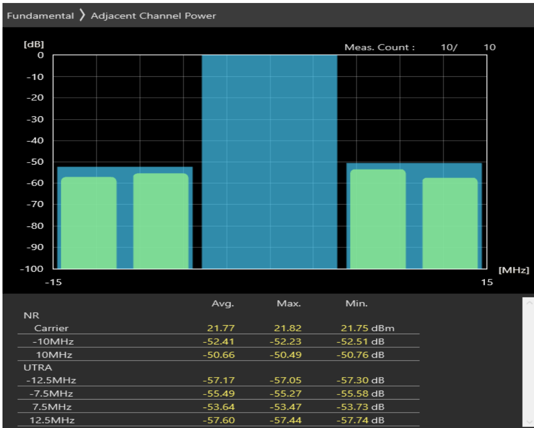
n38 SCS=30kHz DFT_QAM64 BW=10MHz Channel=523000 RB=24@0
