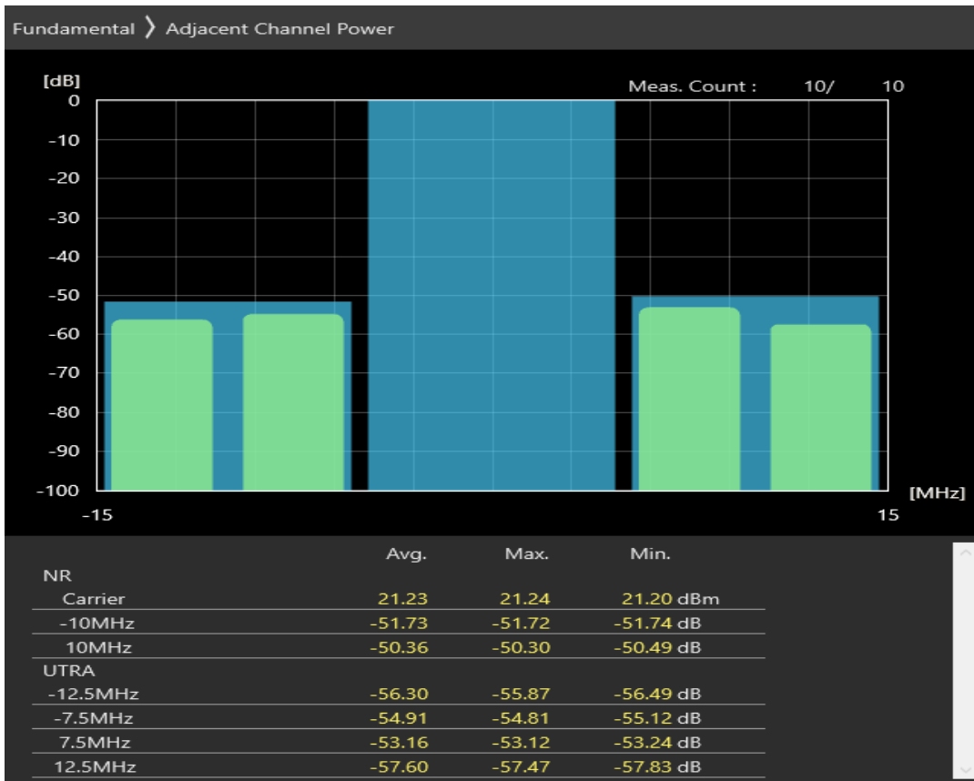
n38 SCS=30kHz CP_QAM16 BW=10MHz Channel=523000 RB=24@0
