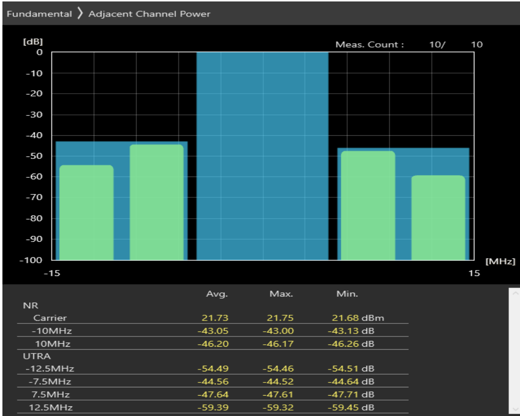
n28 SCS=30kHz CP_QAM16 BW=10MHz Channel=148600 RB=1@23
