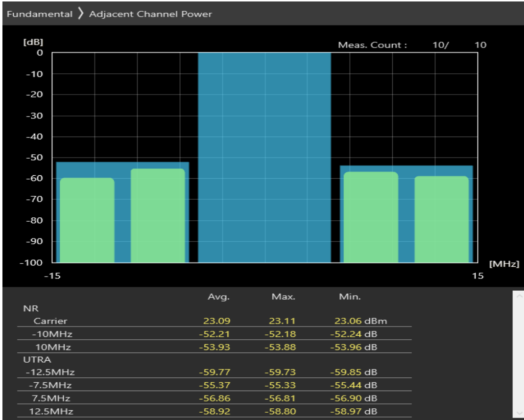
n28 SCS=30kHz DFT_BPSK BW=10MHz Channel=141600 RB=24@0
