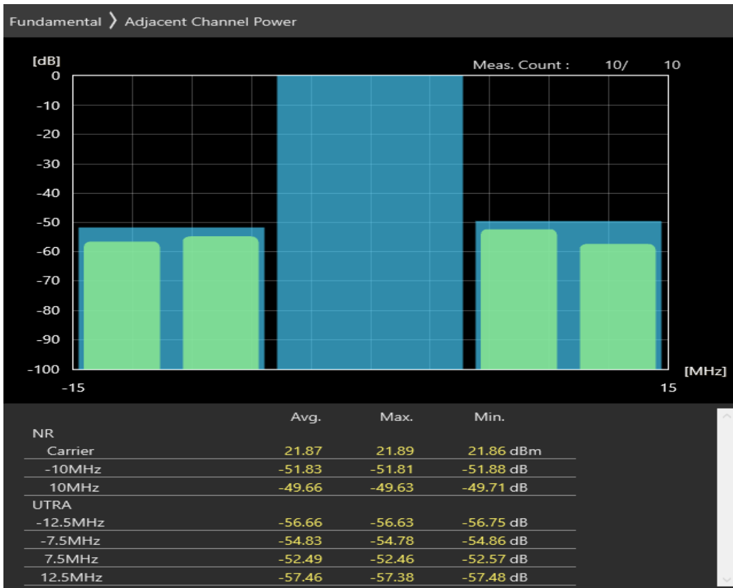
n78 SCS=30kHz CP_QPSK BW=10MHz Channel=653000 RB=24@0
