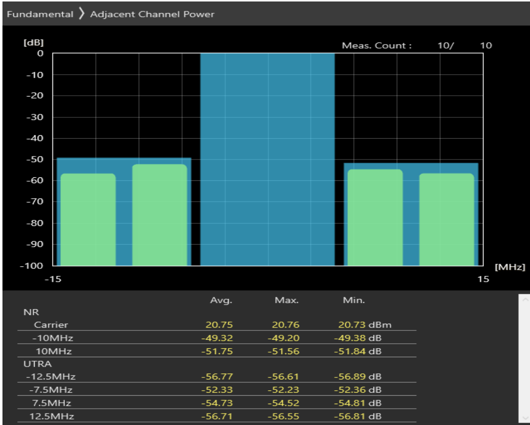
n77 SCS=30kHz CP_QAM16 BW=10MHz Channel=620334 RB=24@0
