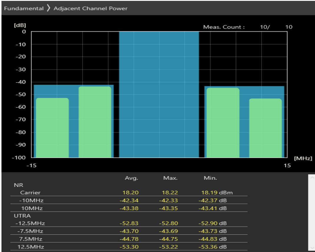
n77 SCS=30kHz DFT_BPSK BW=100MHz Channel=623334 RB=135@67
