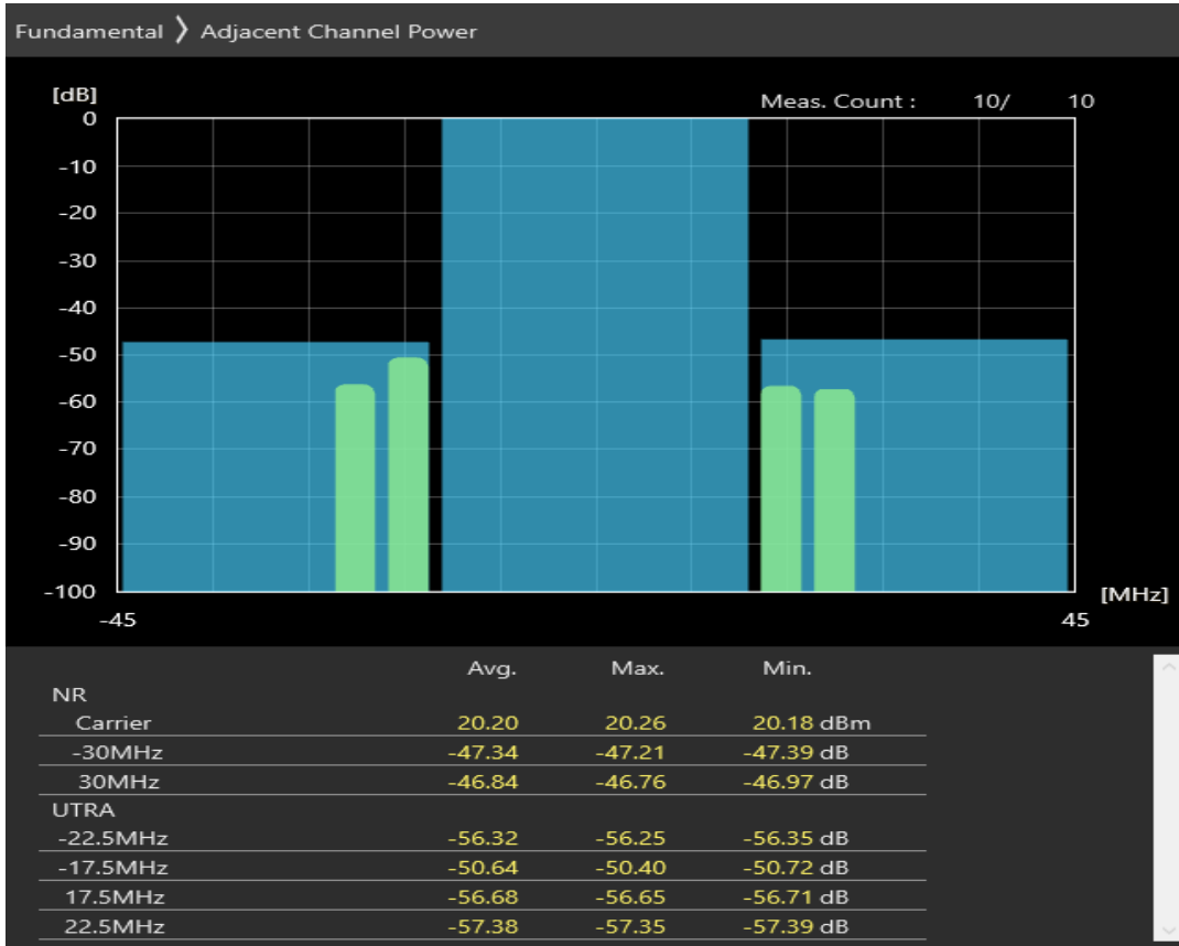
n3 SCS=30kHz DFT_QAM256 BW=30MHz Channel=345000 RB=75@0
