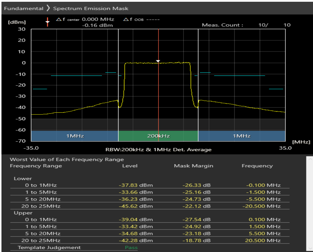
n1 SCS=30kHz DFT_QAM256 BW=20MHz Channel=386000 RB=1@0
