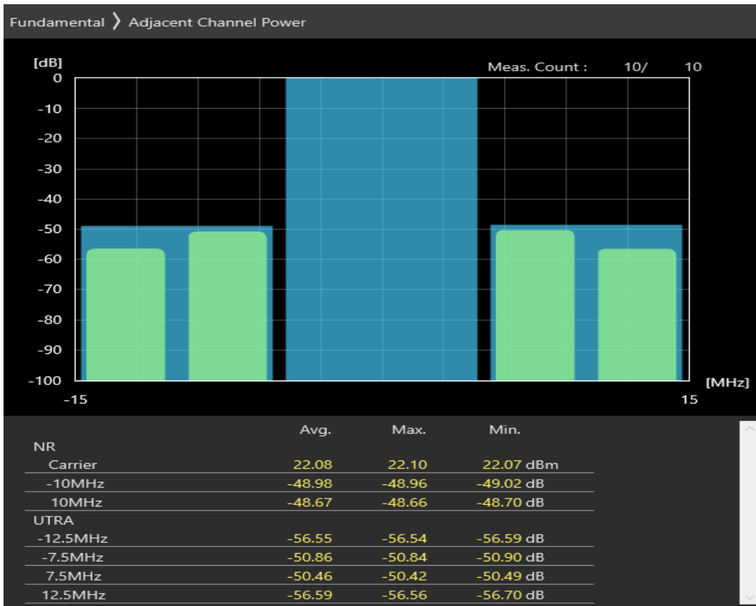
n78 SCS=30kHz CP_QAM16 BW=10MHz Channel=647000 RB=1@0
