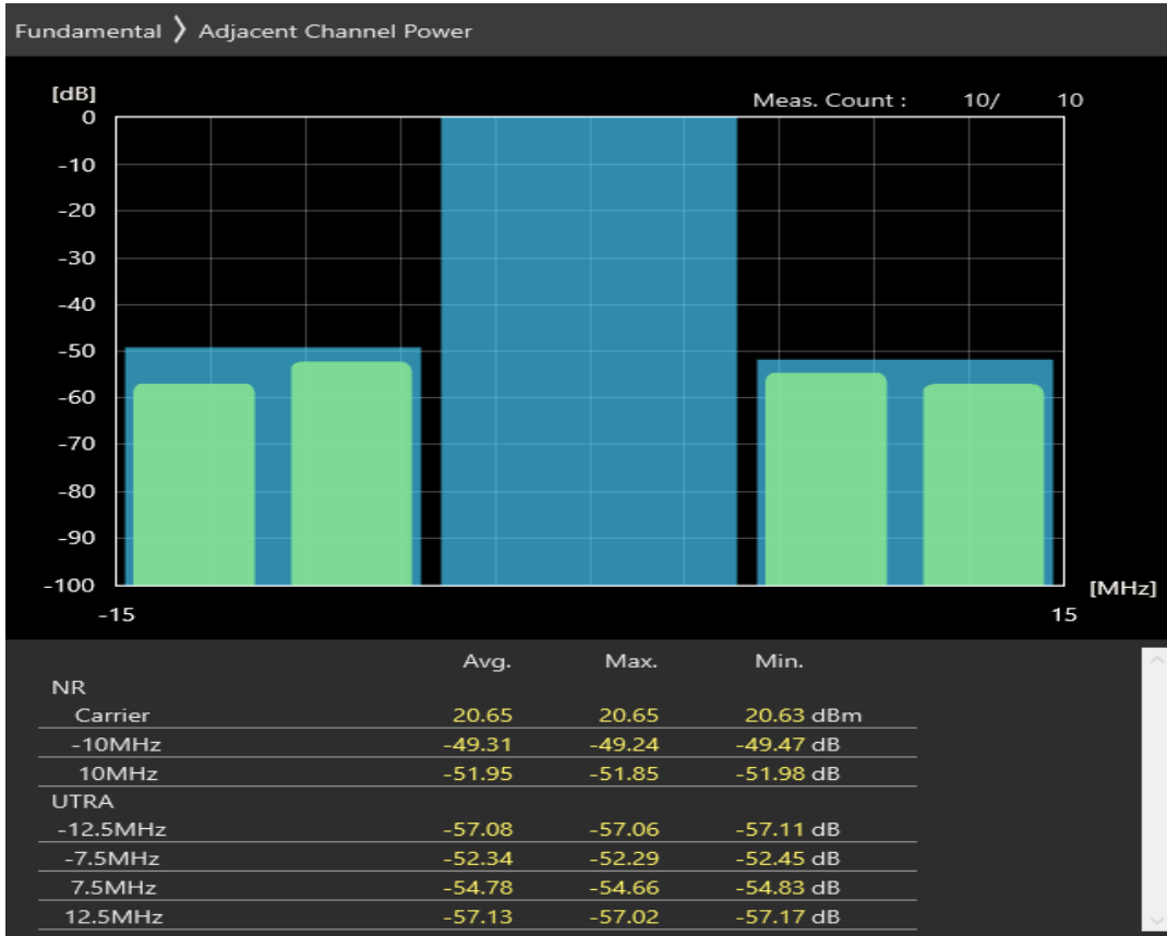
n78 SCS=30kHz CP_QAM64 BW=10MHz Channel=647000 RB=24@0
