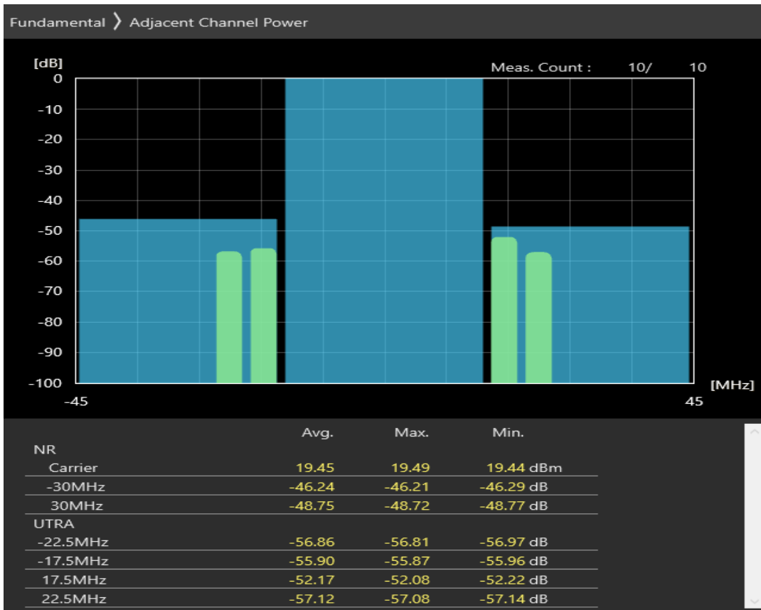
n3 SCS=30kHz DFT_QAM16 BW=30MHz Channel=354000 RB=75@0
