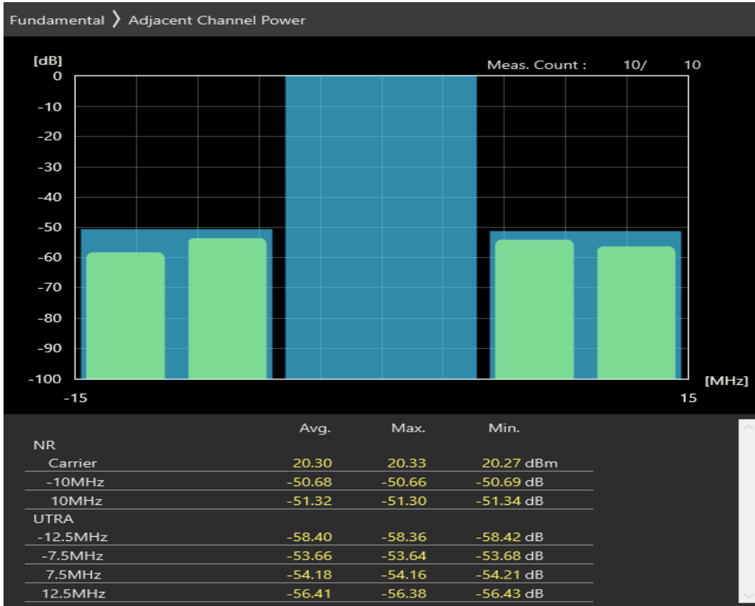
n28 SCS=30kHz CP_QAM16 BW=10MHz Channel=141600 RB=24@0
