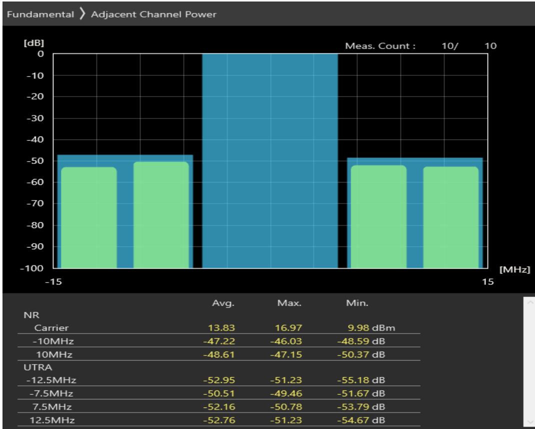
n77 SCS=30kHz CP_QAM256 BW=10MHz Channel=620334 RB=24@0
