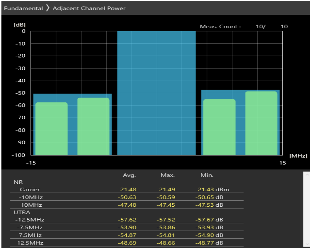
n3 SCS=30kHz DFT_QAM256 BW=10MHz Channel=343000 RB=24@0
