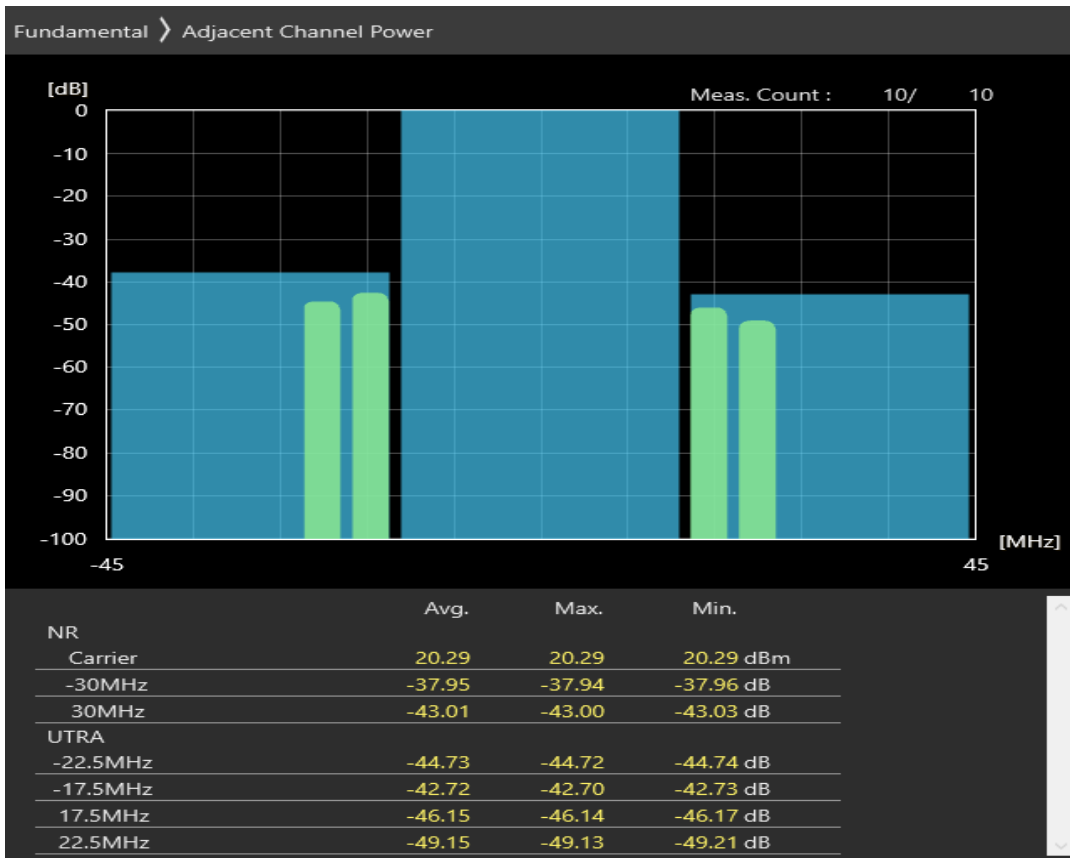
n3 SCS=30kHz CP_QPSK BW=30MHz Channel=354000 RB=1@77
