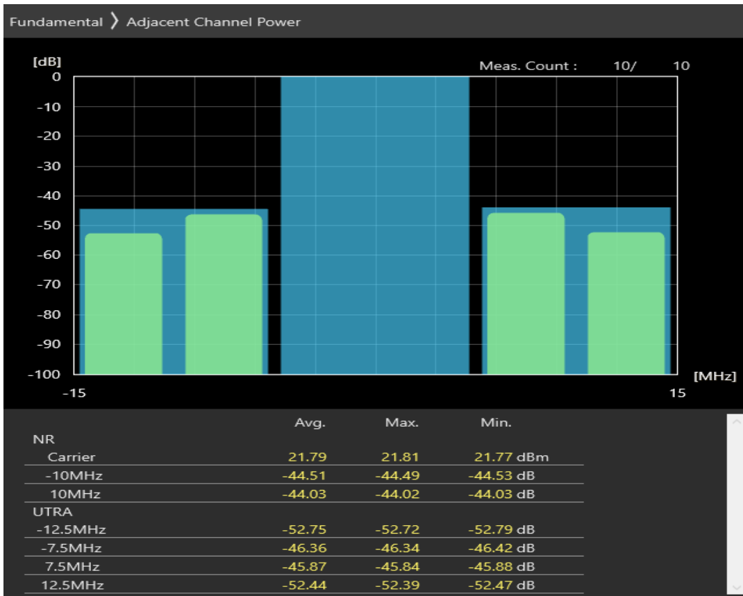
n38 SCS=30kHz DFT_QAM256 BW=10MHz Channel=523000 RB=1@23
