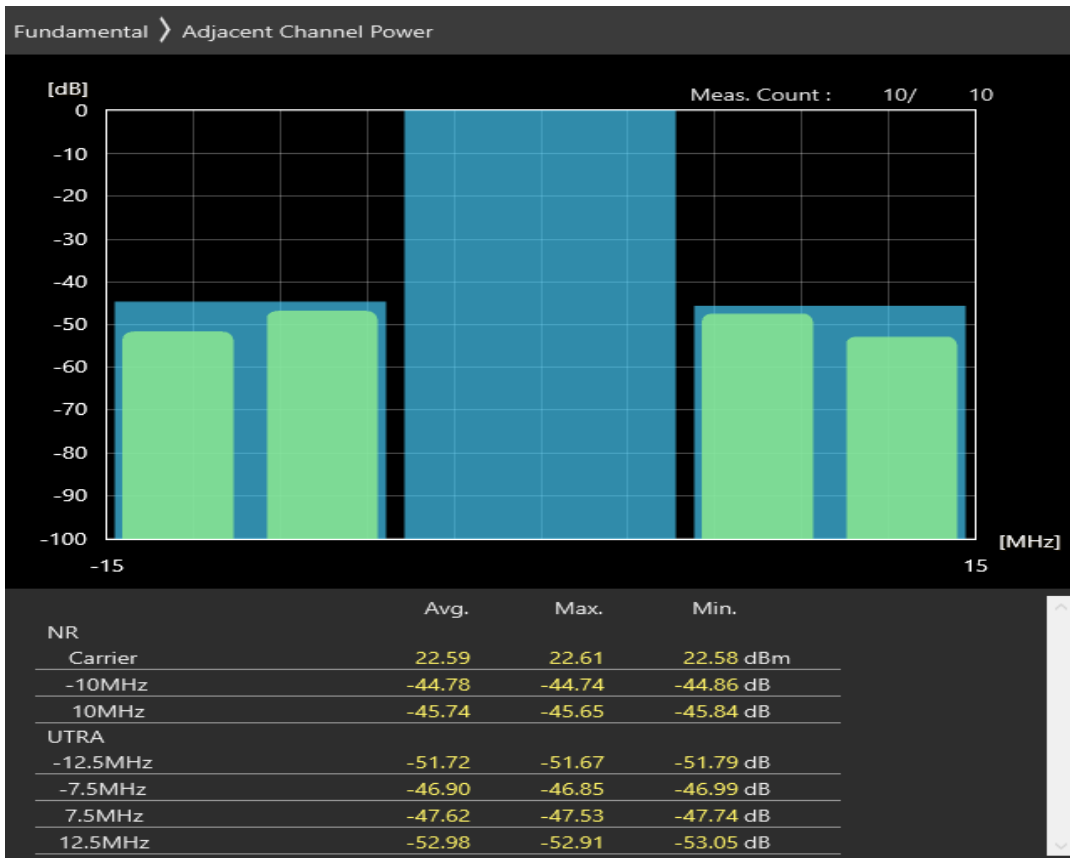
n20 SCS=30kHz DFT_QAM16 BW=10MHz Channel=171400 RB=12@6
