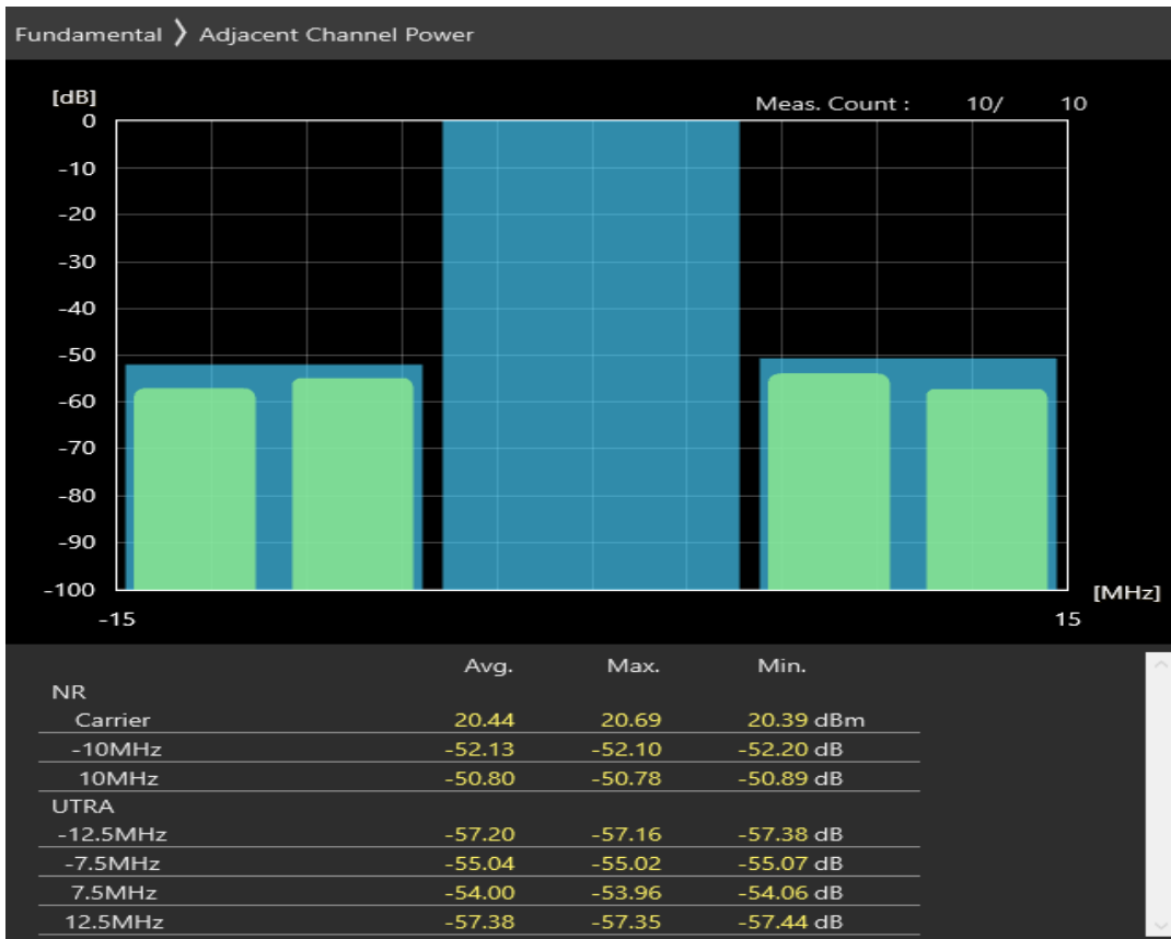
n1 SCS=30kHz DFT_QAM64 BW=10MHz Channel=395000 RB=24@0
