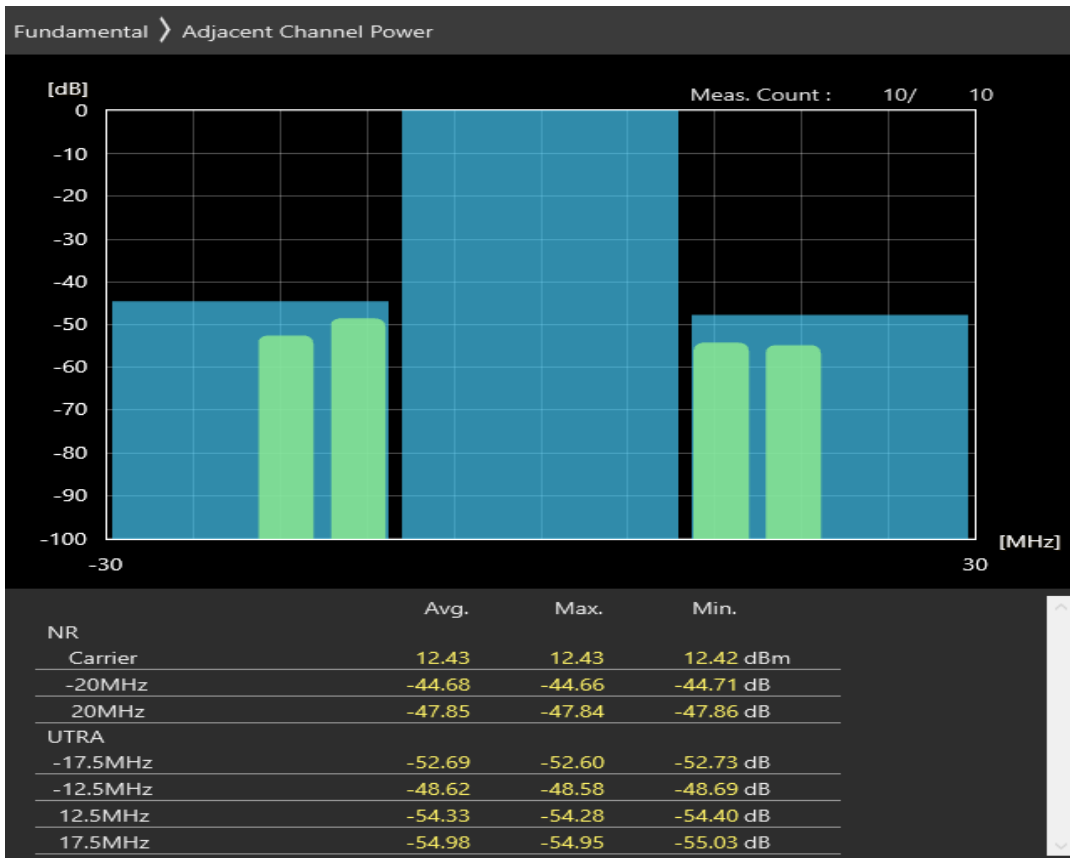
n28 SCS=30kHz CP_QAM64 BW=20MHz Channel=147600 RB=51@0
