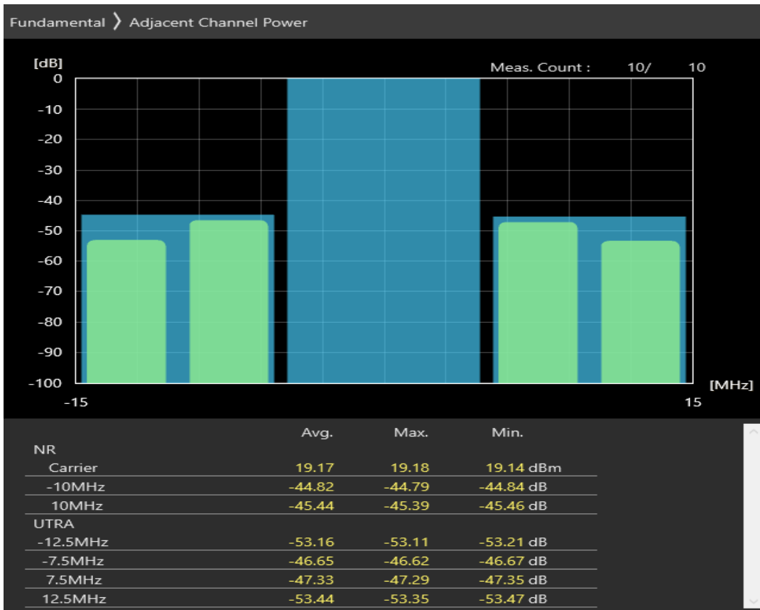
n77 SCS=30kHz CP_QPSK BW=10MHz Channel=620334 RB=12@6
