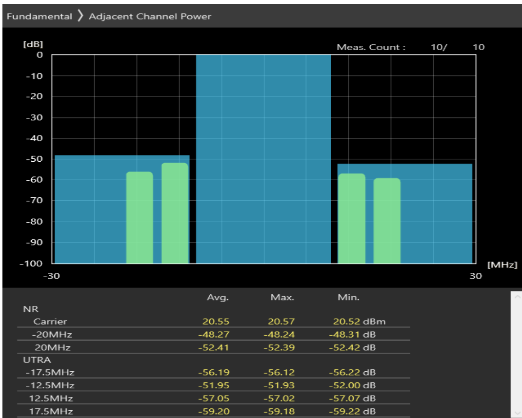
n20 SCS=30kHz CP_QAM16 BW=20MHz Channel=170400 RB=25@12
