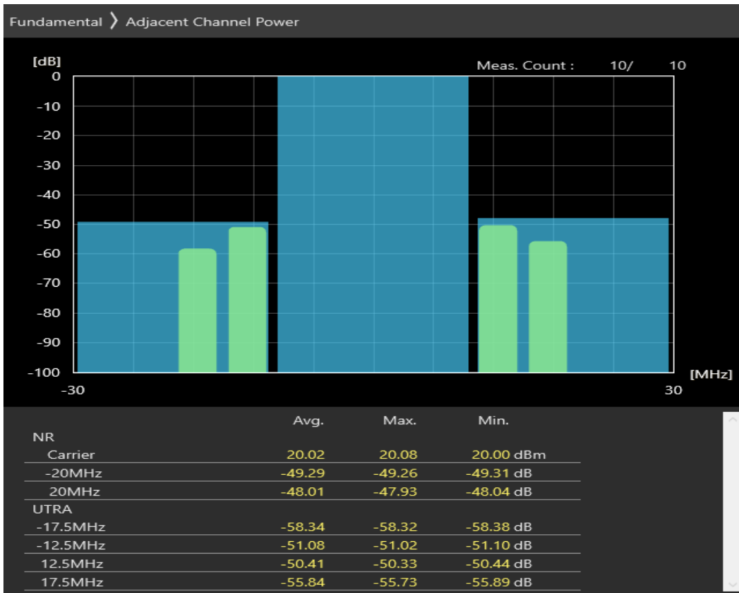
n20 SCS=30kHz DFT_QAM16 BW=20MHz Channel=168400 RB=1@0
