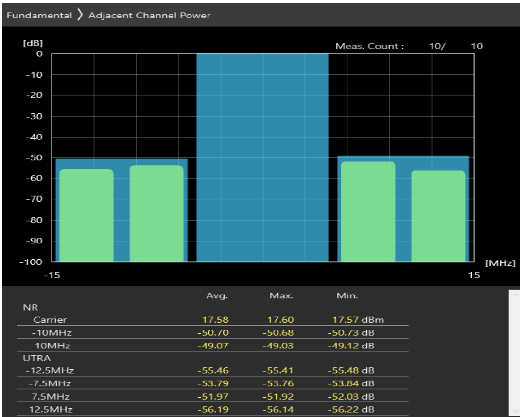
n77 SCS=30kHz CP_QAM256 BW=10MHz Channel=679666 RB=24@0
