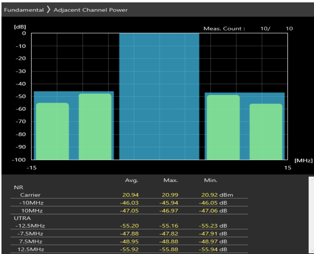
n1 SCS=30kHz CP_QAM16 BW=10MHz Channel=395000 RB=1@23
