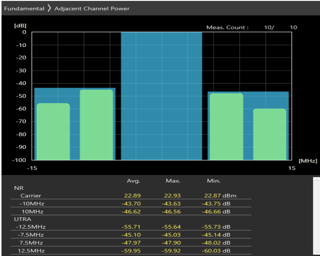
n28 SCS=30kHz DFT_QAM16 BW=10MHz Channel=148600 RB=1@23
