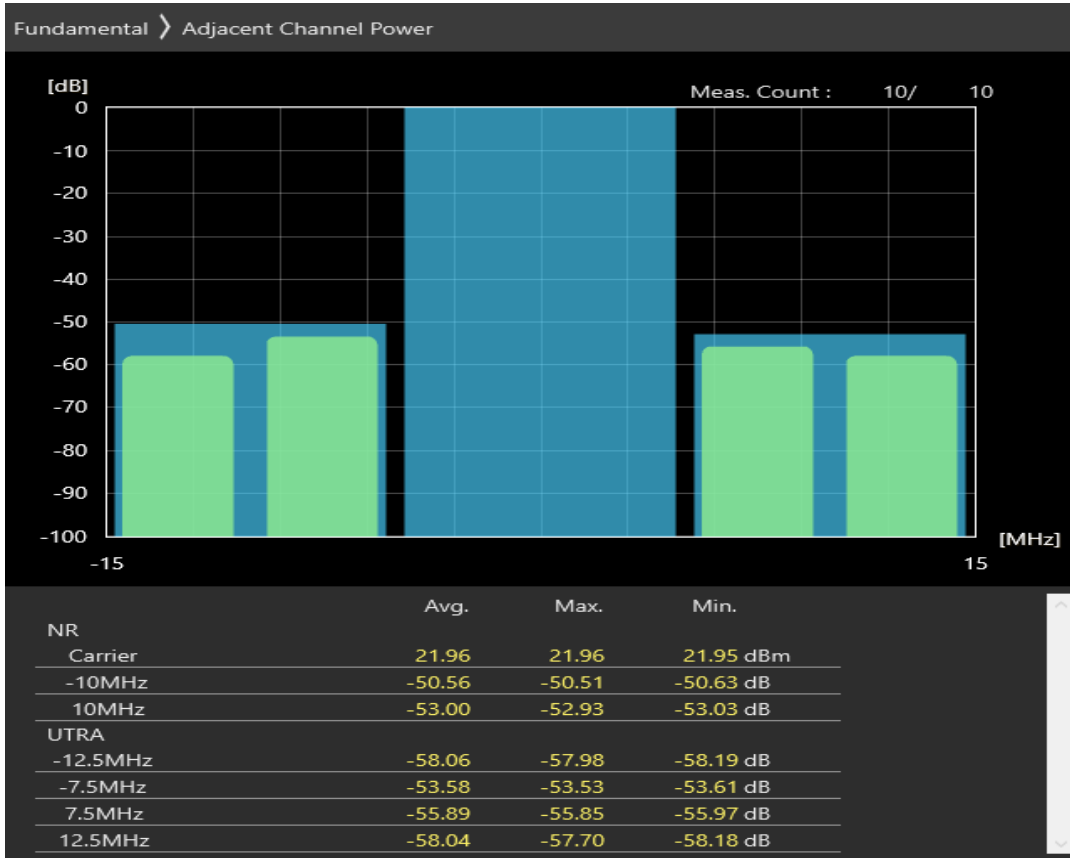
n38 SCS=30kHz DFT_QAM64 BW=10MHz Channel=515000 RB=24@0
