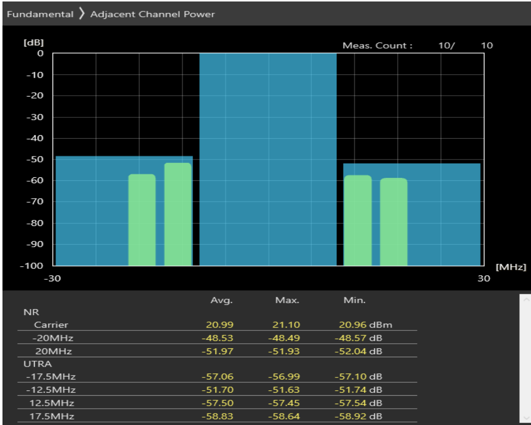
n38 SCS=30kHz CP_QAM64 BW=20MHz Channel=522000 RB=1 @50
