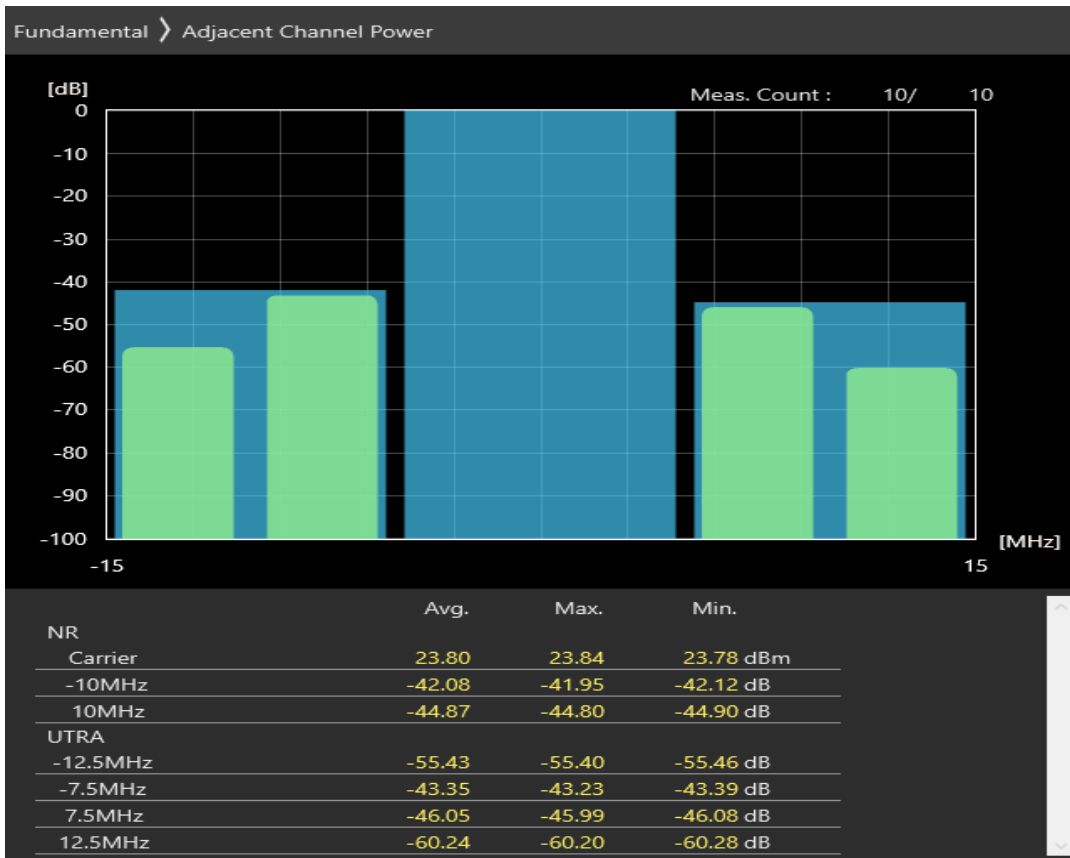
n28 SCS=30kHz DFT_QPSK BW=10MHz Channel=148600 RB=1@23
