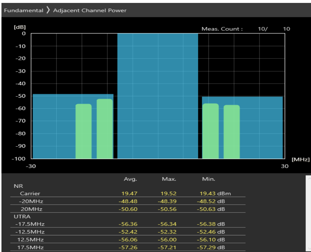
n1 SCS=30kHz CP_QAM64 BW=20MHz Channel=386000 RB=51 @0
