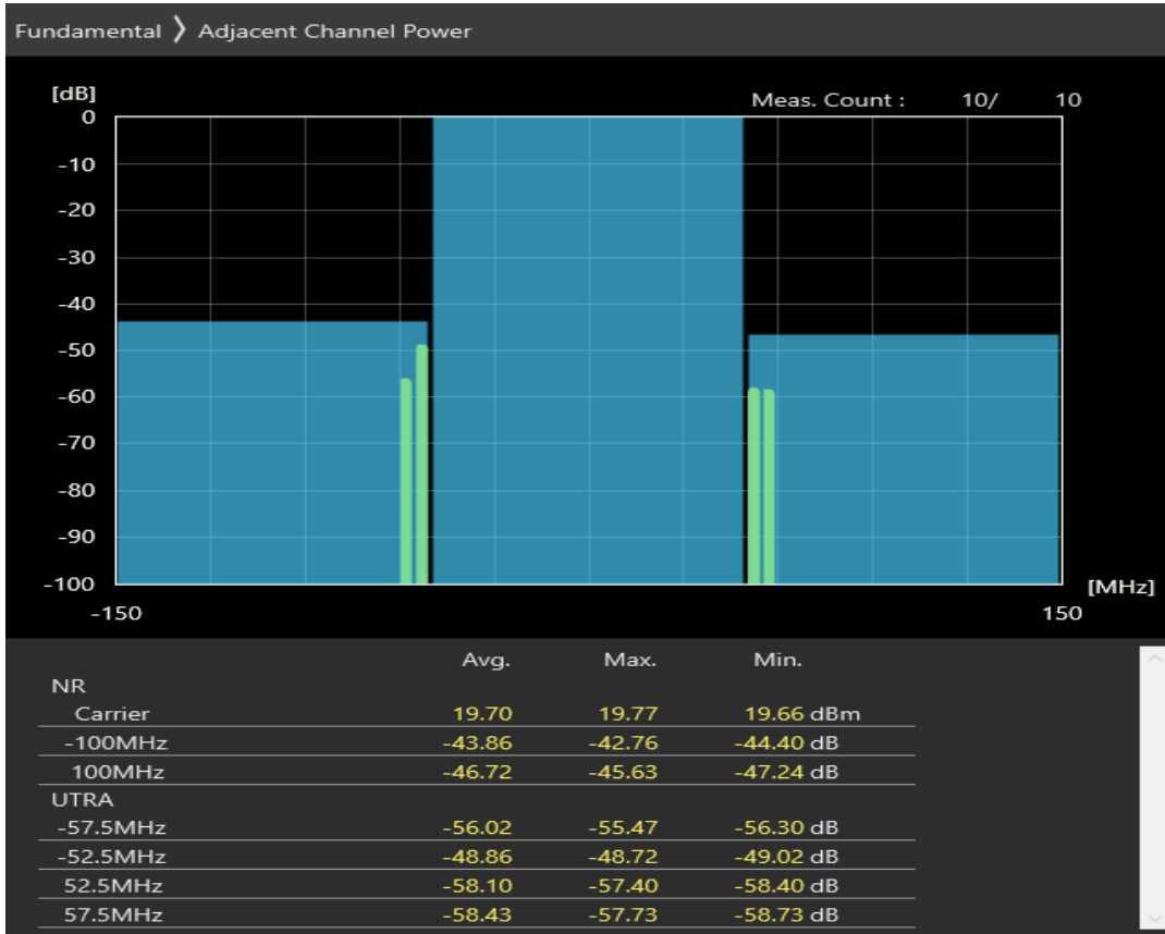
n78 SCS=30kHz DFT_QAM16 BW=100MHz Channel=650000 RB=270@0
