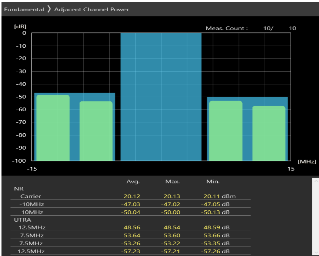
n3 SCS=30kHz CP_QAM16 BW=10MHz Channel=356000 RB=24@0
