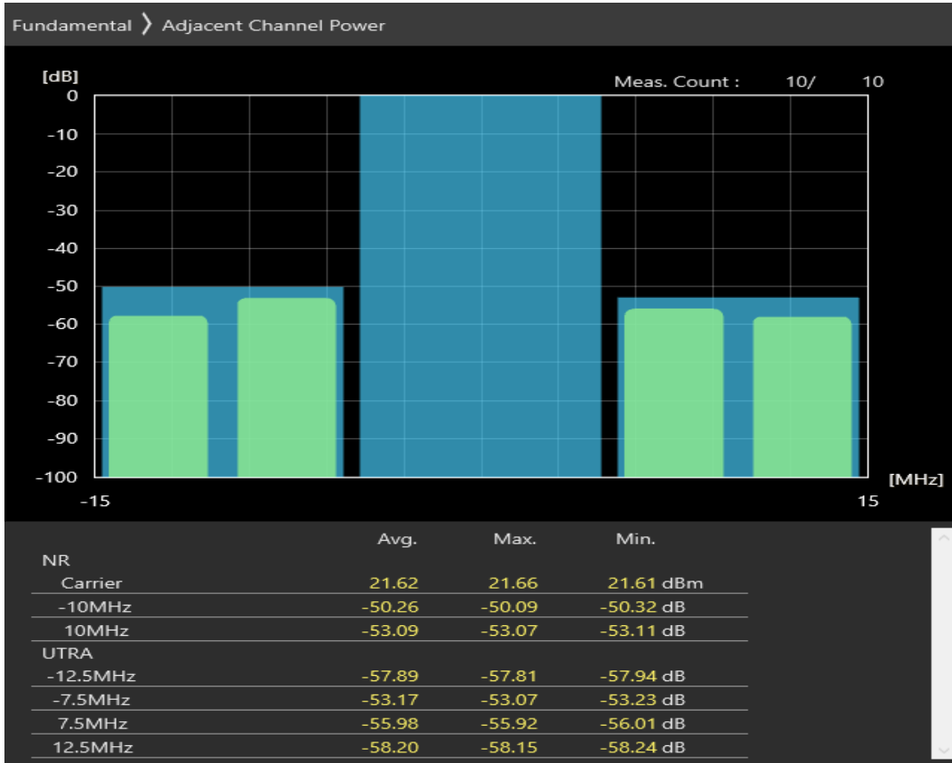
n78 SCS=30kHz DFT_QAM64 BW=10MHz Channel=647000 RB=24@0
