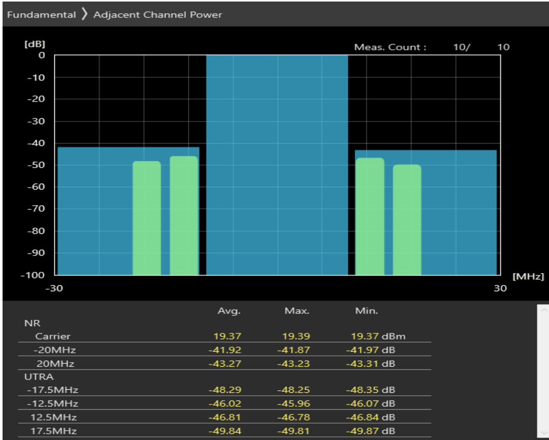
n1 SCS=30kHz DFT_QAM64 BW=10MHz Channel=385000 RB=1@0
