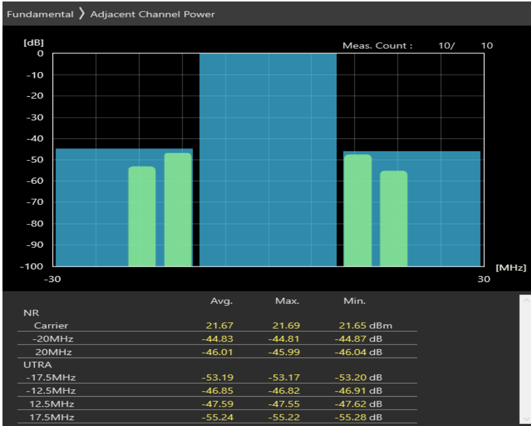
n20 SCS=30kHz CP_QAM16 BW=20MHz Channel=170400 RB=1@50
