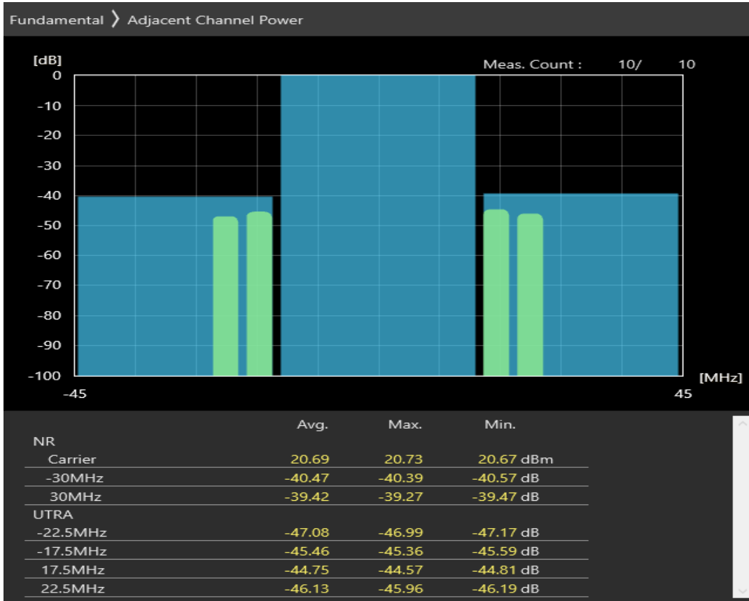
n3 SCS=30kHz CP_QPSK BW=30MHz Channel=345000 RB=1@0
