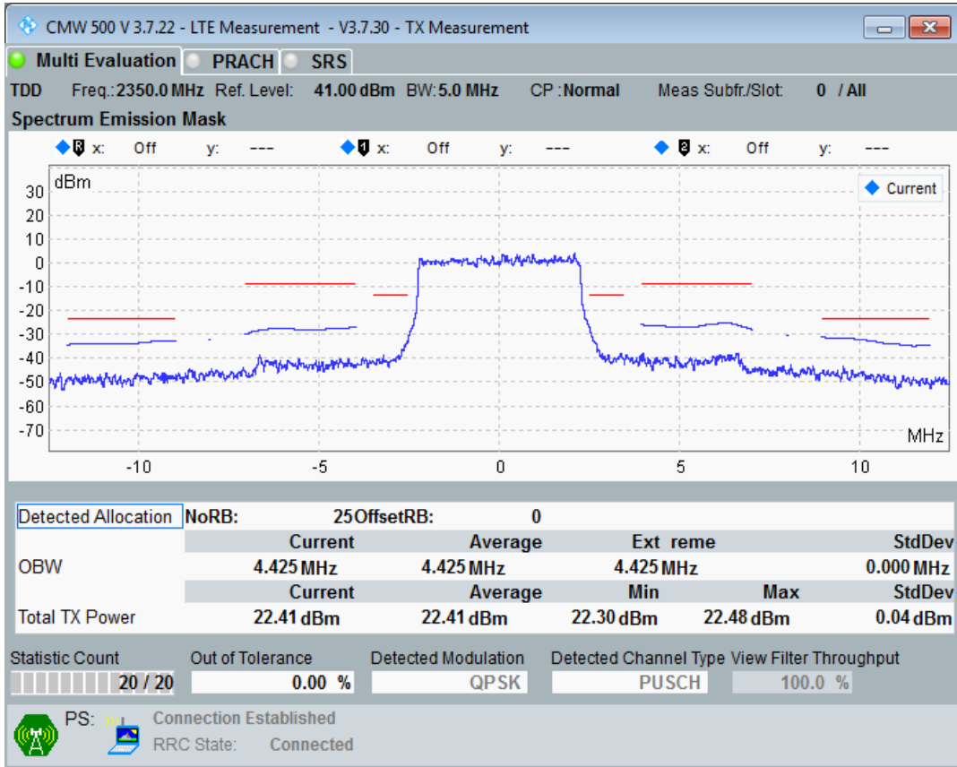
Band40 QPSK BW=5MHz Channel=39150 RB Size=8 Position=#0
