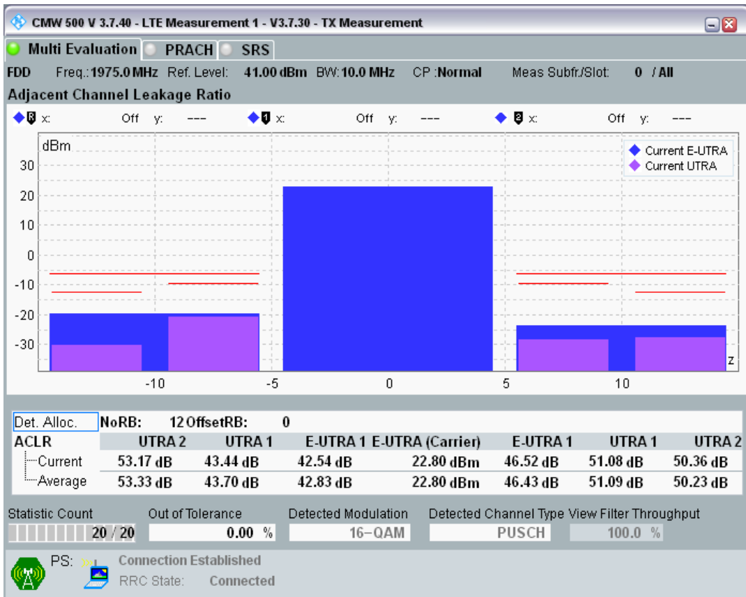
Band1 QAM16 BW=10MHz Channel=18550 RB Size=12 Position=#Max
