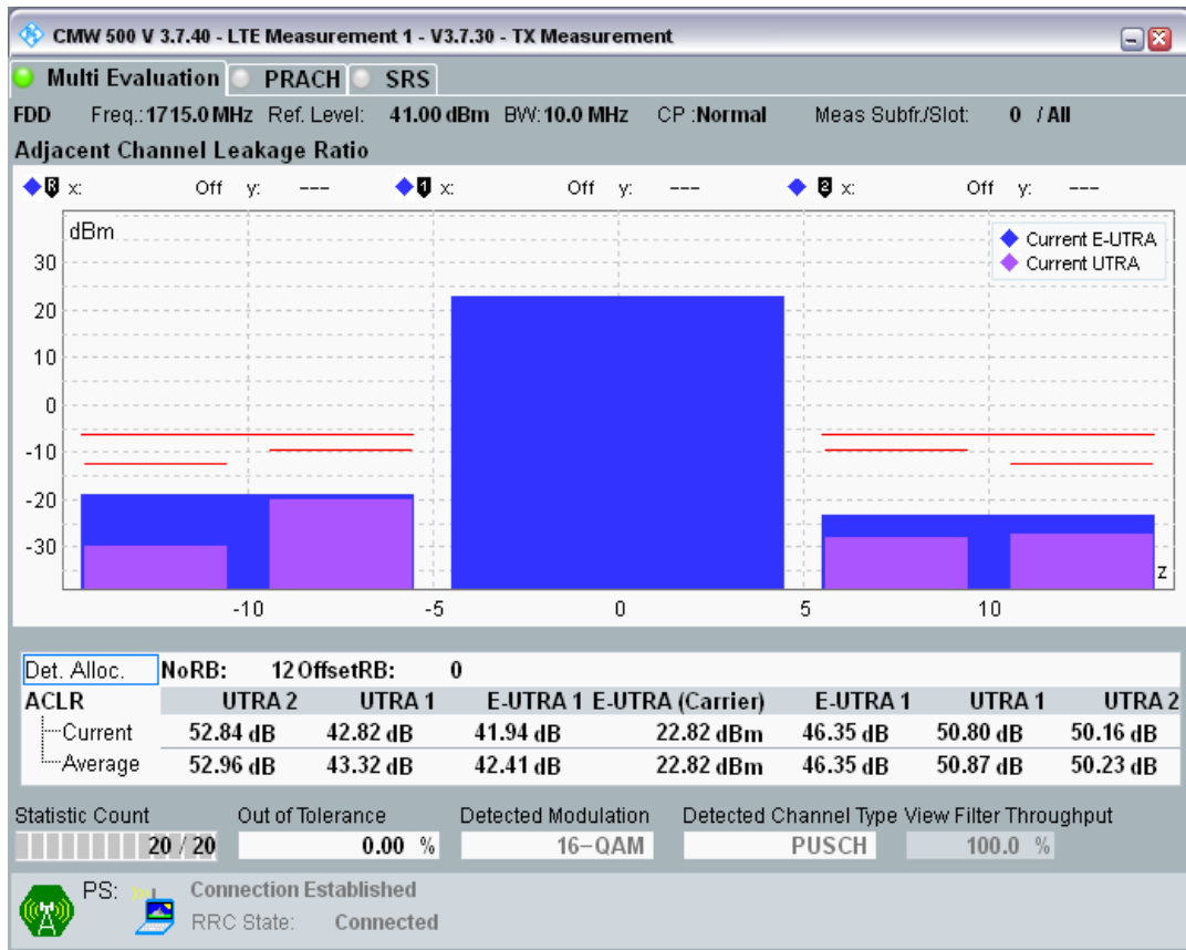
Band3 QAM16 BW=10MHz Channel=19250 RB Size=12 Position=#Max
