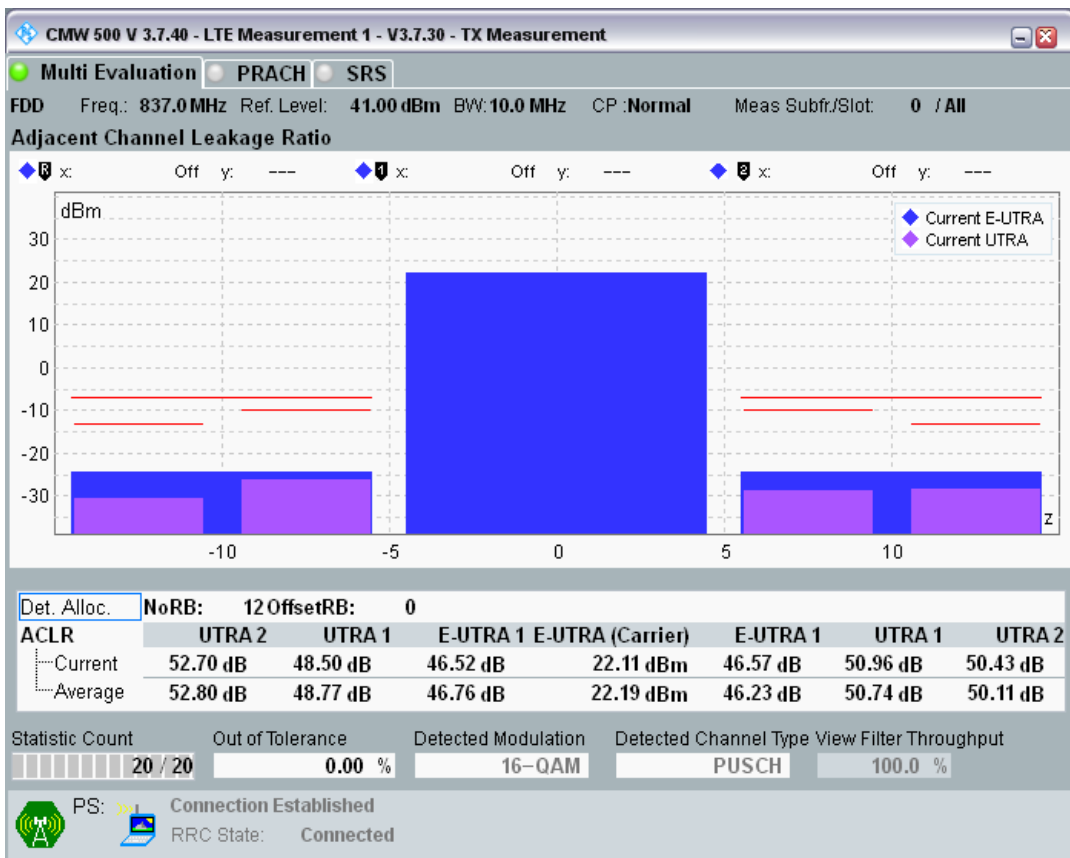
Band20 QAM16 BW=10MHz Channel=24200 RB Size=12 Position=#Max
