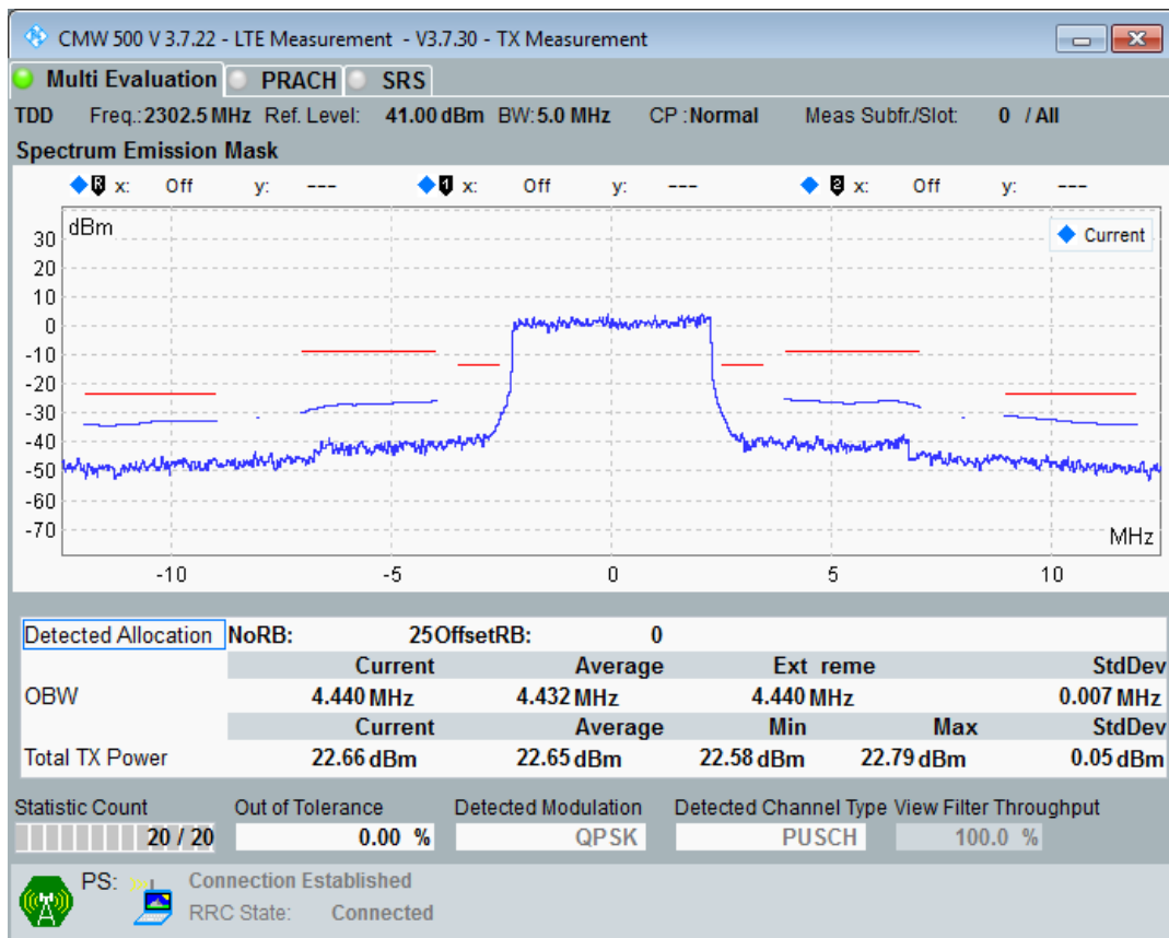
Band40 QPSK BW=20MHz Channel=39550 RB Size=100 Position=#0
