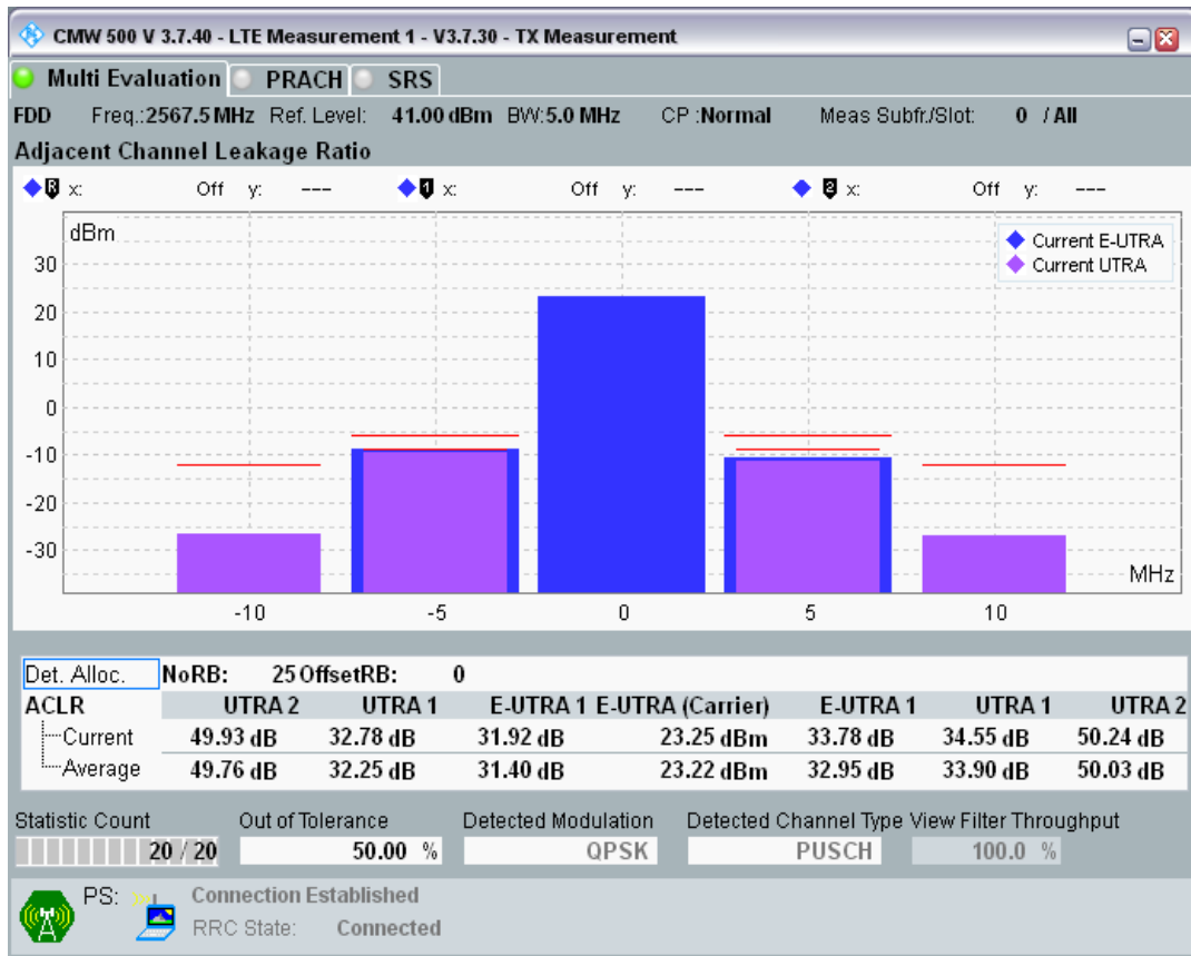
Band7 QAM16 BW=5MHz Channel=21425 RB Size=8 Position=#0
