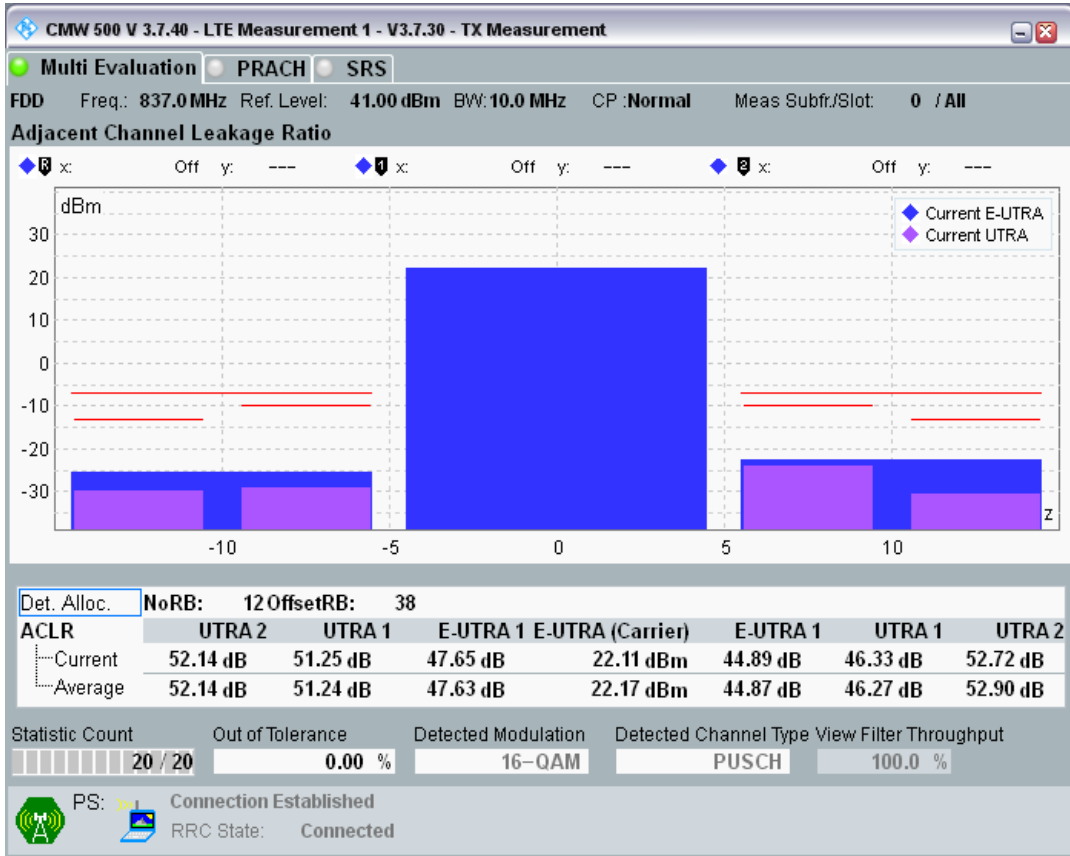
Band20 QAM16 BW=10MHz Channel=24200 RB Size=50 Position=#0
