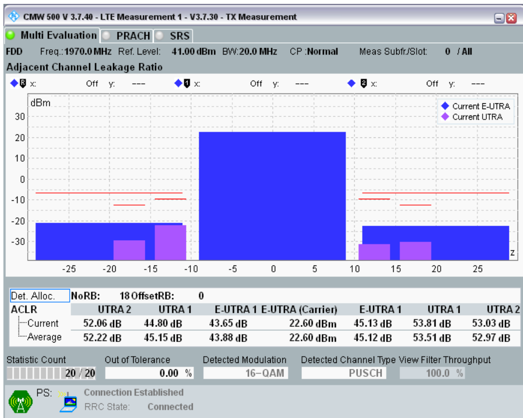
Band1 QAM16 BW=20MHz Channel=18500 RB Size=18 Position=#Max
