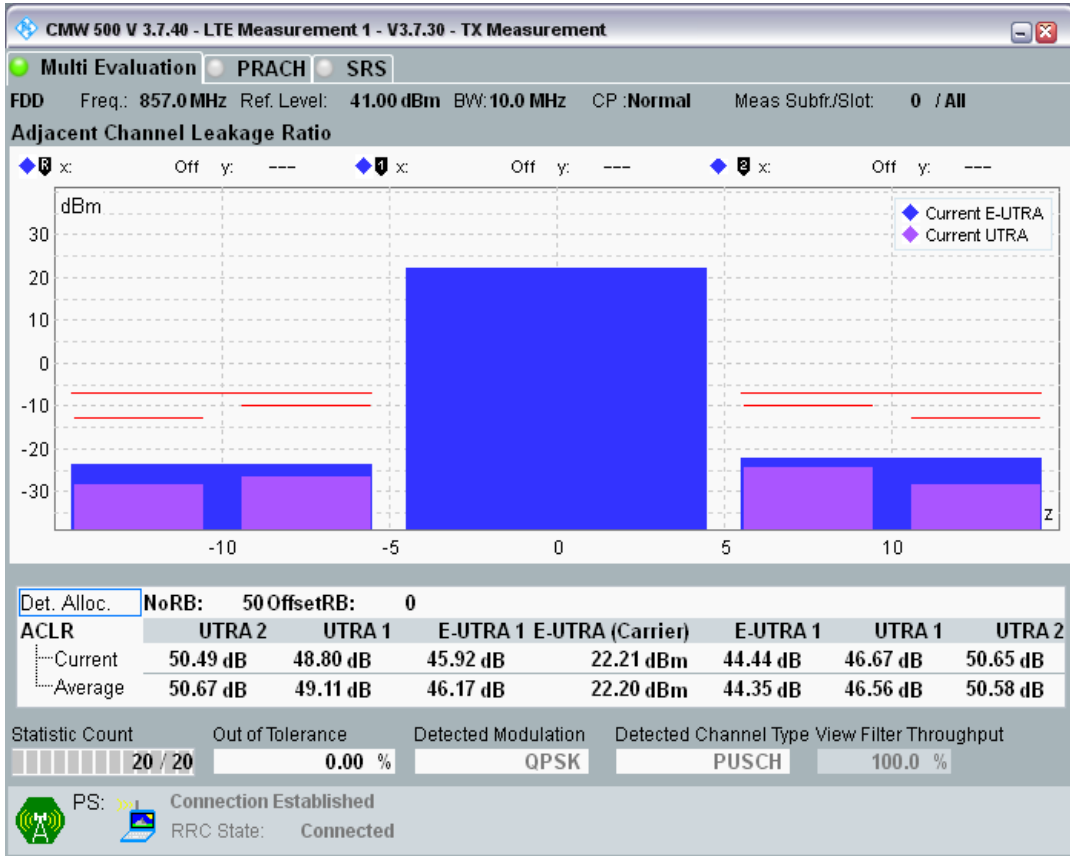
Band20 QAM16 BW=10MHz Channel=24400 RB Size=12 Position=#0
