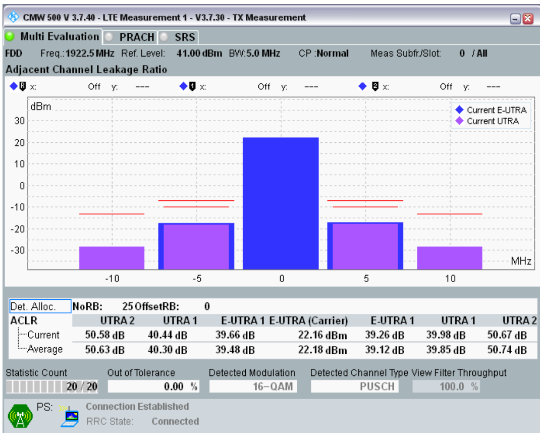
Band1 QPSK BW=5MHz Channel=18300 RB Size=8 Position=#0
