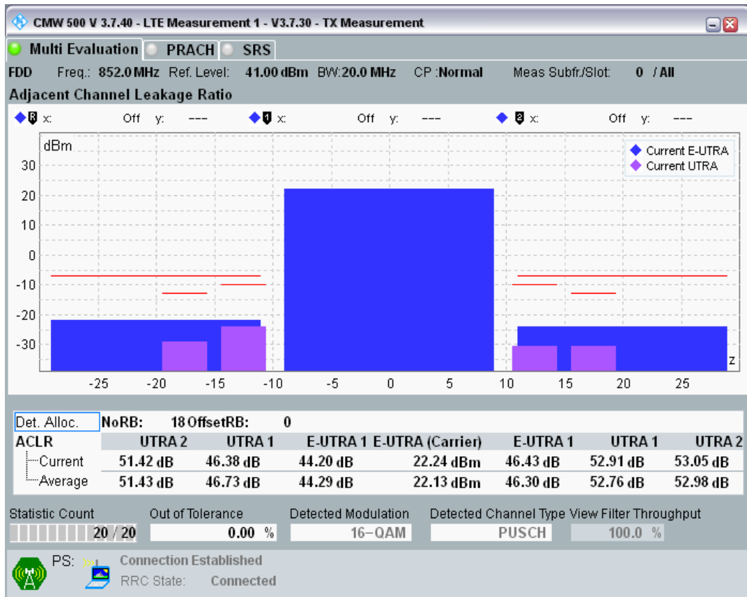
Band20 QAM16 BW=20MHz Channel=24350 RB Size=18 Position=#Max
