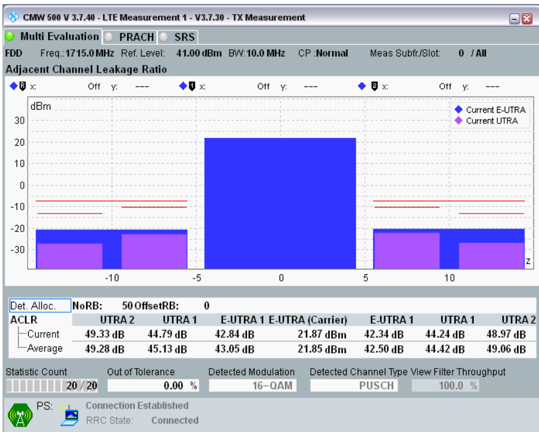
Band3 QPSK BW=10MHz Channel=19575 RB Size=12 Position=#0
