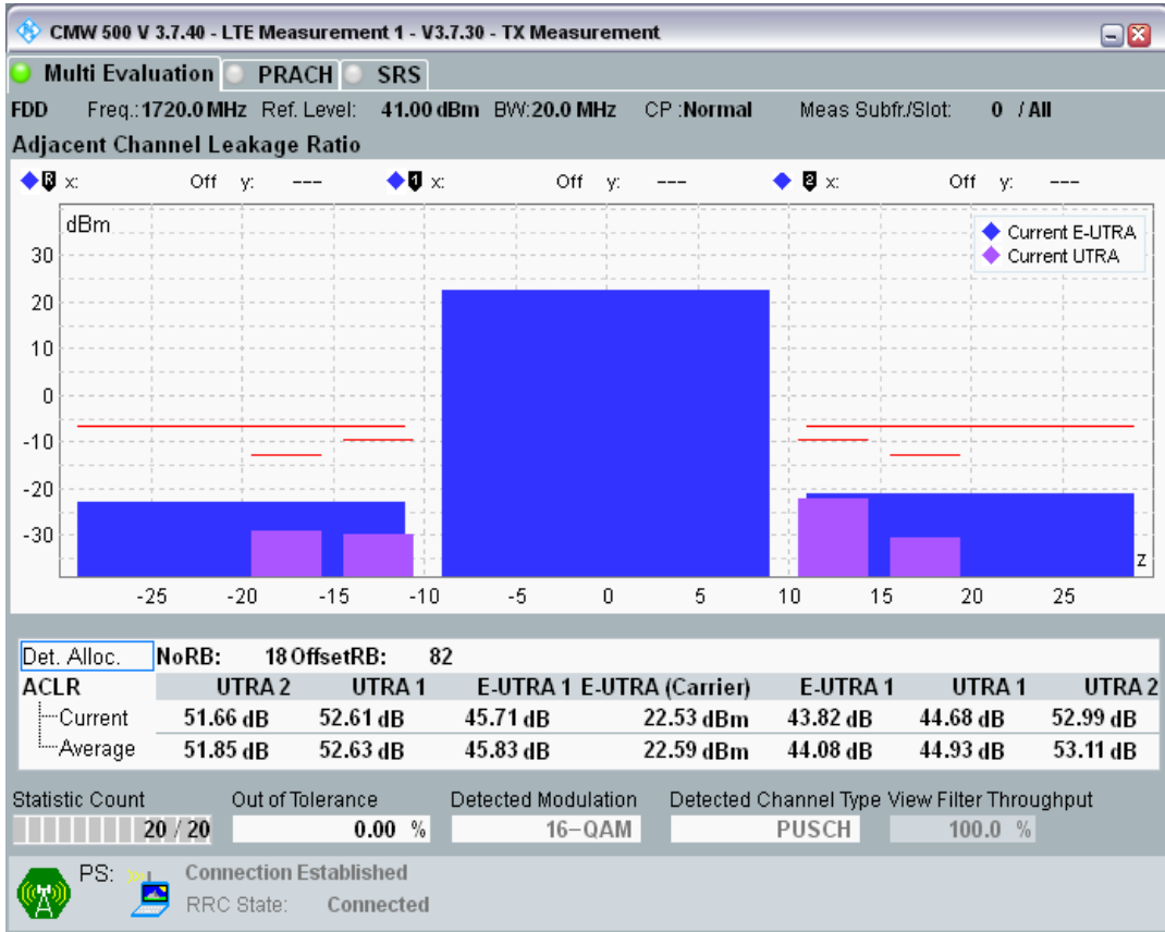
Band3 QAM16 BW=20MHz Channel=19300 RB Size=100 Position=#0
