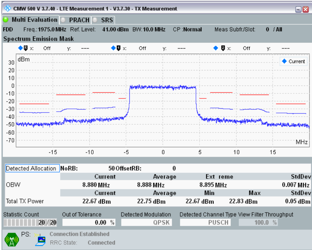
Band1 QAM16 BW=10MHz Channel=18550 RB Size=12 Position=#0
