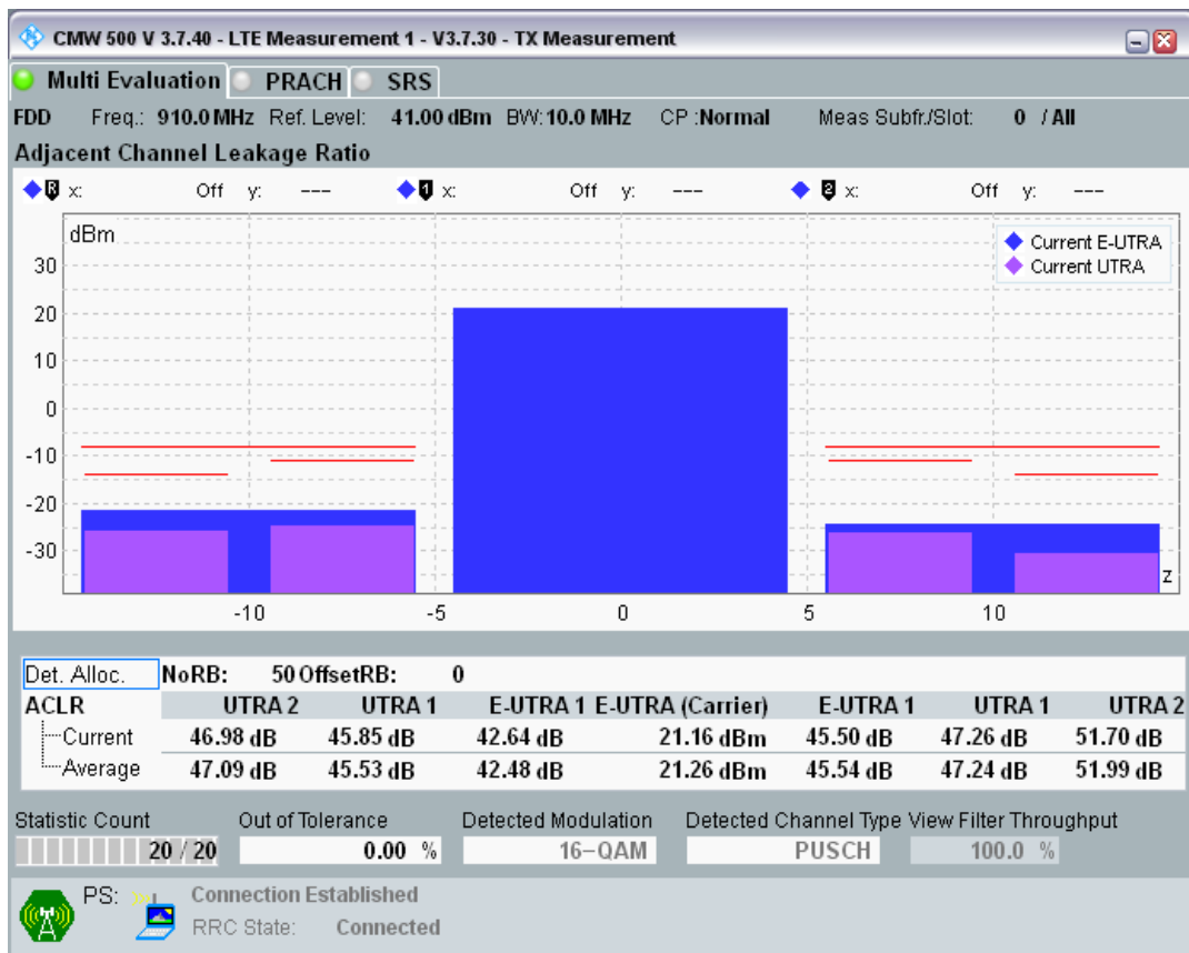
Band8 QAM16 BW=10MHz Channel=21750 RB Size=50 Position=#0
