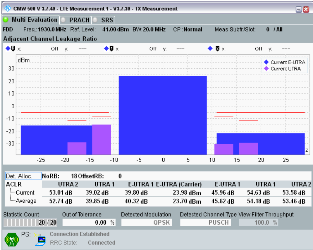
Band1 QPSK BW=20MHz Channel=18100 RB Size=18 Position=#Max
