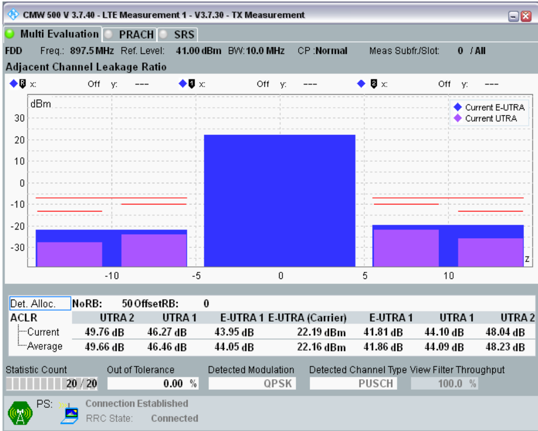
Band8 QAM16 BW=10MHz Channel=21625 RB Size=12 Position=#0
