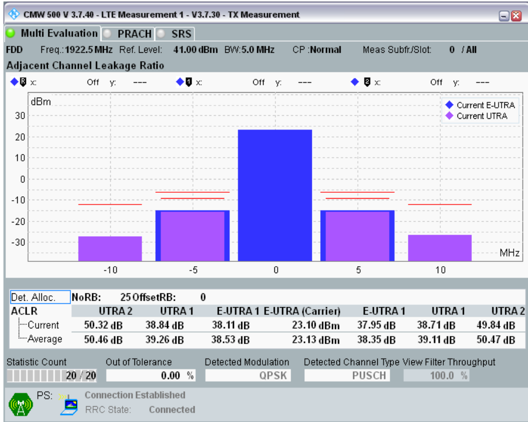
Band1 QAM16 BW=5MHz Channel=18025 RB Size=8 Position=#0
