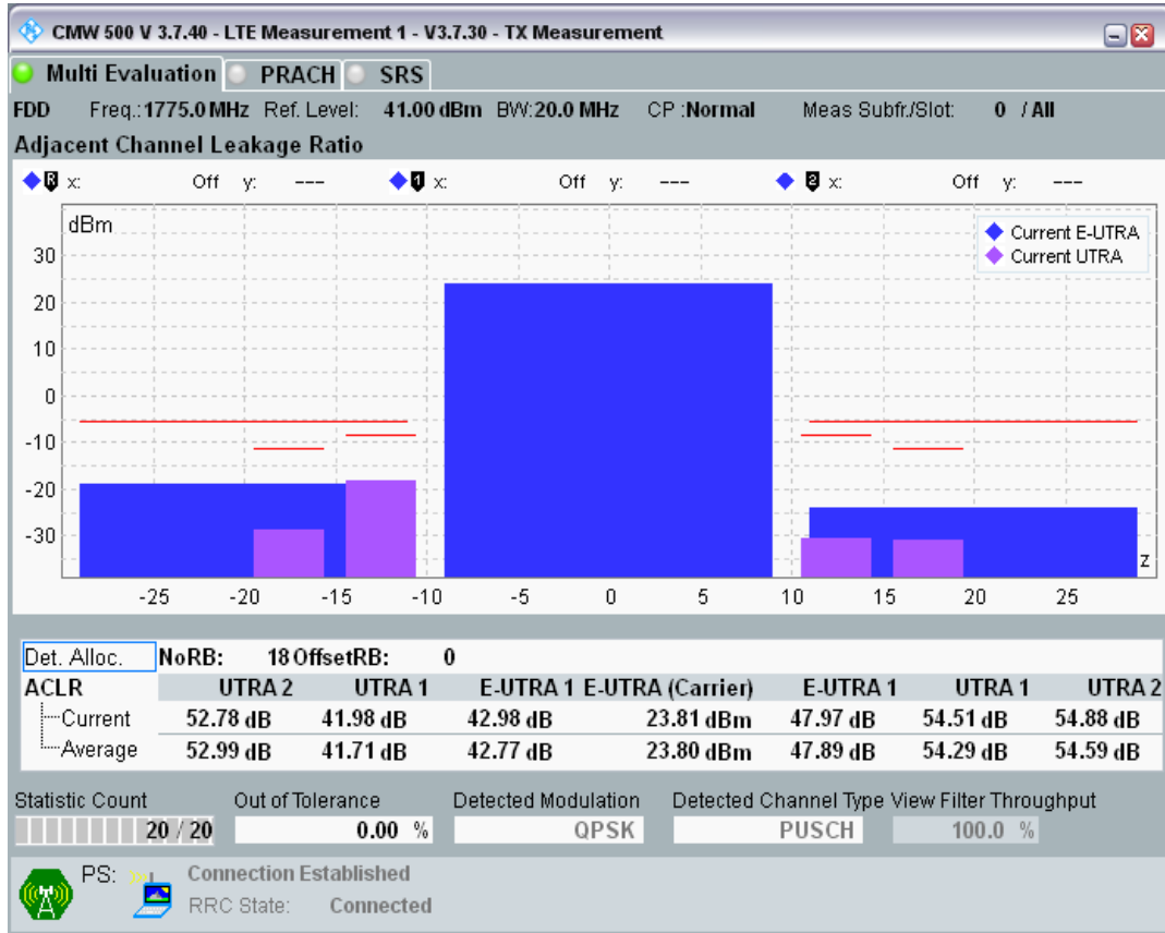
Band3 QPSK BW=20MHz Channel=19850 RB Size=18 Position=#Max
