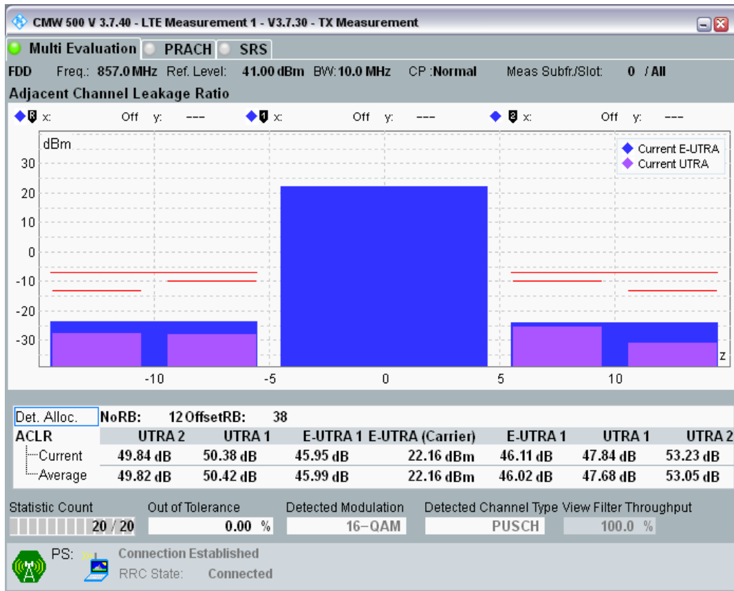
Band20 QAM16 BW=10MHz Channel=24400 RB Size=50 Position=#0
