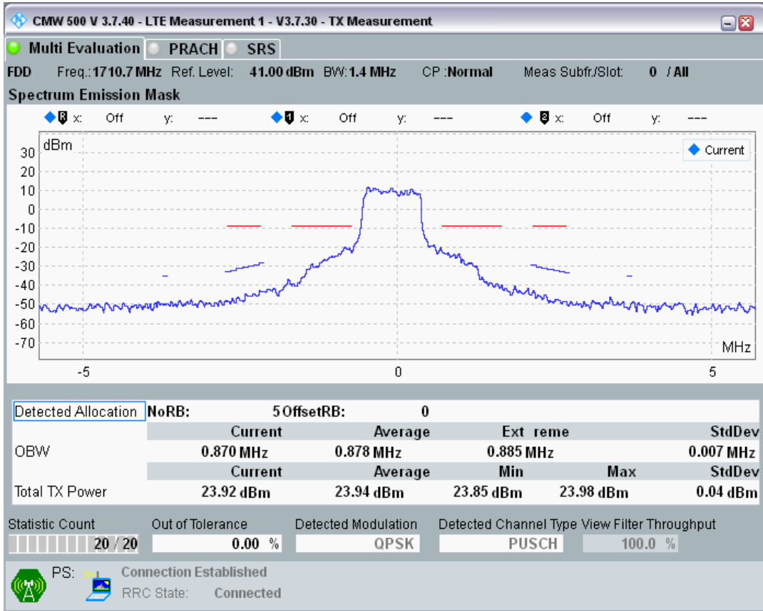
Band3 QPSK BW=1.4MHz Channel=19207 RB Size=5 Position=#Max
