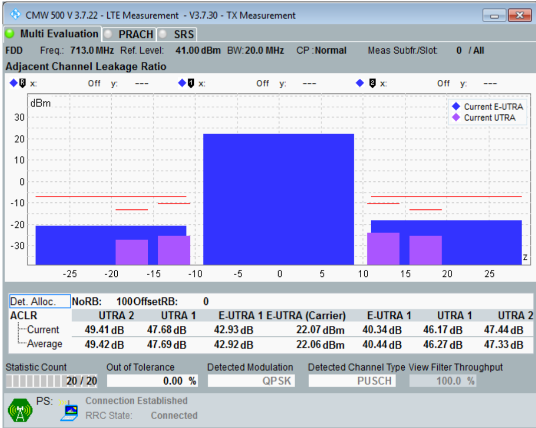
Band28 QAM16 BW=20MHz Channel=27310 RB Size=18 Position=#0
