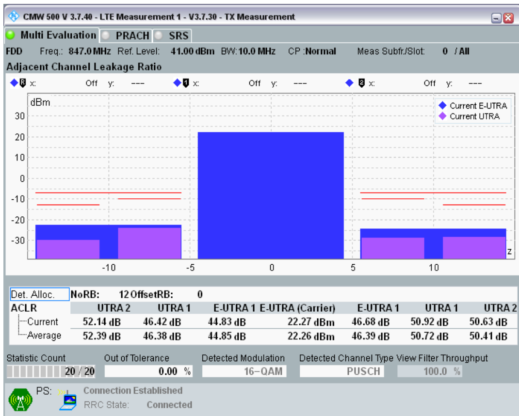
Band20 QAM16 BW=10MHz Channel=24300 RB Size=12 Position=#Max
