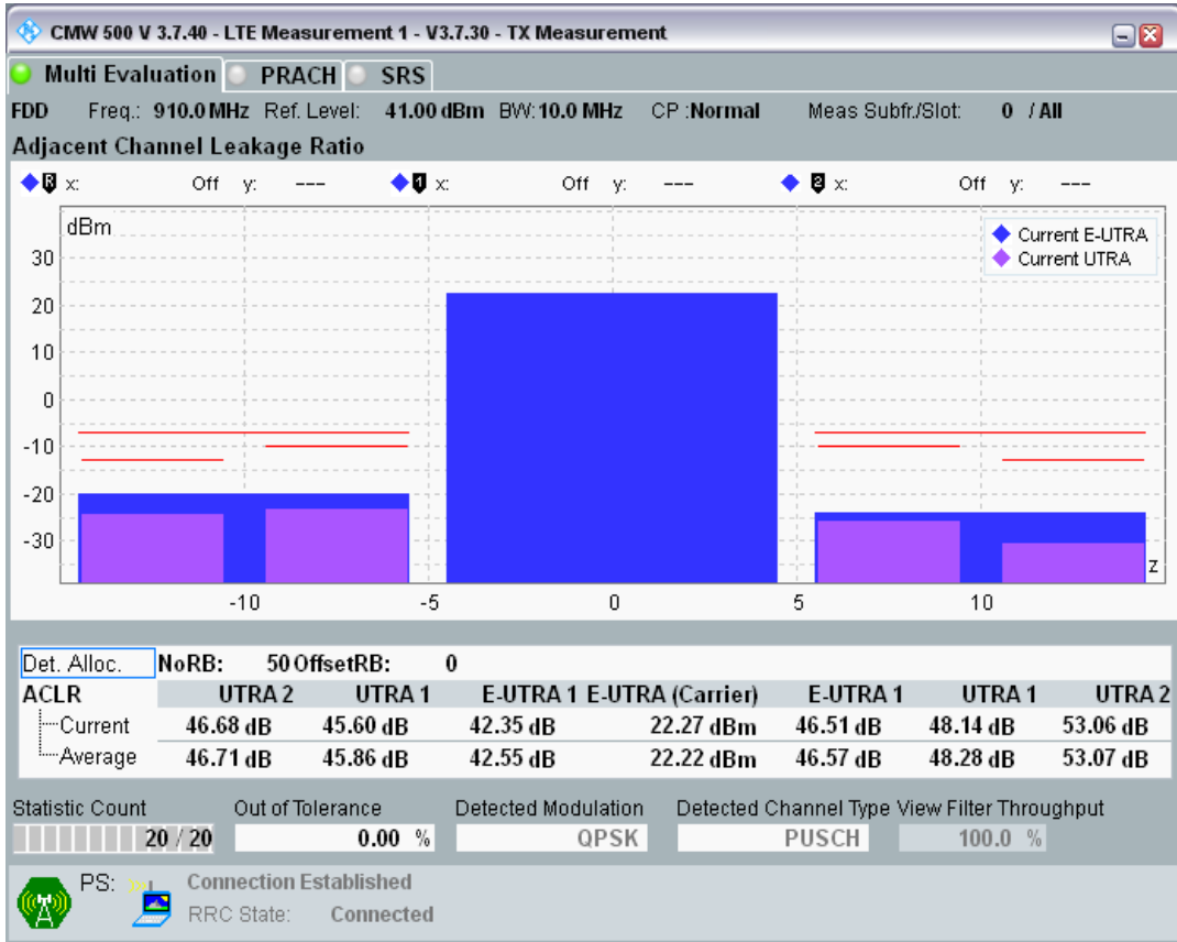
Band8 QAM16 BW=10MHz Channel=21750 RB Size=12 Position=#0
