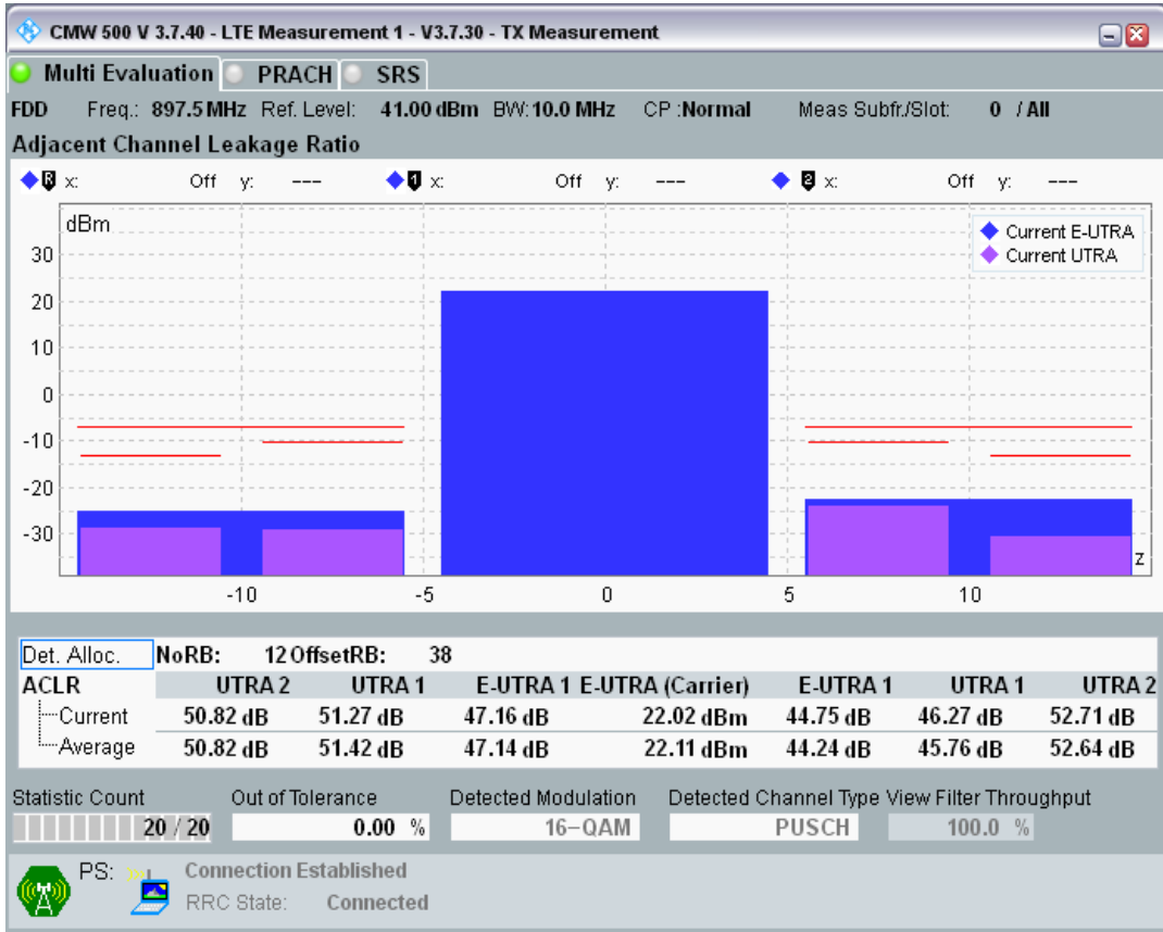
Band8 QAM16 BW=10MHz Channel=21625 RB Size=50 Position=#0
