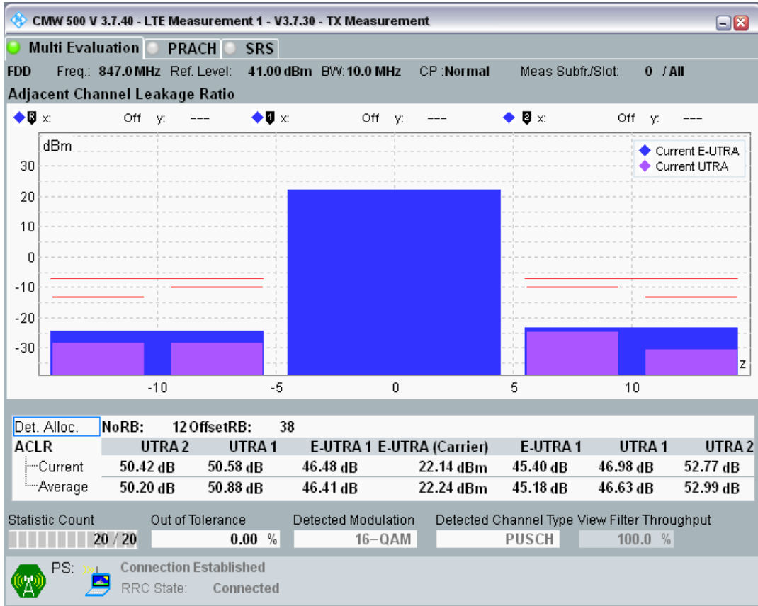
Band20 QAM16 BW=10MHz Channel=24300 RB Size=50 Position=#0
