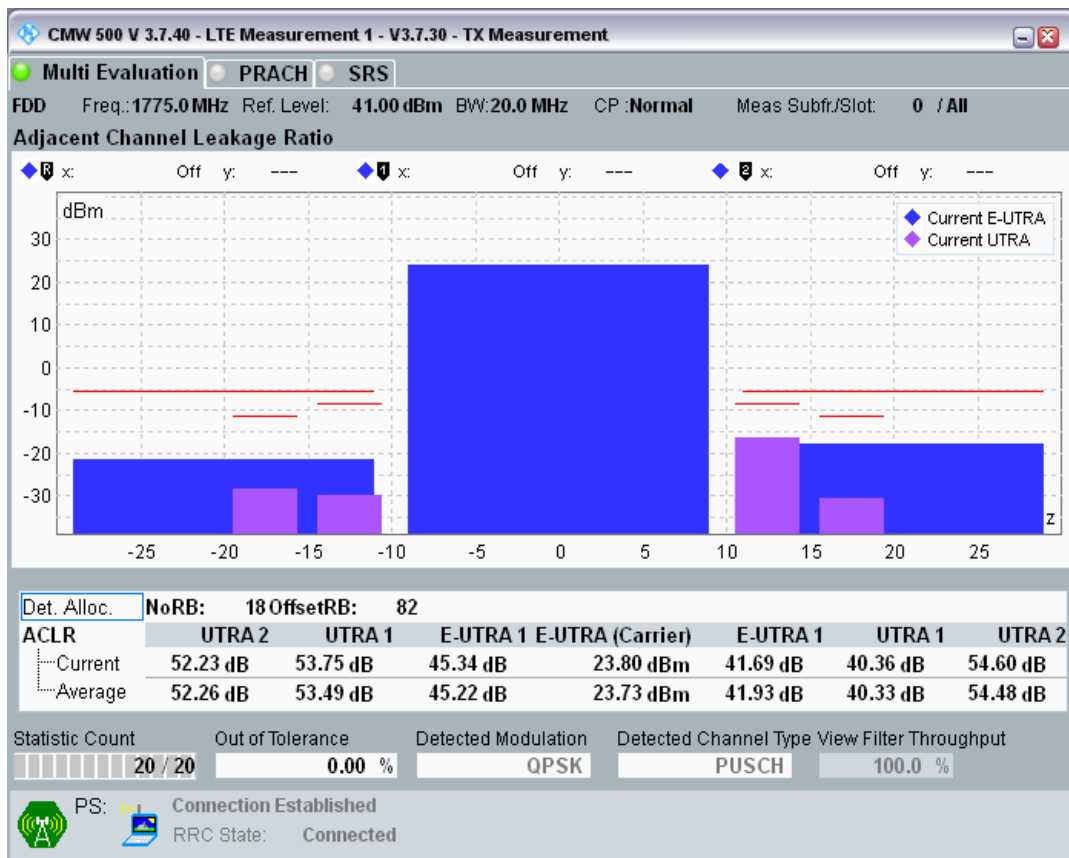
Band3 QPSK BW=20MHz Channel=19850 RB Size=100 Position=#0
