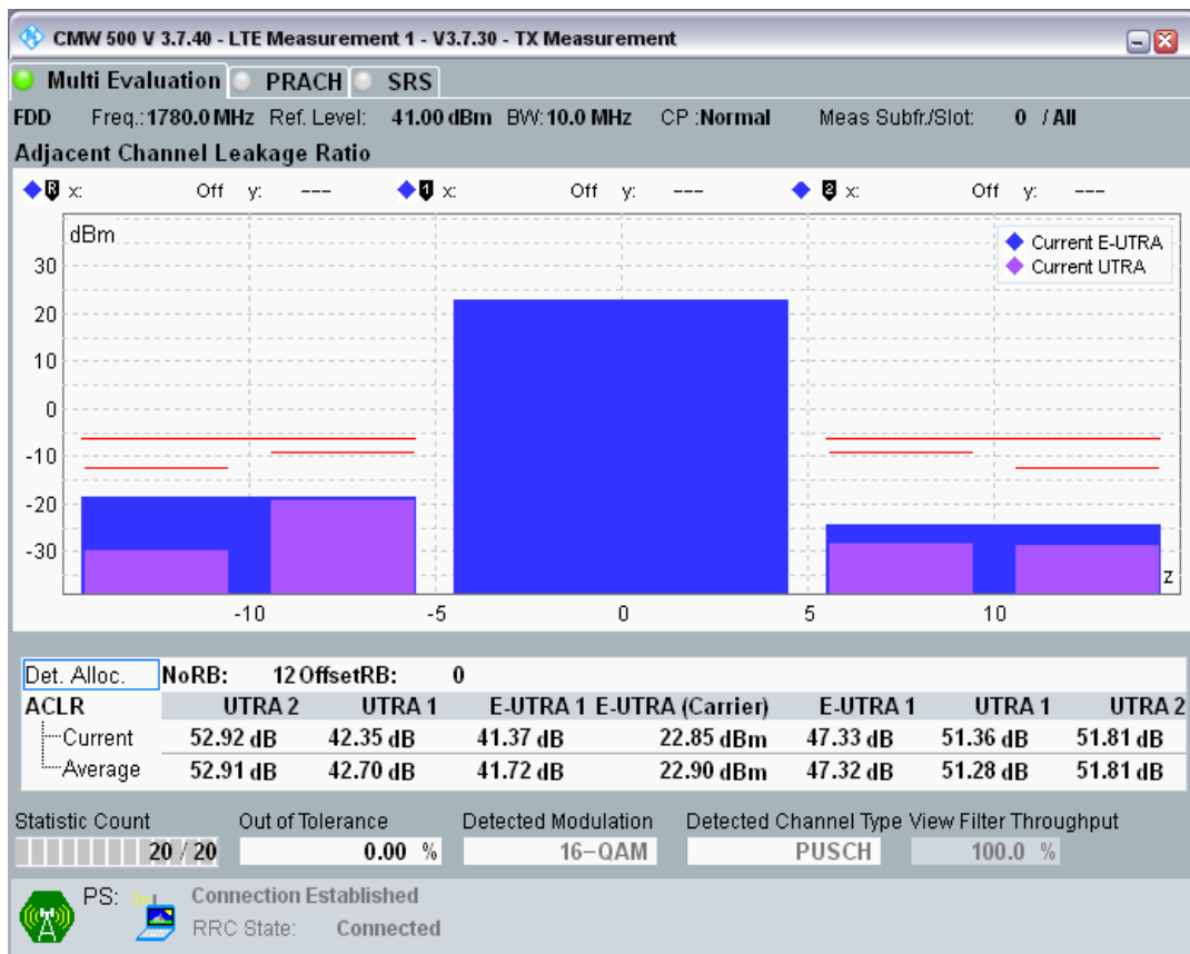
Band3 QAM16 BW=10MHz Channel=19900 RB Size=12 Position=#Max
