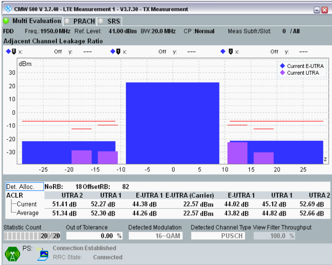
Band1 QAM16 BW=20MHz Channel=18300 RB Size=100 Position=#0
