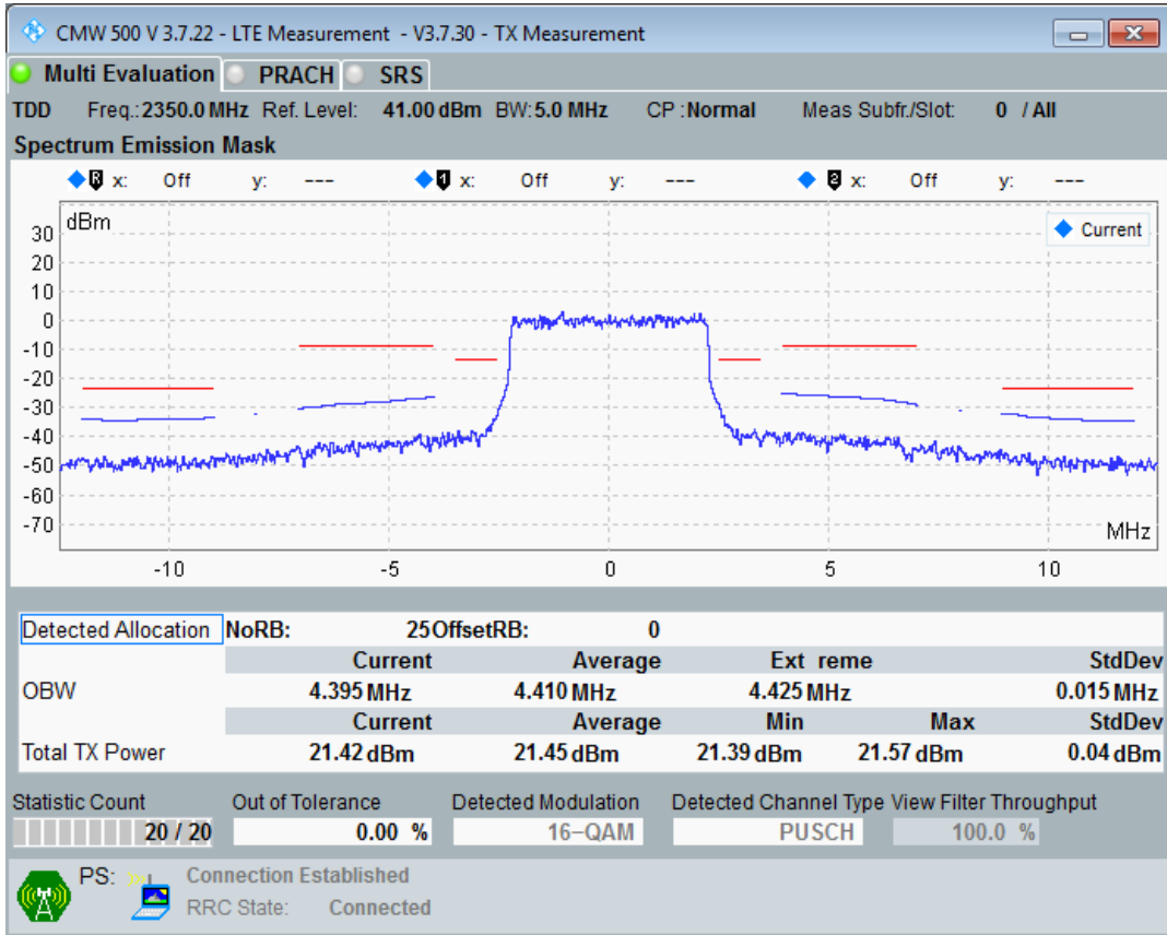
Band40 QAM16 BW=5MHz Channel=39150 RB Size=8 Position=#0
