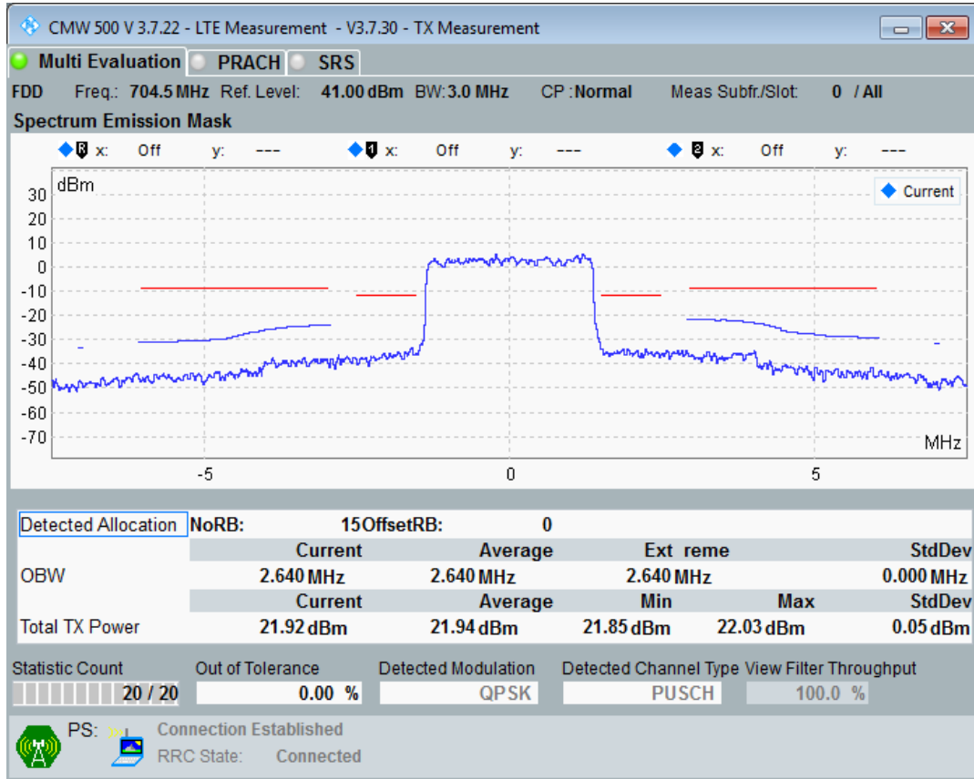
Band28 QAM16 BW=3MHz Channel=27225 RB Size=4 Position=#0
