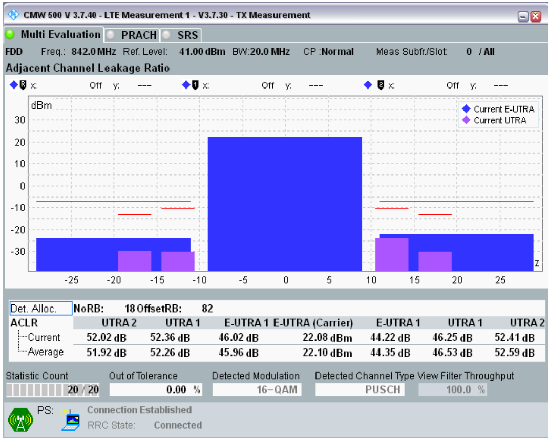
Band20 QAM16 BW=20MHz Channel=24250 RB Size=100 Position=#0
