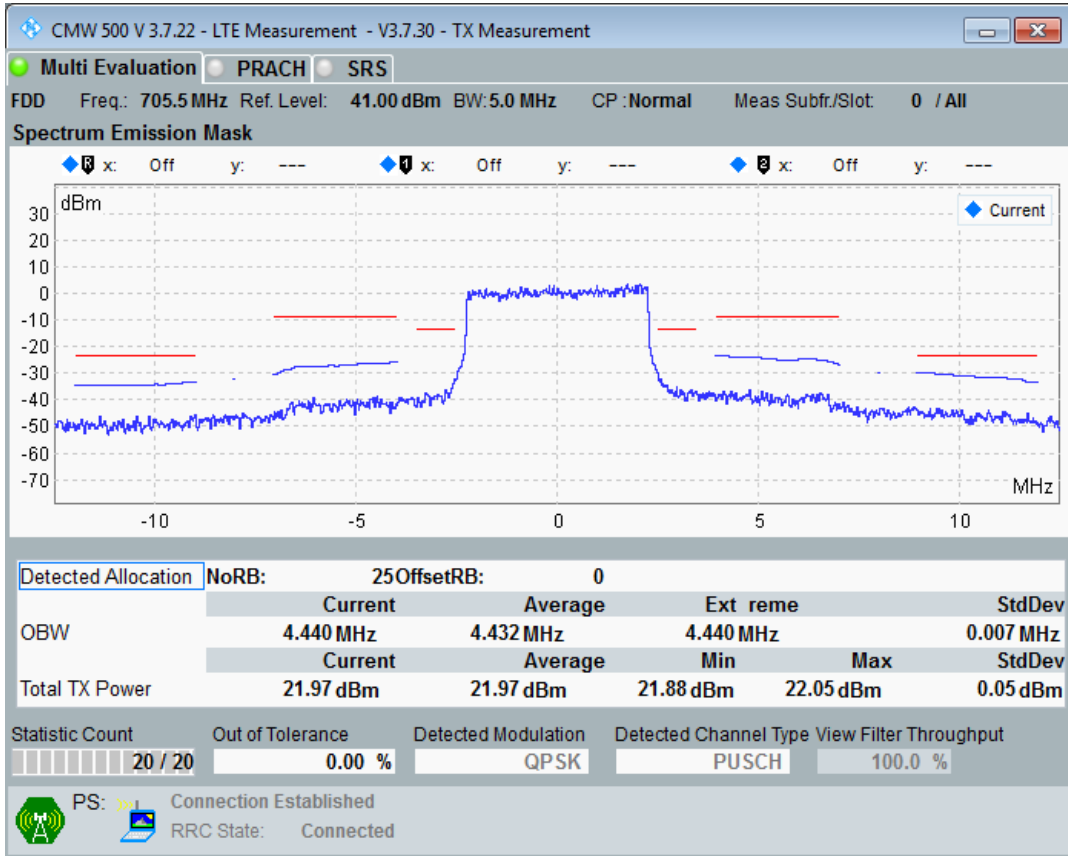
Band28 QAM16 BW=5MHz Channel=27235 RB Size=8 Position=#0
