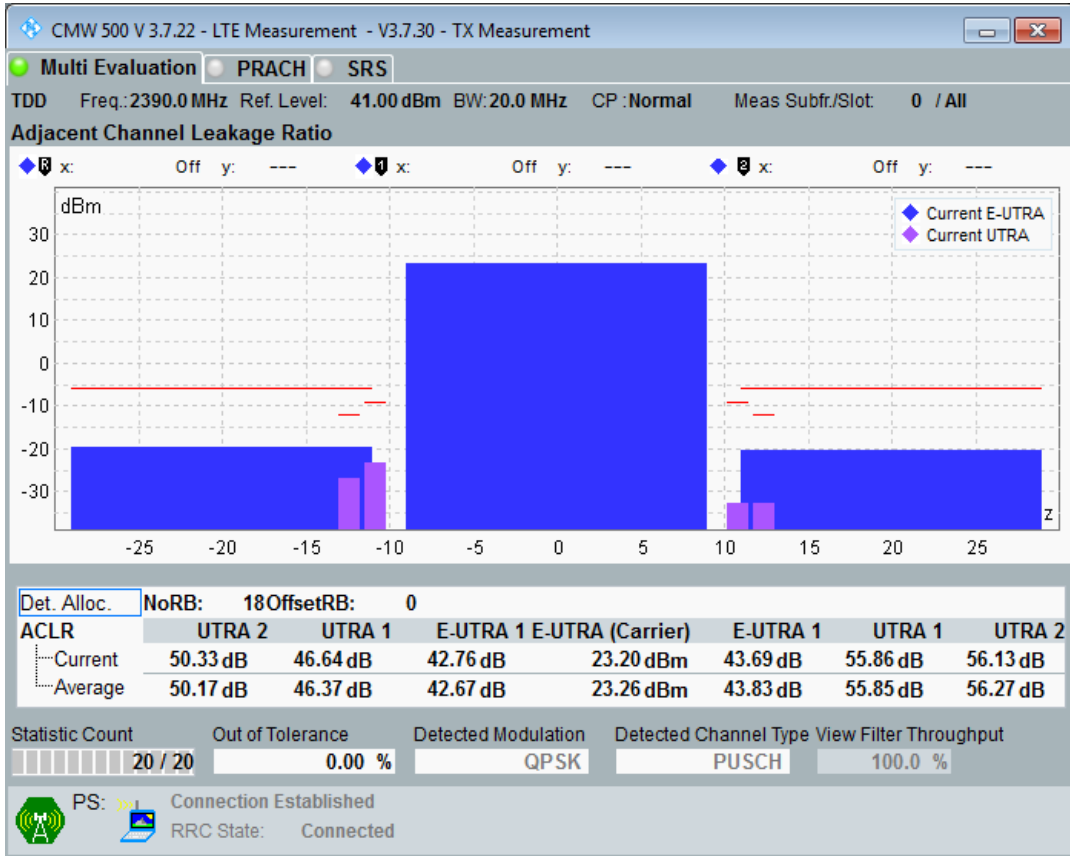
Band40 QPSK BW=5MHz Channel=38675 RB Size=25 Position=#0
