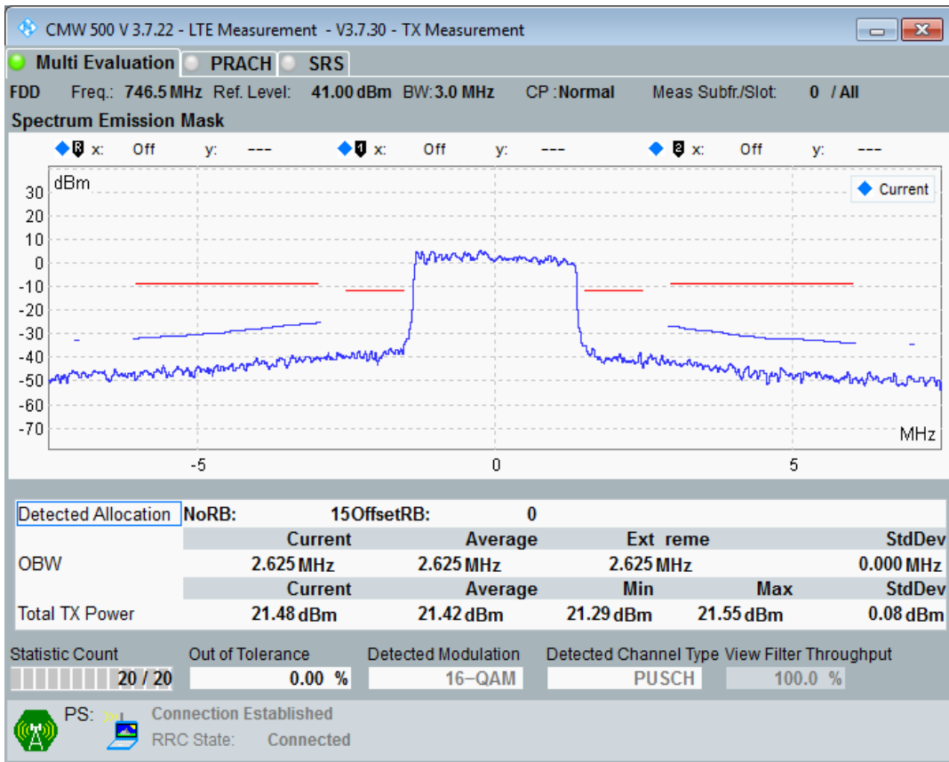
Band28 QPSK BW=5MHz Channel=27235 RB Size=8 Position=#0
