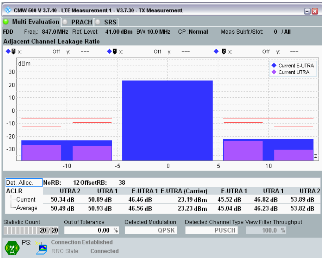
Band20 QPSK BW=10MHz Channel=24300 RB Size=50 Position=#0
