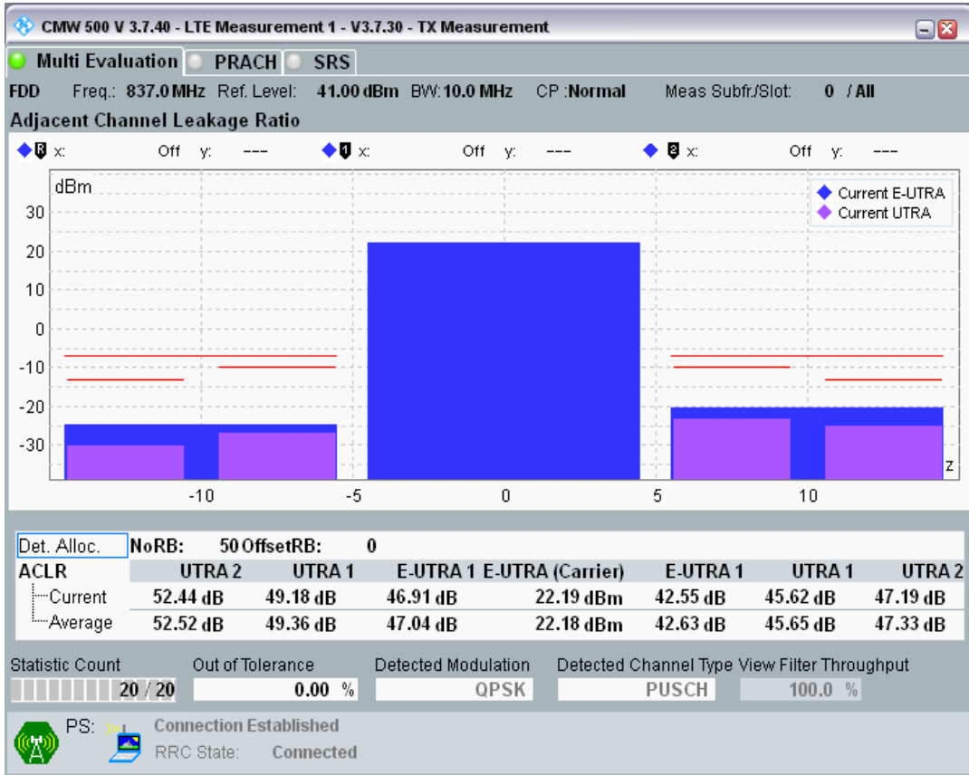
Band20 QAM16 BW=10MHz Channel=24200 RB Size=12 Position=#0
