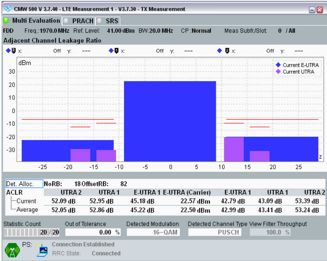
Band1 QAM16 BW=20MHz Channel=18500 RB Size=100 Position=#0
