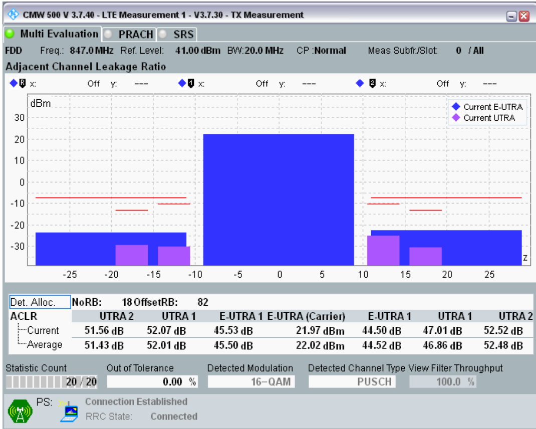
Band20 QAM16 BW=20MHz Channel=24300 RB Size=100 Position=#0
