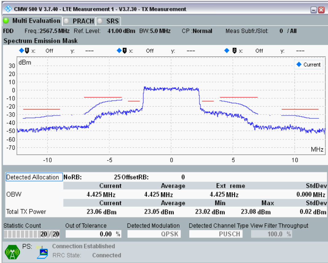
Band7 QAM16 BW=5MHz Channel=21425 RB Size=8 Position=#0
