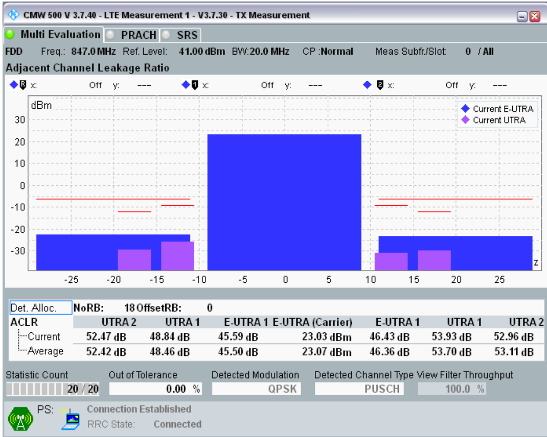
Band20 QPSK BW=20MHz Channel=24300 RB Size=18 Position=#Max
