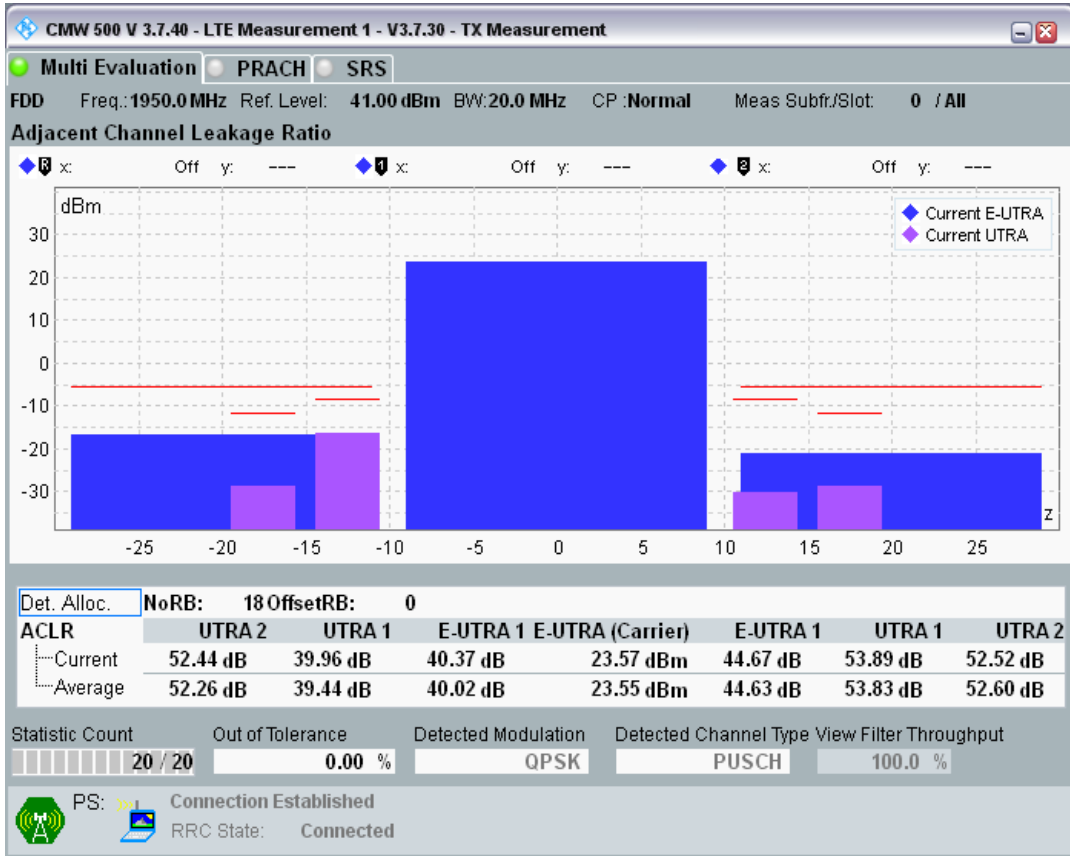
Band1 QPSK BW=20MHz Channel=18300 RB Size=18 Position=#Max
