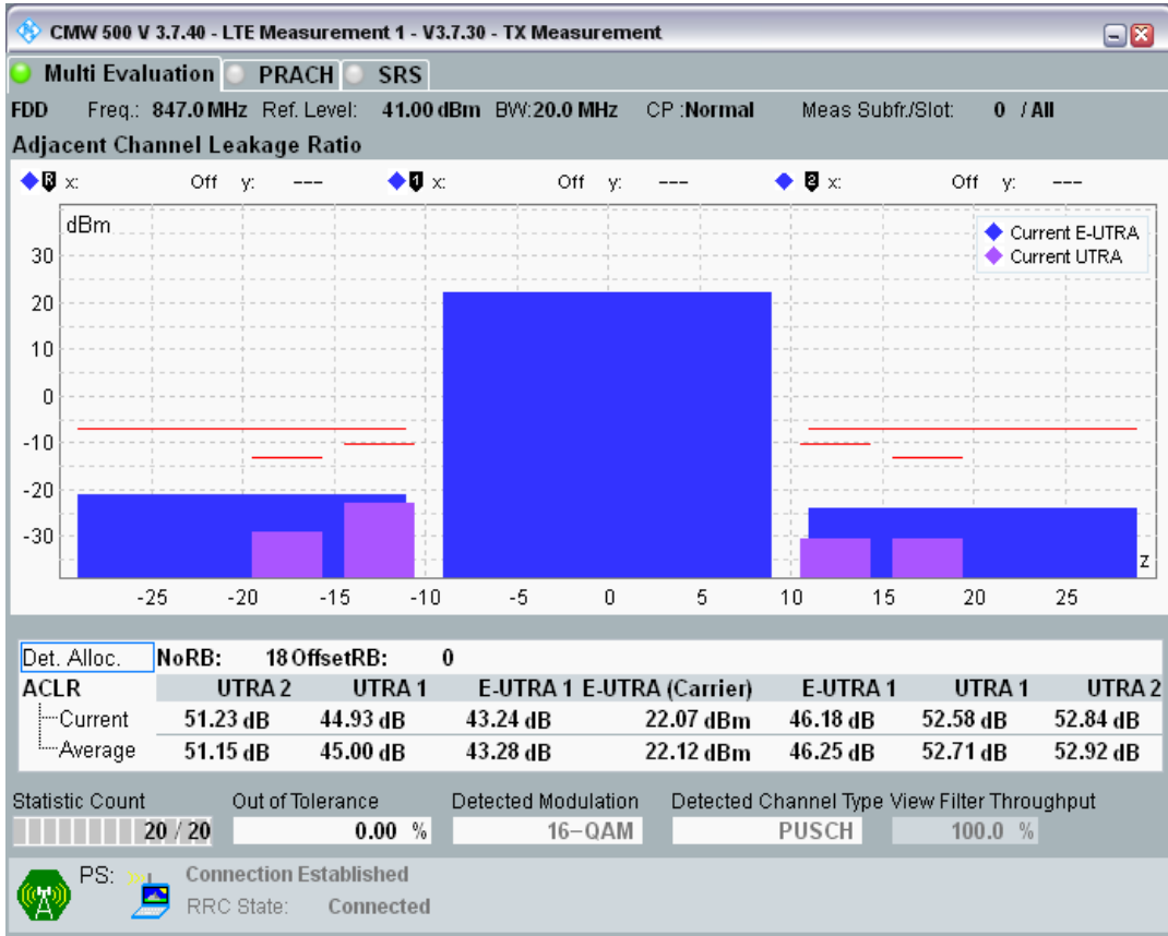
Band20 QAM16 BW=20MHz Channel=24300 RB Size=18 Position=#Max
