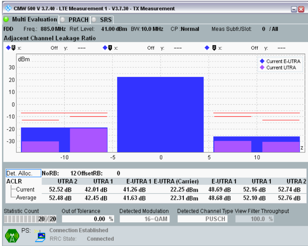
Band8 QAM16 BW=10MHz Channel=21500 RB Size=12 Position=#Max
