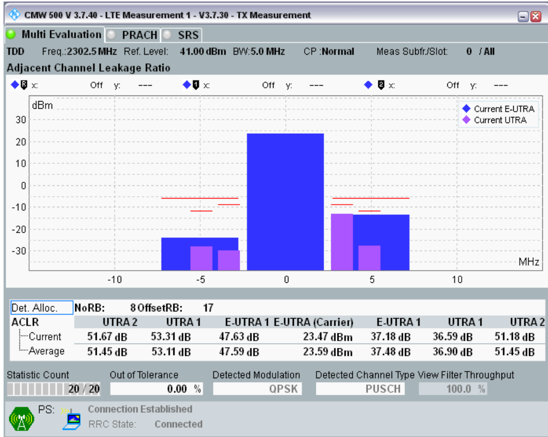
Band40 QPSK BW=5MHz Channel=38675 RB Size=25 Position=#0
