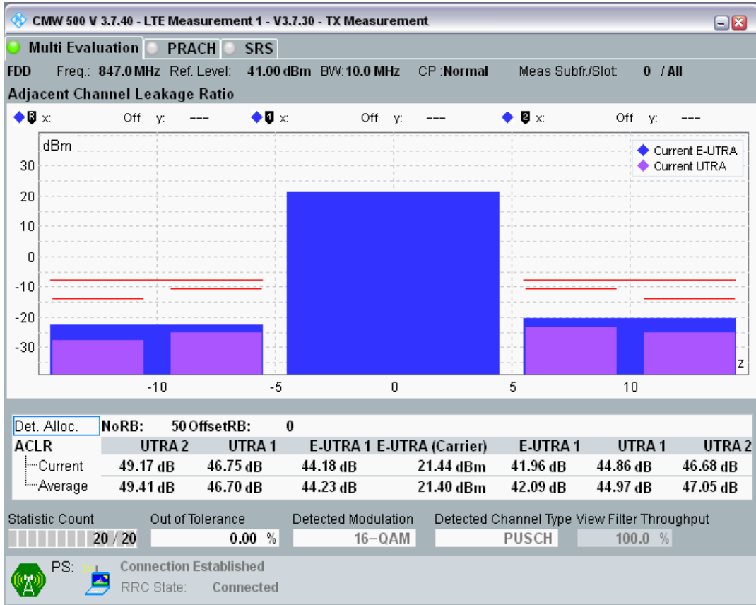
Band20 QPSK BW=10MHz Channel=24400 RB Size=12 Position=#0
