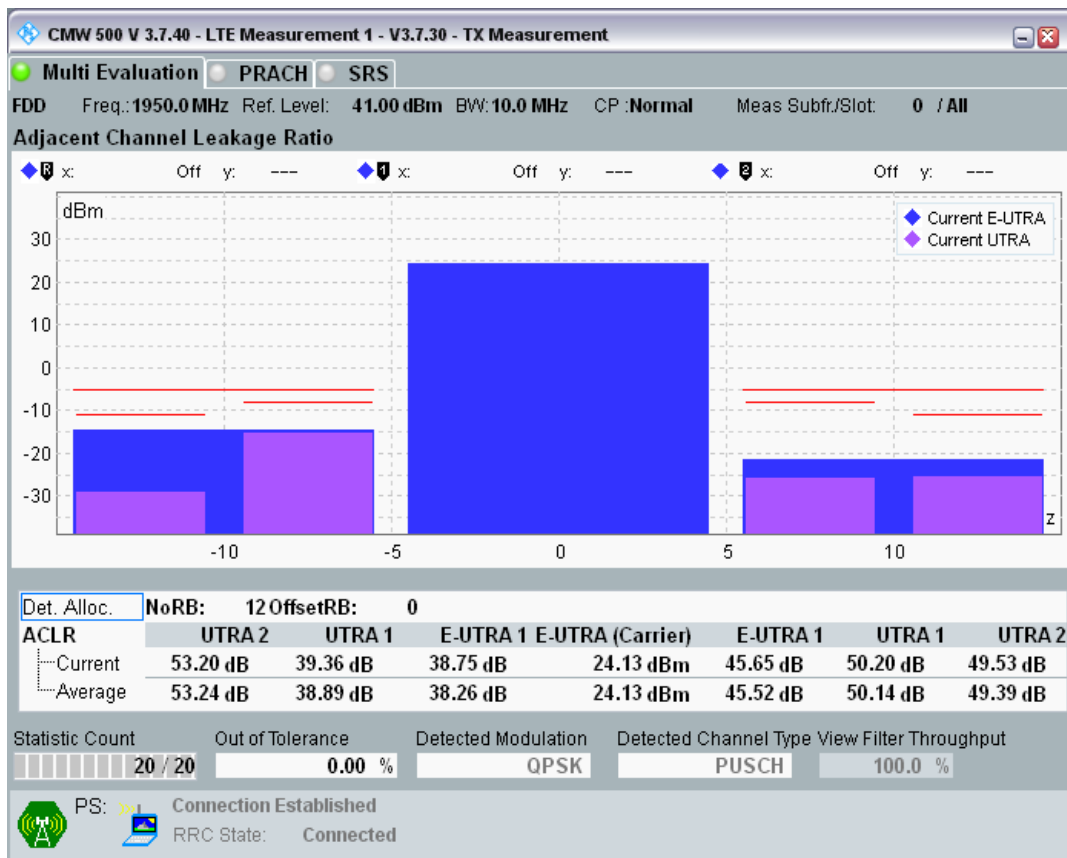
Band1 QPSK BW=10MHz Channel=18300 RB Size=12 Position=#Max
