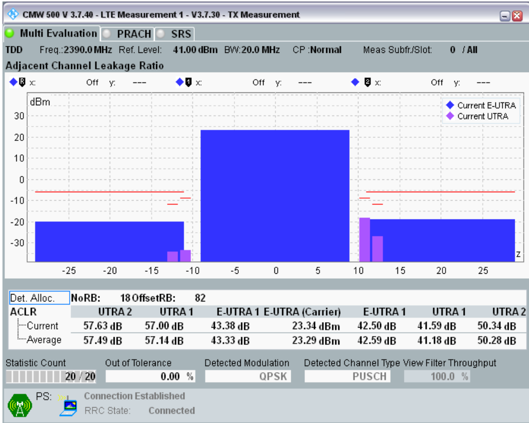
Band40 QPSK BW=20MHz Channel=39550 RB Size=100 Position=#0
