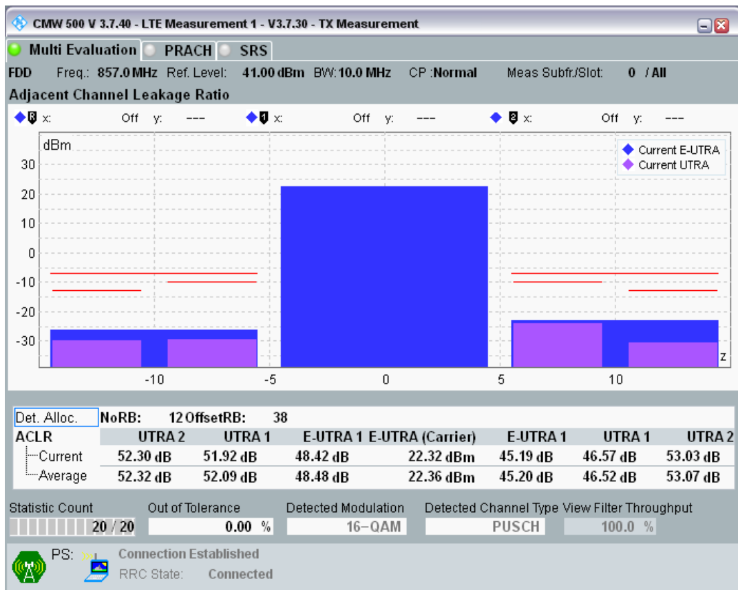
Band20 QAM16 BW=10MHz Channel=24400 RB Size=50 Position=#0
