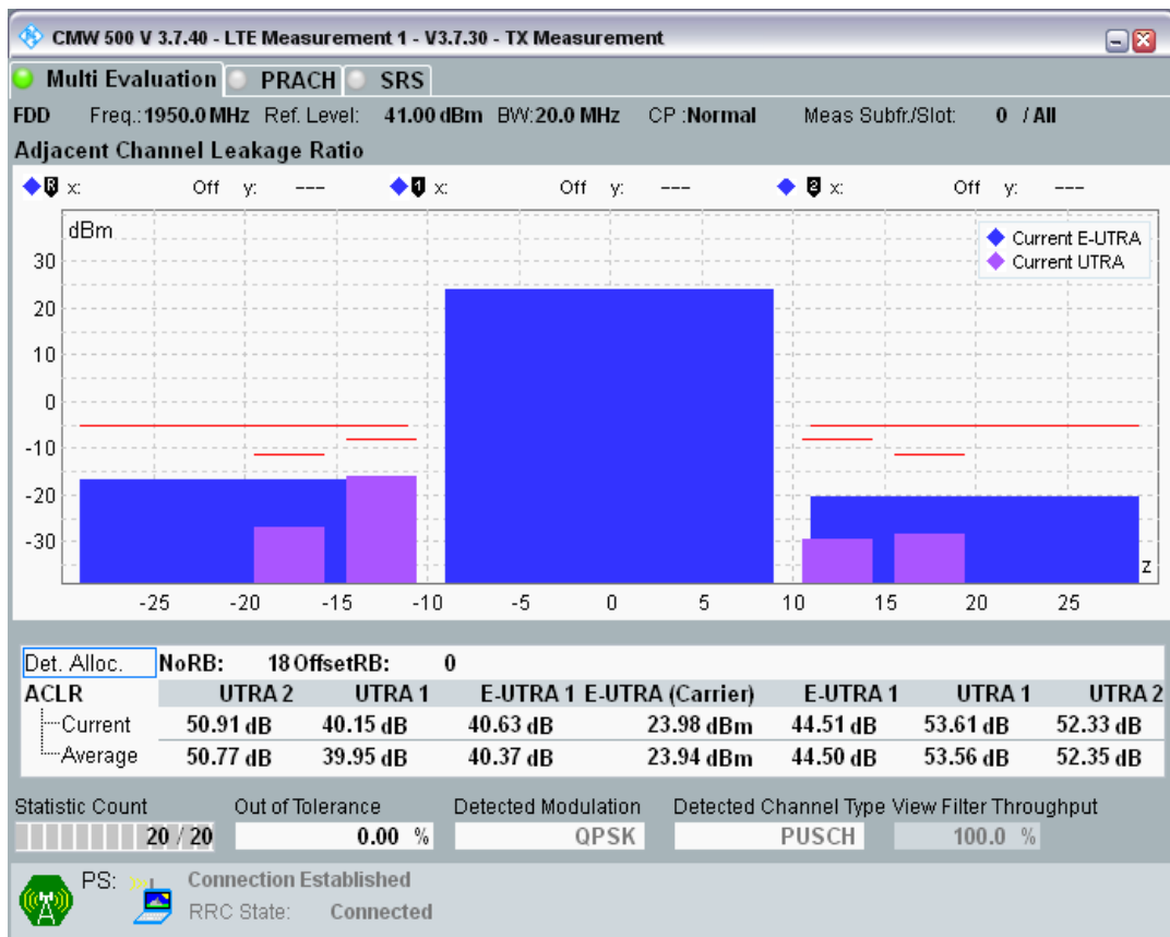
Band1 QPSK BW=20MHz Channel=18300 RB Size=18 Position=#Max
