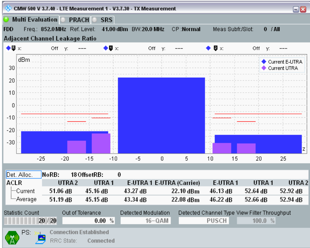
Band20 QAM16 BW=20MHz Channel=24350 RB Size=18 Position=#Max
