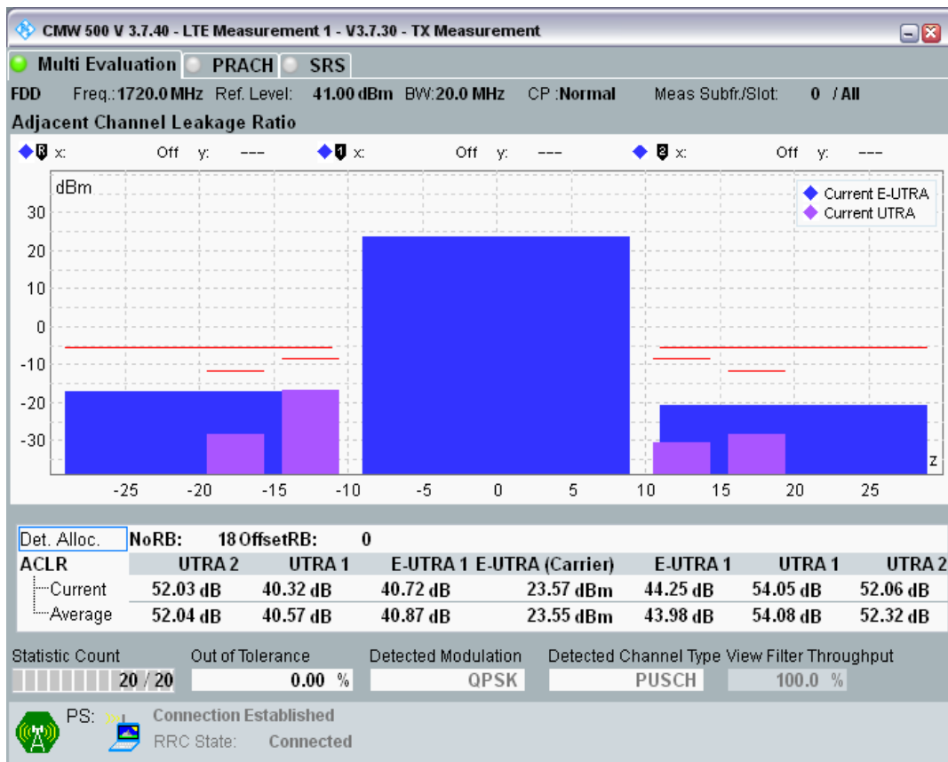
Band3 QPSK BW=20MHz Channel=19300 RB Size=18 Position=#Max
