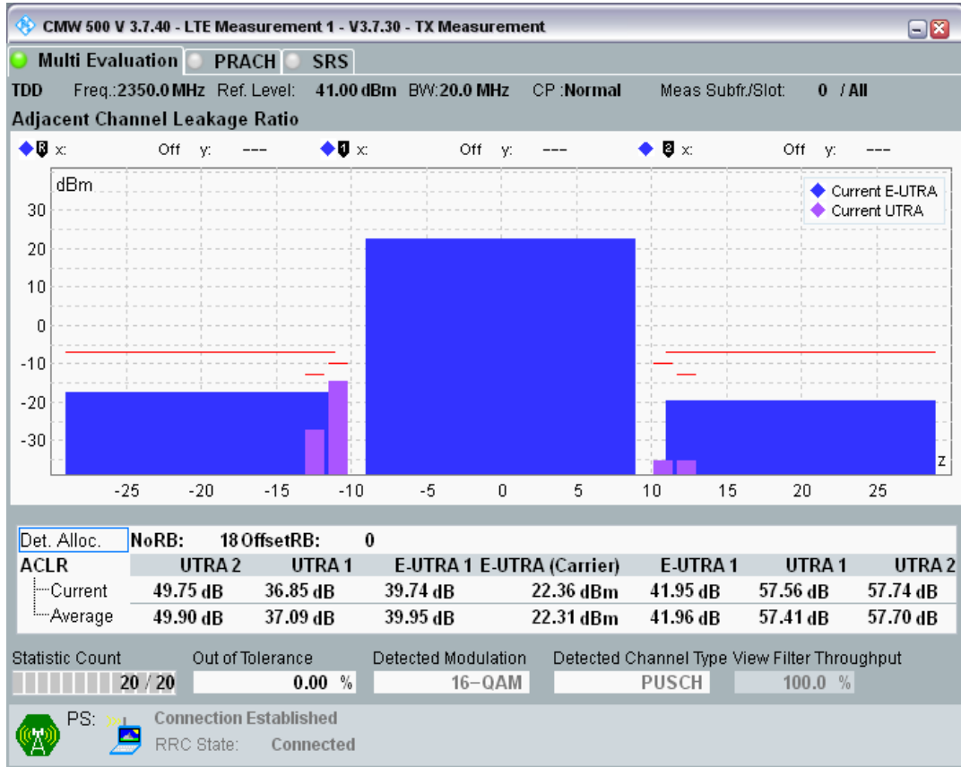
Band40 QAM16 BW=20MHz Channel=39150 RB Size=18 Position=#Max
