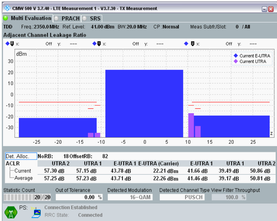
Band40 QAM16 BW=20MHz Channel=39150 RB Size=100 Position=#0
