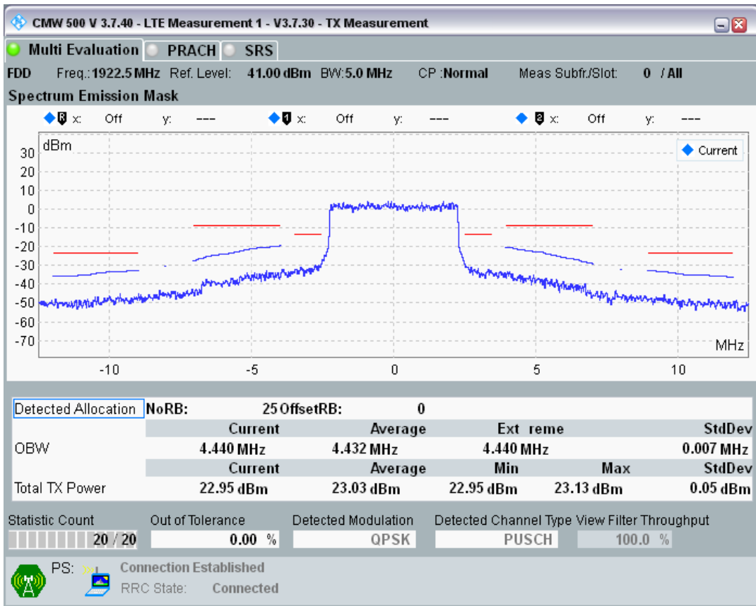
Band1 QAM16 BW=5MHz Channel=18025 RB Size=8 Position=#0
