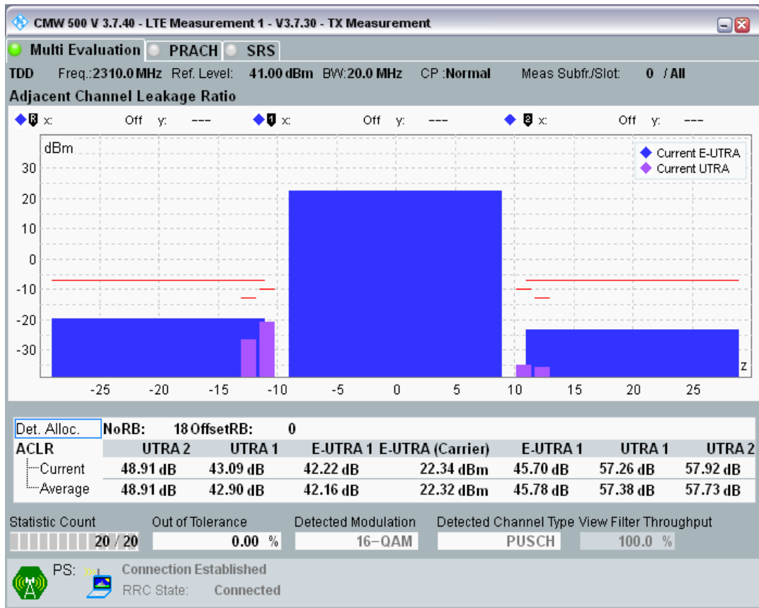
Band40 QAM16 BW=20MHz Channel=38750 RB Size=18 Position=#Max
