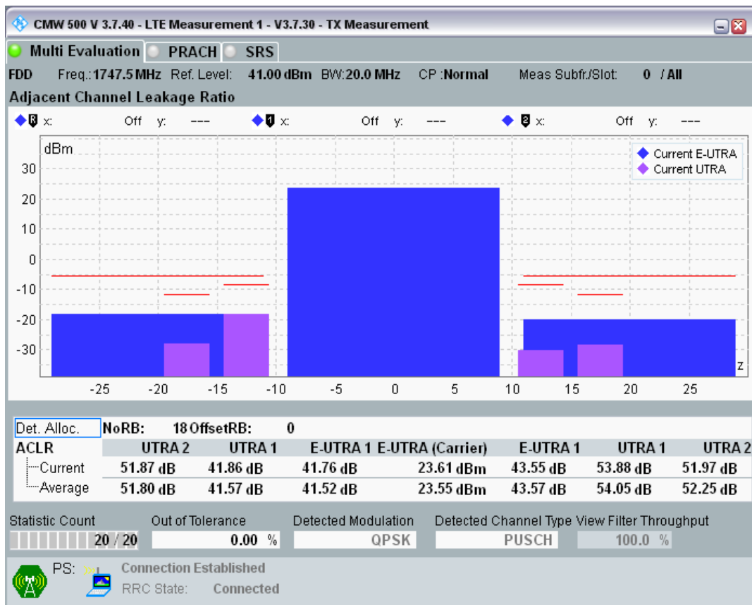
Band3 QPSK BW=20MHz Channel=19575 RB Size=18 Position=#Max
