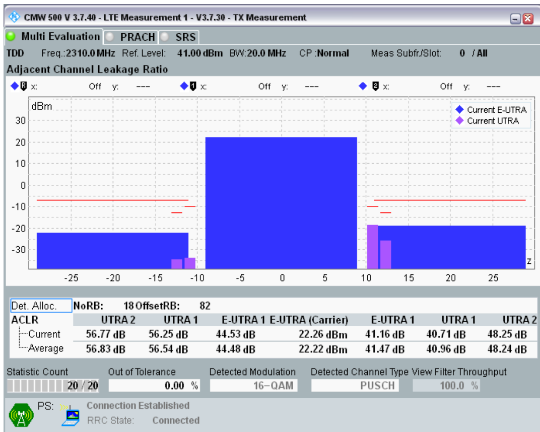
Band40 QAM16 BW=20MHz Channel=38750 RB Size=100 Position=#0
