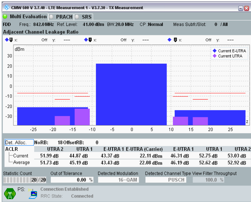
Band20 QAM16 BW=20MHz Channel=24250 RB Size=18 Position=#Max
