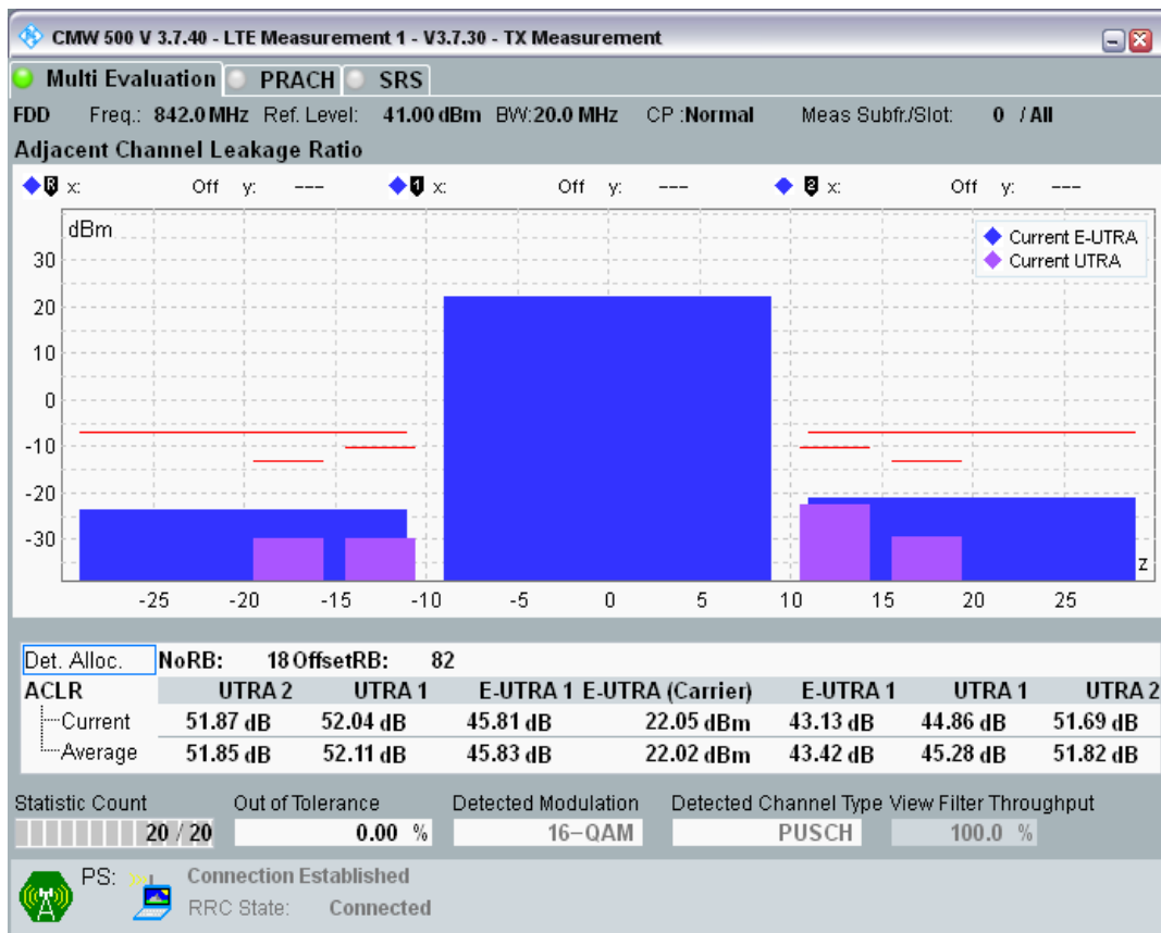
Band20 QAM16 BW=20MHz Channel=24250 RB Size=100 Position=#0
