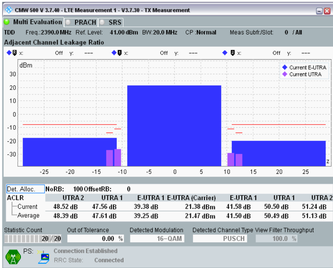
Band7 QPSK BW=5MHz Channel=20775 RB Size=8 Position=#0
