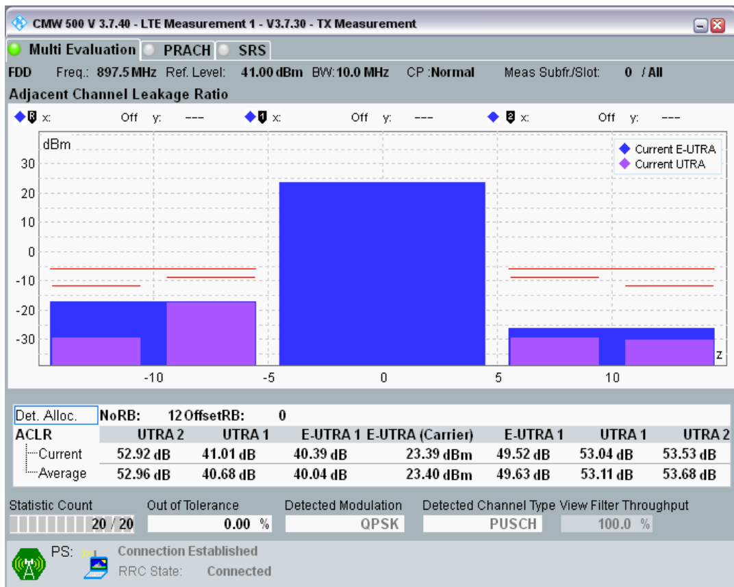
Band8 QPSK BW=10MHz Channel=21625 RB Size=12 Position=#Max
