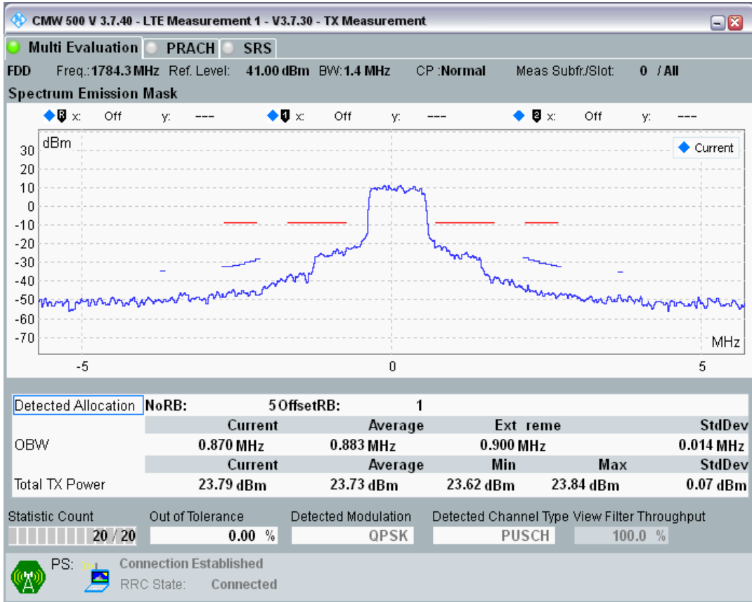
Band3 QPSK BW=1.4MHz Channel=19943 RB Size=6 Position=#0
