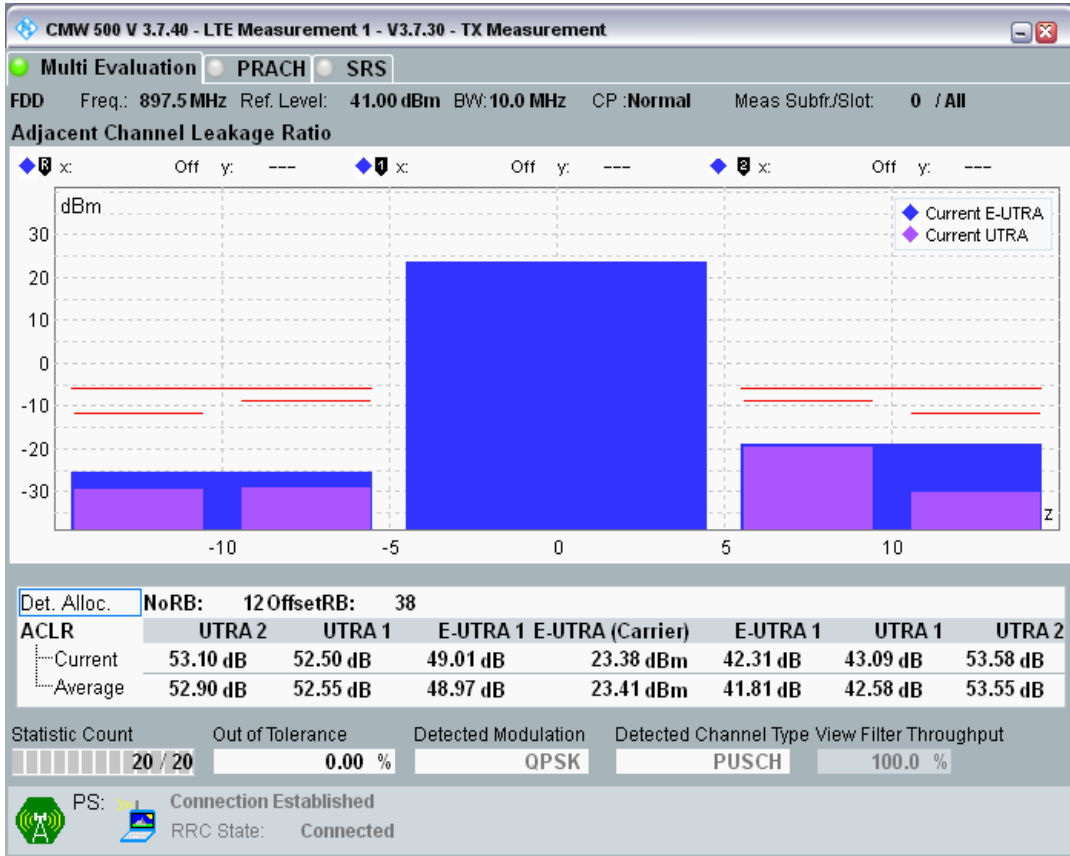
Band8 QPSK BW=10MHz Channel=21625 RB Size=50 Position=#0
