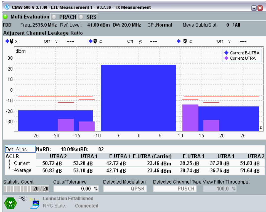
Band7 QPSK BW=20MHz Channel=21100 RB Size=100 Position=#0
