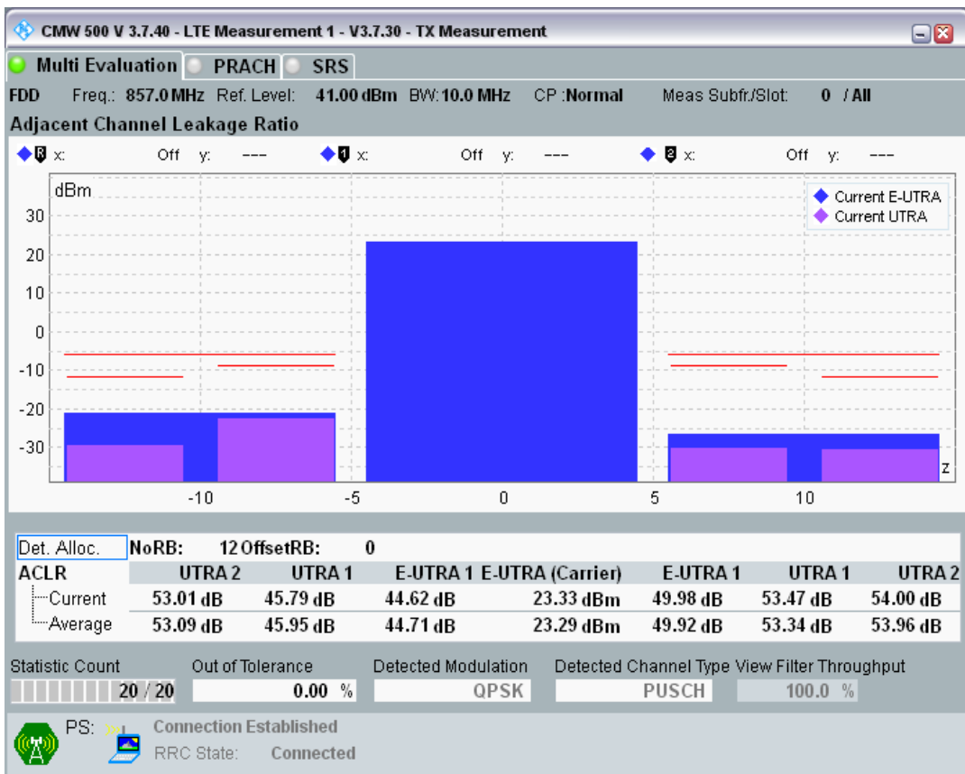
Band20 QPSK BW=10MHz Channel=24400 RB Size=12 Position=#Max
