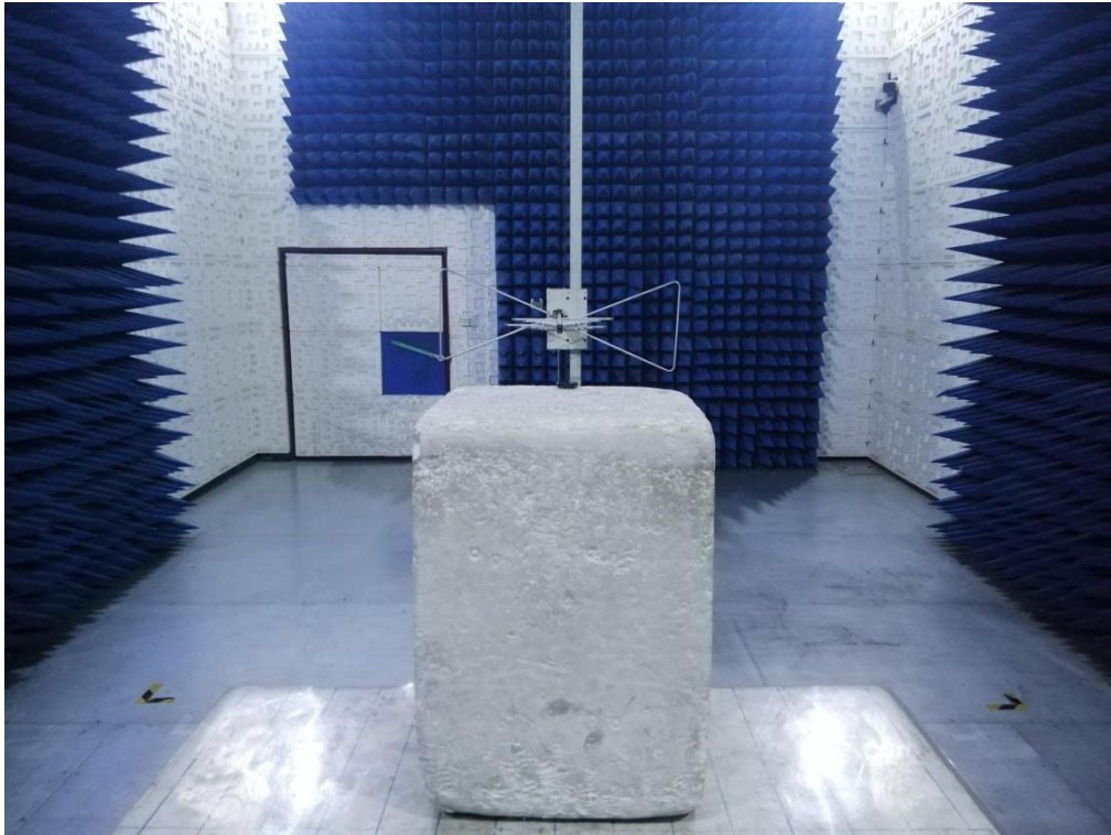
RADIATED SPURIOUS EMISSION ABOVE 1G TEST SETUP
