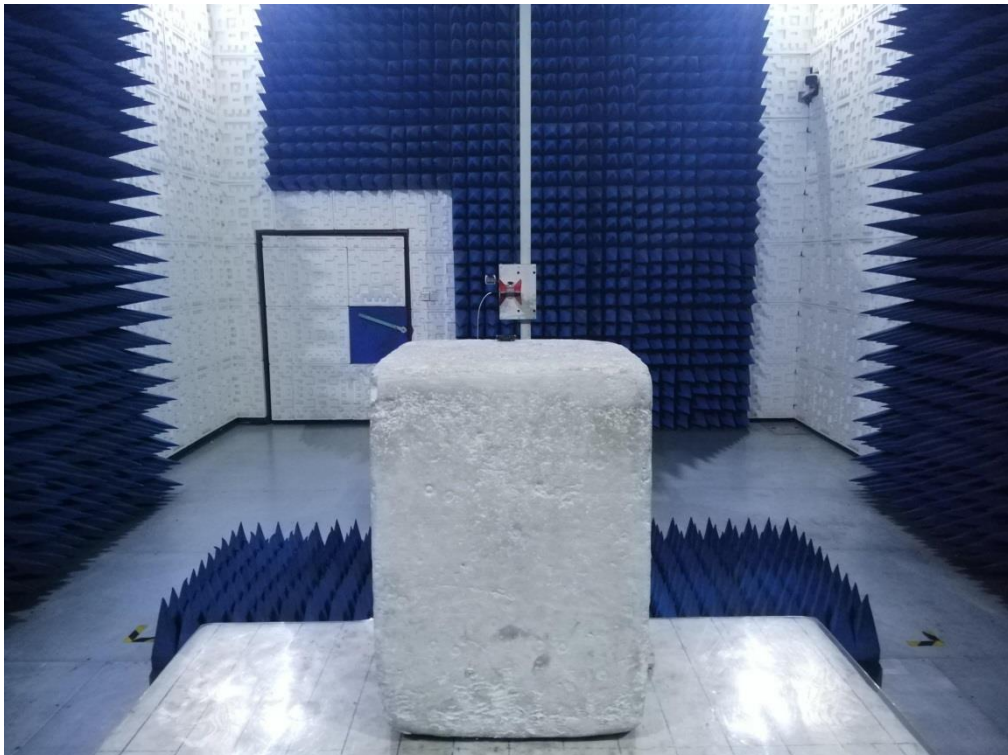
RADIATED SPURIOUS EMISSION ABOVE 1G TEST SETUP
