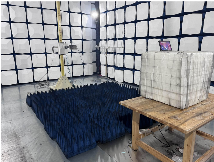
RADIATED EMISSION ABOVE 1G TEST SETUP
