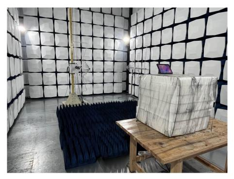
RADIATED EMISSION ABOVE 1G TEST SETUP
