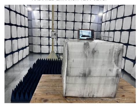
RADIATED EMISSION ABOVE 1G TEST SETUP
