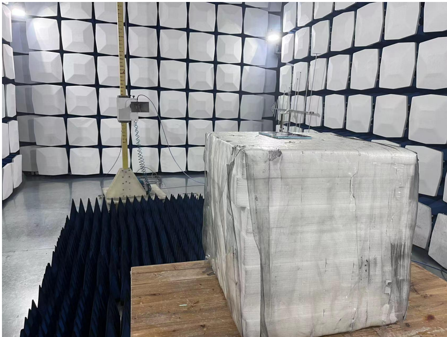
RADIATED EMISSION ABOVE 1G TEST SETUP
