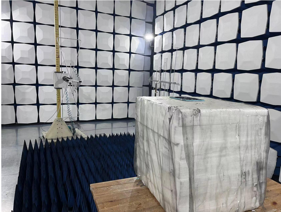
RADIATED EMISSION ABOVE 1G TEST SETUP
