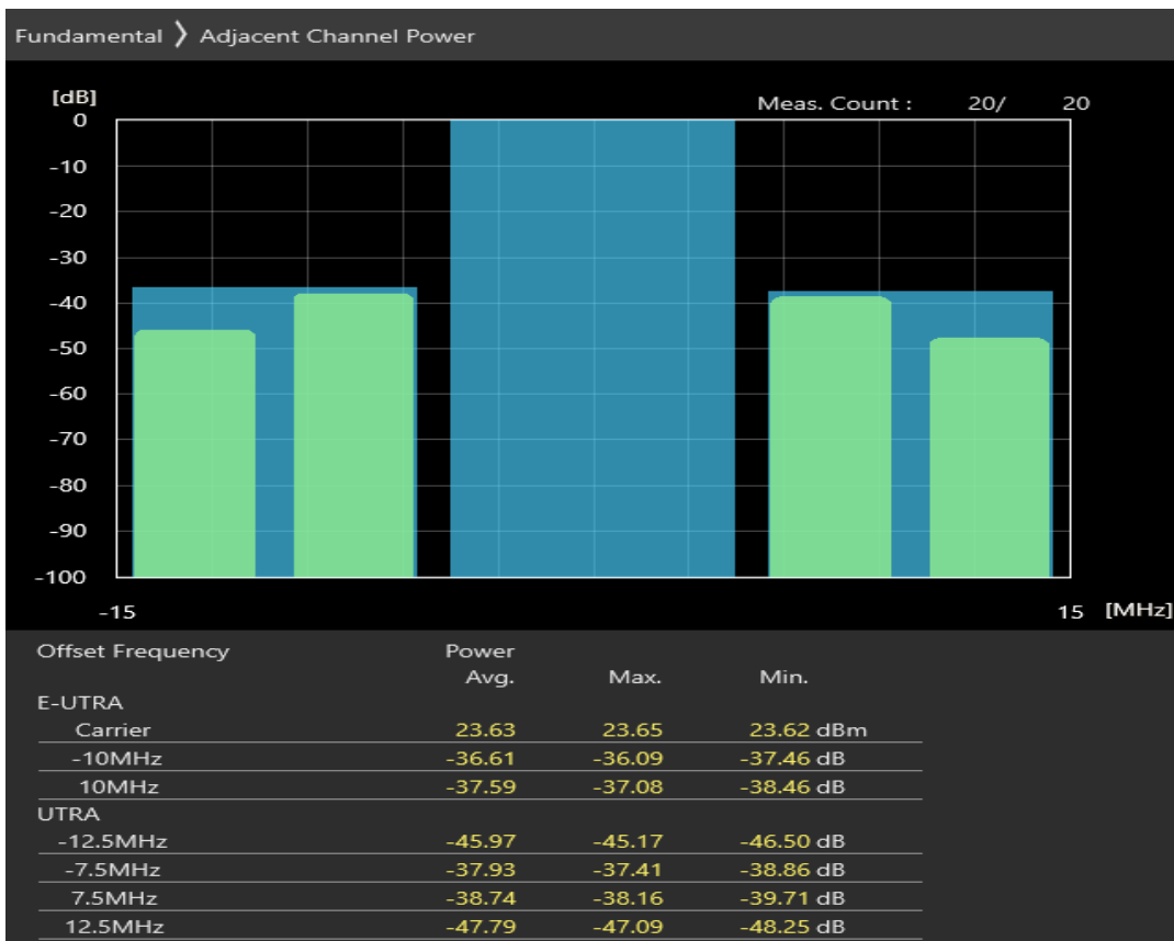
Band1 QPSK BW=20MHz Channel=18100 RB Size=100 Position=#0 Band1 Normal
