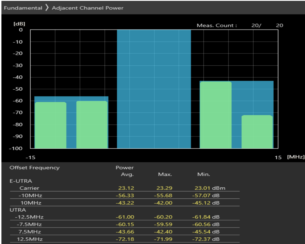
Band8 16QAM BW=10MHz Channel=21750 RB Size=50 Position=#0 Band8 Normal
