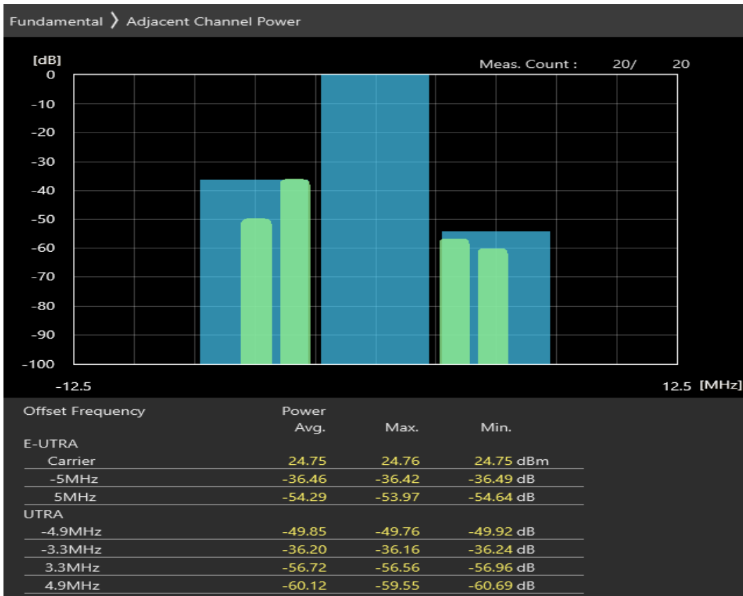
Band40 QPSK BW=5MHz Channel=38675 RB Size=8 Position=#Max Band40 Normal
