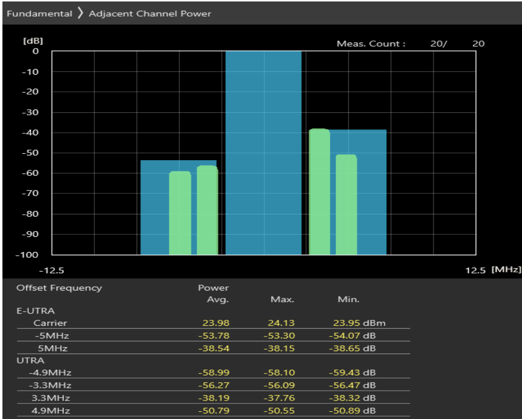
Band40 QPSK BW=10MHz Channel=38700 RB Size=12 Position=#0 Band40 Normal
