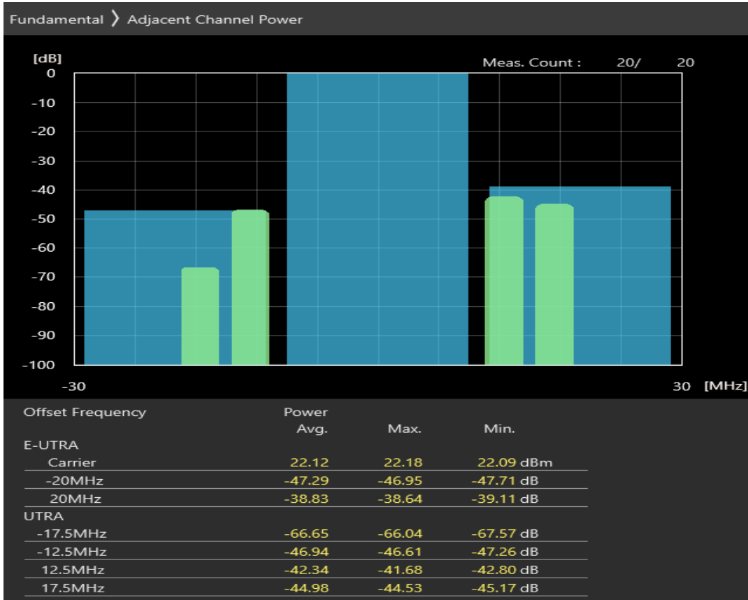
Band20 QPSK BW=20MHz Channel=24250 RB Size=18 Position=#0 Band20 Normal
