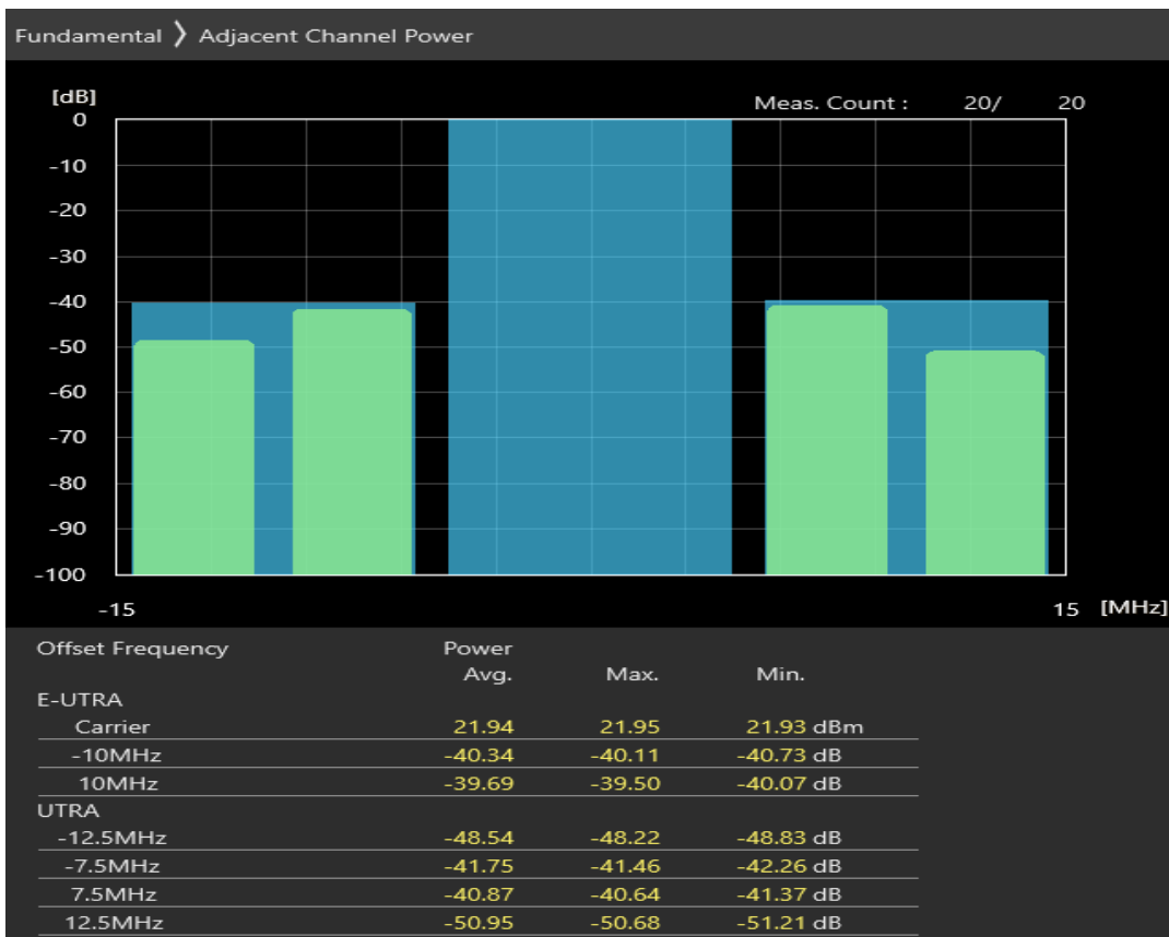
Band20 QPSK BW=20MHz Channel=24250 RB Size=100 Position=#0 Band20 Normal
