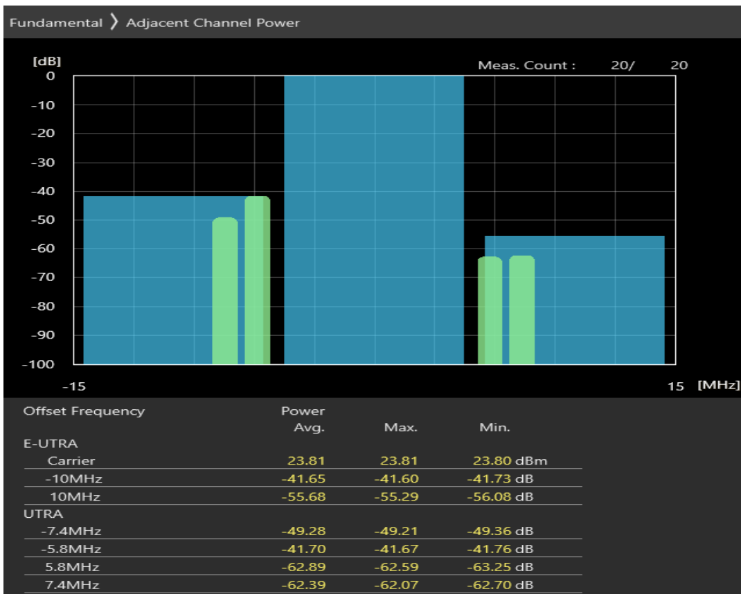
Band40 16QAM BW=10MHz Channel=39150 RB Size=12 Position=#Max Band40 Normal
