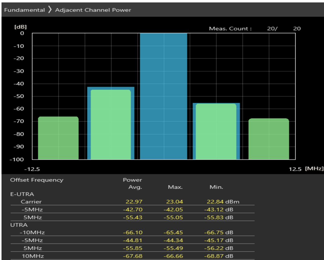
Band3 16QAM BW=5MHz Channel=19575 RB Size=8 Position=#Max Band3 Normal
