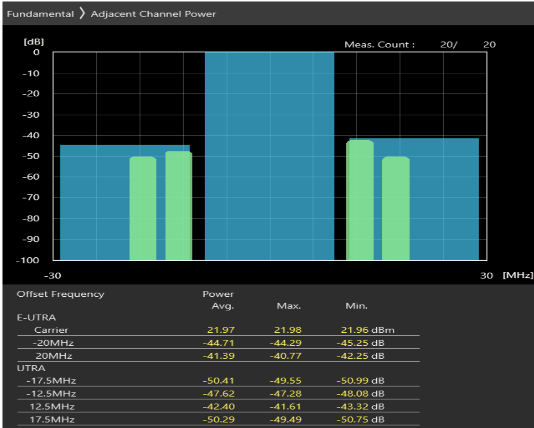
Band20 QPSK BW=20MHz Channel=24350 RB Size=18 Position=#0 Band20 Normal
