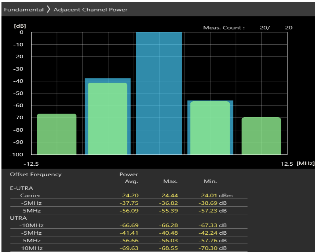
Band1 16QAM BW=5MHz Channel=18025 RB Size=8 Position=#Max Band1 Normal
