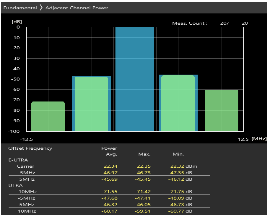
Band8 QPSK BW=5MHz Channel=21625 RB Size=25 Position=#0 Band8 Normal
