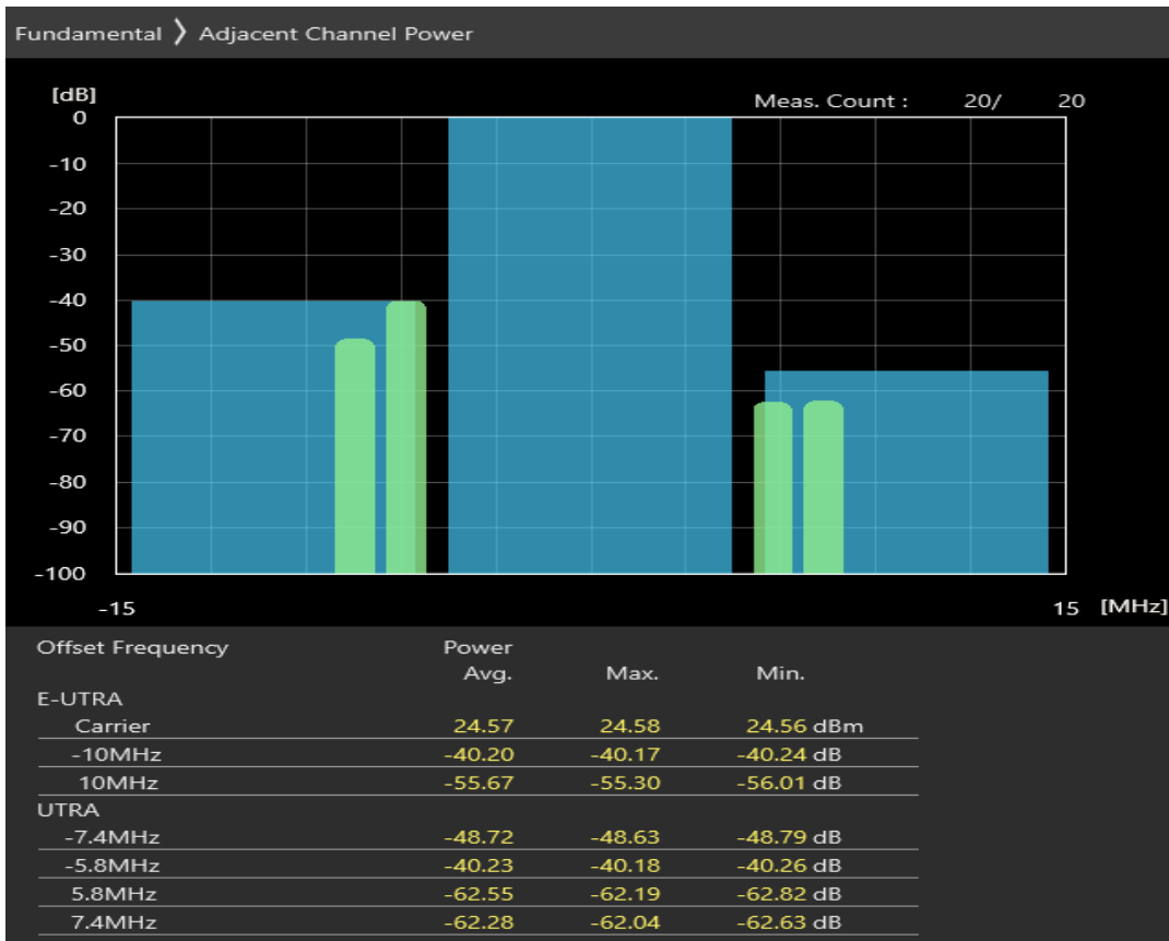
Band40 QPSK BW=10MHz Channel=39150 RB Size=12 Position=#Max Band40 Normal
