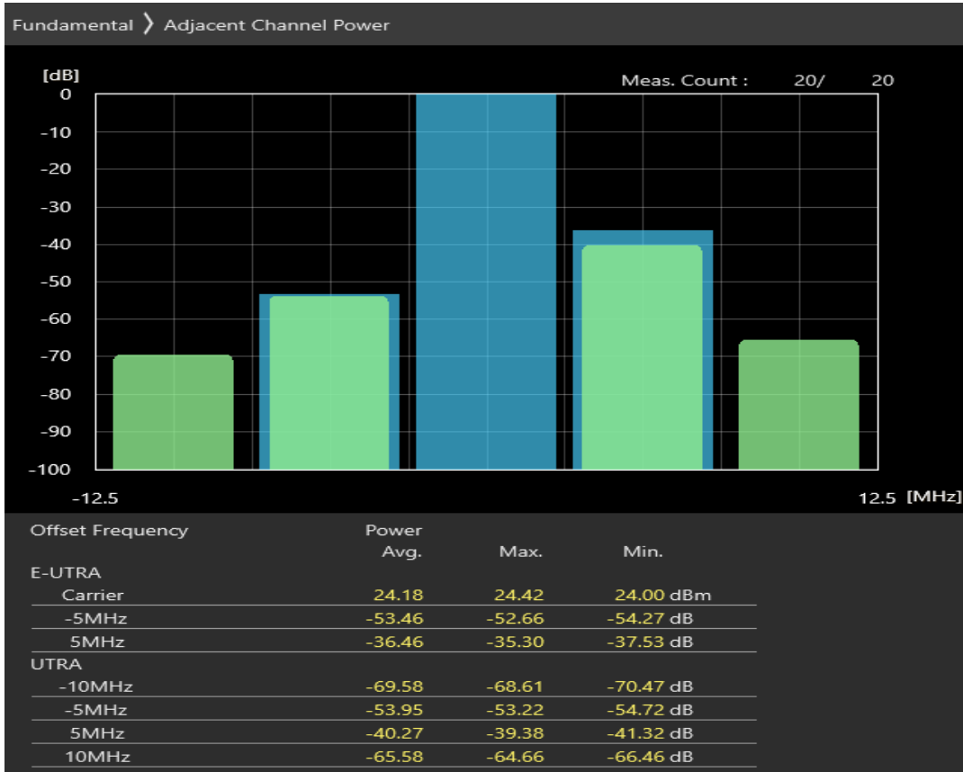
Band1 QPSK BW=10MHz Channel=18050 RB Size=12 Position=#0 Band1 Normal
