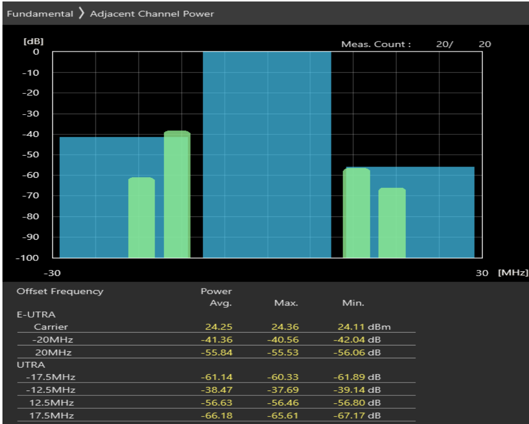
Band1 16QAM BW=20MHz Channel=18500 RB Size=18 Position=#Max Band1 Normal
