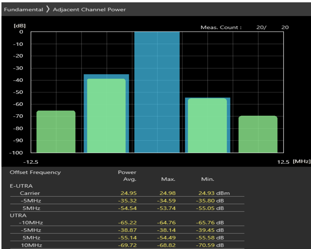
Band1 QPSK BW=5MHz Channel=18300 RB Size=8 Position=#Max Band1 Normal
