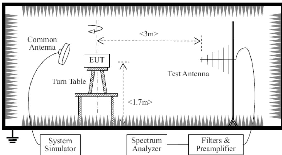
The EUT, which is powered by the Battery charged with the AC Adapter, is located in a 3m Full-Anechoic Chamber; the cable loss, air loss and so on of the site as factors are pre-calibrated using the "Substitution" method, and calculated to correct the reading.
