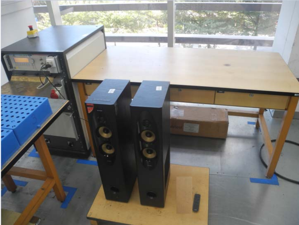
Photo 9 Voltage Dips and Interruptions Immunity Test
